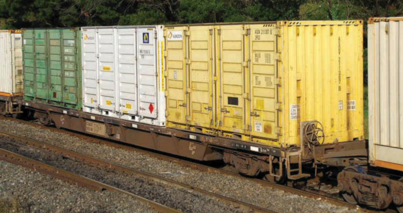
QR National (later Aurizon, now part of the Linfox group) was a big user of side-door containers. They provide safe and secure side-loading and unloading access similar to a curtain-sided container, but the side doors are less prone to damage. The doors can be ventilated to allow air flow.
