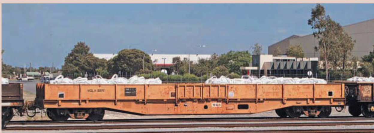
WGLA 30119 was built from a WF series flat wagon. The sides are fabricated to carry bagged nickel. Two of these wagons were regularly used as barrier wagons at Esperance fuel siding.
