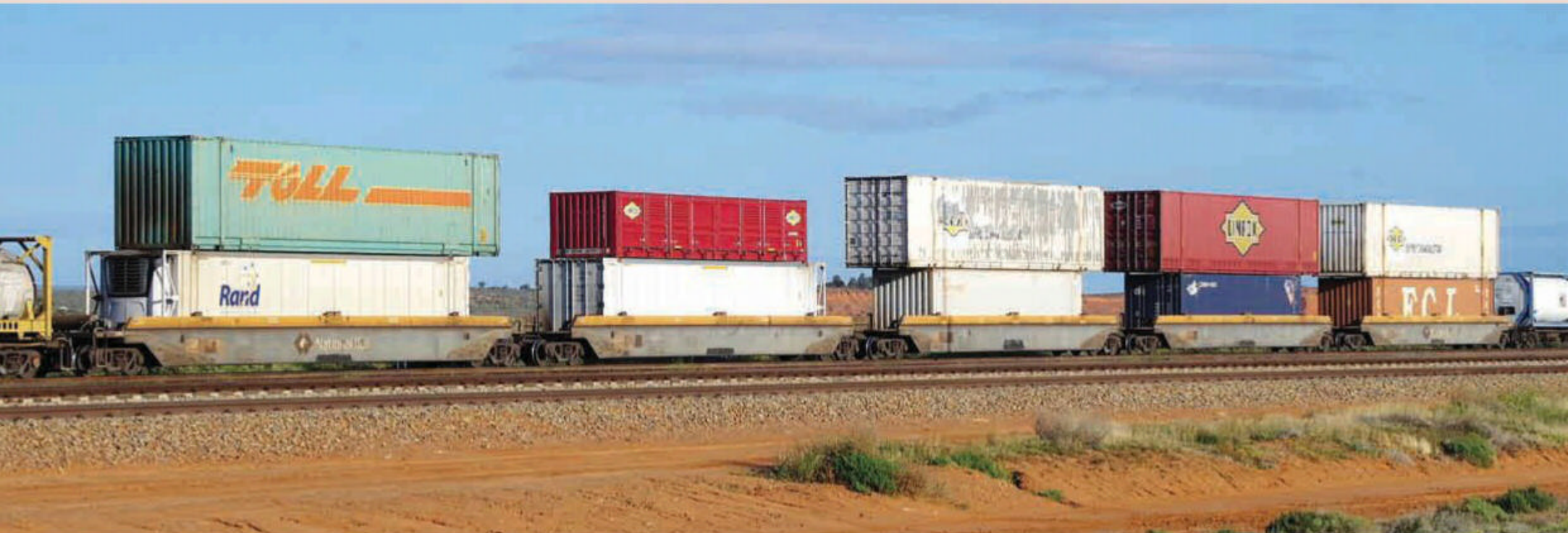
Captured in September 2016 is an RQZY bar-coupled well wagon set, with a mixed double-stack load including some refrigerated containers (aka ‘reefers’), a half-height and some 53 foot Linfox containers.
