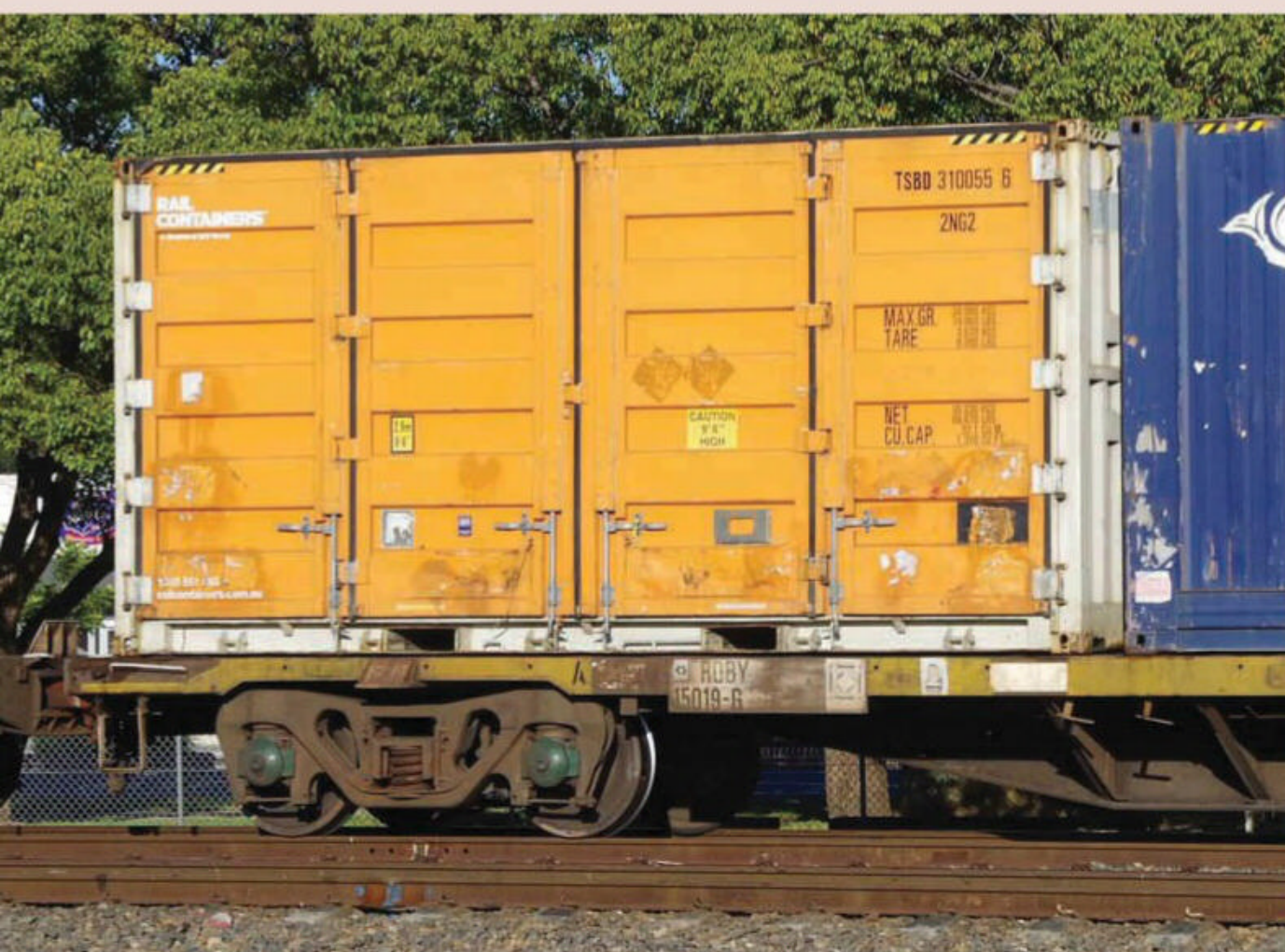
SCF pioneered side doors made from plastic in 2010. The plastic doors were about one quarter the weight of steel doors yet provided the same strength rating. Apart from the orange side-door SCF containers they seem to be no longer used.
