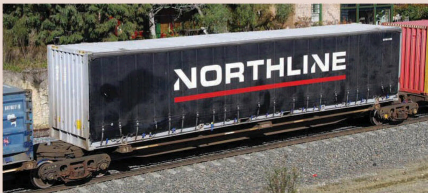
This recently-built Northline curtain-sided container is 48 foot long and on hire from SCF. From a weathering perspective, the black curtain shows a lot of dust and the internal curtain straps are clearly visible in the dust. Most modern curtain-sided containers have solid ends for structural performance due to the lack of solid sides.
