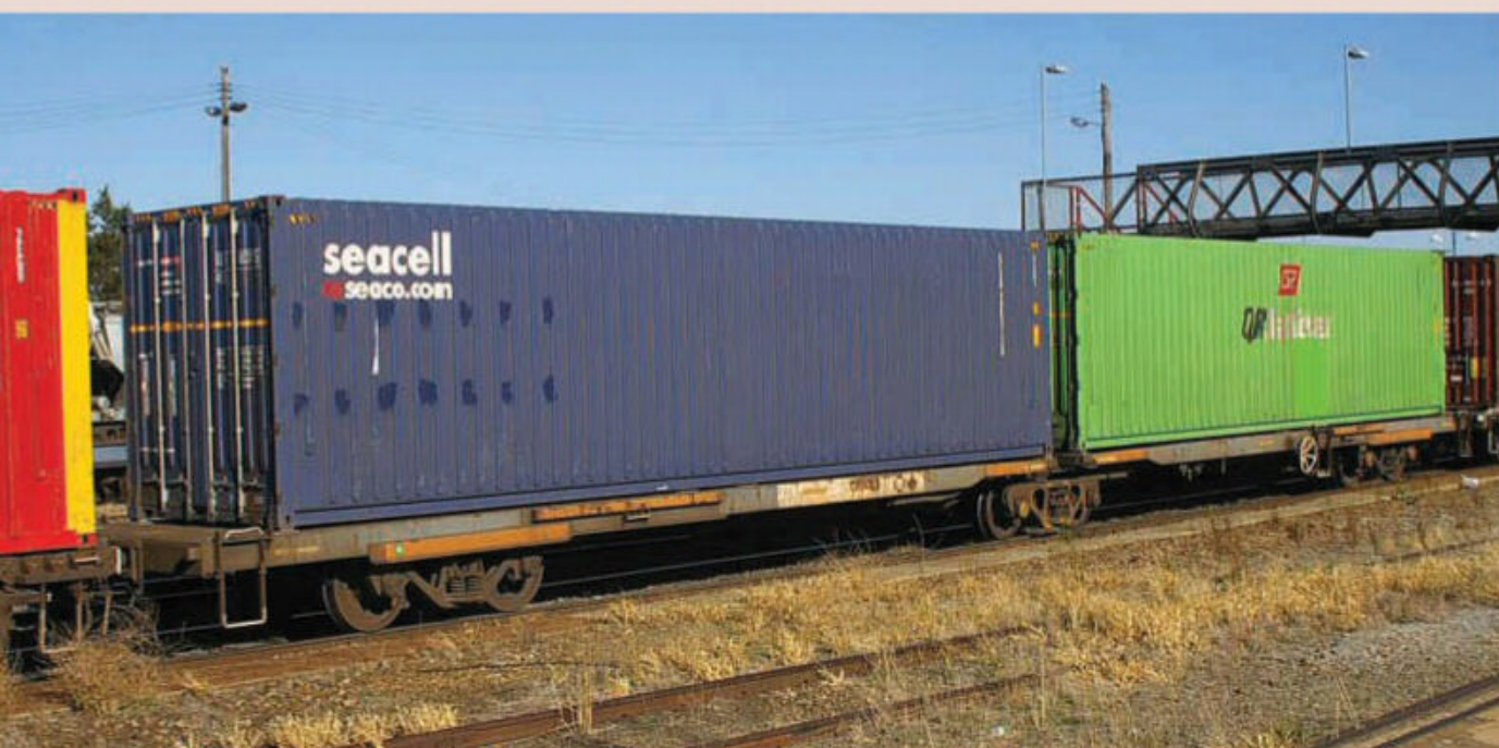
In 2006, a pair of 40 foot Seacell containers ride on an RQEY articulated two-pack wagon. Container lessor GE Seaco pioneered the Seacell concept; QR National (owner of the green container) had a reasonable-sized fleet in operation during the 2000s.
