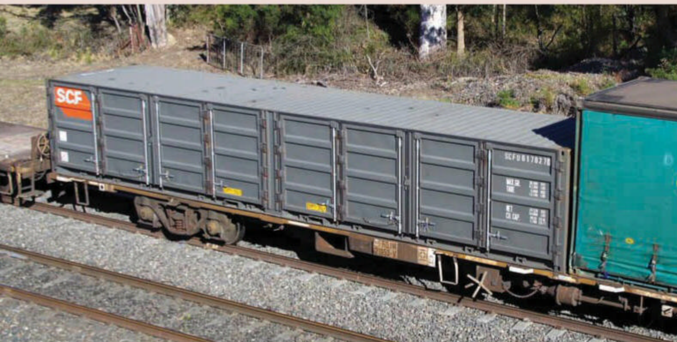
Recent years have seen an increase in 'half-height' side-door containers. These are ideal for heavy pallet-loaded products that can not be stacked efficiently into a normal-height container. These containers also make good base containers for double-stacking on flat wagons.
