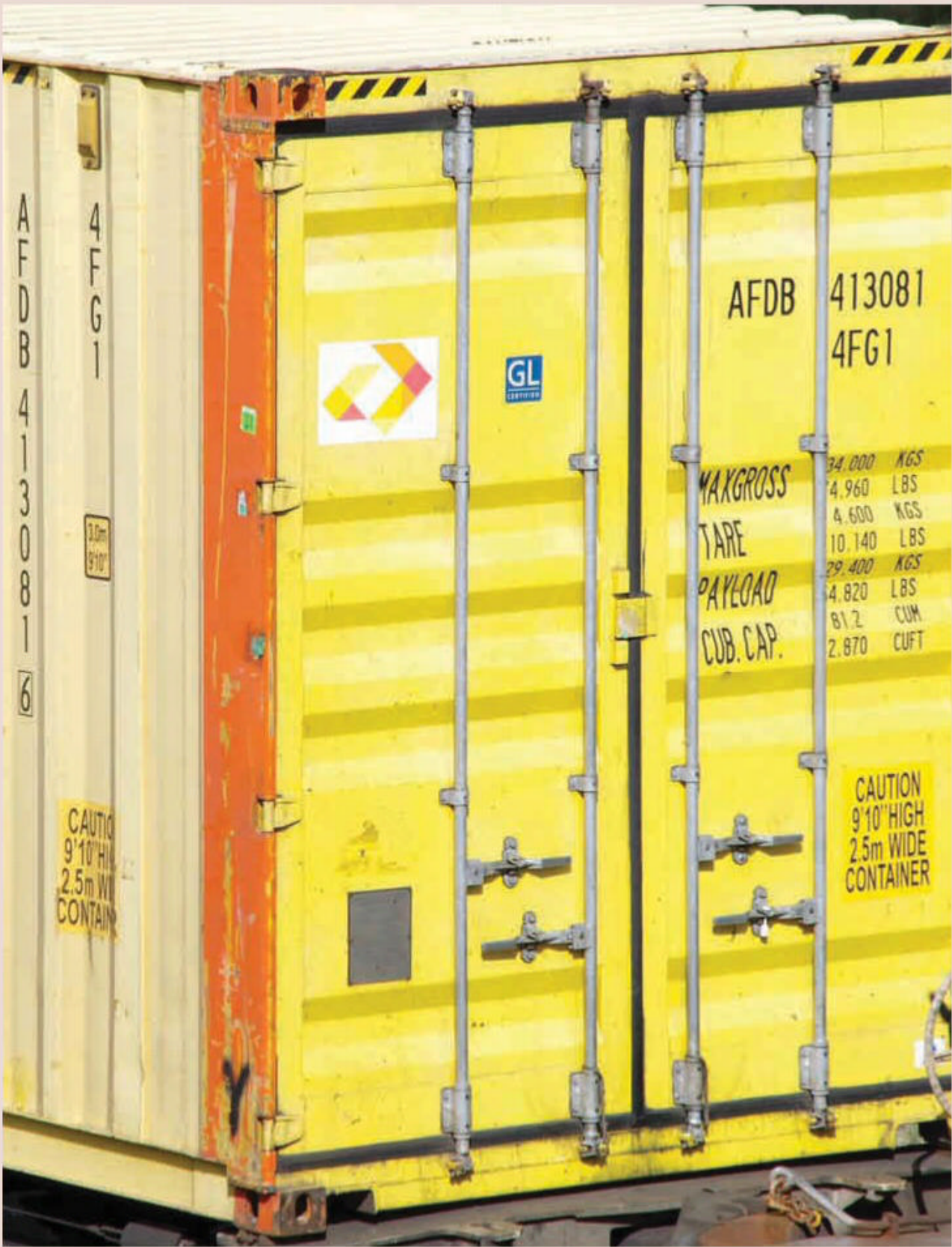
Former Aurizon-operated container AFDB 413081-6 showing its information carried on the end doors.
