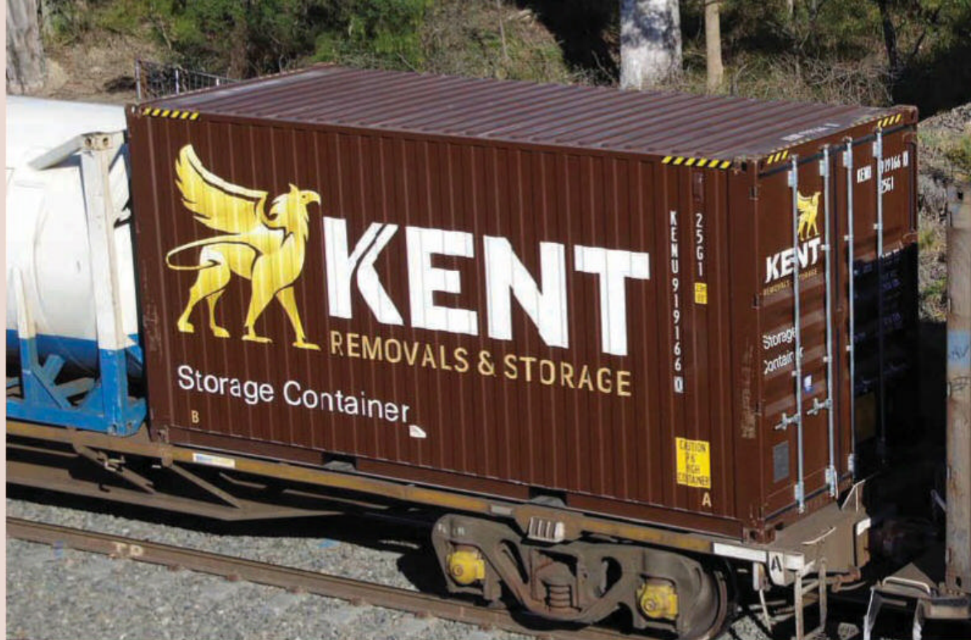
Removalist companies operate many 25G1 containers; Kent is one of the largest. When photographed in late 2018 this container was almost new and has the interesting feature of having doors at both ends for easy access; a feature that is not common on most 25G1 containers.
