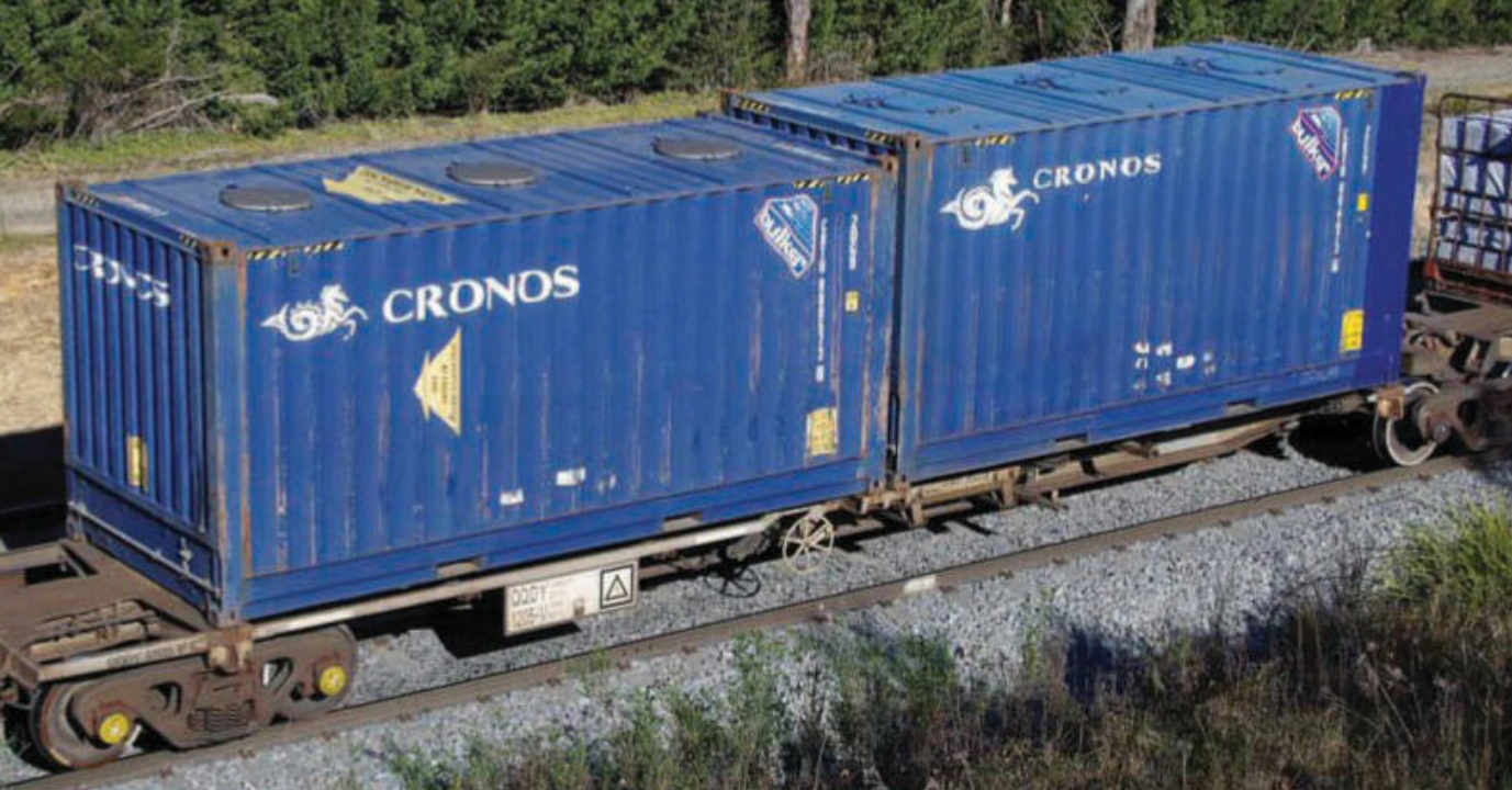
A pair of Cronos 20 foot bulk container on board a QQDY wagon that was built for Aurizon, but now owned by Pacific National. The container on the left is unusual in that it is a 9 foot high container making it a 2DG9 type. It has three roof hatches and the 'letter box' slot for unloading that is clearly marked by the yellow arrow pointing to the unloading end.
