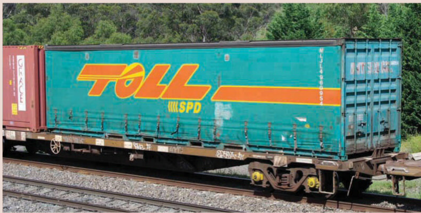
More than 20 years old, this former Interlink curtain-sided container still shows its origin on the end doors. Now marked for Toll SPD, many of these containers are being refurbished and marked with the new Toll logo and darker green livery. The end designs of curtain-sided containers vary greatly.
