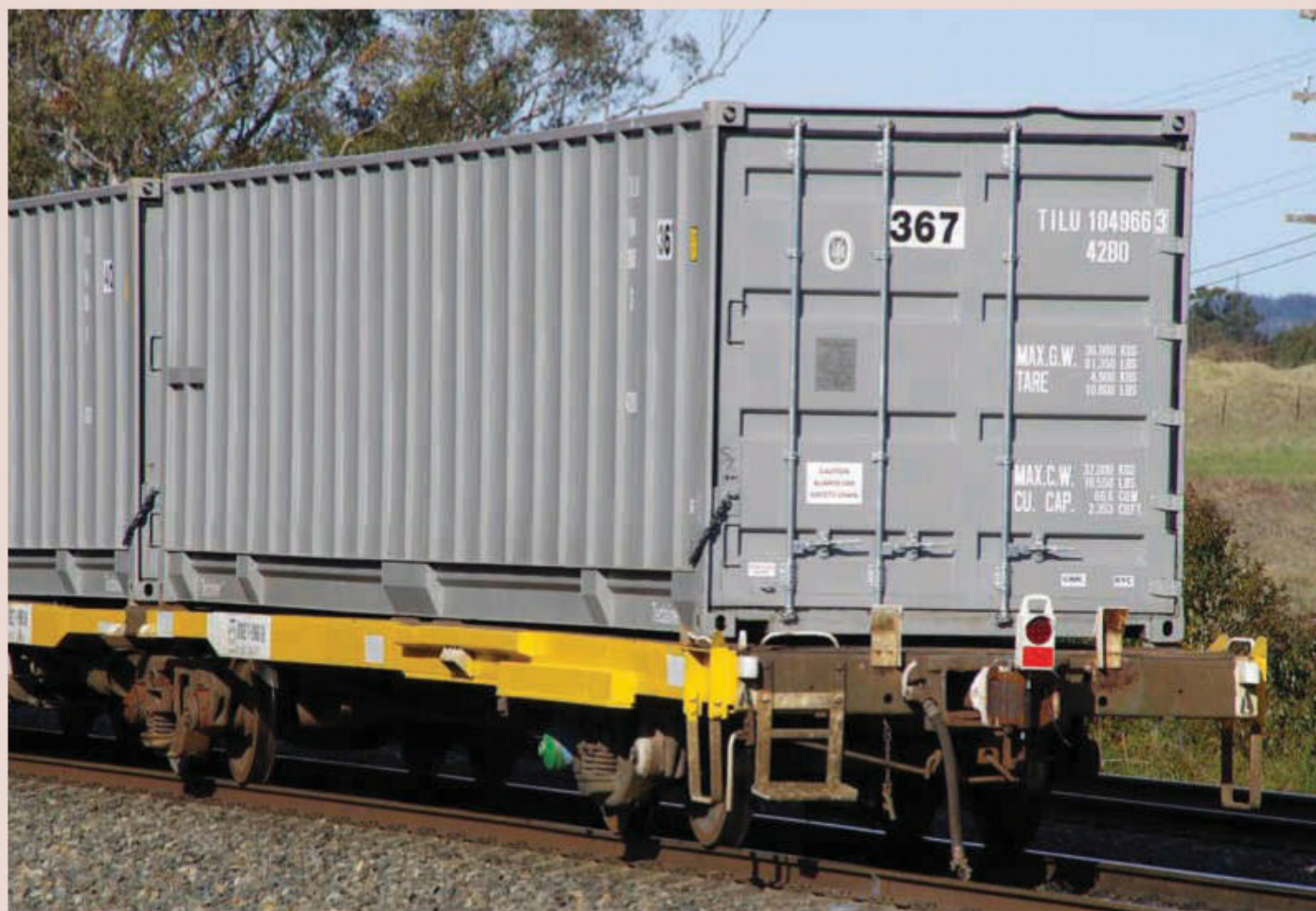
Built for a very specific task, garbage containers are currently used to move Sydney's waste to Tarago (between Goulburn and Canberra). The rear door is hinged on only one side and is designed to aid loading and unloading.
