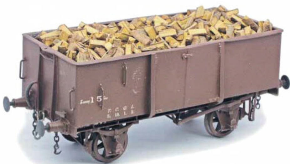
'Tommy Bent' style high-sided steel I wagon (c. 1890), scratch-built from styrene, with VR Casts buffers and a Veteran Models white-metal underframe. Split wood load are sticks from the back yard.
