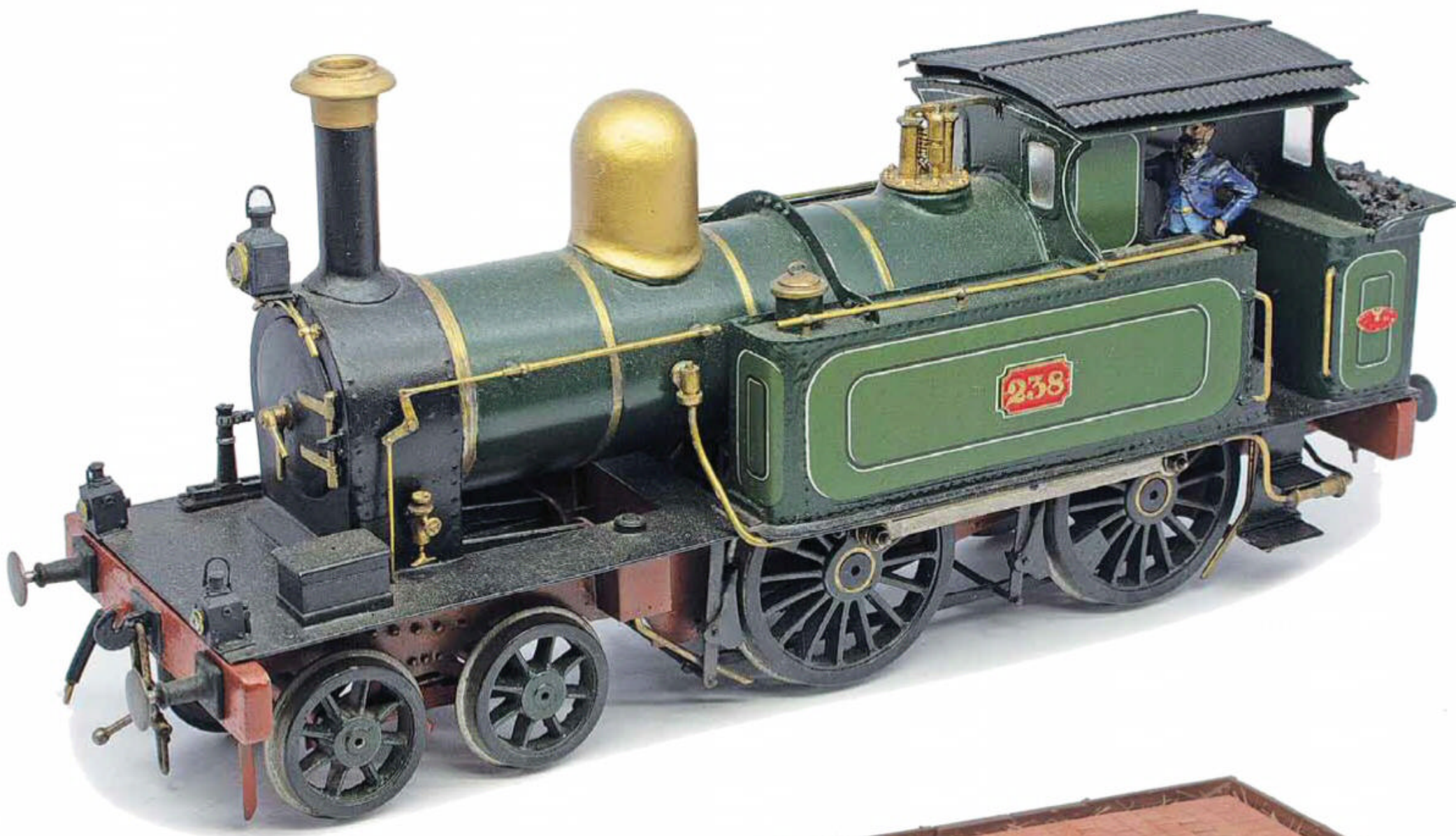
▲ M class suburban steam passenger locomotive No. 238 (c. 1885 — as delivered). Scratch-built in brass and nickel-silver then fitted with batteries and radio control.
