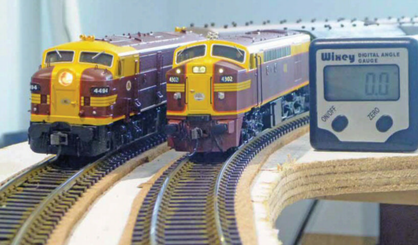
Locomotive 4494 is on superelevated track. 4302 is on flat track, as evidenced by the zero reading of the baseboard showing on the angle gauge.
