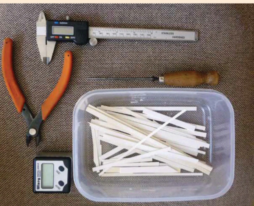
Suggested tools for installing superelevation — an angle gauge, a supply of packing strips, vernier caliper to measure strip thickness, track pin lifter for lifting track pins and a probe for pushing strips into position.
