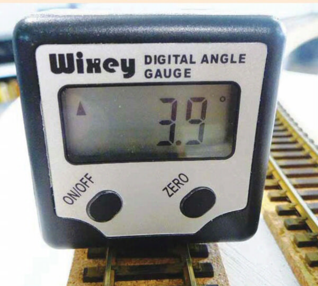
An angle gauge is essential to pick up the subtlety of superelevation. This gauge is showing superelevation of 3.9 degrees, near the limit of most prototypes.
