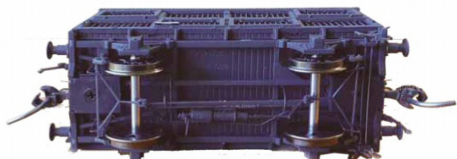
The underbody detail of the GSV wagon.
