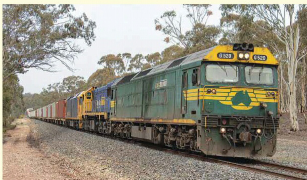
G520, X50 and BL31 lead No. 7901V on 9 August 2018. G520 shows a bit of neglect in its PN patch livery and is starting to fade. G520 previously had an early GPS set-up that was bolted to the headboard. A patch can be seen on the headboard where the GPS was installed. Photo Brad White.
