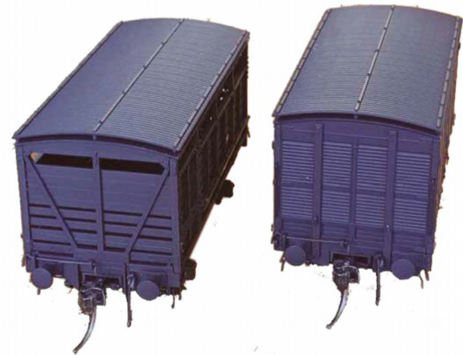
The end detail of the CW and LV wagons.
