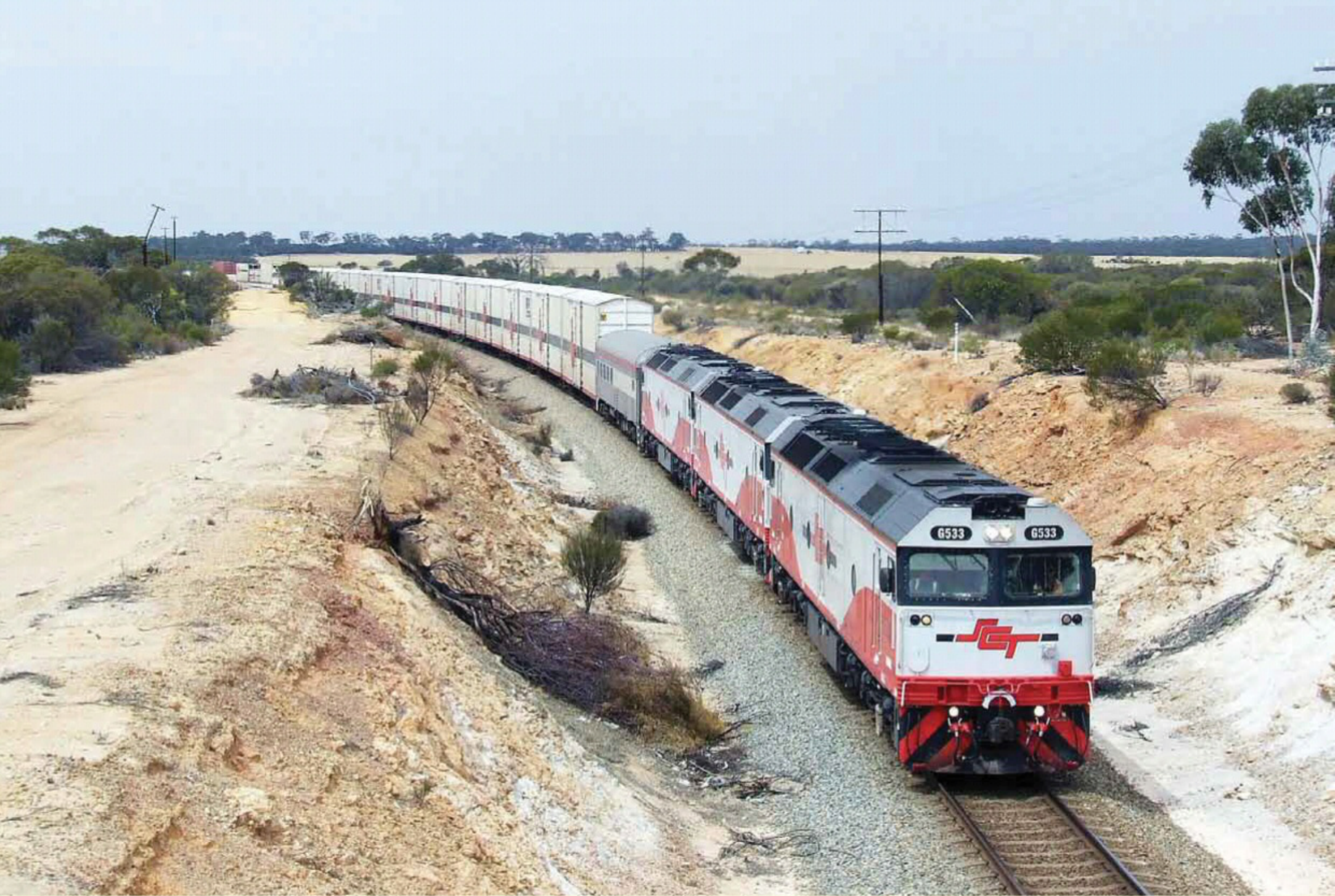
Not long after their release from overhaul, G533 leads G513 and G515 in SCT ownership continue westward through Moorine Rock in Western Australia with 7GP1. G533 has ditch lights installed, in-line refuelling, revised coupler lift bar position and a GPS installed on the cab roof. Photo Simon Barber.
