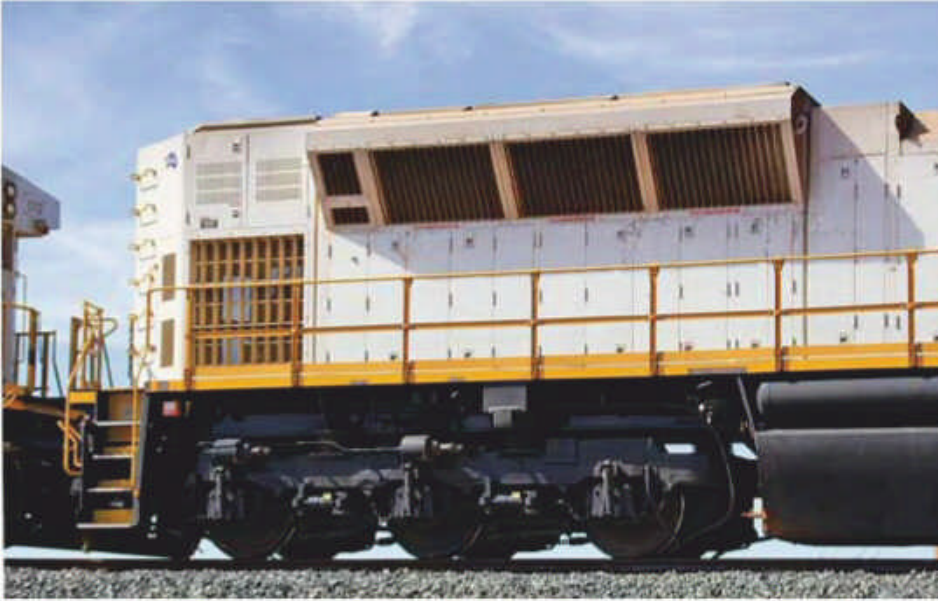
Prototype comparison radiator hood FMG SD9043MAC 907; the fire extinguisher activators are under the walkway near the step wells. Note this is an SD9043MAC and there are differences such as the bogie frames and the door configuration under the radiators.
