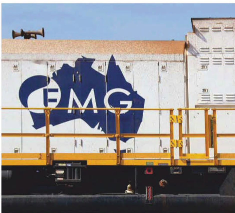
Prototype comparison engine hood FMG SD9043MAC 907, has a swing-gate in the double-rung handrails and a digital fuel gauge, with the road number on it.
