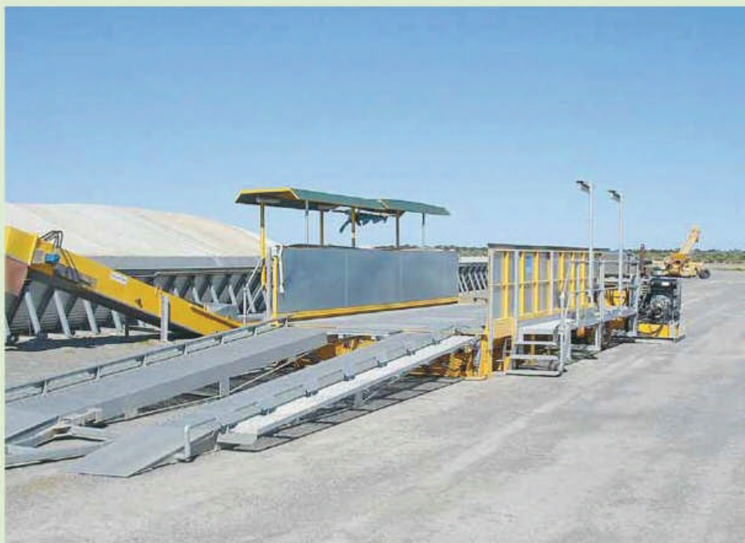
To store grain at the semi-permanent bunkers, these moveable dumpers are used to feed the bunkers, a road vehicle dumps the grain through the grates, and then the auger arm drops the grain into the bunker.
