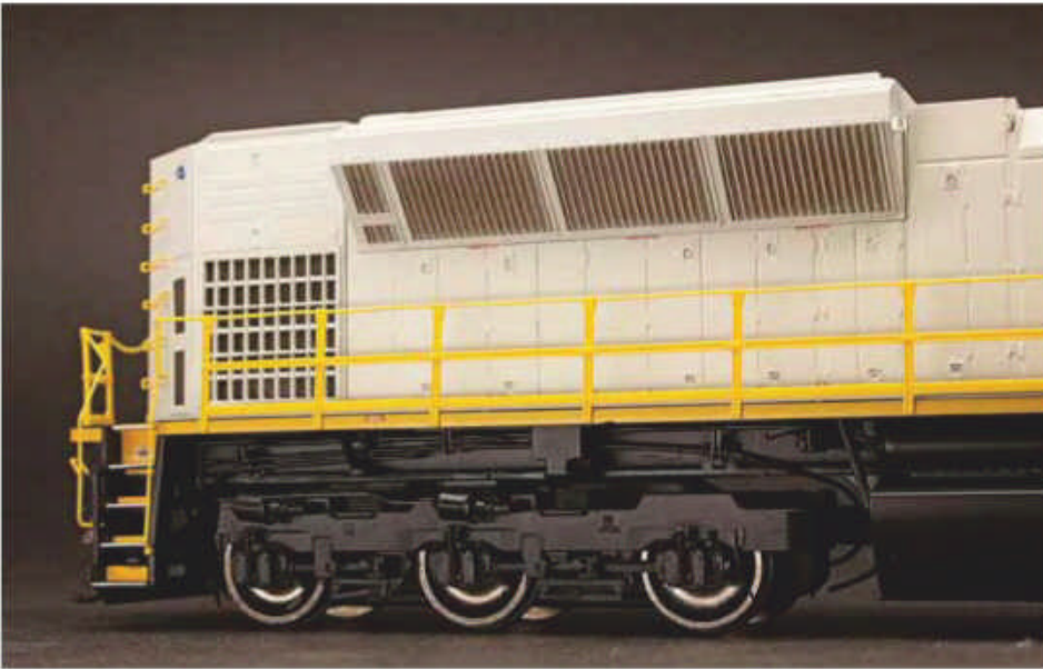
Prototype comparison radiator hood FMG SD9043MAC 907; the fire extinguisher activators are under the walkway near the step wells. Note this is an SD9043MAC and there are differences such as the bogie frames and the door configuration under the radiators.
