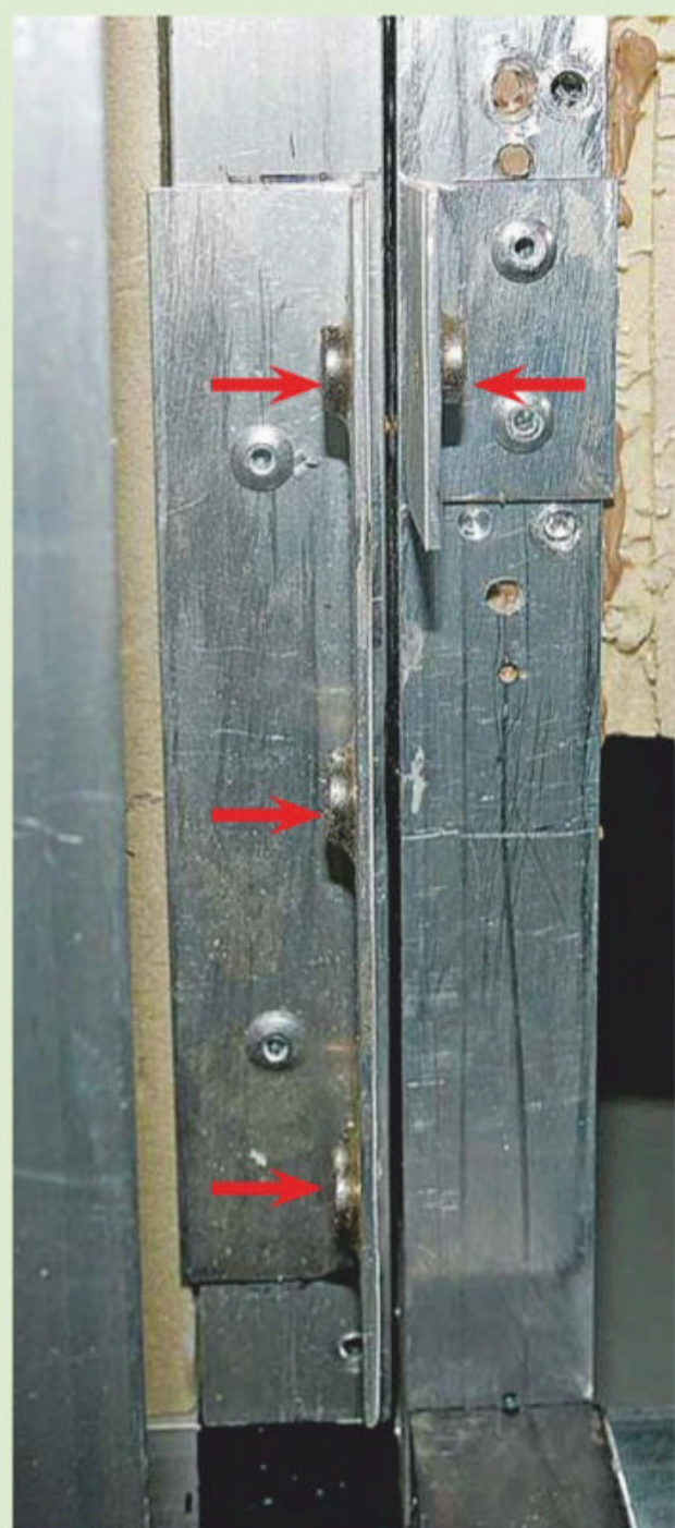
A close-up of the magnets (arrowed) that maintain automatic alignment of the tracks on the traverser with the rest of the layout when the traverser deck is moved.
