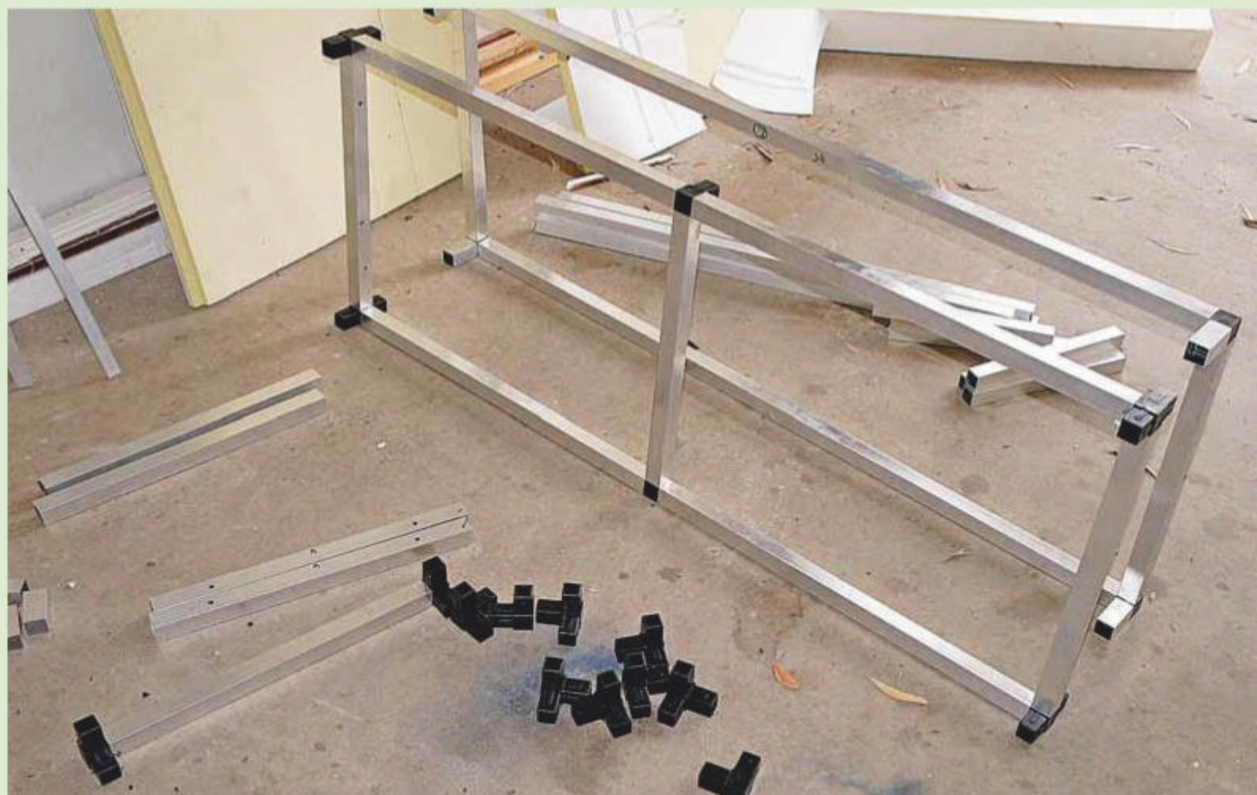
The 'kit' of Qubelok parts, partially assembled into the baseboard frame for Reeves.
