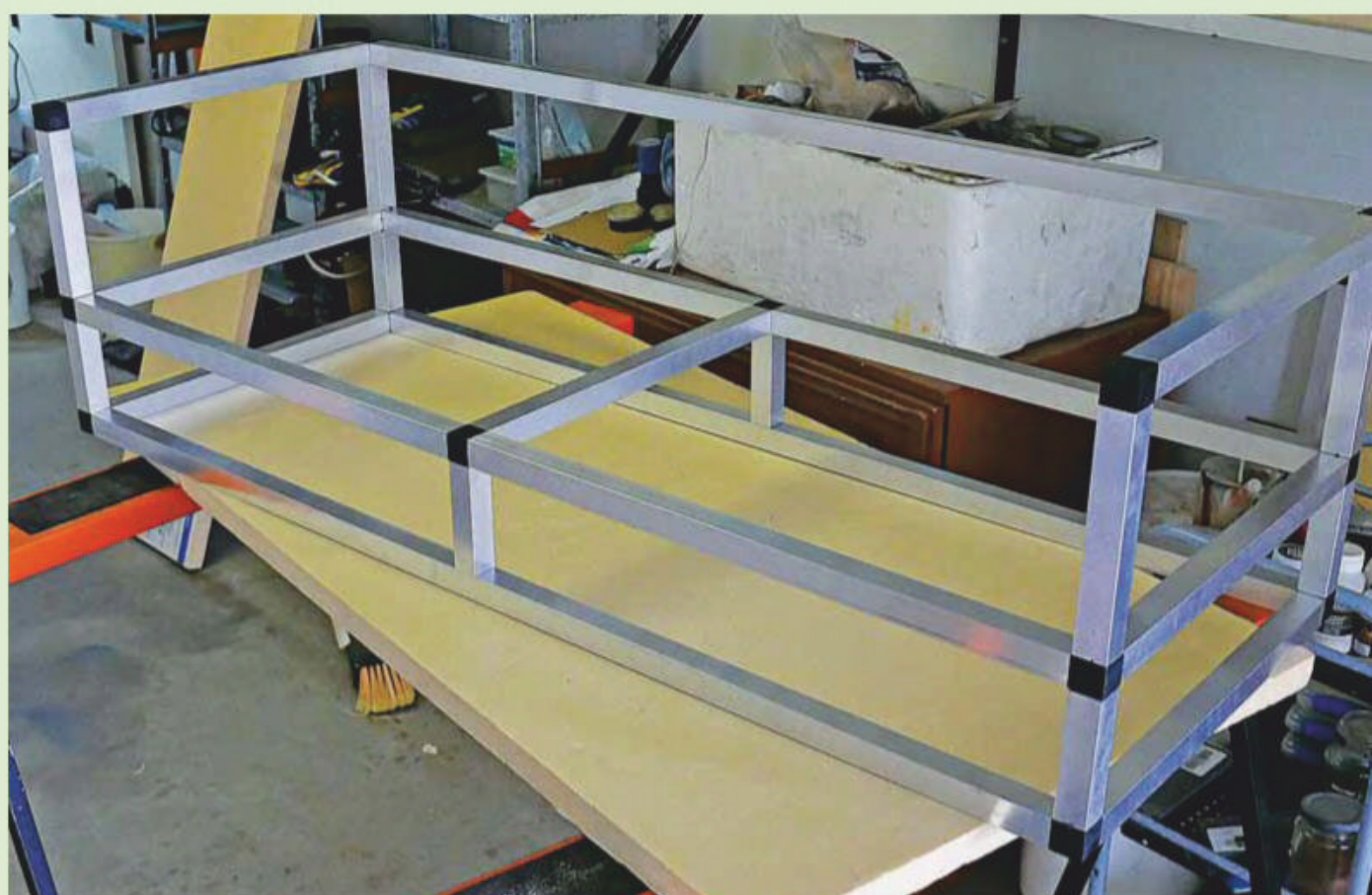
The Qubelok is complete and ready to receive the 25mm extruded foam that forms the baseboard surface.
