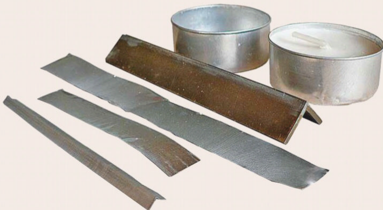
The components needed to create ridge capping. From the rear, new and burned out tea-light candles, the jig described in the text, a strip of foil wrapper from a tea-light candle, a strip cut to width ready for forming, then a strip of ridge capping folded up ready for attaching to a roof.
