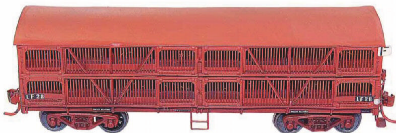
The other 'half' of stock transport on the railways was the rolling stock, which produced some very distinctive vehicles. This HO scale model of VR bogie sheep wagon, LF28, was displayed at the 2016 PMF by Alan Greenhill. The model features a scratchbuilt roof and underframe, while the body was kitbashed from two SEM L class four-wheel sheep van kits, suitably widened, using a photograph of the prototype LF28 as a guide to detailing.
