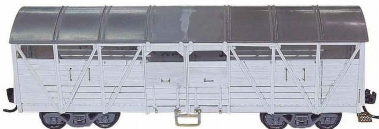
Sheep were not the only type of stock transported by rail, and this under construction, HO scale, VR MF bogie cattle van represents the type of vehicle used to transport said cattle. Also displayed by Alan Greenhill at the 2016 PMF, this bogie cattle wagon was being scratchbuilt using Evergreen styrene strip and sheet. Some proprietary parts were being used, such as the roof, kitbashed from two Steam Era Models (SEM) four-wheel M cattle wagon roof sections, as well as SEM bogies and Kadee couplers.
