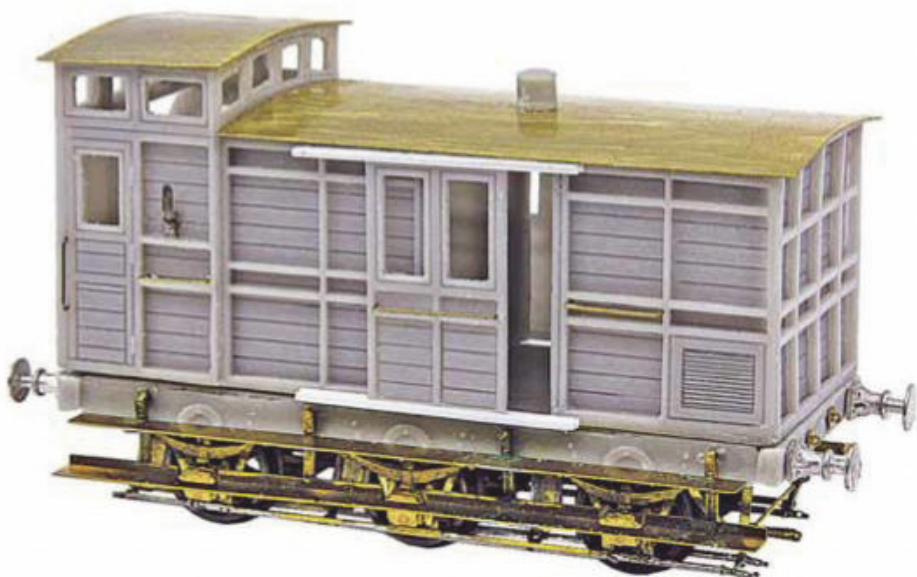
Nearly complete, but unpainted, model, showing the styrene door slides added by the reviewer.
