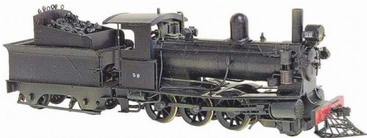
A scratchbuilt HOn3 model of SAR narrow gauge Wx class 2-6-0 No.56 by Adrian Crimes. The model includes brass and nickel silver in its construction, which occupied the best part of twenty years. Featuring some special-order Steam Era Models driving wheels and a 'Minimotor' in the tender, driving a gearbox in the engine via a double universal shaft through the cab.
