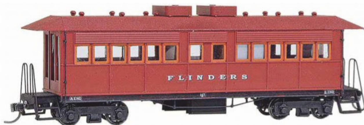
Maddie Collins built this Sn3½ SAR narrow gauge 'Short Tom' car, named 'Flinders', using 3D printed parts and painted it in the standard SAR red livery with orange window frames. The prototype of this particular vehicle has been preserved and can be seen running on the Pichi Richi Railway at Quorn.
