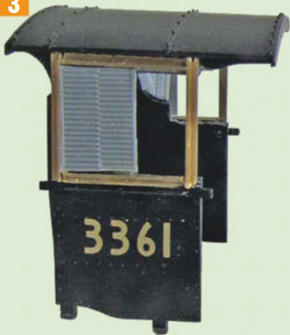
The modified cab, showing the new frames and louvred shutters.
