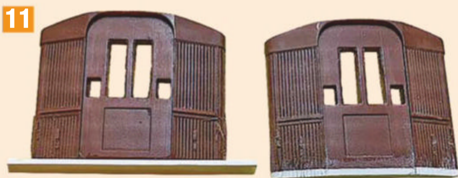
Comparison between an original end, with a 1mm 'packing strip' added to bring it up to the same (scale) height as the sides, and the modified end with the grooves between the timber siding extended onto the packing piece.
