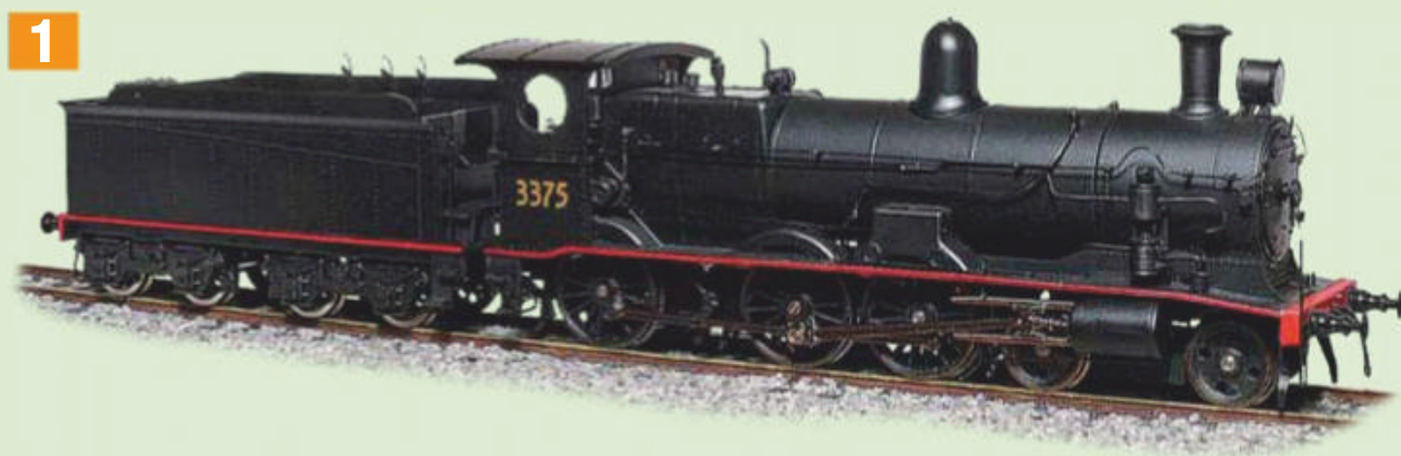
A standard Ixion straight footplate 32 class. Comparison with the prototype photos of G1 and G2 will reveal the differences between the CR G class and the NSWGR 32 class and indicate the detail that has to be added (cowcatcher, air tank on footplate, cab windows and tender extension) or changed (frames below smokebox, chimney and whistle location, plus changing the position of the clack valves). Photo by James McInerney.
