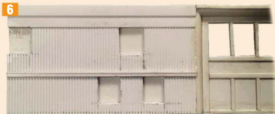
The cut-outs for the coffin chambers and dog boxes have been constructed and the base plates installed. The next step is to construct the louvred doors.
