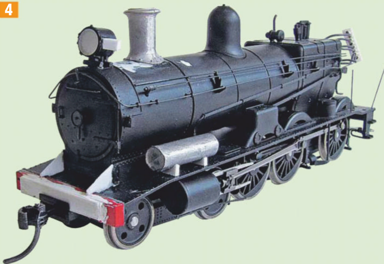
The front end of the locomotive showing the modified buffer beam, front frames and headlight, plus the holes left by the removed NSWGR clack valves and chimney. The resulting holes are filled and sanded, new air reservoir added and the new chimney attached in its prototypical location further back on the smokebox than the NSW version. The whistle is yet to be moved to its CR (and original NSWGR) location on the cab roof.
