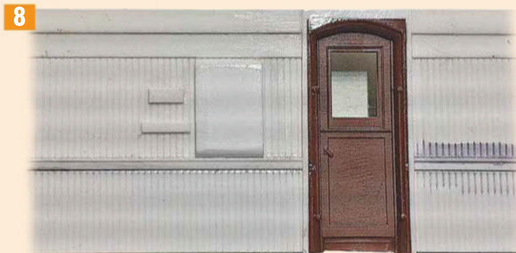
The guard's door, ducket, letterbox and mailing instructions notice board have been added.
