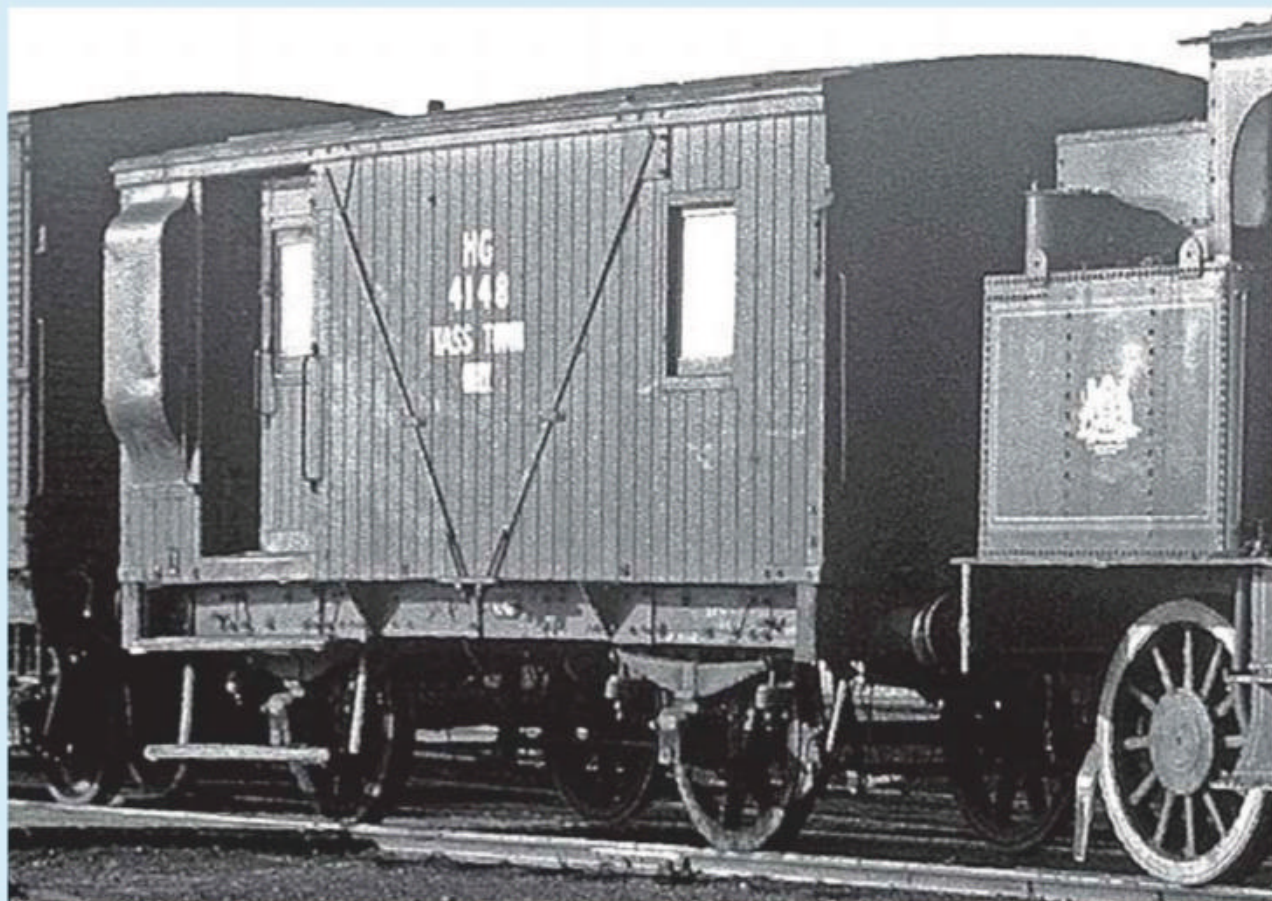
After its 1961/62 rebuild, HG4148 presented quite a different appearance from when it was recorded by Ron Preston in the late 1950s. This photo shows just a single window where the passenger door had formerly been, plain boarding right along the side, and steel 'V' strapping. The footboards have been shortened and the lettering is now 'Yass Town Only'. Photo by R T Clarke.
