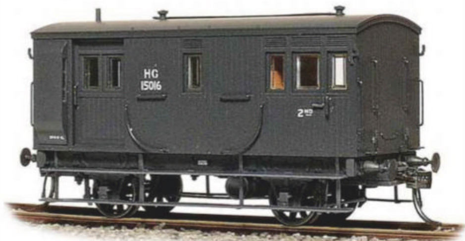
HG15016 from the second Ritchie Bros contract. This contract was the last to be delivered with the centre window in the van. (Casula designation HG1.)
