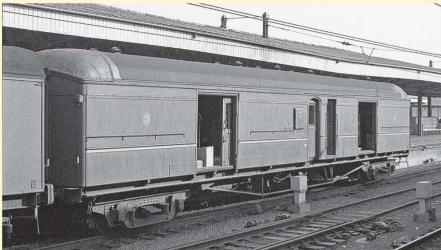
Showing its final form as a VHO with plain side sheeting with no letterboard, as well as the second type of modified guard's compartment, VHO2650, one of the Clyde Engineering-built vehicles delivered in 1928, stands at one of the Sydney Terminal platforms. The image was captured some time between September 1974, when it was renumbered from 1805, and December 1980, when it was rebuilt as an MHO. Photo from the Ian Dunn collection.
