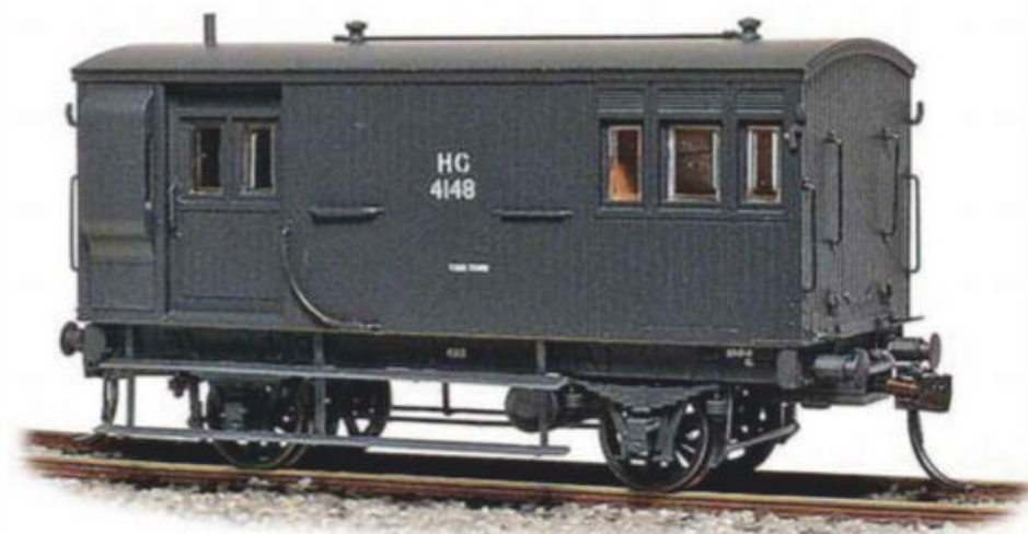
HG4148 is also available in its pre-1962 appearance, as allocated to the Yass Town branch in the 1950s, featuring a boarded-up passenger compartment and short guard's duckets. (Casula designation HG5.)
