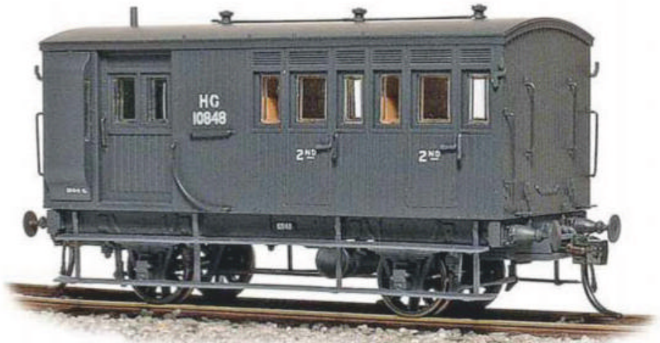
One of the elusive two-compartment vans, HG10848, as fitted with the 'long' guard's ducket. (Casula designation HG9.)
