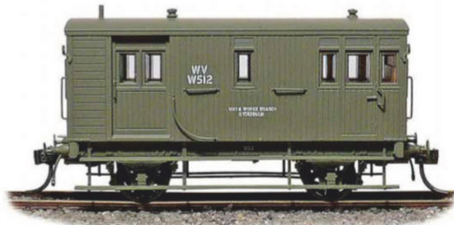
With guard's duckets modified for Way & Works use, similar to L117, W512 carries the pre-1960s dark grey W&W colour scheme. (Casula designation HG15.)
