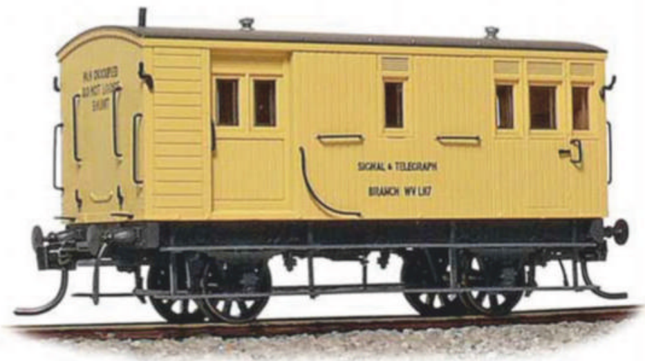
As modified for Signal & Telegraph branch service with the duckets removed and the resulting gap filled with horizontal planking, L117 wears the Ways & Work cream colour scheme introduced in the early 1960s. (Casula designation HG16.)
