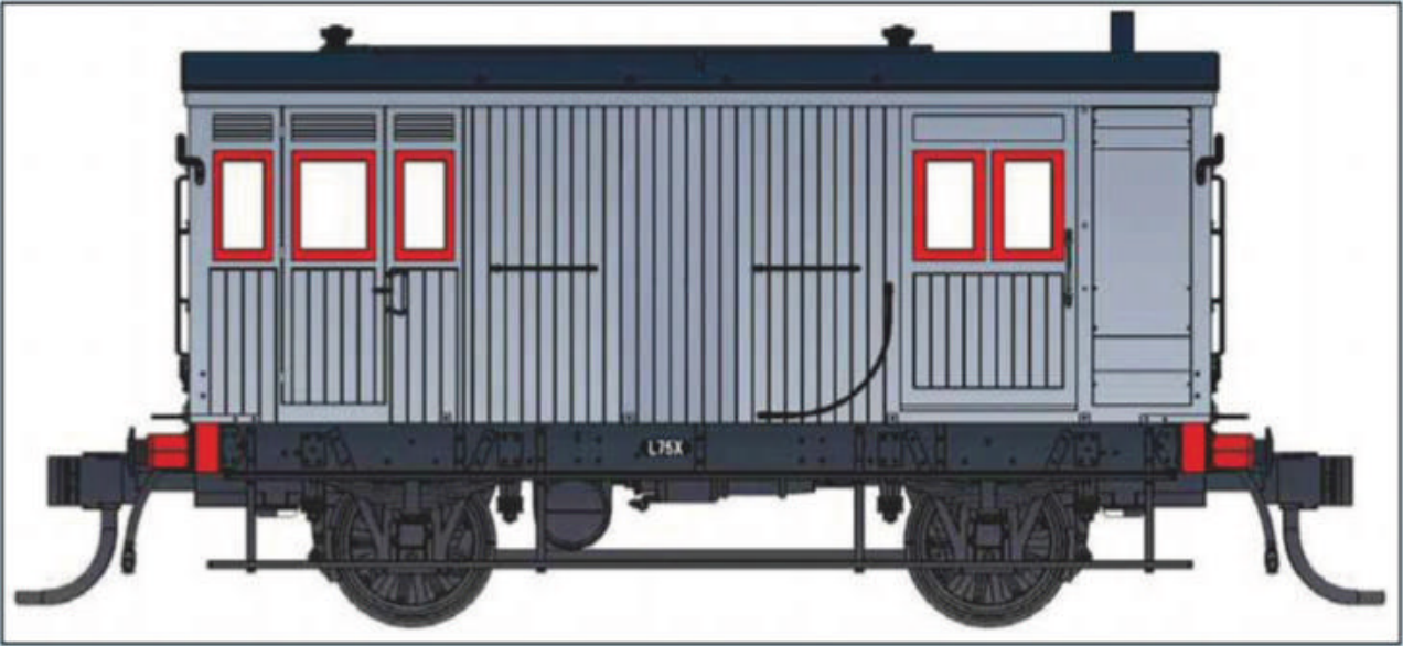
Two more illustrations showing the vans in Way and Works service, after they had been removed from revenue traffic. The image of L75X in a pre-1960s medium grey colour shows a vehicle with minimum modifications, while post-1960s W&W cream-liveried L117 has been more extensively modified, most prominently with the removal of the guard's ducket as per the image of W429.
