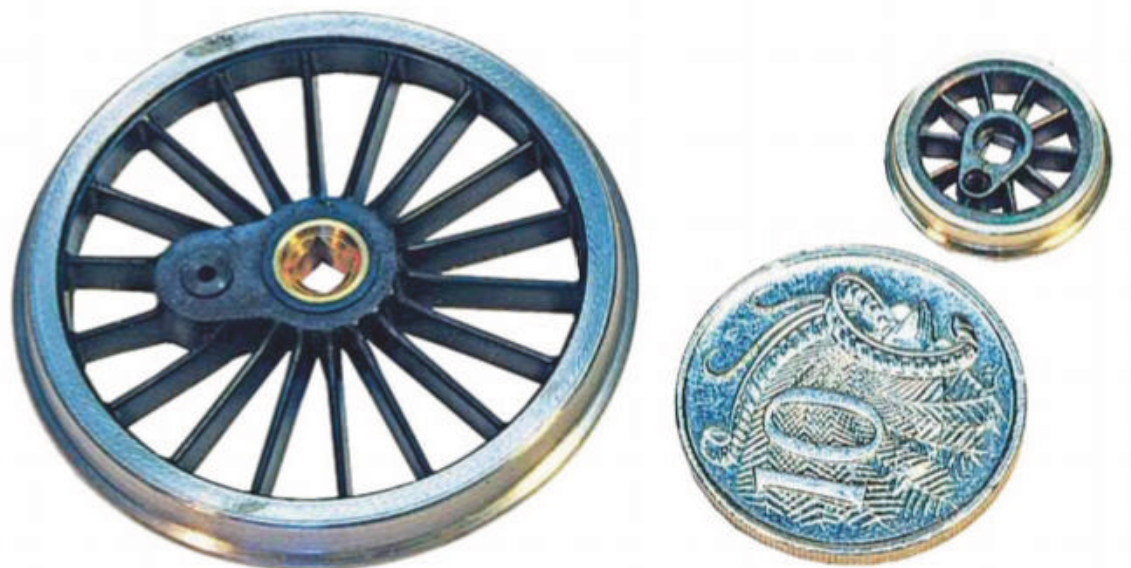
A comparison of two O scale locomotive driving wheels; NSWGR 36 class on the left and NSWGR narrow gauge Krauss 0-4-0T on the right.
