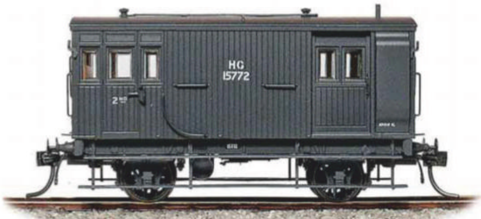
HG15772 from the second Ritchie Bros-built contract without the centre window in the van. (Casula designation HG3.)
