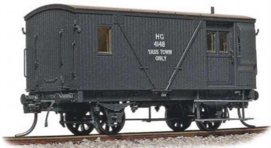
HG4148 in its post-1962 configuration with 'Yass Town Only' lettering. (Casula designation HG8.) The two other vans that were rebuilt in this form are also available (HG5434, used around Taree and HG12351, used for metropolitan goods working) and are identical in appearance, except that they do not have the 'Yass Town Only' lettering.
