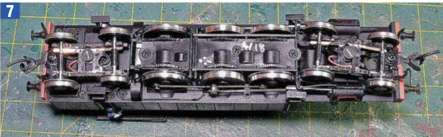
A before and after comparison. The rear bogie has been modified whereas the front bogie is standard. The rear bogie can now swing noticeably further on curves.
