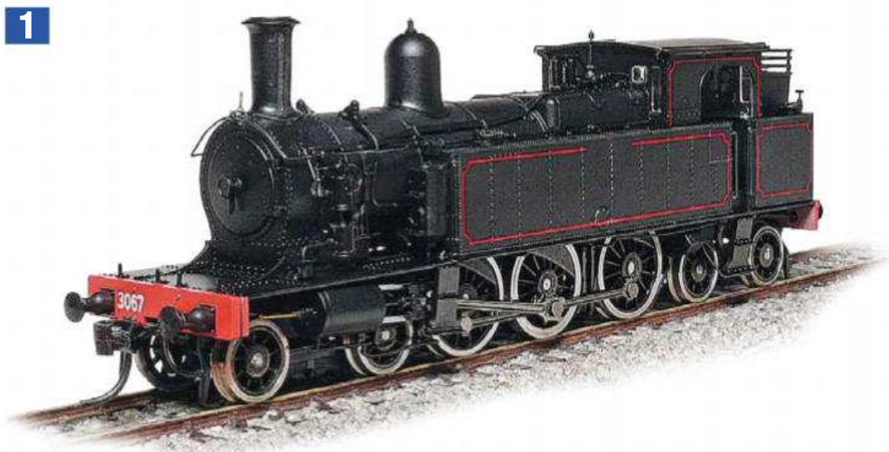
The new front lamp iron and the replacement piston tail rod have been fitted. The tank-side numbers (and part of the lining) have also been removed to allow replacement with brass etched numbers in the correct location.
