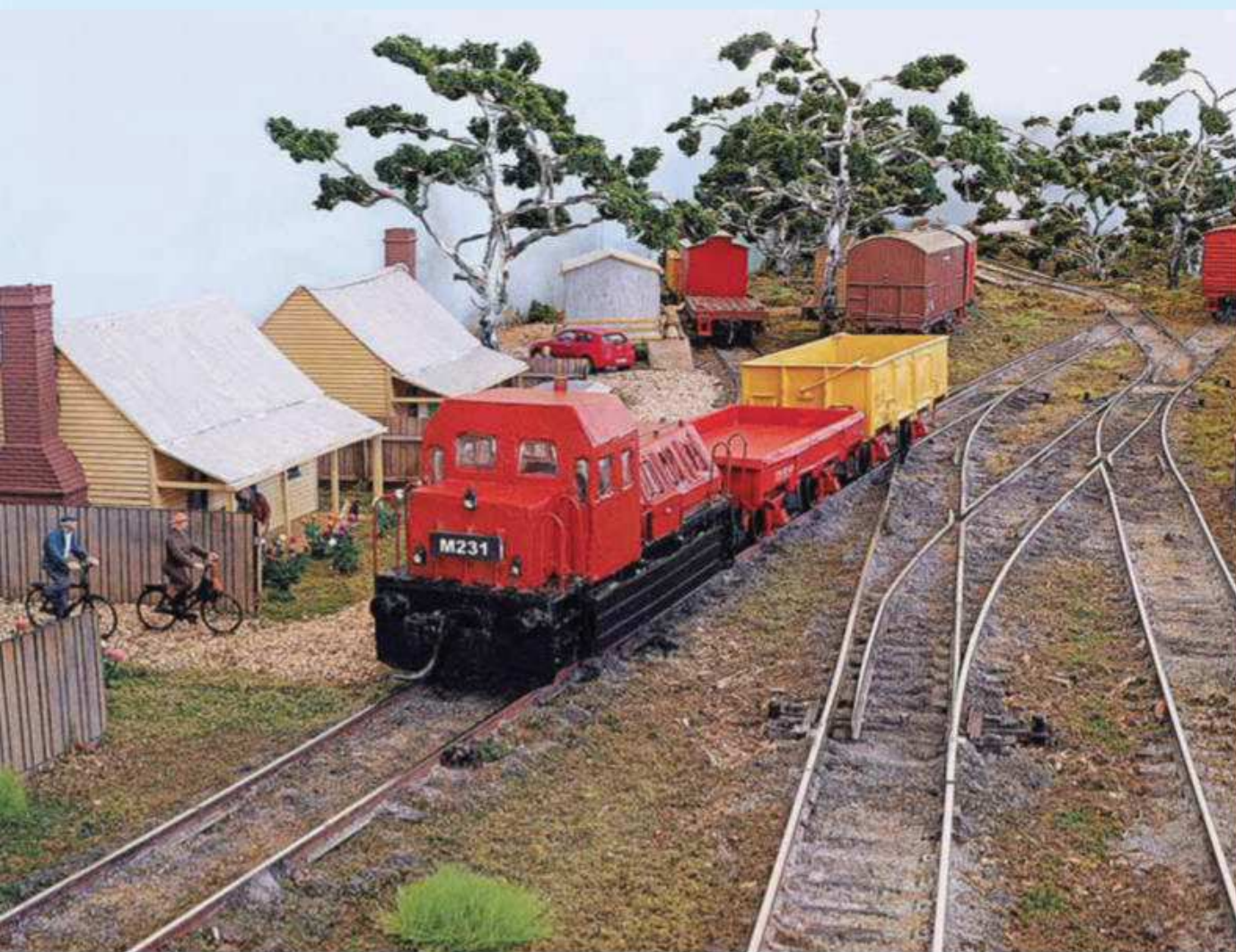
One of the VR's light shunting locomotives, M231, rearranges wagons in the yard. The model is a Lyndon's Trains kit, powered by an SEM Black Beetle. Although the prototype M is a six-wheel locomotive, the model has only the Black Beetle's four wheels, though this is not apparent due to the covering over the side frames. The M class is the only VR red locomotive on the layout. The cyclists are from Preiser and come in a set of three. The third cyclist has been placed on a different part of the layout.
