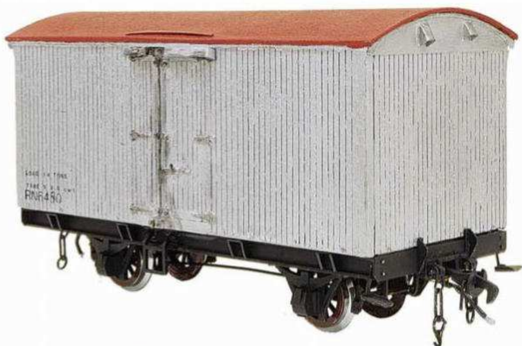
Modelling narrow gauge subjects in large scale (1:24) results in spectacularly sized models that can be well detailed, but are not as overwhelming in size as a standard gauge model would be in the same scale. This model of Port Lincoln Division refrigerated van RN6480 was scratchbuilt from timber, styrene and some 3D-printed parts by Scott Taylor.
