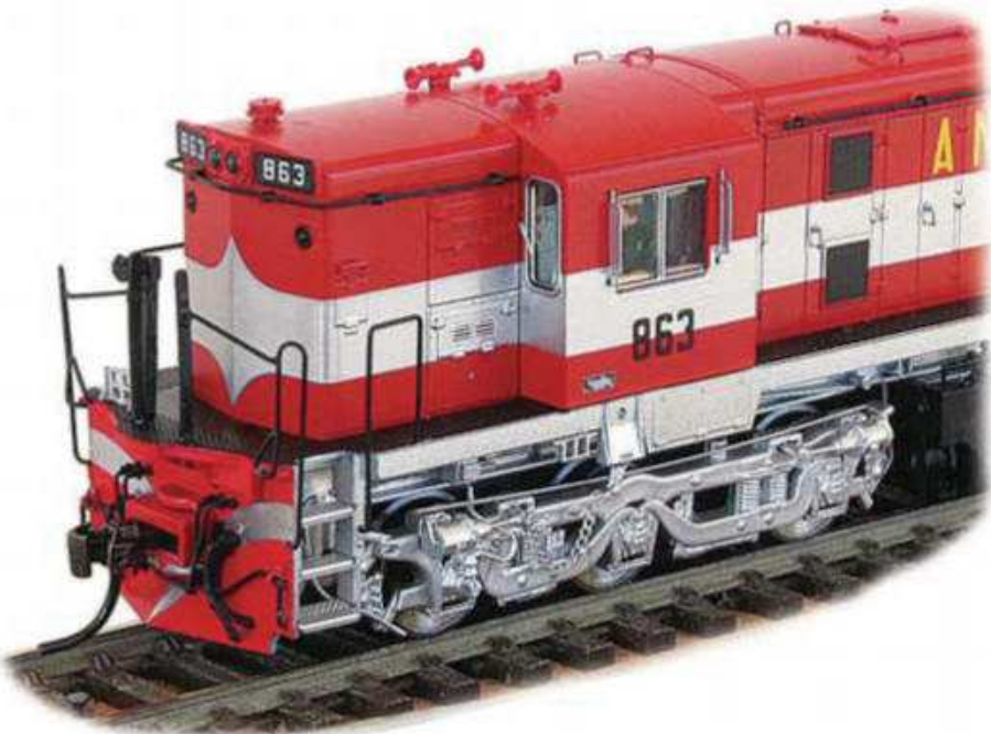
A view of the cab area of ANR red/silver 863. The cab detail, such as the control stand, is clearly visible through the cab windows. The different versions have different details, as appropriate to the prototype, such as the destinations board frame on the SAR 830 and buffing plates on the NSW 48.
