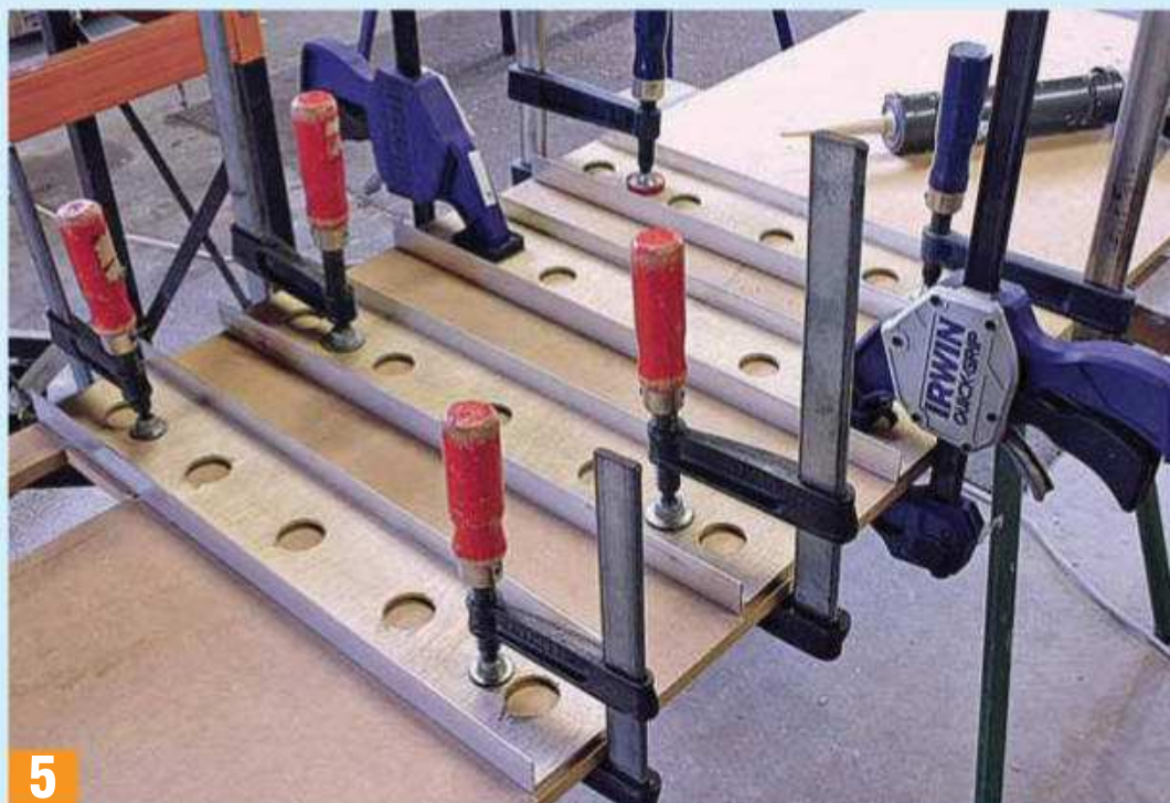
5 Four crossbeams under construction with the aluminium channel glued to the ply. When the glue sets 1/8" holes will be drilled through the web of the aluminium and the ply and rivets used to secure the aluminium to the timber.
