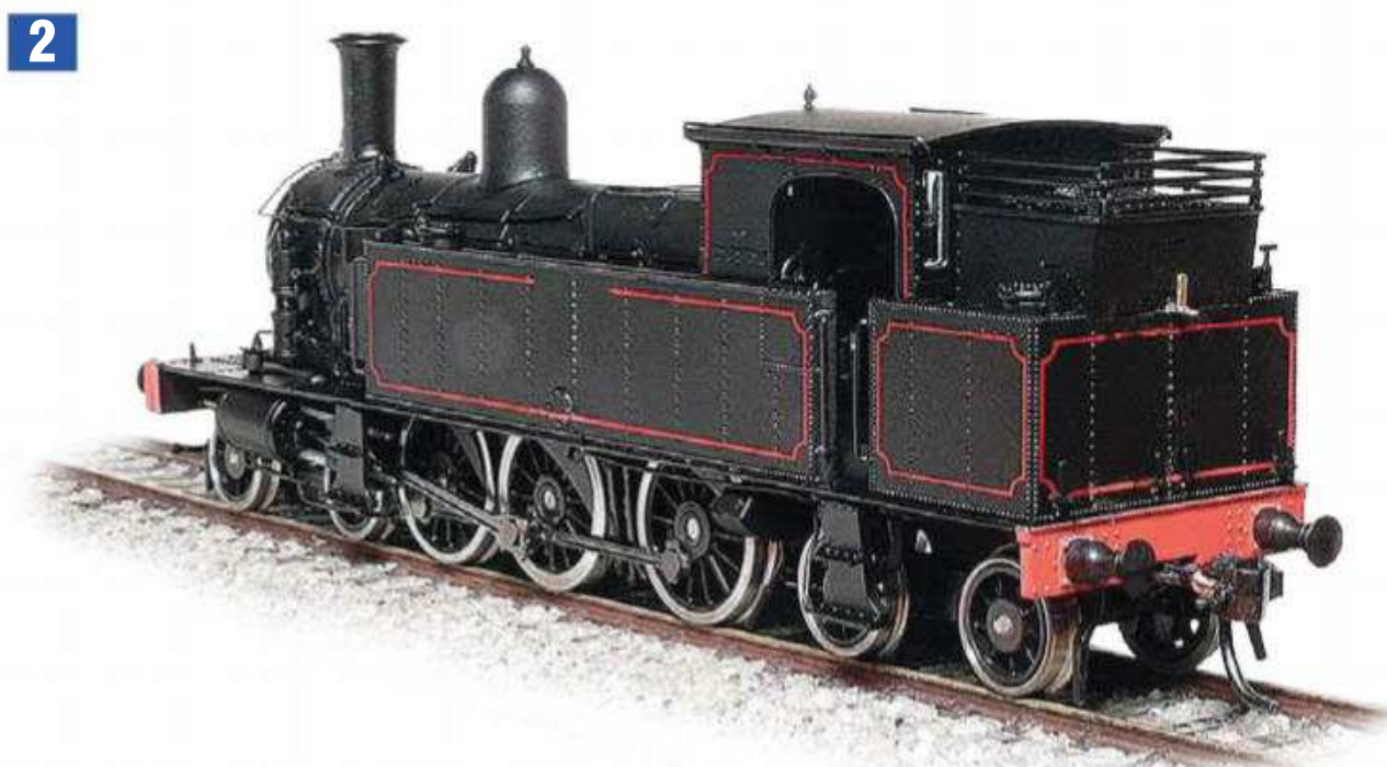
The new top lamp iron has been fitted to the bunker and the rear numbers have been removed. This photo was taken long before the author found out about the underscale width cab roof.
