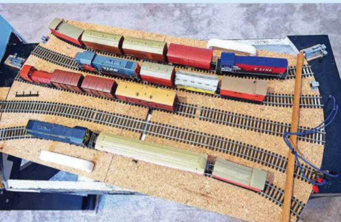
An overhead view of the 'train-table'. The two white handles are used for turning the table. The bolts are there to hold it in place when being transported. The stick is a safety measure to prevent a train coming off the end of the track and also visible is the highly 'complicated' wiring used to select which train is to be run. Photo by Les Ryan
