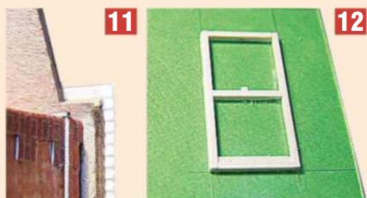
▲ Constructing the window frames from styrene strip glued to clear plastic.
