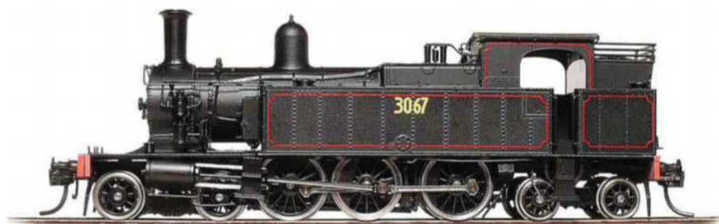
The front bogie has had the scale-sized wheels fitted, while the rear bogie retains the standard, smaller than scale, wheels. Fitting the optional wheels is a simple matter of popping out the old wheels and then slotting the optional wheels back into the axle slots. It is not even necessary to remove the bogies to do so and the instructions included in the box specifically advise that it is neither necessary nor advisable to remove the bogies to fit the optional wheels.
