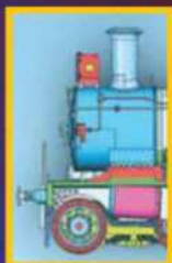
Superheated drumhead smokebox
