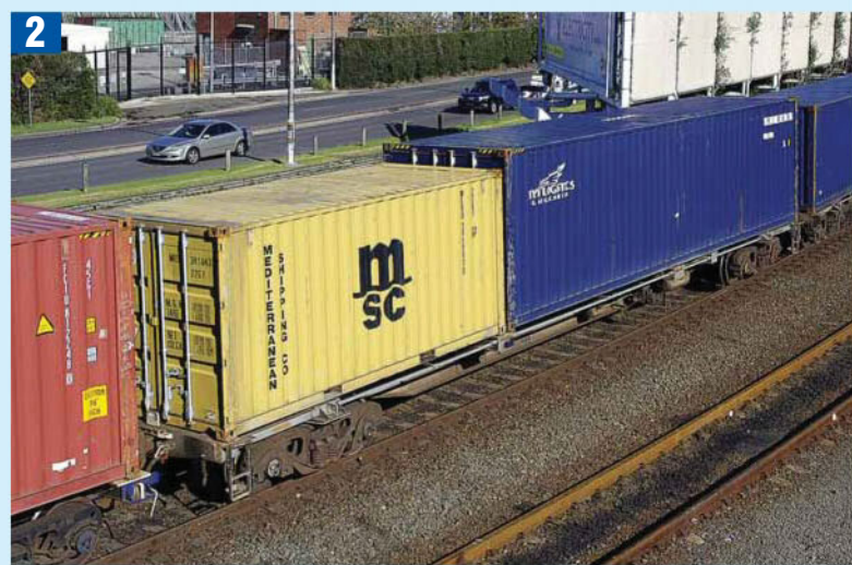
2 Arriving at Port Botany on 1 July 2013, these MSC 22G1 and NYK 45G1 containers show the two most common types used in Australia. The photo also shows the one foot height difference between the two types. The containers are on a QUBE owned LQAY wagon as part of a port shuttle consist from Minto to Port Botany.
