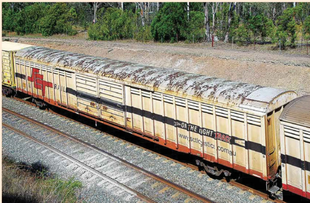
► Hauled as part of an Aurizon service, ABSY4472 displays a badly rusted, but original, roof skin at Bargo on 22 January 2017.
