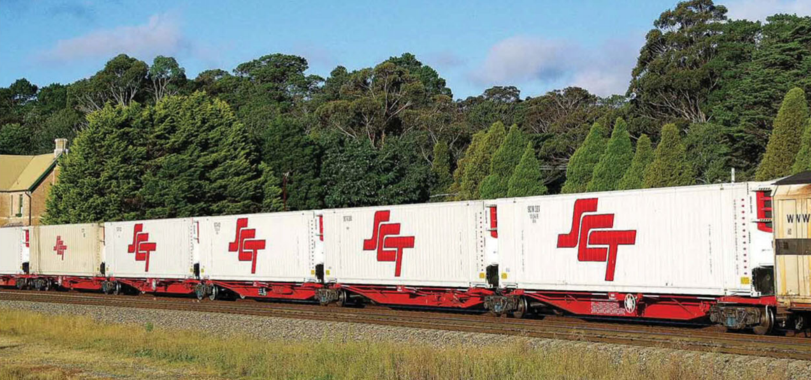
▲ Five-pack PQQY50008 south-bound at Mittagong on 19 April 2017, loaded with five SCTR 48'+ refrigerated containers. The first four containers are in the 300 series and the fifth container with the smaller logo is in the 200 series.
