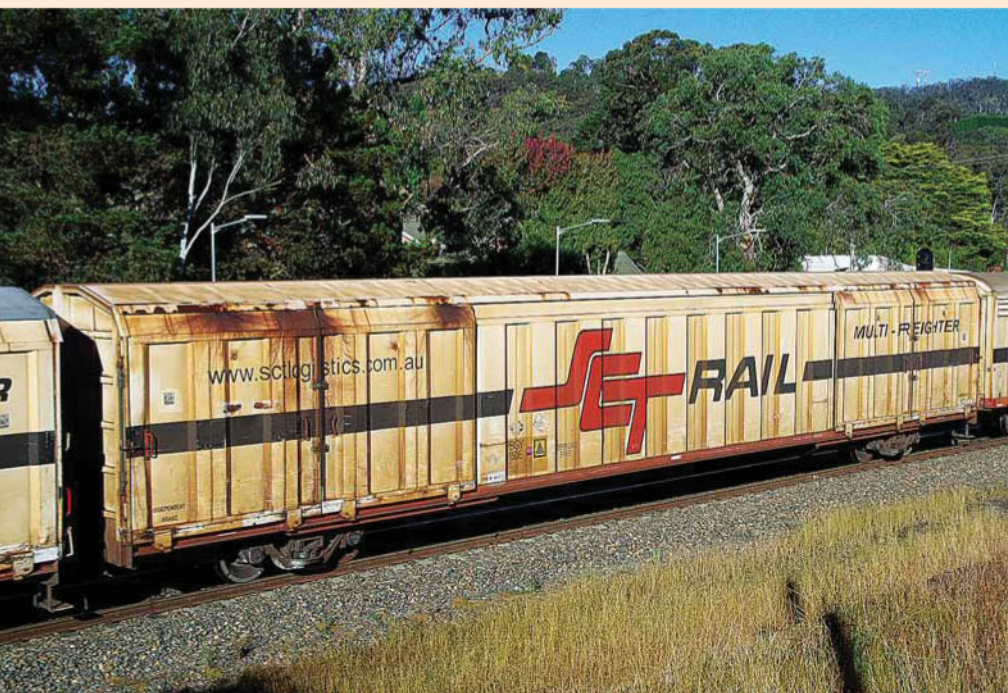
▼ Van PBGY0150 heading north at Mittagong on 21 May 2017. This vehicle still has the original roof and has significant rusting around the tops of the doors.
