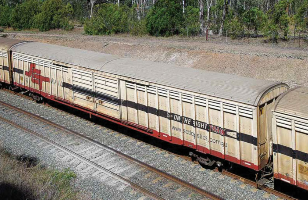
▲ ABSY2819 displays a new corrugated metal roof at Bargo on 22 January 2017, photographed as part of the same Aurizon train as ABSY4472.
