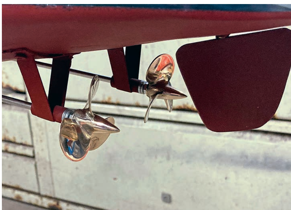
The new twin propellers and rudder are shown here in place. The original single shaft was removed to provide better redundancy in the event of a breakdown, and the propellers are beautifully cast items from Prop Shop.
