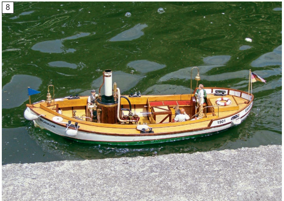
The beauty of an open-hulled model is the fact that you can run it past where you are standing on the bank and quickly check both steam pressure and water level as frequently as you feel necessary.
