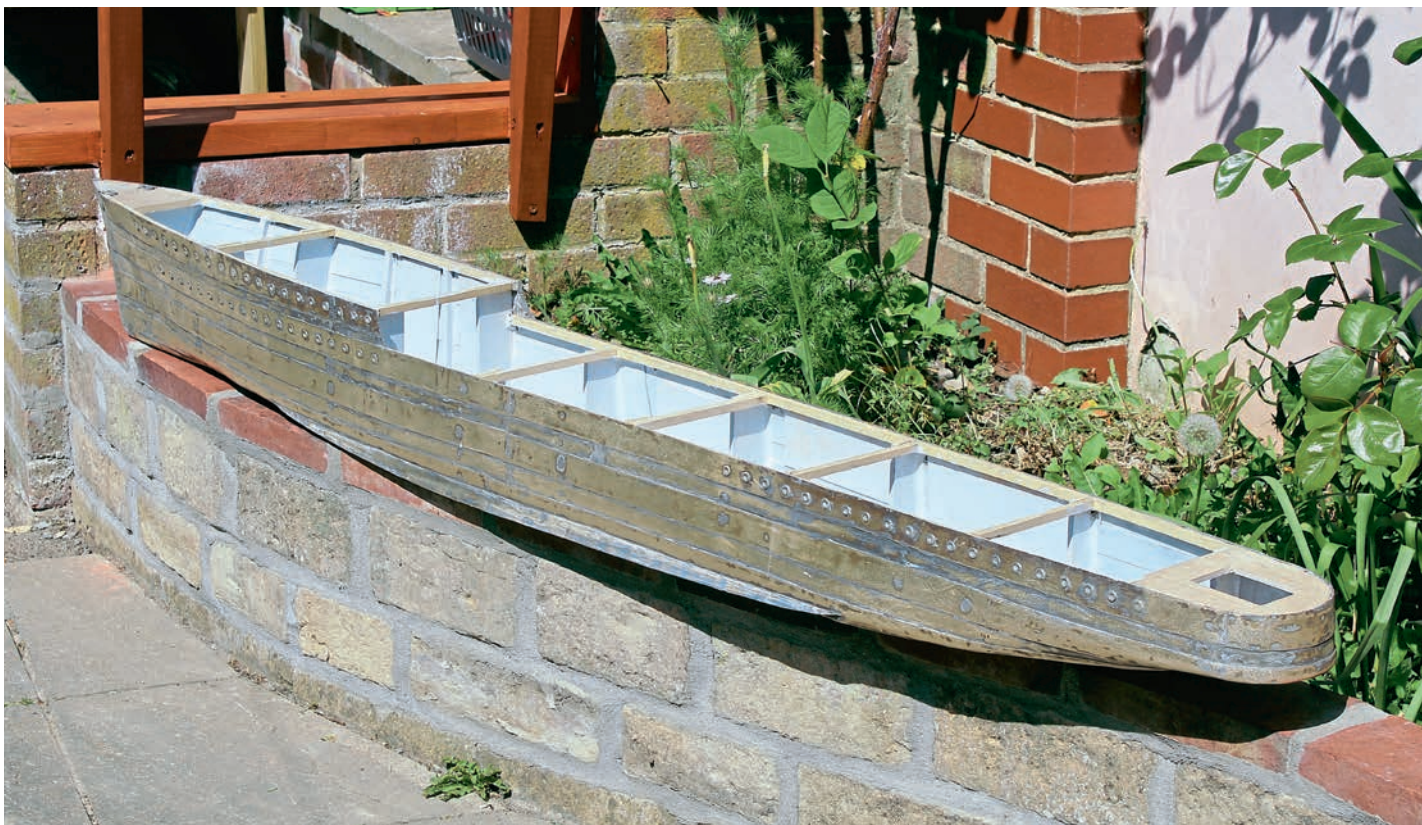
New deck beams were fitted to help retain the brass-plated hull sides, improving the model's durability both on the lake and during transport. As you can see here, the interior was painted white to help seal the structure and make any future issues easier to spot.
