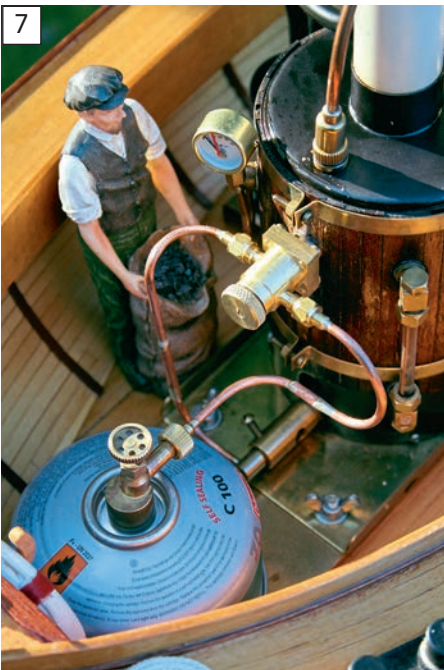
A useful addition to save steam, and therefore gas, was the Forest Classics attenuator valve, which while unusually mounted directly on the boiler shell has proven to be effective and reliable for many years.
