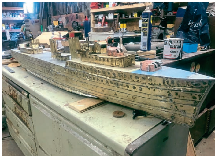
In much the same way as the hull, the superstructure was treated with paint remover and carefully reshaped to restore its original form and profile. At this stage, the new deck had been fitted and covered with lithoplate to recreate the appearance of metal plating.
