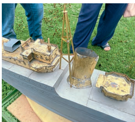
First sea trials. Initial primer had been applied to the hull, but she was still leaking through numerous tiny gaps in the plating. The superstructure was temporarily fitted with some of the detail parts to assess how she sat and behaved on the water.
