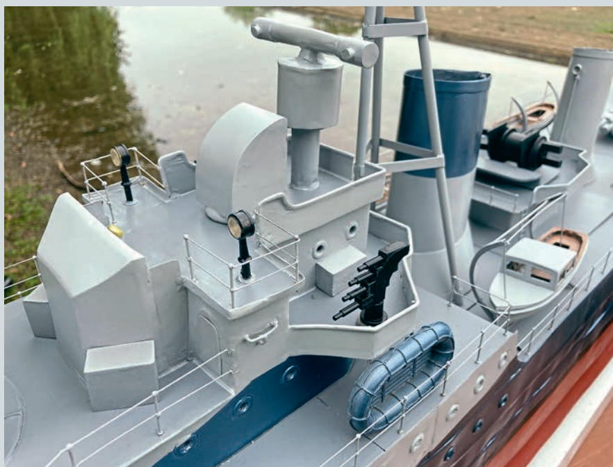
The torpedo tubes, four-barrelled pom pom mount and director tower all required either complete scratch building or substantial reconstruction. The brass section in your model shop will be your best friend for projects like this.
