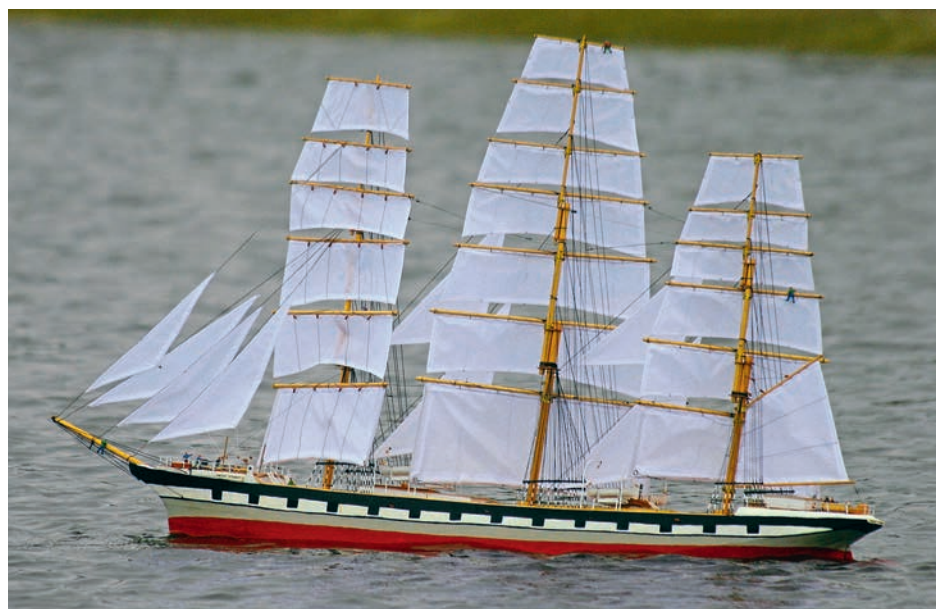
This is tacking. The boat has been on the starboard tack, taking the wind from the starboard side. The rudder has been turned hard to starboard, into the wind, and the bows have gone around across it. The main and mizzen yards have been braced round on to the port tack, and the foremast sails, still on the starboard tack, are pushing round the bows to complete the manoeuvre.
