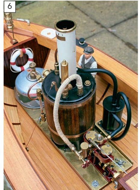
The twin oscillating engine is simple to operate and maintain, and the model can be turned around on the bank almost as quickly as some electrically powered models. Richard has a good feel for its operation as it has served him well for many years.
