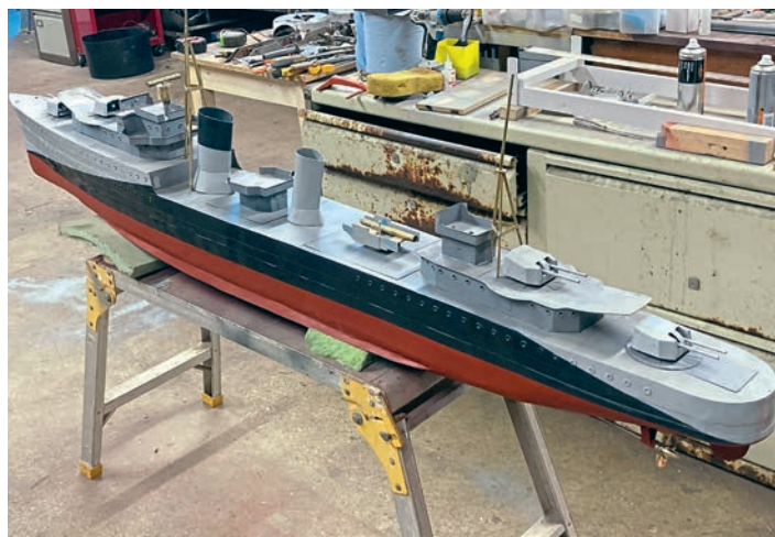
The final colour scheme being applied to the model, once again using paints from the Halfords car paint range. This scheme was carried by the original HMS Eskimo during World War II and, while not 100 per cent accurate, gives a good impression of the full-size ship.
