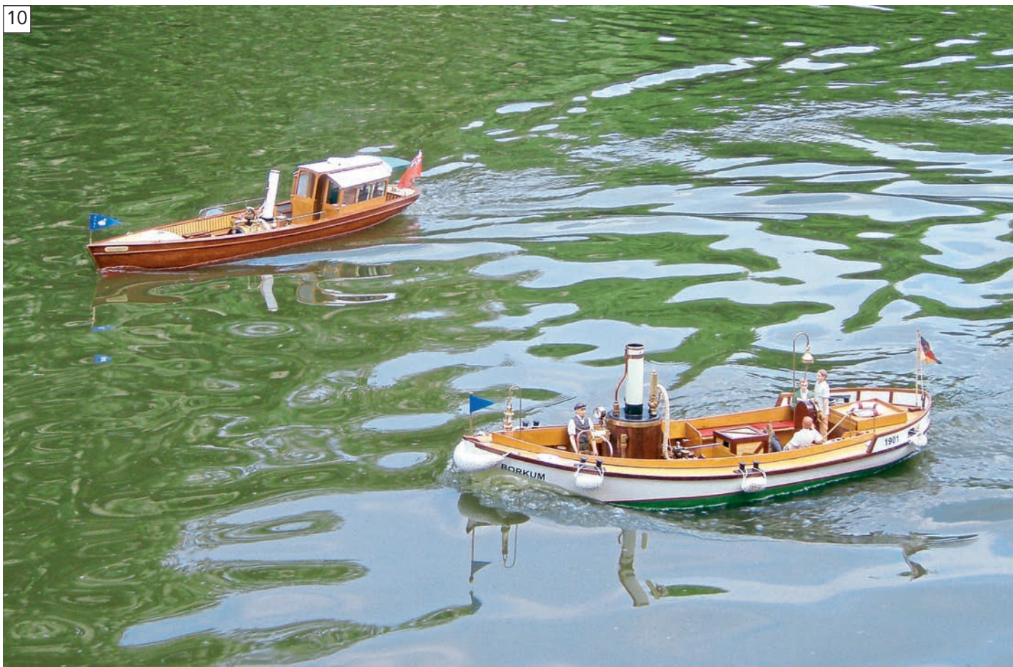
Despite being a relatively small engine, the Puffin certainly pushes the Borkum at a brisk pace. Not surprisingly, this uses steam a great deal faster, so the frequent water level checks are necessary to make sure there is enough left.
