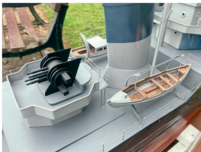
Further outfitting work included the installation of ships' boats, ammunition lockers, searchlights, and additional operational fittings characteristic of warship service. The mast assemblies are shown fully constructed and finished with the same paint to match the hull scheme.
