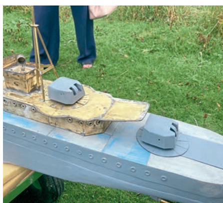
First sea trials. Initial primer had been applied to the hull, but she was still leaking through numerous tiny gaps in the plating. The superstructure was temporarily fitted with some of the detail parts to assess how she sat and behaved on the water.
