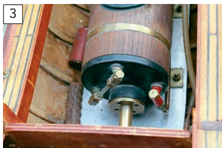
A more common arrangement with horizontal boilers is to have the sight glass mounted entirely on the end plate of the boiler, as is the case with this Stuart Turner boiler.
