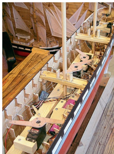
In this view, looking aft, the sail arm for the foremast is to the fore of the picture, with the ones for the overlapping masts beyond. The 'thwarts' which support the deck can also be seen locating the masts and fairleads.
