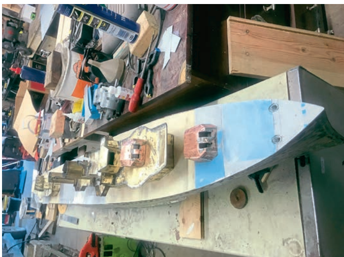
In much the same way as the hull, the superstructure was treated with paint remover and carefully reshaped to restore its original form and profile. At this stage, the new deck had been fitted and covered with lithoplate to recreate the appearance of metal plating.
