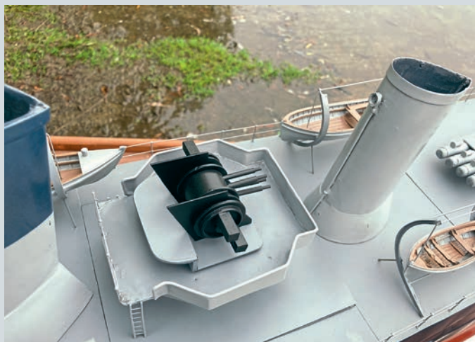
The torpedo tubes, four-barrelled pom pom mount and director tower all required either complete scratch building or substantial reconstruction. The brass section in your model shop will be your best friend for projects like this.
