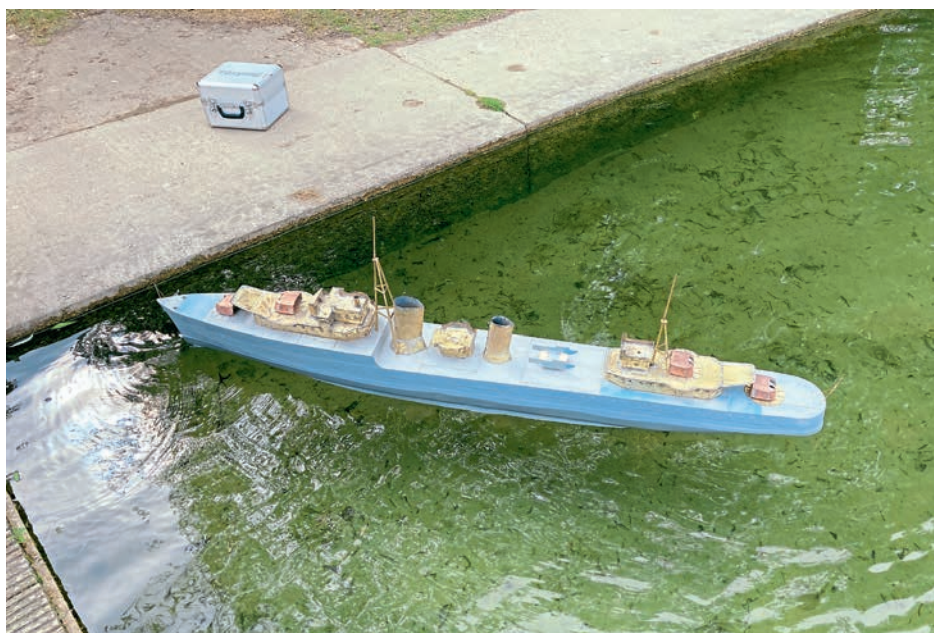
First sea trials. Initial primer had been applied to the hull, but she was still leaking through numerous tiny gaps in the plating. The superstructure was temporarily fitted with some of the detail parts to assess how she sat and behaved on the water.
