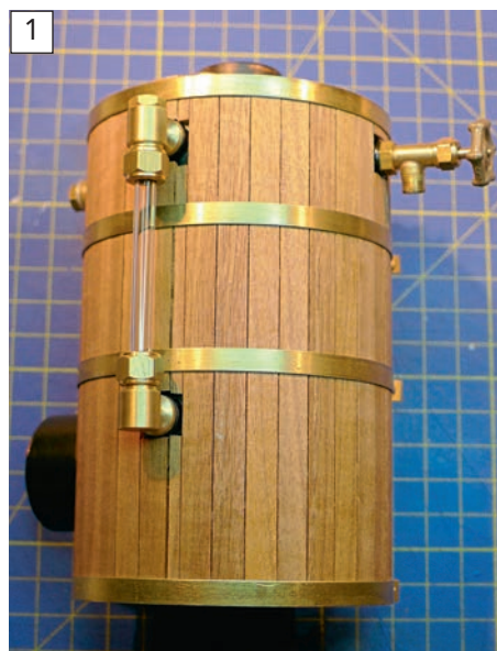
Sight glasses can be mounted on the side plating of a vertical boiler, such as is the case with this Pendle 3-inch boiler.
