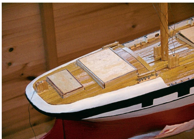
The 'turtleback' again, after decking. It can now be seen how much of the deck space is reduced by this piece of elegance. Note the fairleads, sticking well up above the deck at either side of the mizzen mast. The lines through them will form the braces for the main mast yards.
