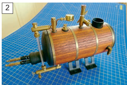
You can also find sight glasses mounted on the side plating of a horizontal boiler, such as the Hemmens boiler pictured here. This gives a relatively long sight glass, which is good for determining water level but can also be a bit vulnerable.
