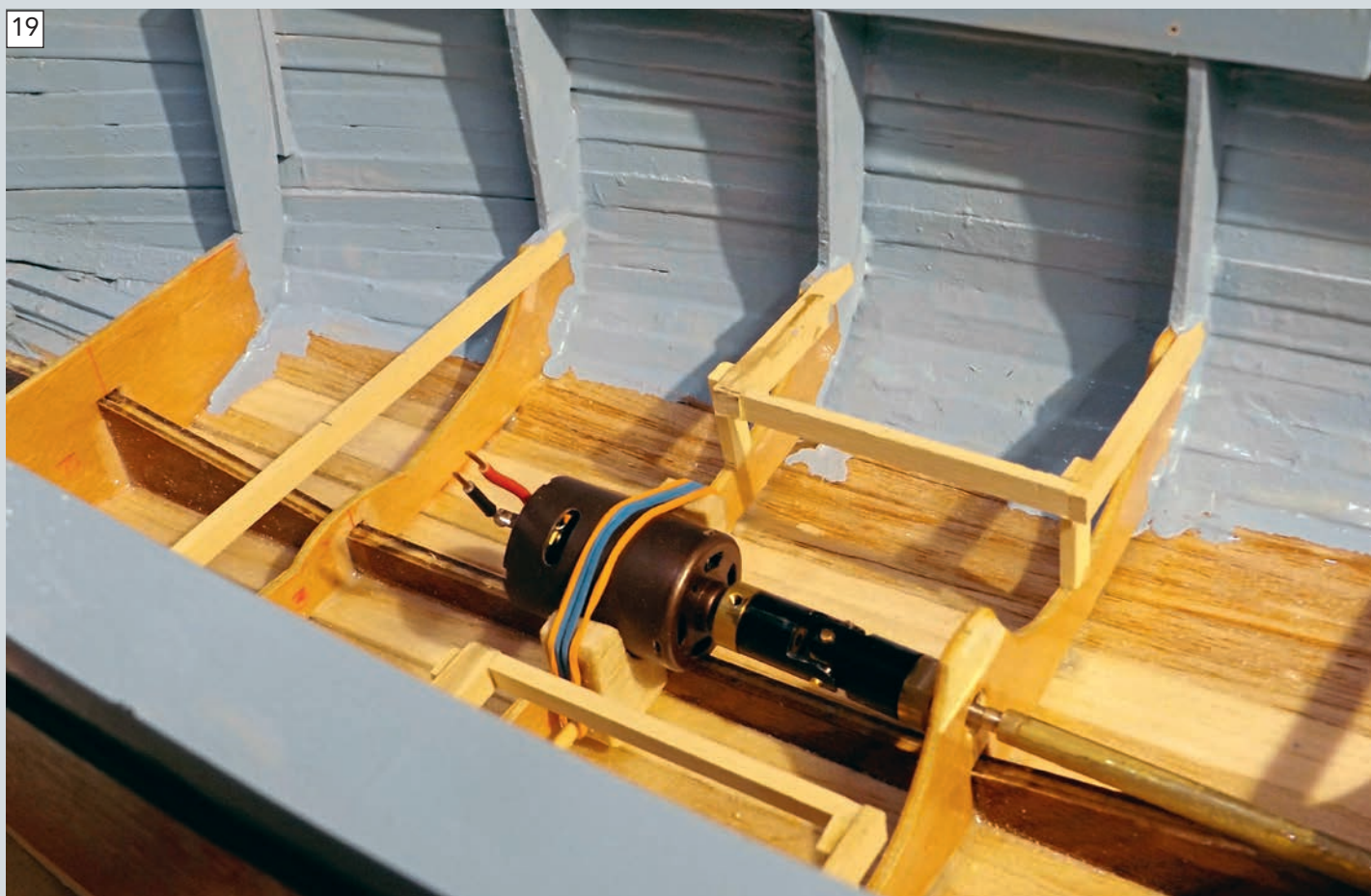
The motor secured in place. In my model, the Huco type coupling rattles so much that some people think I have a sound unit fitted! The side decks and cockpit side coamings are created from 1/32-inch ply. As you can see, the internals in my model were given two coats of Humbrol light blue enamel.
