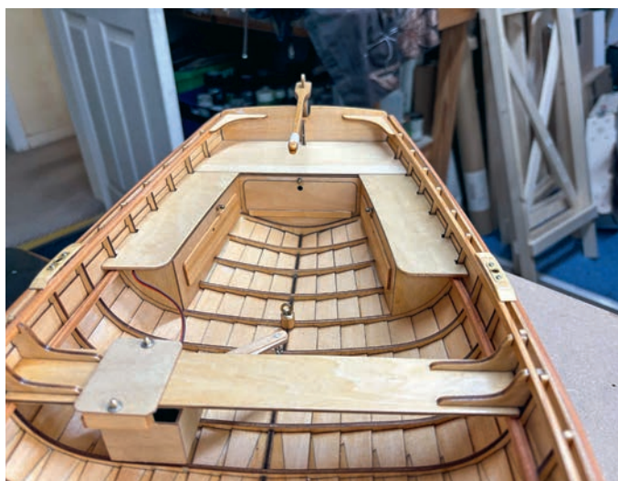
The seat at the rear of the boat houses the servo for the rudder, while the receiver and batteries are neatly tucked away beneath the boxed-in benches.
