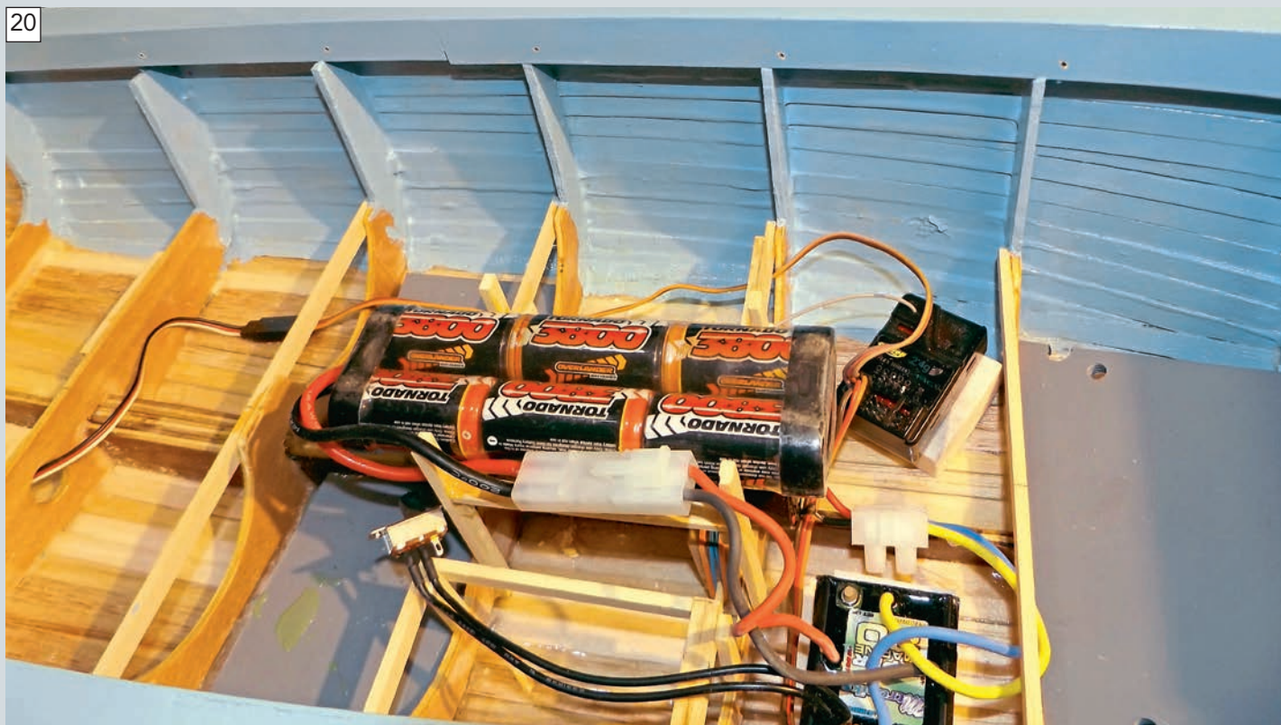
The 7.2-volt Nicad pack sits on a simple obeche framework over the motor inside the engine box. The ECU and receiver can be mounted with Velcro patches on blocks to keep them high and dry, just in case there is any seepage of water into the bilge.
