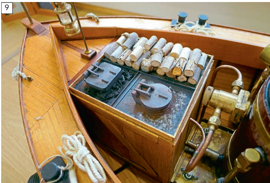
When using disposable gas tanks, it's worth coming up with some sort of enclosure to hide the tank. Richard decided to go for a bunker arrangement, which incorporates a water tank, coal bunker and wood store.
