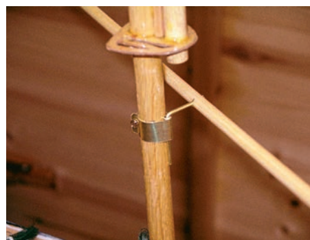
The attachment of a yard to a mast. You can see the yard is about 15 mm ahead of the mast, vital to its ability to rotate 'around' the mast and reach within 30 degrees of the hull's centreline.
