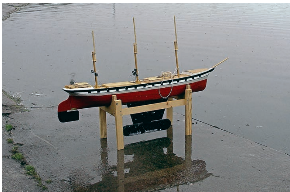
A trim trial at the pond in Tynemouth. Here, the oversized rudder and large, removable sailing keel can be seen. Only the lower masts and topmasts are in at this stage, the topgallant masts will be fitted next.
