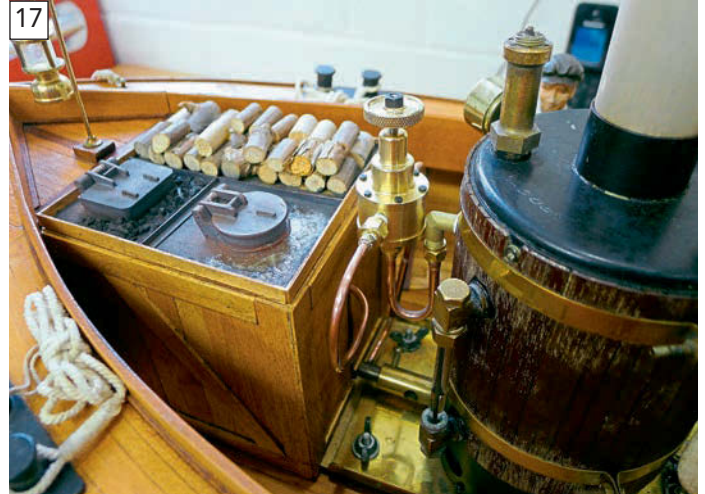
Mounting vertically also allowed the bunker to be replaced, so a much better arrangement.
