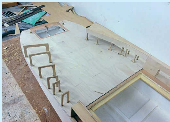
Removed from the building stocks, the hull was then flipped to start the work on the deck, with the deck plating and railway tracks being laid down.
