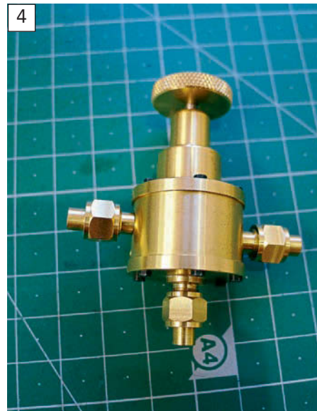
Nuts and cones came fitted to all three connections and ready to solder to pipework. Richard did, however, find the fitting for the steam connection was designed for a slightly smaller diameter pipe than used with his previous valve.
