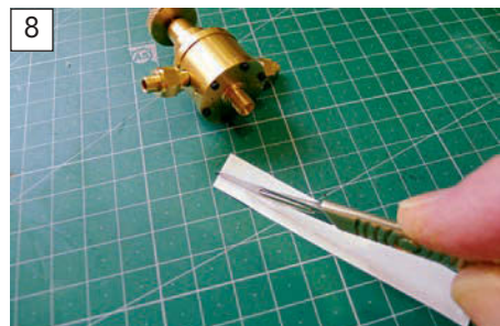
A twist of PTFE tape on the valve steam connection threads ensured a sealed joint on the boiler.
