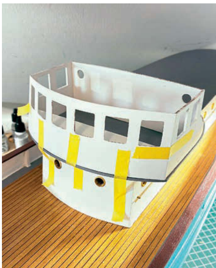
Assembling the wheelhouse.
