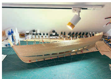
Making a start on planking Nordkap's hull. The entire hull will be filled later, but to make work faster and easier, pins can temporarily be used to secure your planks in place.
