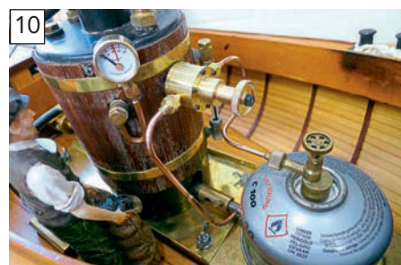
Back in the Borkum with everything looking neat and ready for a run. The control knob certainly proved easier to turn, probably because the spring rate is quite a bit lower than that of the original.
