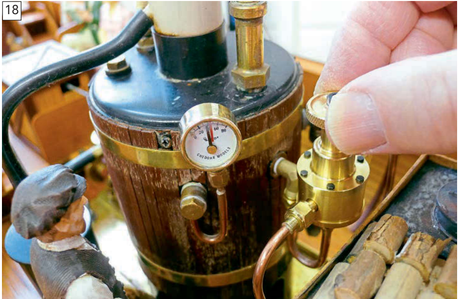
Another test run proved that the valve worked perfectly proportionally to the requirements of the engine. Before Richard puts the model on the water again, he will mark the control knob with a spot of paint at the point of normal working pressure.
