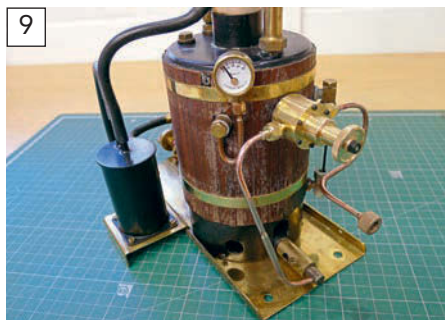
Richard was hoping for a direct swap over using the same original pipes, but the threads on his new valve differed slightly from those on his old valve, so new pipes had to be made up.
