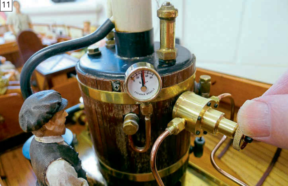
Once the pressure reached Richard's desired point, the control knob was backed off until the flame was heard to die down. Depending on your boiler, you may have to listen carefully for this, but you should be able to tell.
