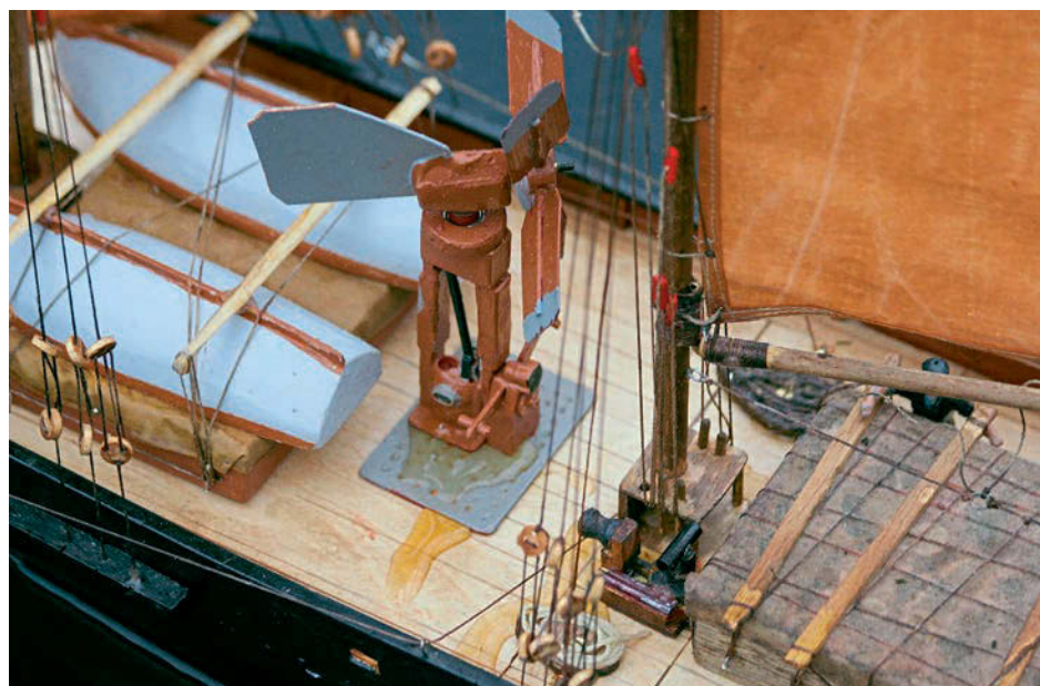
The windmill 'pumping': there is dirty water on the deck, which the screen washer pump has lifted out of the tank and sent to the scuppers from the outlet of the windmill pump, which is the grey oval at the pump's base, exactly as the real thing.
