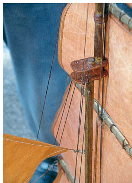
The yards are mounted on a long shaft located in front of the foremast and are supported by a bracket under the topgallant (next to top) yard. The royal (topmost) yard is carried on lifts and can thus be lowered in strong winds. The yards are braced by braces attached to the foreyard (the bottom one).
