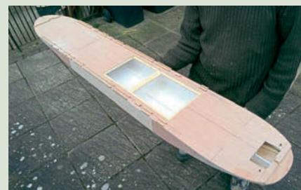
The hull was built upside down working from the deck towards the keel. It was planked with thin plywood in ½-inch wide strips and then plated with scale 8'x4' sheets.
