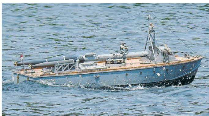
HMS Bloodhound, one-off torpedo boat with an amidships mounted single torpedo tube giving a wide arc of fire.
