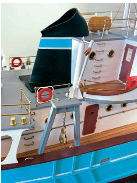
The removable section featuring the funnel behind the wheelhouse, provides access to the R/C gear and batteries within the hull.
