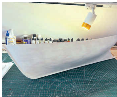
The hull prepared for filler primer.
