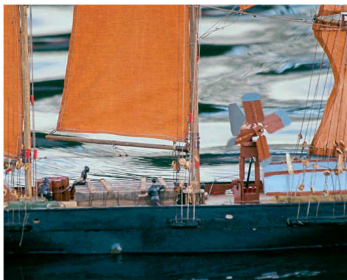
Amidships on the model, with the starboard inlet for the pump just above the waterline to the left of centre, and the windmill to the right, forward of the mainmast.
