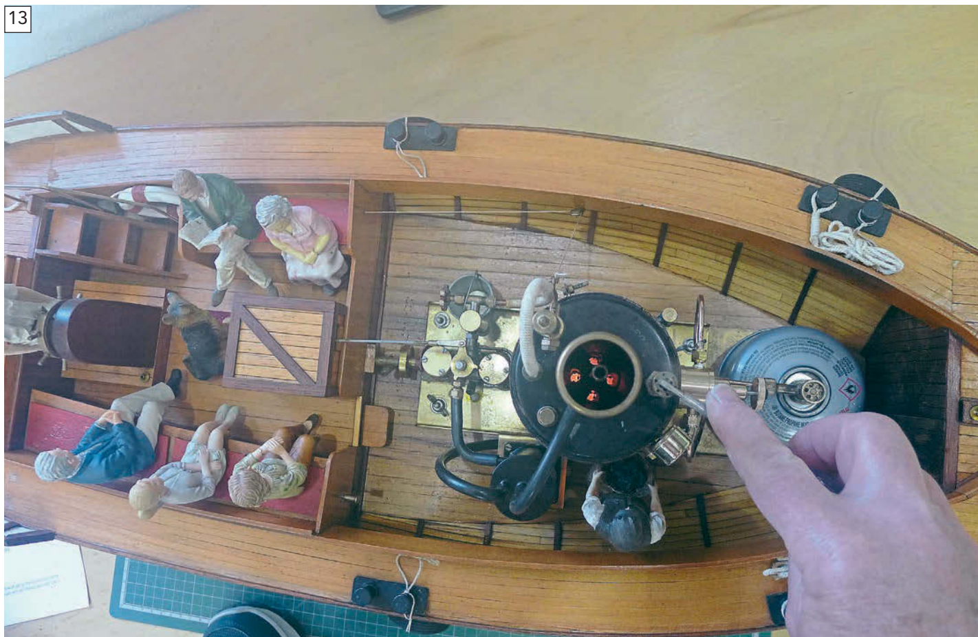
Visible down the flue is the burner turned down to a pilot flame. The screwdriver on the safety valve is there just to prevent a bit of weeping, which was misting up Richard's camera.
