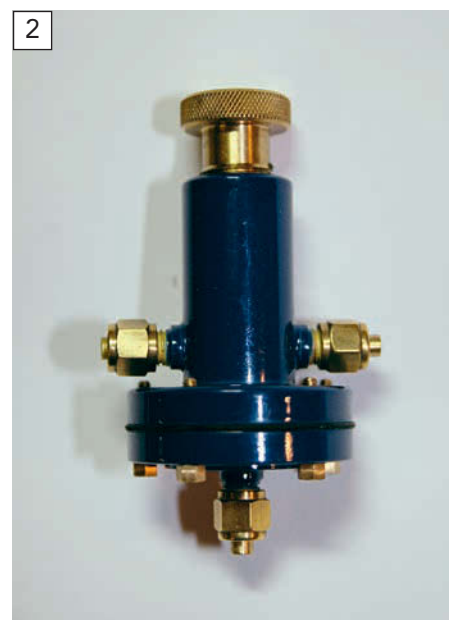
It is still possible to find a John Hemmens attenuator valve. With Hemmens no longer in business, however, you will be on your own should you need to replace its diaphragm.
