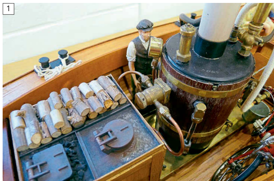
This original Forest Classics attenuator valve has seen many years' service, working well on a Cheddar 3½-inch boiler in Richard's Borkum model. Unusually mounted directly onto the boiler shell, the only challenge was that its control knob used to get quite hot.
