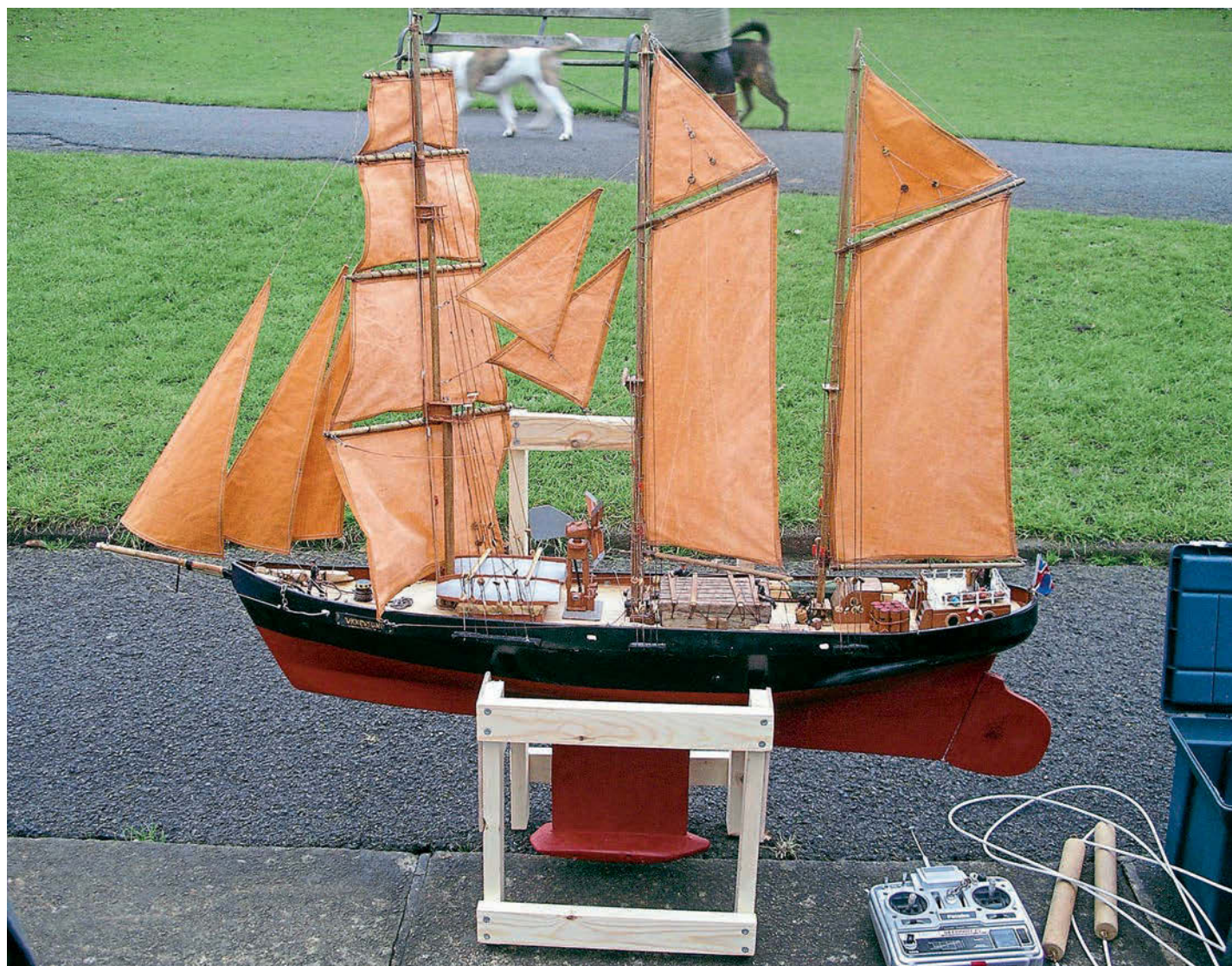
The model prior to sailing. The removable keel is attached, at the pond side, to bolts in the keel, while the vessel is supported in her stand. The launching slings are on the right. The 'inherited' hull has had its shape altered by the addition of extra wood.
