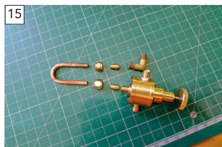
The bits laid out ready to silver solder the cones onto the ends of the pipe. For the pipe to work as a siphon, the valve should be mounted higher than the boiler elbow, but that would have required the other pipes to be remade as well. This is a task Richard will tackle in the future.
