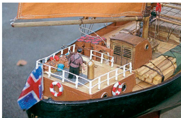
The helmsman at the stern. Note the deck cargo of timber, long a feature of these vessels. It was not unusual for the entire deck to be covered in cut timber, with the top of the pile used as the 'deck'.
