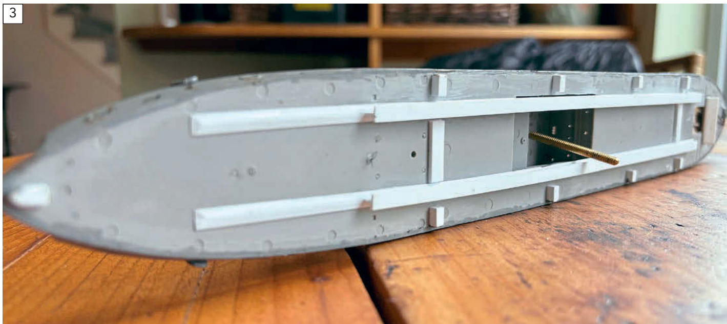
The three deck pieces joined and reinforced with the Plastrut I-beams to make a single, fully removable deck. The attaching brass screw bolt is also shown poking down from the funnel base.
