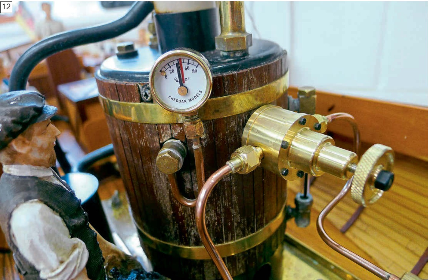
On opening the steam to the engine and running the engine a few times, Richard saw very little variation in boiler pressure. When the engine was stopped, the pressure settled at the set point and stayed there without the safety valve lifting.
