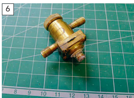
Being held together by only four screws put inconsistent pressure on the diaphragm, which can be seen by the fact that it squeezed out at the sides.
