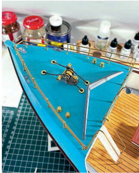
Nordkap's bow section with railings, anchor winch and breakwater
