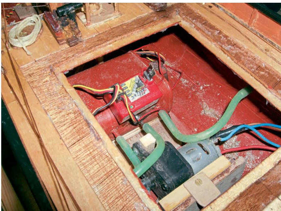
The unusual heart of this model, the tank, which takes in water as the model is sailing so that the electric pump can pump it out again as if from the windmill pump's outlet. The inlet hoses can be seen leading from the ship's sides, with the outlet hose en route to the pump in the centre of the picture.
