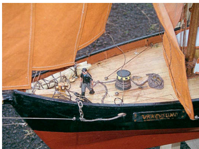
The fo'c'sle head, with mooring line and capstan.
