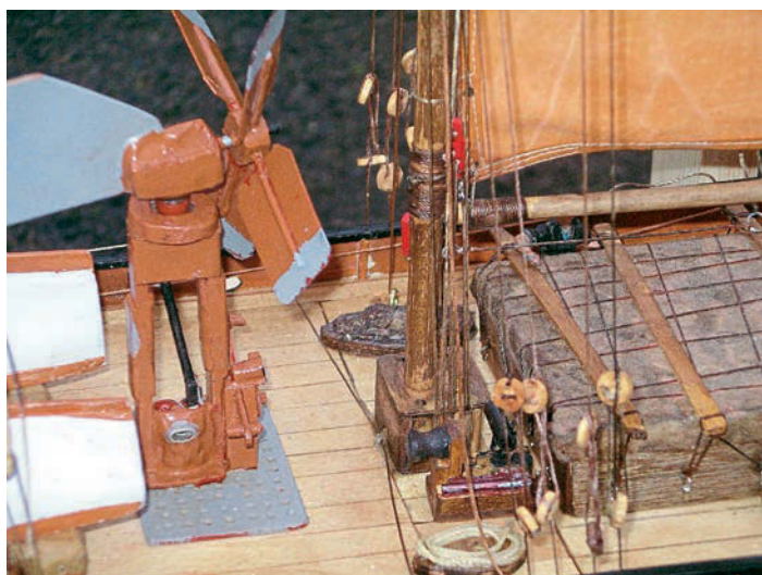
The windmill pump. On the model, there is a 'wind vane' to turn the pump to face the wind. Aboard the real ship, it was turned manually, and the sails were like those of a land windmill, with canvas that could be furled when necessary.
