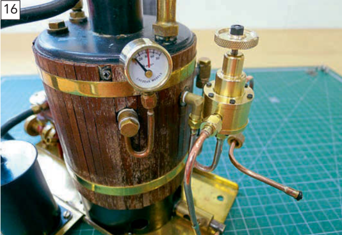
A much better arrangement both for isolating the valve from the boiler and accessing it when the boat is in operation. The control knob and the valve should remain a lot cooler.
