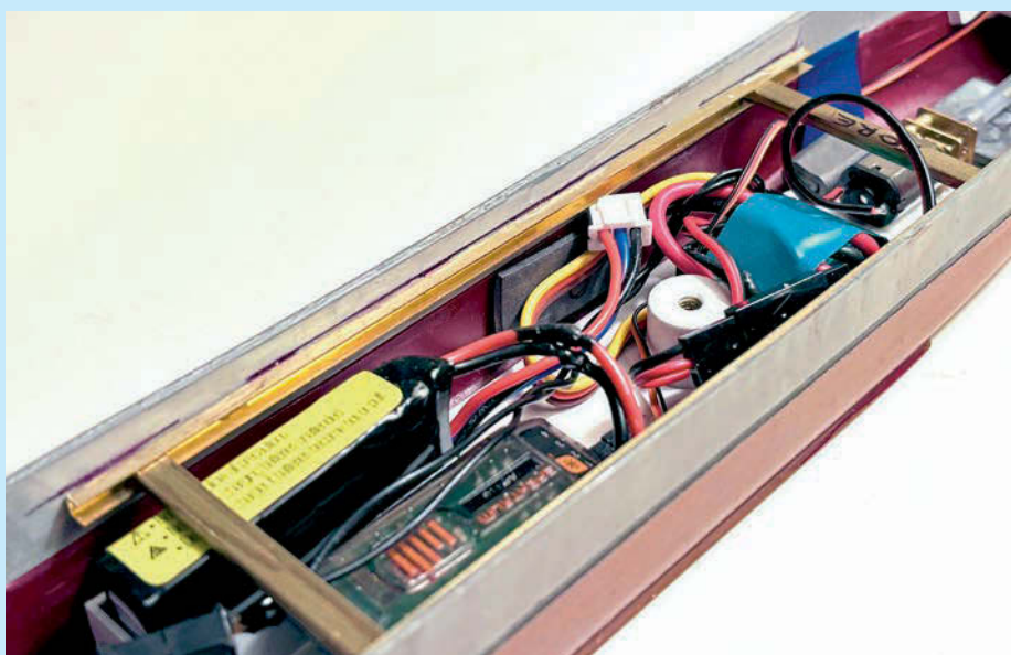
The square section brass channel and easily removable (slide out) rectangular section brass cross-braces to space out the hull side.
