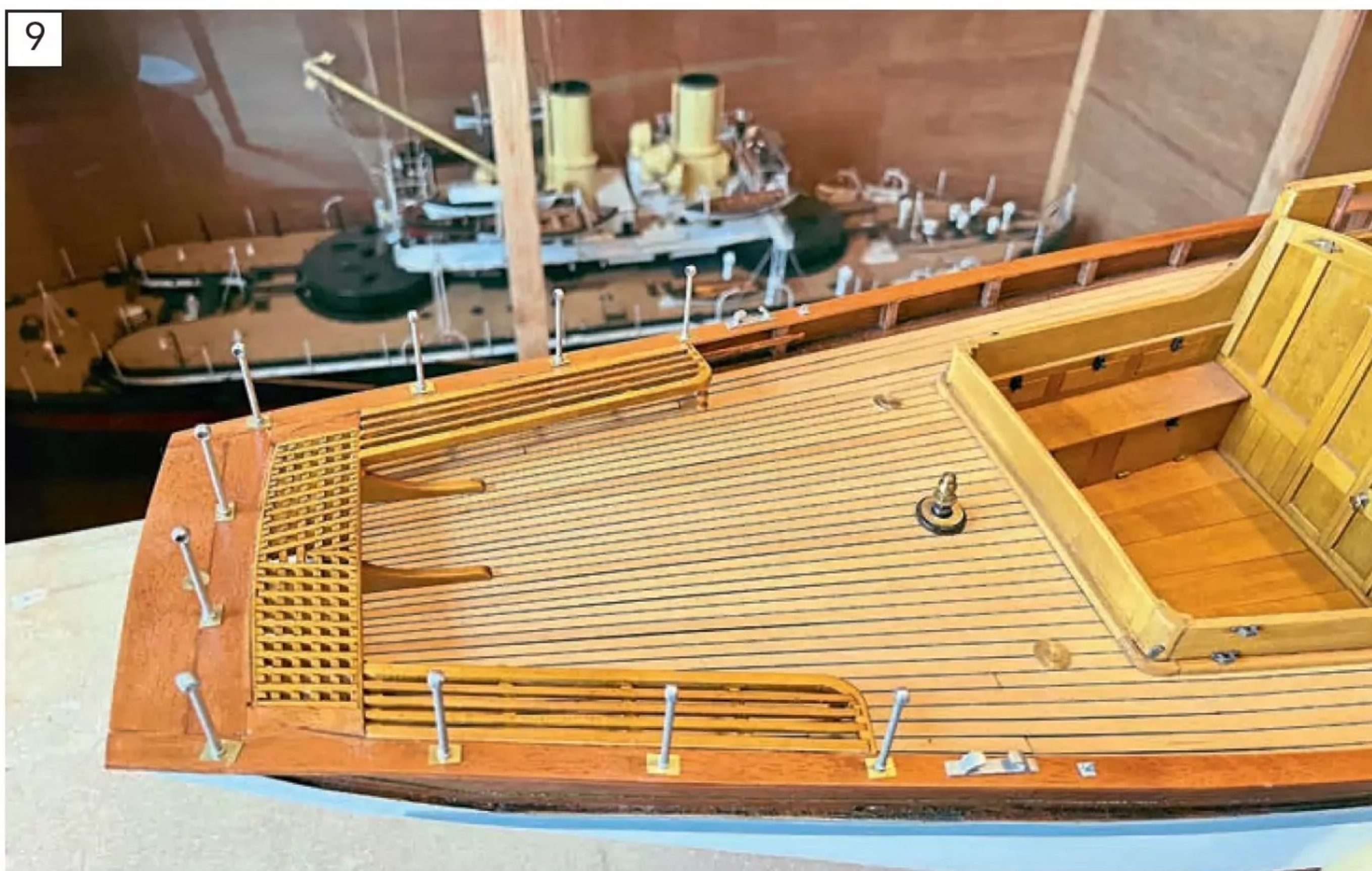
The finalised rear seat arrangements, stanchions and tapered planking.
