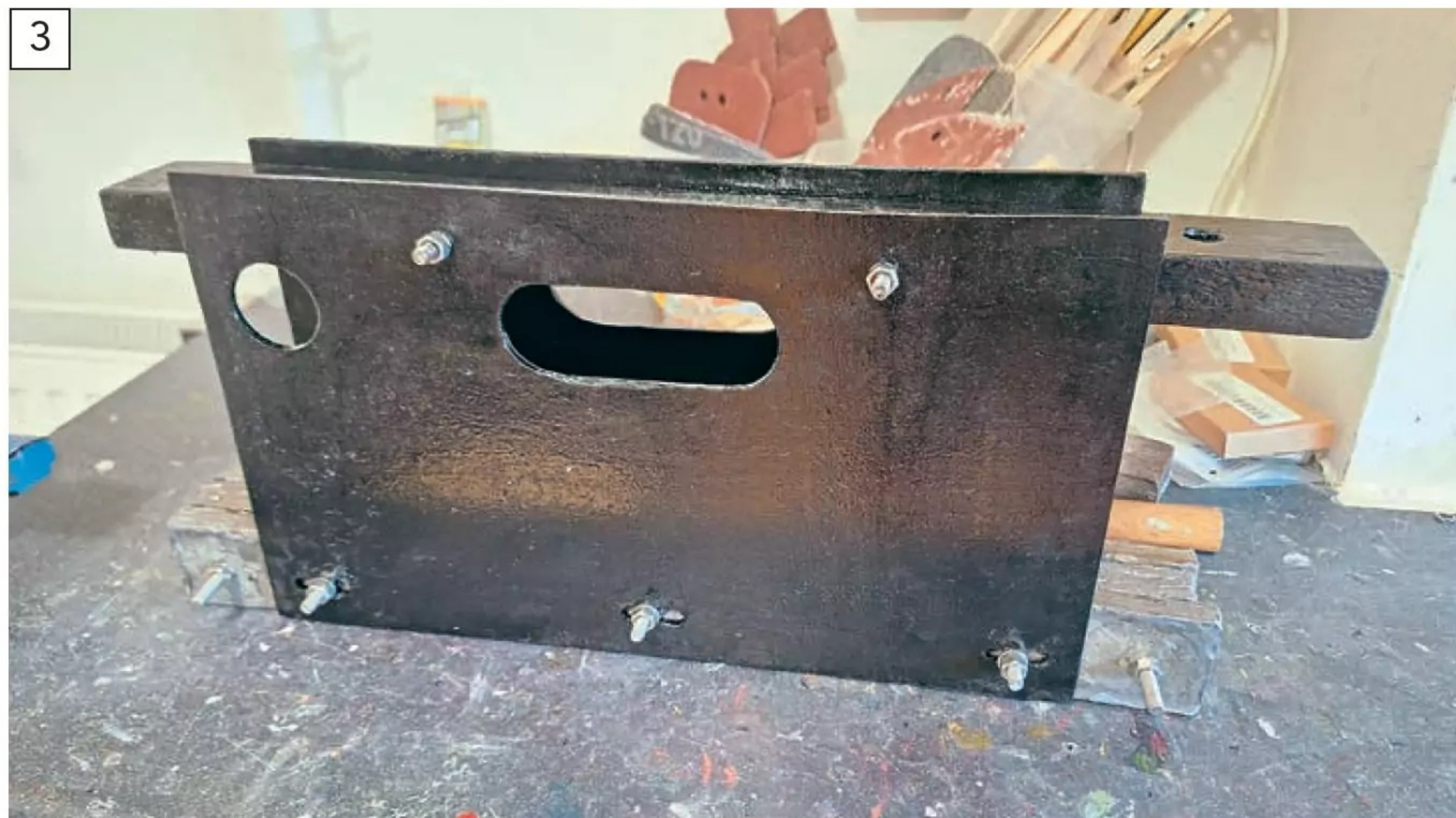
The completed detachable sailing keel with cast lead ballast.
