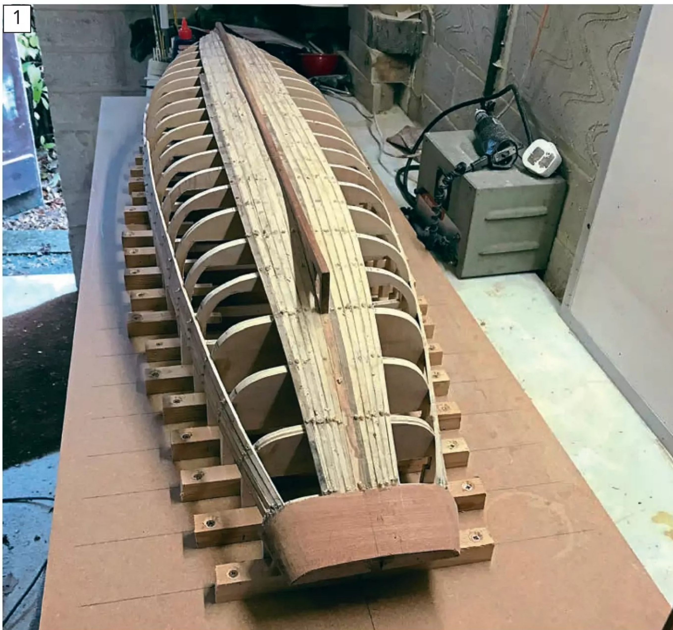
Work on the wherry yacht's planking started and with the wooden block used to form the end of the counter stern fitted.
