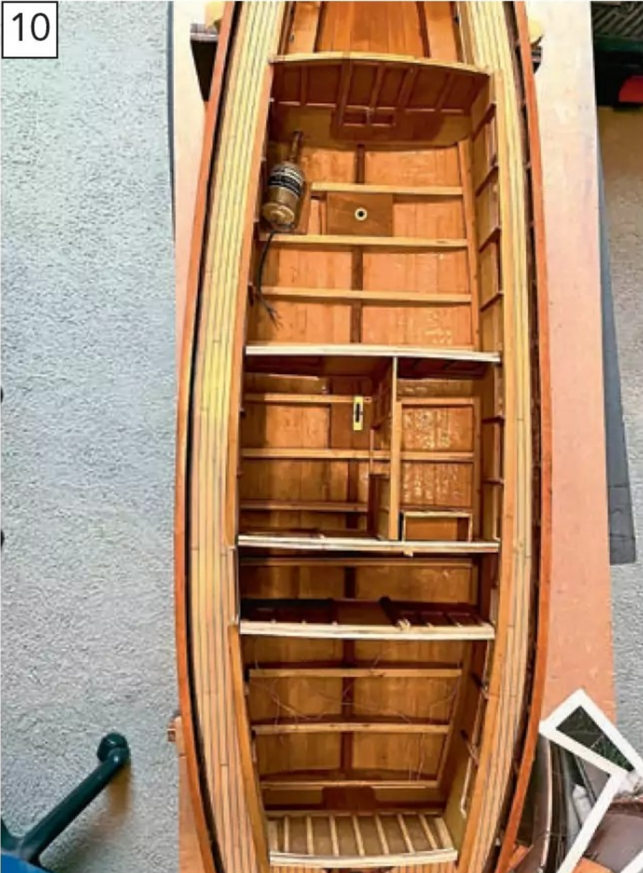
The cabin sides in place, together with the bulkheads.
