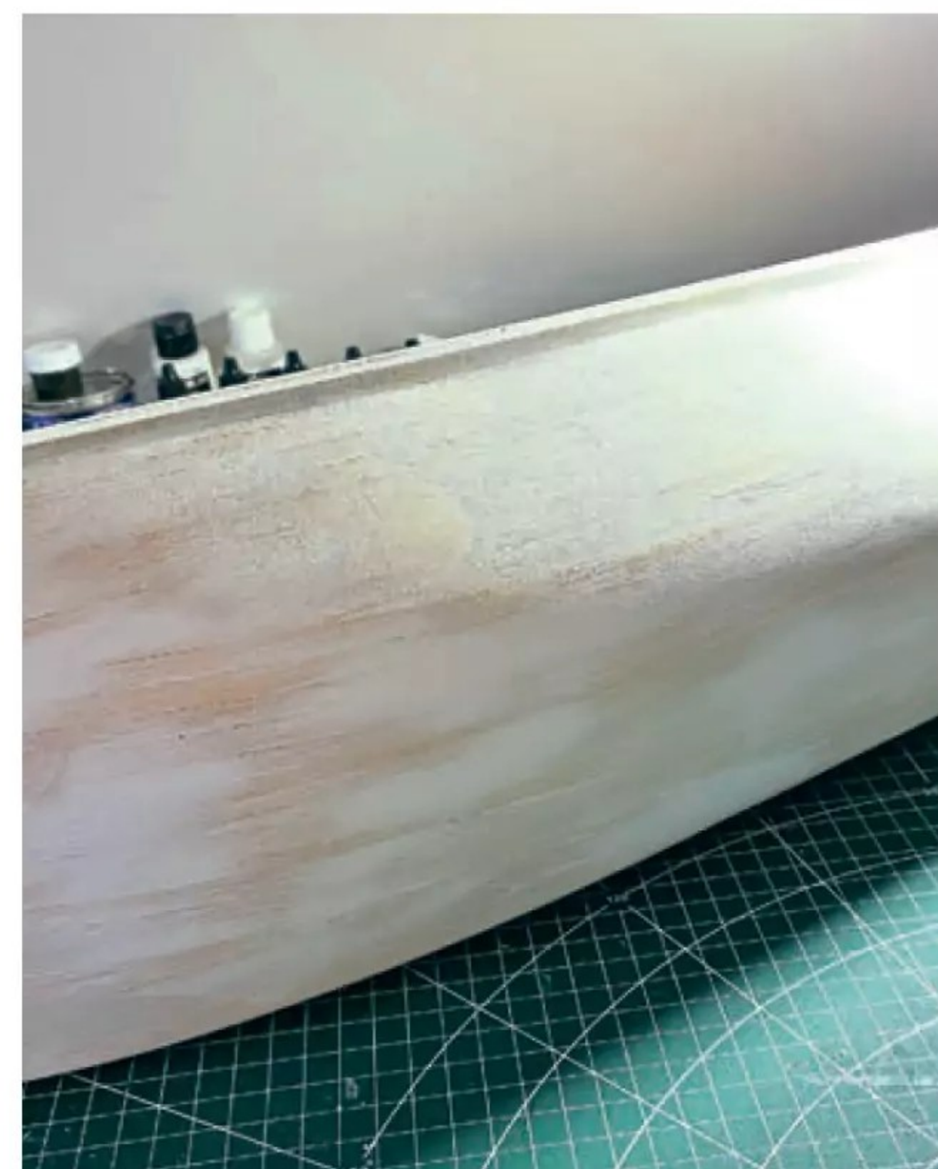
First layers of putty, with some large and medium holes filled.
