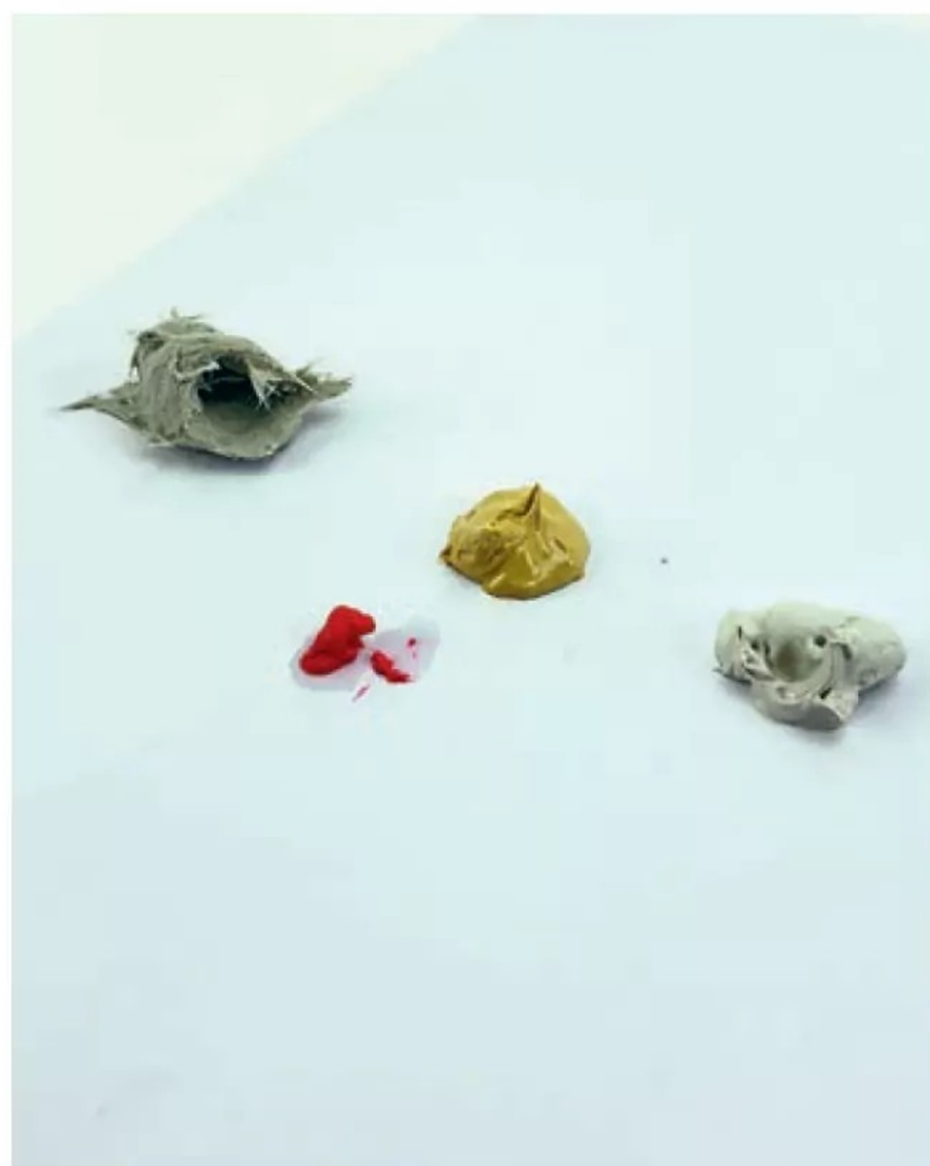
Three different automotive putties (from left: fiberglass, universal and finish), along with the pink hardener.
