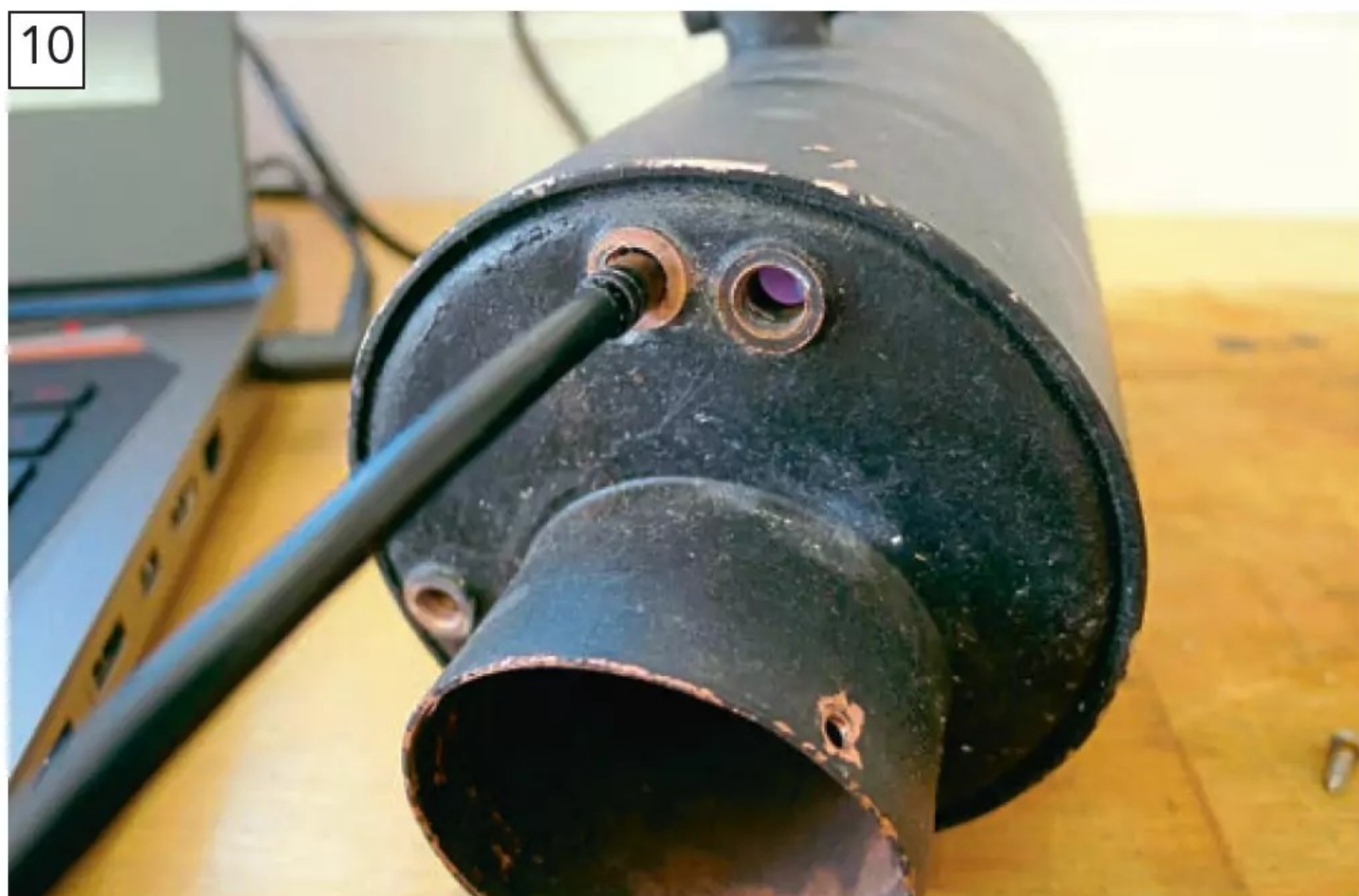
A cheap and cheerful 4mm head camera is an incredibly useful device for looking at the insides of a boiler and can actually be slid through a few of the brass boiler bushes.
