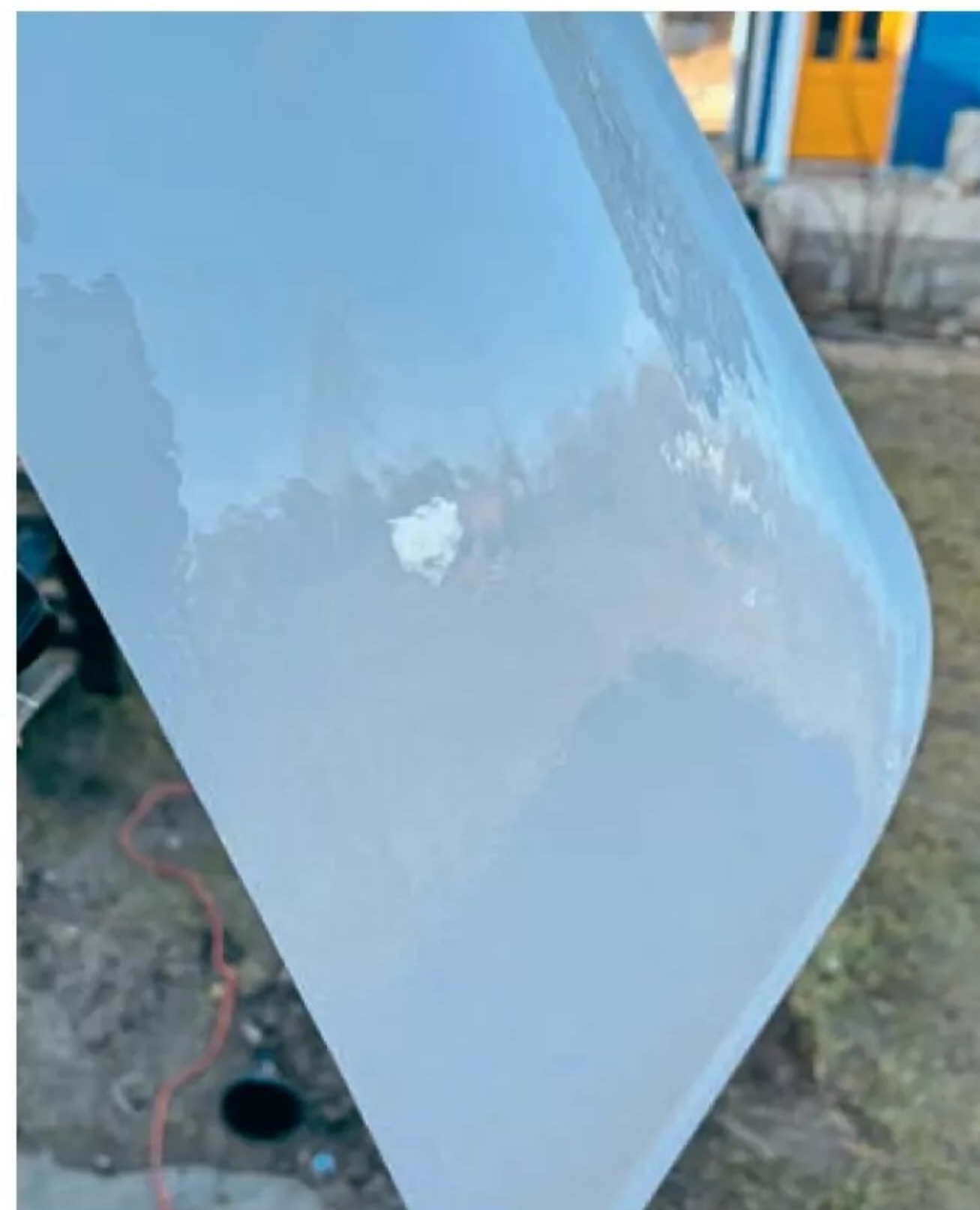
The first thick, still wet, layer of filling primer paint. Once dry, this will be rubbed down with wet and dry sandpaper before the second layer is applied.
