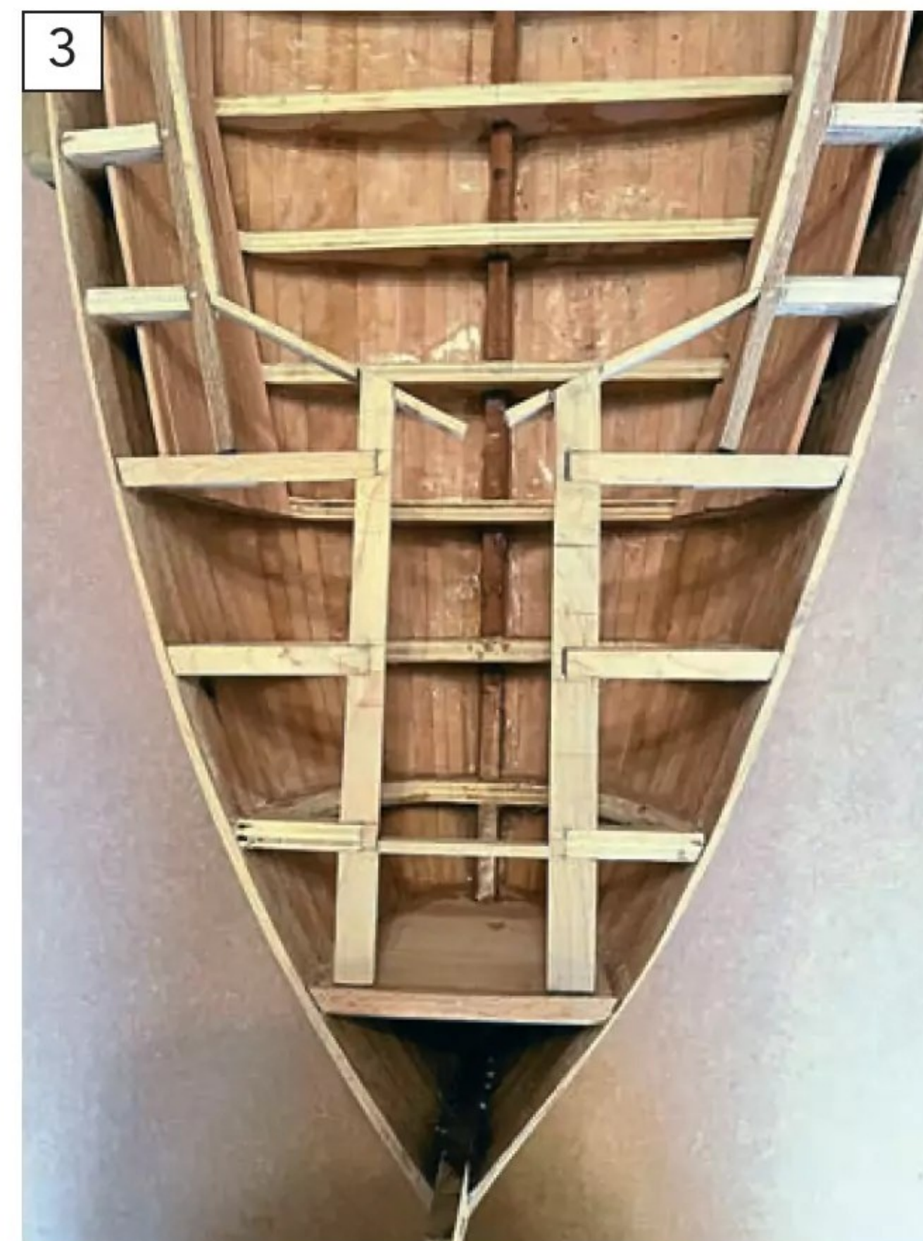
The inside of the hull fibreglassed, with deck beams installed and with the interior now also planked.
