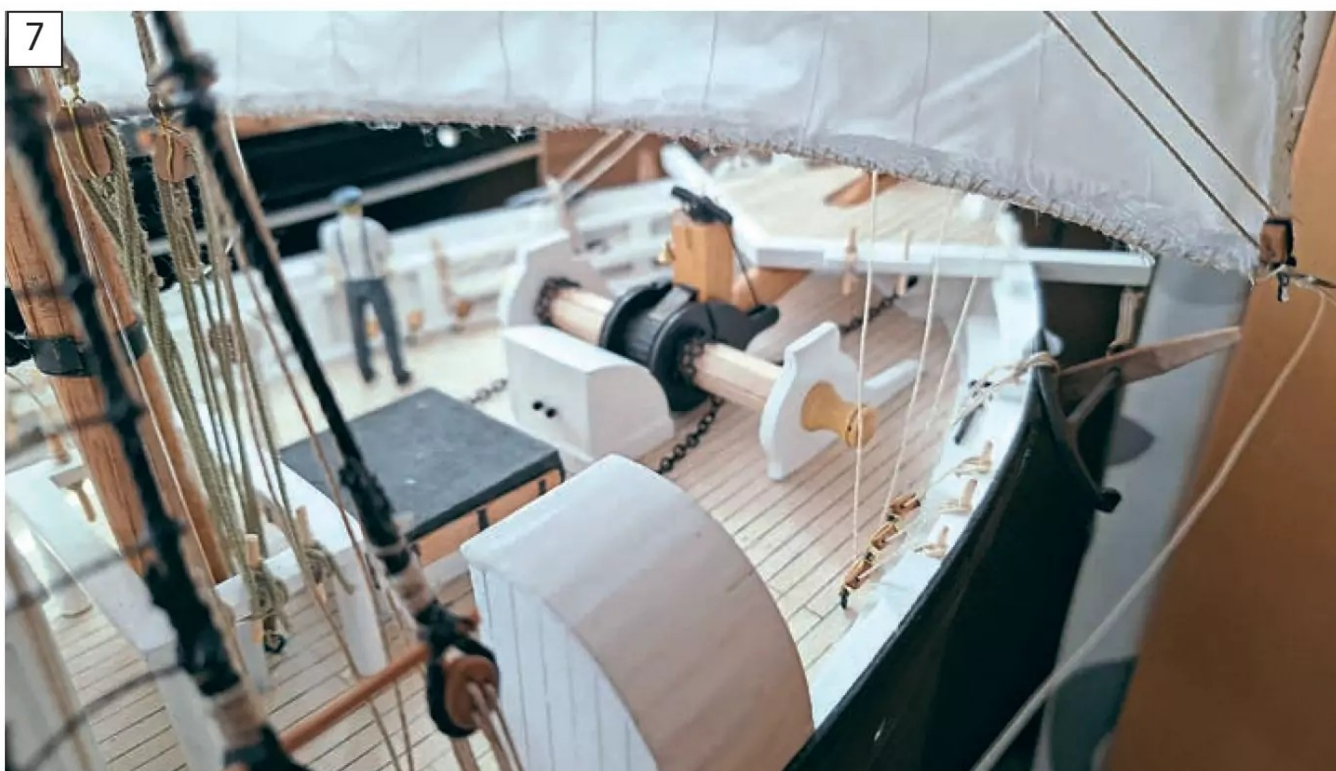
The foredeck, showing the windlass with its 3D-printed pawl housings and ratchet wheels.
