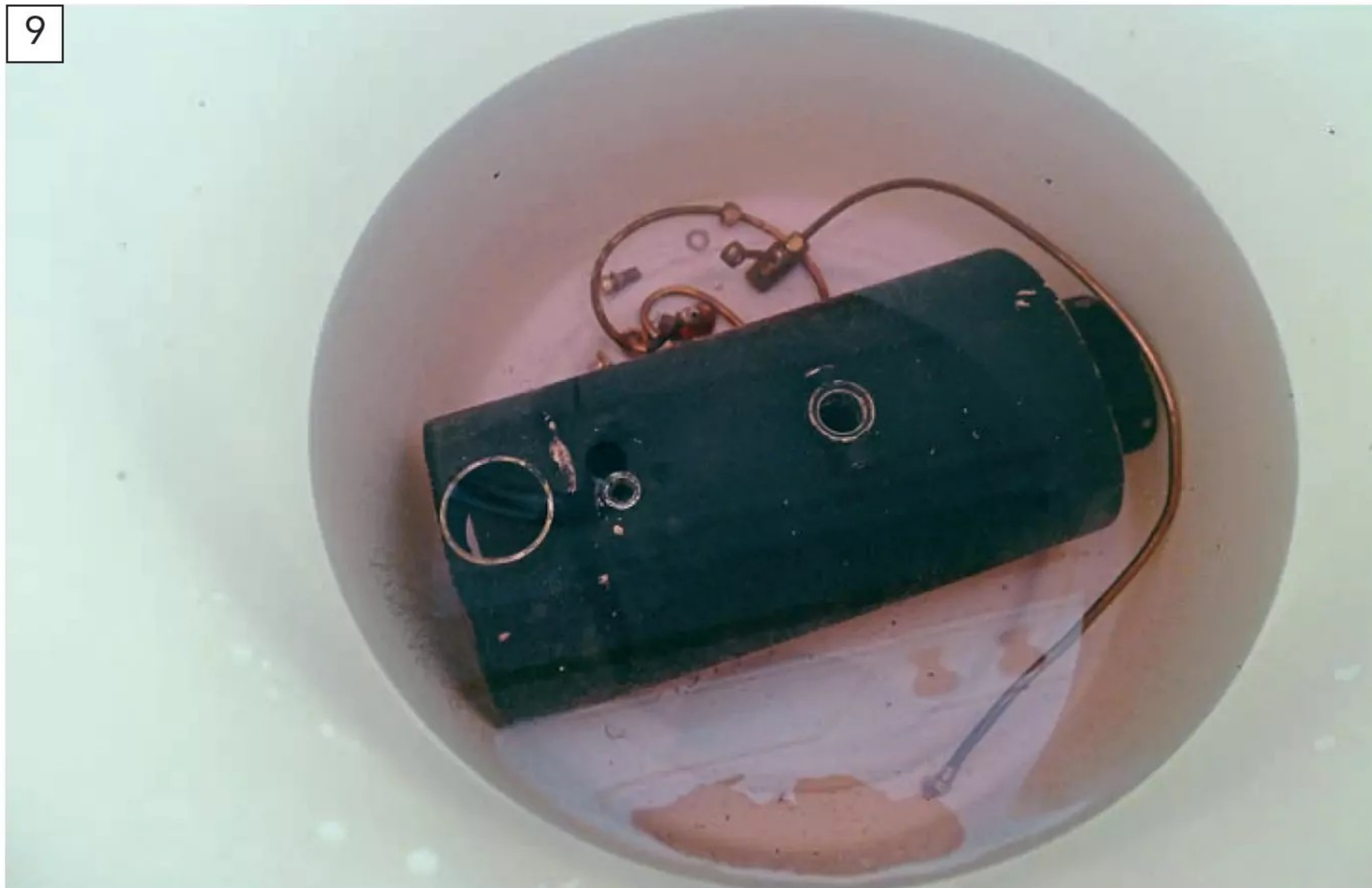
Citric acid and hot water will usually prove effective for a general clean up and limescale removal. Verdi gris inside a boiler might require a more aggressive cleaner.
