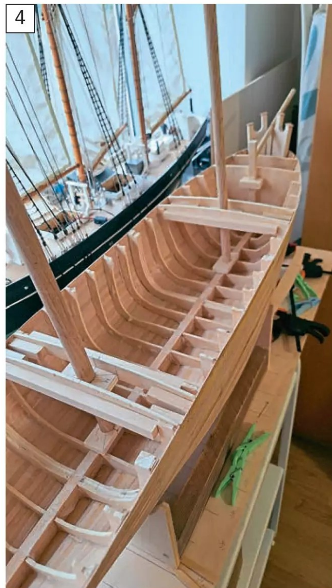
The hull, well on its way to completion, showing the mast steps and partners, with the unfinished masts resting in place.
