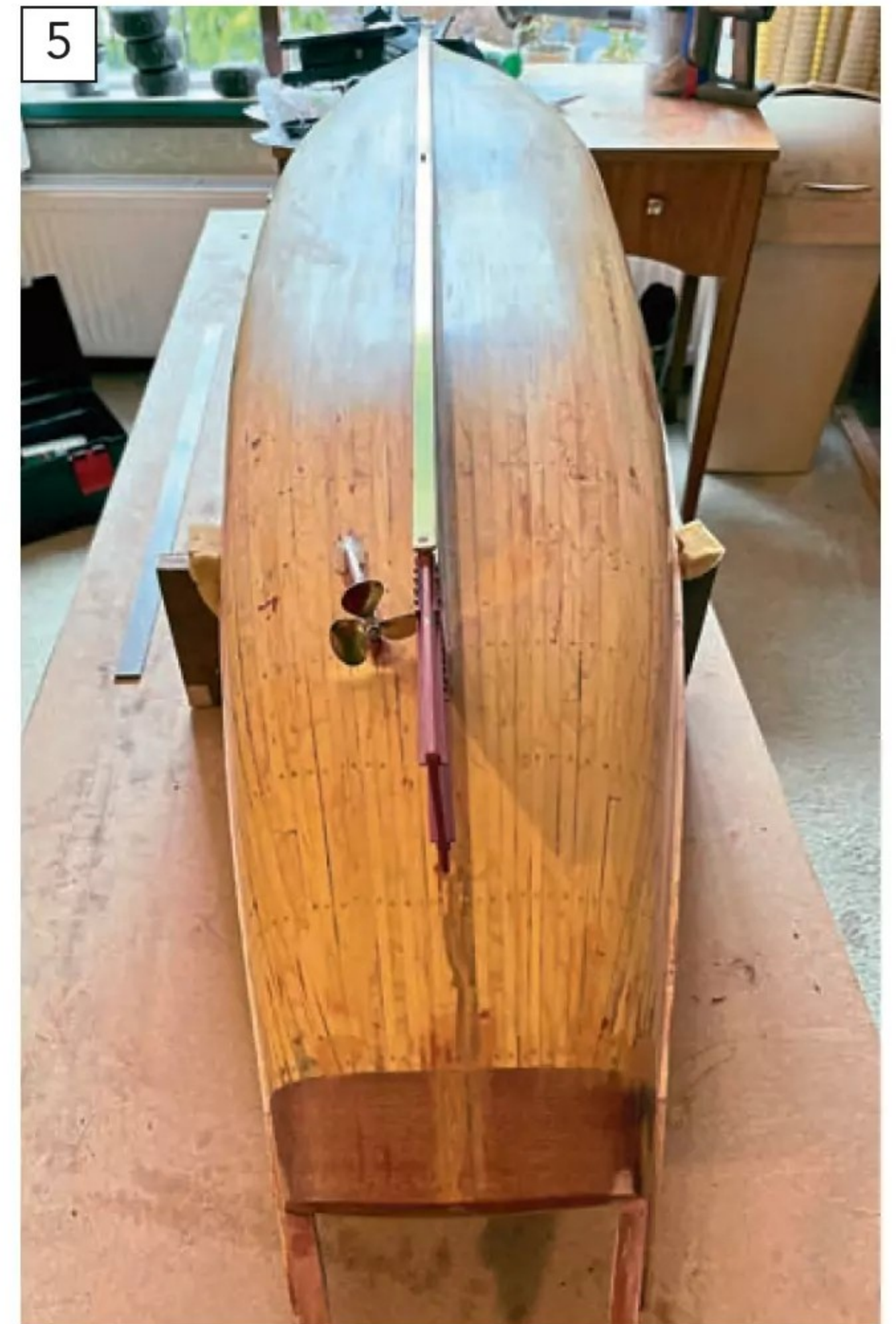
The offset propellor shaft, brass keel and false keel slot.
