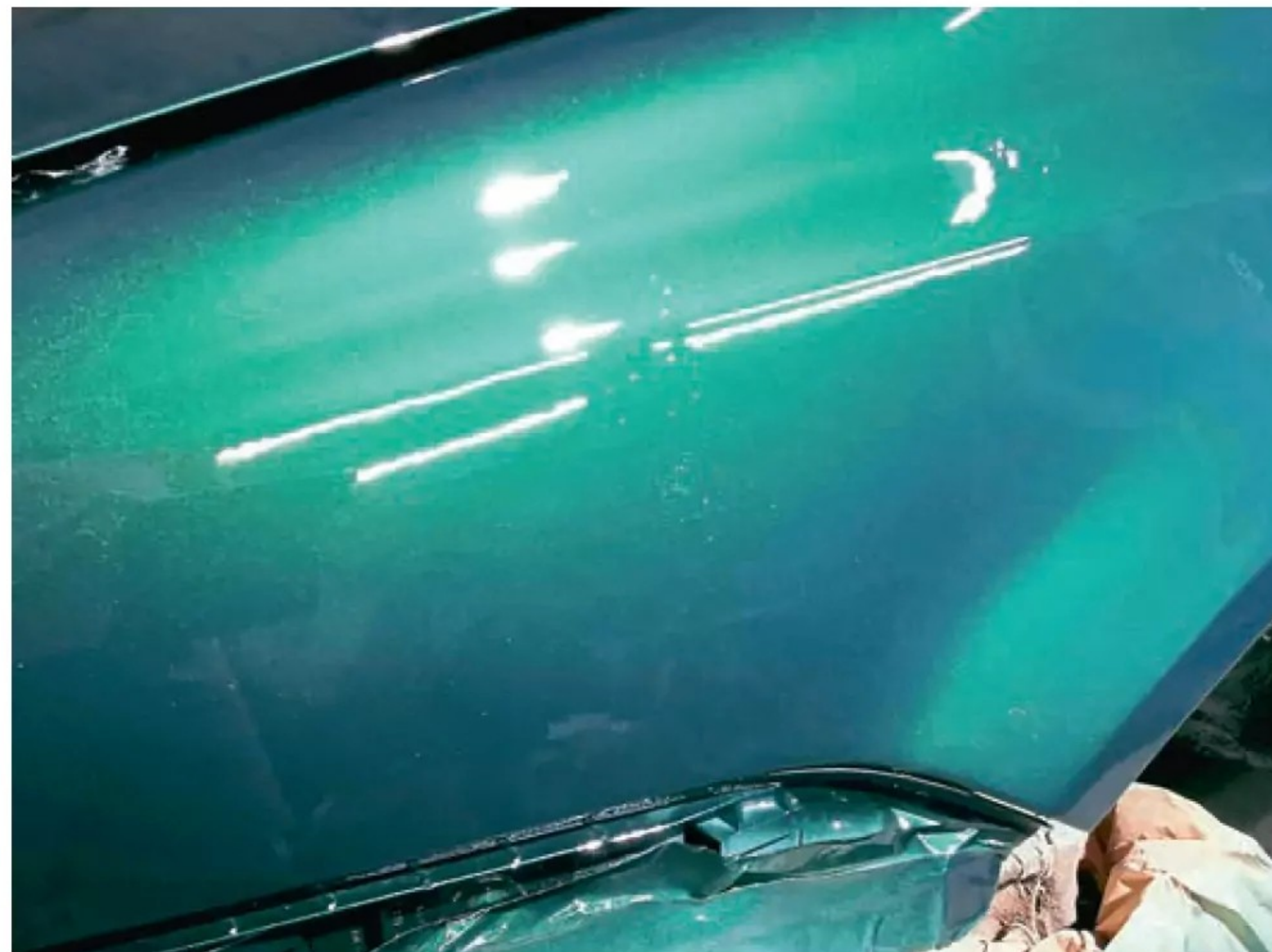
The pearlescent paint after being covered with clear coat. Note the visible difference in colour and reflection compared to the paint directly after application.
