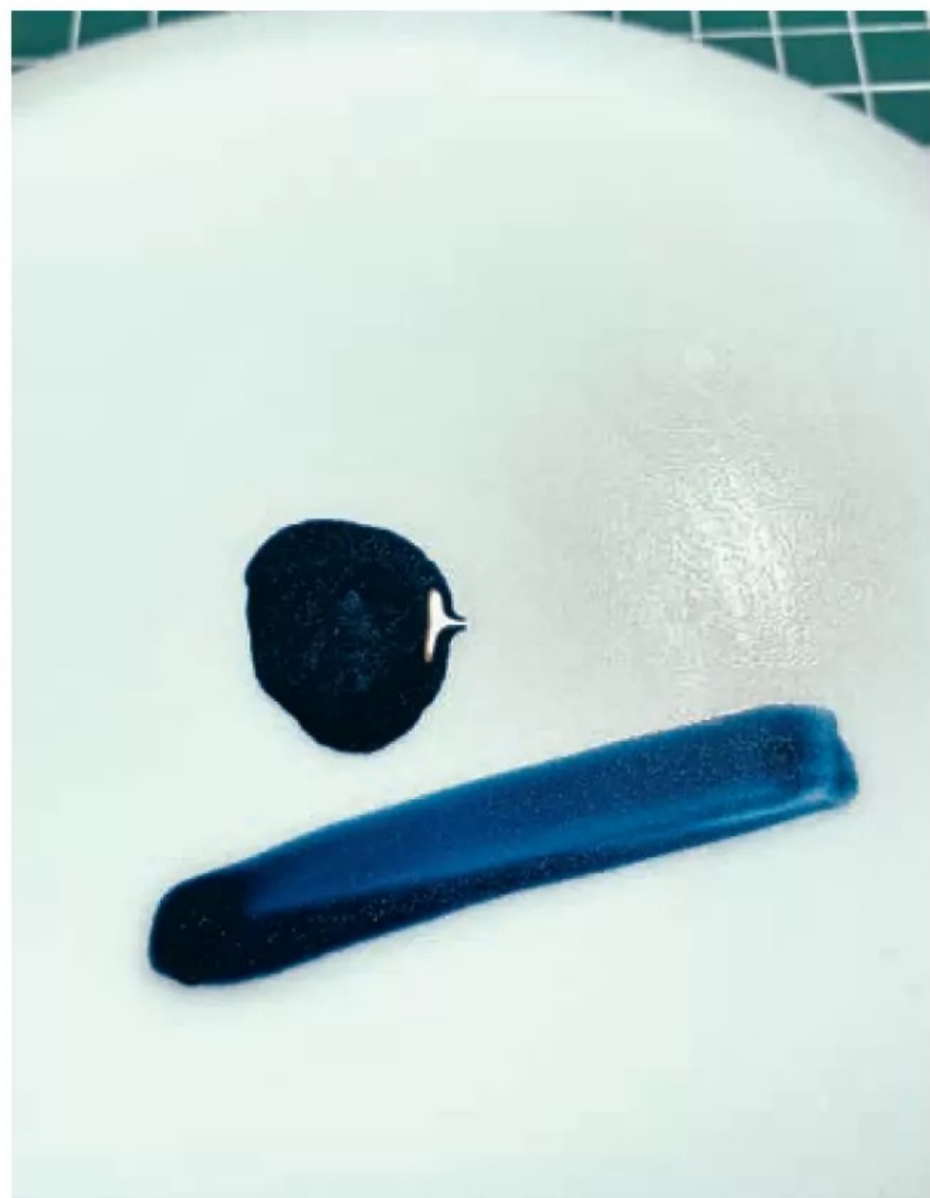
Metallic paint – depth of colour will be affected by the primer chosen as a base and the number of coats of paint applied.
