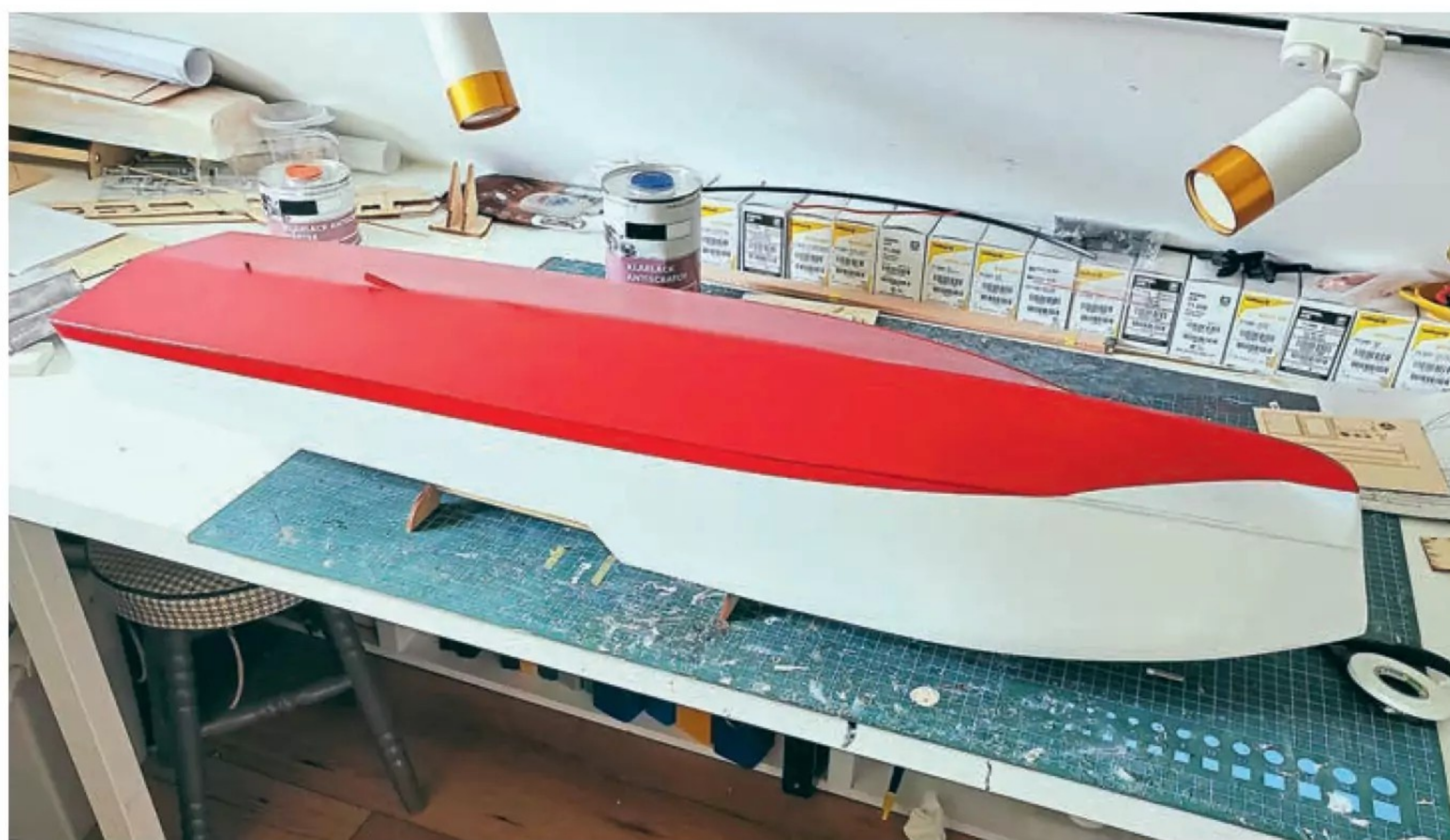
A painted hull ready to receive its first clear coat.
