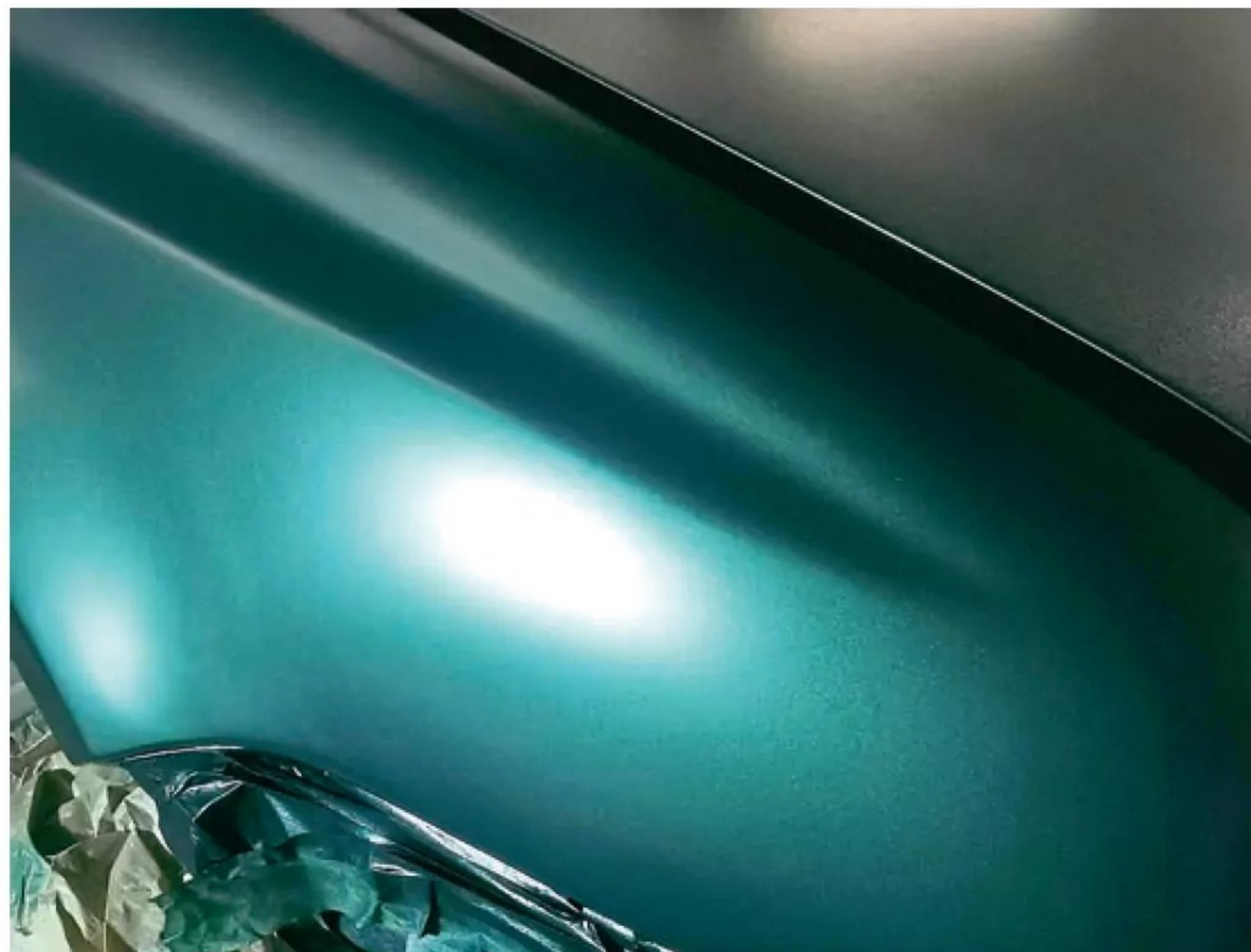
Automotive pearlescent paint right after application and initial flash-off.
