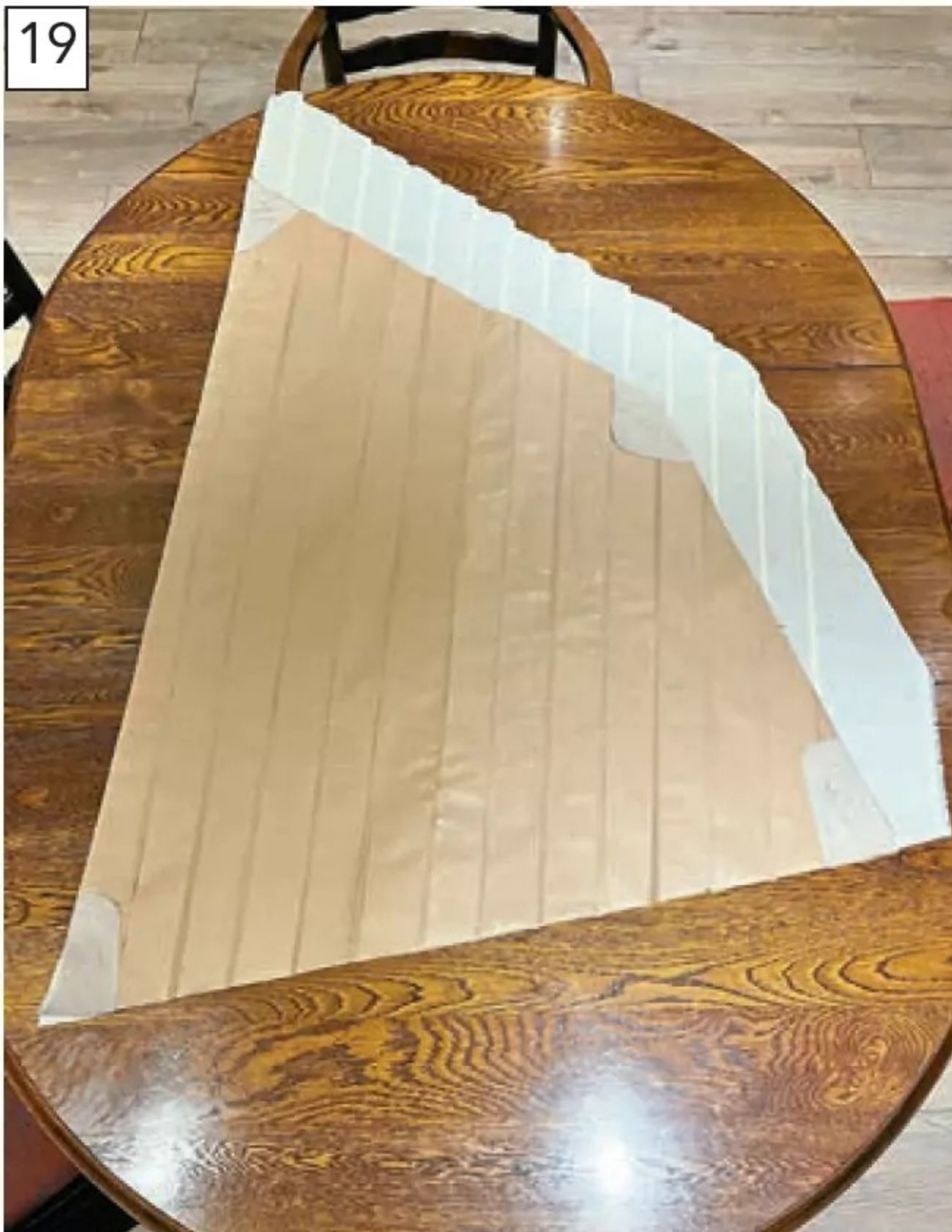
The paper template for John's sail laid on the sail cloth to which panels have already been pre-sewn.
