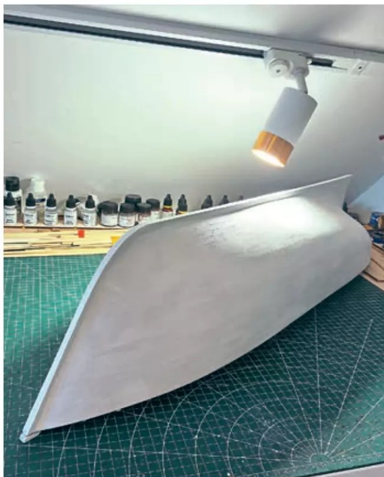
The less than perfectly prepped hull seen here will be used to demonstrate how it's possible to hide a multitude of sins by using thick layers of this filling primer.
