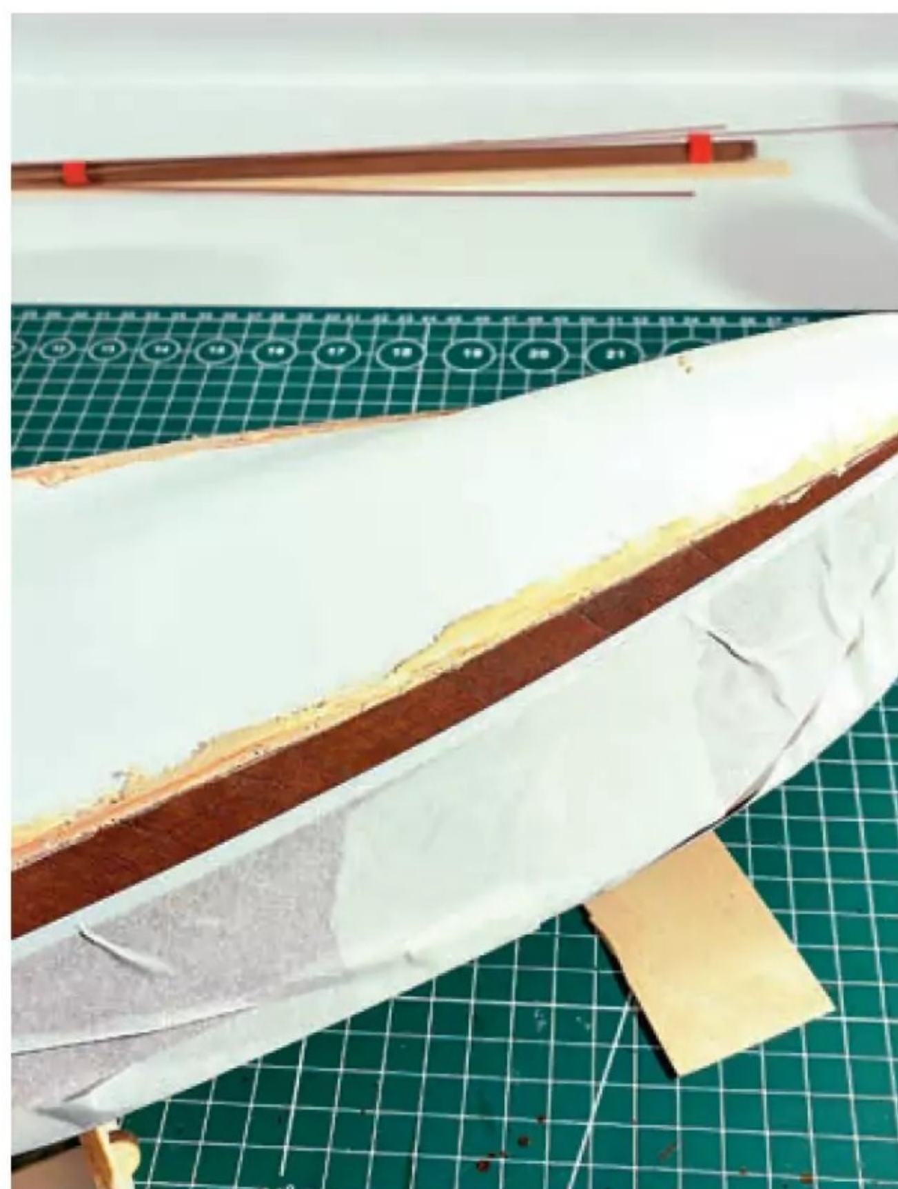
Filling small defects with universal putty.
