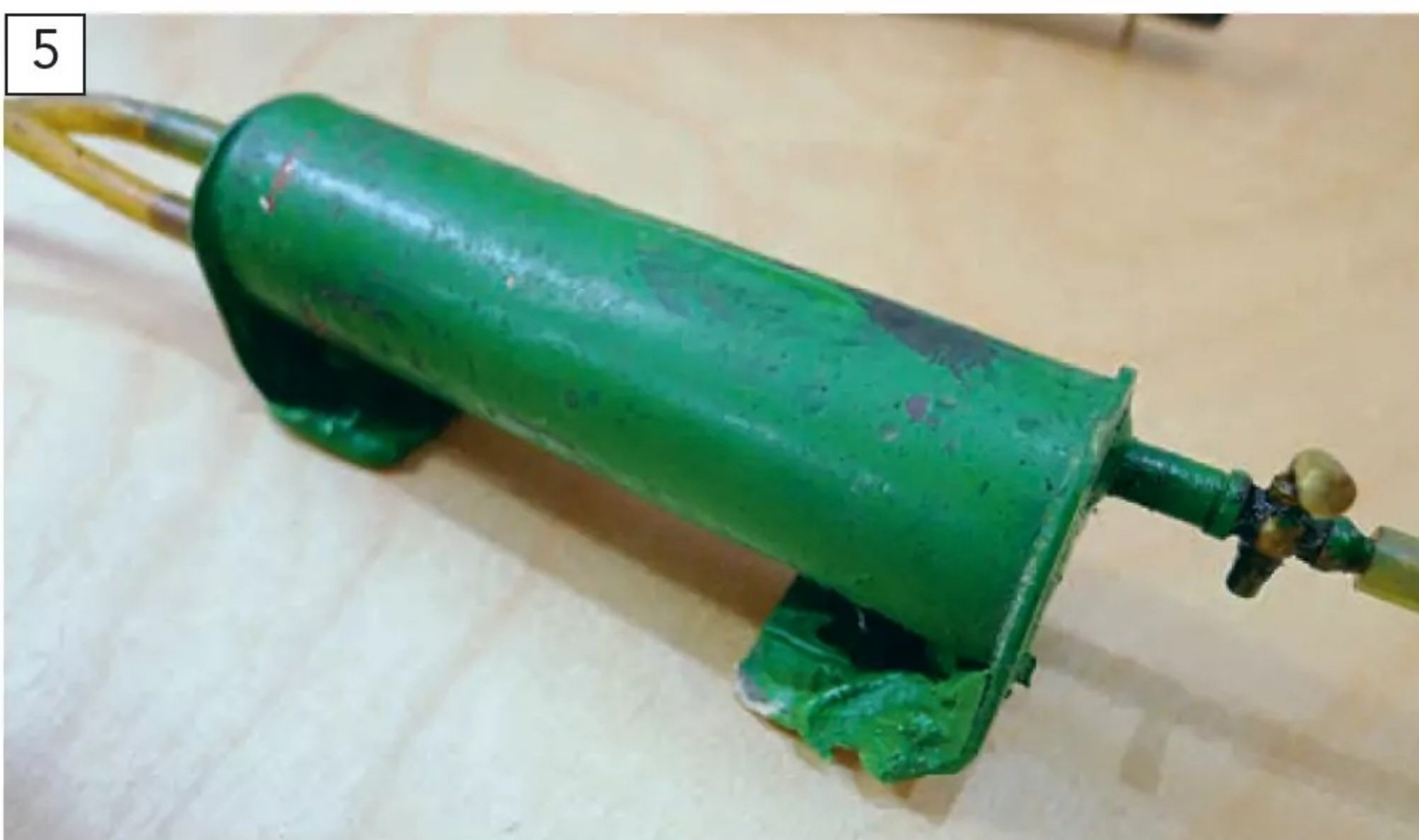
Separator tanks work best when they are vertical and narrow rather than horizontal. The contents will rarely separate effectively in a tank like this, so the contents have to all be dealt with as waste oil.
