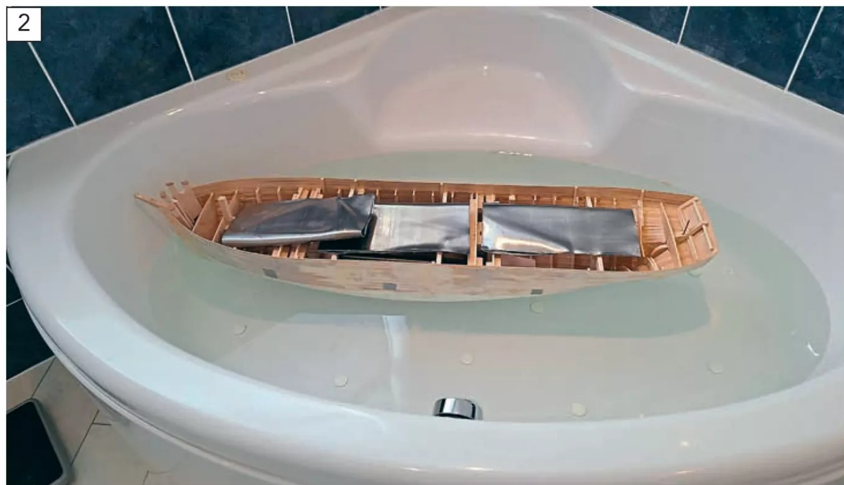
Determining the ballast required in the bath.
