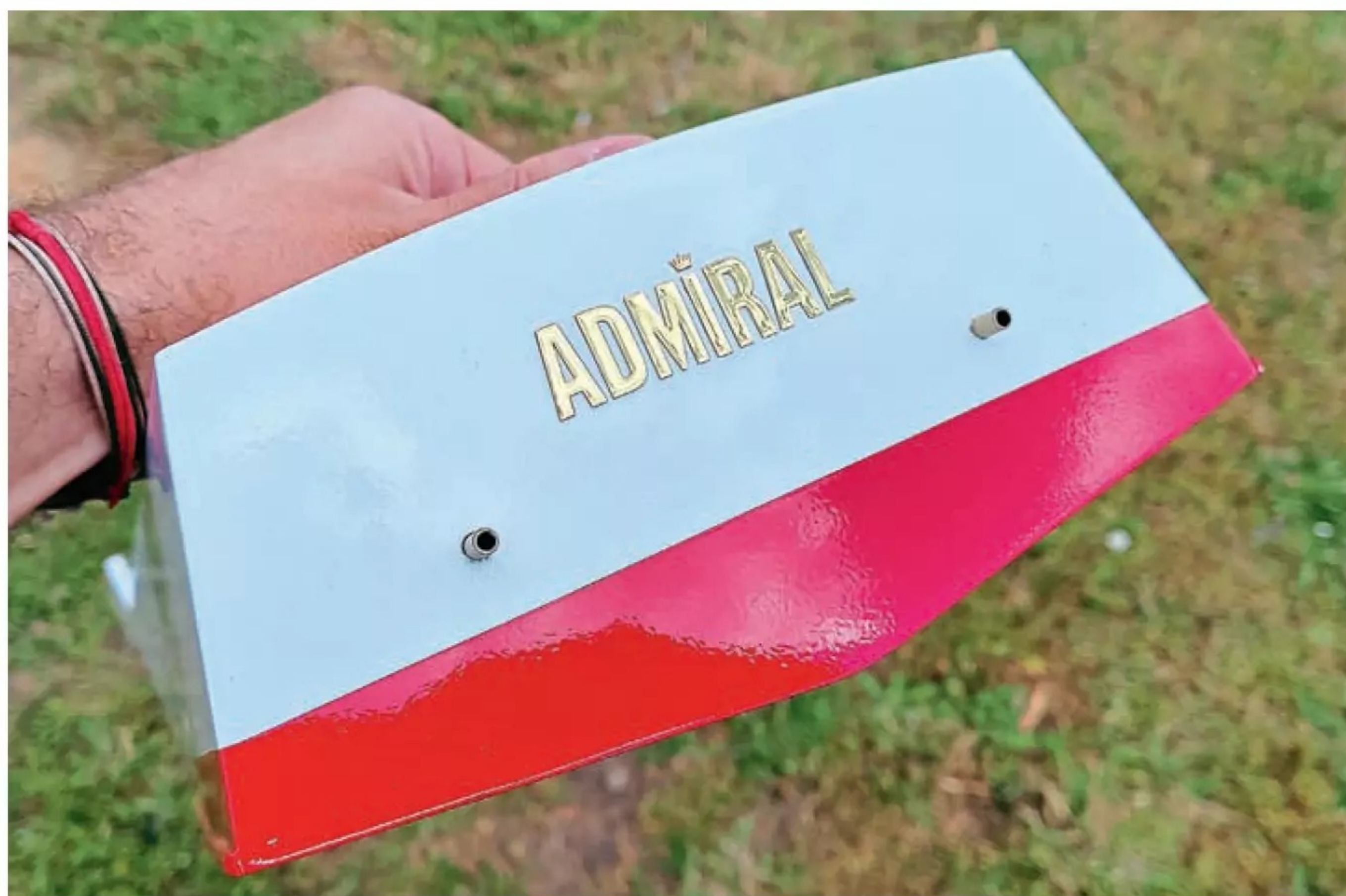
The final clear coat layer. Note the visible orange-peel effect.
