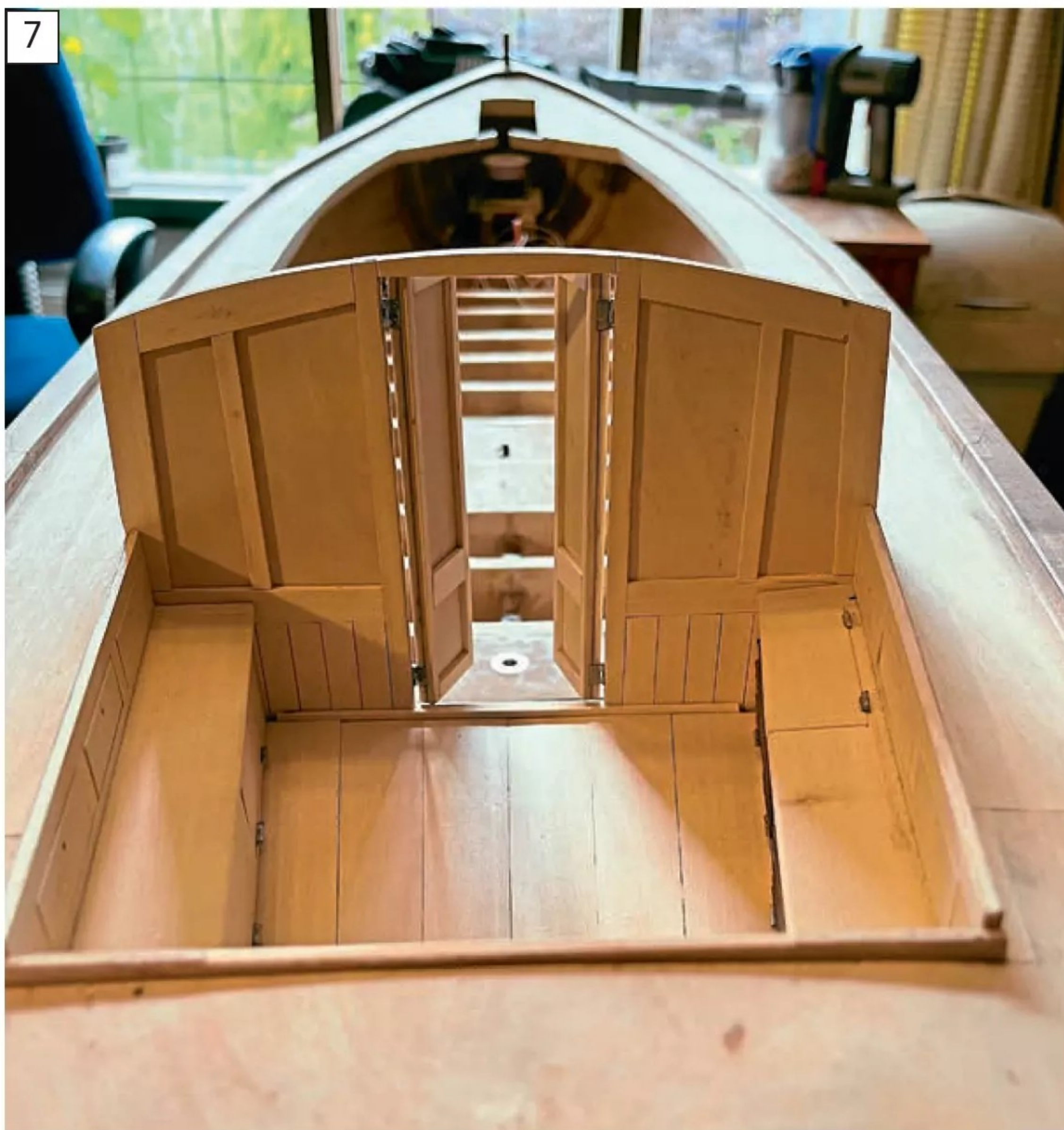
The steering position showing the initial bulkhead plus seats after wood staining.
