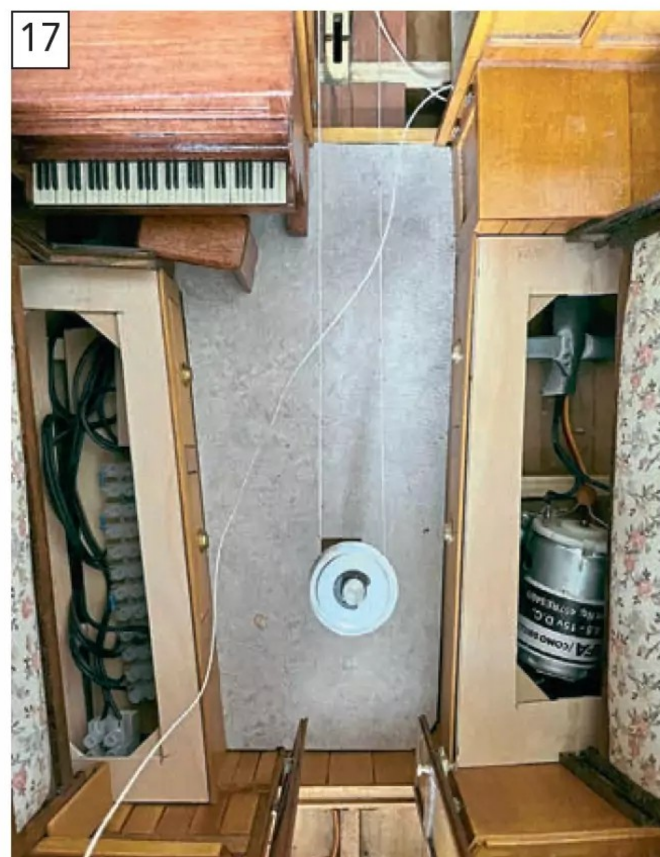
The aft cabin, with the concealed motor and lighting electrics revealed.
