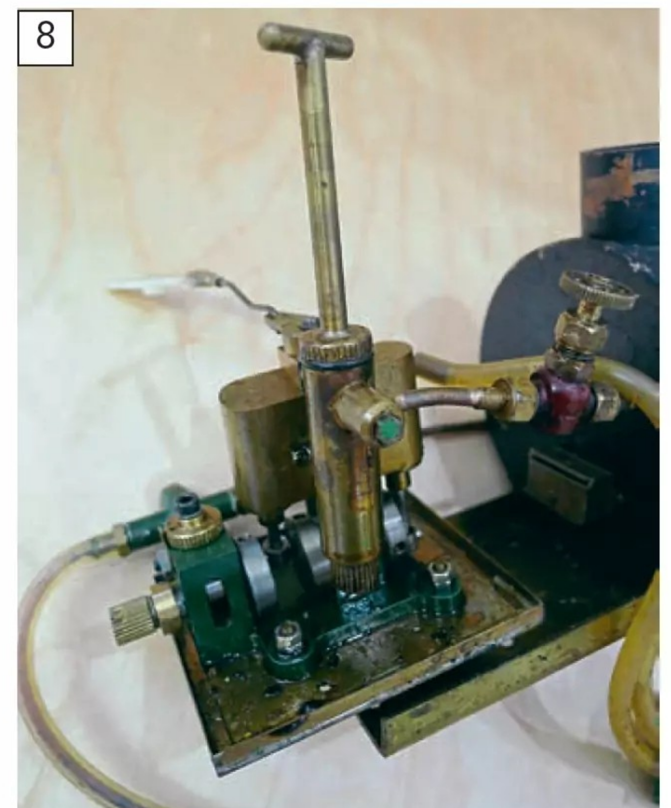
Richard also likes the filling cap on the engine mounted lubricator with the extended spindle to make removing the cap easy.
