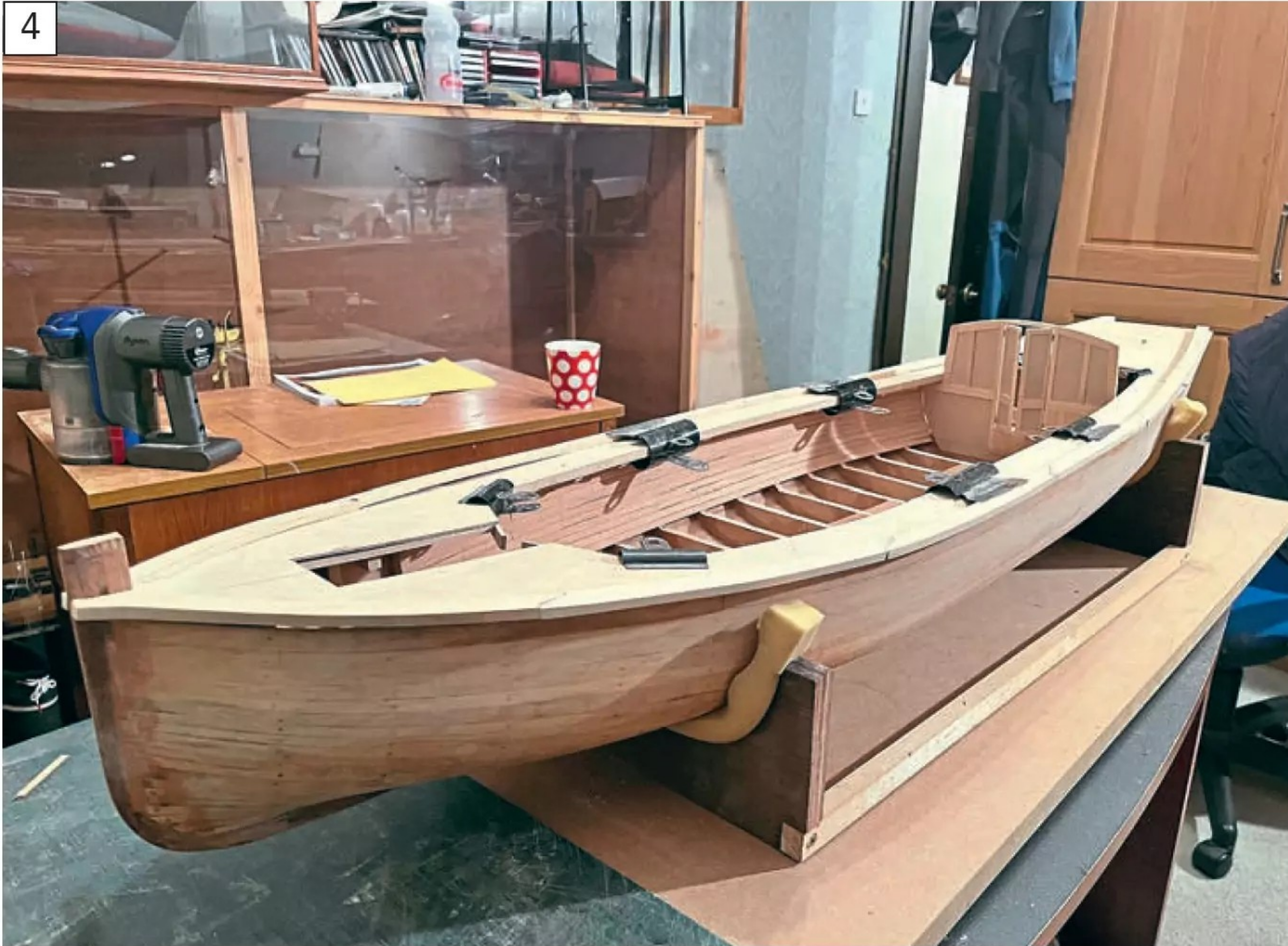
The false deck and the initial rear bulkhead.
