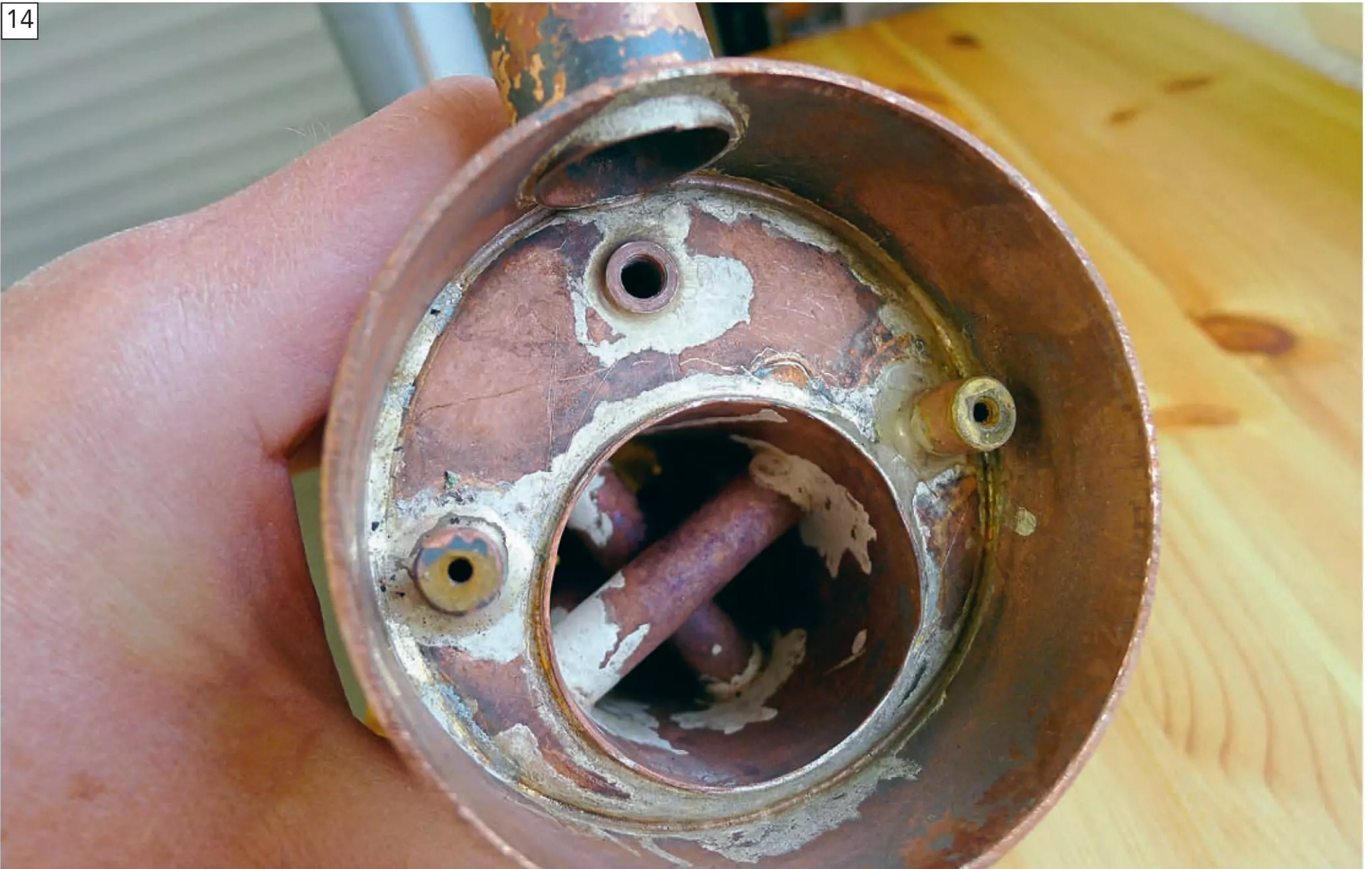
When Richard received the boiler back from the specialist repairers it was fitted with two new threaded bushes to replace the originals, enabling the end plate to be fitted again in exactly the original manner.
