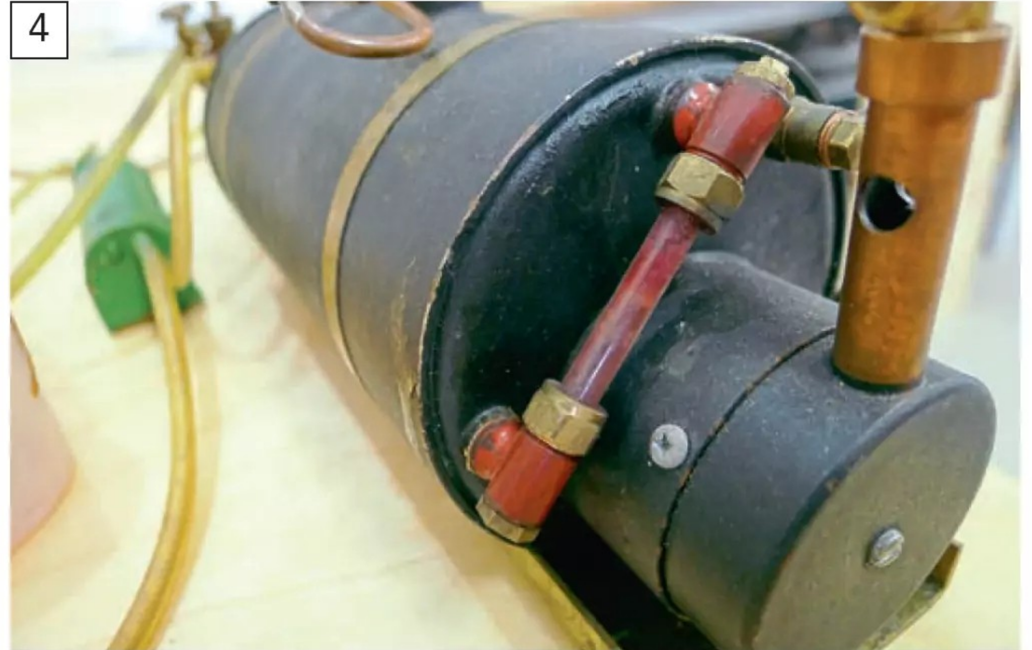
One of the biggest concerns was the red dye in the sight glass. Using a dye to help see the water level isn't unheard of, but it always ends up with a dirty sight glass that you can't see anything in. Then it's a lengthy cleaning process.
