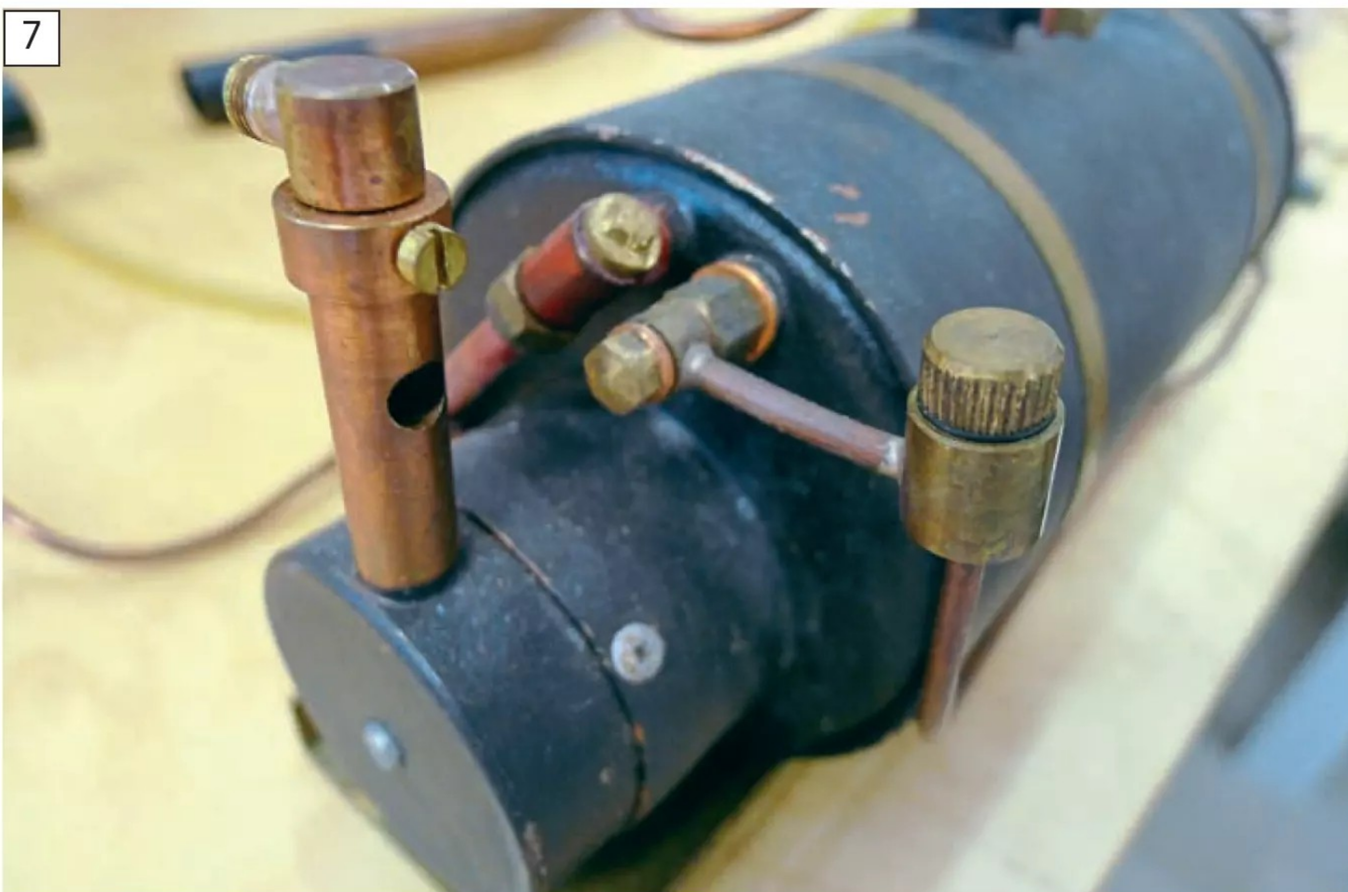
Another interesting little device was the pipe mounted non-return valve. Inside is simply a ball bearing sat on a machined seat. The ball is forced onto the seat by steam pressure but lifts when the feed water pressure rises to above it from the pump.
