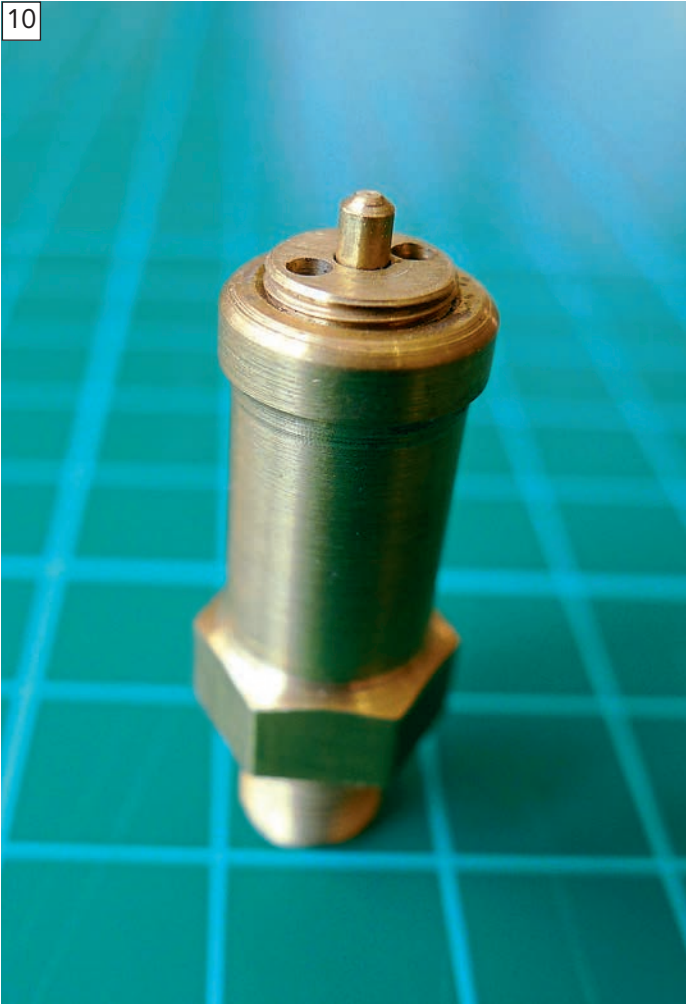
When adjusting a valve under pressure there's the danger of slackening the adjusting disc off so much that it comes adrift. Make sure you're well aware of how much thread is available by measuring before you start the process.
