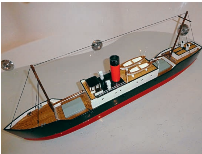
The bathtub test proves Nick's calculations correct, as Unity floats almost exactly on her waterline. Next stop, maiden voyage!
