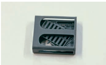
A common style of 3D-printed fittings with a 'cage' and scaffolding supports surrounding the fitting. The resin is brittle and can shatter if snips or a scalpel is used to remove them.
