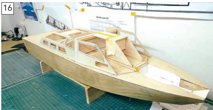
Building up the cab and after superstructure with a combination of 1:32nd marine ply and 4mm thick balsa sheet (which is extremely light yet structurally robust).
