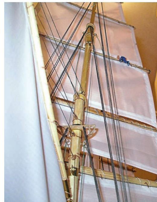
The captain's view of the sails on the main mast, with a sailor on the footrope of the upper topsail yard.
