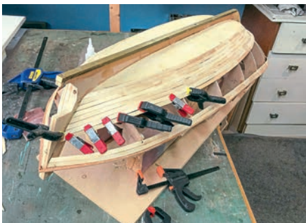
Work in progress on planking the hull.
