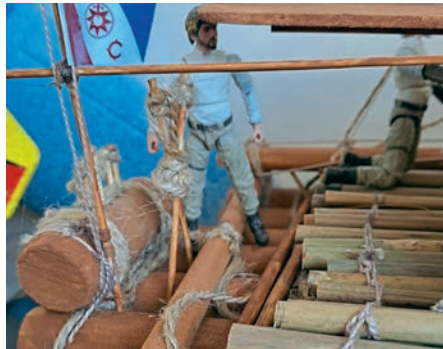
The rudder section, with ropes set up that allow the rudder to work either with or against the wind.
