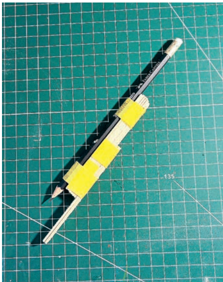
The simple homemade tool Tomasz uses for drawing symmetrical plank lines.
