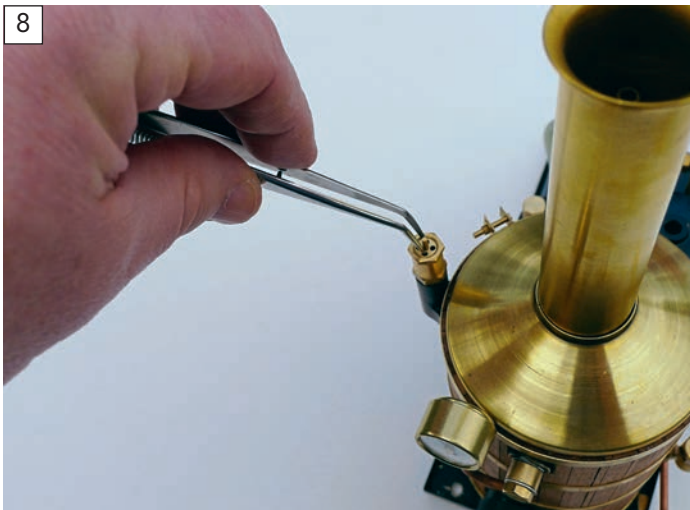
8 Richard likes angled ended tweezers for adjusting this type of valve because being able to see what you're doing makes things much easier. Also, if you do decide to adjust the valve while under pressure, which Richard doesn't recommend, be sure to keep your hands out of the way of the vented steam.
