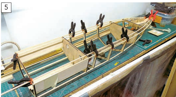
Securing the stringers and fitting the bow ramp.
