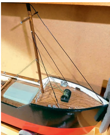
One of the best discoveries made during this project was the use of 1/16in diameter split pins as anchors for the mast rigging. The rigging itself was made from steel fishing trace (this is available in different sizes and is easy to install).
