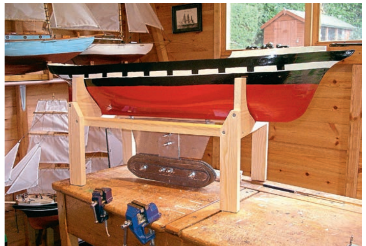
The finished hull on its stand, with the sailing keel attached. The legs of the stand allow the keel to be attached by the side of the pond, and the layout of aluminium sheet and lead strips can be seen on the keel.
