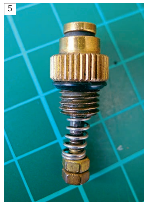
Another internal arrangement, but this time adjustable. It is a bit of a performance having to vent the boiler, remove the valve, make the adjustment, refit the valve and bring it up to pressure again to see if the adjustment was correct. It usually takes a few attempts.
