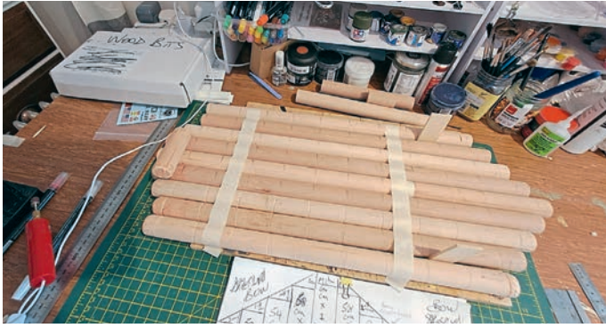
The broom handles with their ends chopped off and grooves cut into them, laid out ready to shape ready to tie together.
