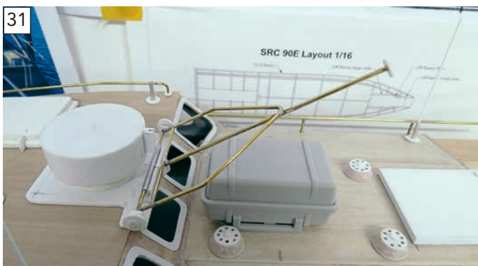
31 The lower 2mm brass spar of the mast has been inserted through a length of aluminium tube, this allowing the mast to retract.
