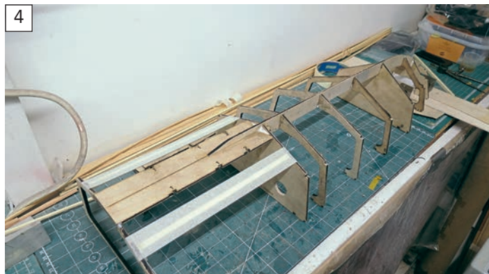
Assembling the frames to the keelson and incorporating the jet drive intake flat.
