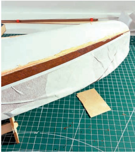
Finishing the underwater edge, using putty to seal any areas any potential leakage points in the masking.
