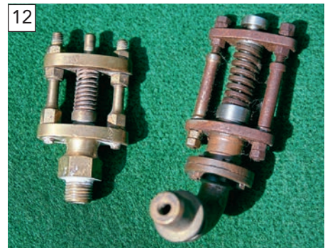
These valves are of a much more substantial build and would normally only be found on much larger, higher pressure boilers. As you can see adjustment is by moving the top beam up or down to adjust the pre-load on the spring.
