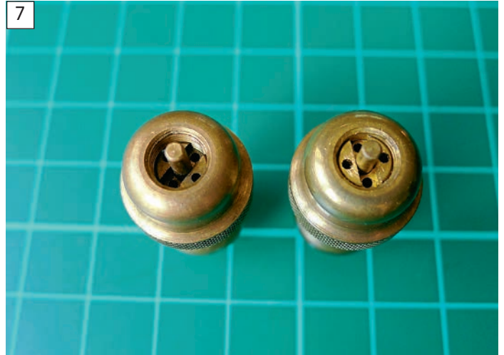
7 Adjusting discs can be rotated by either putting a pair of tweezers into the vent holes or making a bladed tool that fits over the end of the spindle and sits in the slot.
