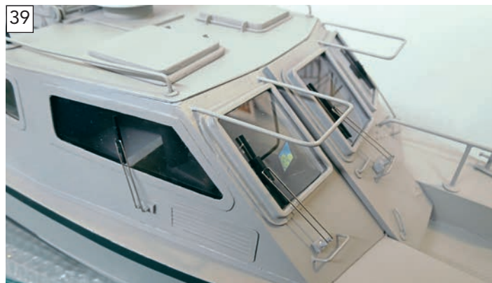
With the model glazed, the front and side wipers are fitted.
