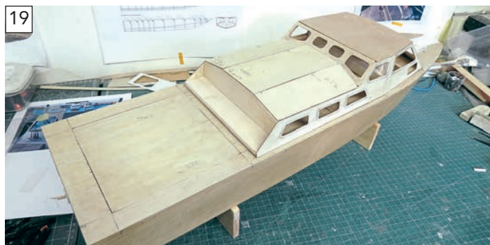
The cab roof and three superstructure roof panels cut to size, with only the latter fixed into place at this stage.
