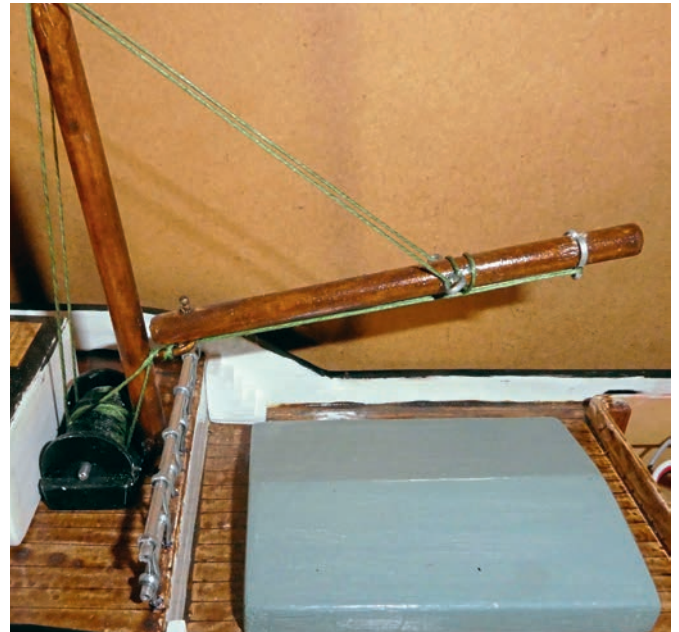
Derricks, made from 6mm dowel, with rope guides fashioned from 1/16in split pins. Dowel/scrap ply was also used for the two deck winches and wire spindle, with coarse cotton thread representing the ropes wrapped around them and secured with CA glue.
