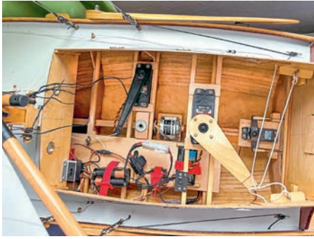
In this shot of the interior, note the wooden arm that controls the jib.
