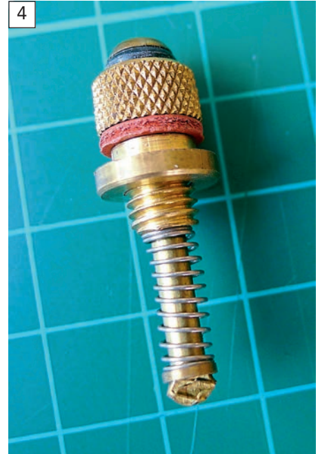
A safety valve in its most basic form frequently found on low pressure boilers of the LS and LO type. Despite being non-adjustable, these valves still have to meet the requirements of the Boiler Test Code, 2018.
