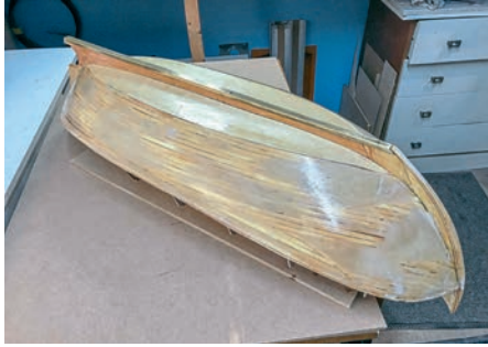
The planked hull coated with glass tissue.
