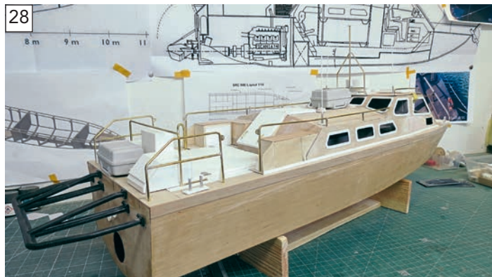
28 The construction thus far; it's worth noting that the transom platform had to be set higher up the transom than it is on the full-size vessel to ensure clearance for the reverse bucket.
