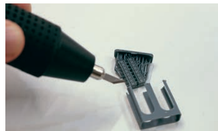
An ultrasonic cutter makes quick work removing the cage around a component; in this case revealing a radar set from a new 1:350 scale Type 42 Destroyer by ForeArt Models.
