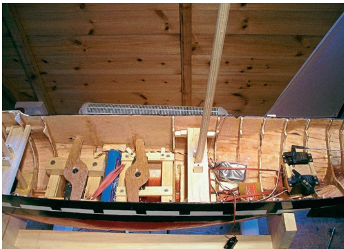
The interior of the hull, with the two sail arm servos for the yards between the masts, and those for the spanker and rudder at the stern.
