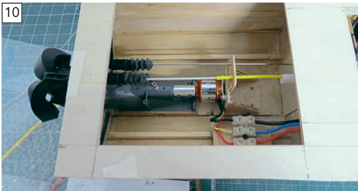
10 The 22mm jet drive, 2200KV brushless motor and linkages fitted into the hull but yet to be fixed.
