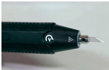
The blade, which can be easily changed easily via a grub screw, is small but very sharp.
