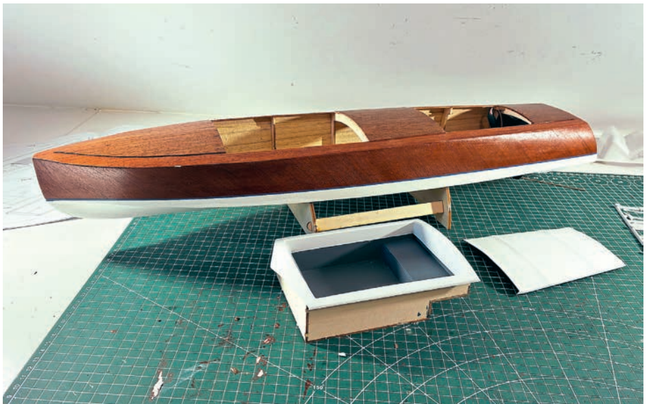
The planked hull, with the cabin compartment construction and hatch cover yet to be installed.
