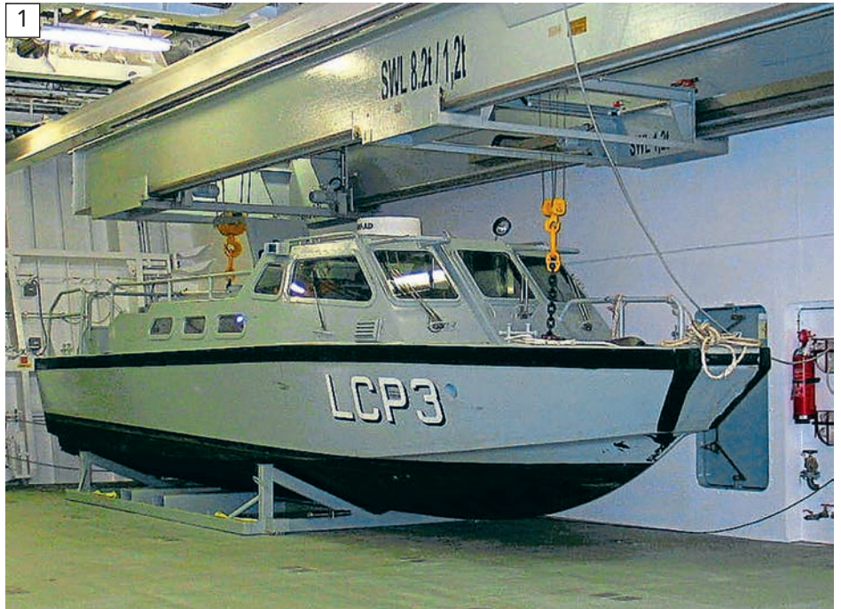
1 One of two SRC90-E LCPs, fitted to the launch and recovery hoist within the mission bay of the Absalon. Image courtesy of Wikipedia.
