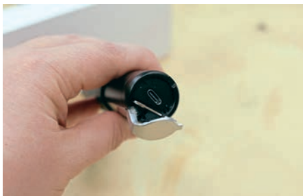
The charging point is a conventional USB-C connection that you can plug into a standard USB plug. The storage for the Hex drive is next to this connection.
