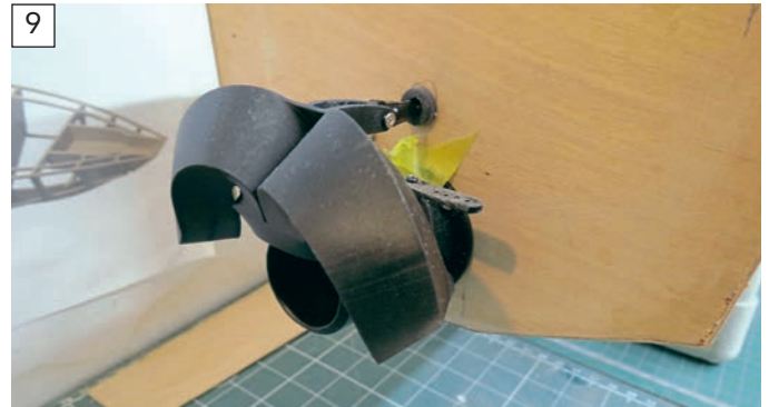
9 The water jet drive, stator and 3D-formed bucket fitted but not yet fixed into position. The shape of the bucket has been modelled as per its full-size counterpart.
