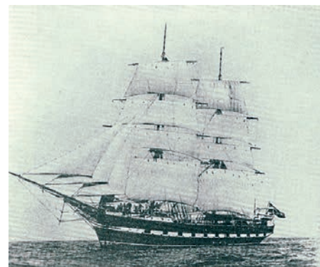
Fame minus her royals (the topmost square sails). Note the pilot boat hanging from davits at the stern in front of the ship's ensign.
