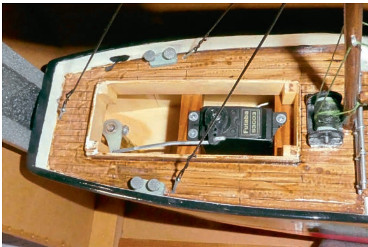
Bollards created from galvanized 2mm in diameter nail heads, epoxied, in pairs, through a scrap piece of 3mm ply, and painted. The plan suggested the positions for these around the deck.
