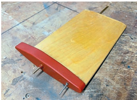
The lead weights bolted to the removable keel.
