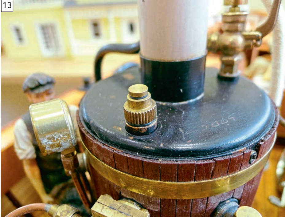
13 Many Cheddar boilers were supplied with the same safety valve fitted, which can be removed to adjust – certainly the safest procedure, if perhaps not the most convenient.
