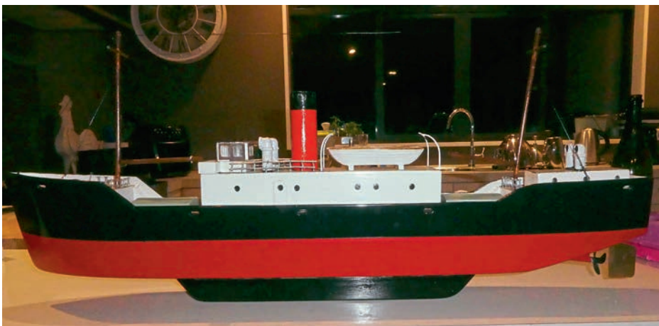
SS Unity with the painted keel screwed to her bottom prior to a first bathtub test.
