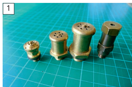
A small selection of different manufacturers' safety valves in various capacities.
