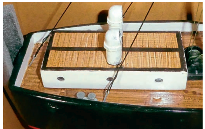
The rear hatch, simply made from scrap 1/8in ply and 1/16in bass sheet. Portholes were glazed on the inside with the same repurposed material used for the bridge windows – once again, secured with 5-minute epoxy. The deck was painted using a thinned 'wash' of wood stain to simulate decking boards.
