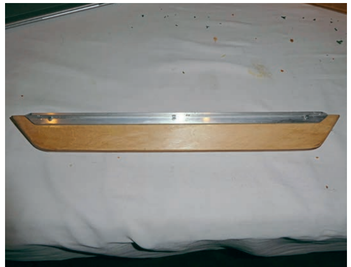
The keel glued and screwed to brackets prior to painting.
