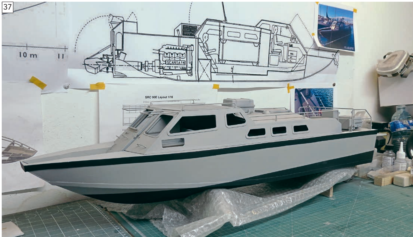
Several coats of Mr Hobby super clear semi-gloss finishing spray applied prior to glazing.
