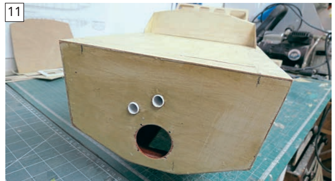
11 Forming the linkage tubes to the bucket and nozzle steering.
