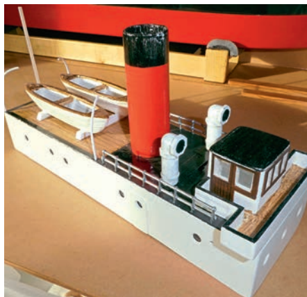
1/16in split pins were wrapped around aluminium to create railings. However, having since read Glynn Guest's 'Nailing railing' article in the July 2025 issue of Model Boats, Nick intends to use the less fiddly method of soldering his railings from copper wire in future.
