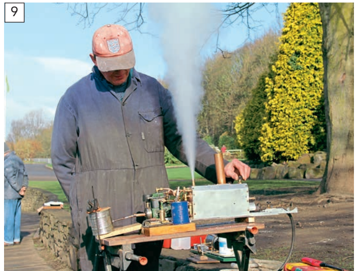
9 Note the amount of steam that can be released when a safety valve lifts fully with the boiler burner under full flame. Wearing gloves and goggles is a sensible idea, as is keeping well out of harm's way.
