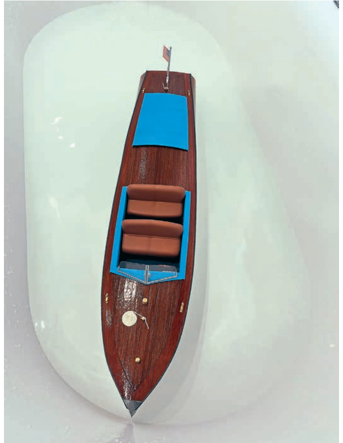
Phantom gets a bathtub test – note, this should not be done until varnish has had time to fully cure.
