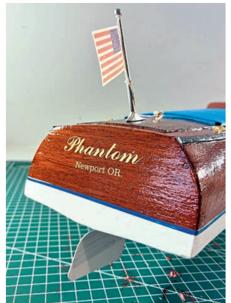
The decal, applied after a first coat of varnish, and the flag flying mast fitted.
