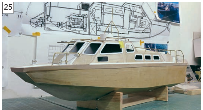
25 Each of the window frames after being marked, cut from .50mm styrene sheet and fixed.
