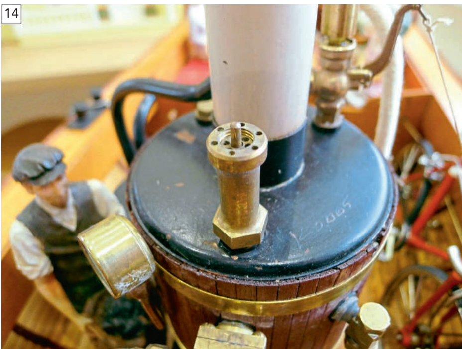
14 These are often replaced by modellers with an externally set valve, which is more convenient to use and doesn't have the 'O' ring valve that will be subject to deterioration over time.
