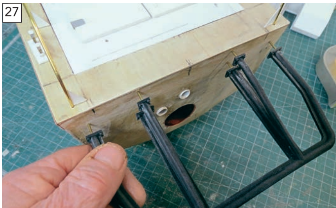
27 Locating the transom platform securing pins to their pre-drilled locations.
