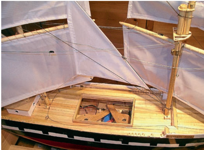
The two sail arm servos seen through their hatch, with the servo arms overlapping, and the yards on opposite tacks.
