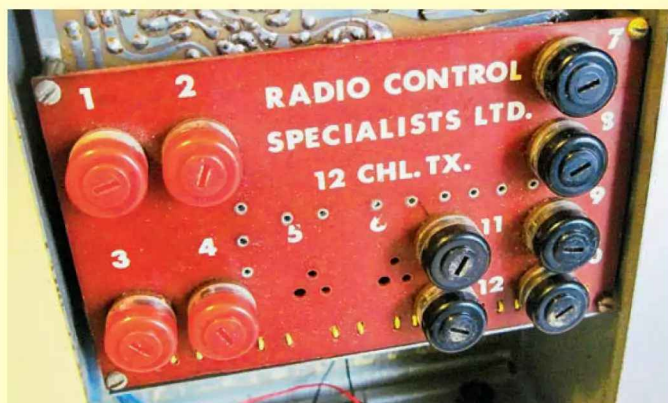
The RCS Competition-10 transmitter. Note all the internal controls that required adjustment before every use.
