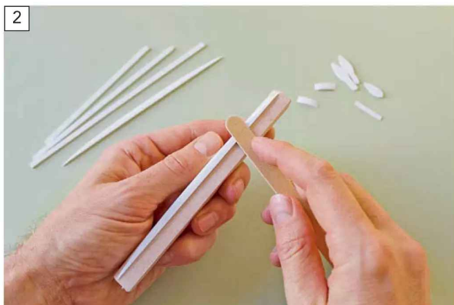
Double-sided tape was used to hold the pieces in place while Ross sanded them.
