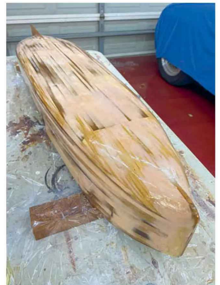
With the hull construction completed, and its surfaces filled and sanded, it now receives an epoxy coating to make it waterproof and provide a smooth surface for the aluminium foil tape riveted plating to adhere to.
