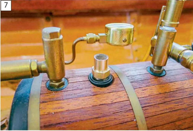
Older Hemmens boilers like Richard's feature unusual threads, so a one-off adapter was necessary to convert the boiler thread to the 1/4-inch x 40 tpi thread needed for the sensor.
