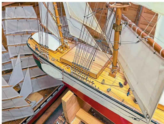
The deck between mizzen and jigger now has a proper hatch, under which lies the new sail arm servo. The lifeboats now have to be able to swing outboard to give access. If you look either side of the masts, you'll see the oblong blocks containing the fairleads.
