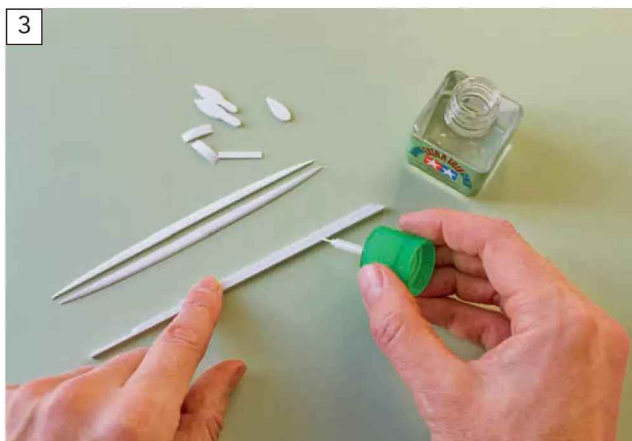
The main structure was laminated together using Tamiya extra-thin cement.
