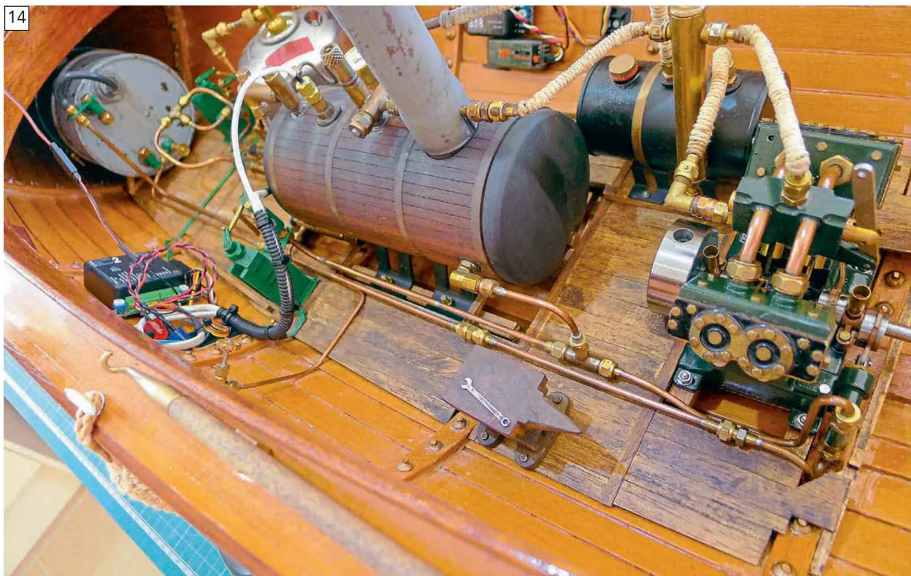
The completed water system with all piping reconnected and the valve set-up and connected into the ABC2 unit.
