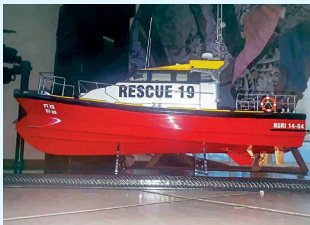
Doug's next mission will be the conversion of this 3D-printed static ORC (Offshore Rescue Craft) model – the replacement for the now being phased out NSRI Brede-class lifeboat – for R/C operation.
