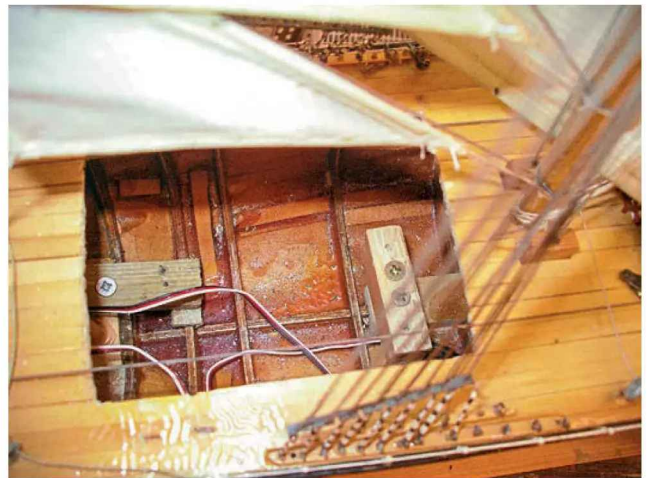
Fitting wooden blocks in the bottom of the hull.
