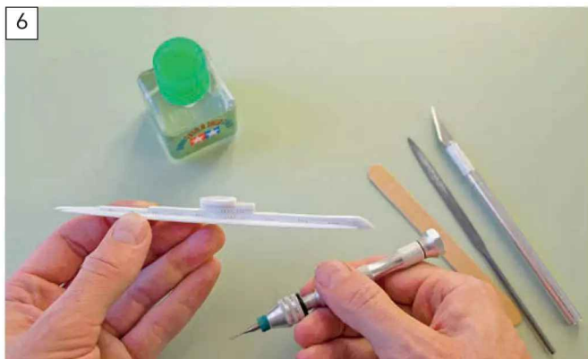
Ross marked the limber holes with a pencil and then drilled them with a pin vice.
