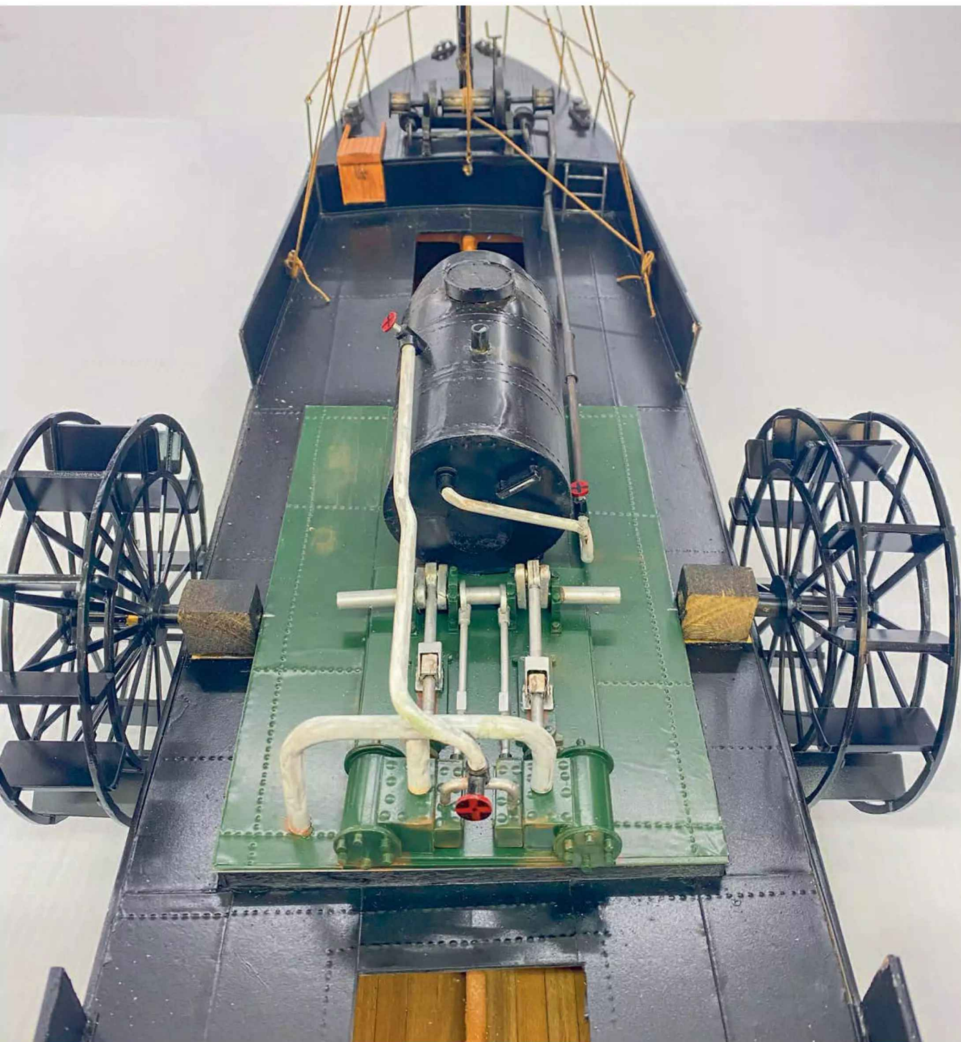
A mock-up of a boiler and engine. The boiler started life as a can of coconut cream, while the engine was fashioned from various polystyrene shapes. The two paddle wheels have been installed onto wood blocks, which will be hidden by the steps once the superstructure is in place.
