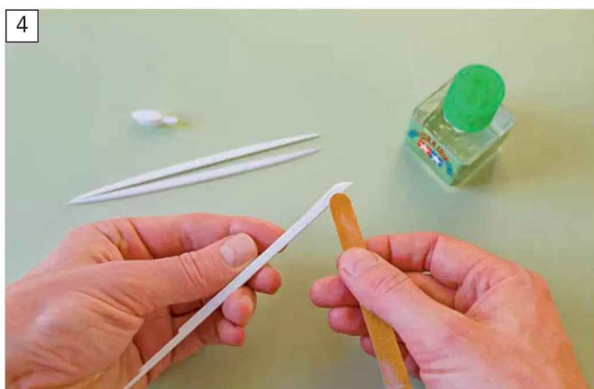
Ross beveled and smoothed the sub's ram-shaped bow with an emery board.
