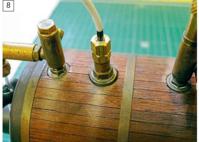
Once fitted, the sensor sits neatly into the steam space of the boiler.
