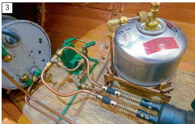
All the existing gas pipework and valve arrangements are exactly the same as they were on Denes Designs' original ABC, and as Richard already had the latter installed in Hereward, nothing needed be changed when swapping this out for the ABC2 unit.
