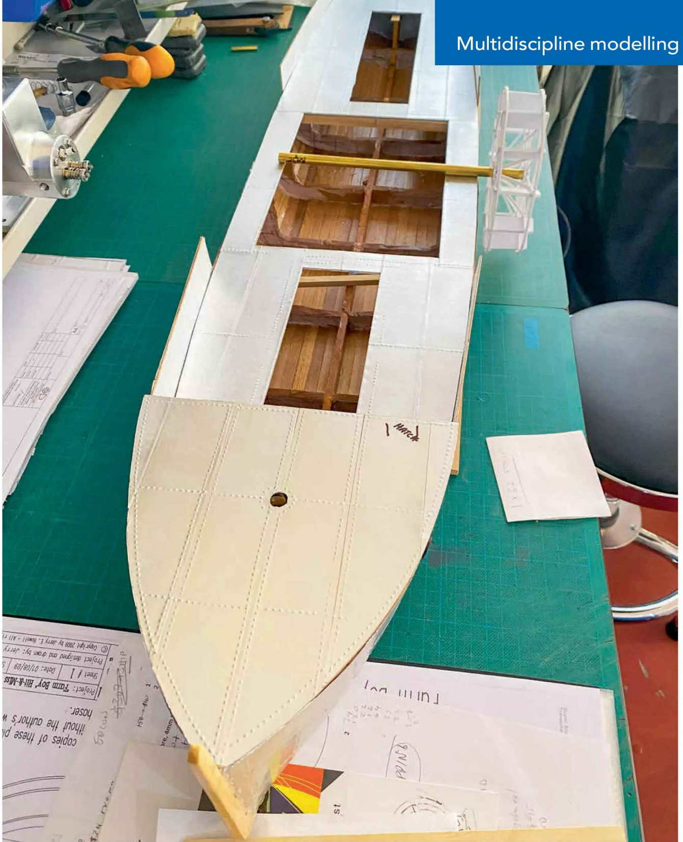
The deck plating completed. Fwd, aft and engine hatches are removable, allowing access to the ship's hull for possible future R/C installation.
