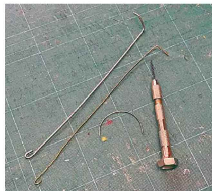
From left to right, some of the tools Nev used to get at inaccessible places below deck: two long hooks, a circular needle and a pin vice – all indispensable!
