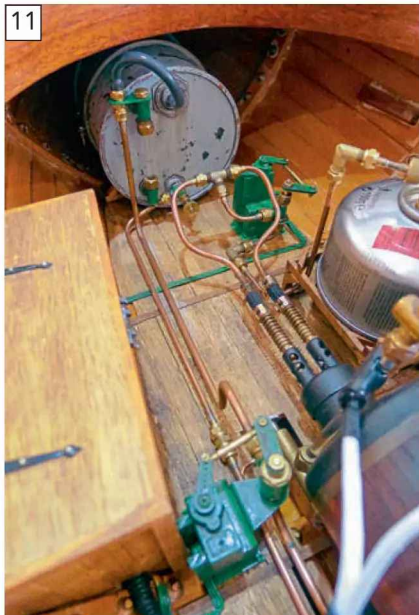
All the gas pipework refitted, and the gas valve connected up to the ABC2 unit. The gas tank has a cover to hide it when the boat is in operation.
