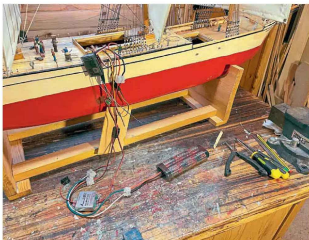
The other part of the refurbishment was a good look at all the other electrics on the boat. Here, the wiring/battery hang out of the midships hatch for inspection. Nev changed the UBEC and both the other sail arms.
