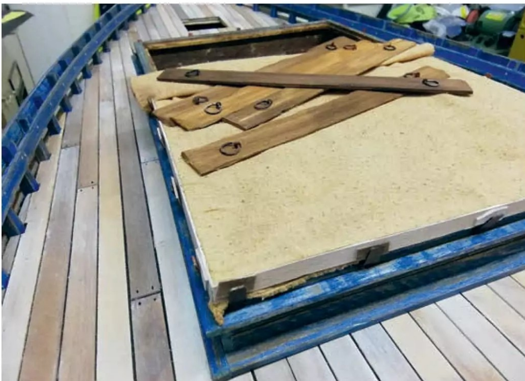
The first of the deck fittings to be made was the hold. The whole assembly lifts out to gain access to the hold in which the two batteries are located. The cover is made up from plywood boards, with the cloth tarpaulin glued on covering about 2/3rds of the opening. The removed boards have been 'thrown' on.
