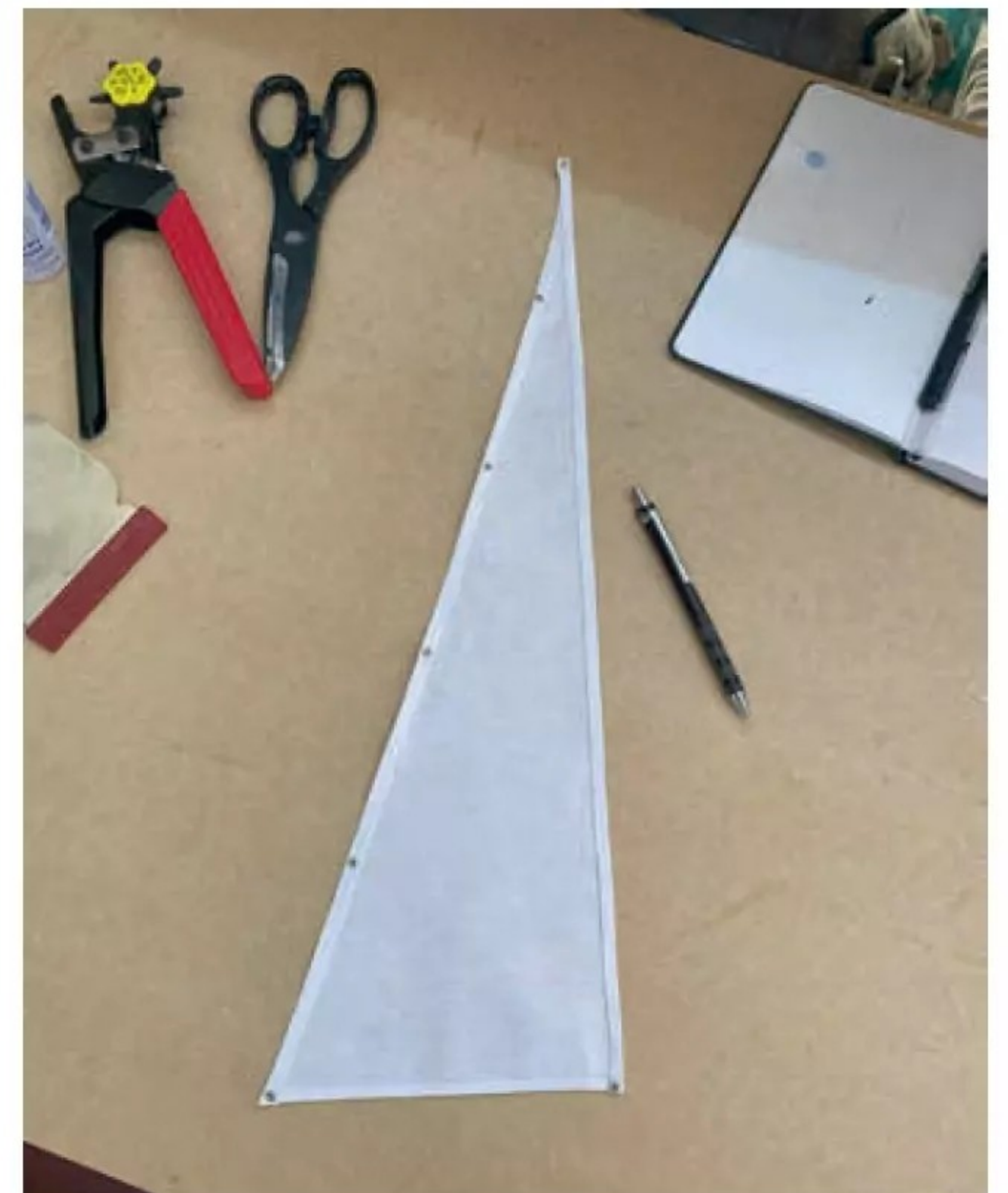
The fore sail under construction. Note the tiny stainless-steel grommets used for the rope lashing to the fore stay, mast top and sheet.
