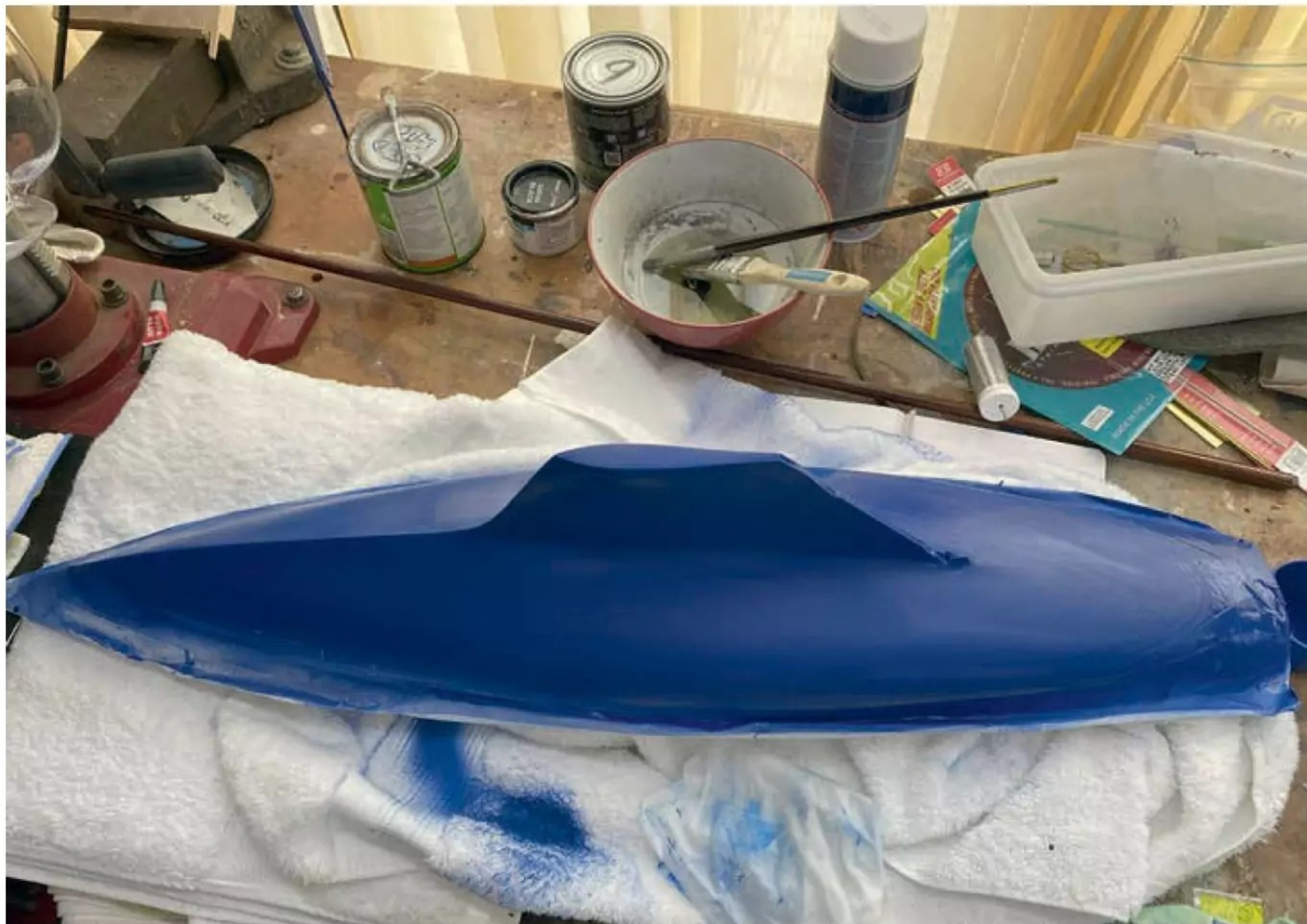
Sanding the final coats of paint with 2000 grit wet and dry paper prior to polishing with car polishing compound.
