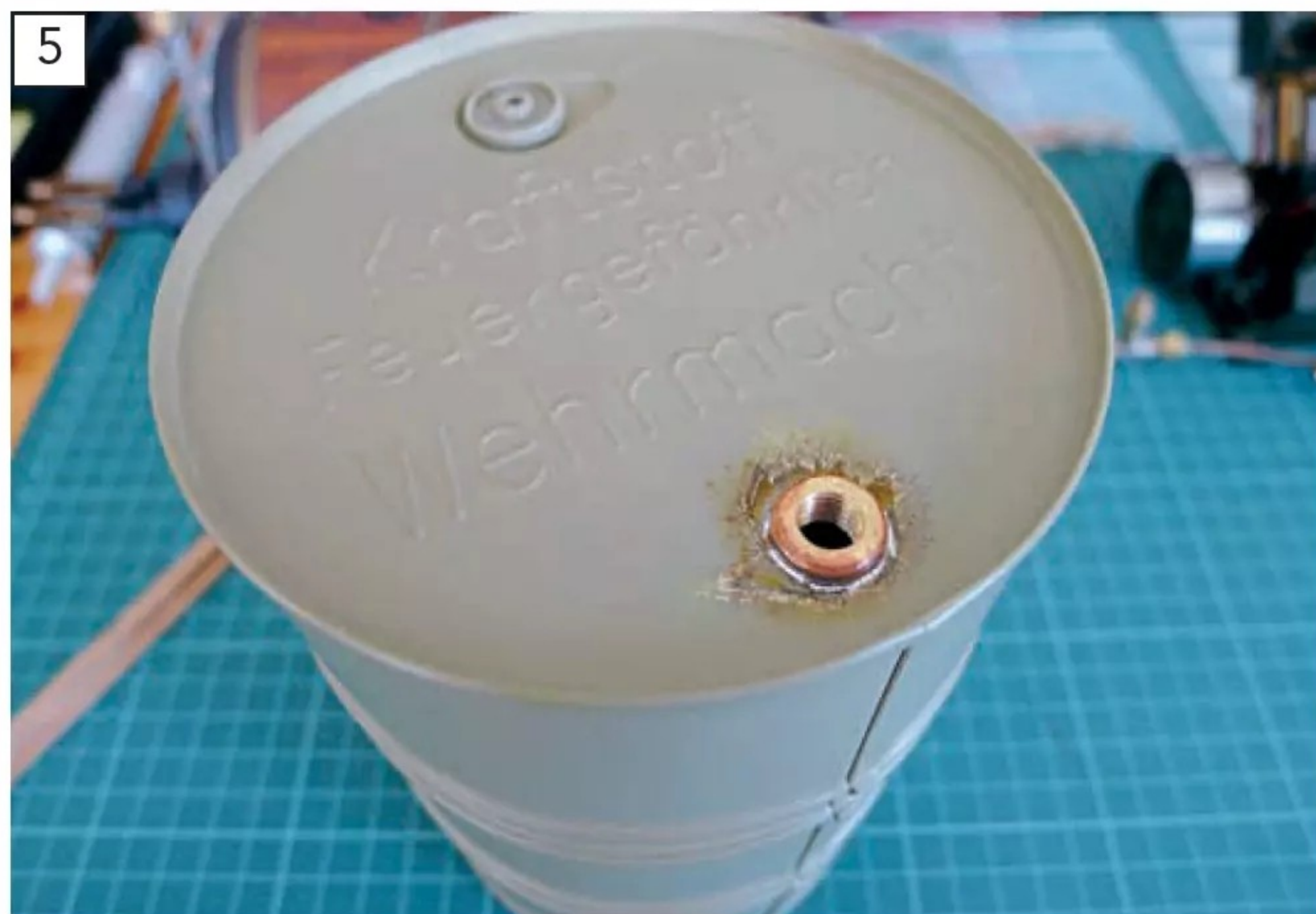
The original oil drum, being tinplate, took soft solder perfectly, so the bushes for the sight glass and the outlet valve were soft soldered in place.
