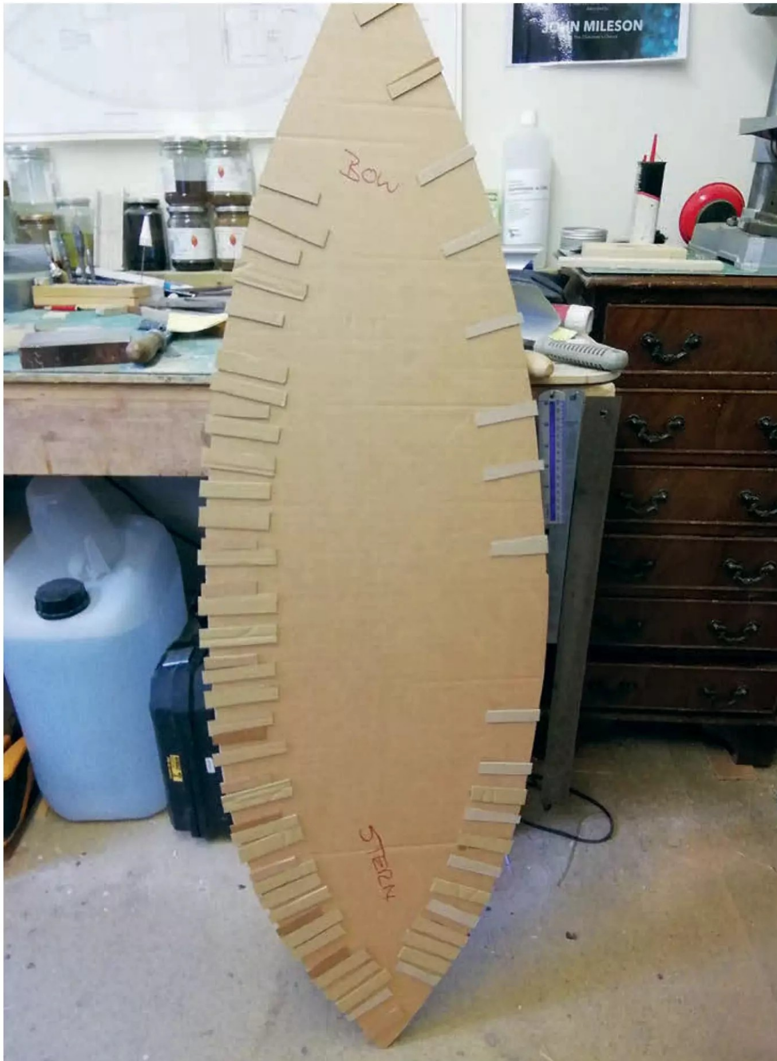
To establish a reasonable fit for the sub deck, a card template was made, loosely fitted and 'fingers' of card glued on to identify the final shape of the deck. The template was then placed onto the 3mm plywood sub deck and the final shape outlined in pencil prior to cutting out with a craft knife.
