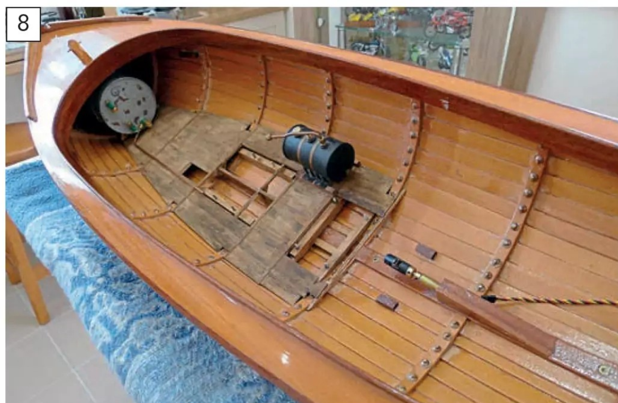
The deck, complete with feed tank and separator tank, forms a single removeable unit. It sits on a vertical beam on the main keel, with notches cut in so that it locates around the side frames.
