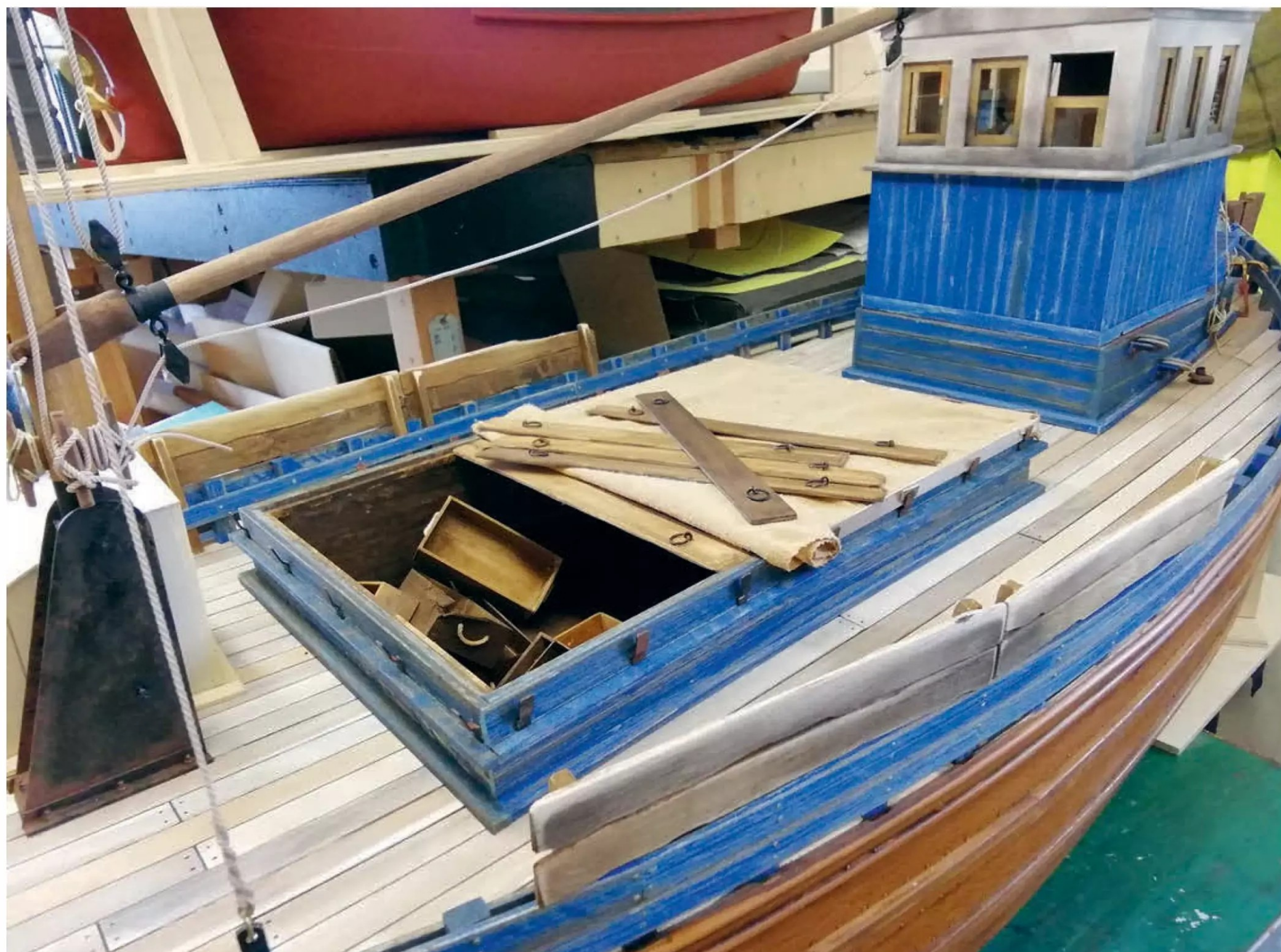
With the wheelhouse and fish hold, both of which are removable for access to batteries and electronic equipment, it was time to start adding details. Note, too, the main mast and boom now in place.
