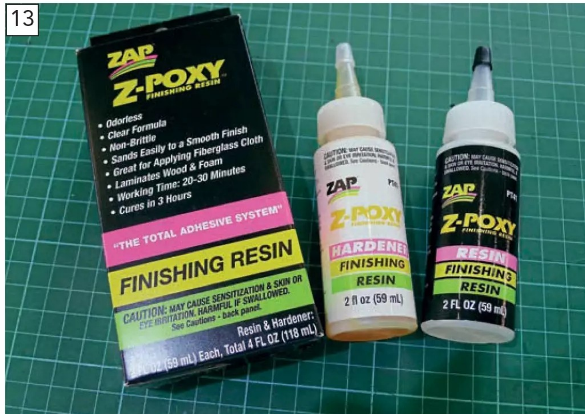
The interior of the new 3D-printed tank was given a coat of Z-Poxy finishing resin. This two-part product was simply mixed (50-50) in a small, graduated beaker and painted on with a cheap disposable paint brush.
