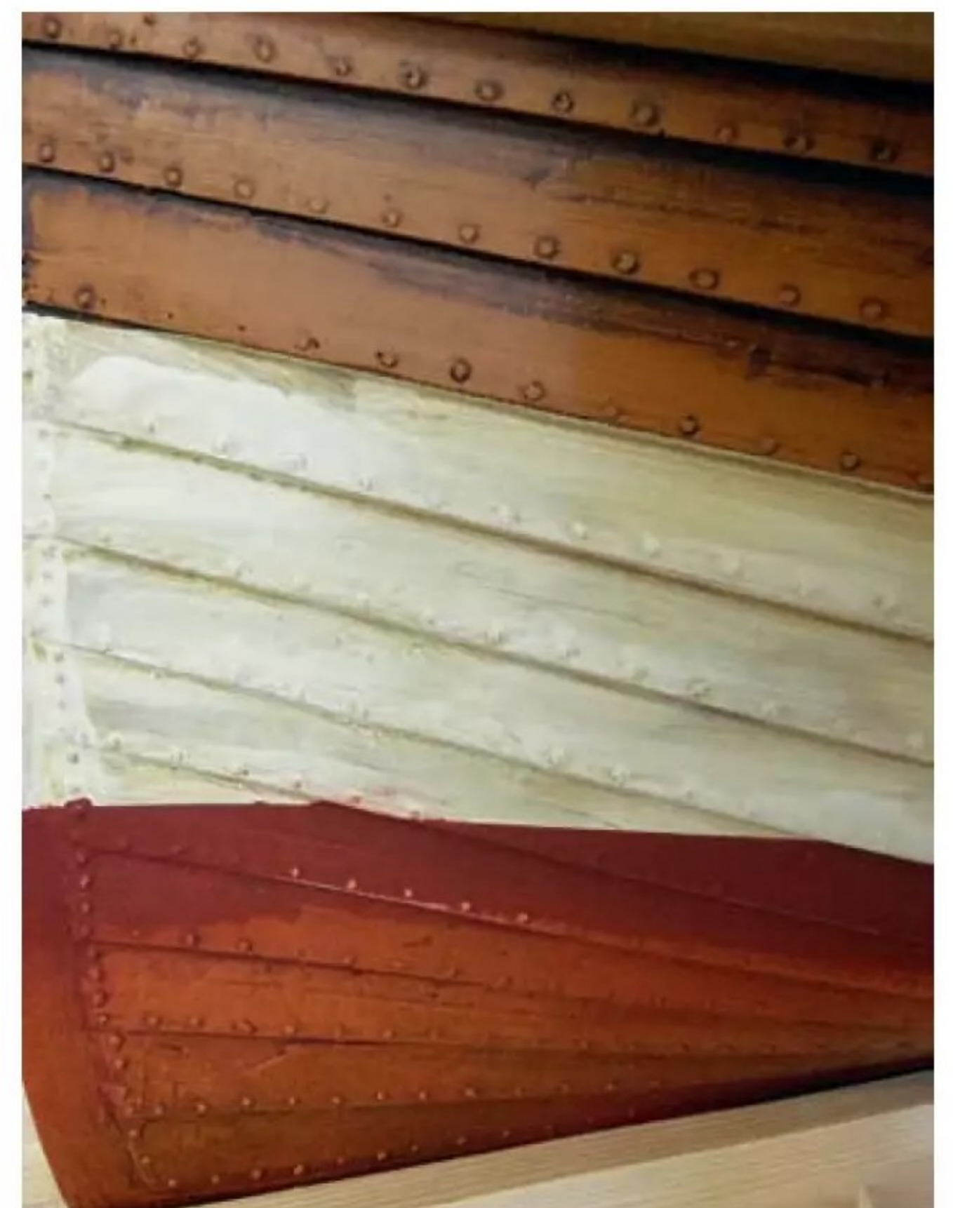
A similar effect was achieved with the application of just one coat of red oxide to the lower portion of the hull.
