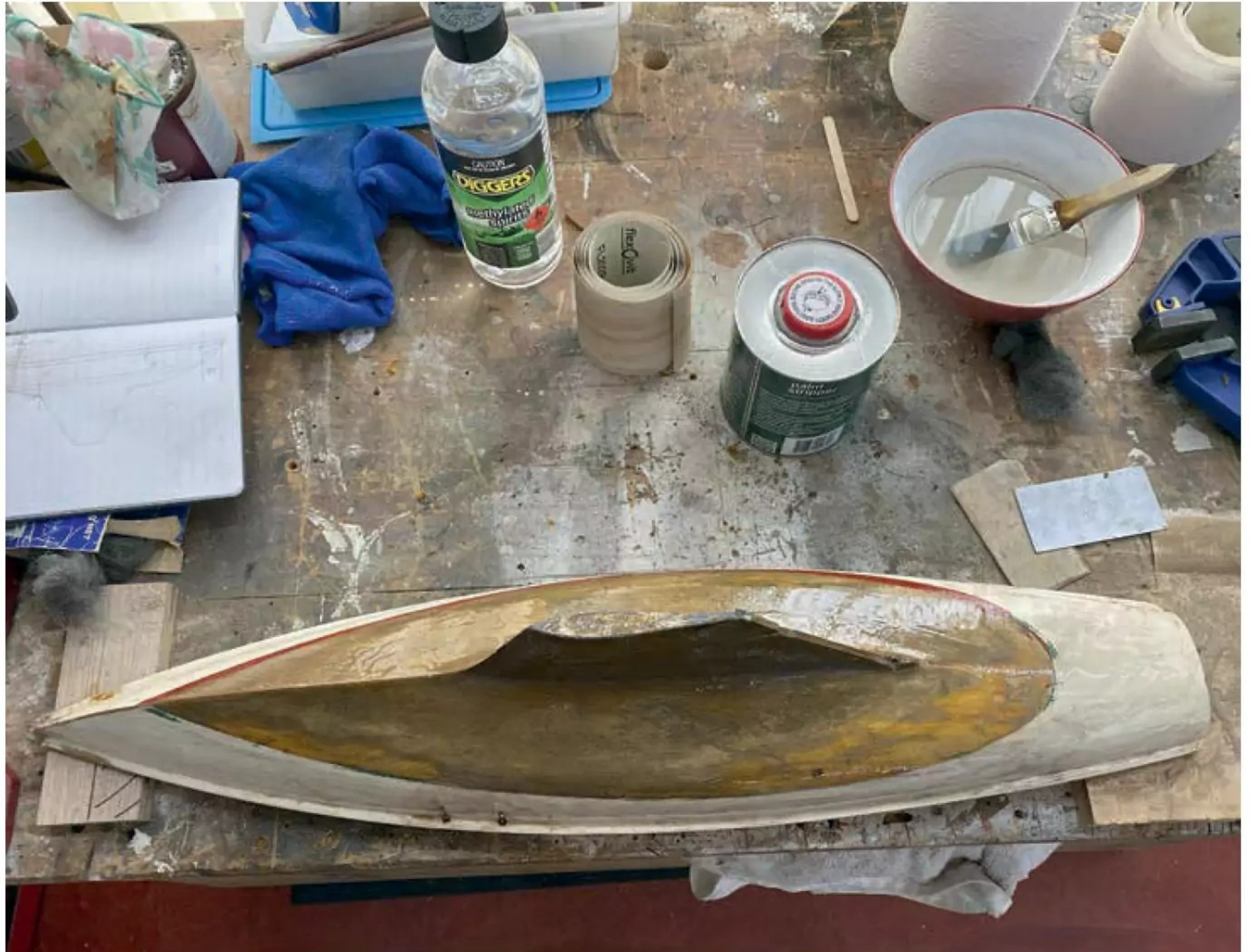
Stripping the very stubborn to remove paint from the hull took several attempts and involved lots of paint stripper, scrapping and vigorous sanding.
