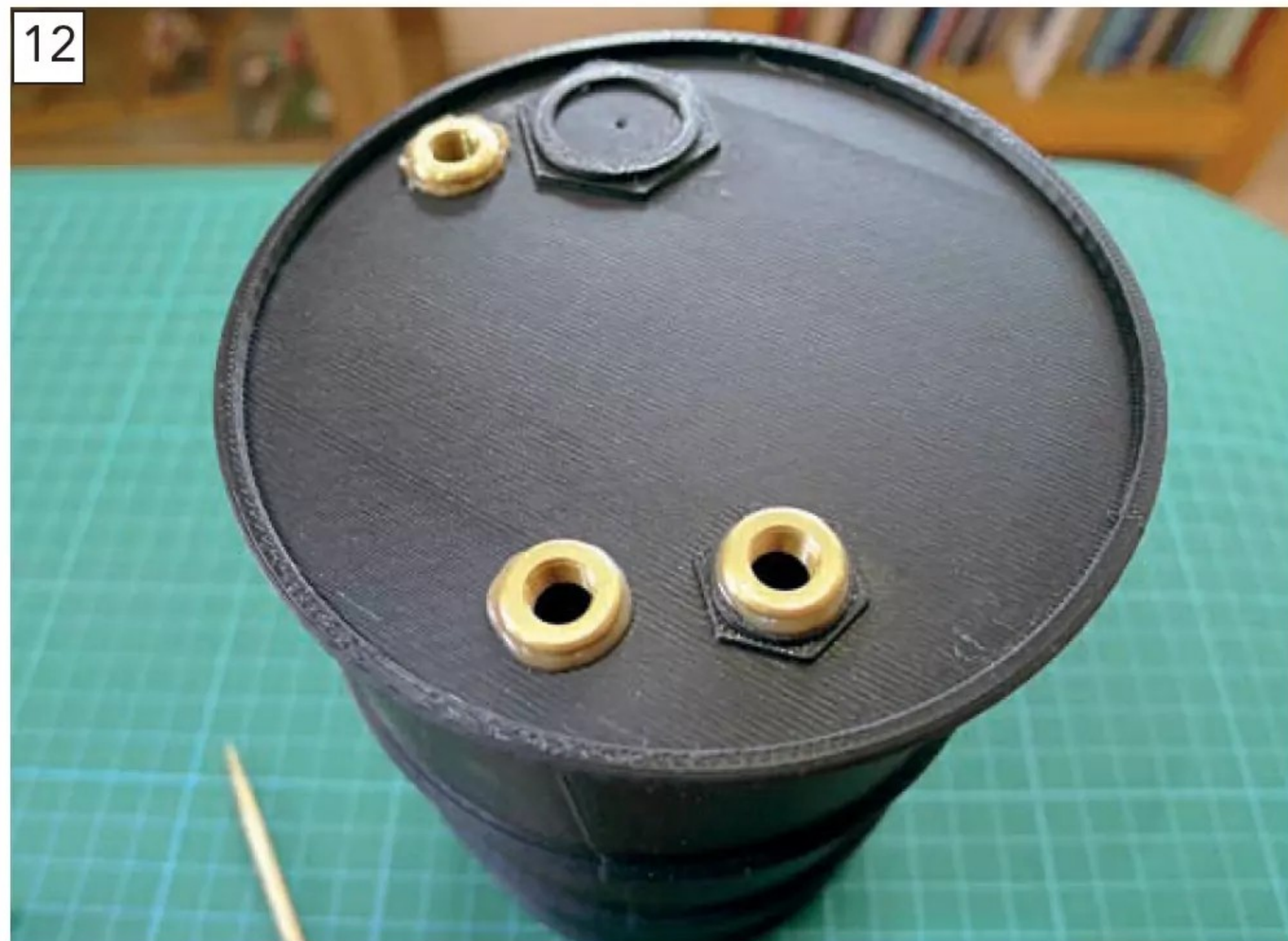
The fitting bushes were glued in place with Stabilit Express , which doesn't actually dissolve the plastic surface but does have an incredibly strong grip on it – so should provide enough strength for the job.
