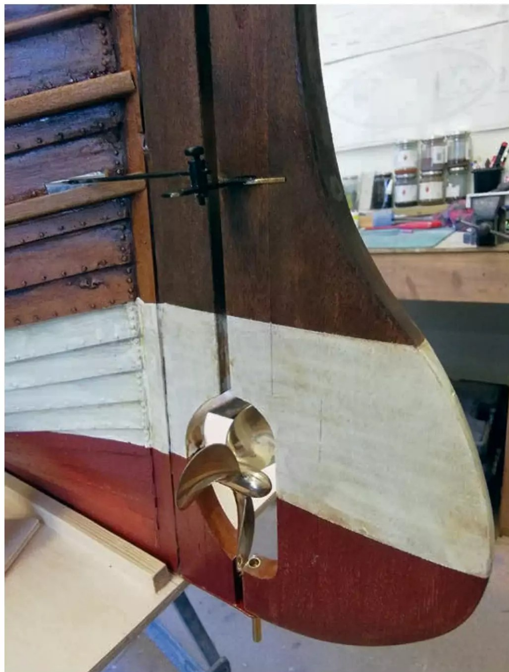
With the motor and shaft installed, the large rudder was fashioned from teak offcuts. With this in place, the propellor was fitted in readiness for testing.
