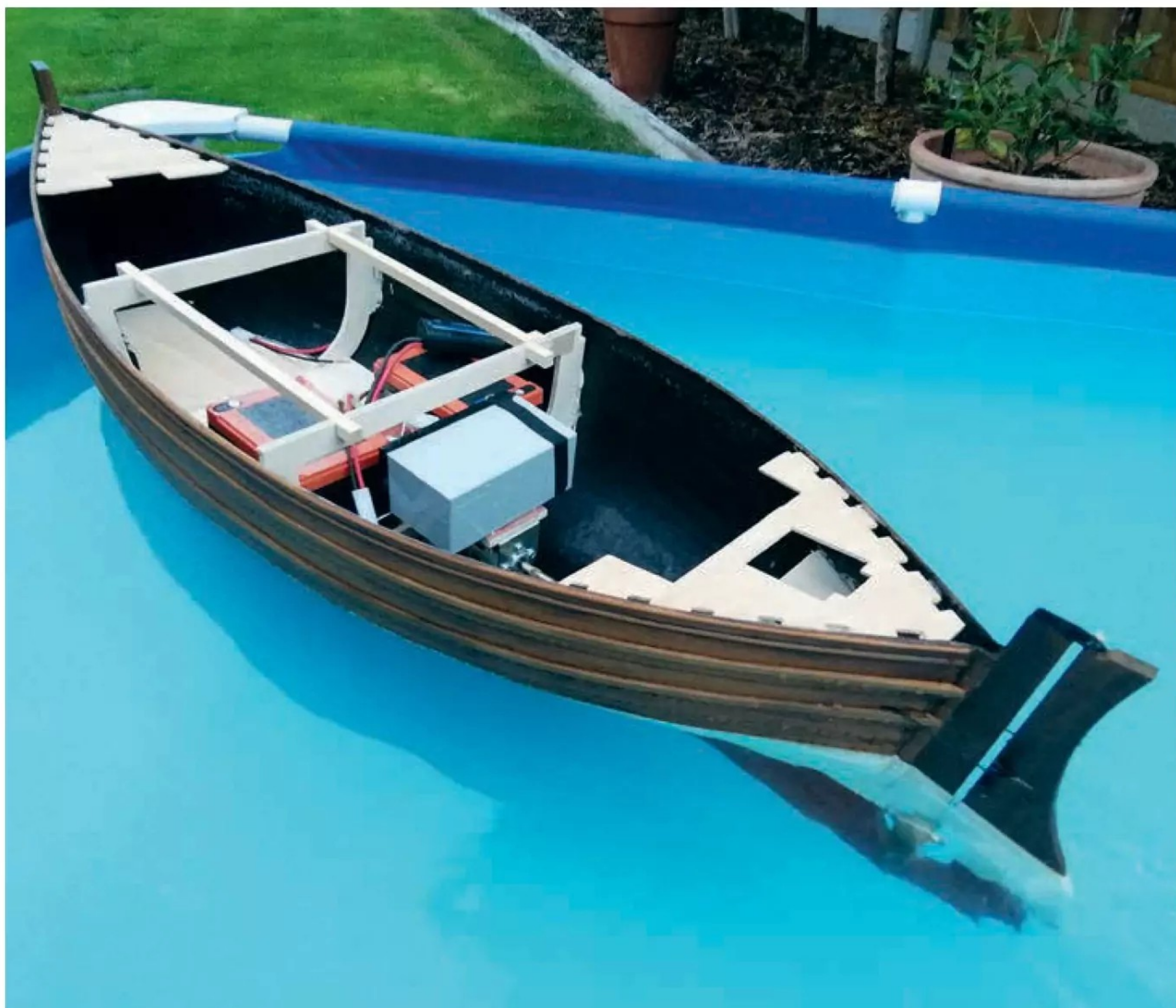
Mark's paddling pool, in which he and John established the amount of ballast that would be required by their boats (this shot taken in more clement weather). To lower the hull to an acceptable waterline, it was necessary to use both lead acid batteries plus an estimated 7lbs of additional ballast.
