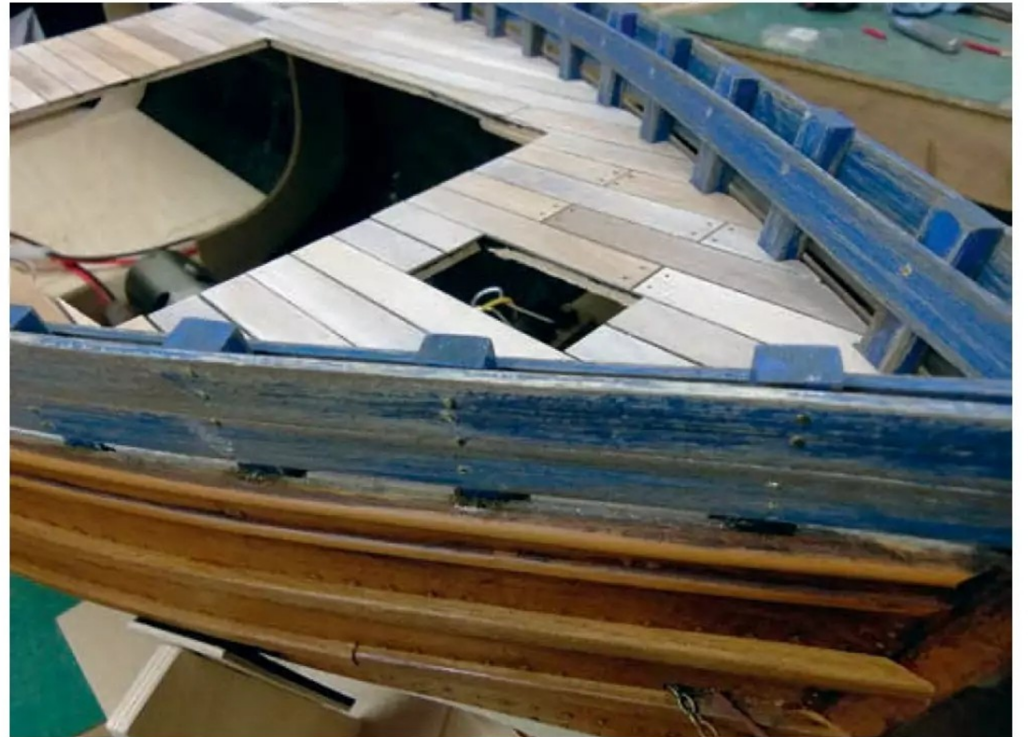
The bulwark extensions were weathered first, while the planks on the deck were individually weathered before gluing down. These were stained with Dark Oak or Antique Pine water-based wood stain, which while still wet was over painted with white enamel paint that was immediately wiped off. This would be further enhanced with weathering powder.
