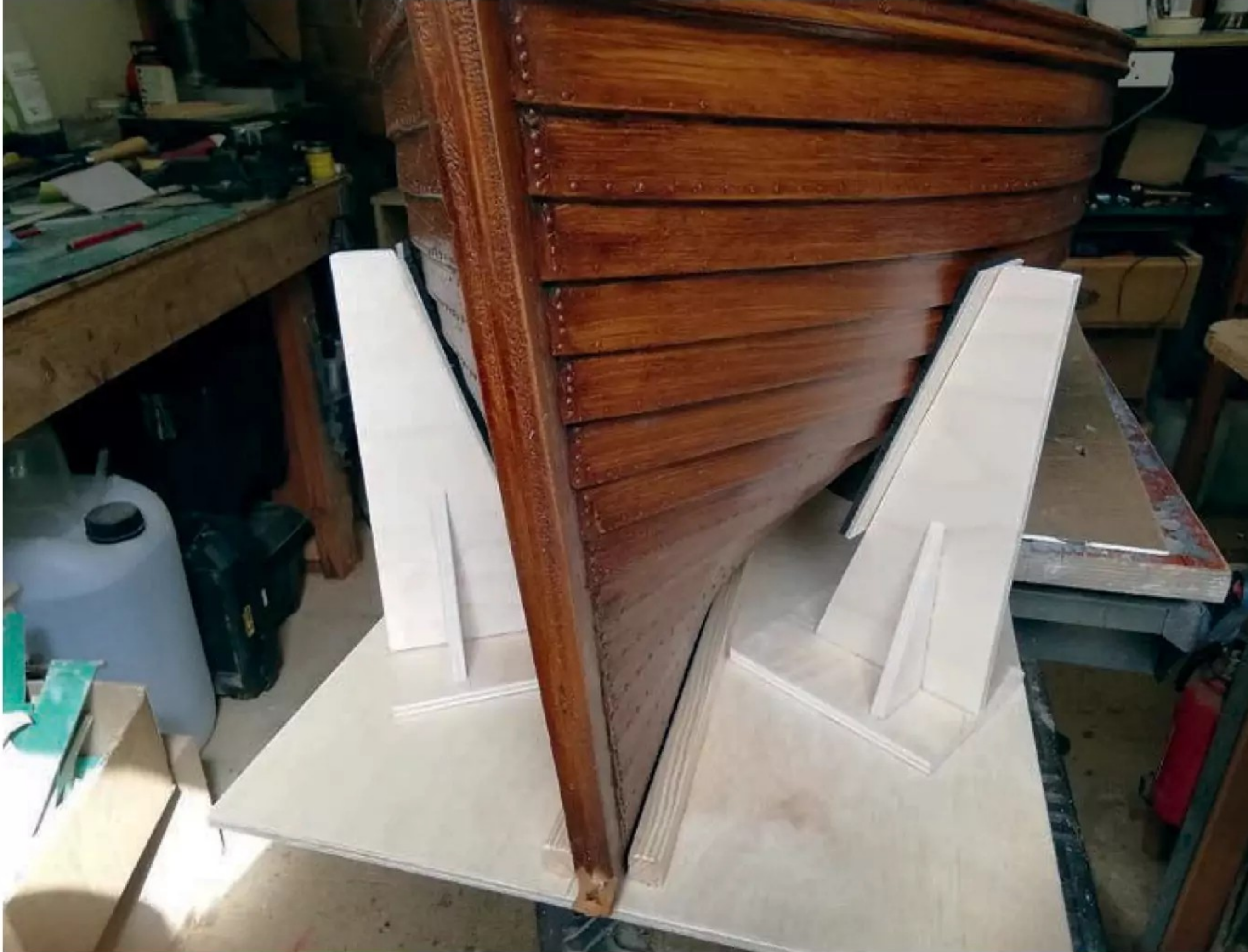
Being quite difficult to handle, John built two smart but robust cradles for the Fifies from plywood.
