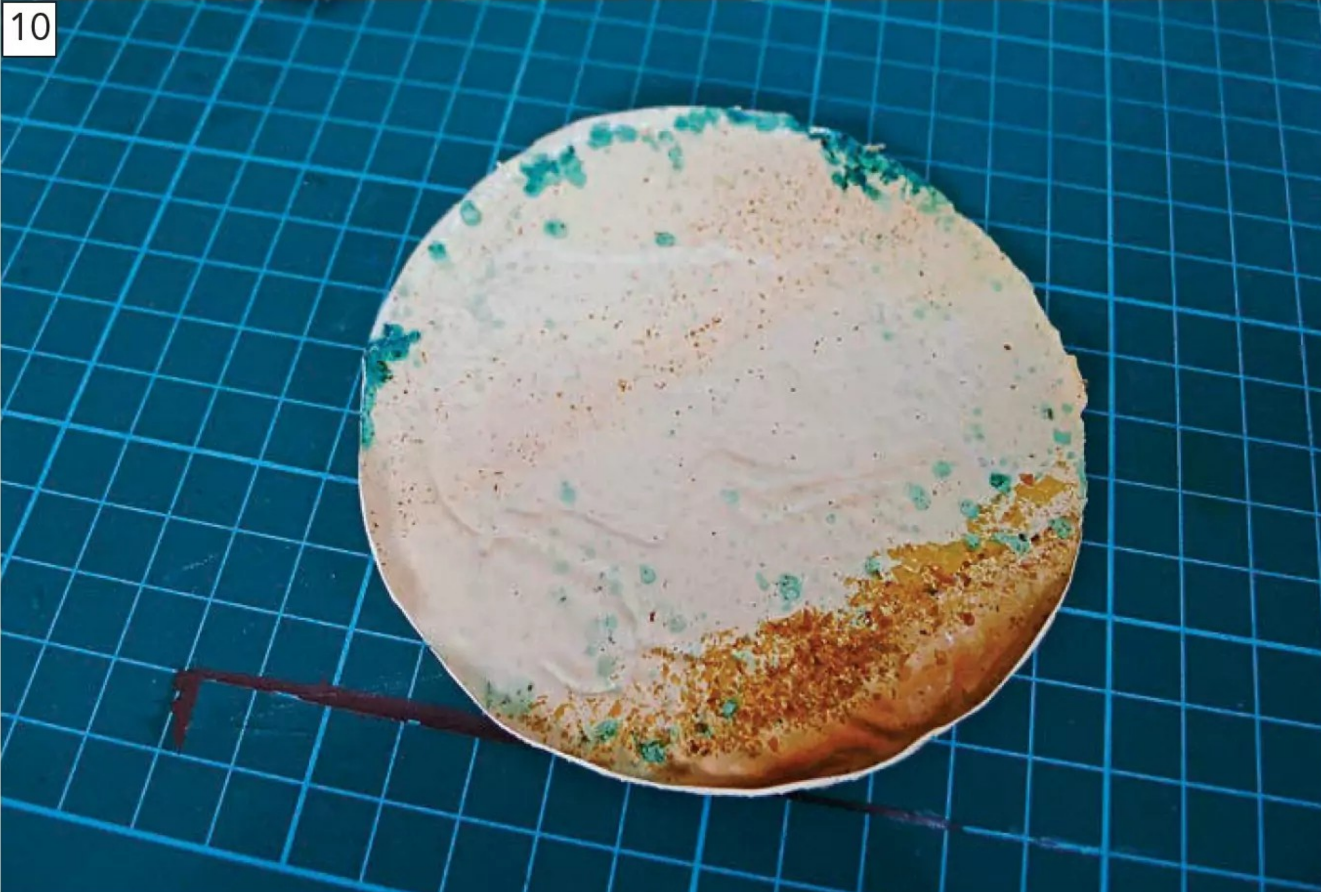
Also very noticeable were the Verdi Gris deposits, caused by the corrosion of the copper pipes inside the tank as they interacted with the tin tank shell.
