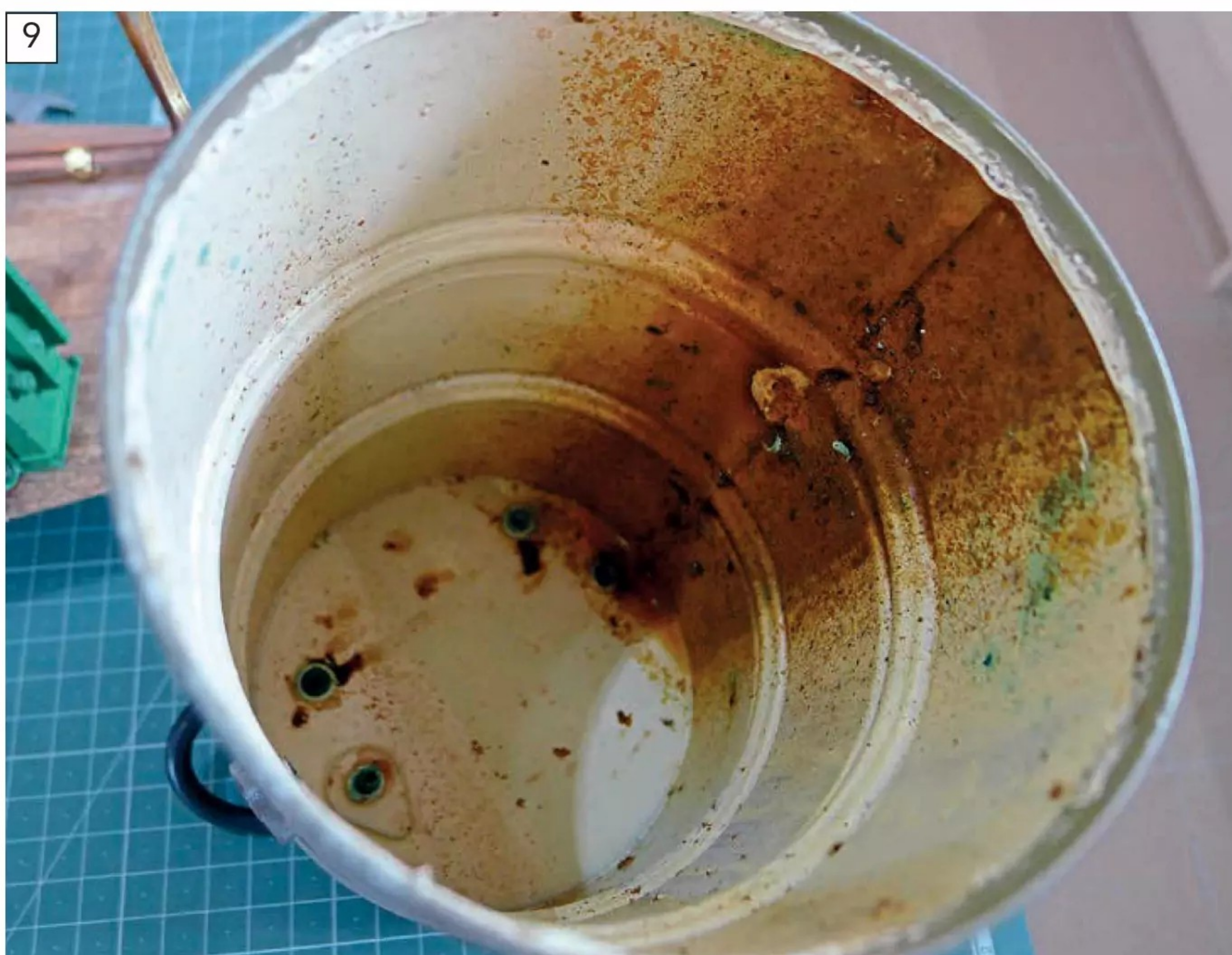
The sorry state of affairs that greeted Richard when he opened up the feed tank. The internal enamel coating he'd applied had failed to seal everything completely, so unfortunately rust had formed in the tank joint.
