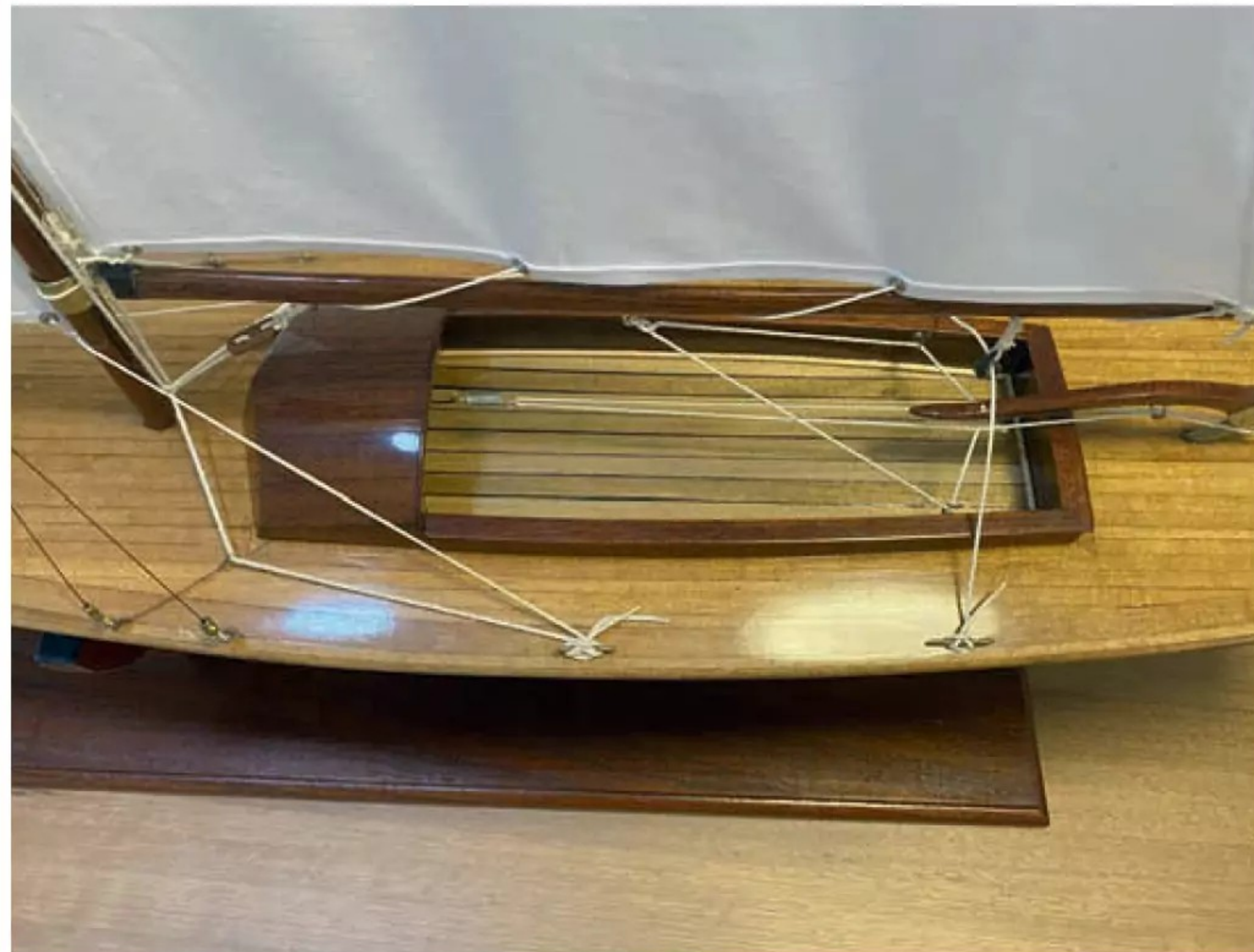
Stuart's version of the pond yacht's self-steering system.
