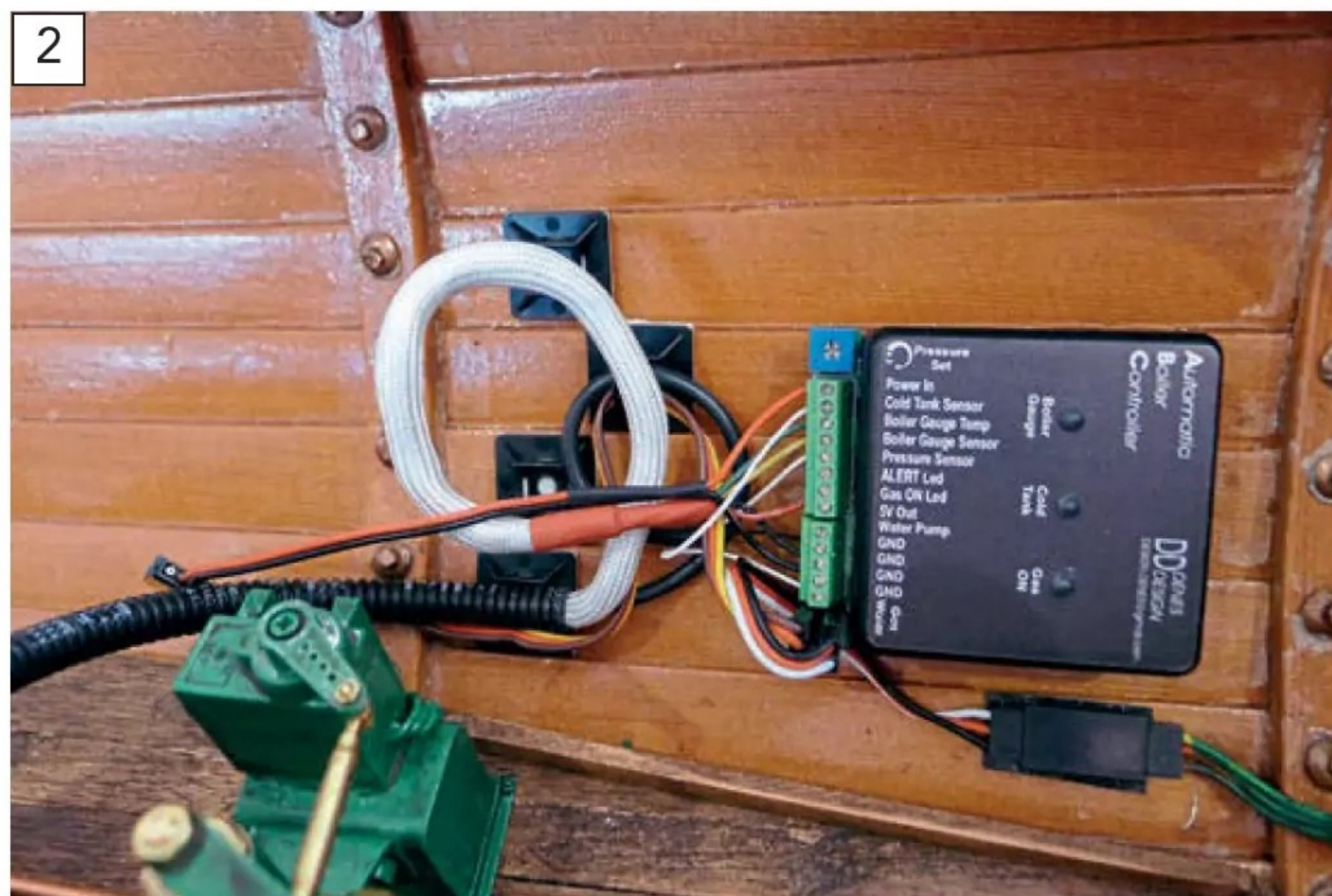
The Automatic Boiler Control Unit sits neatly inside the side box, with the sensors from the boiler, the servos to operate the gas valve and the water valve and the connection for the power supply all connected.
