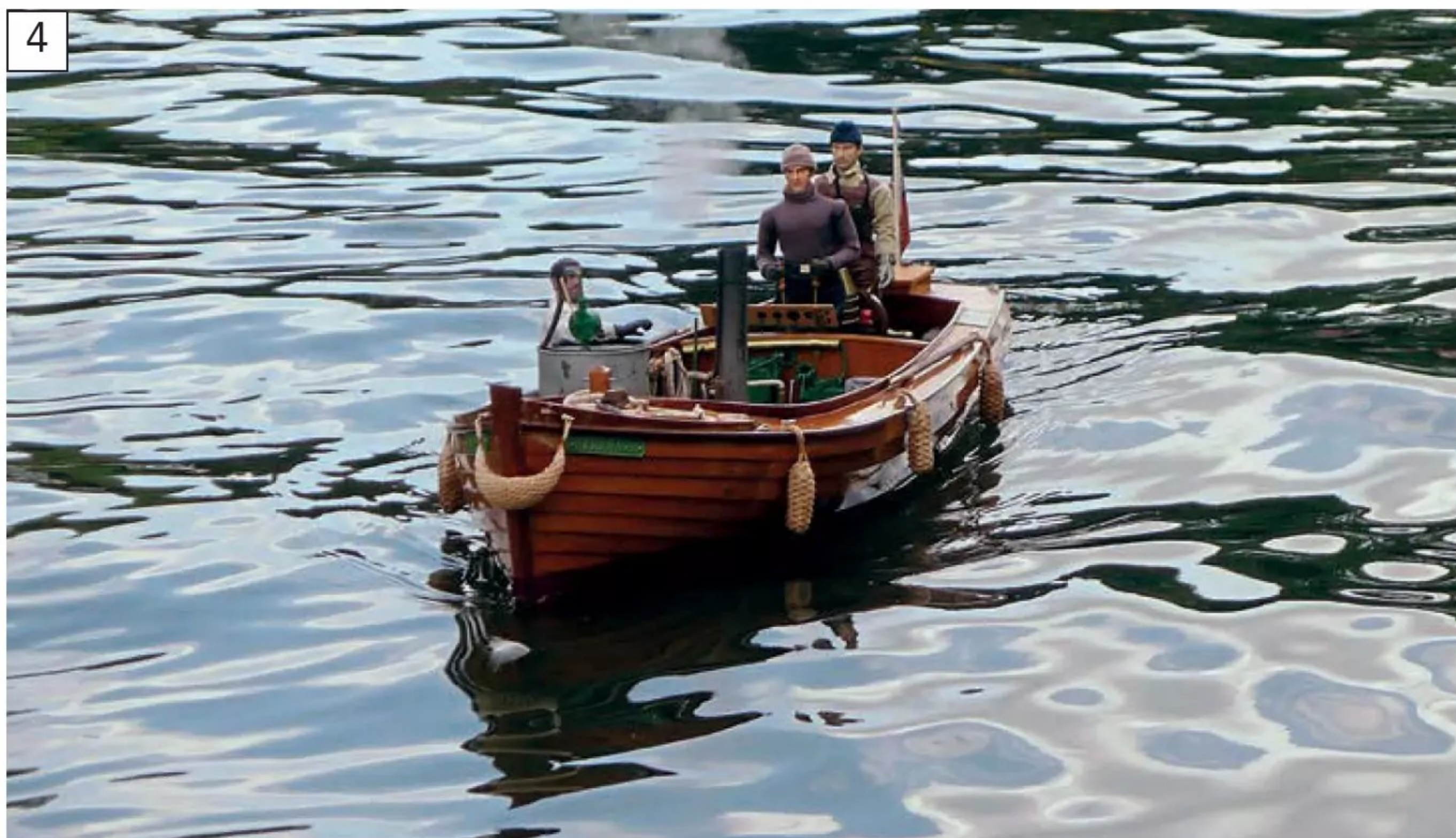
Initial trials went well, with everything working as it should, apart from when, on a couple of occasions, a screw became loose, resulting in the engine locking up. Fortunately, Richard was able to rectify the situation at the pondside.
