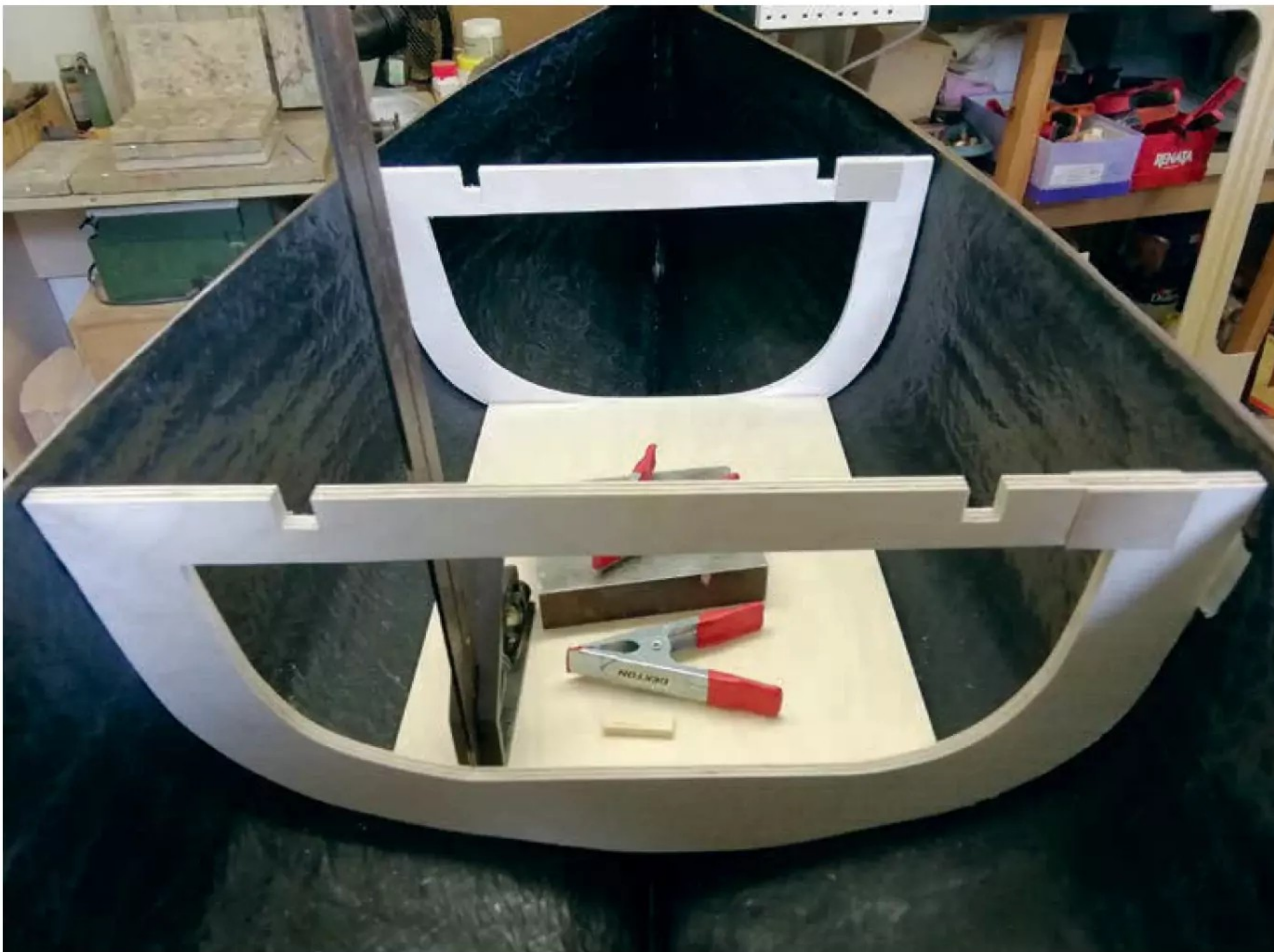
The robust nature of the Orion hull meant only two bulkheads, with a platform between them, were necessary. This 'platform' would accommodate the two large lead acid batteries. Only one of these batteries would be used at any one time, the second being used for ballast. Even with the batteries located, however, more ballast would be required.
