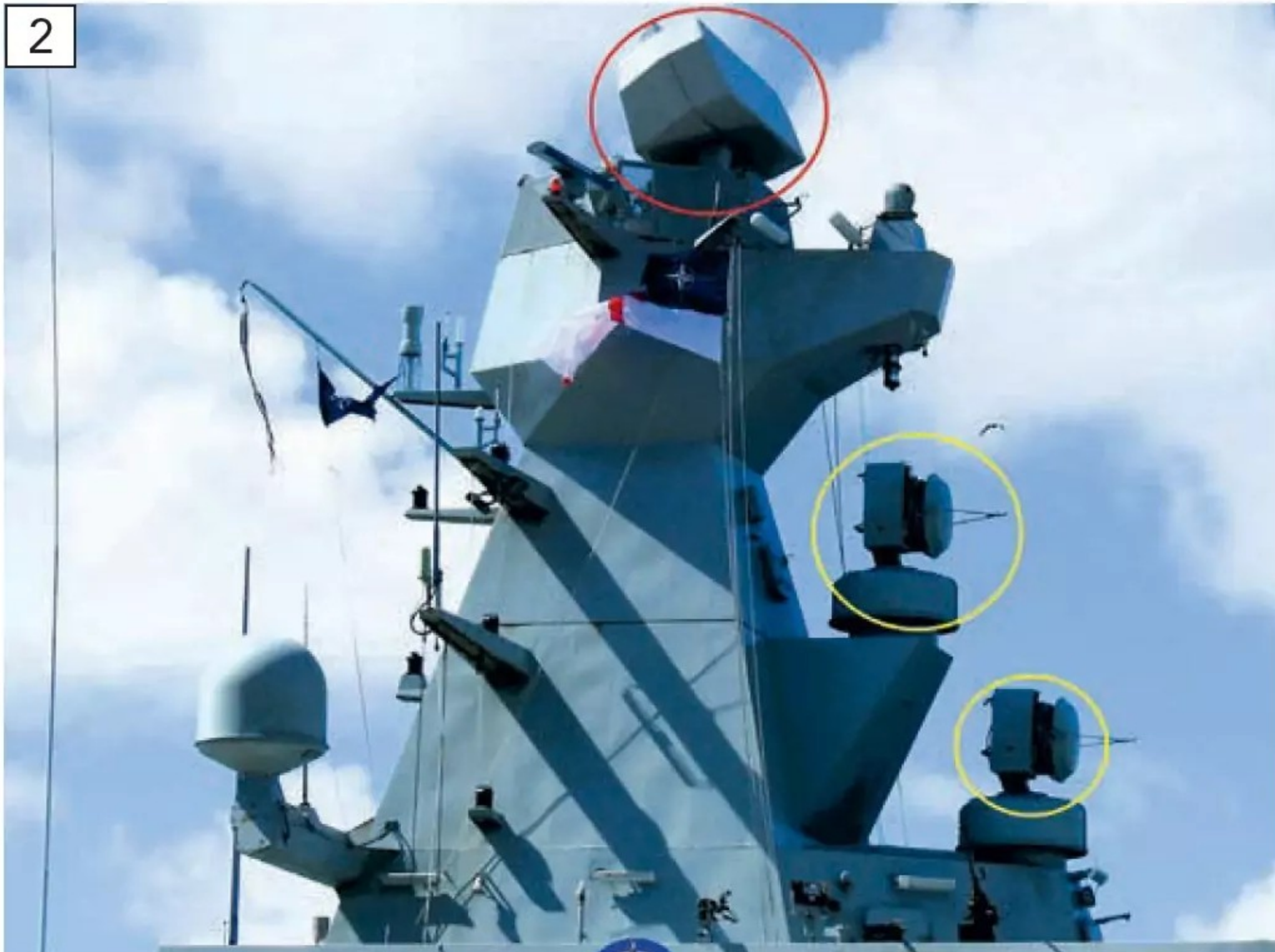
A detailed shot of the forward tower, highlighting the air search and fire control radars.
