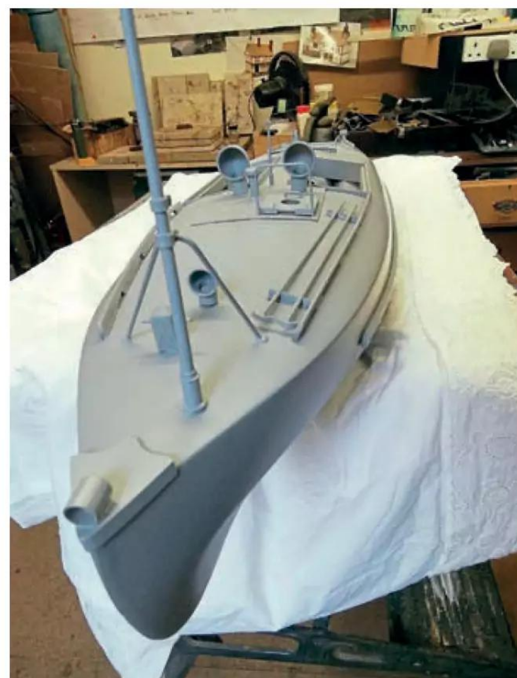
In this bow shot, details are starting to be added. The first coats of Halford's grey primer have been applied. It will take six coats of paint to produce a reasonable finish, followed by a coat of protecting matt lacquer.
