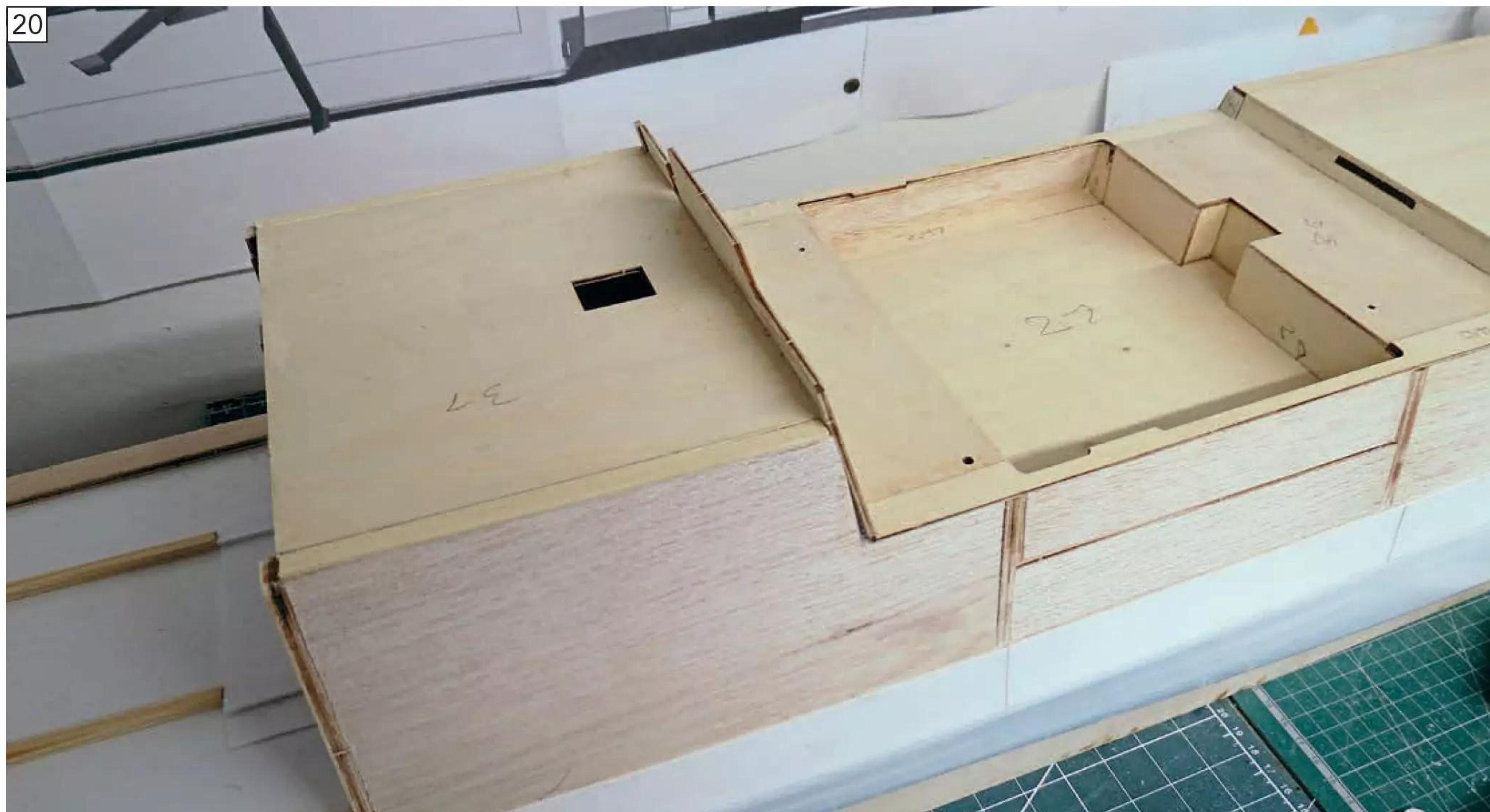
Balsa sheet fitted into the open side panels of the fixed frame to add strength and provide a greater surface area to affix the outer ply sheets to.
