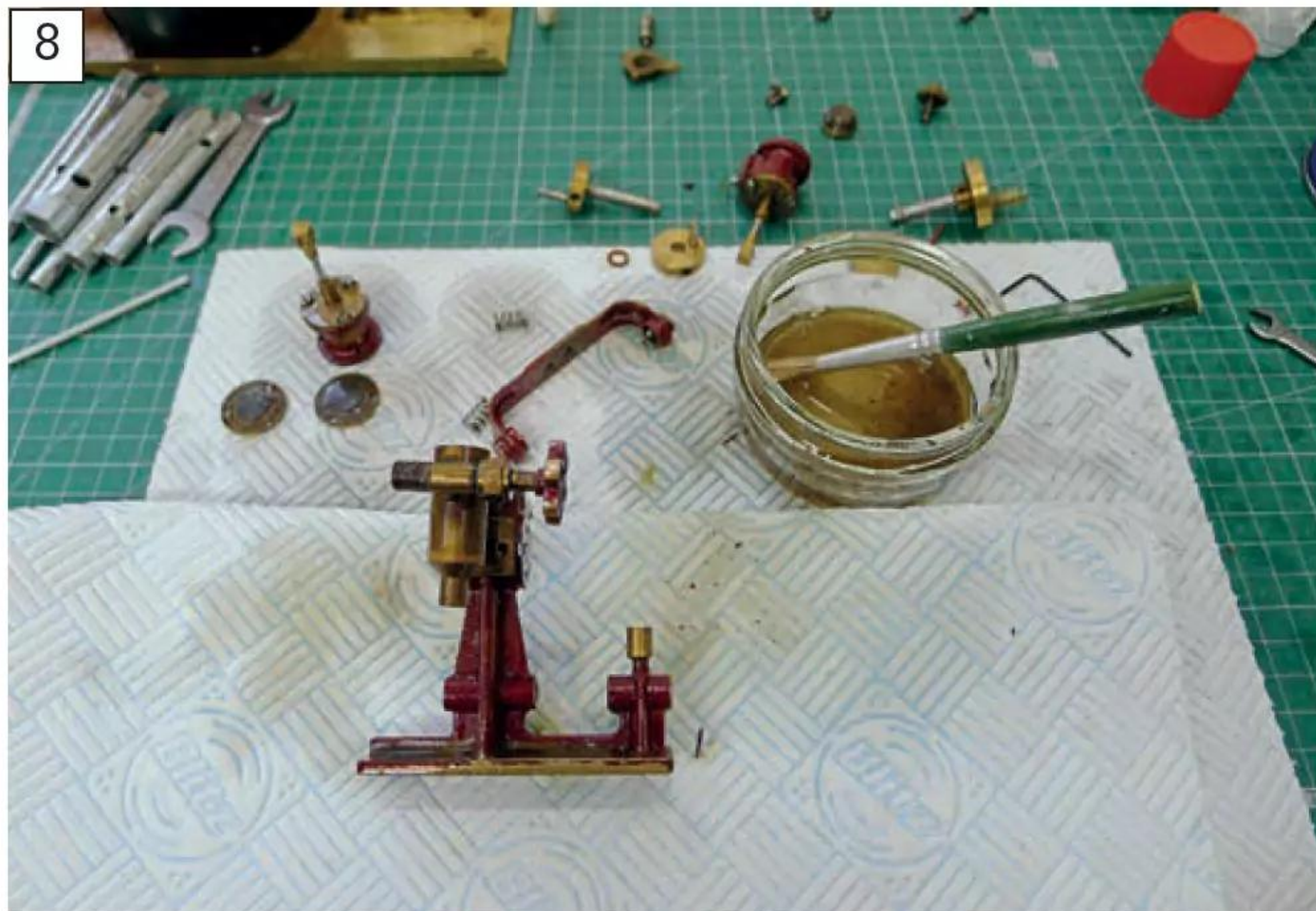
WD 40 can easily be decanted into a dish so that parts can be soaked in it and washed down with a stiff brush. It makes a great degreaser and general cleaner while at the same time not harming your seals or paintwork.
