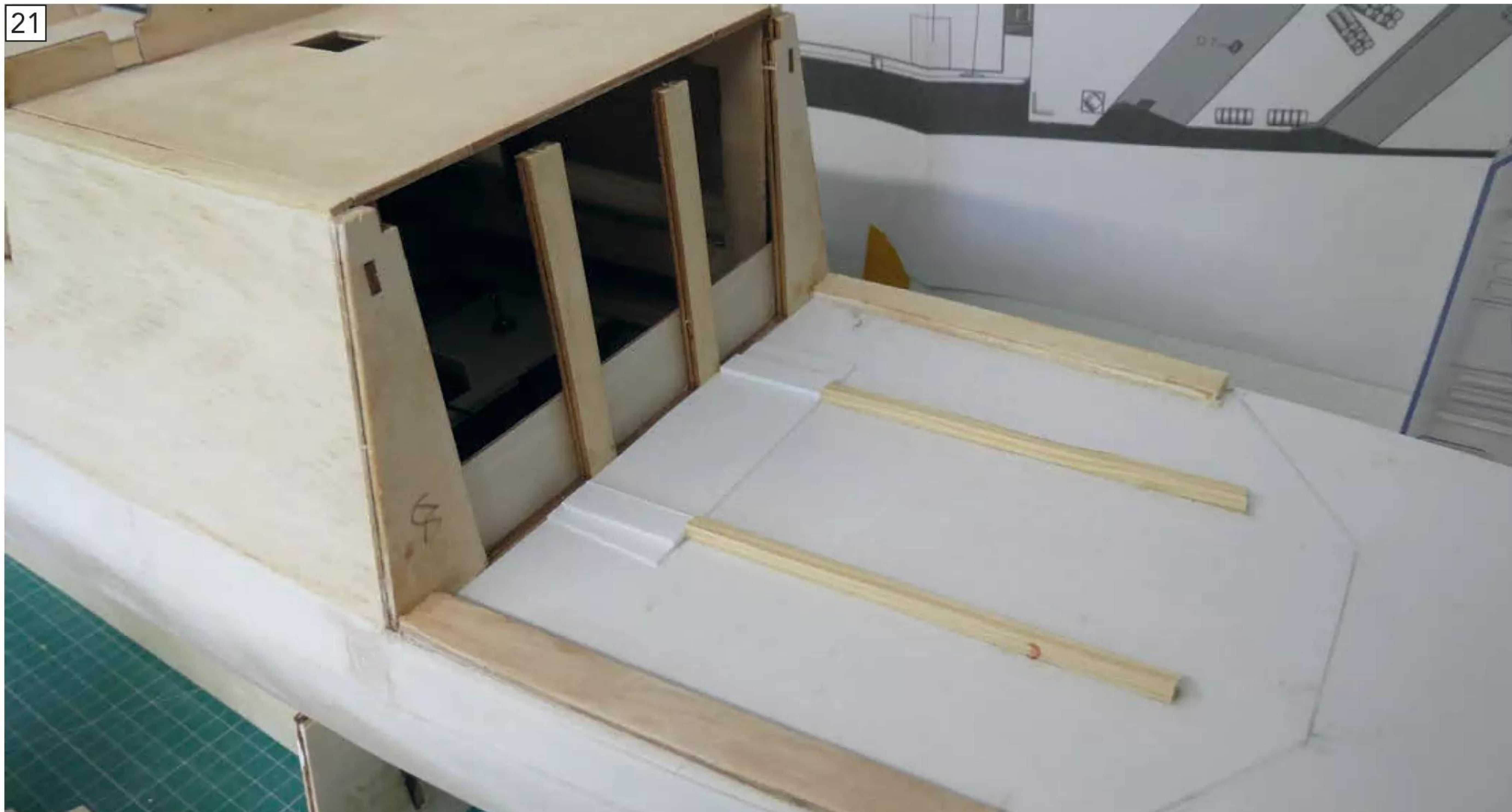
As an aid to accuracy in locating and fixing the bridge assembly timber guide, strips are added.
