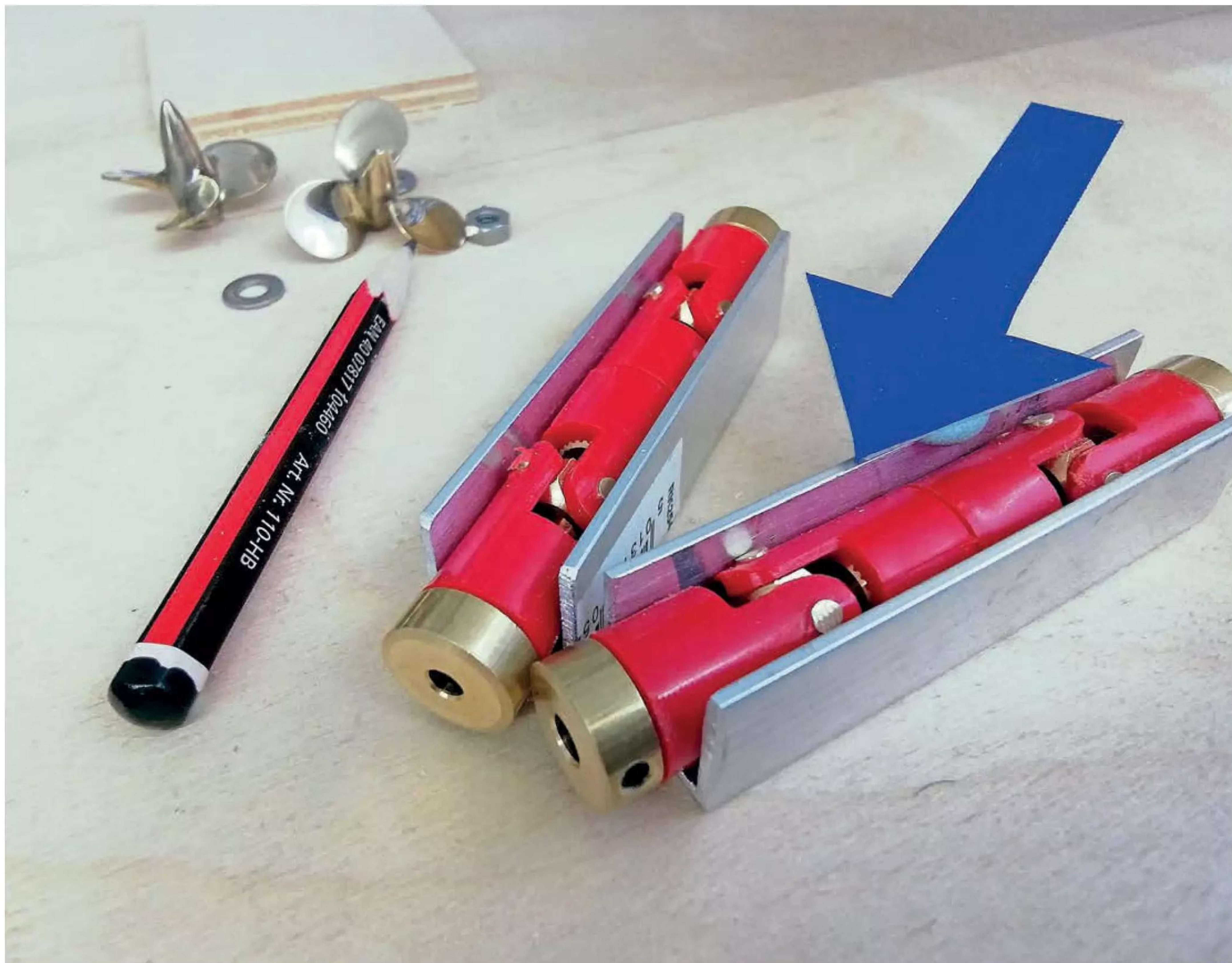
Using aluminium channel from Wickes, John's universal joints are held firmly in line while setting up the motors. Once in place, the channel can then easily be removed.
