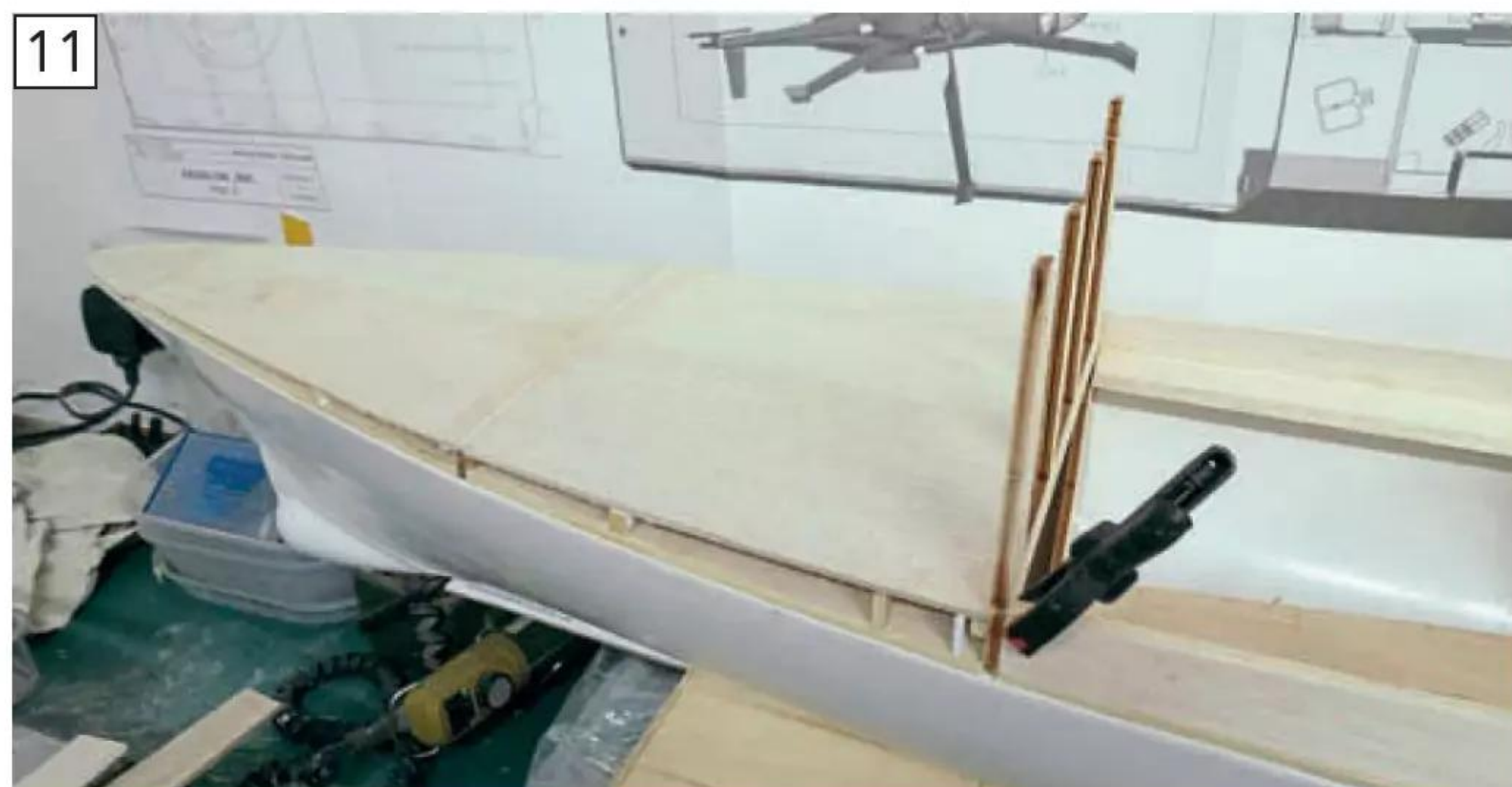
The balsa forecastle deck is raised above the knuckle so as to marry with the top of the balsa side deck edge panel.
