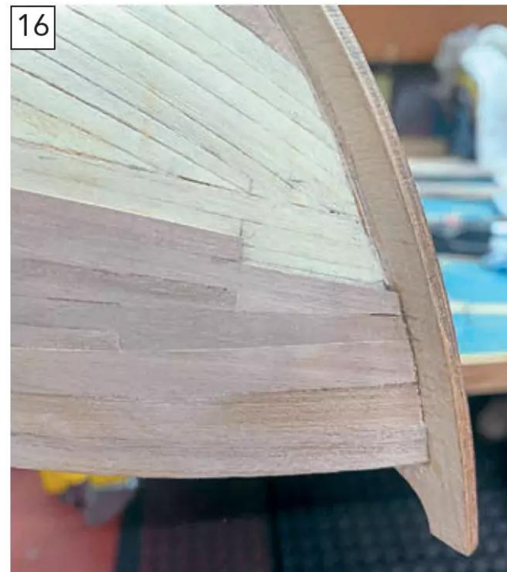
The third and final layer of planking being installed over the middle layer.
