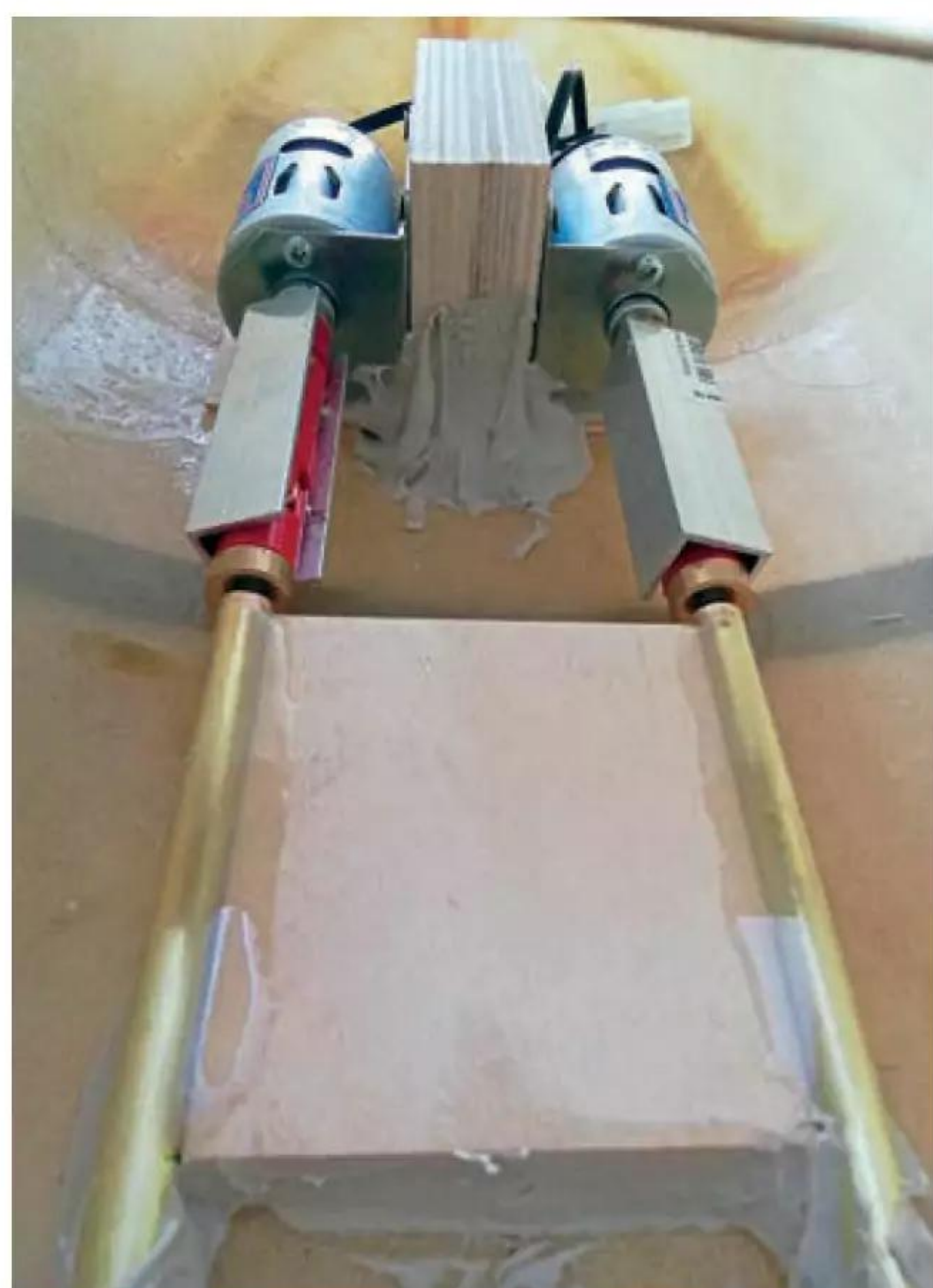
The two motors bonded into the hull. The aluminium channel can be clearly seen. The propeller shafts are firmly glued to a plywood 'plate', which in turn is bonded to the hull on pads of P38.
