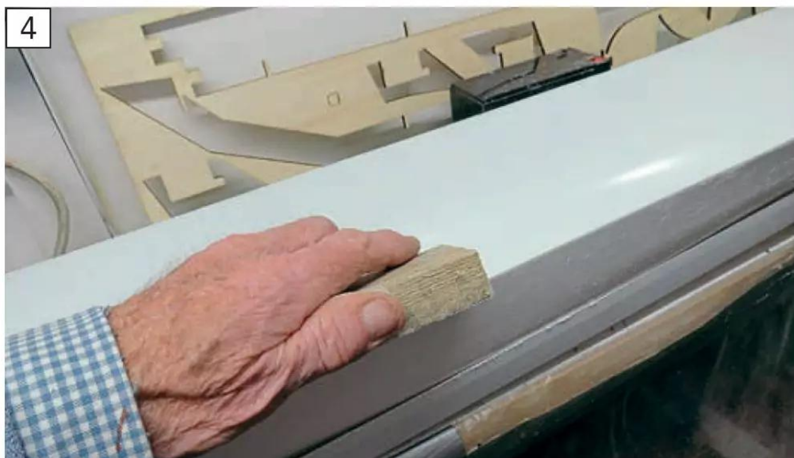
Preparing the ABS hull by removing unwanted material from the knuckle line.
