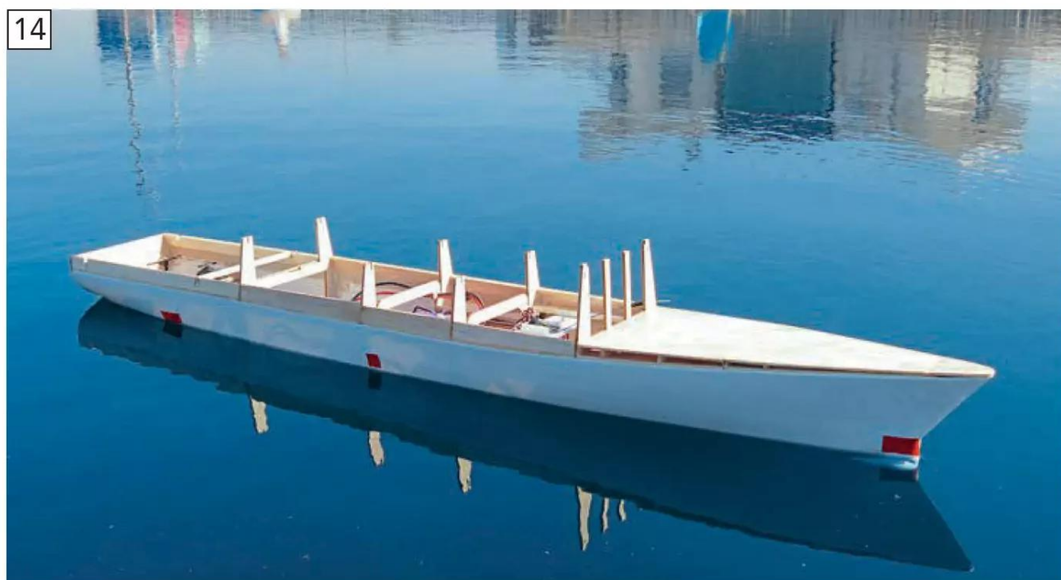
Using tape to indicate the waterline for ballasting.
