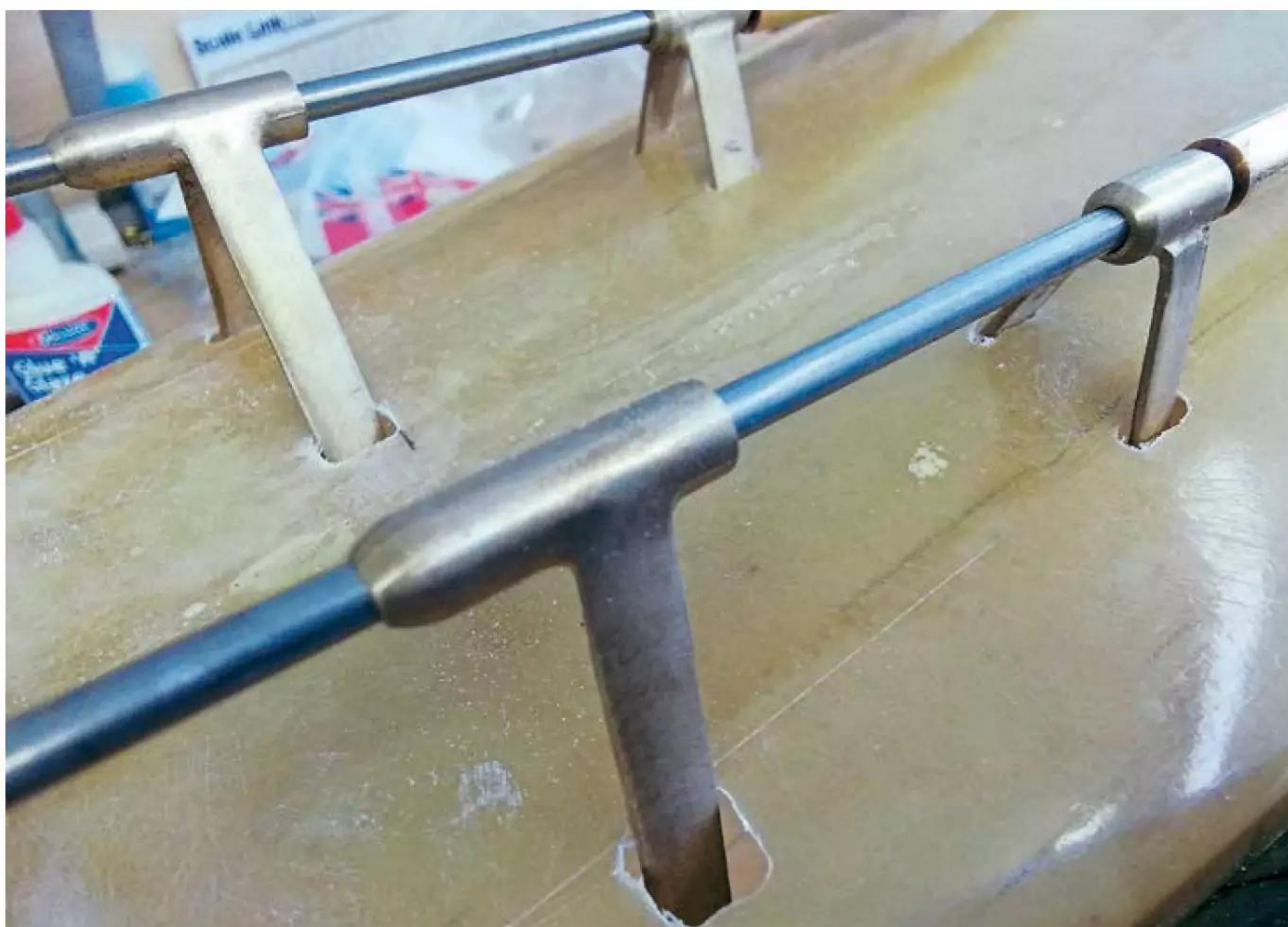
Setting up the propeller shaft external rear mounts. The bracket legs pass through slots in the hull and are bonded in place inside it using P38.
