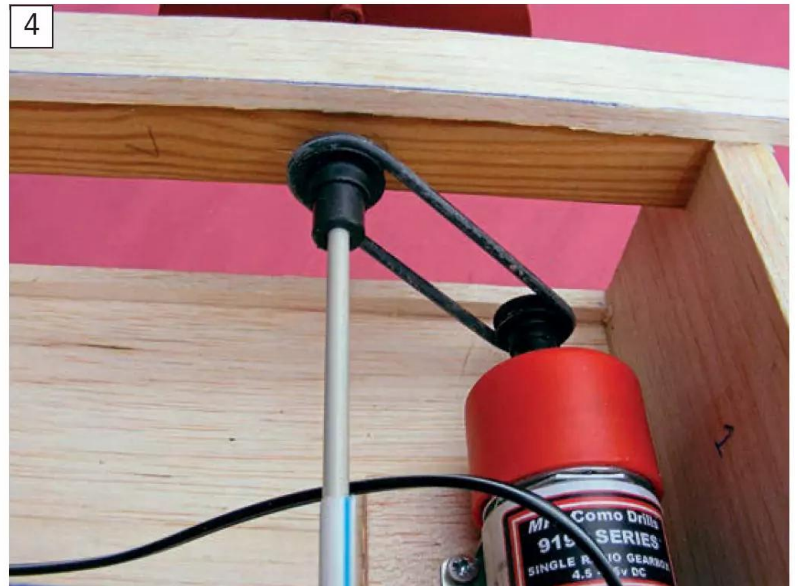
A pulley drive adjusted for correct belt tension.
