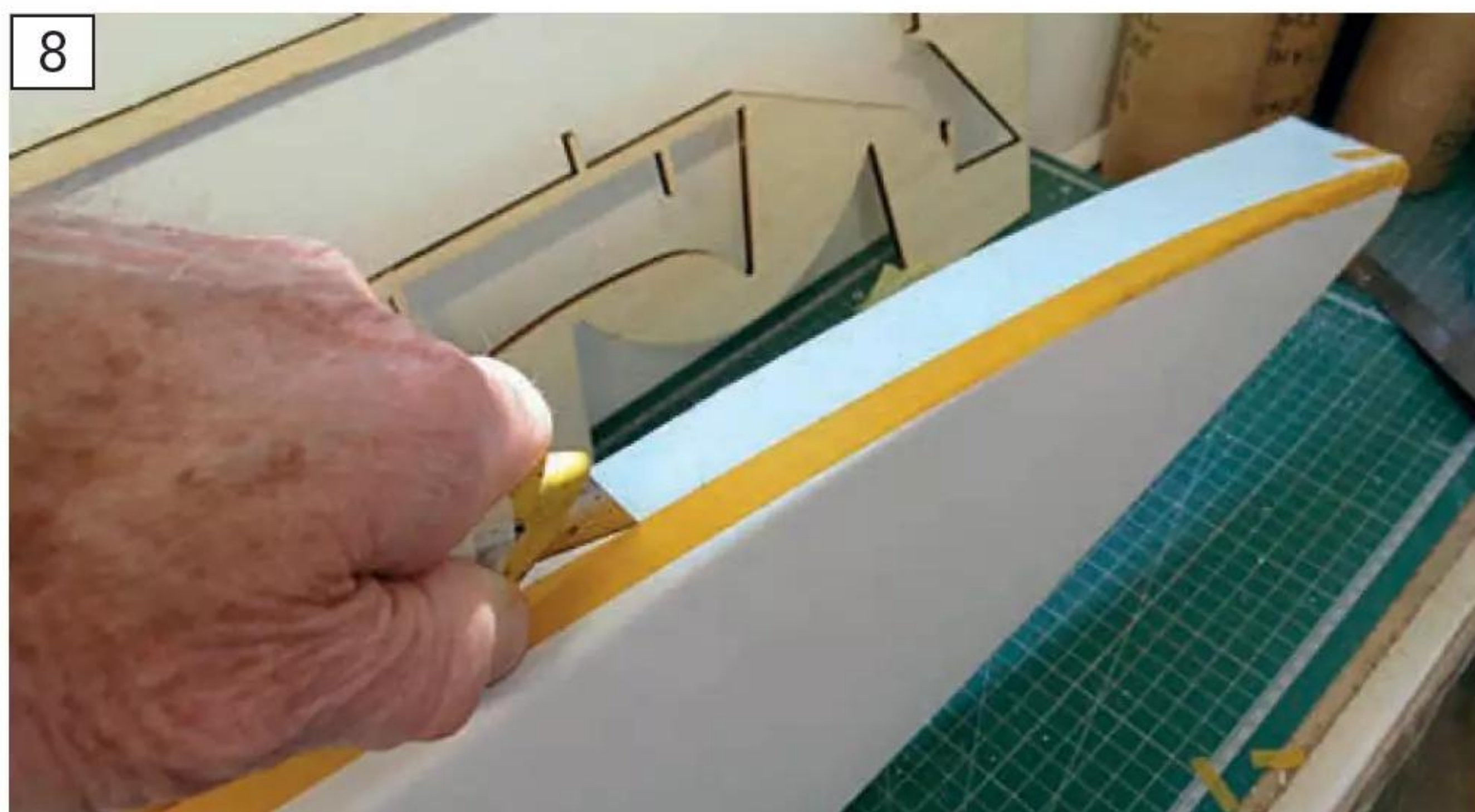
Preparing the ABS deck assembly for removal of unwanted material.
