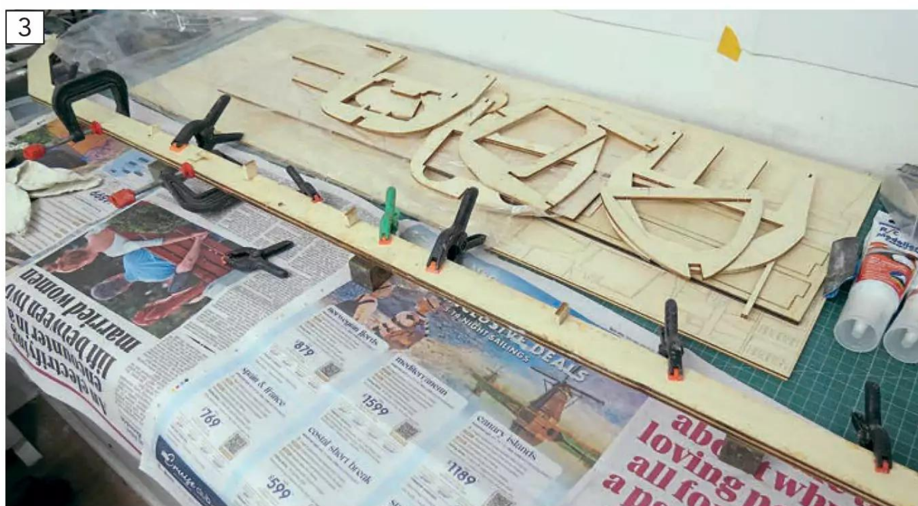
Commencing assembly of the keelson.
