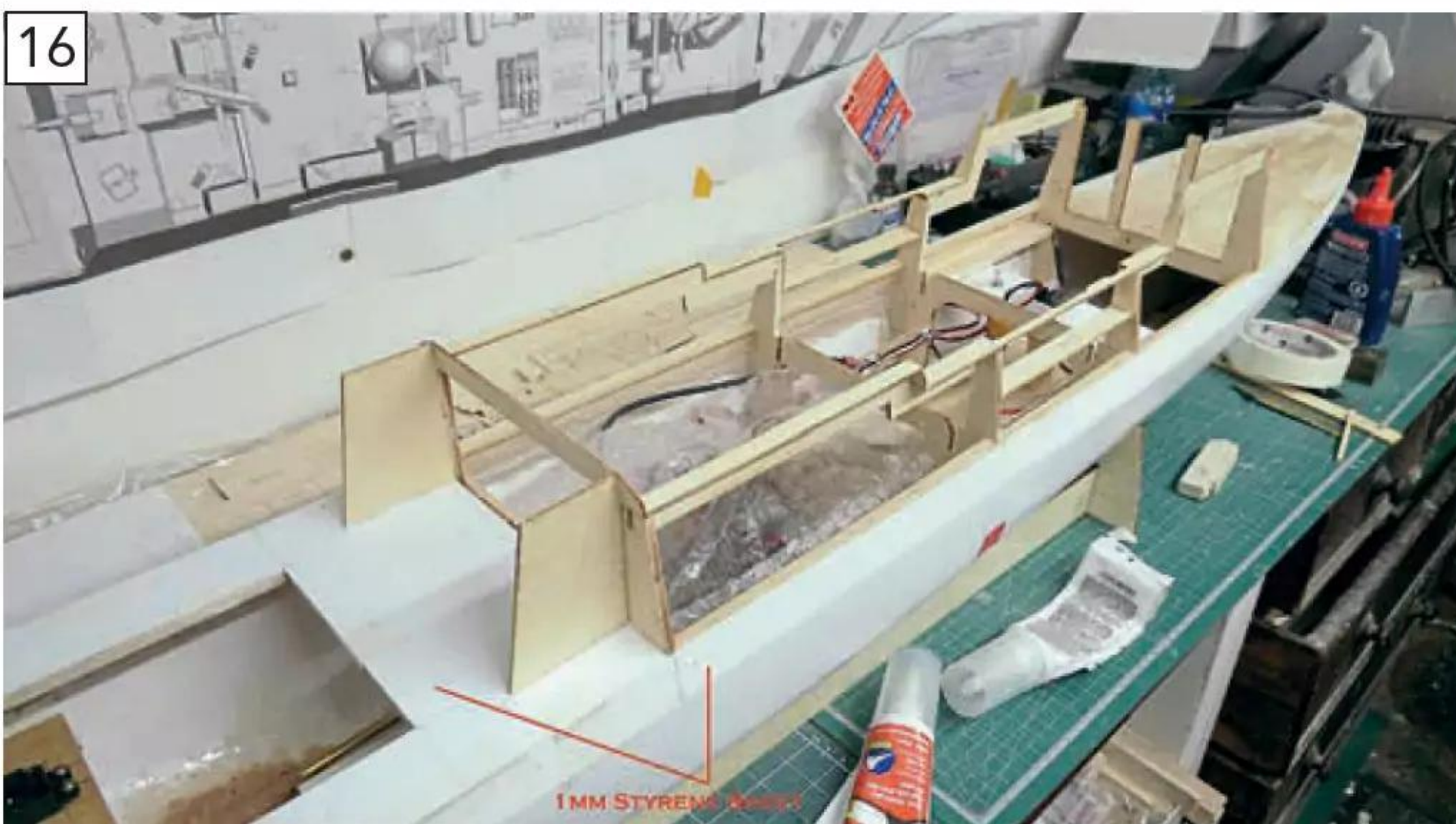
Building up the internal fixed framework.
