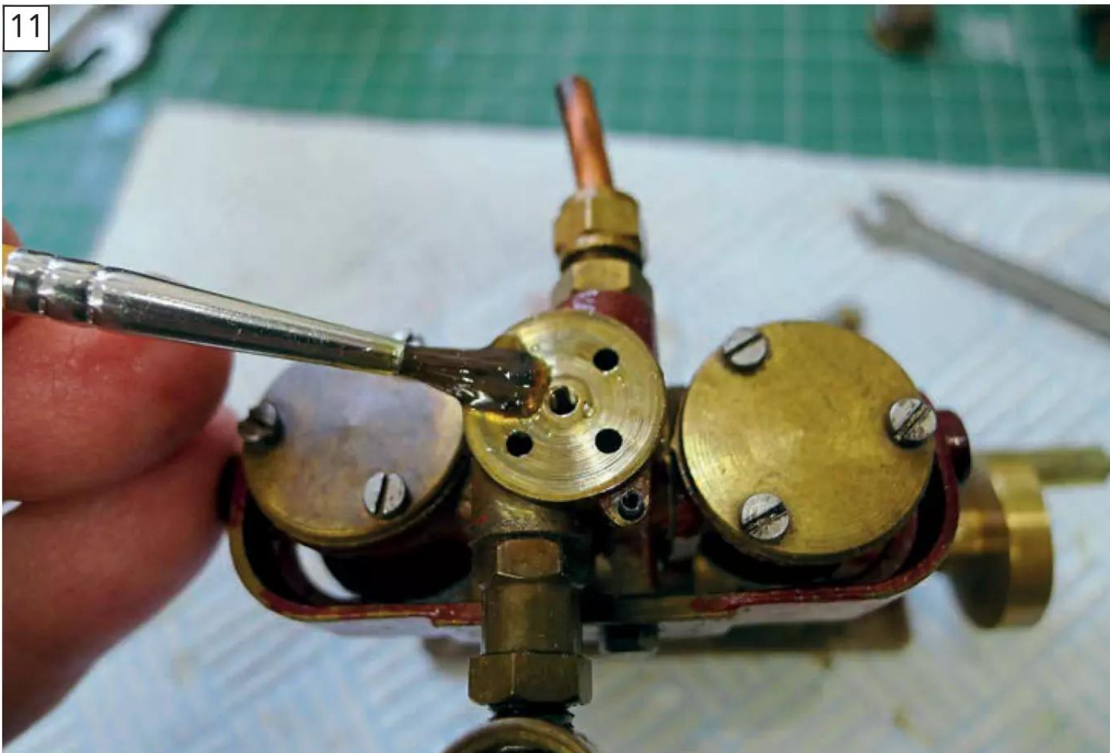
Universal Steam Oil easily paints on with a soft brush and was noted as being nice and sticky on the port faces, bearings and shafts.
