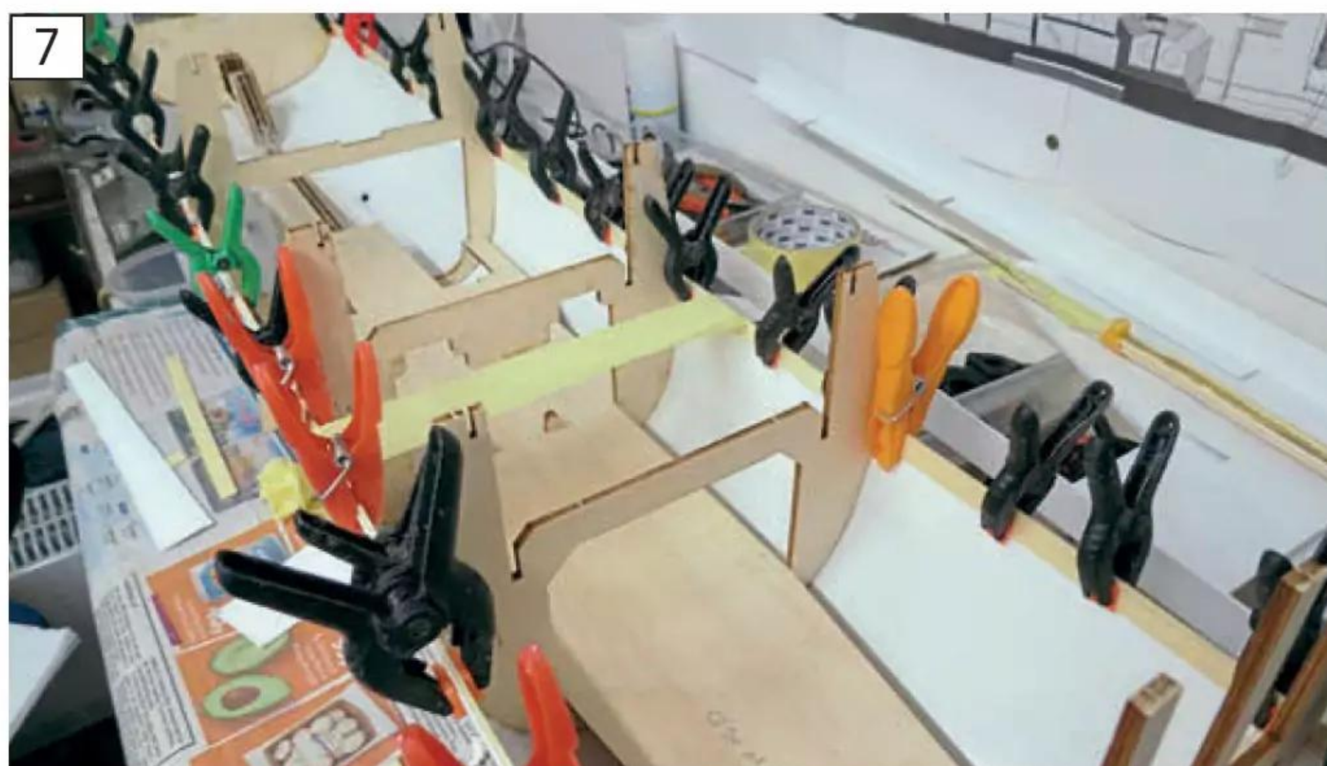
Installing the motor battery and ESC platform within the frame assembly.
