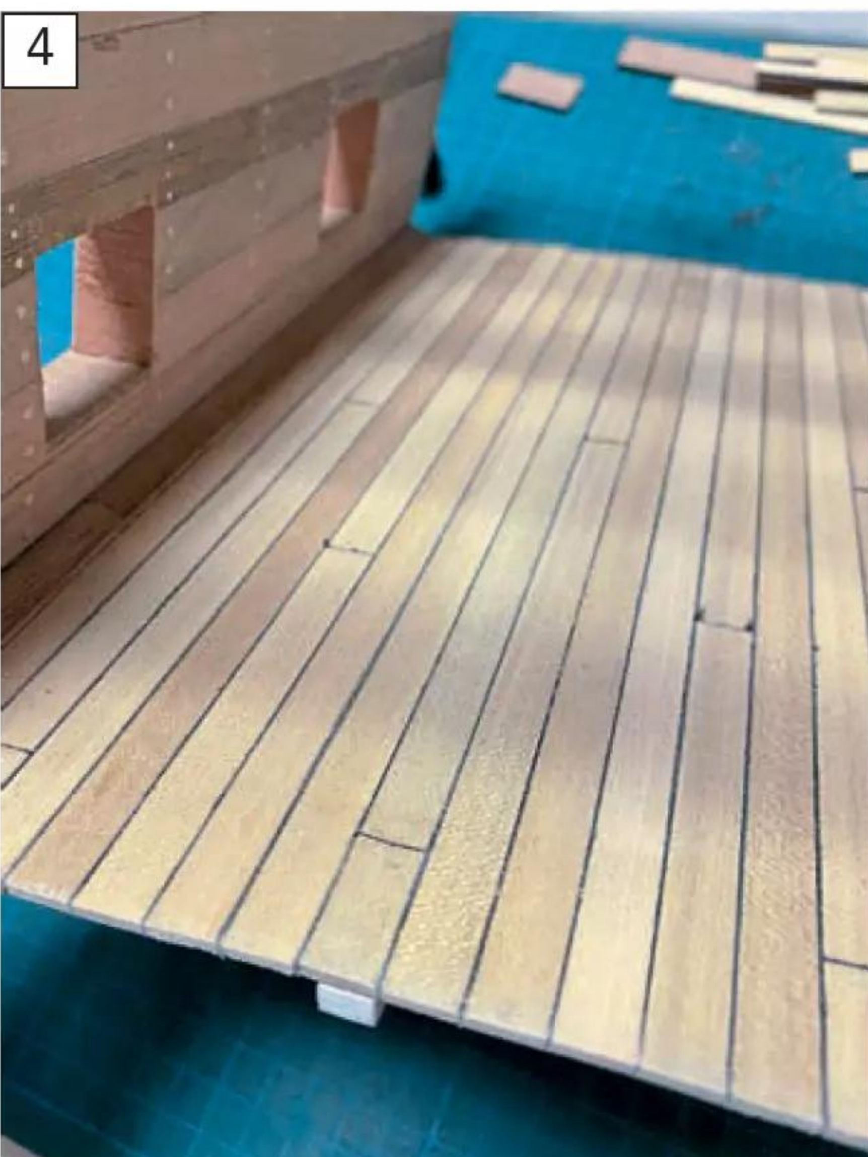
Deck planking installed. Note the black card caulking.
