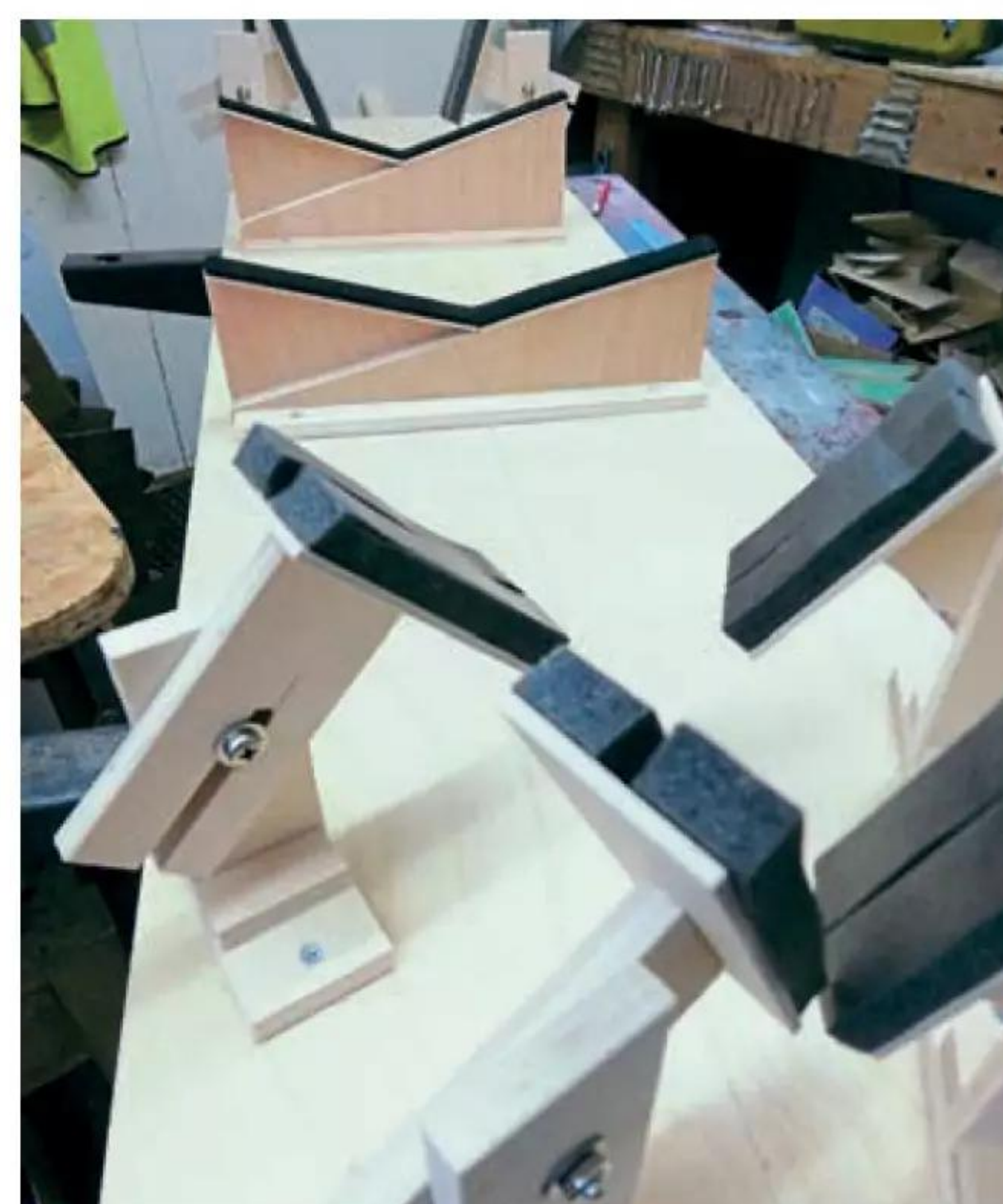
The first job was to construct the support /carrying stand. John has learnt from previous experience how important it is to make a good purpose-built stand.
