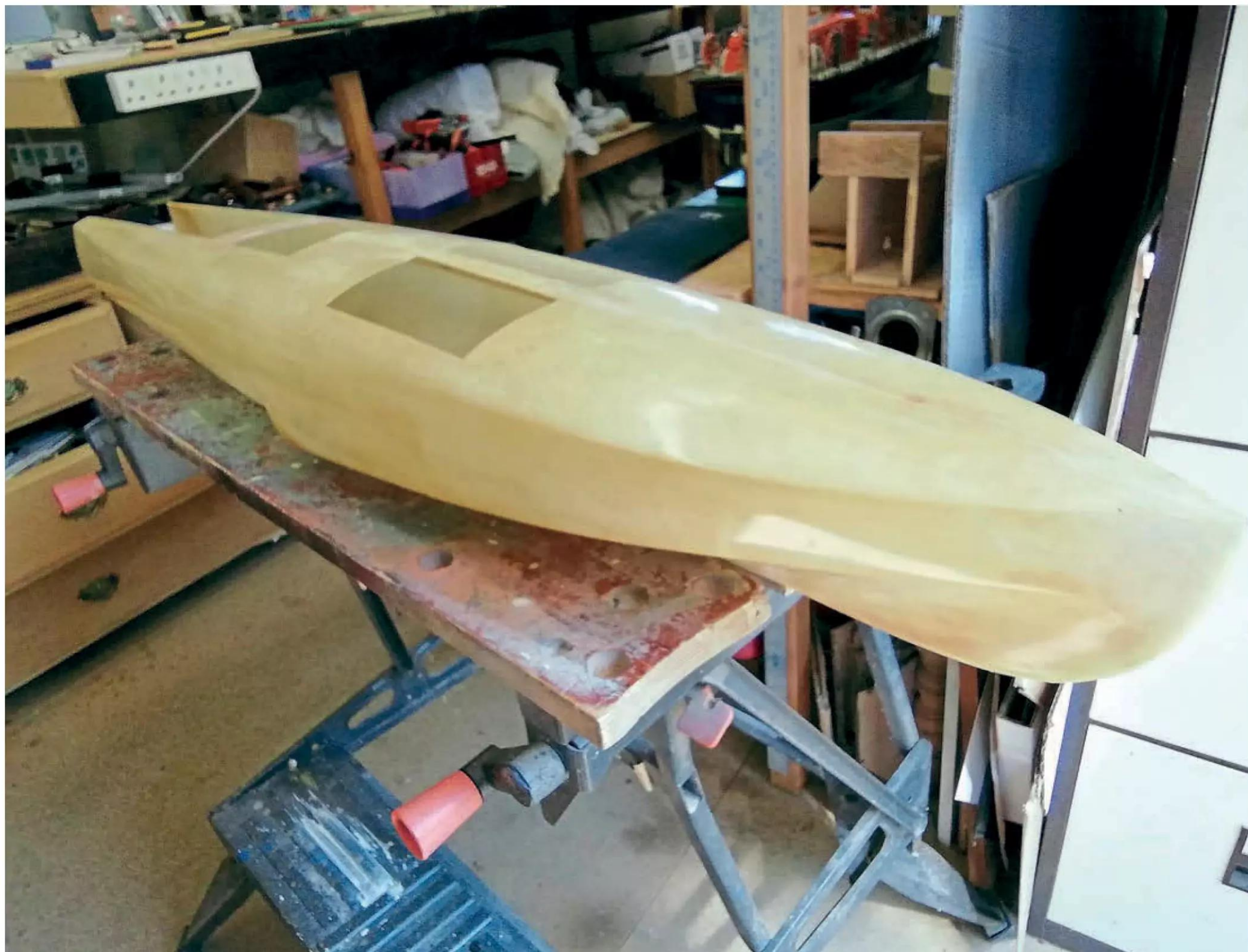
The glassfibre hull as purchased. The very fine surface finish can be seen in this photograph.
