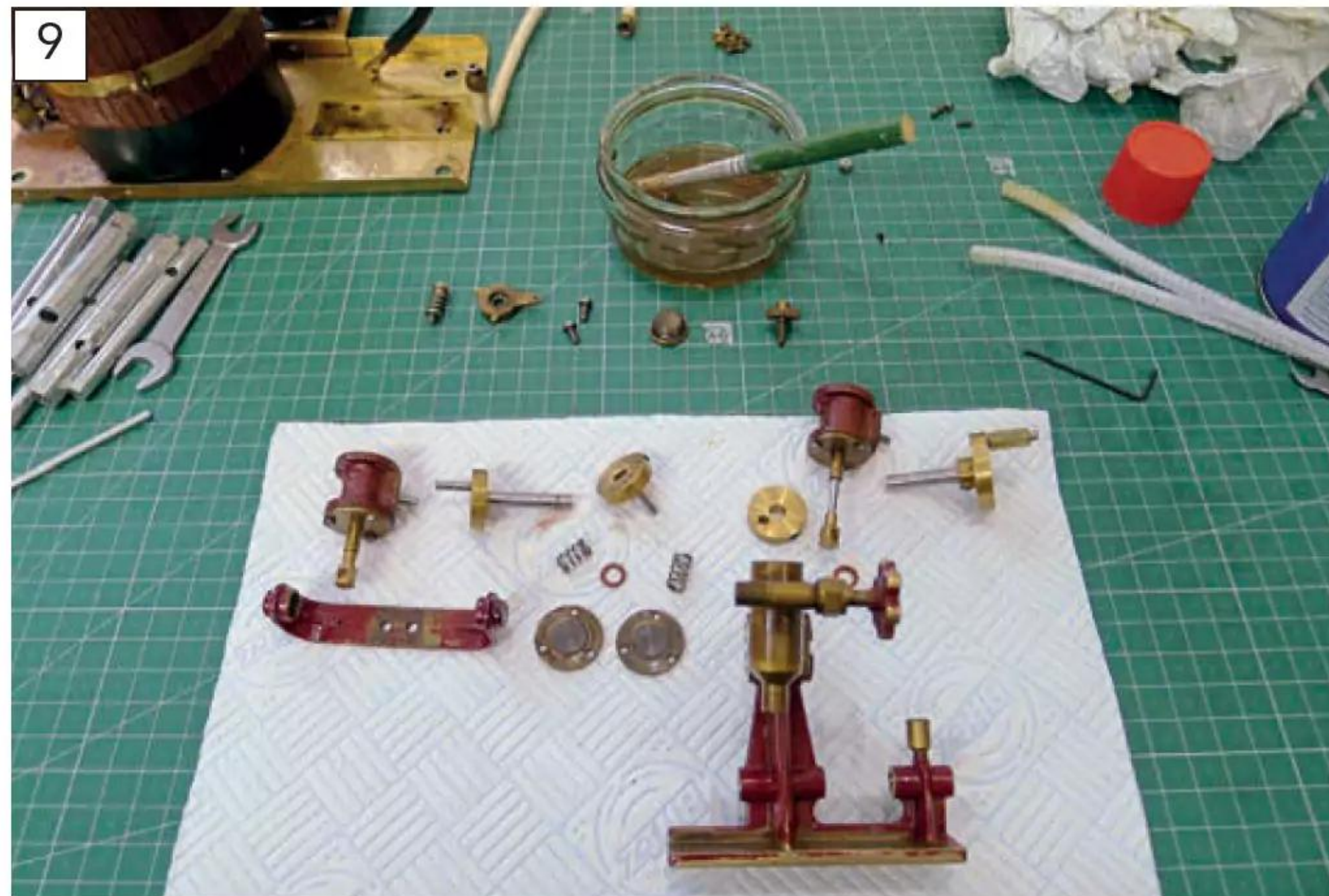
Once clean, everything was simply wiped down with kitchen roll (a lint free rag can also be used). Ports and bearings were also run through with pipe cleaners dipped into the WD 40, before being blown through with an airline.
