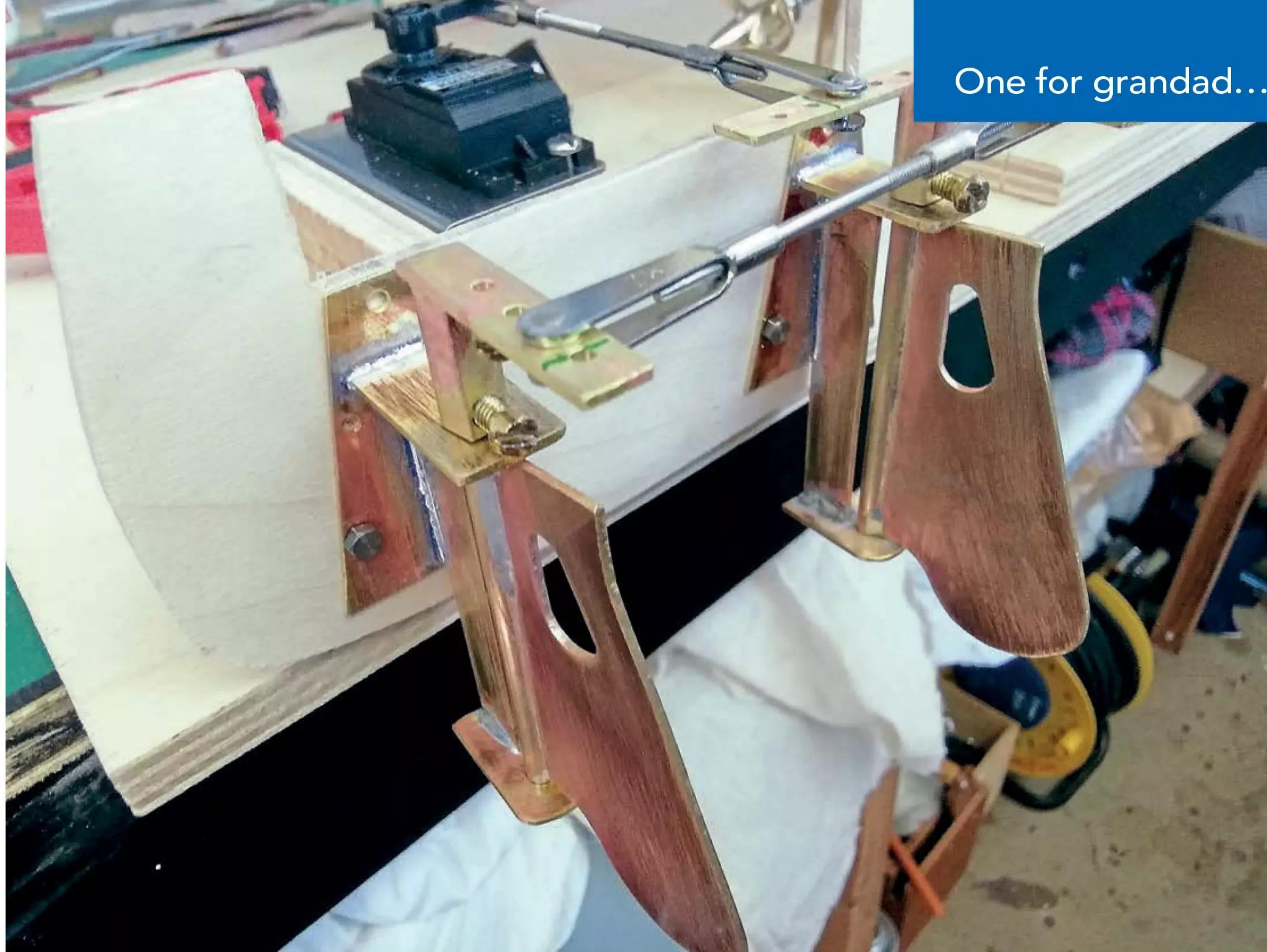
The twin rudder system. This was initially set up on the bench to ensure it worked properly.
