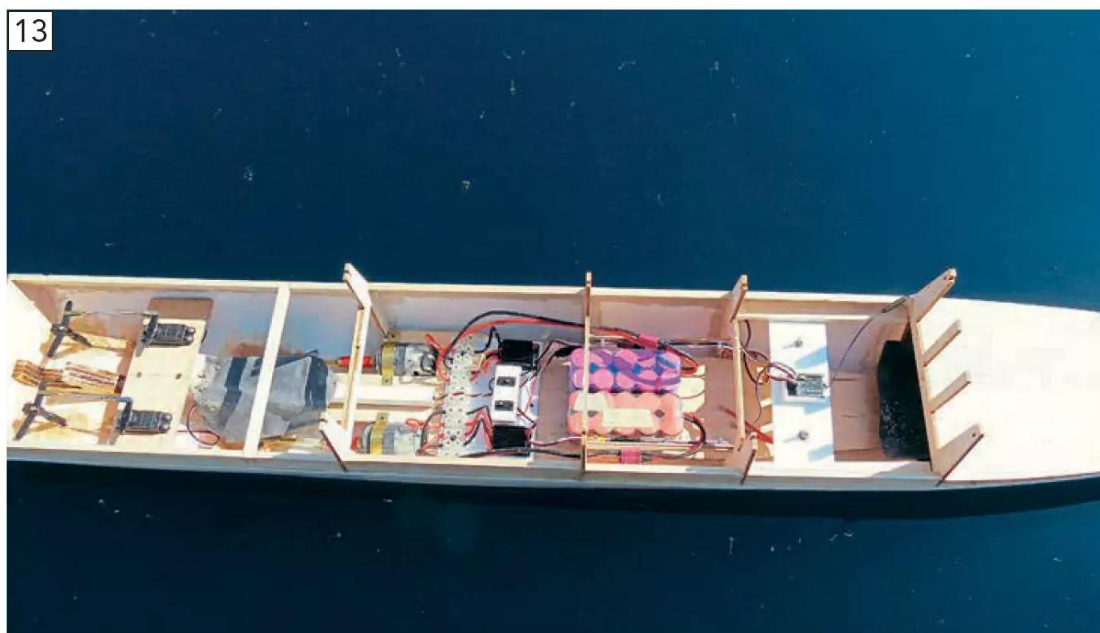
Installing the twin 12v packs of NiMHs, with temporary ballast weights added right forward and right aft.
