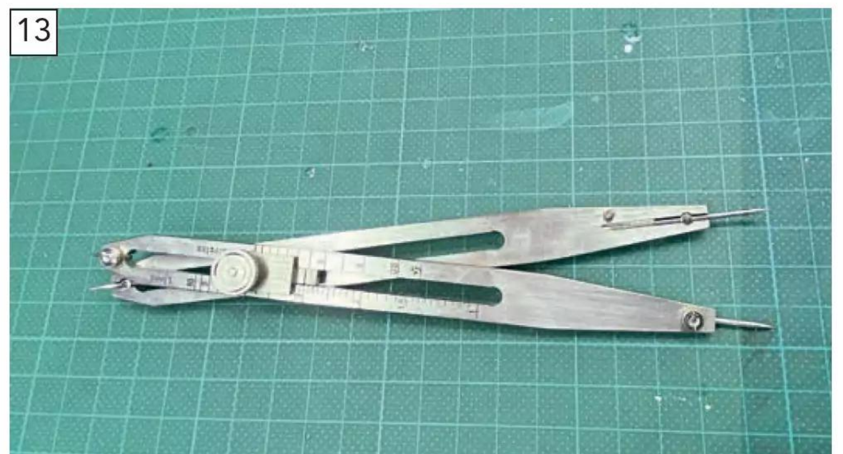
Proportional dividers: almost a 'must have' tool for accurately sizing and tapering hull planks.
