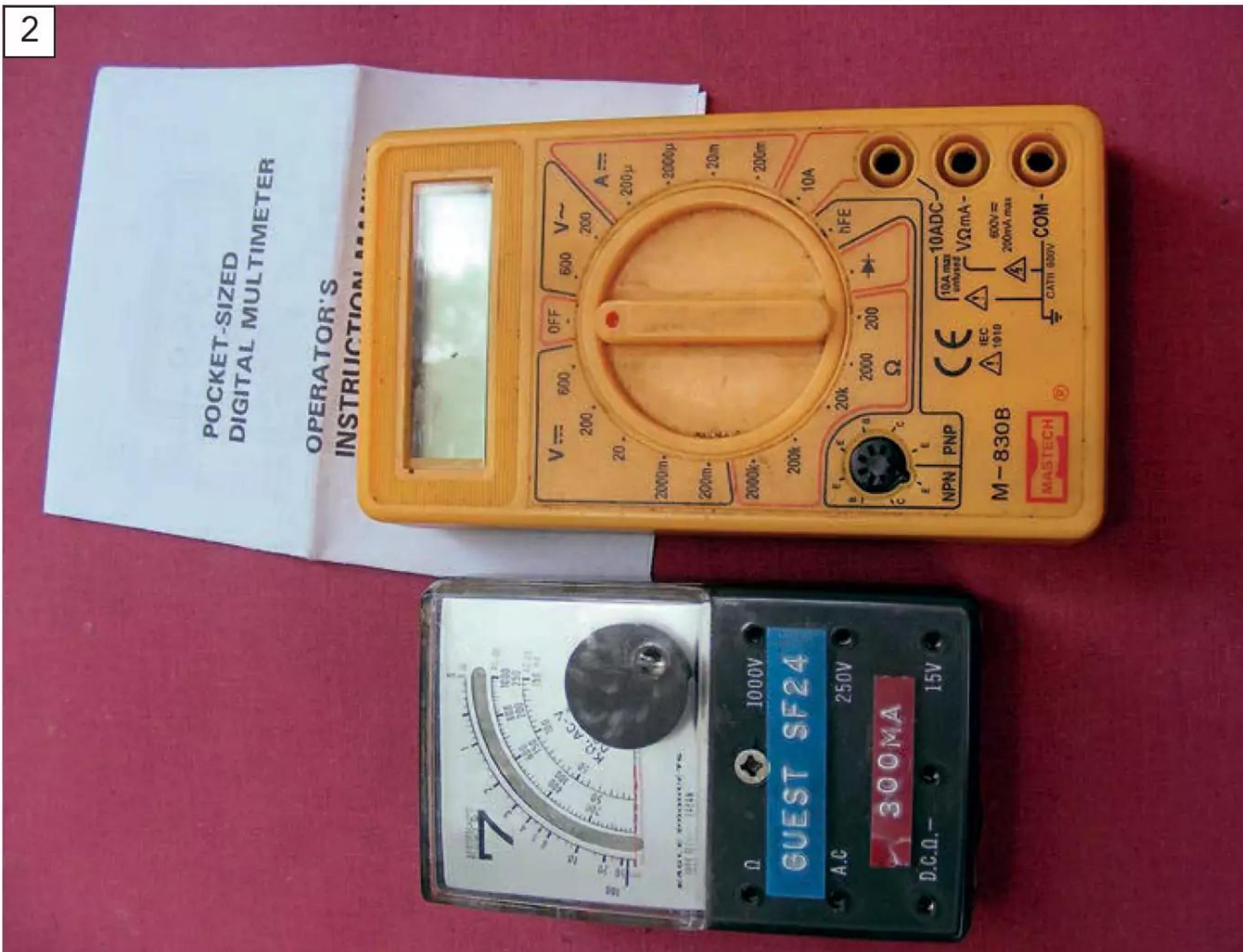
A handy small Multimeter, but it cannot measure currents greater than 300mA.
