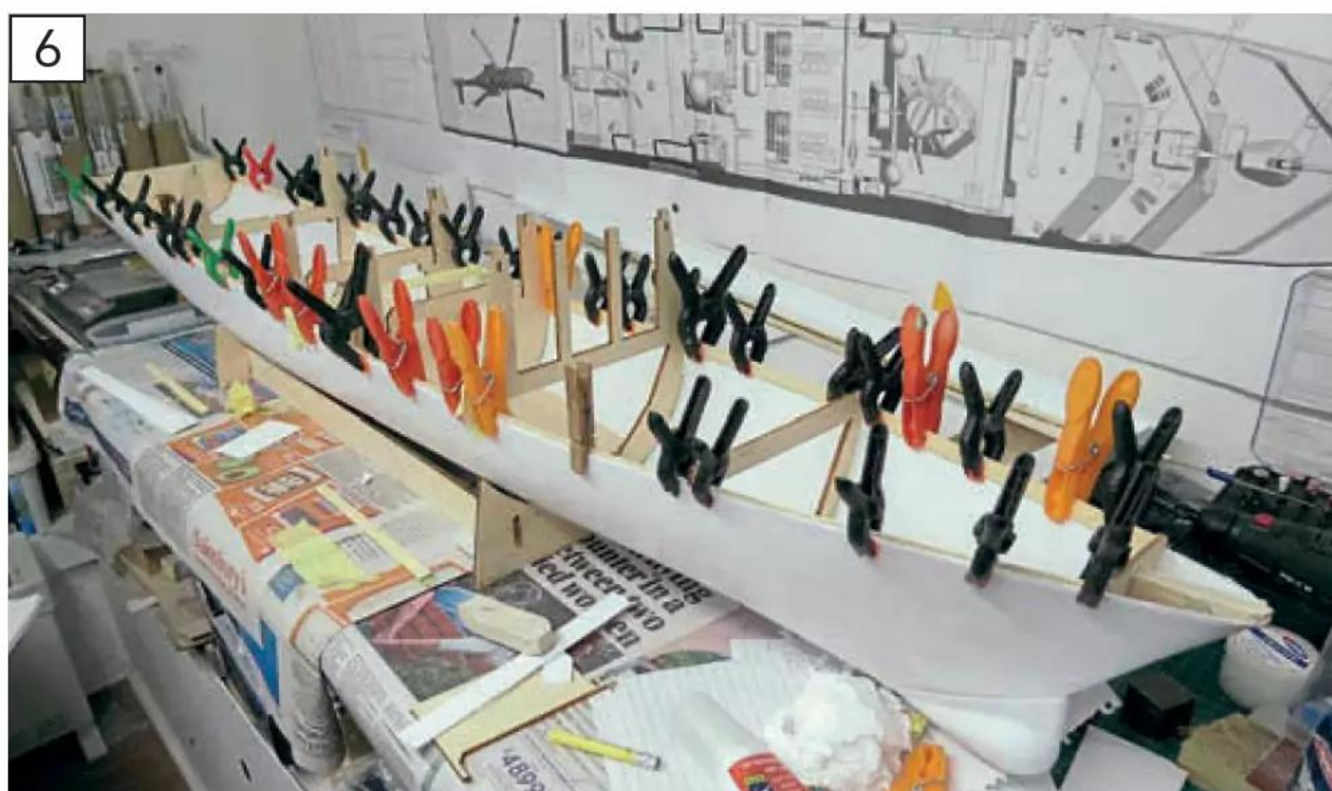
Locating and fixing strips of timber to the inside of the knuckle line.
