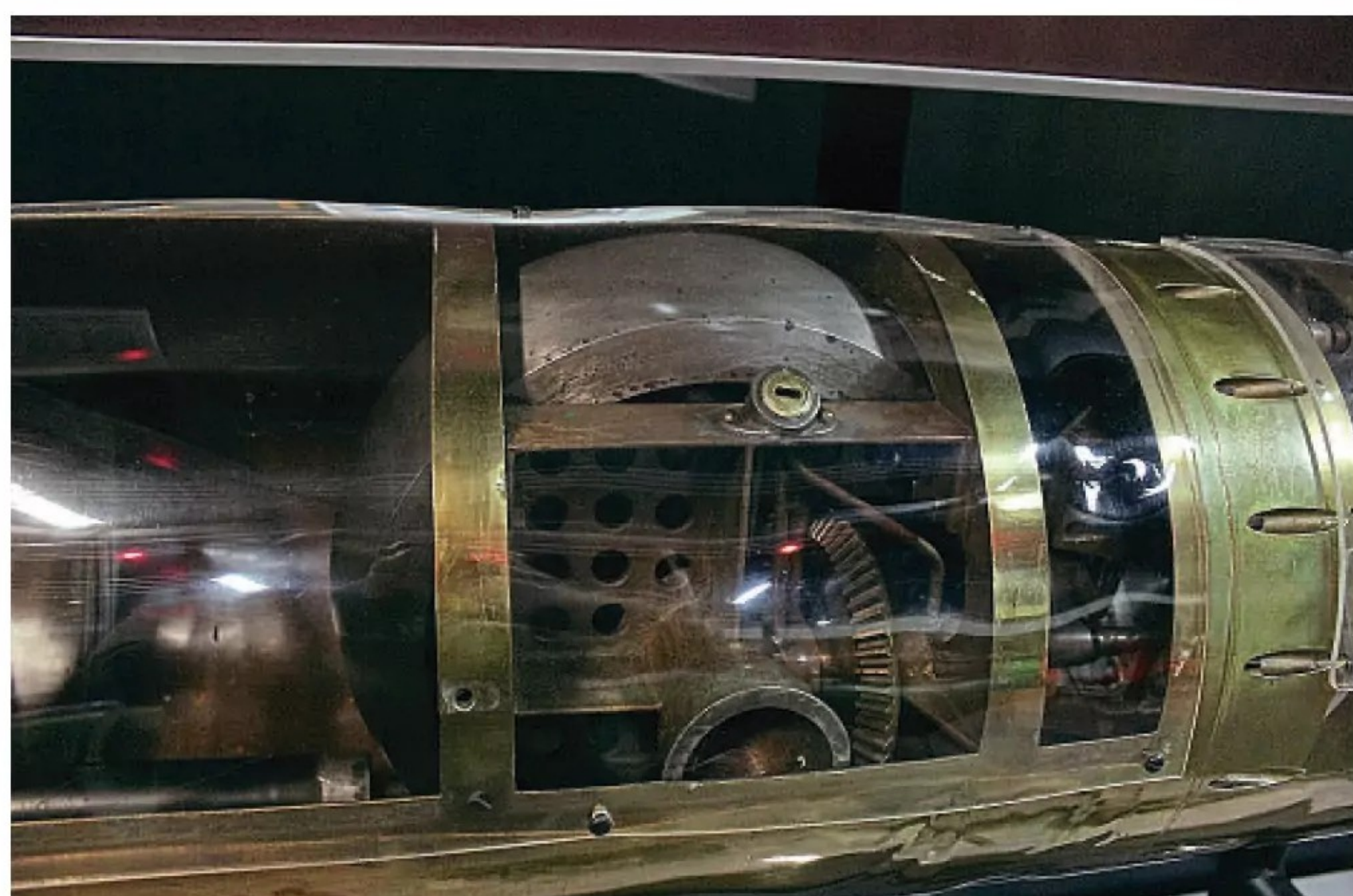
The flywheel of a Howell torpedo.
