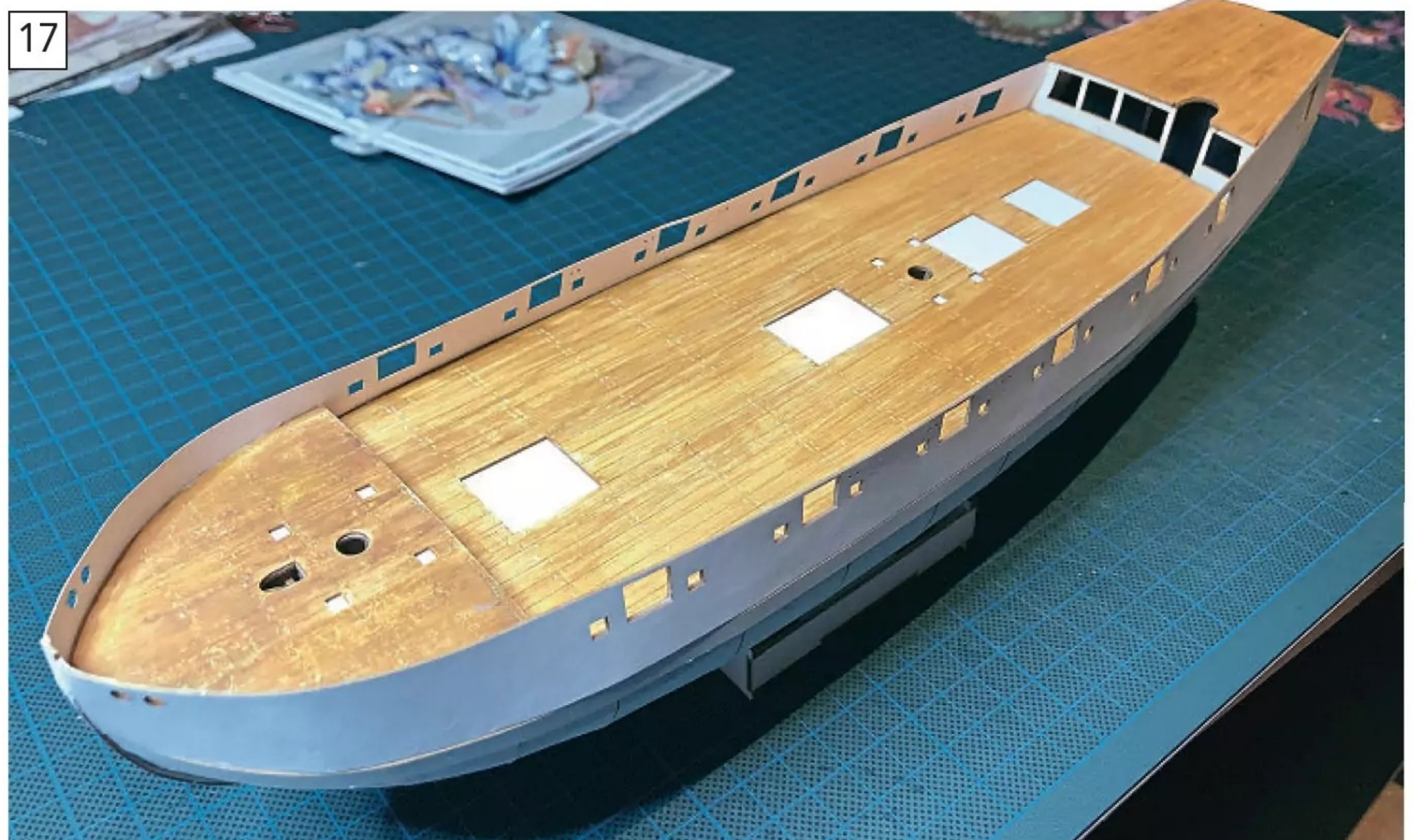
The first layer for the hull consists of pre-shaped sheets of card.
