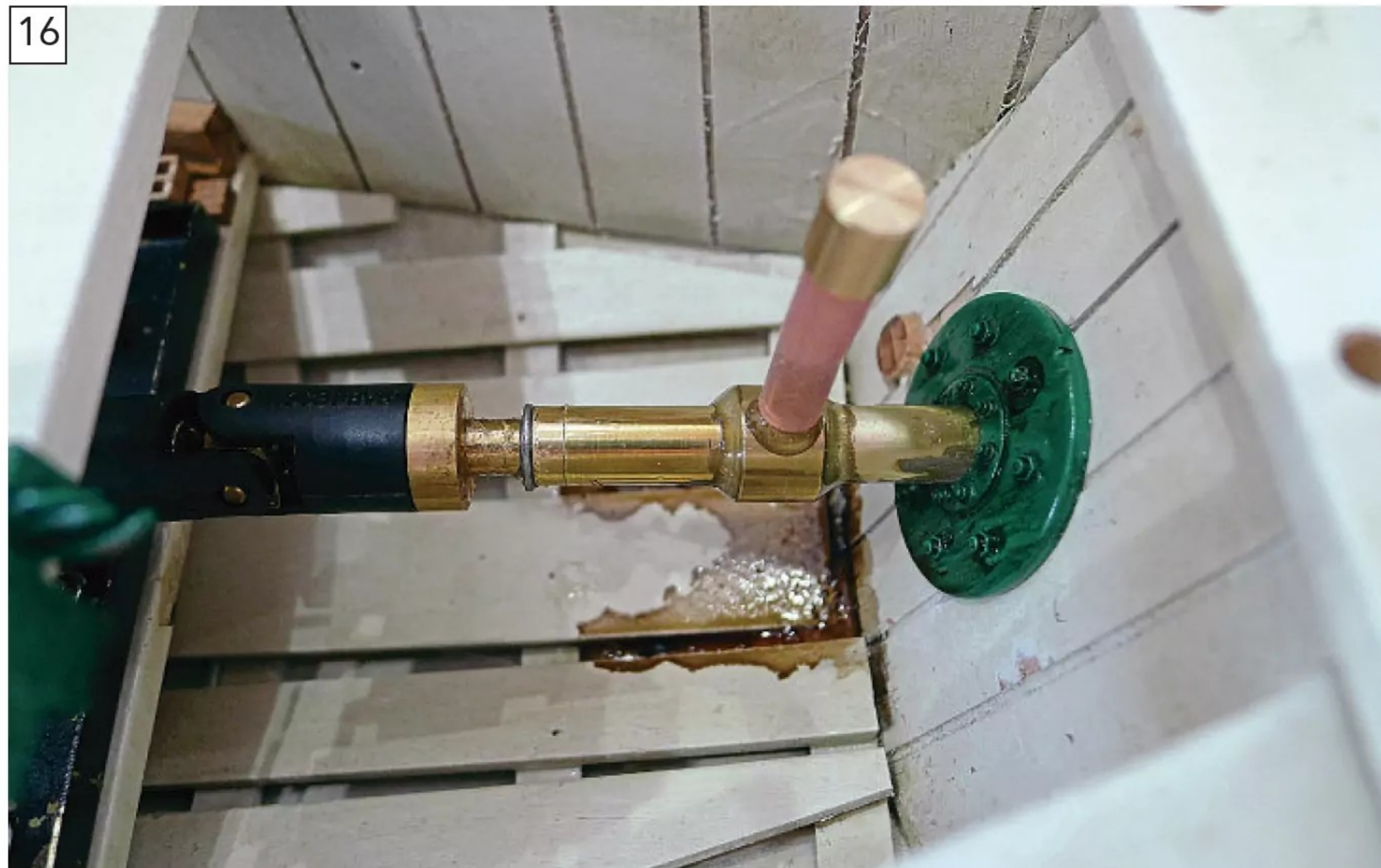
If a huco type coupling is used it's so much easier if the splines simply slide apart. Unfortunately, nowadays many are quite tight, but the all-metal type usually slide apart a lot easier.
