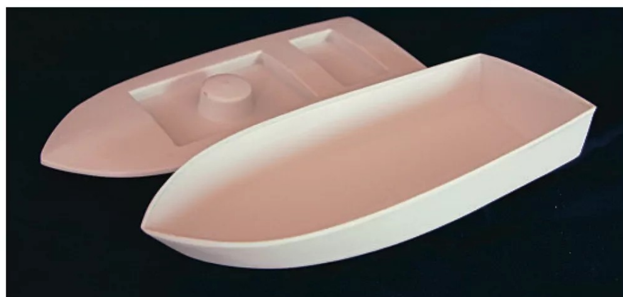
The smart vac-formed hull and deck show off the clean lines of the LSSC. The dome-like item is the optional radome cover.
