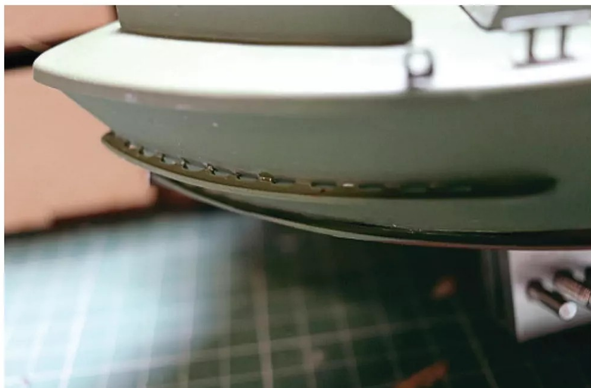
The chine was moulded to shape with heat from Nick's hands and glued in sections with superglue.
