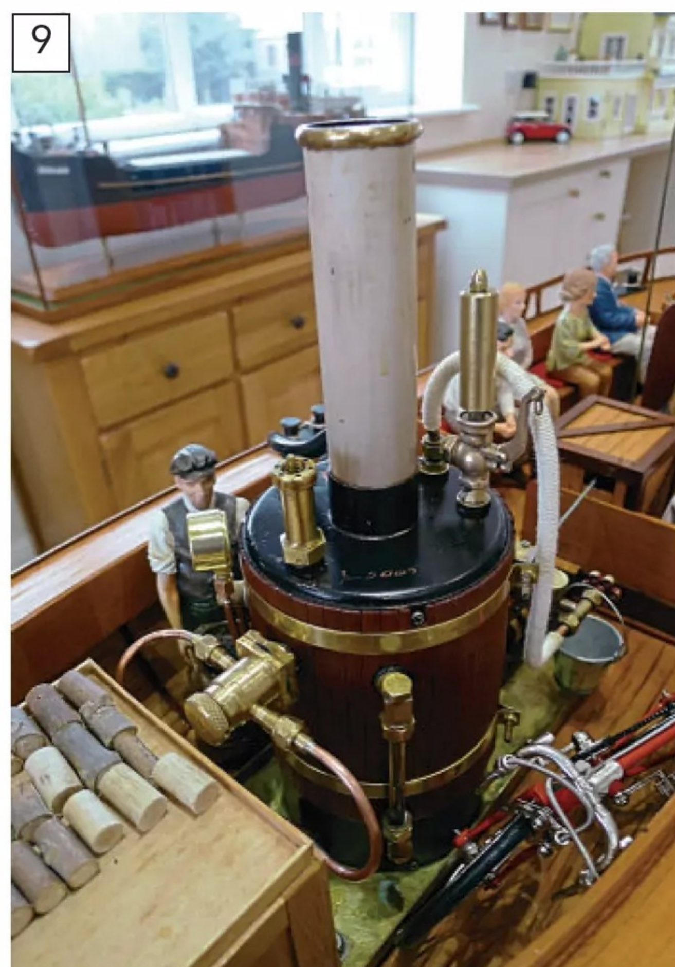
Fitting the attenuator valve to the boiler shell means that removing the entire plant remains as quick and easy as it was before fitting it.
