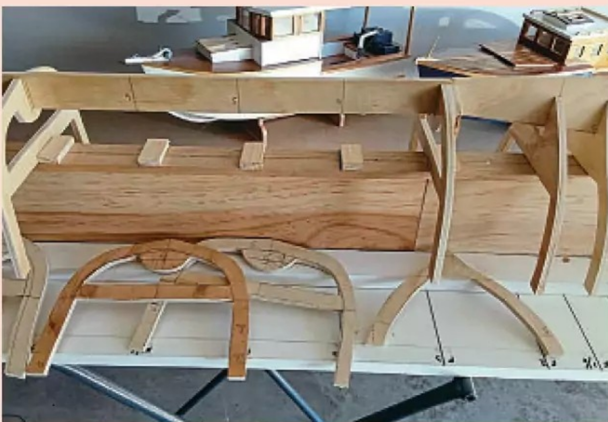
Plotting and cutting out bulkheads and fixing to jig.
