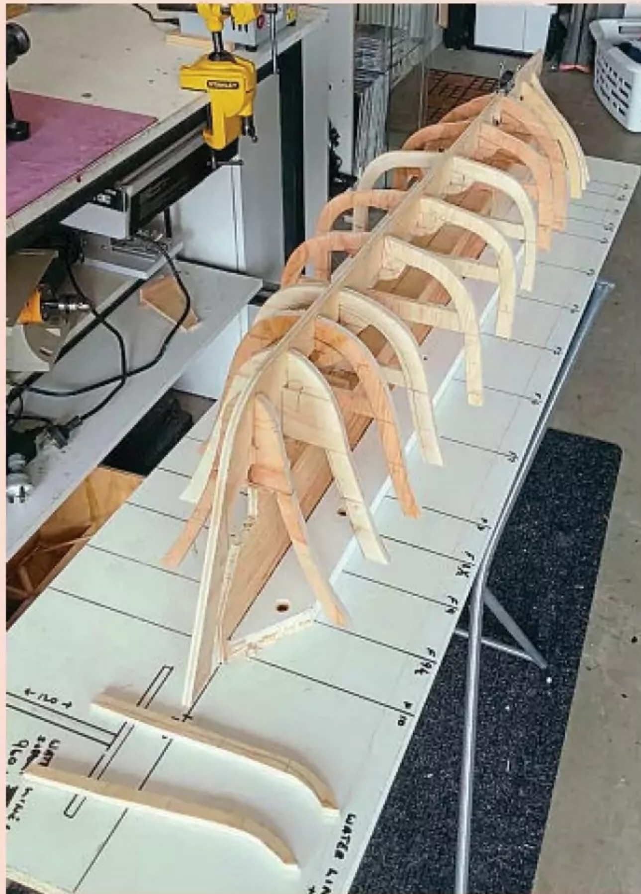
Plotting and cutting out bulkheads and fixing to jig.
