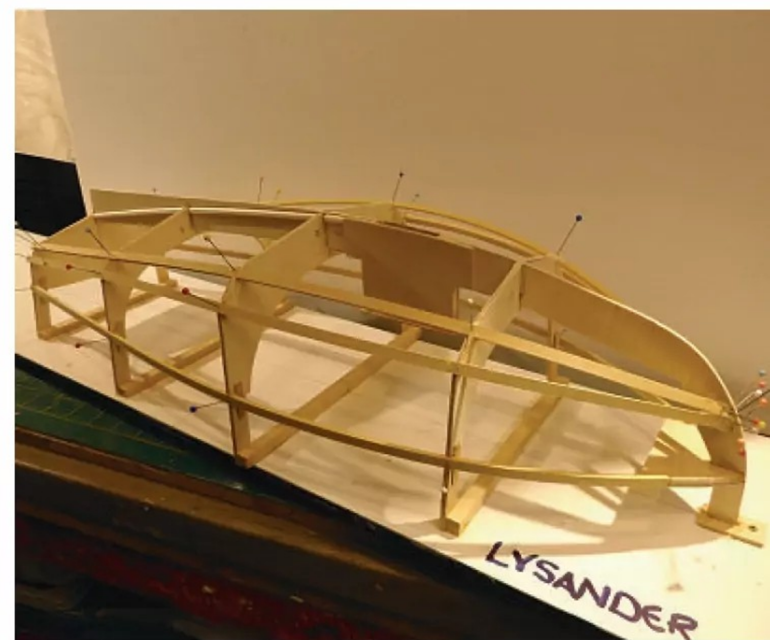
The bulkheads need to be mounted on your building board, with cross beams on a centre line to keep it true. Please note, the transom must be at a slight angle rather than completely vertical; I used 1/8-inch x 1/8-inch square balsa doublers each side of the keel to create a gluing surface for the bottom skins. I made my double chine rails up from 1/8-inch x 1/4-inch obeche strip, which I find bends nicely. Care must be taken with the shaping where they attach to the stem. At the bow there is a small breast hook (again, see B1 on the plan). To achieve the correct deck shape and provide a good gluing surface to accept the plywood skins, some fettling and sanding is required to the chines and gun whale.
