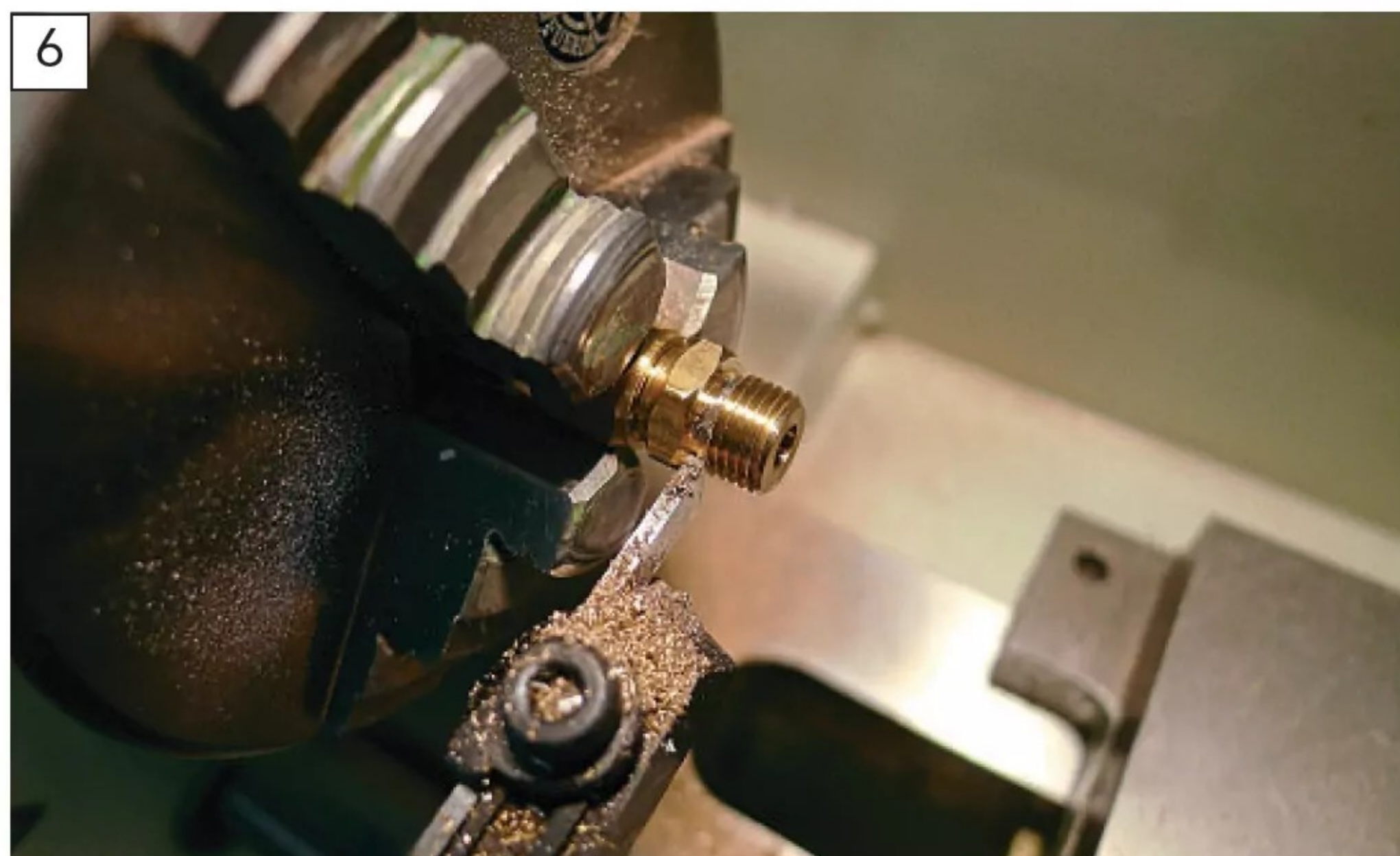
Parting off the thread from the new fitting is a lot more straightforward when you can fit the cone and nut to the other side to enable it to be held in a lathe.
