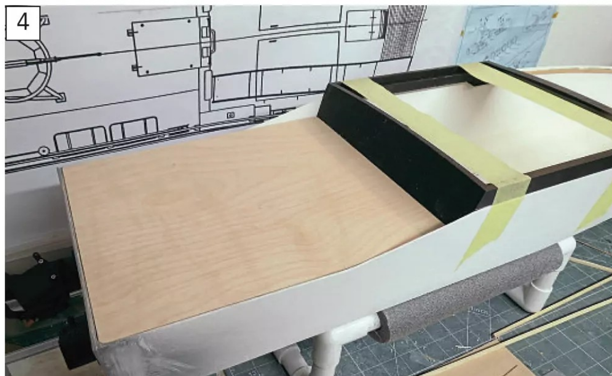
The rear deck formed from 2mm marine ply.
