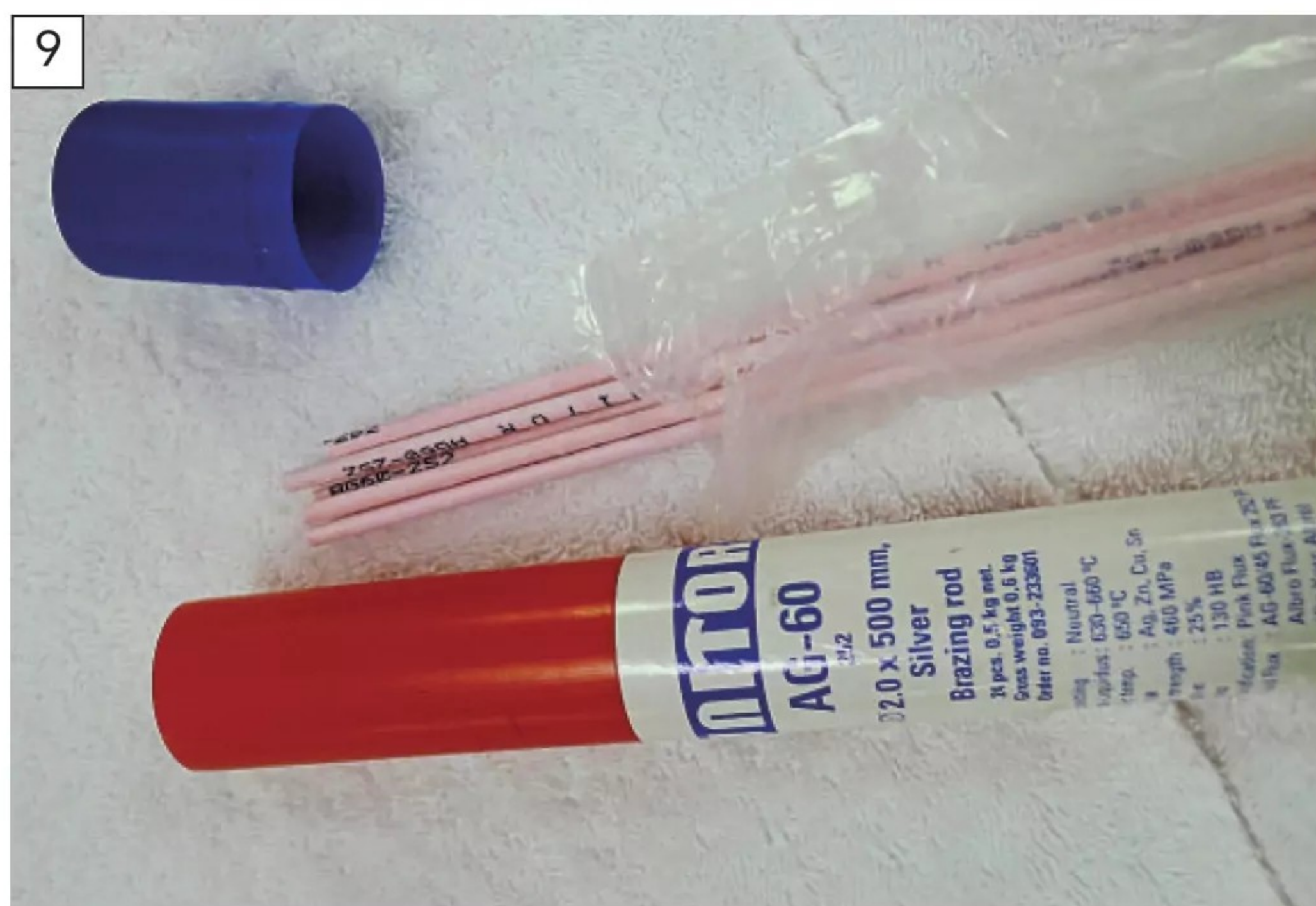
These are probably one of the most expensive silver soldering rods you can find; however, a single rod is enough for a very large number of pipework and fitting joints. Many modellers favour separate solder and flux, but Richard prefers having the flux coating on the rod.
