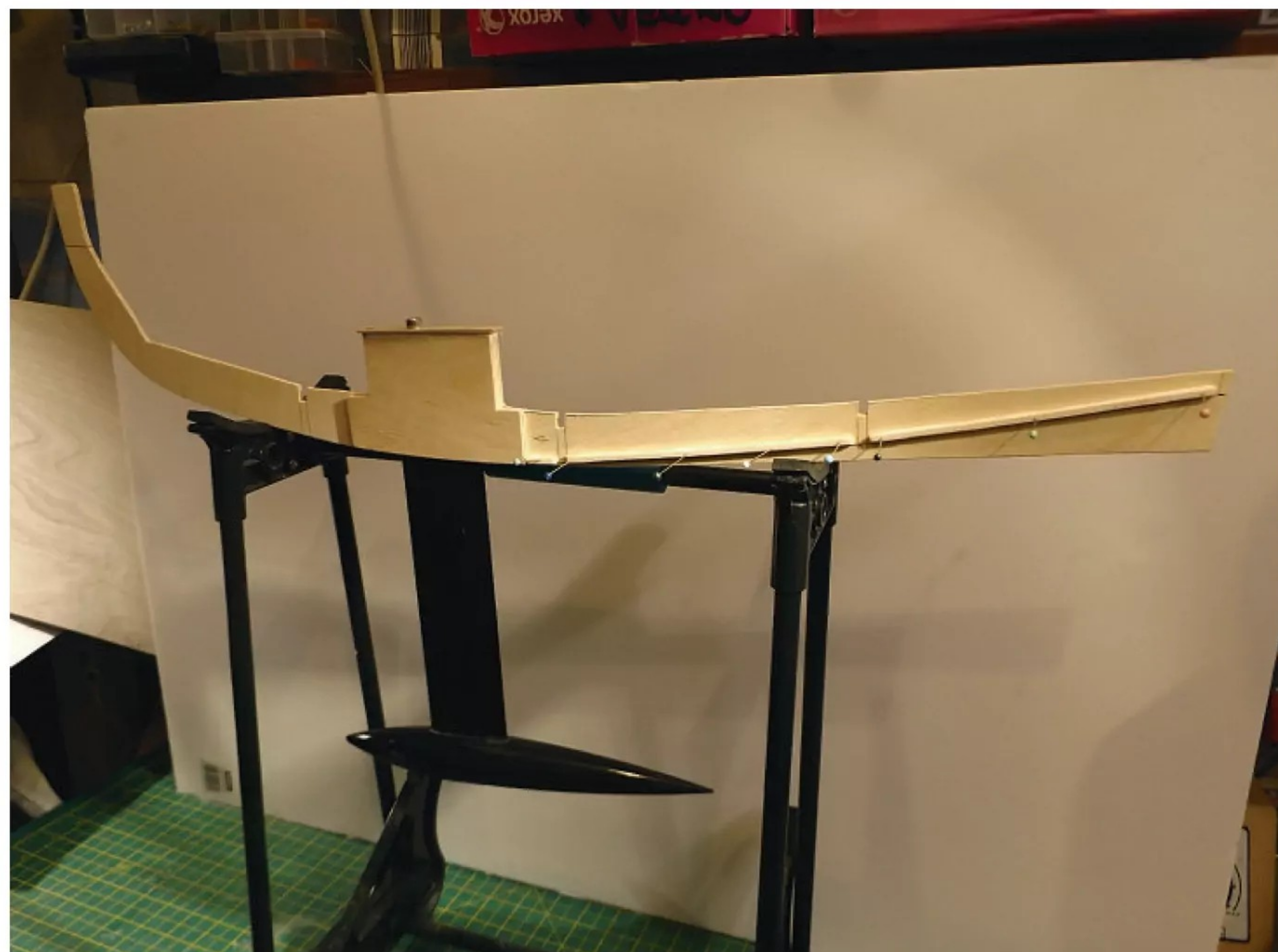
Here, the fin keel is shown being trial fitted with a 1/16-inch ply capping piece incorporating the retention cap head bolt which comes with the keel; accurate drilling is required. The capping piece is held in place with two small screws and glued (I used Gorilla woodworking glue for all the timber-to-timber joints).
