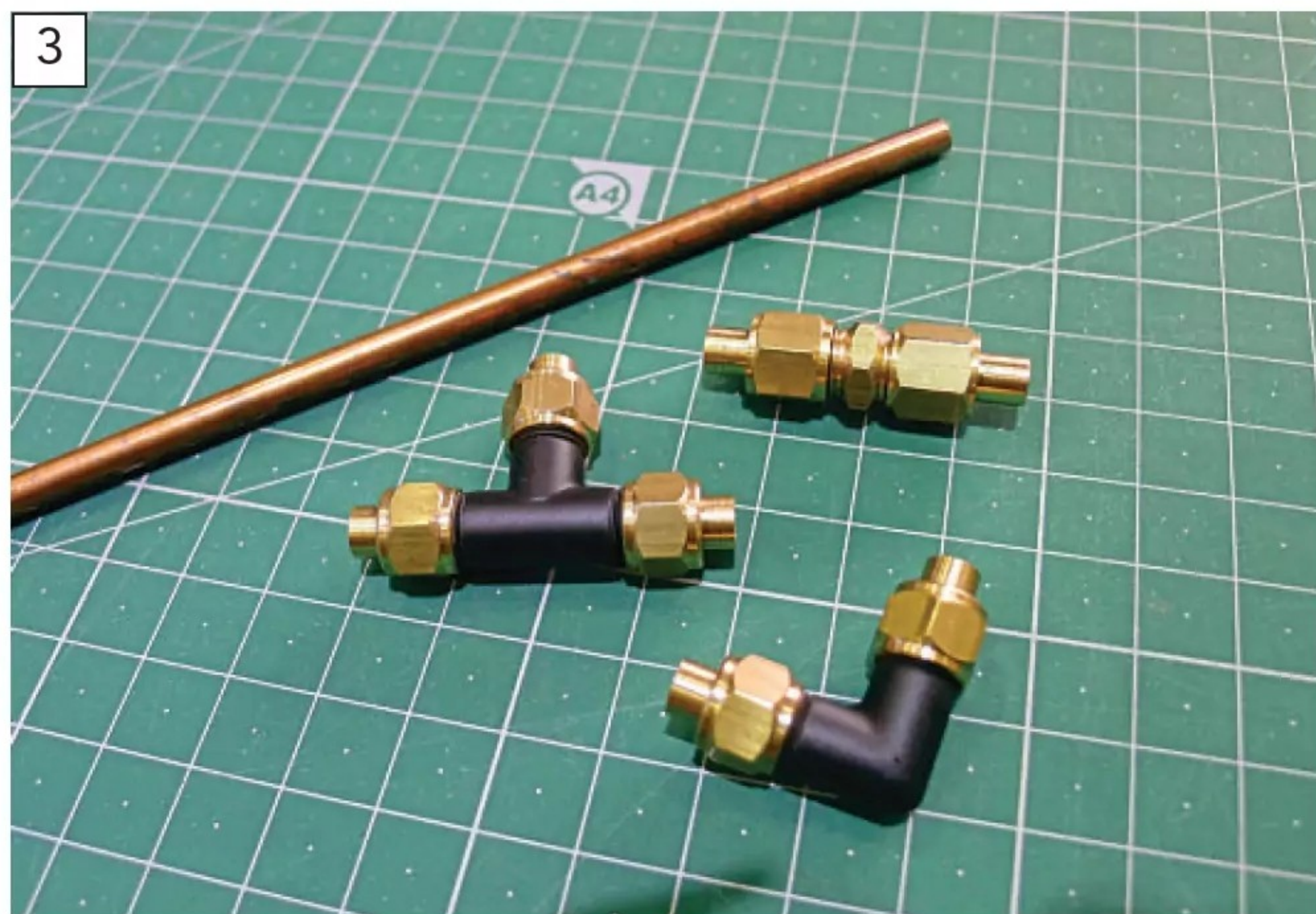
Readily available modern 3/16th copper pipe and brass conical fittings. Getting hold of these was the easy part of the job.
