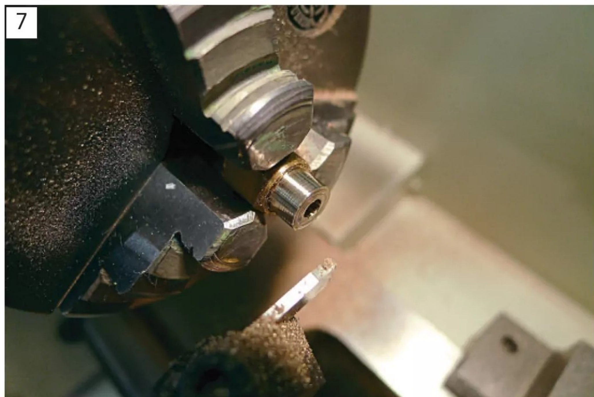
Richard didn't want the diameter to be any greater than the original fitting to avoid interference, so the hexagonal section had to be turned down as well.
