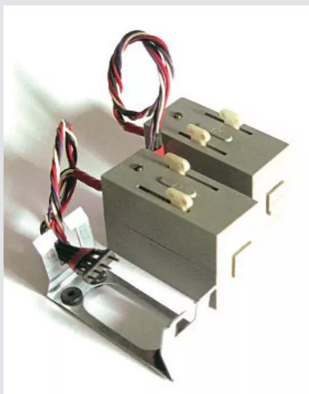
The famous Sprengbrook 'Micro-Lok' linear servo (in grey case) – sourced, like the control sticks, from Micro-Avionics Inc of California, alongside a later version (in black mouldings) fully modernised by the author.
