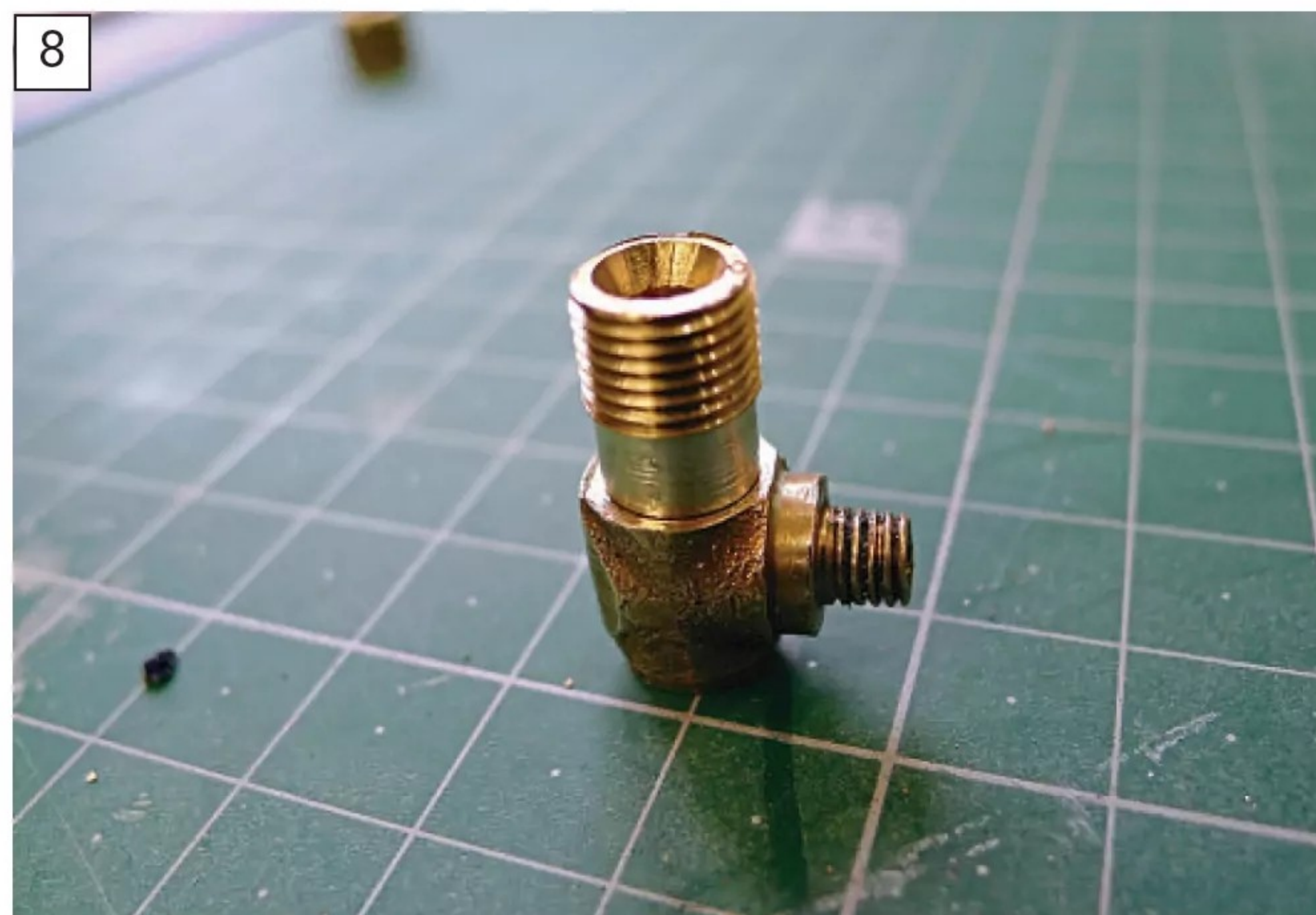
The best surface area Richard could arrange for the strongest possible joint, while also allowing for a nice fillet of solder on the outer surface.
