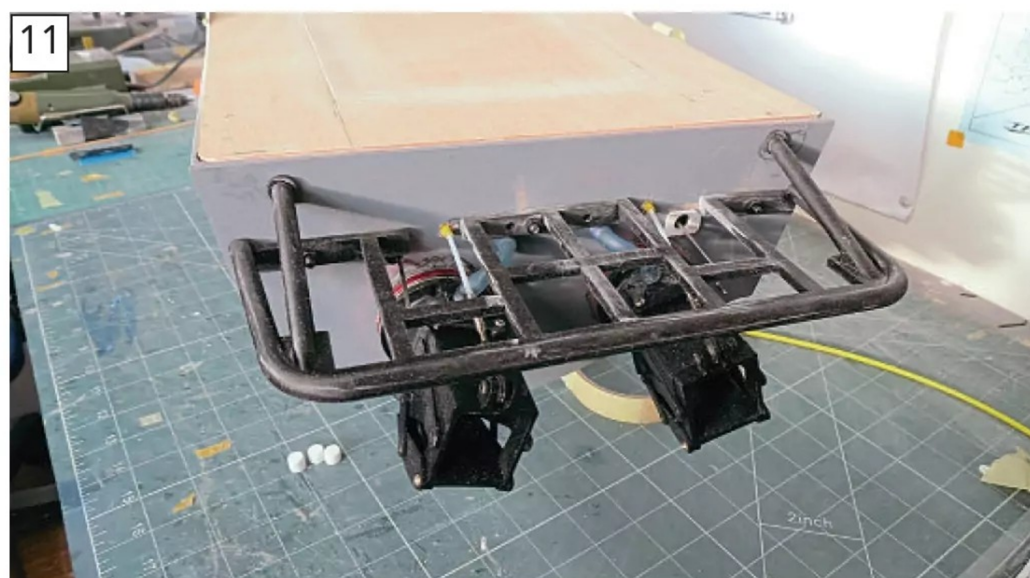
The transom platform and jet assembly protection.
