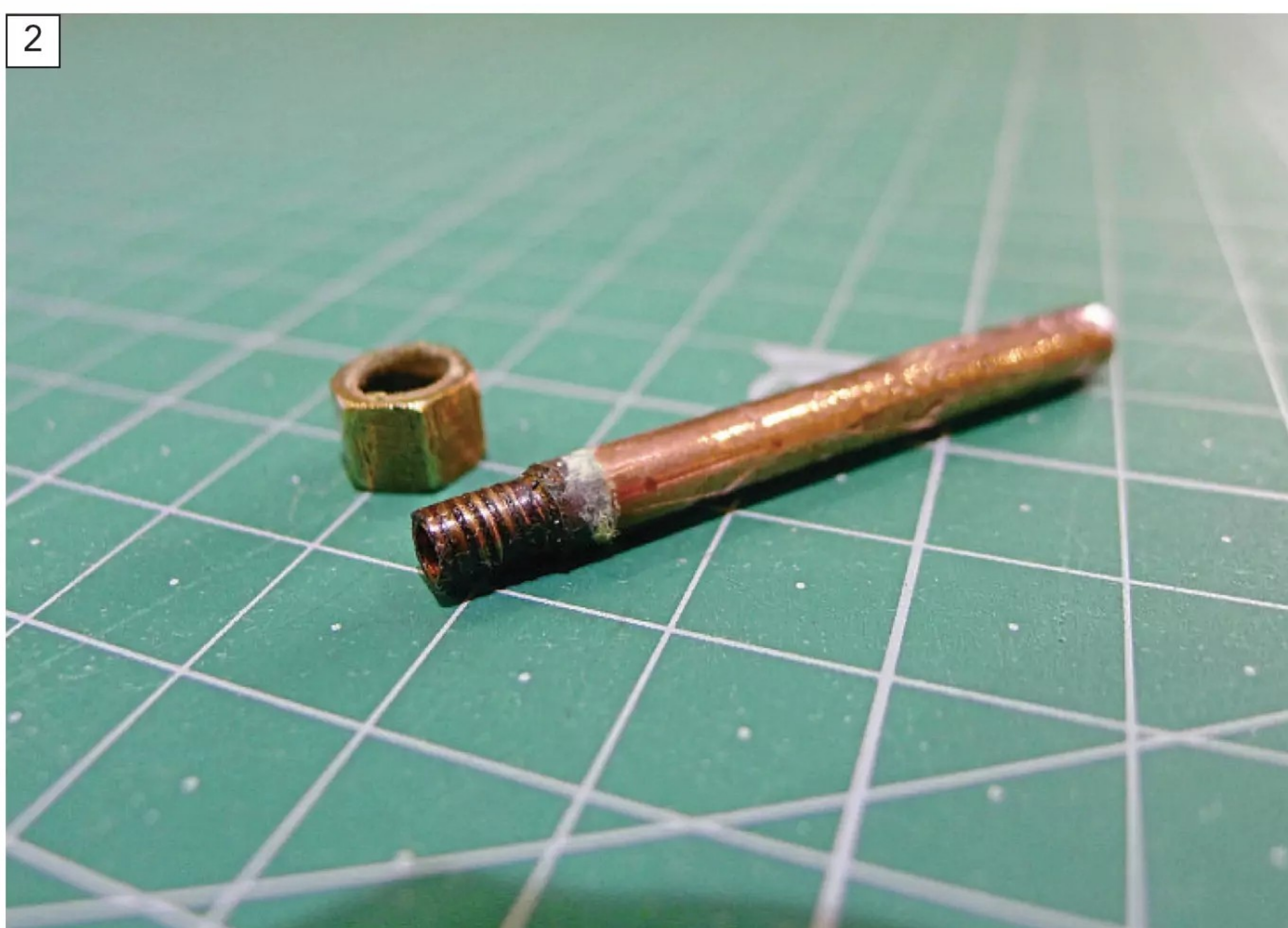
2 Richard had never come across a piece of copper pipe with a 'sort of' thread on the end! The nut was purely decorative. The problem was that this was the only male thread he had that fitted the engine.
