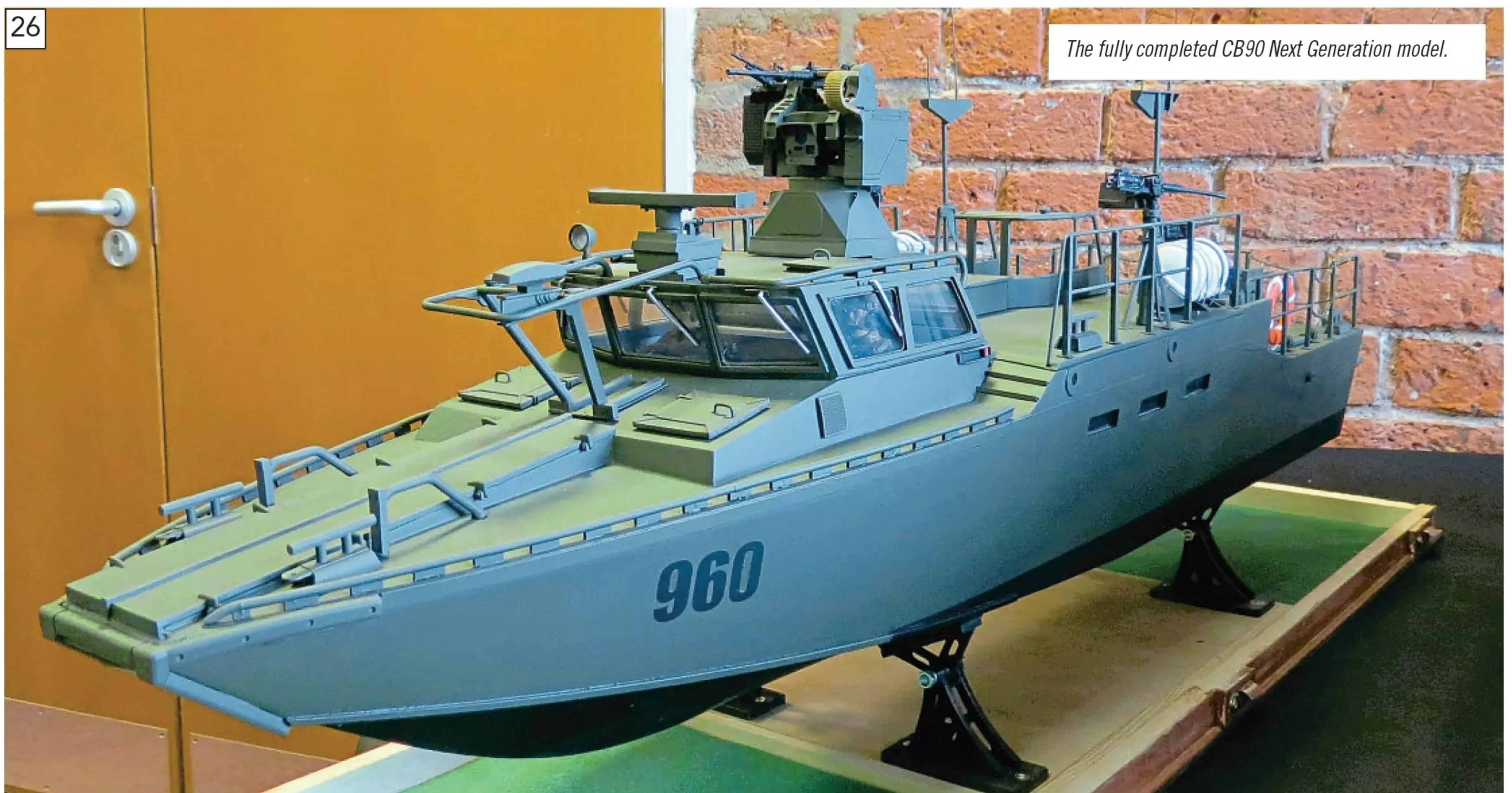
Additionally, five more 50 calibre MG and swivels mountings were 3D generated.
