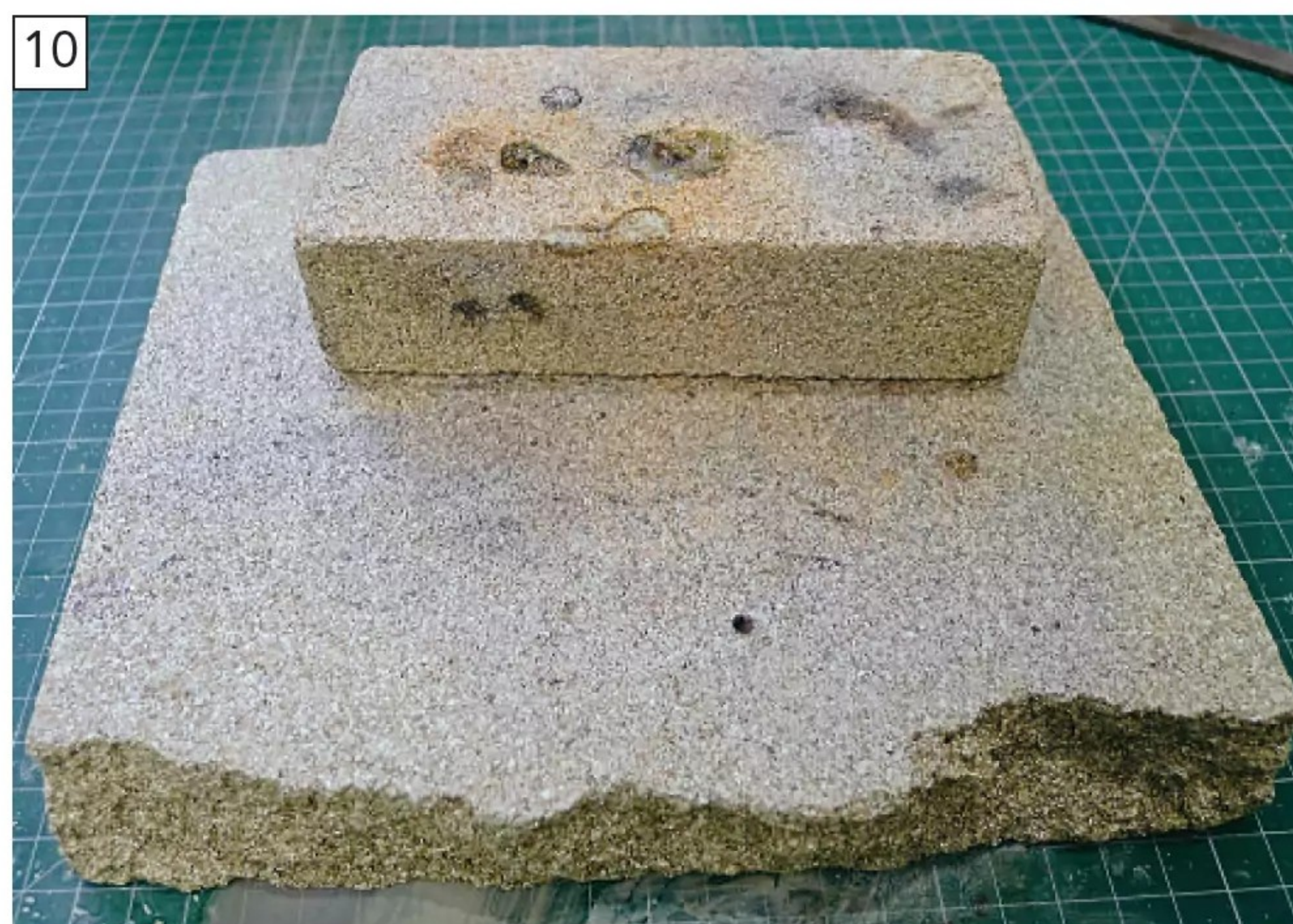
Vermiculite blocks are readily available from engineering suppliers. Richard was lucky enough to get a couple of large pieces when new insulation for a wood burning stove arrived broken and as a result were duly replaced.
