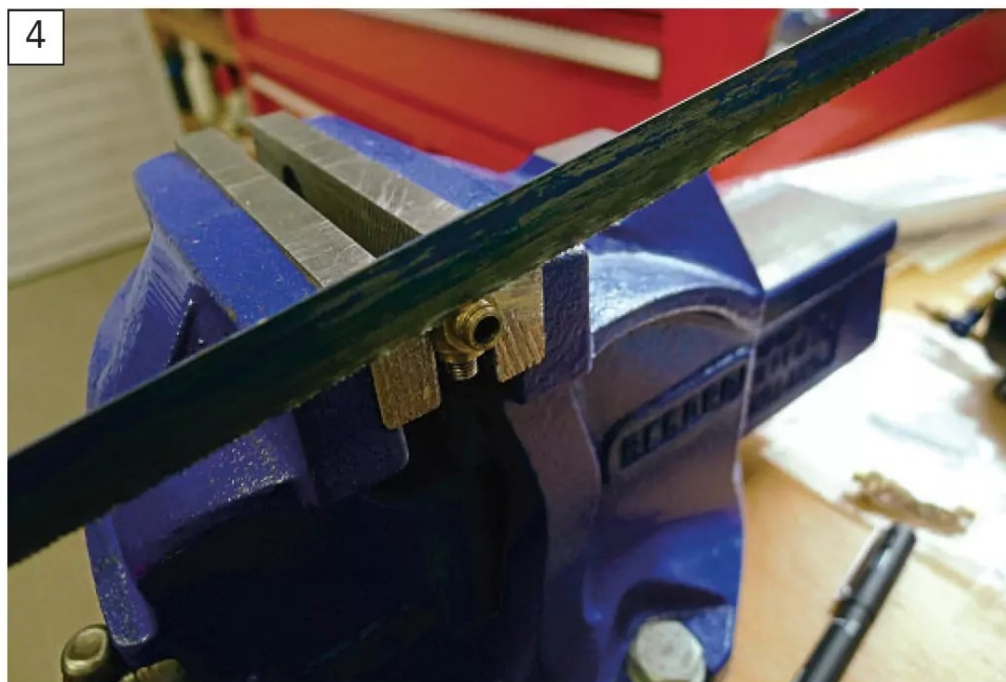
There is always a slight lump in the throat when you attack a 100-year-old brass fitting in the knowledge that it is almost certainly irreplaceable but it's the only way to preserve that valuable thread.
