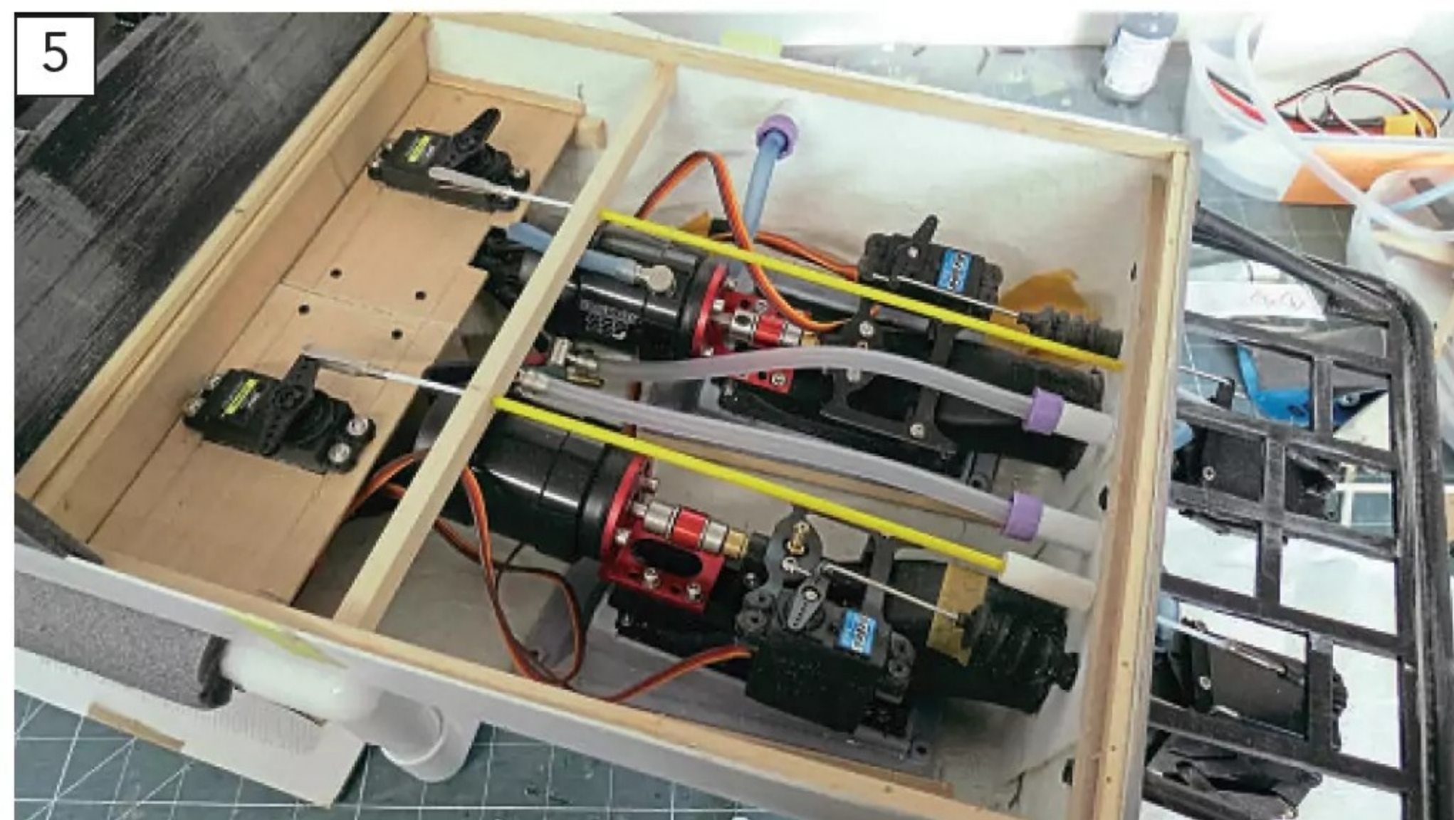
Water jet drives, and servos for the reverse thrust mounted unlike the steering nozzles on a dedicated platform.
