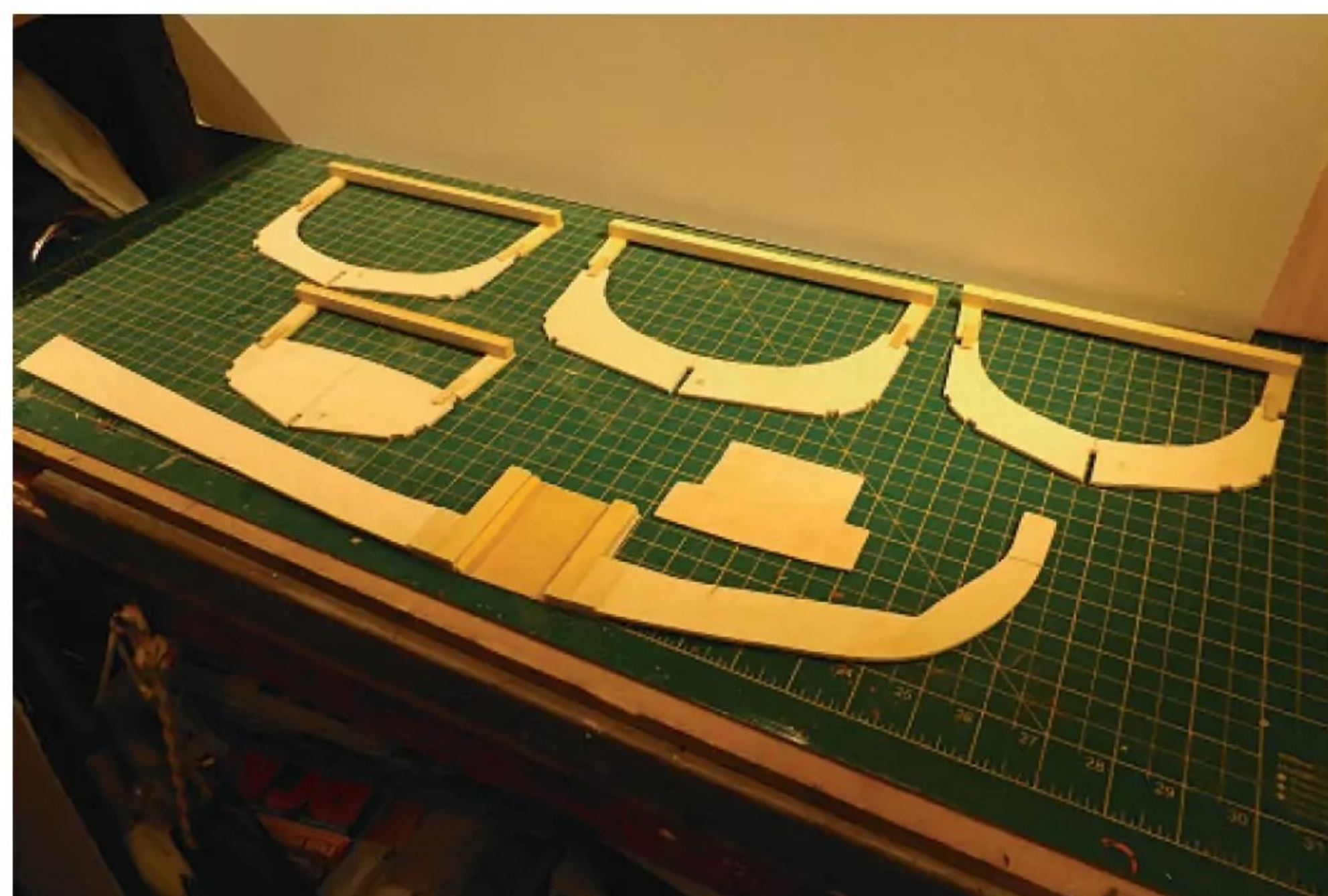
The main bulkheads and transom need to be cut from 3mm plywood (I purchased mine from Wickes). The extensions to the building board can be cut off once the hull is complete. The keel is constructed from 1/4-inch ply, while the keel box (marked B1 on the plan) is made up, in position, from 1/16-inch ply, remembering to paint or varnish the inside before final assembly to keep the water out.
