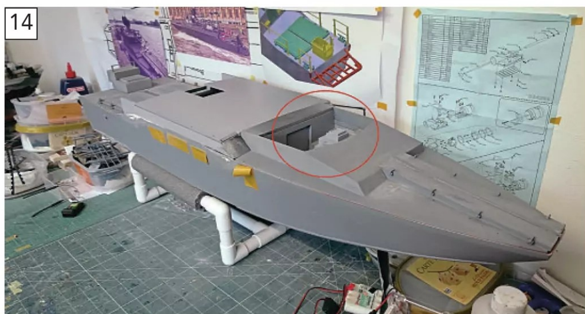
There are three windows along the side amidships; on each side these have been glazed and covered over.
