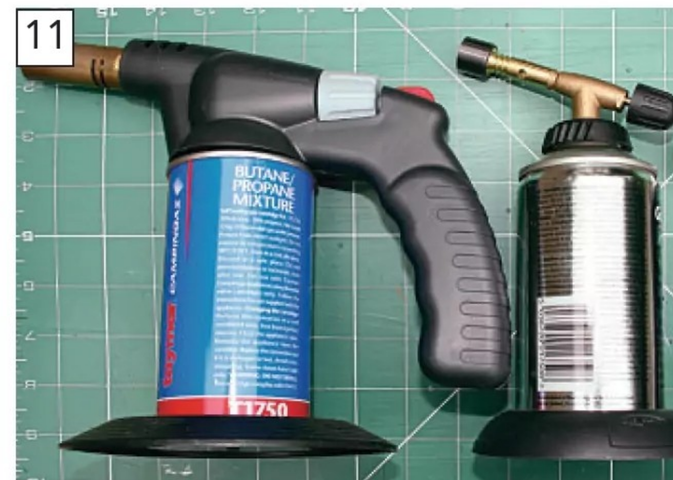
A couple of handy sized torches for most hobby silver soldering work. Serious jobs might require oxy-acetylene equipment, but pipework and fittings can easily be done with plumbers' type torches.
