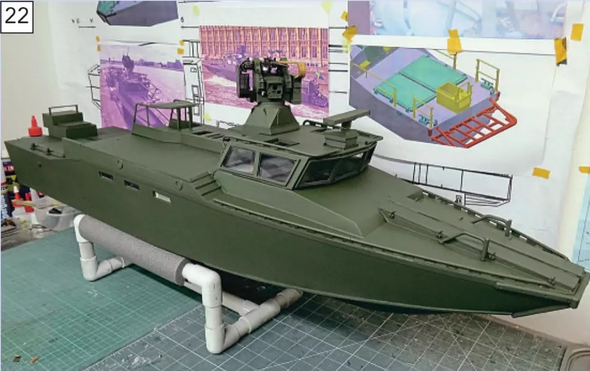
The 3D printed Trackfire gun, plus mounting and wheelhouse onto which the Trackfire mounting fits, added to the model.
