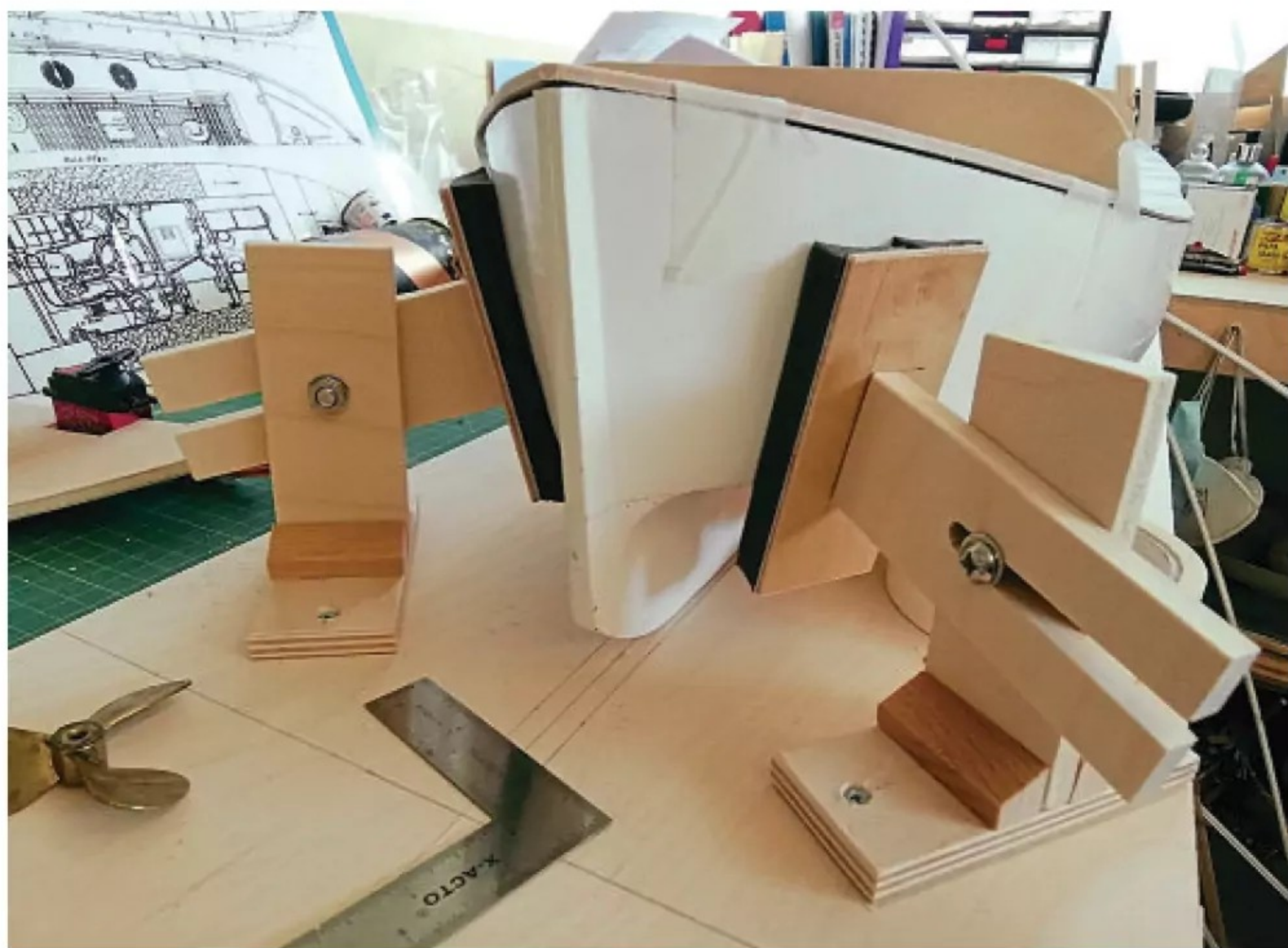
The supports in use. These are screwed to the baseboard and can be easily moved if necessary.
