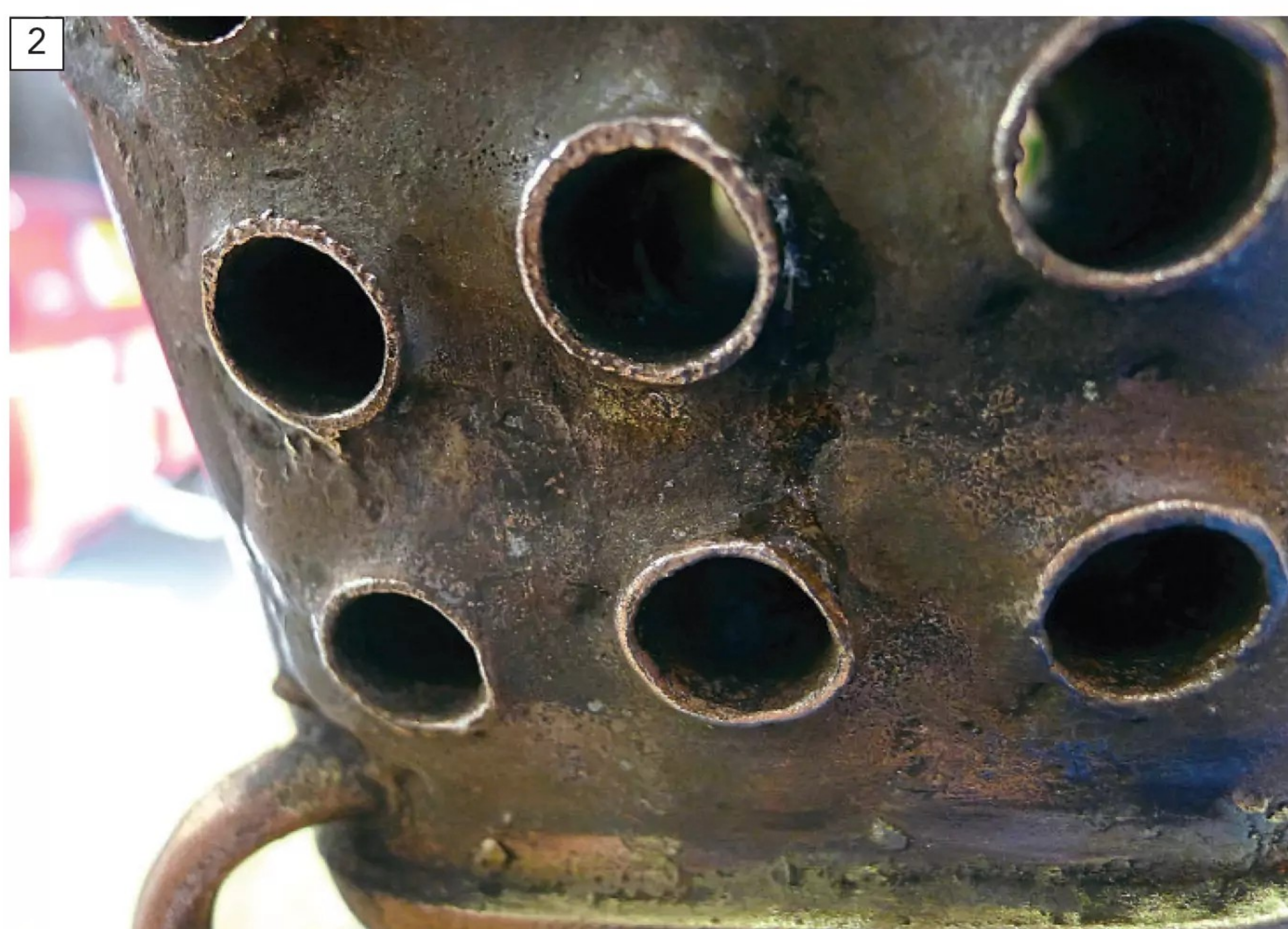
It wasn't a great surprise when a number of leaks revealed themselves at the joints between the shell and the tube ends. This is just one of them.
