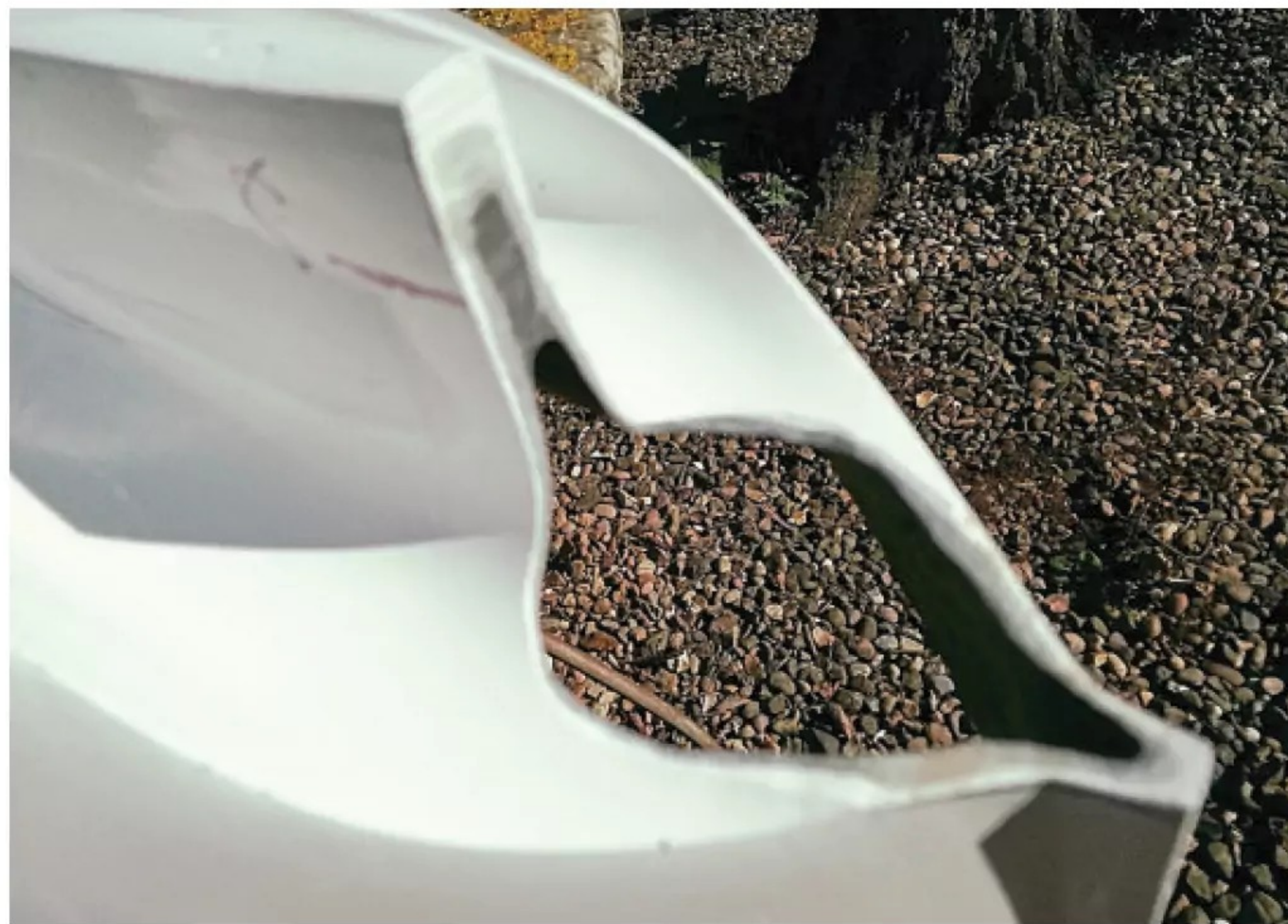
Drastic measures were taken to alter what was a perfectly good hull to allow a single propellor to be used.
