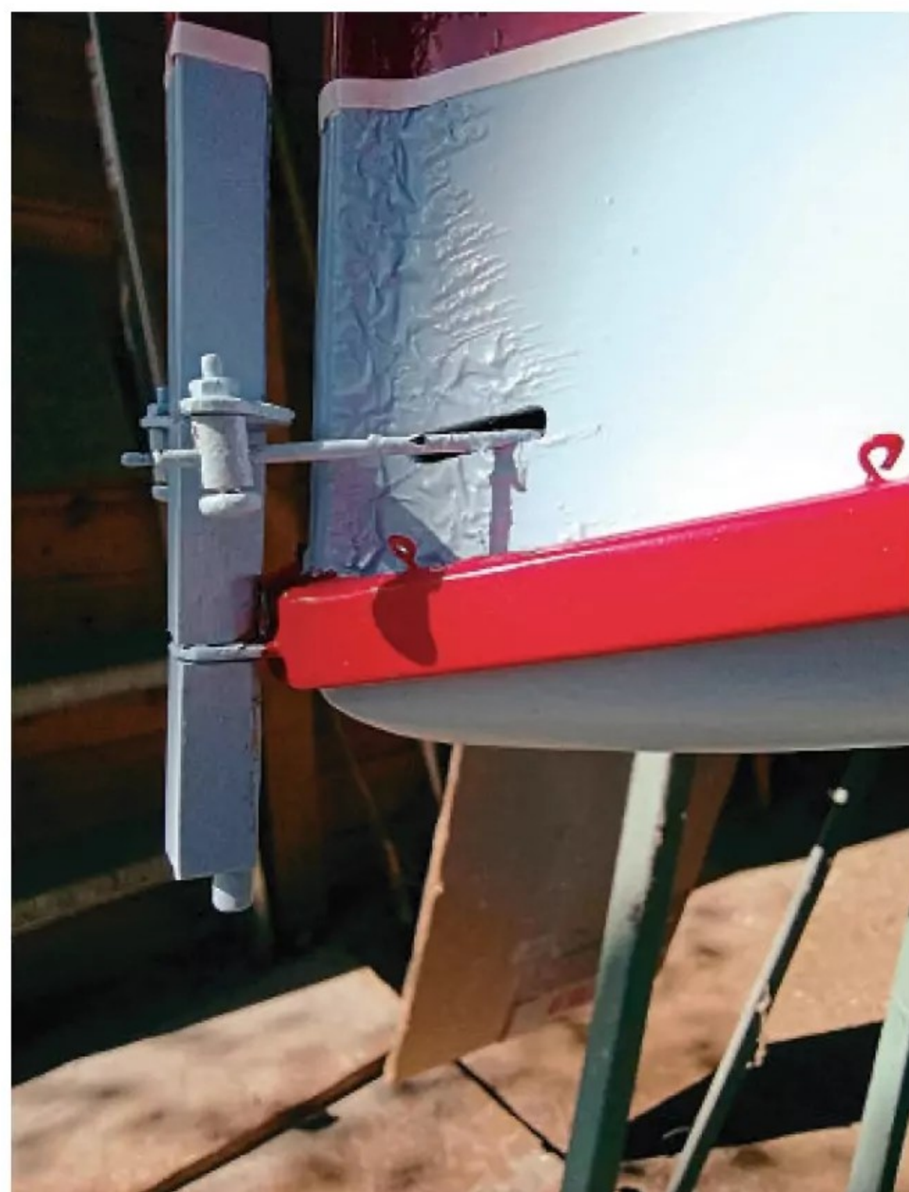
After the application of spray lacquer, John's paintwork began blistering and flaking off!
