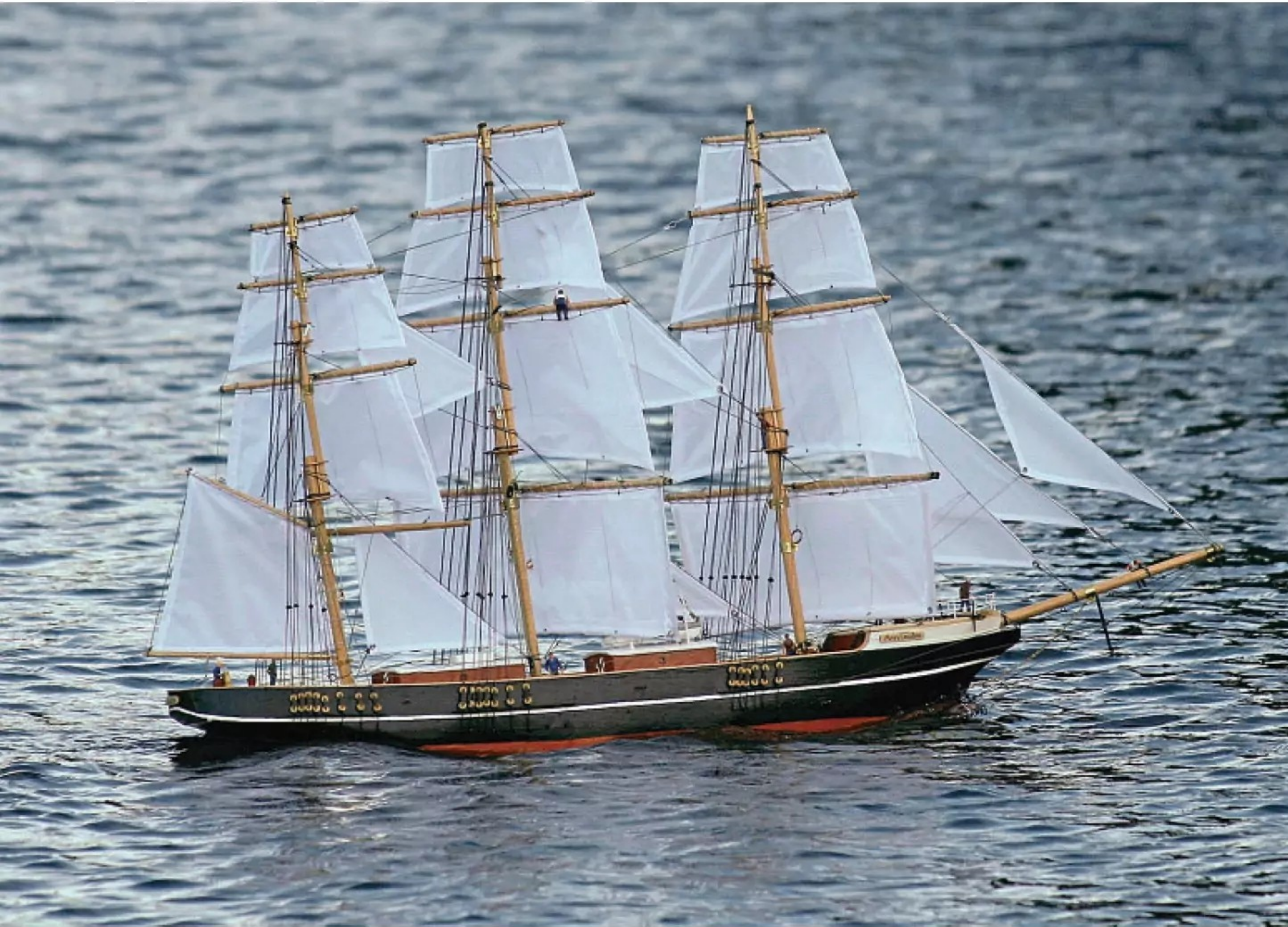
Ann Louise sailing as originally built, with stumpy bowsprit, tiny boats and full-size foresail.
