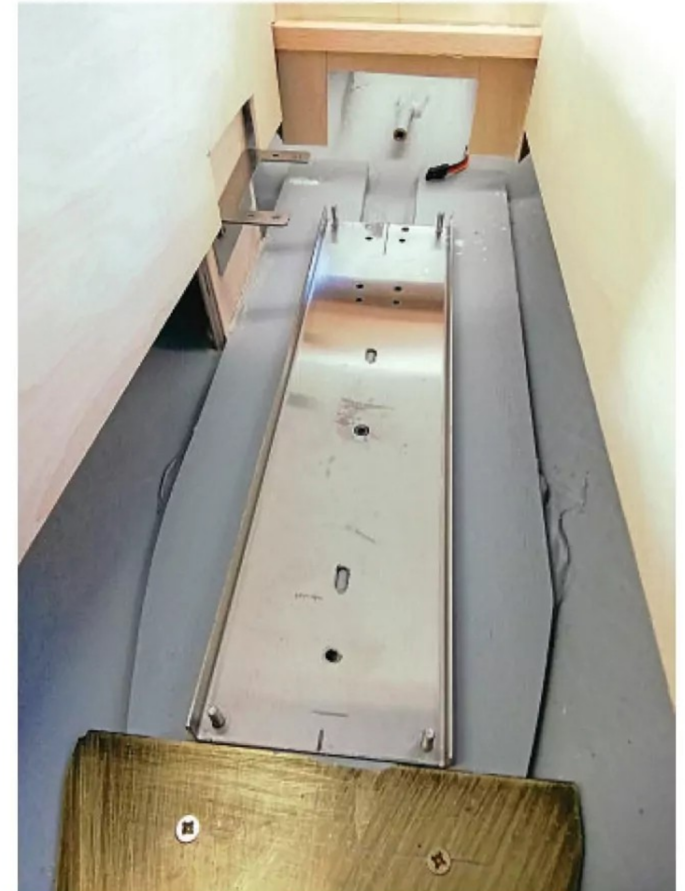
Within the hull, the base for the steam plant, made from 9 mm ply, was bonded in on a bed of P 38. Onto this, was screwed the stainless-steel base.
