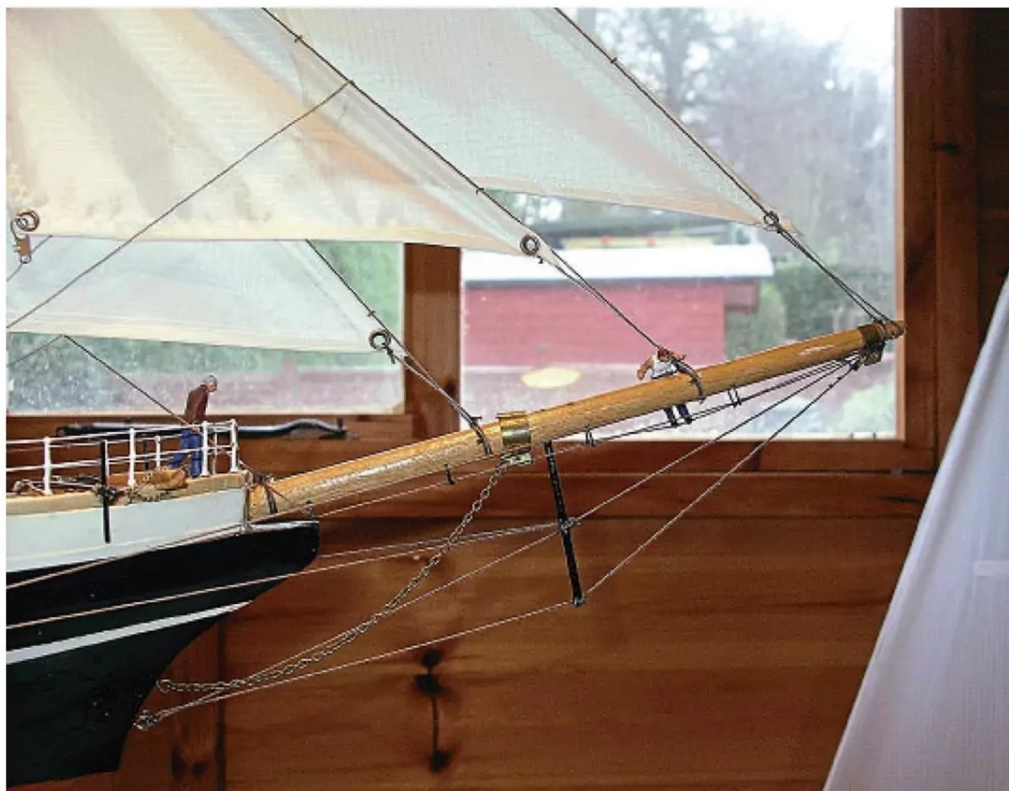
The original bowsprit, in the right place, the right length, but way too thick.
