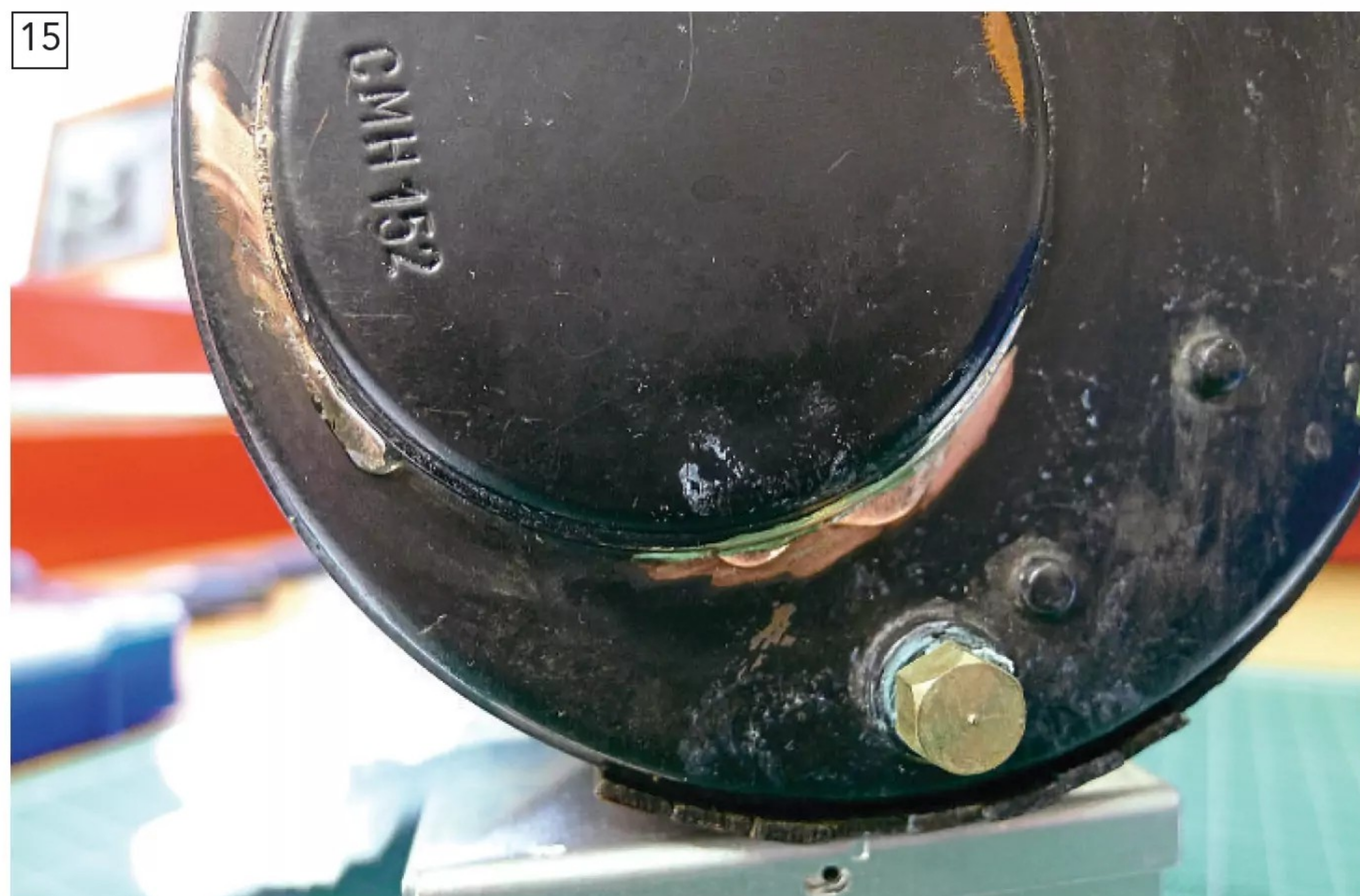
Sadly, with the internal scale out of the way, a couple of areas where leaks were coming through the same joint became evident.
