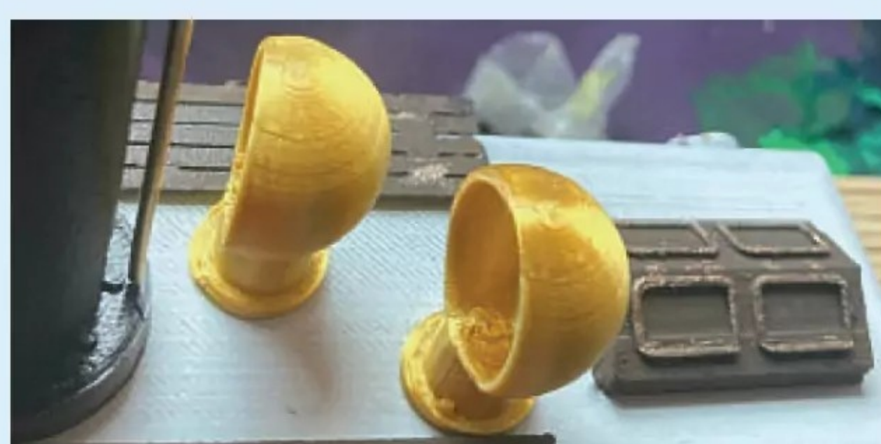
Steven's 3-D designed and printed vents.
