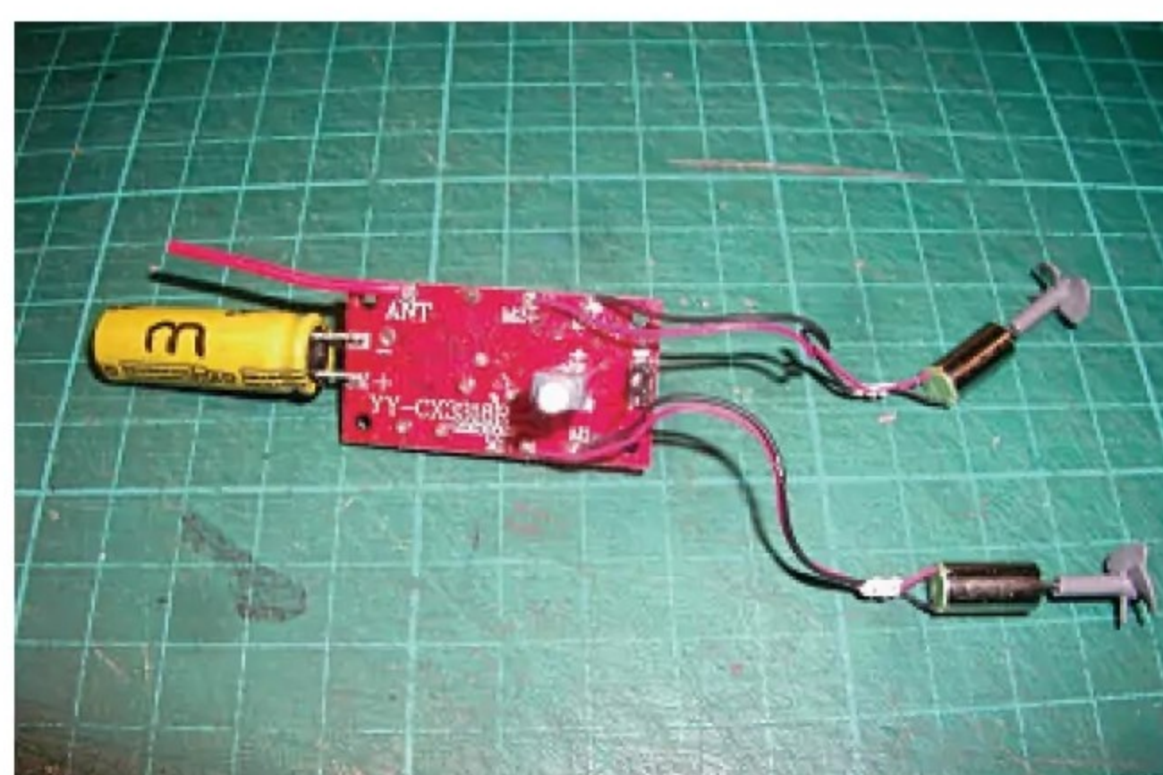
Plan view of radio-control PCB, 25mm x 40mm, with motors and battery
