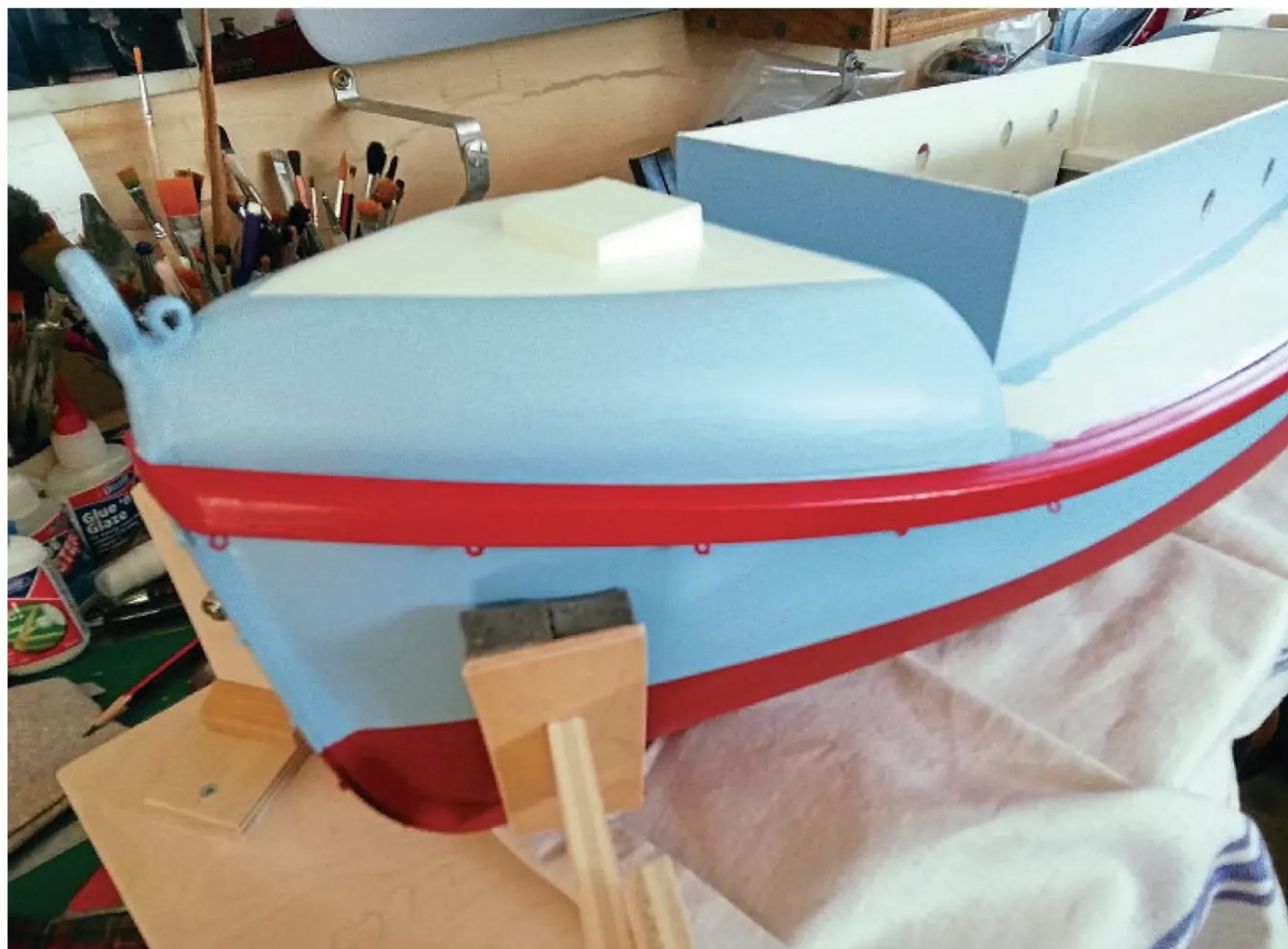
The pale blue achieved by mixing blue and white enamel paint applied. The colour is an approximation of that carried by the prototype. Disaster was lurking round the corner, though!
