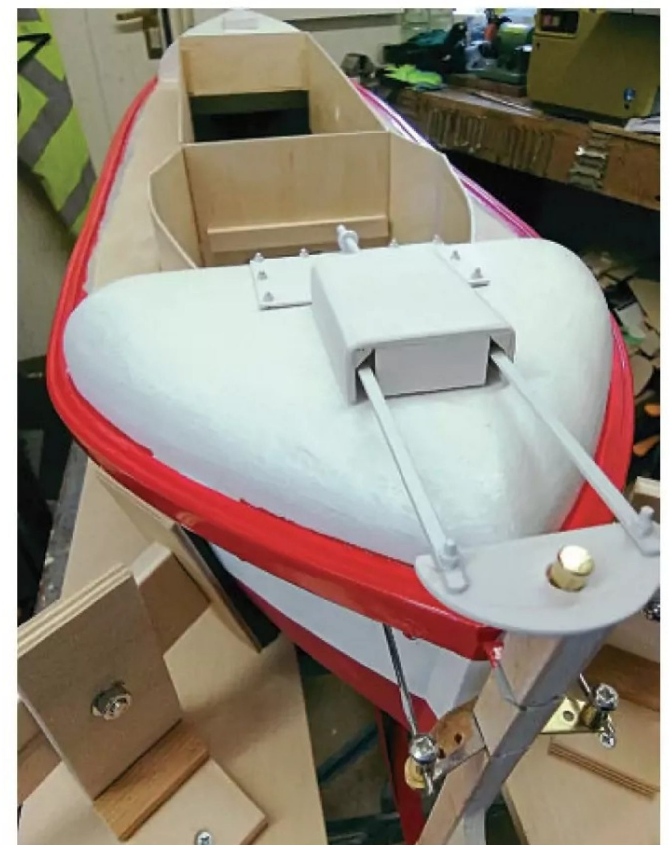
The dummy steering gear in place on the rear deck, with work on the superstructure of the engine/boiler room in progress evident in the background.
