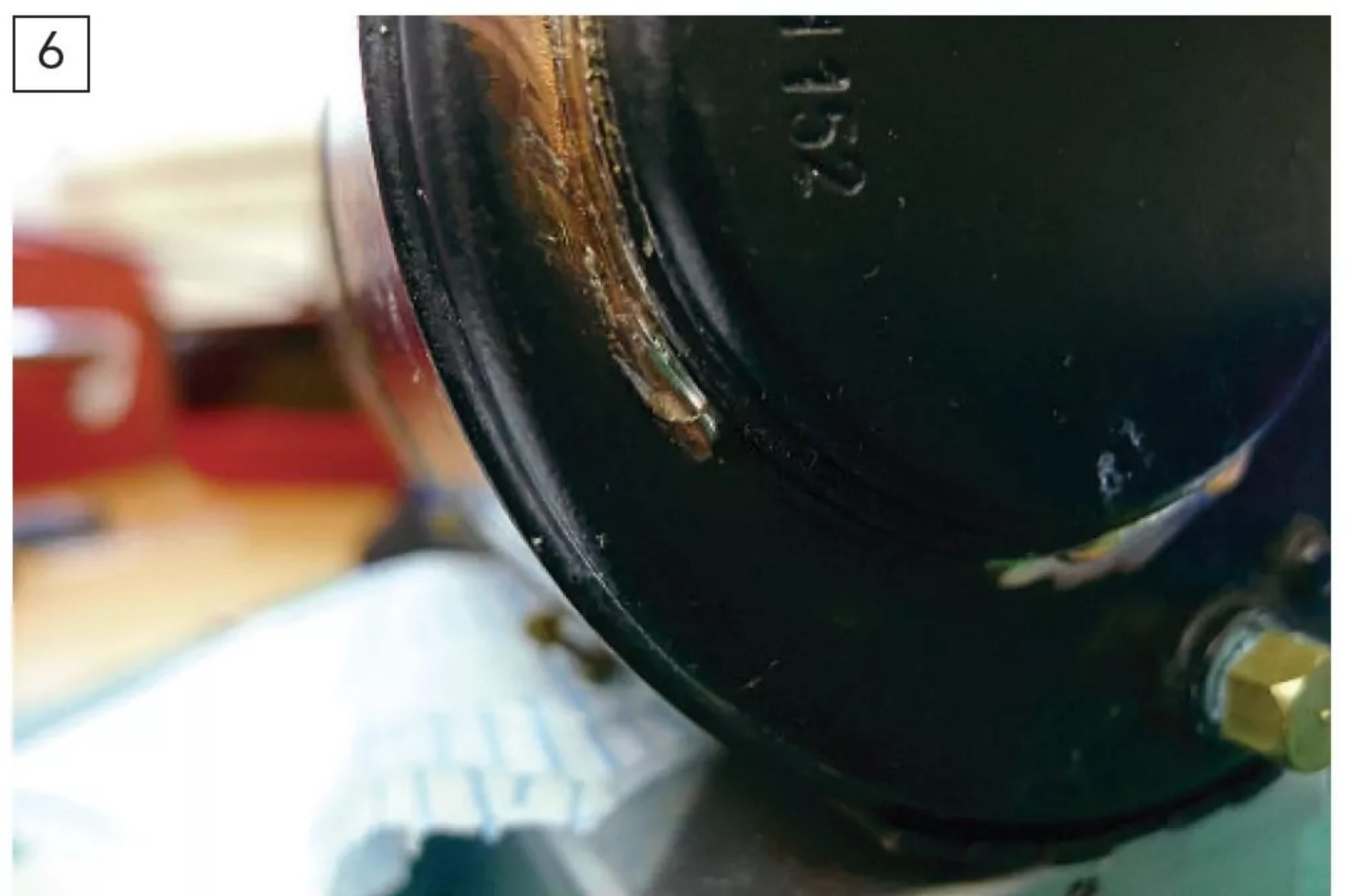
Unfortunately, a leak revealed itself after just a couple of minutes. Initially hoping he was simply looking at a little splash of water, Richard wiped this away and cleaned the paint off the area, but, sure enough, more leakage was evidenced.
