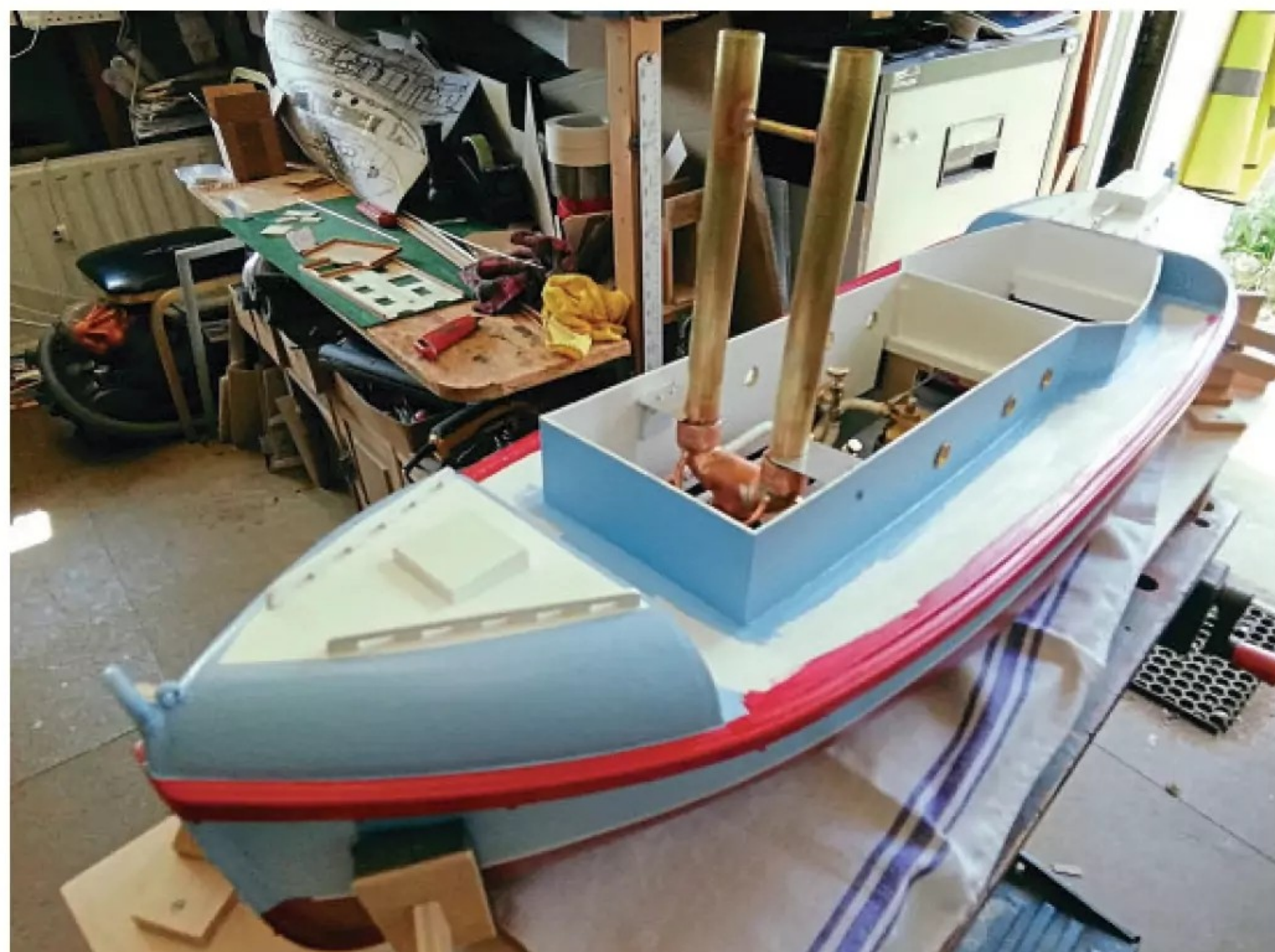
With the steam plant installed, detailing of the superstructure could begin.
