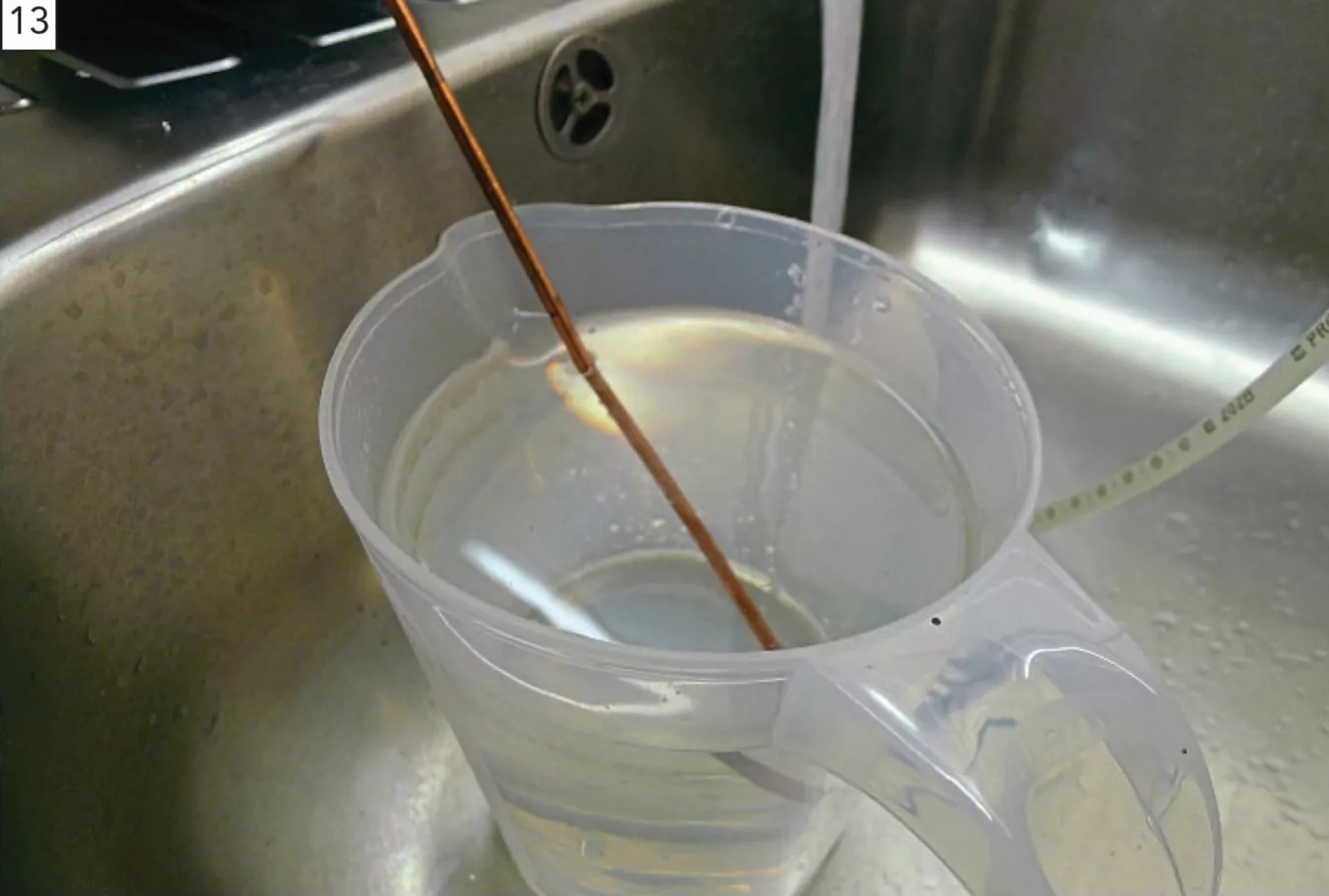
The water eventually runs nice and clean. Once this happens, you can leave it for a further half an hour to ensure the boiler is thoroughly flushed through. Some might like to use a piece of Litmus paper to test for acidity, but Richard sees clean fresh water as good enough confirmation.
