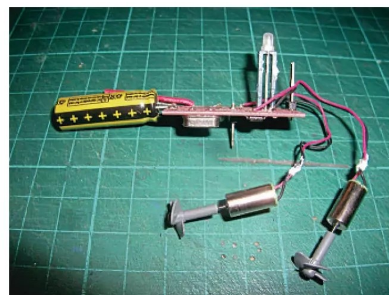
Motors with propellers, control PCB and battery, all taken from the toy frigate. If embarking in a similar project yourself, be careful when sawing the hull in half during the extraction process as the motor wires are VERY delicate!
