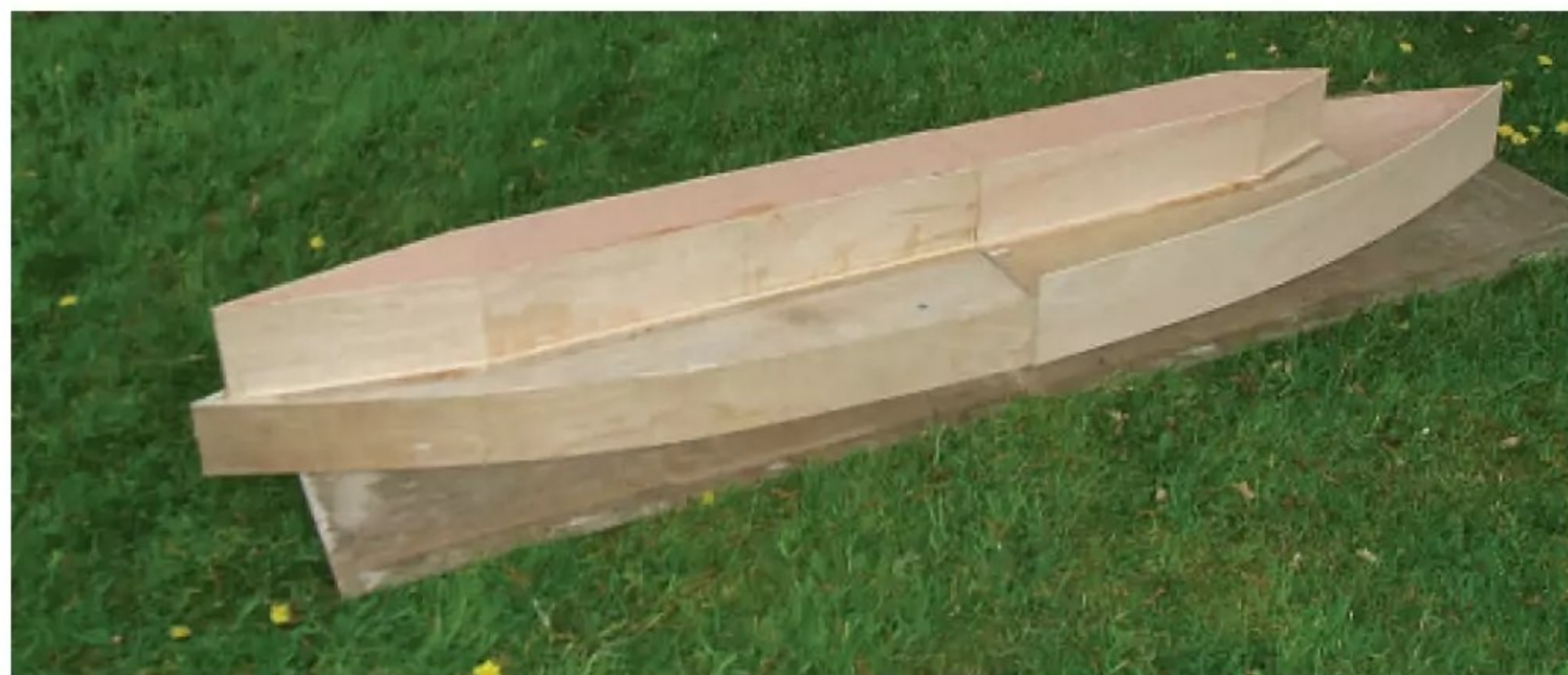
Work in progress on Trev Ford's coastal battleship, a build design of two halves, so that it can easily fit in the boot of his car.
