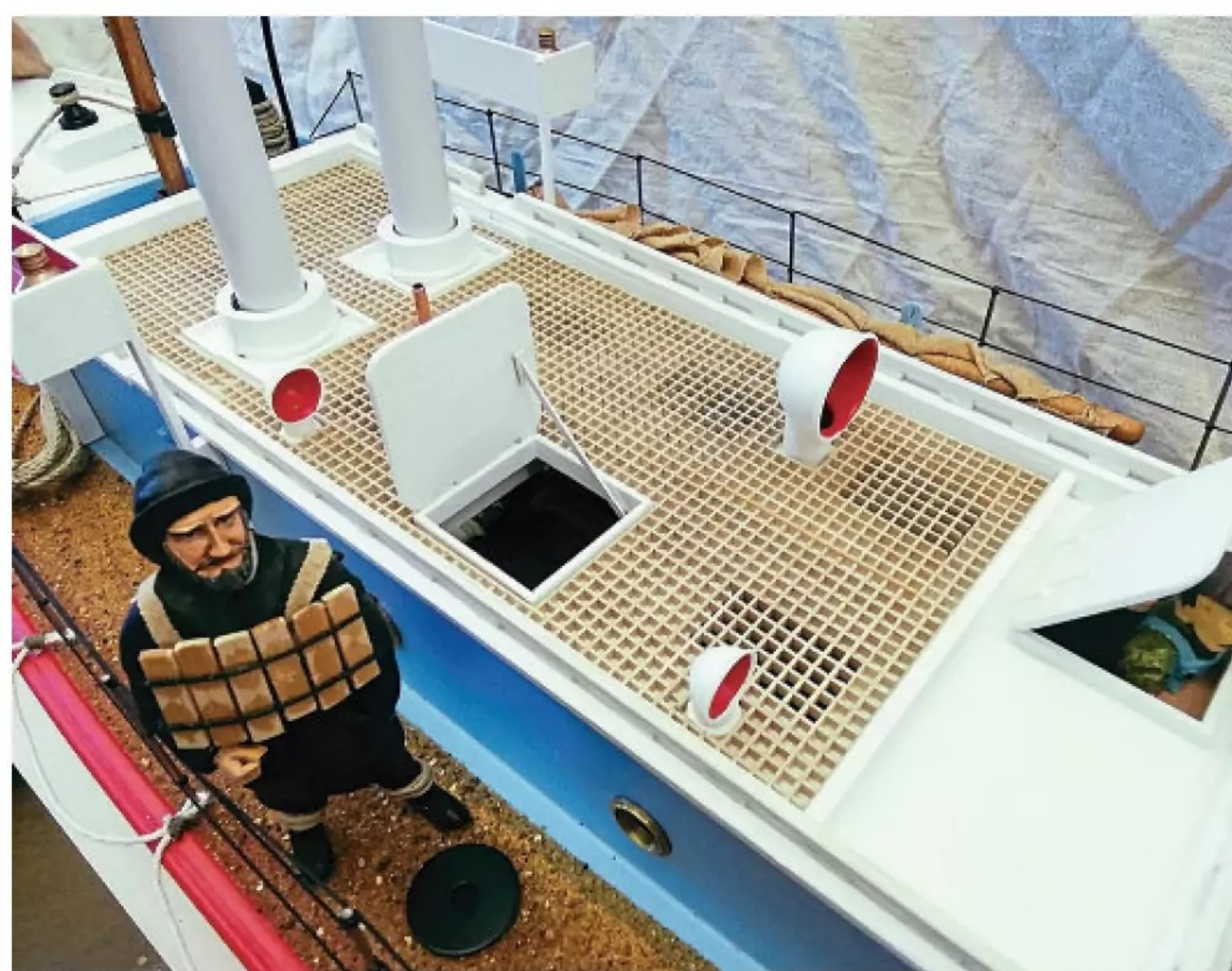
The deck was covered in wooden grating. John found this to be a most tedious task. Not only did his grating keep falling apart but it had to be cut to fit around various obstacles.
