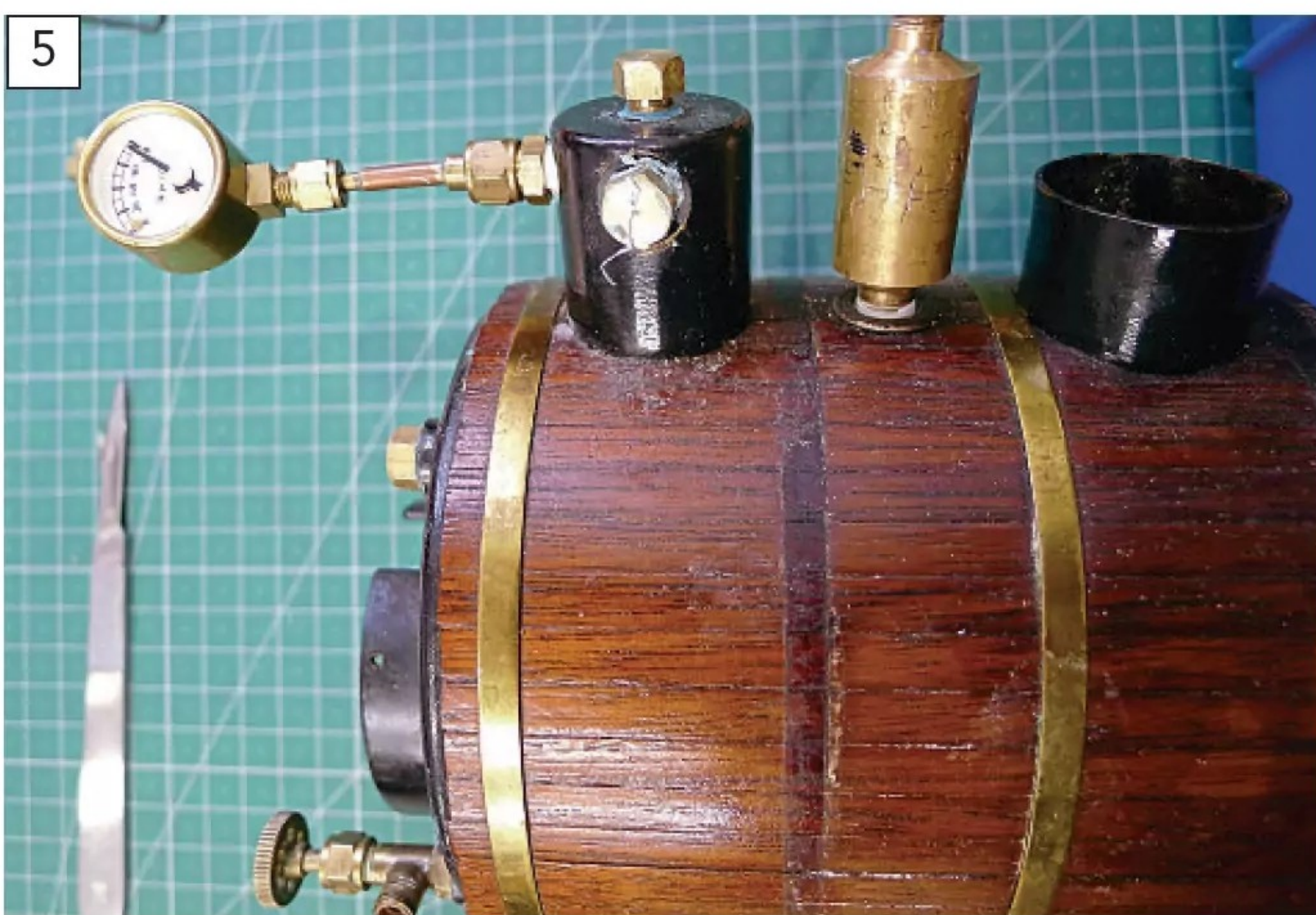
After fitting a pressure gauge, Richard quickly took it up to pressure to test the rig and if necessary, rectify any leaking fittings or plugs.
