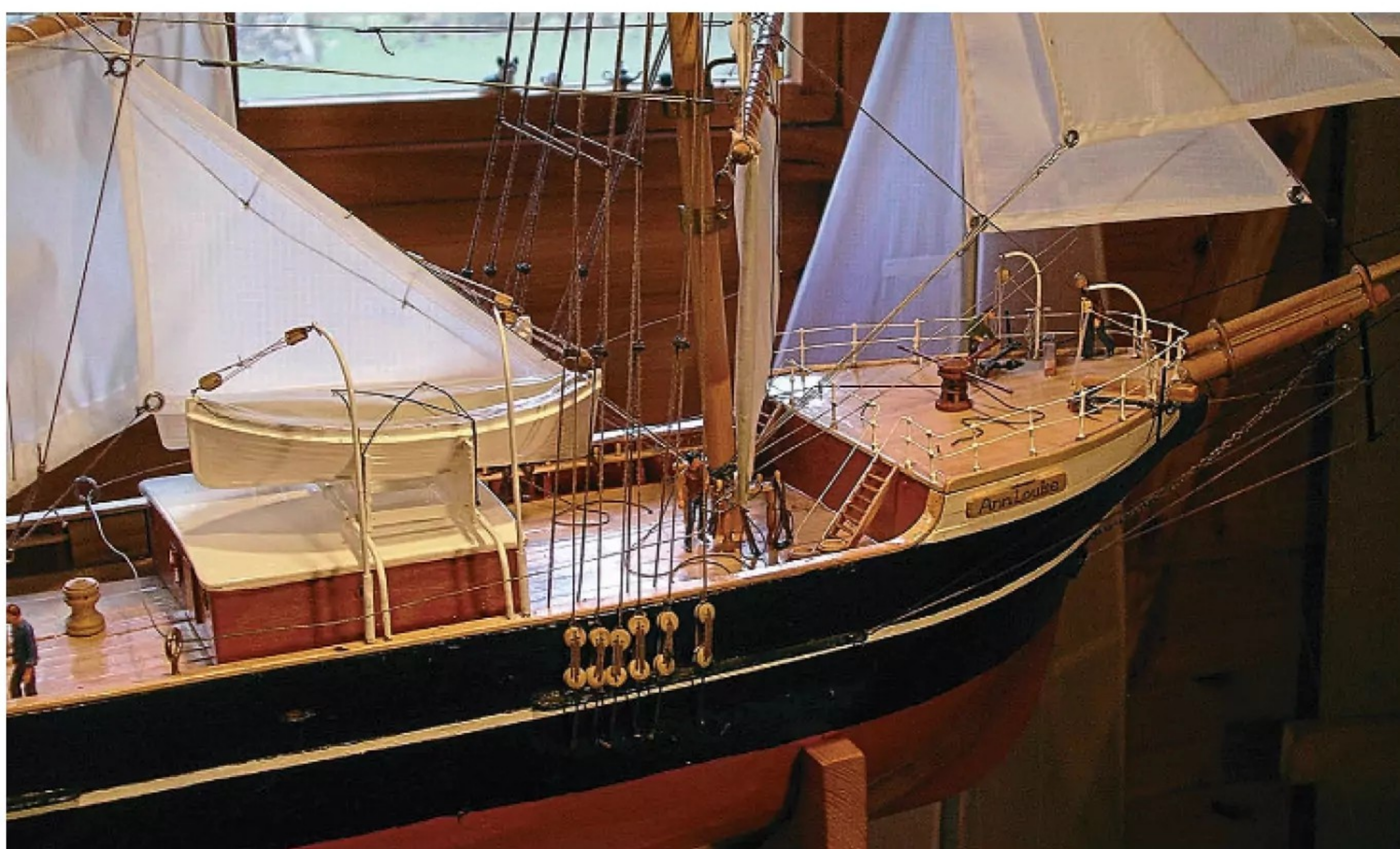
As modified, the boats are much more to scale, the handrailing is complete, and there has even been room to fit two anchor davits on the fo’c’sle head.
