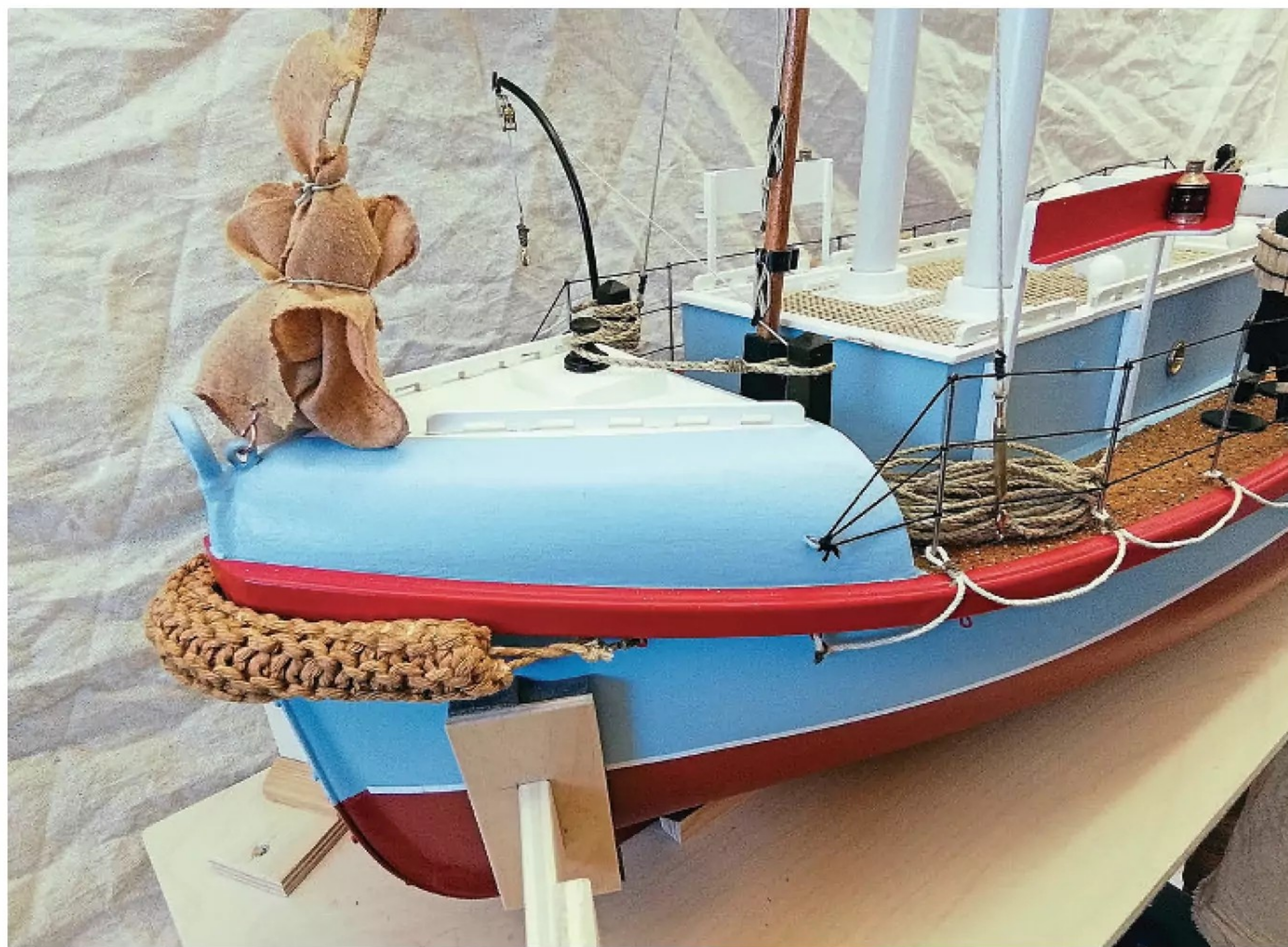
The mast fitted, with a crumpled-up bit of old cloth representing the foresail. Note also the guard rails along the side decks, these having been made from stainless steel rod, notched and thread twisted around each stanchion.
