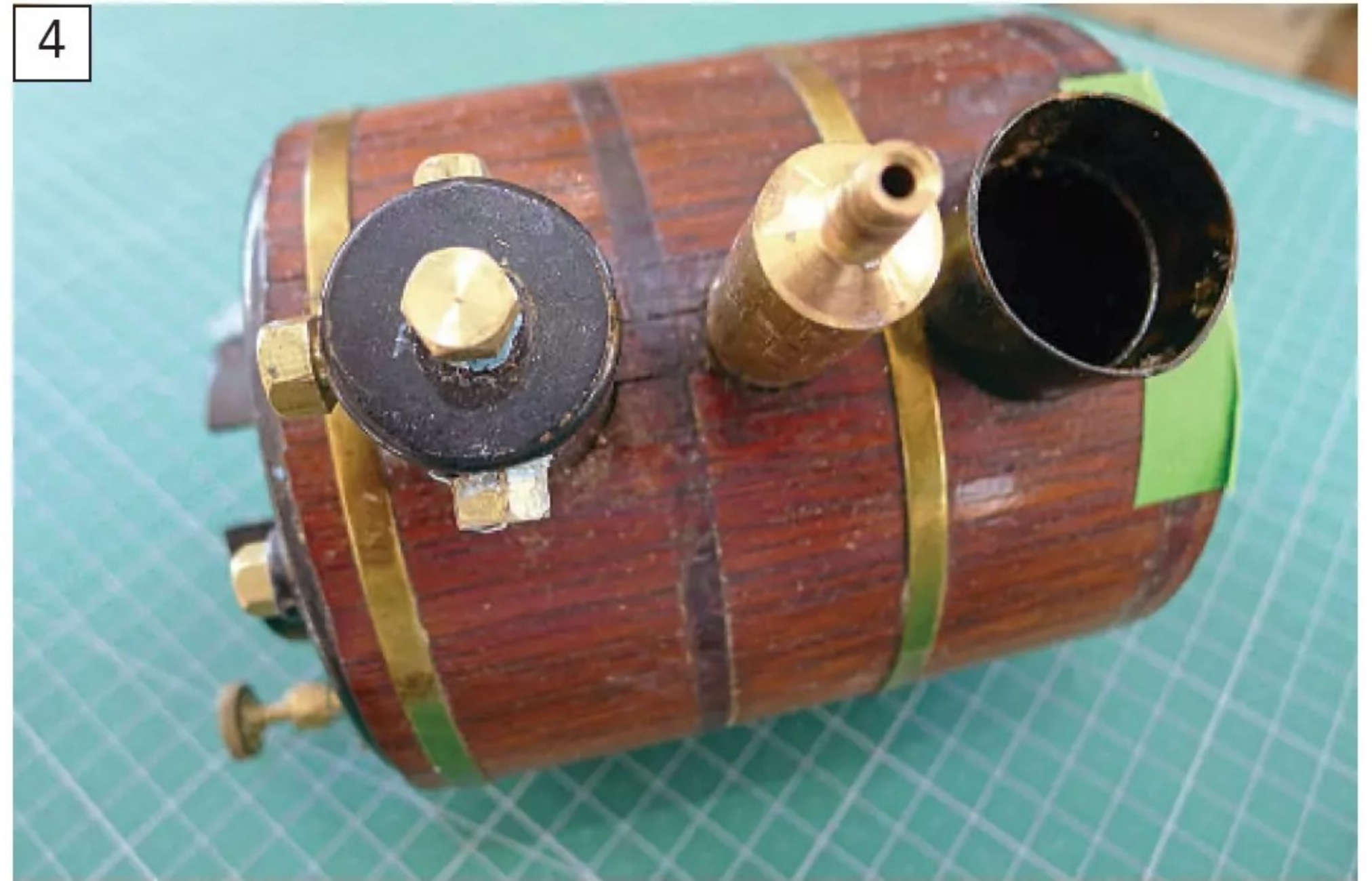
The boiler was presented with plugs in all the bosses, an isolating valve for testing if I chose to use it, plus an adaptor had been made and fitted to the safety valve fitting to make life even easier. Richard had already decided that this shouldn't take too long!
