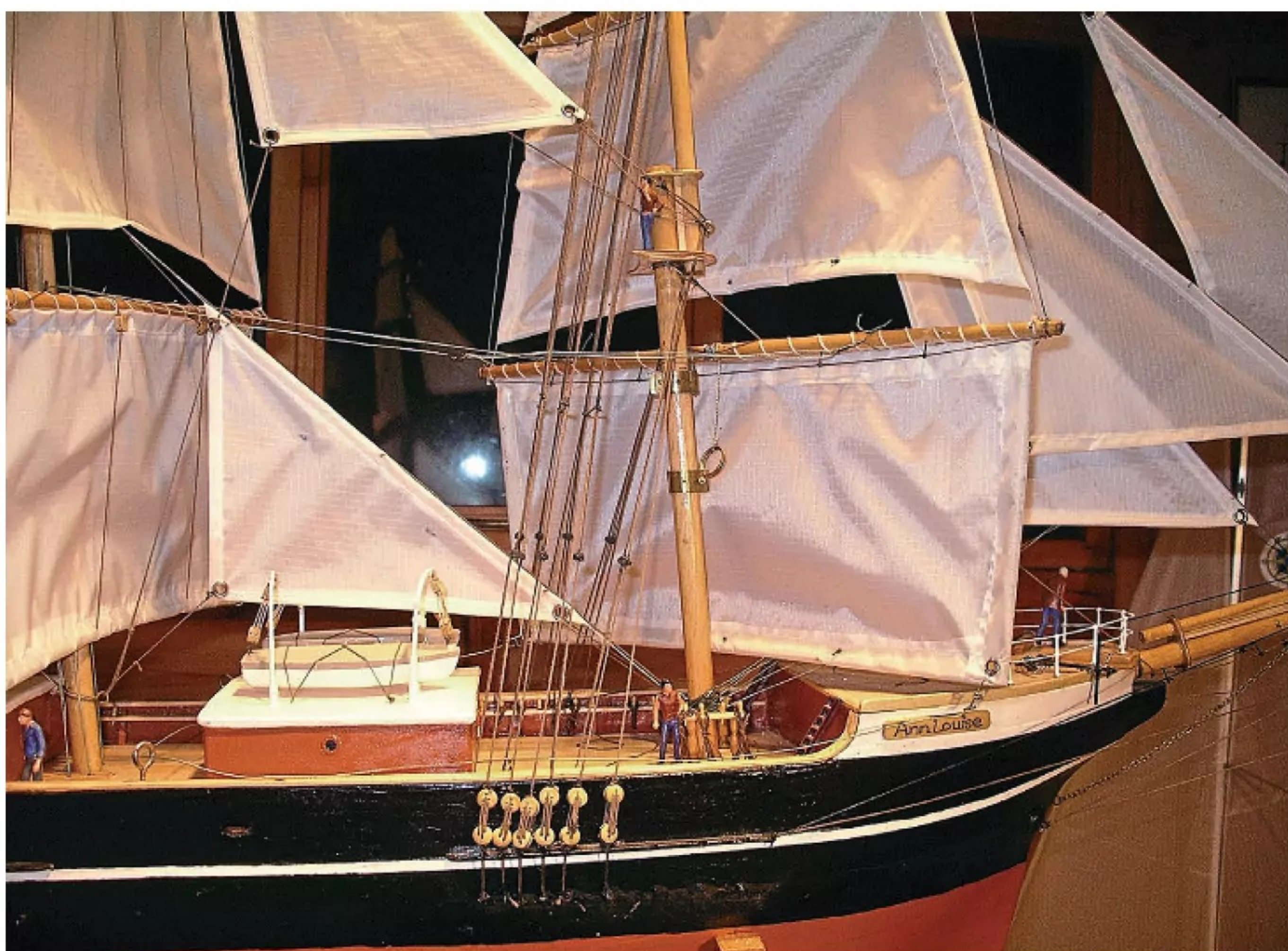
The miniscule boats and peculiar davits on Ann Louise as first built. Also, see the missing fo’c’sle handrails, where the foot of the foresail is.
