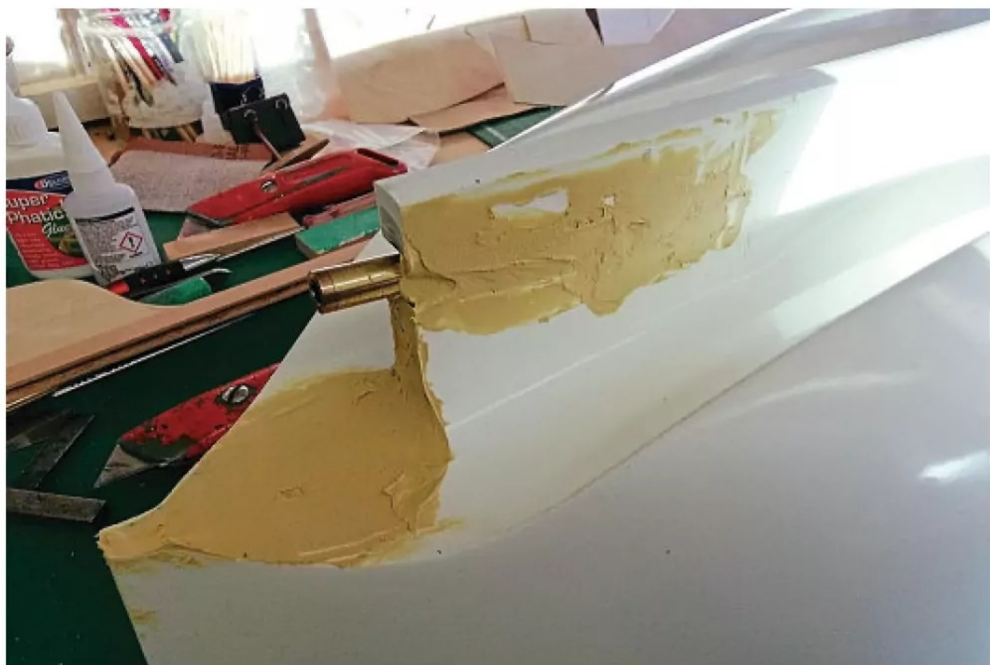
The gaping hole was filled with P38 filler and the propellor shaft bonded in. John approached this latter task with some trepidation, as he knew that if positioned at the wrong angle or slightly off-centre line he would be in big trouble!
