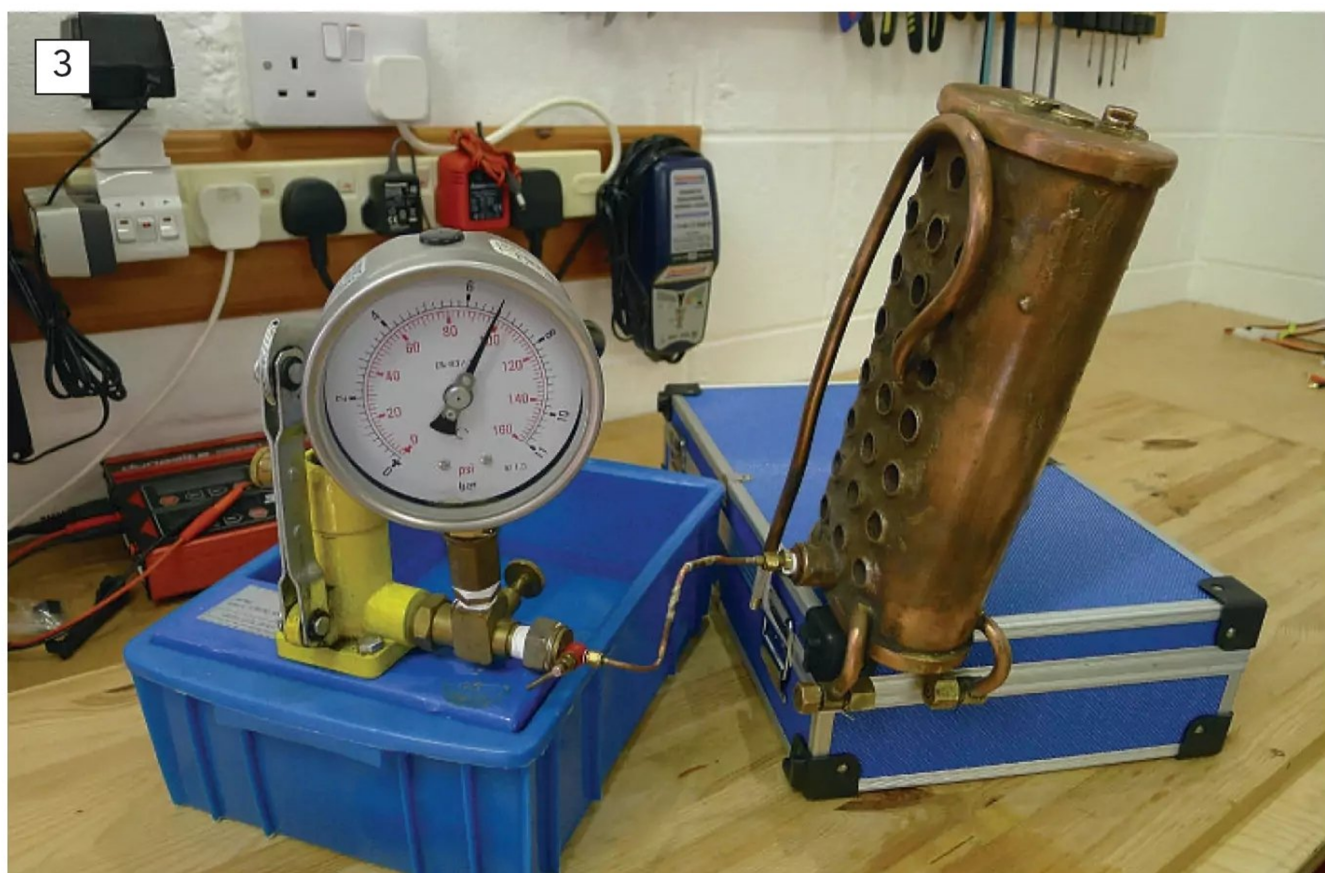
3 Sometimes Richard is asked to simply conduct a brief test to determine whether it's worth setting up properly for a certificated test. In this case, sadly, the boiler had a number of leaks that were not considered as economical to repair.
