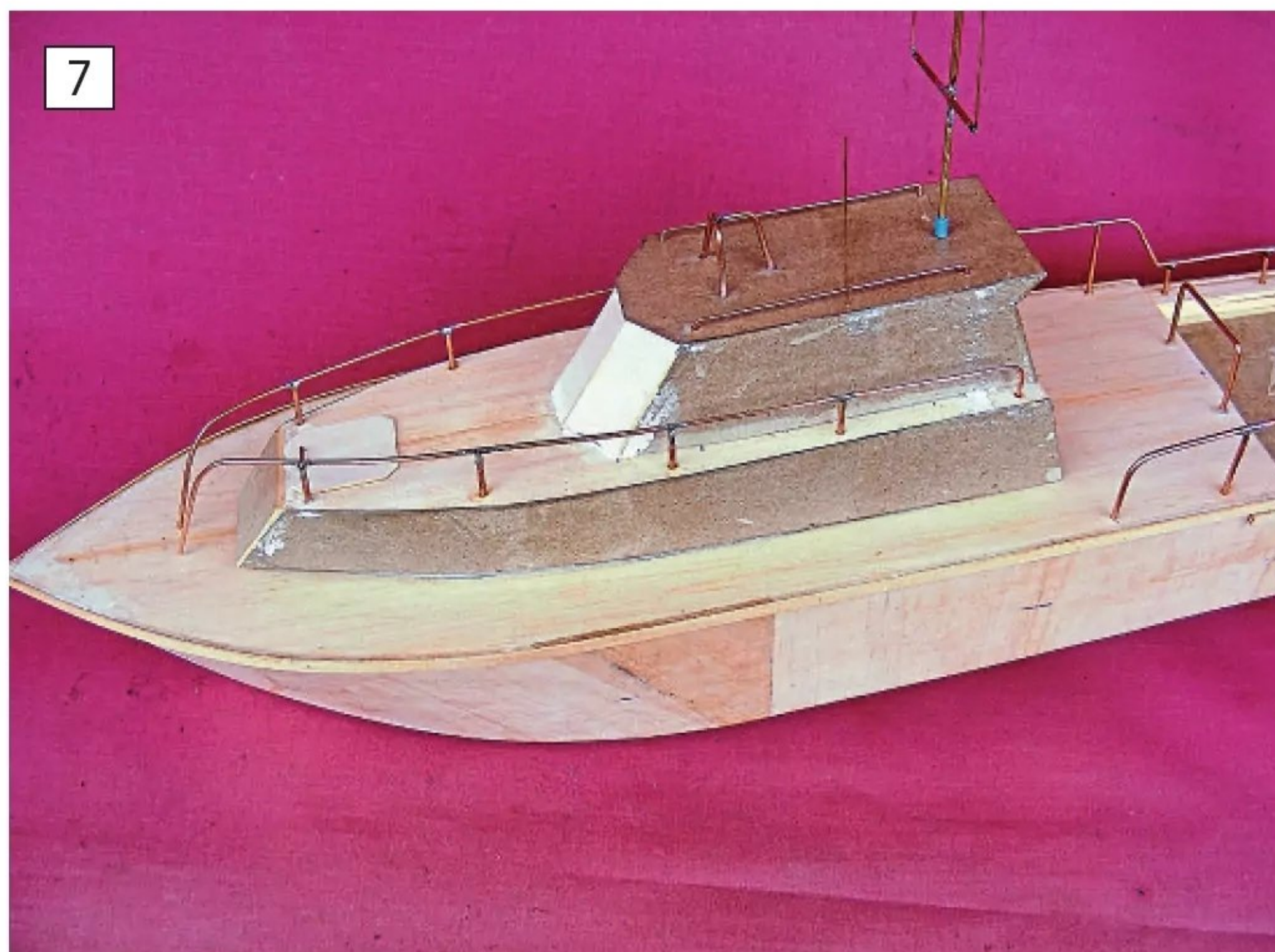
Stanchions glued into deck/hull before adding rails.
