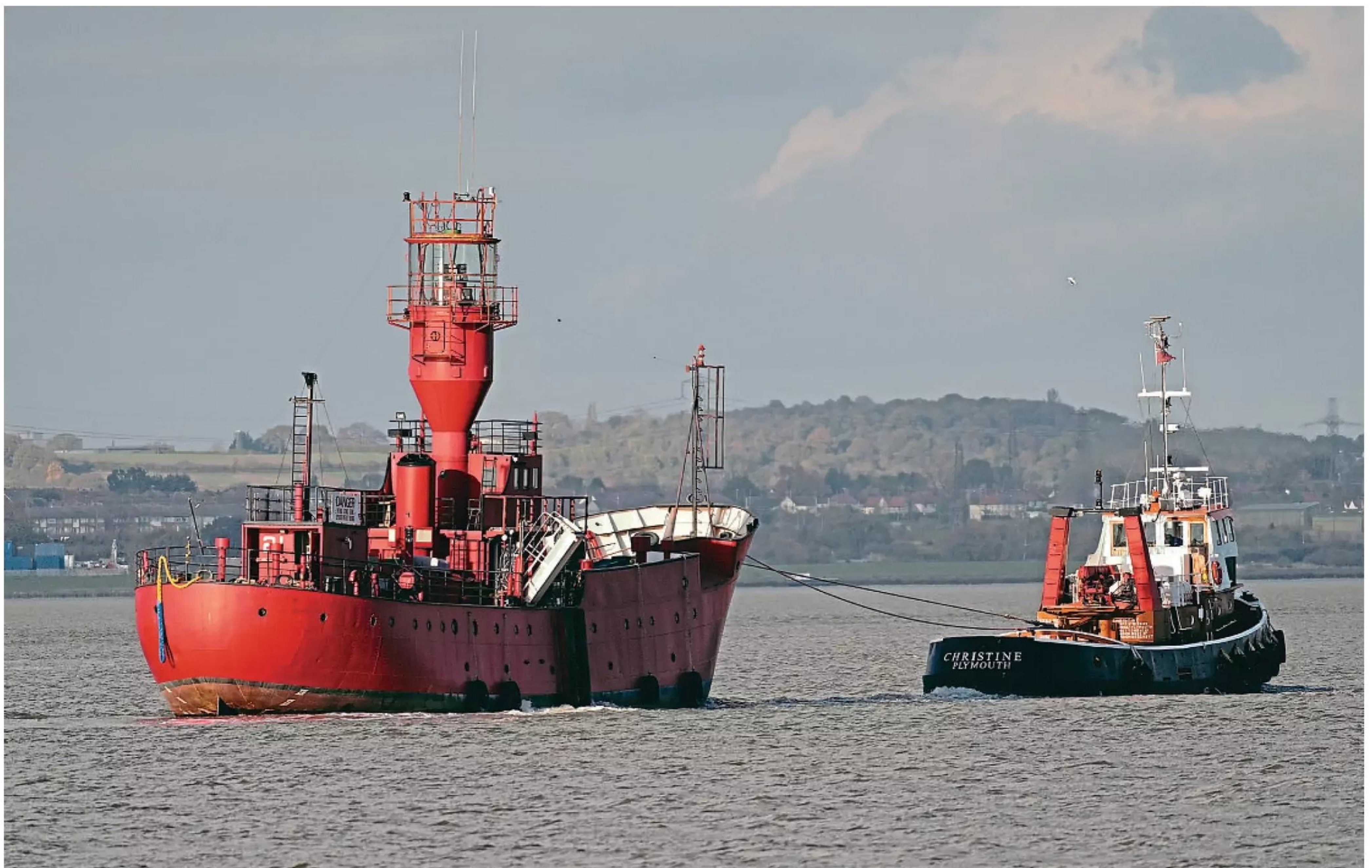
Christine carefully towing LV 21 in the Thames estuary. As LV 21's engine has been removed as part of her conversion, the light vessel is reliant on the tug to navigate the tidal waters of the Thames and commercial vessels inbound to the Port of Tilbury and London Gateway Port. Note the visitor's gangway and tyres placed along her hull to prevent damage. These are necessary modifications for the light vessel's new role as a floating art and performance venue.
