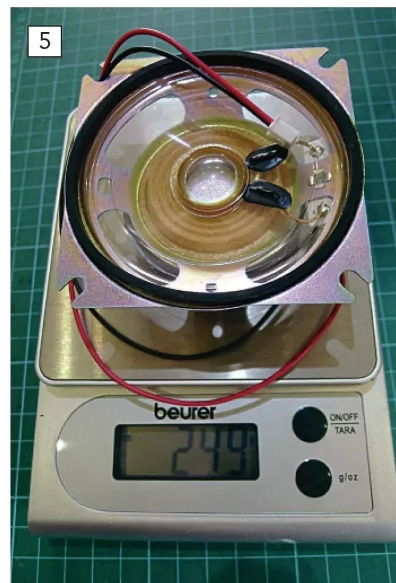
The speaker could be a bit more limiting, especially in a small model and particularly if mounted high in the hull, weighing in at just under 250g.
