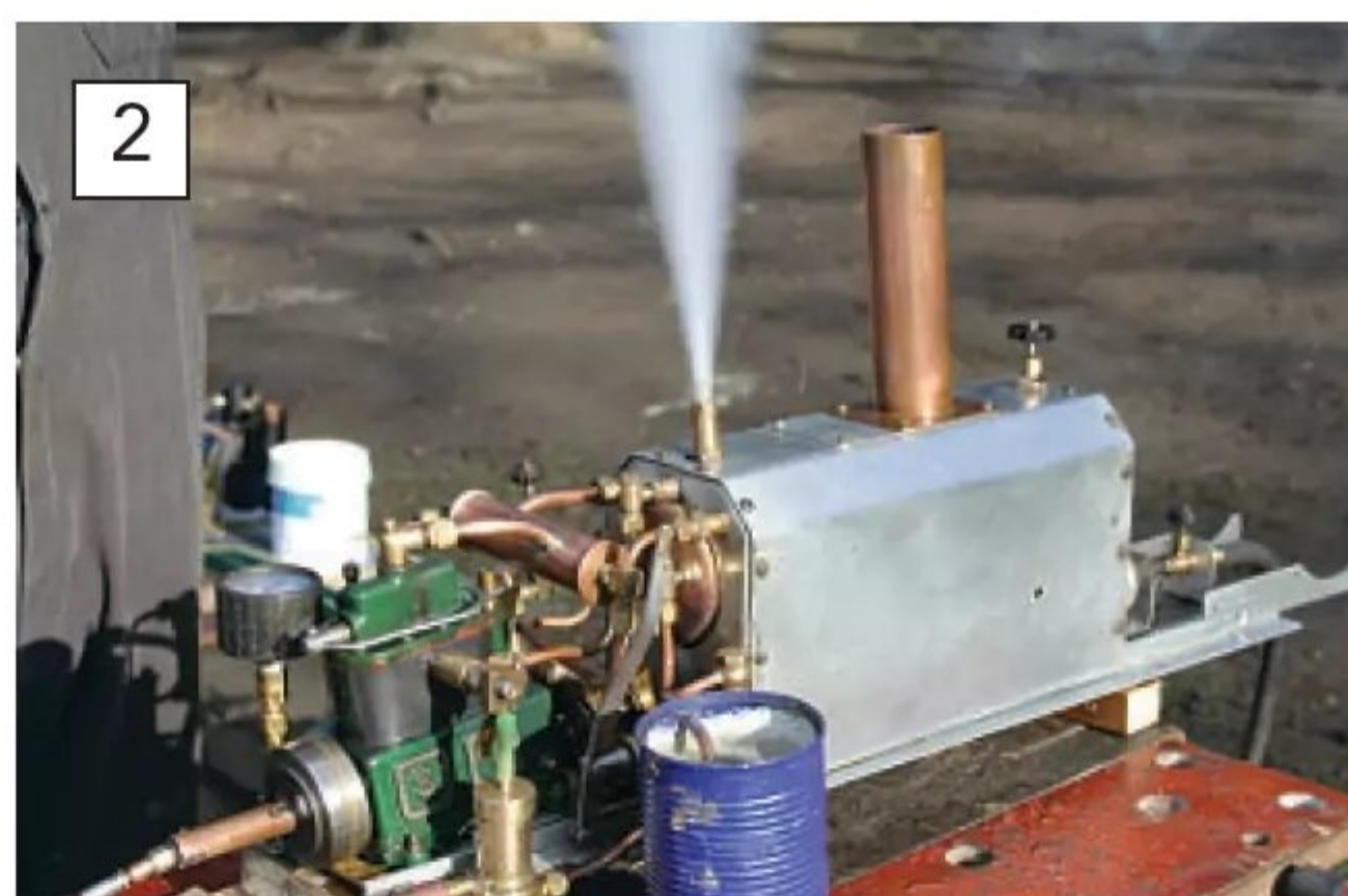
2 An annual steam test is easily conducted at the pondside and, if the plant is in a boat, it can be dropped into the water for a run. In this case, the engine is simply running down the pressure to close the safety valve which has successfully lifted.
