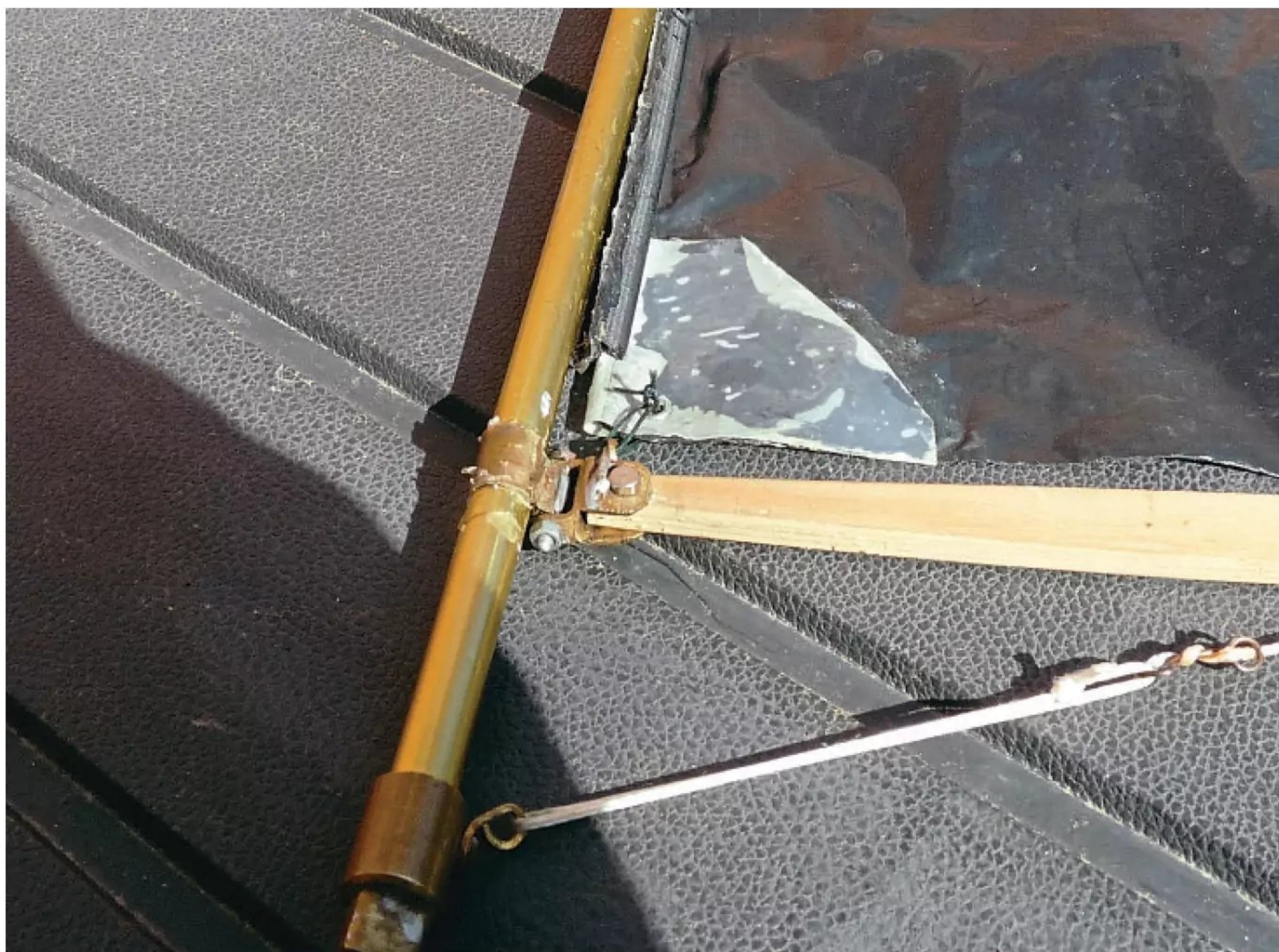
A close-up of the goose neck showing kicking strap with wire bowsie.
