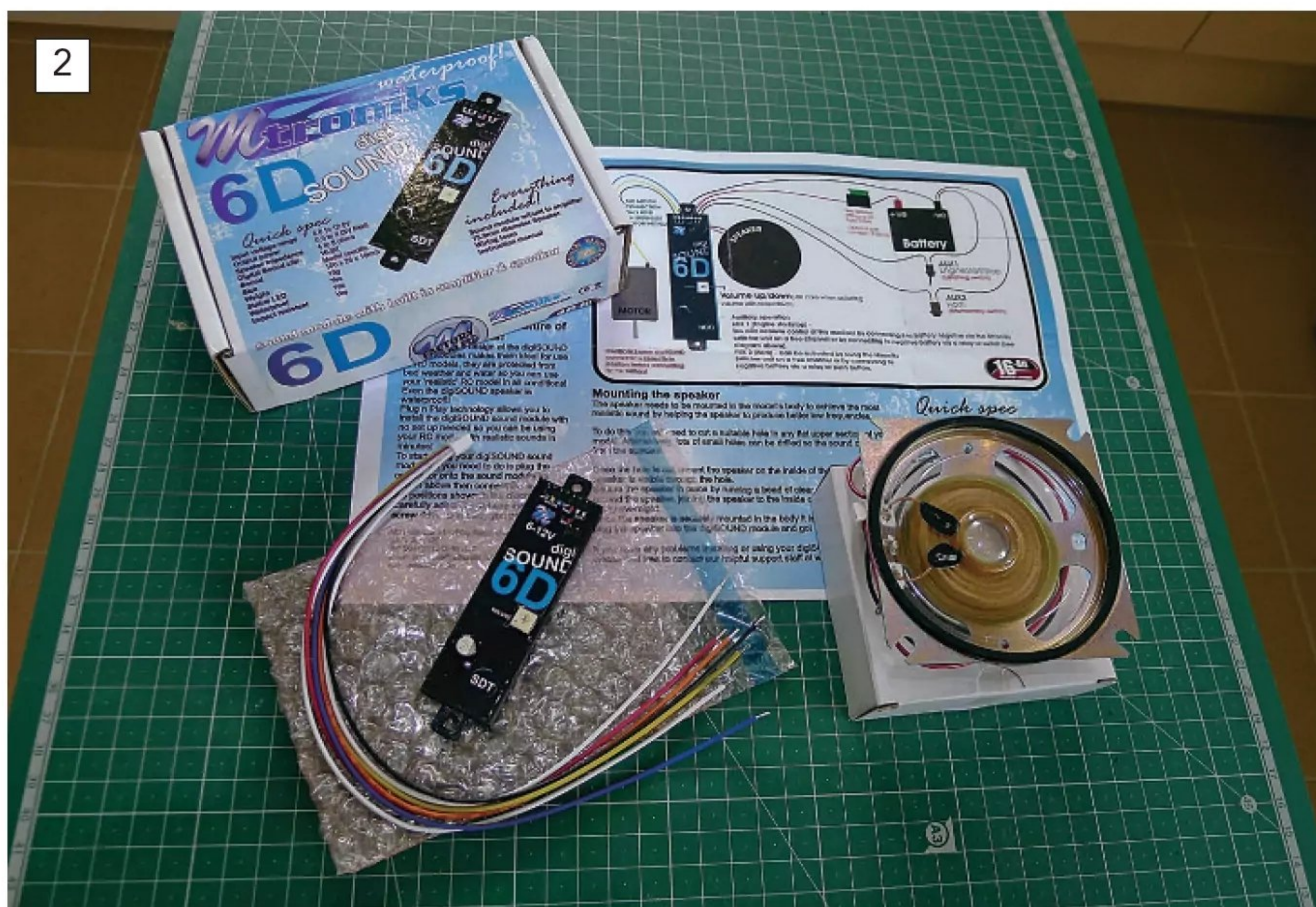
The Digisound 6D bits and pieces as they arrived. Almost all the weight was taken up by the speaker, which is a substantial piece of kit and is robust and waterproof.
