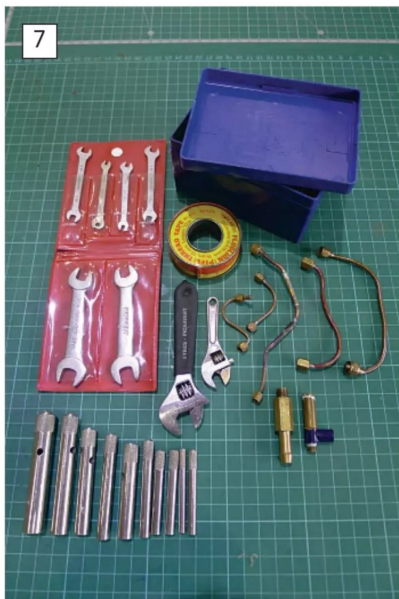
Richard's other box contains a number of spanners, PTFE tape and an assortment of pipes. Owners frequently make use his spanners to remove pressure gauges when they've forgotten to bring their own with them.
