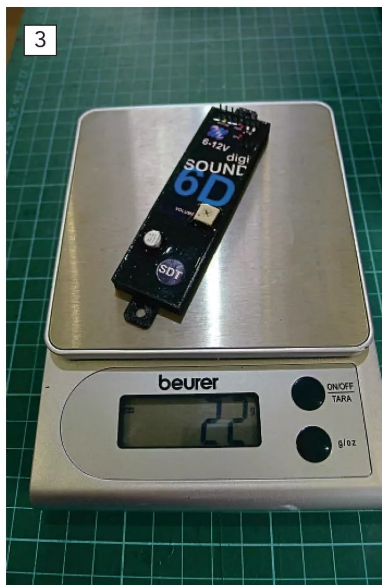
The actual Digisound 6D control unit. At 22g it can probably be squeezed into a very small model with an appropriately sized speaker.
