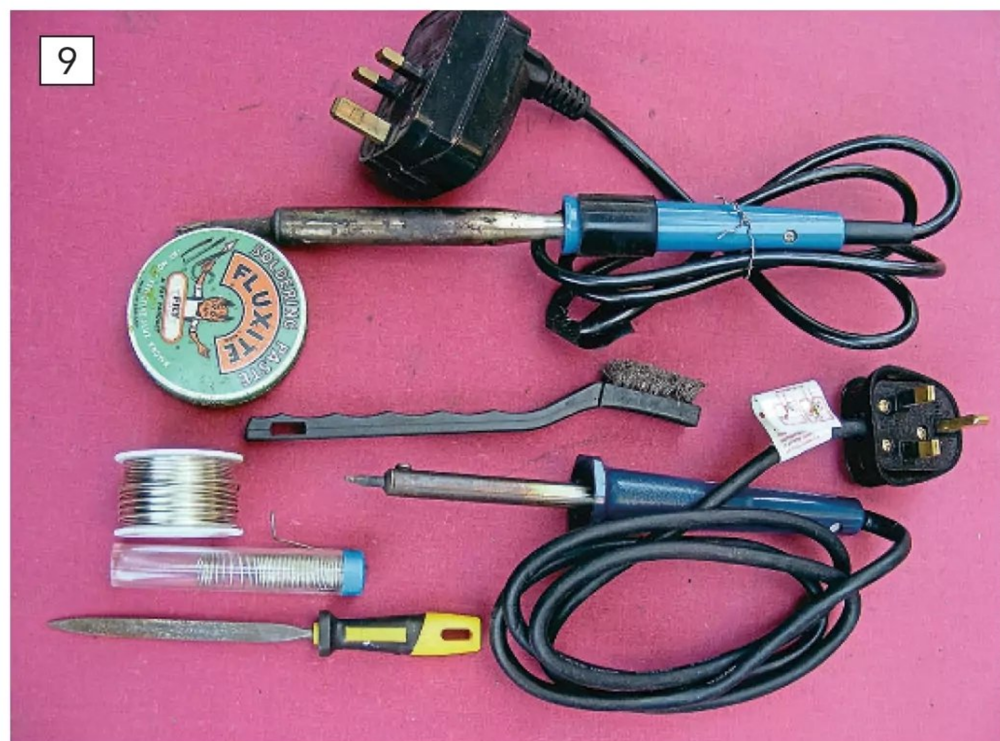
The kit needed to solder copper railings.
