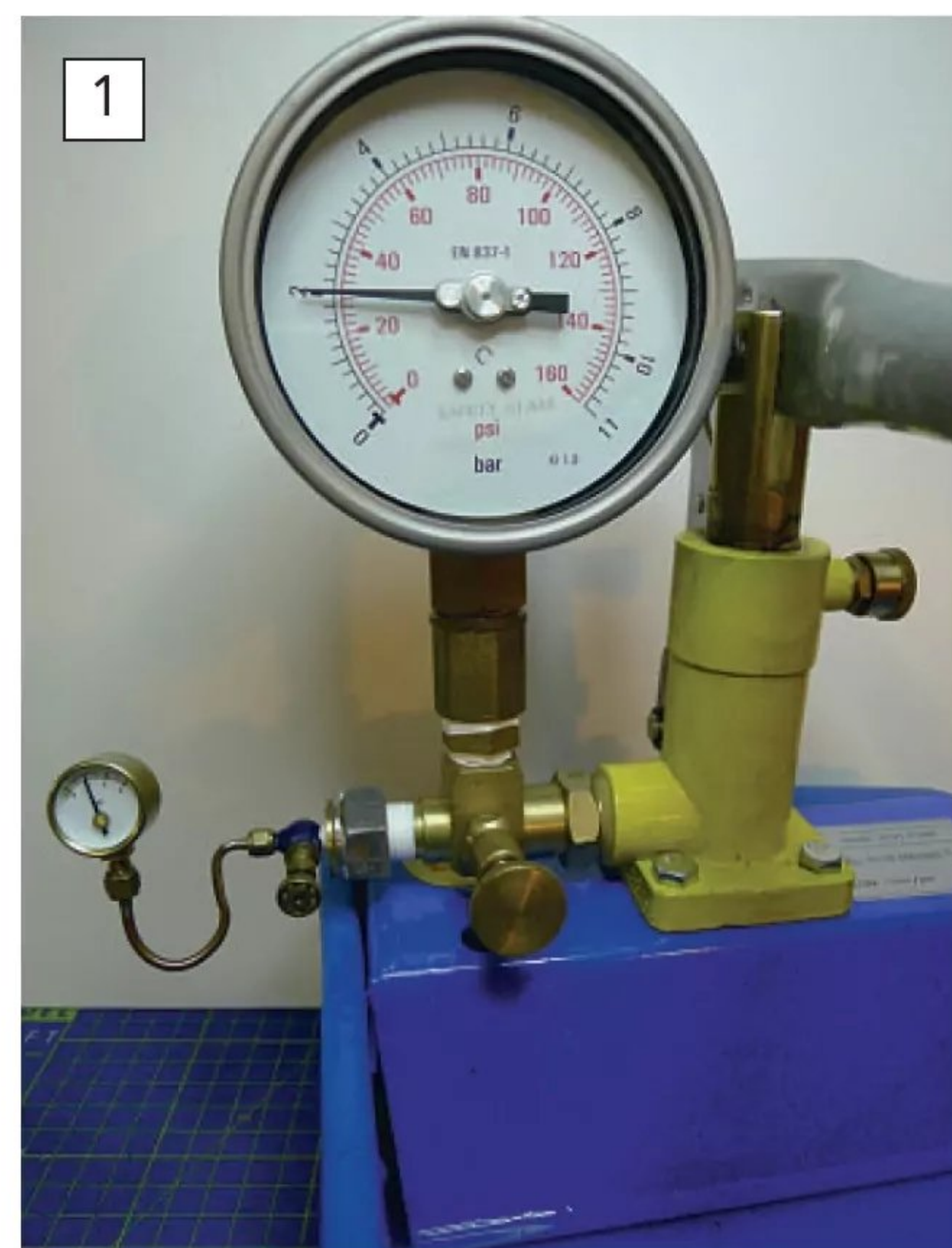
1 There's no point in checking the safety valve lifting pressure if you can't rely on the pressure gauge, so the first step is always to check that the gauge on the boiler is reading correctly. Richard takes it up and down in increments, twice.
