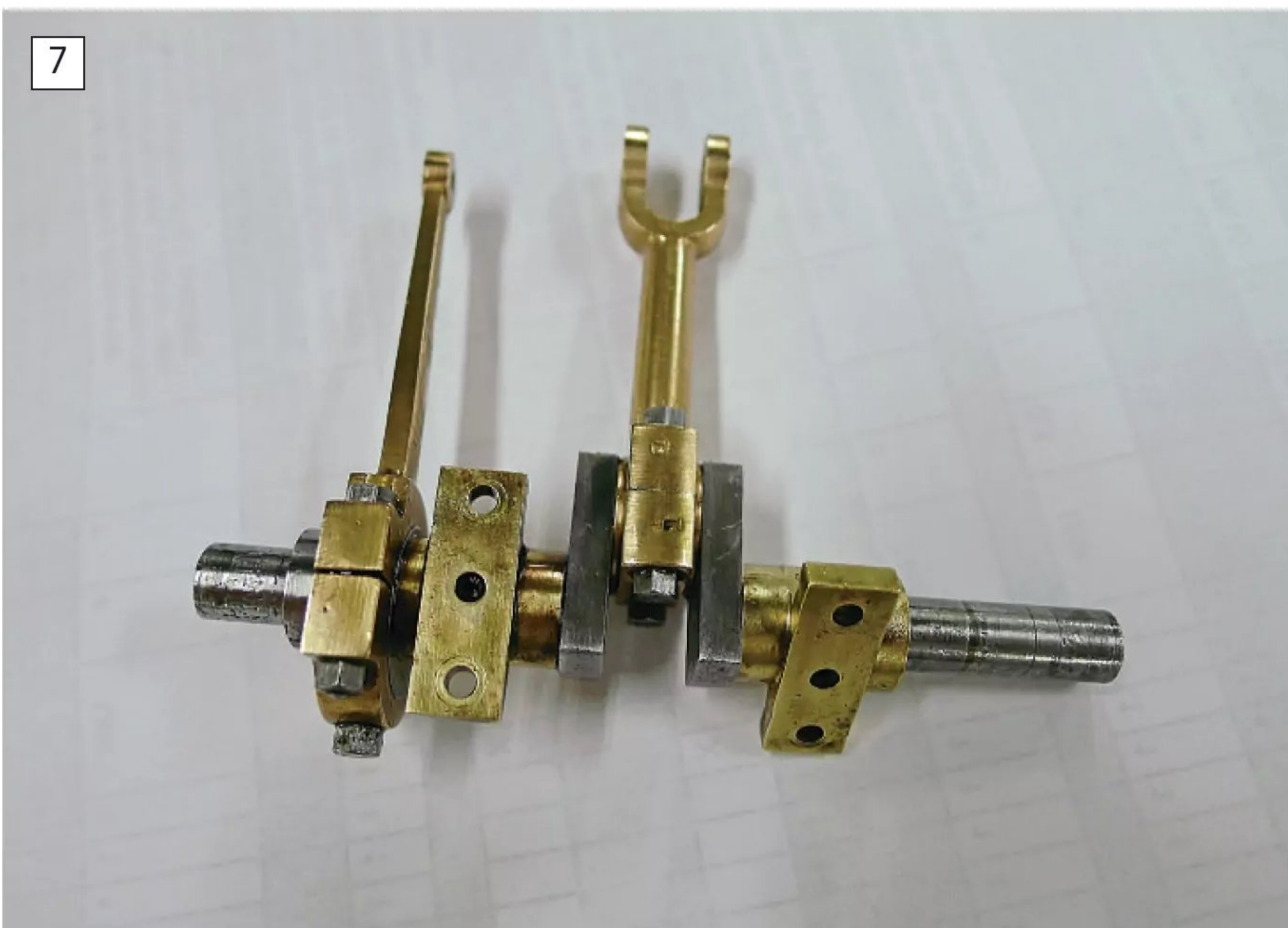
A considerable amount of time went into the careful cleaning up of the 10V's running gear. The result, however, was worth all the effort. Things were free without being slack, so luckily the bearings did not need sleeving.
