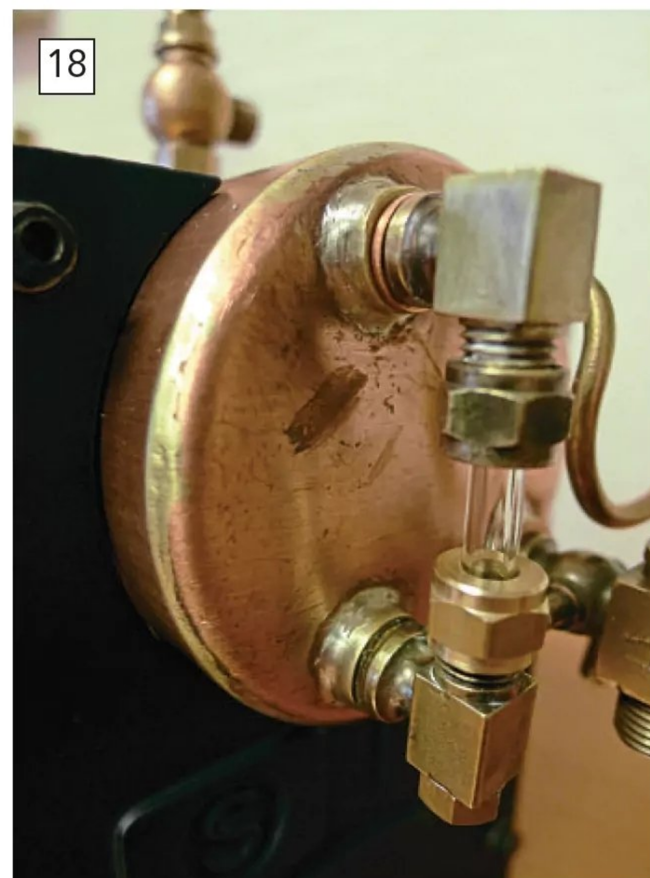
Very oddly, the fittings on the boiler were mounted directly into the threaded end plate – most unsatisfactory. Consequently, bushes were made and silver soldered to the shell to give a much stronger fit.
