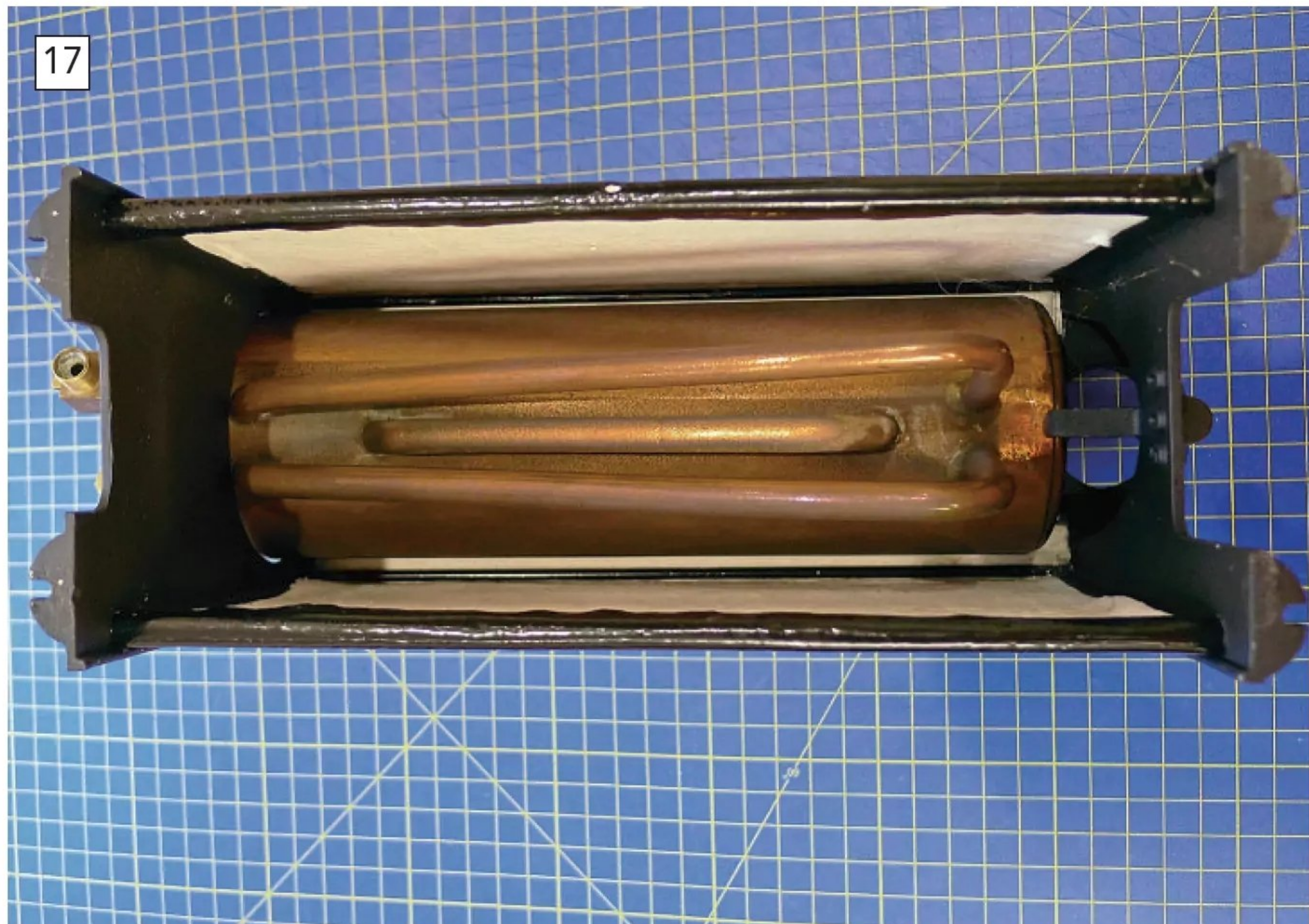
The Stuart Turner range of boilers are identified by the number of external tubes in the burner space. Three tubes mean you are looking at a Stuart Turner 500 boiler.
