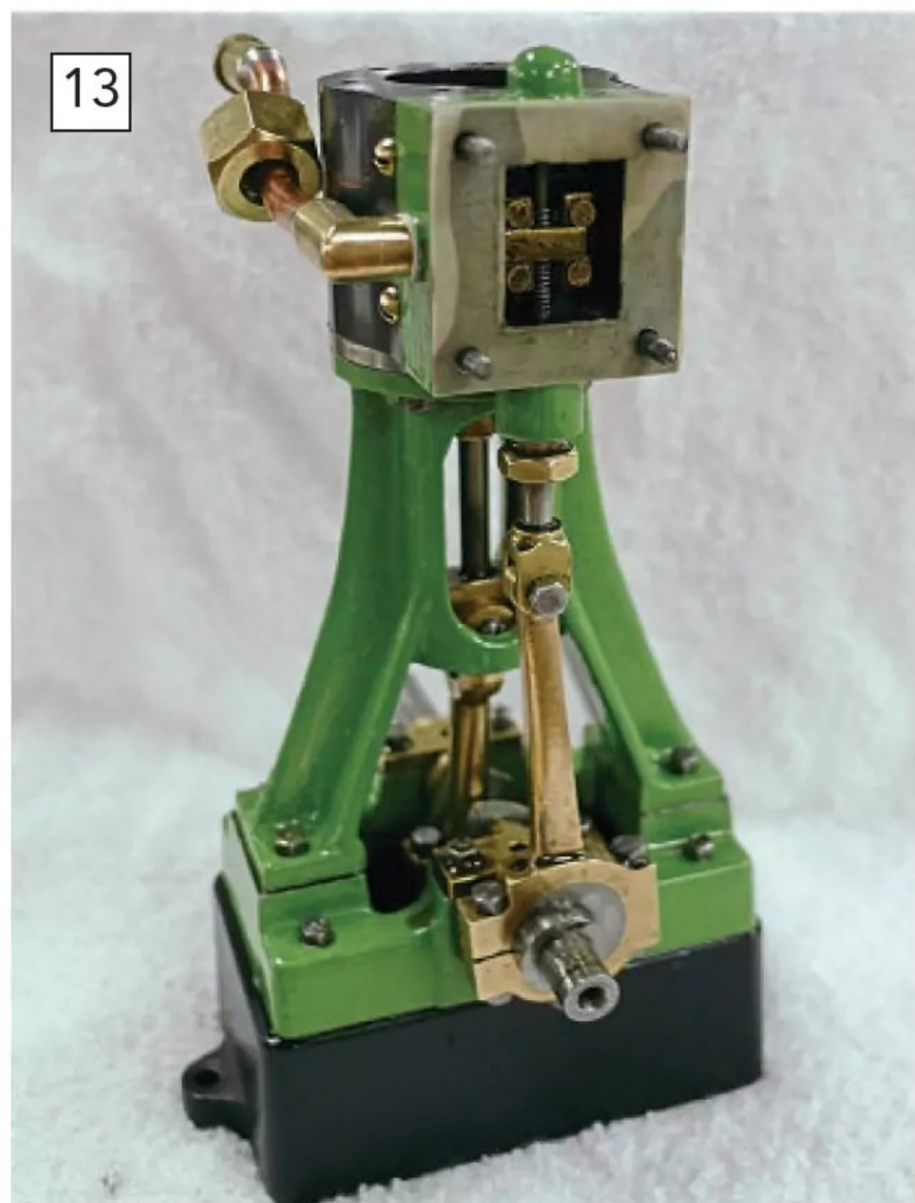
Setting up the piston stroke: the timing went well, probably as a result of the high standard of original manufacture. The slide valve was set centrally and the timing judged by the port cut off.
