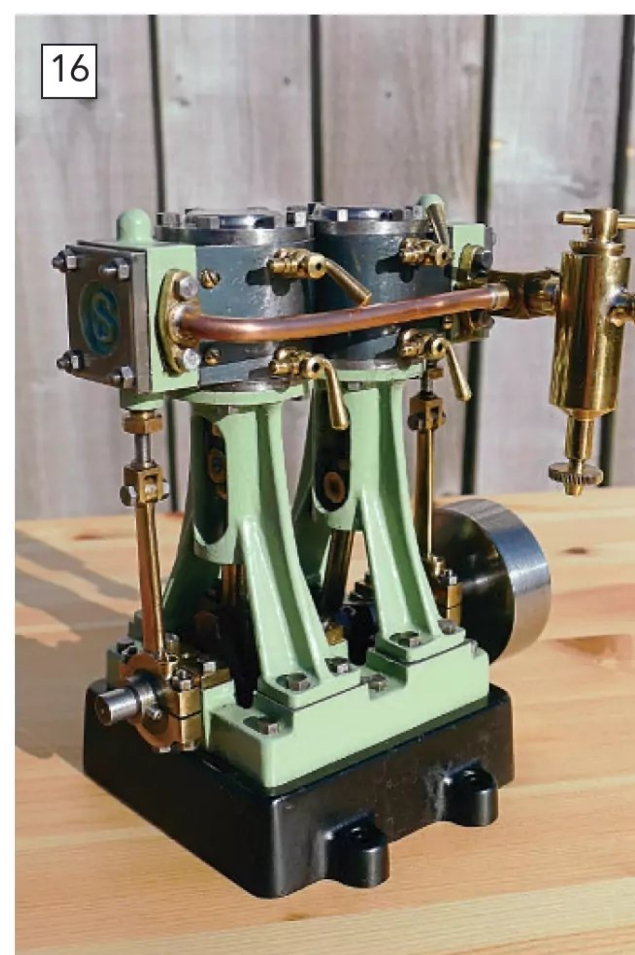
Richard replaced the homemade engine with this secondhand Stuart Turner D10. Being well made and in good order, it simply required a clean and repaint to match the rest of the plant.
