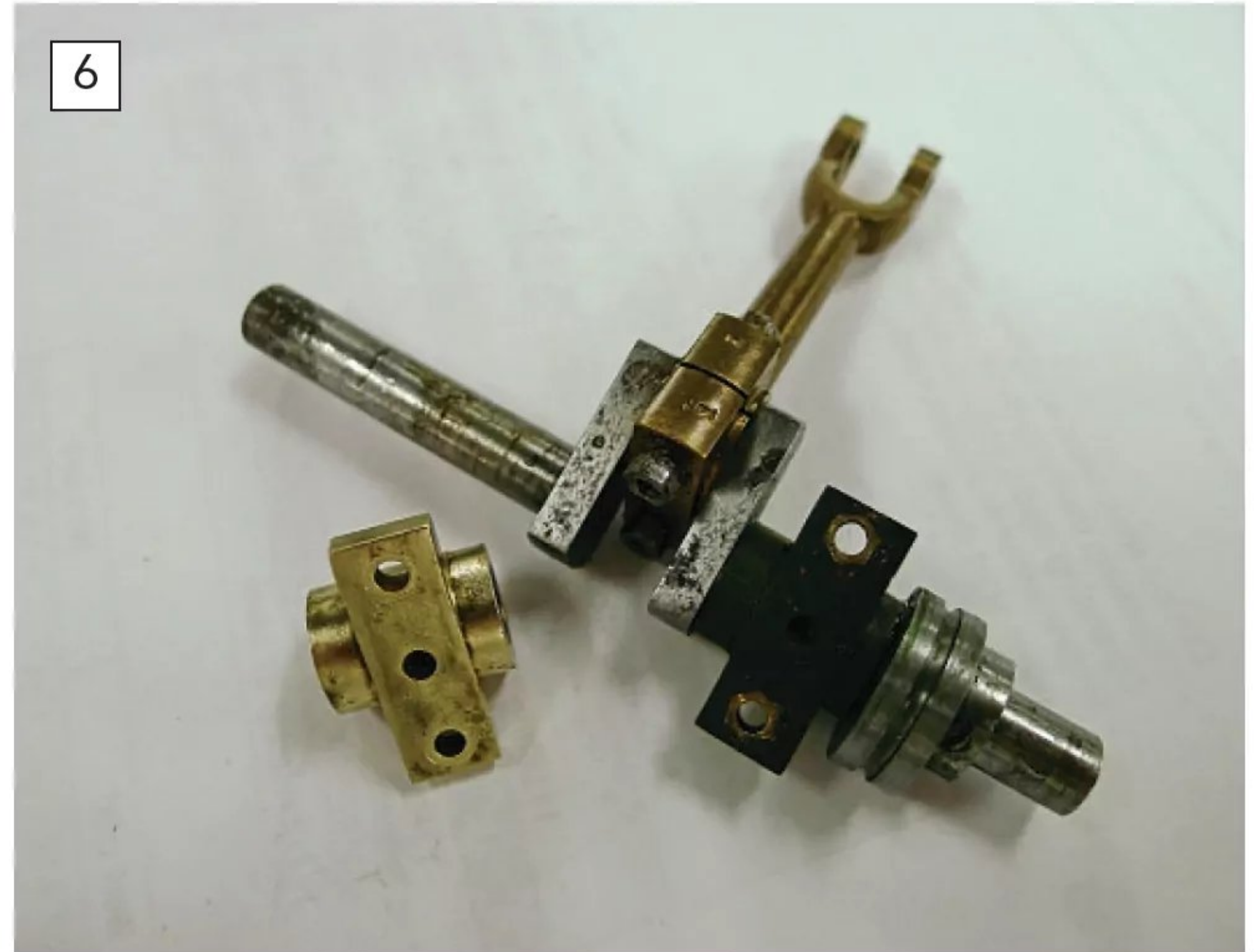
Part way through the restoration of the 10V's running gear; the removed bearing has been cleaned, while the remaining bearing clearly shows the thick build-up of dirt.
