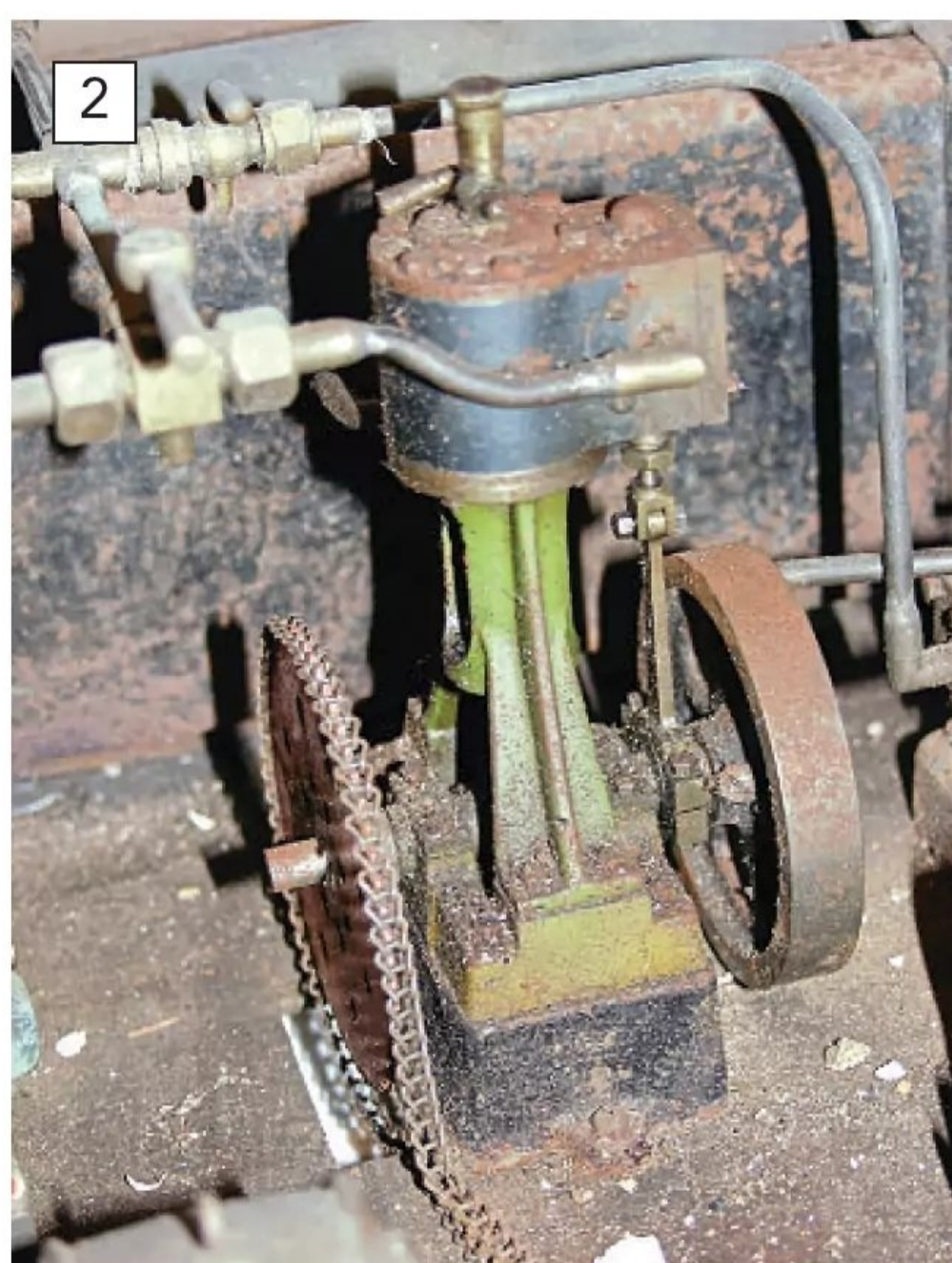
The 10V engine was seized, rusty and covered in solidified lubricant and filth. At least it still had the drive chain, which was intact, although also rusty.
