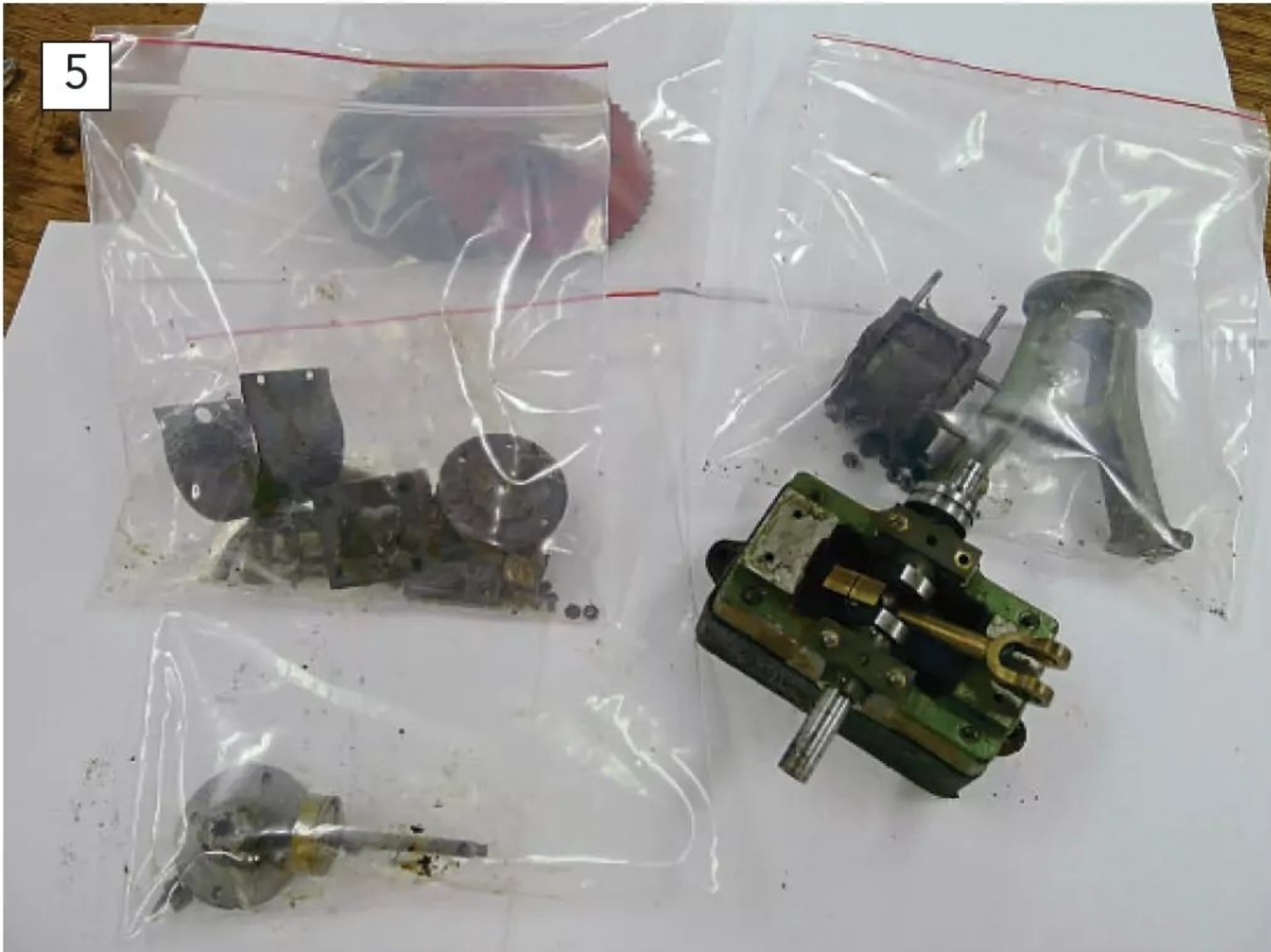
Stripping the 10V down revealed the sheer amount of work required simply to clean it up. Everything was bagged to keep the bits together. Some parts, such as bearings, had already been marked up to ensure they were refitted in the same way.
