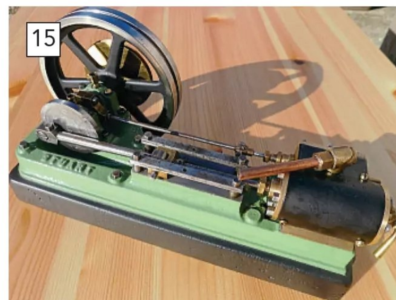
The S50 went through a similar process, with particular care being taken when dismantling the crosshead and guides. At least with this engine you can get access to the sliding faces for a good clean, and the fit can be altered by adjusting the height of the crosshead mounting screw spacers.
