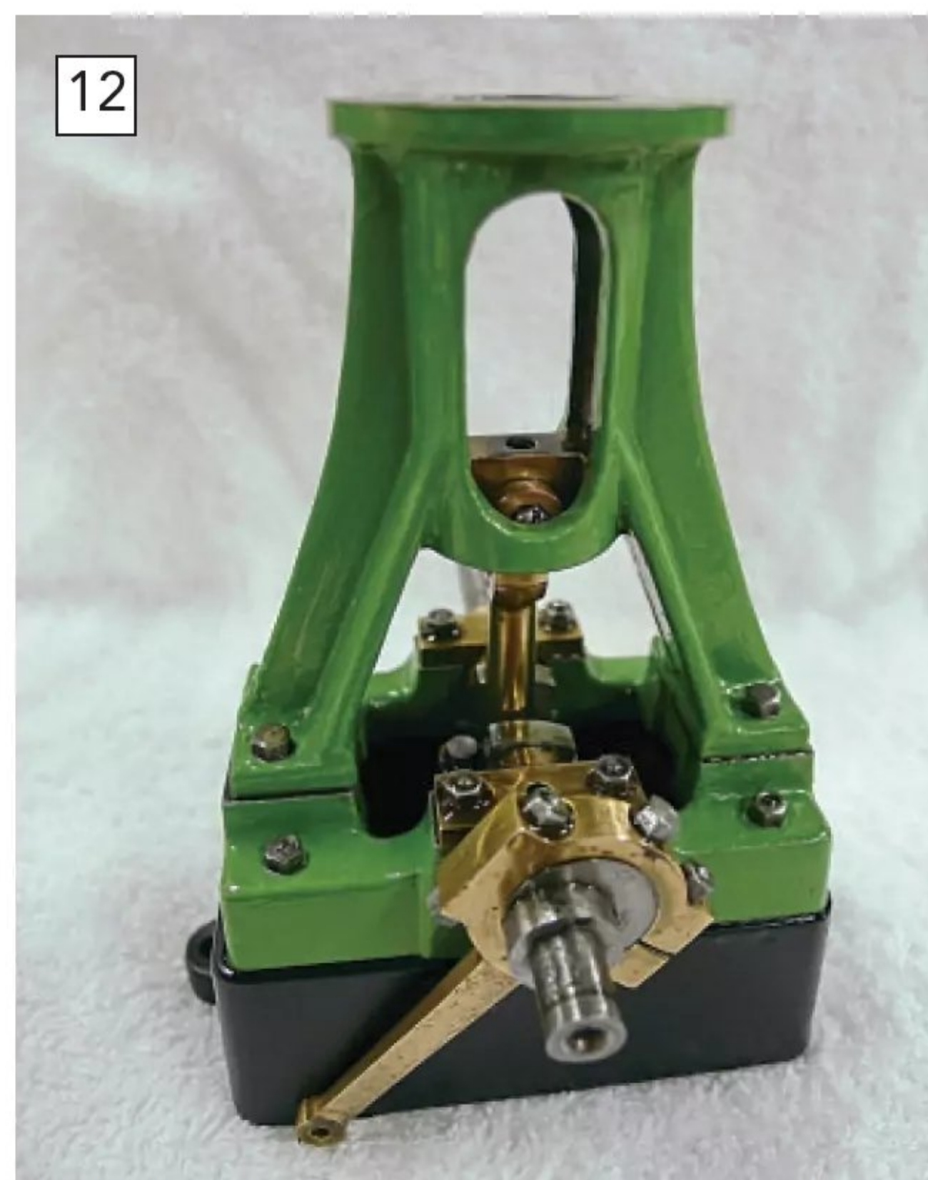
Further reassembly revealed that the crosshead and guide was a decent fit and the engine turned over nice and smoothly. It had probably not done so for many years.
