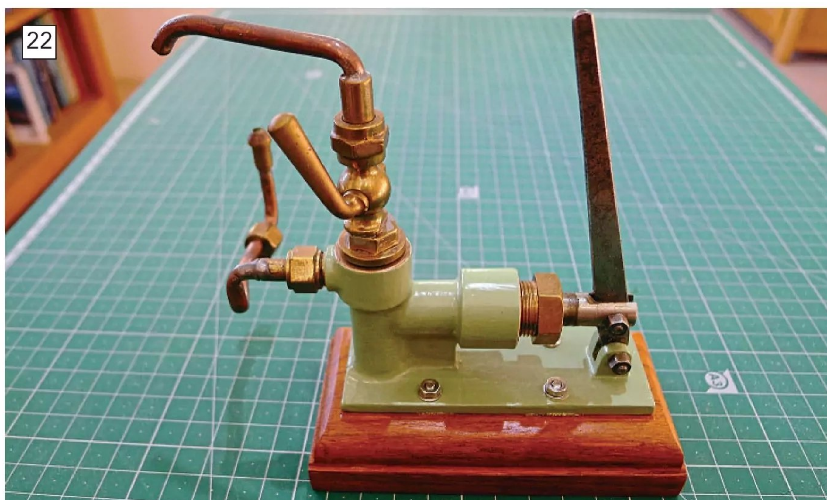
The water feed pump was generally in good condition once the ball bearings were removed and everything was cleaned out. The seats weren't perfect, but they looked good enough to use without recutting. Time will tell!
