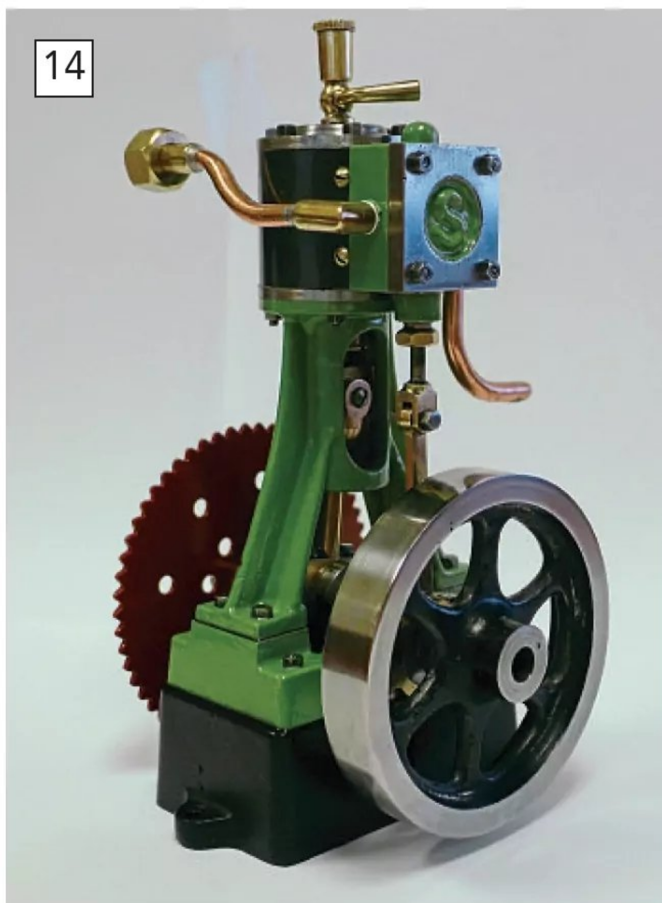
Back to looking how it should! When trialed with compressed air, the 10V was found to run very smoothly on very little air pressure. Even the flywheel and the chainwheel ran true. So, after a lot of work, a good result.
