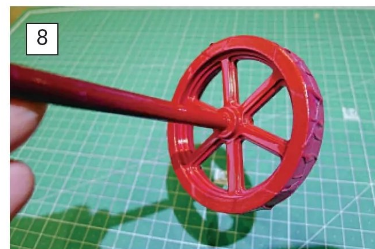
The flywheel was also given a couple of coats of red at the same time. In this close up you can see the kind of surface finish that can be achieved with just two primer coats and two topcoats.
