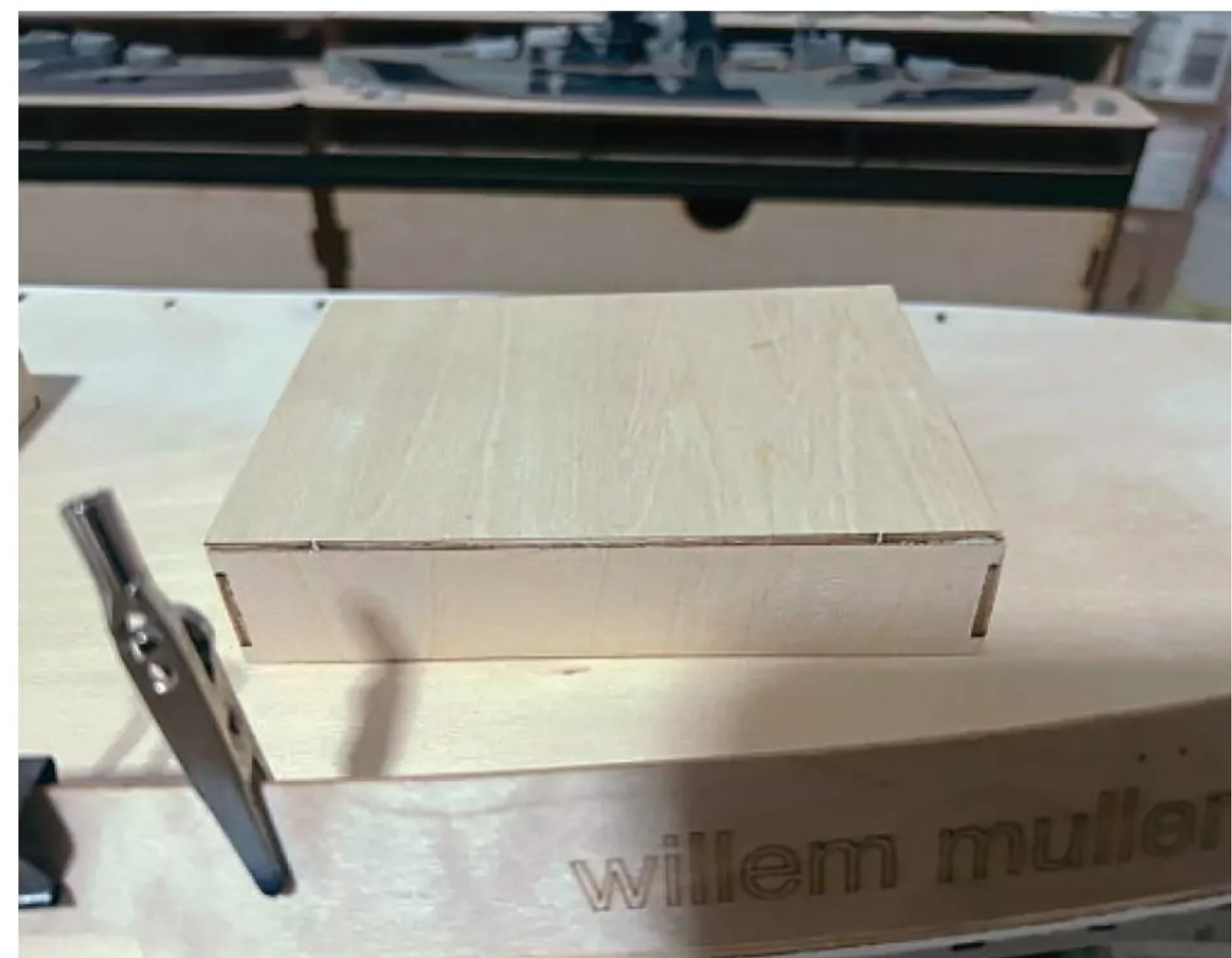
The laser cut plywood is a dream to work with; it's easily removed from its backing sheet and locks together allowing the rapid build of basic structures.
