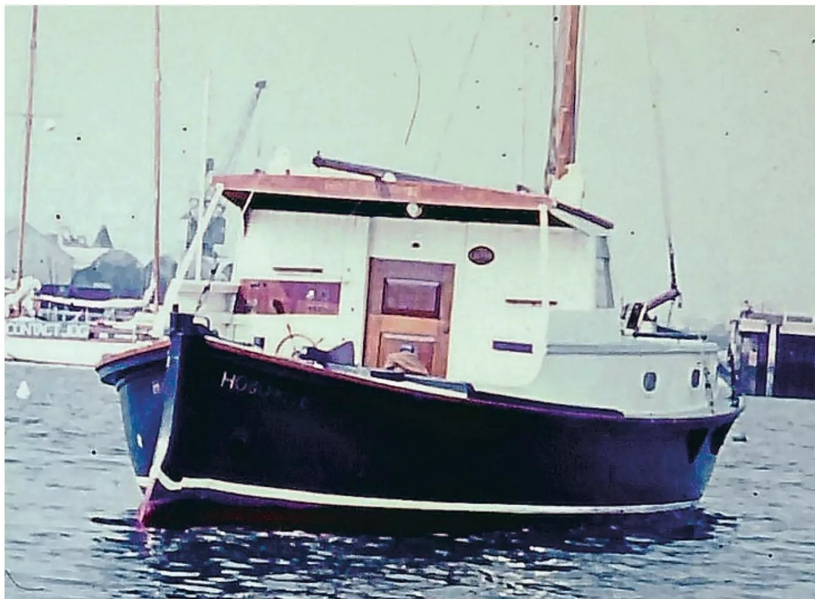
A rear shot, showing the wheelhouse and John and Mike's method of securing Hobo when left on a mooring; closing off the view from the wheelhouse served as a simple but effective theft deterrent, as a thief would not be able to get at the controls or see where they were going.
