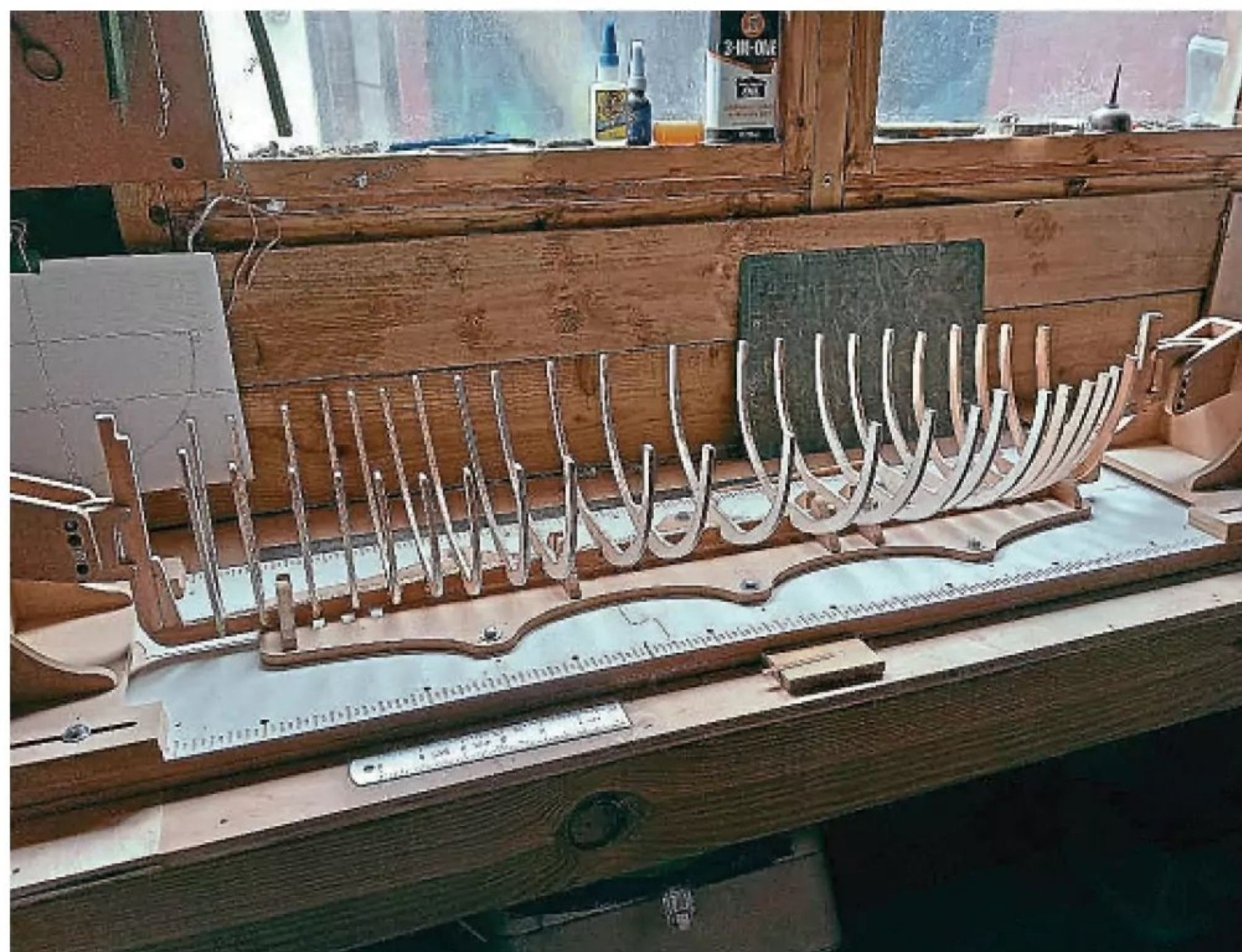
The building dock John purchased proved invaluable when constructing the keel. With everything held firmly in place, all of the frames cut out using his Dremel jigsaw could be glued into position.
