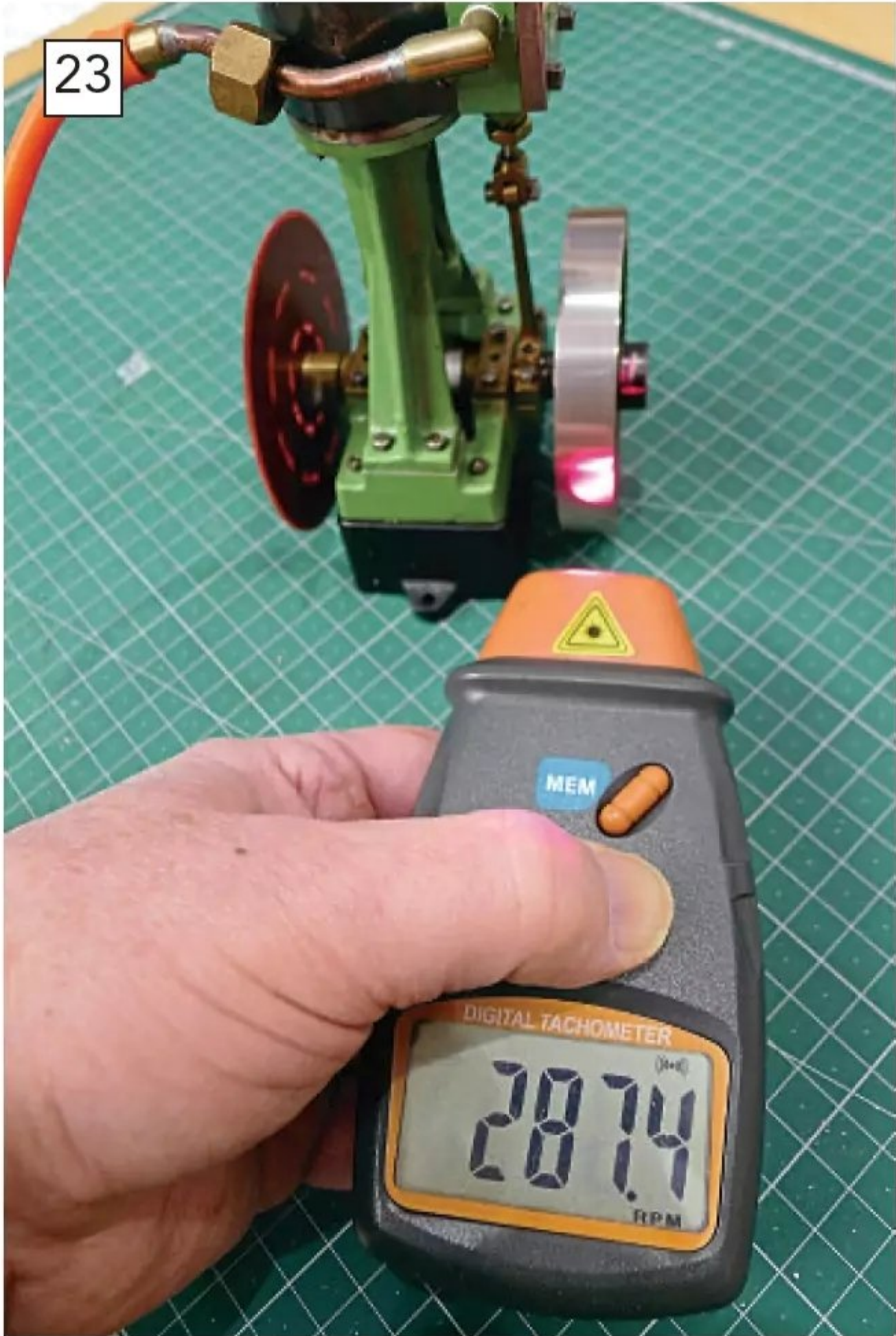
At exactly the same air pressure, the Stuart Turner 10V ran at 287 rpm. As the stroke is slightly greater, the torque will also be increased, so the 10V is probably capable of turning a larger propeller easier.
