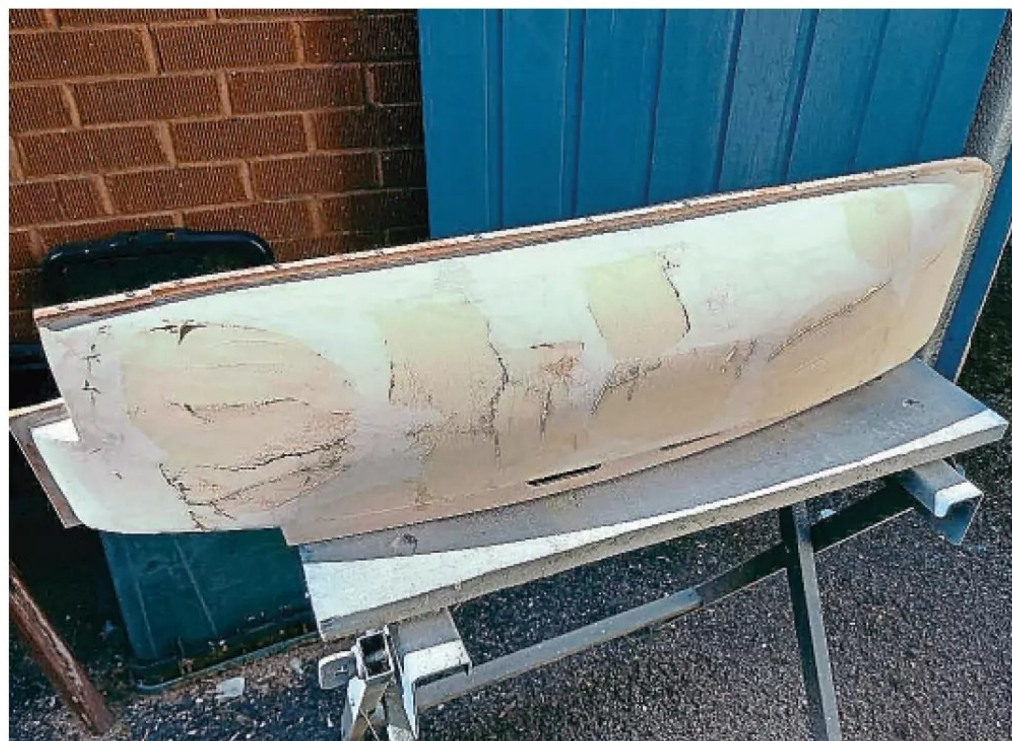
After the resin and matting had been covered with Isopon fibreglass filler, much sanding and filling ensued until John was happy with the final shape.
