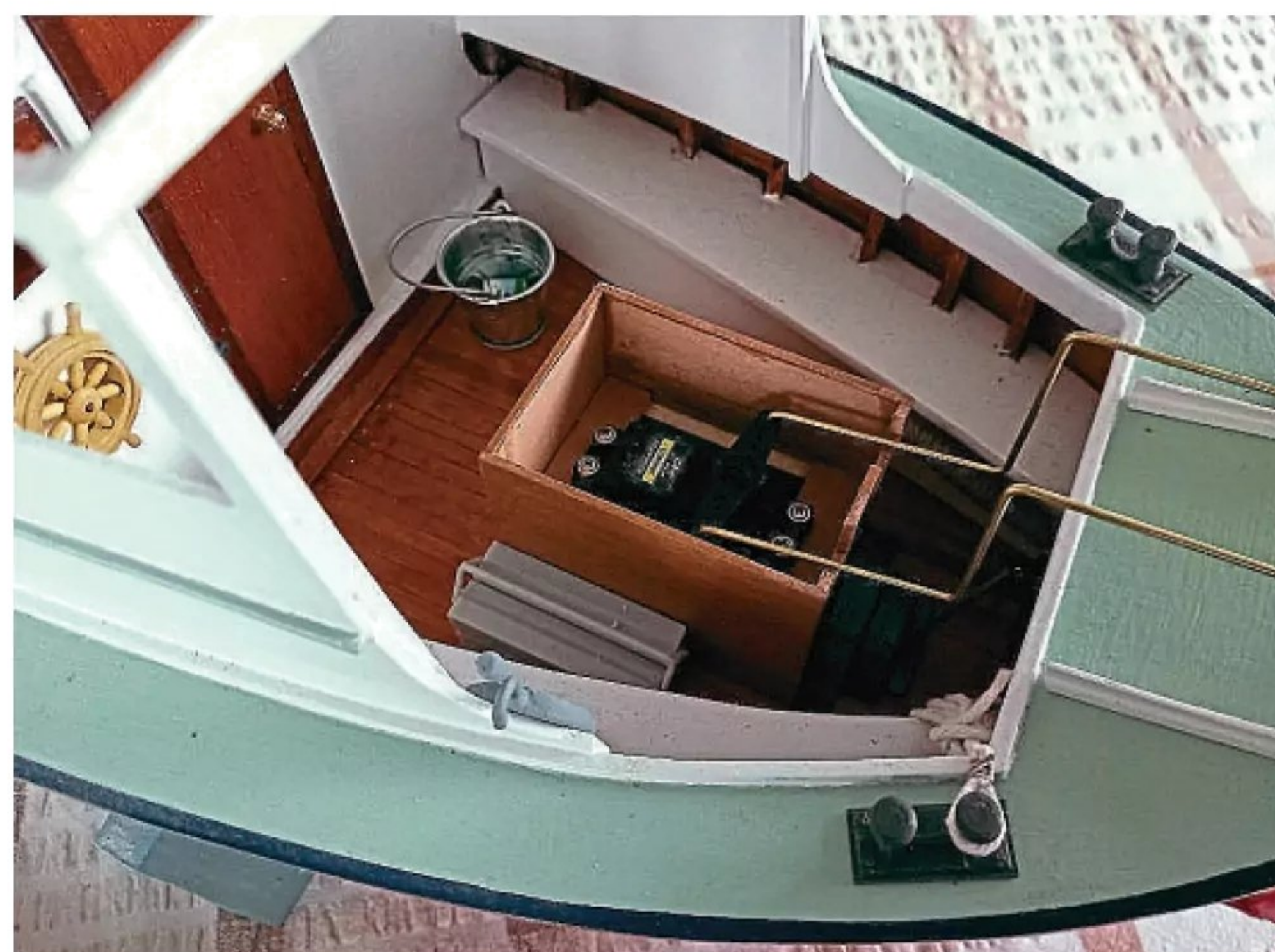
The engine cover removed, showing the servo for the steering and John's method of coupling it up to the rudder.
