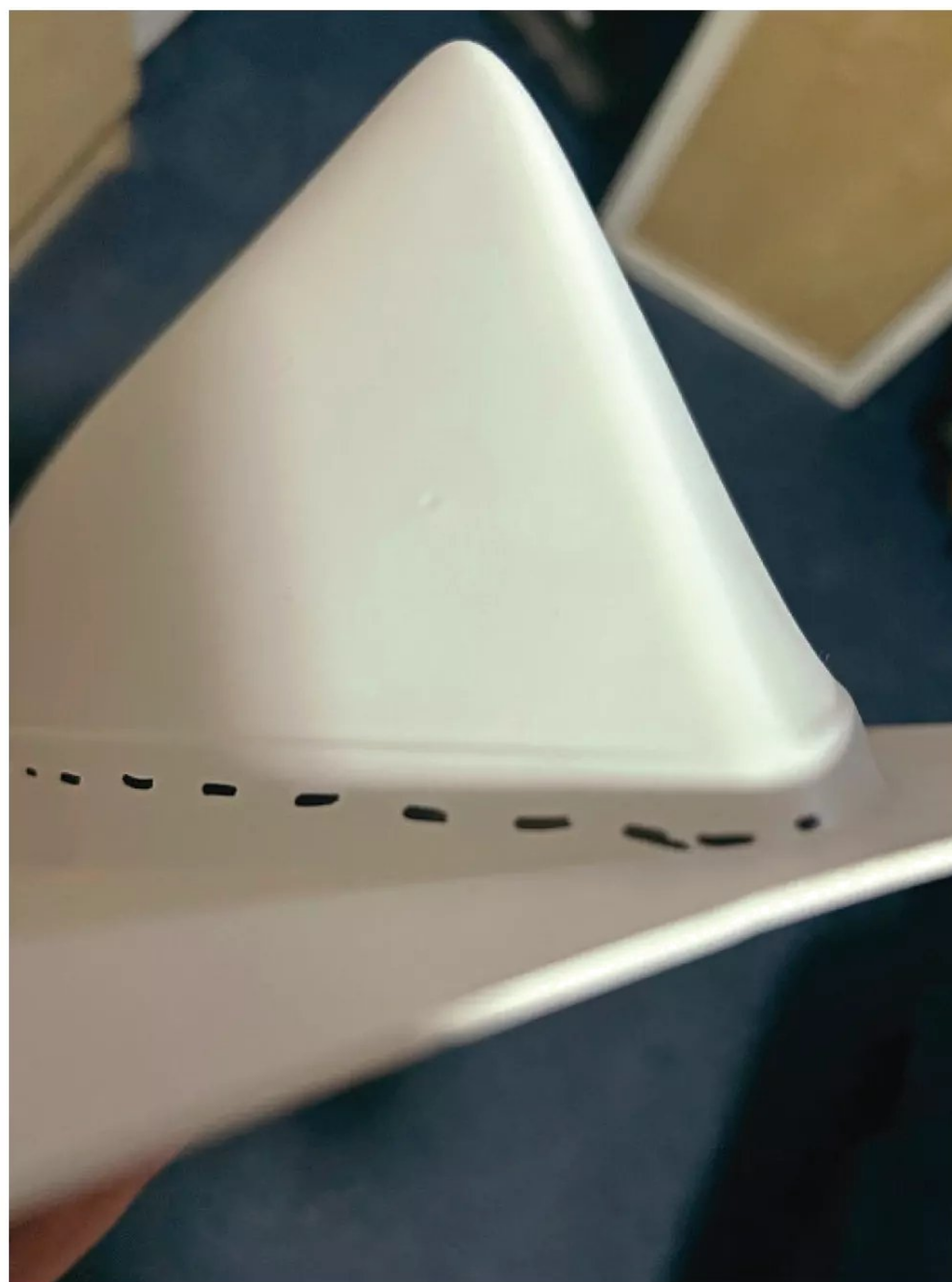
Nick marked the upper line with a Sharpie Pen to identify the correct line to cut to. NB failure to do so will result in the deck sitting proud of the hull.
