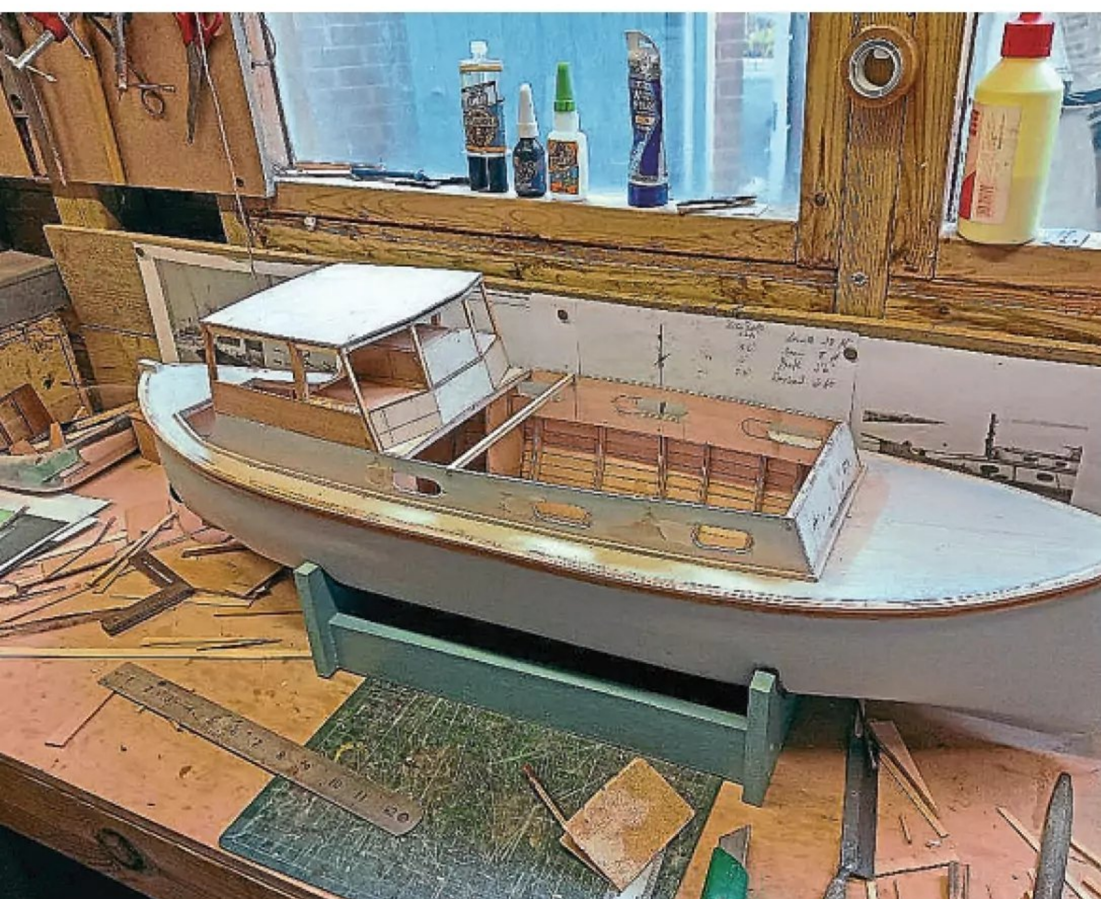
Hobo starting to take shape; John did, however, initially get the position of the window apertures in the cabin wrong, as you can see if you look closely here. Thought also had to be given on how to construct the cabin roof, which needed to be removable to provide access to all the equipment that would make John's model a sailable proposition!
