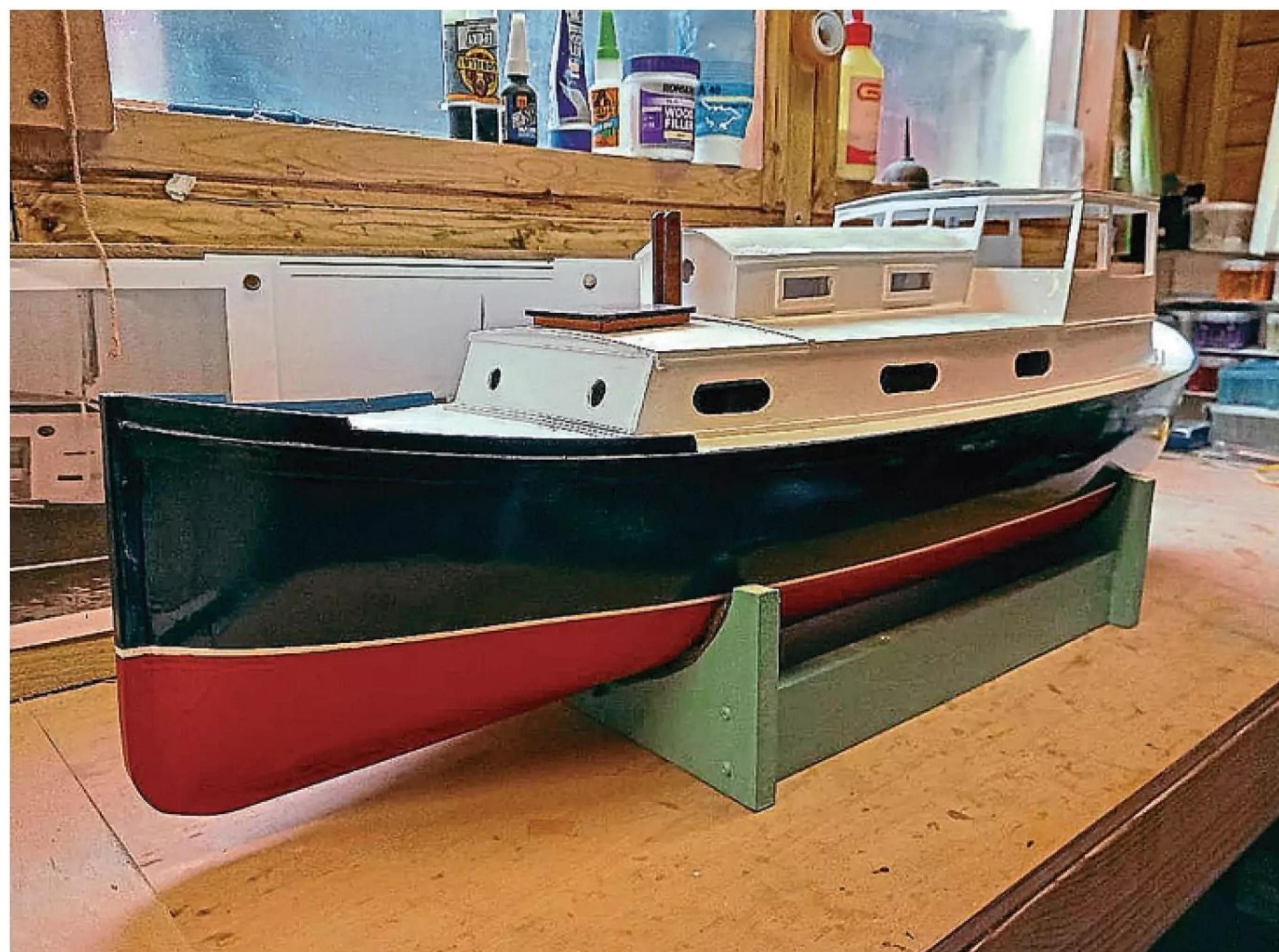
The model was painted using Halfords rattle cans. The waterline (as John recalls, 2ft 6 inches draft on the real vessel) was achieved by using an engineer's scribing block.
