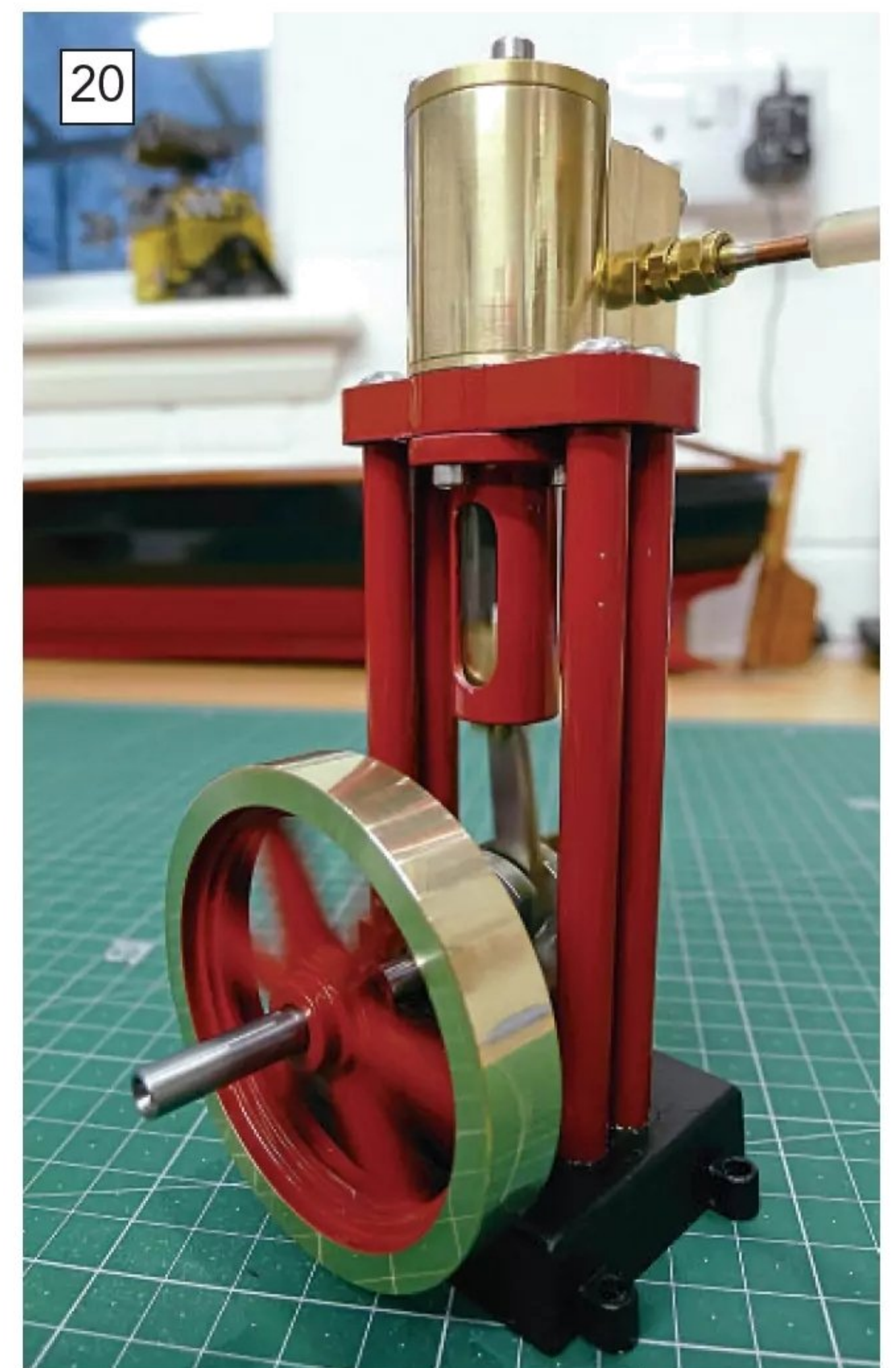
The flywheel was the only remaining part to be added before the engine was given a run on air. A beautifully smooth run on very little air pressure once again confirmed what a superbly designed and machined engine this is.
