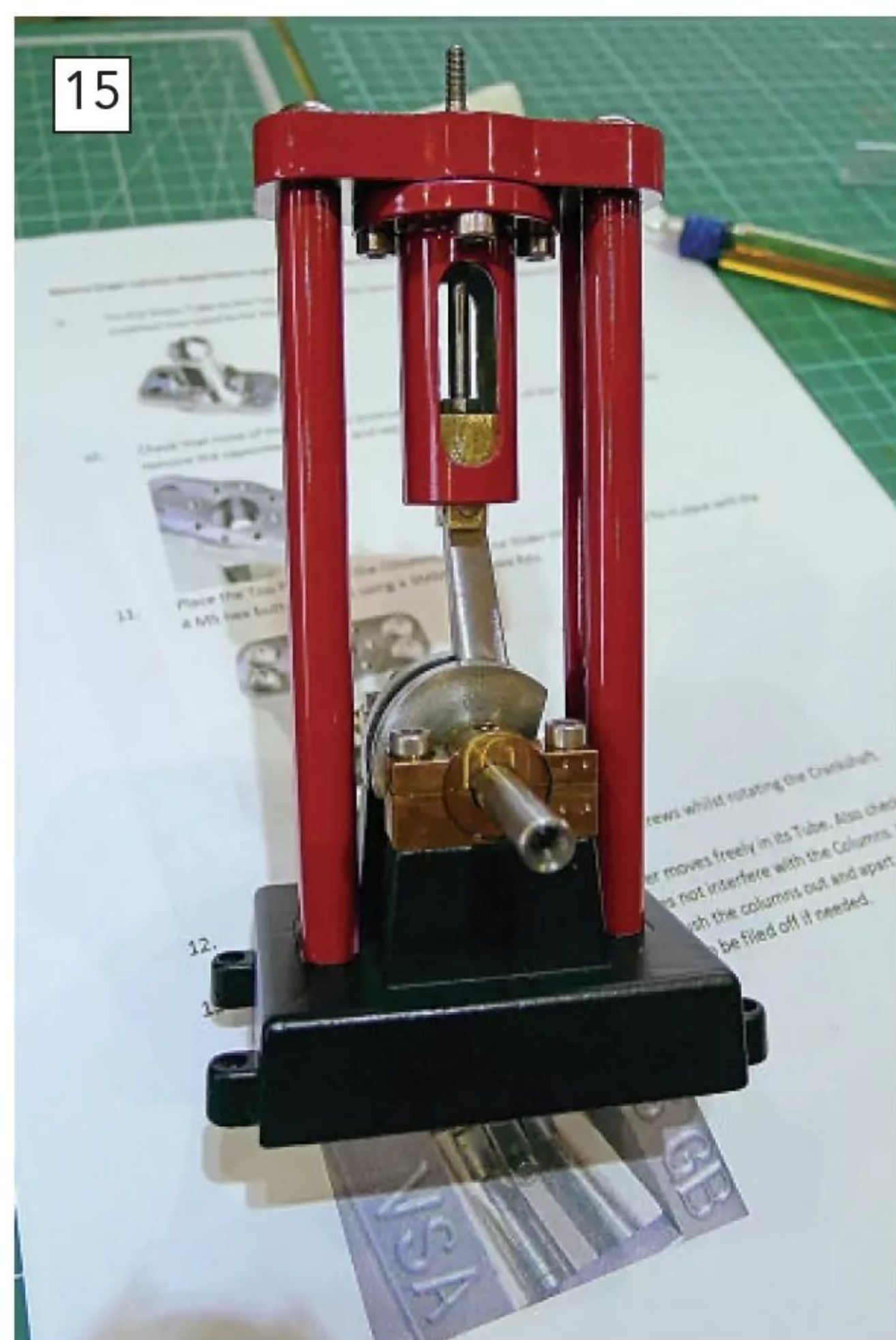
Here the crosshead guide has been screwed to the base of the top plate, then dropped onto the tops of the four columns and the crosshead – again, cautiously, to avoid damaging the paint. The crosshead has been well oiled and the eight screws on the columns all tightened up.
