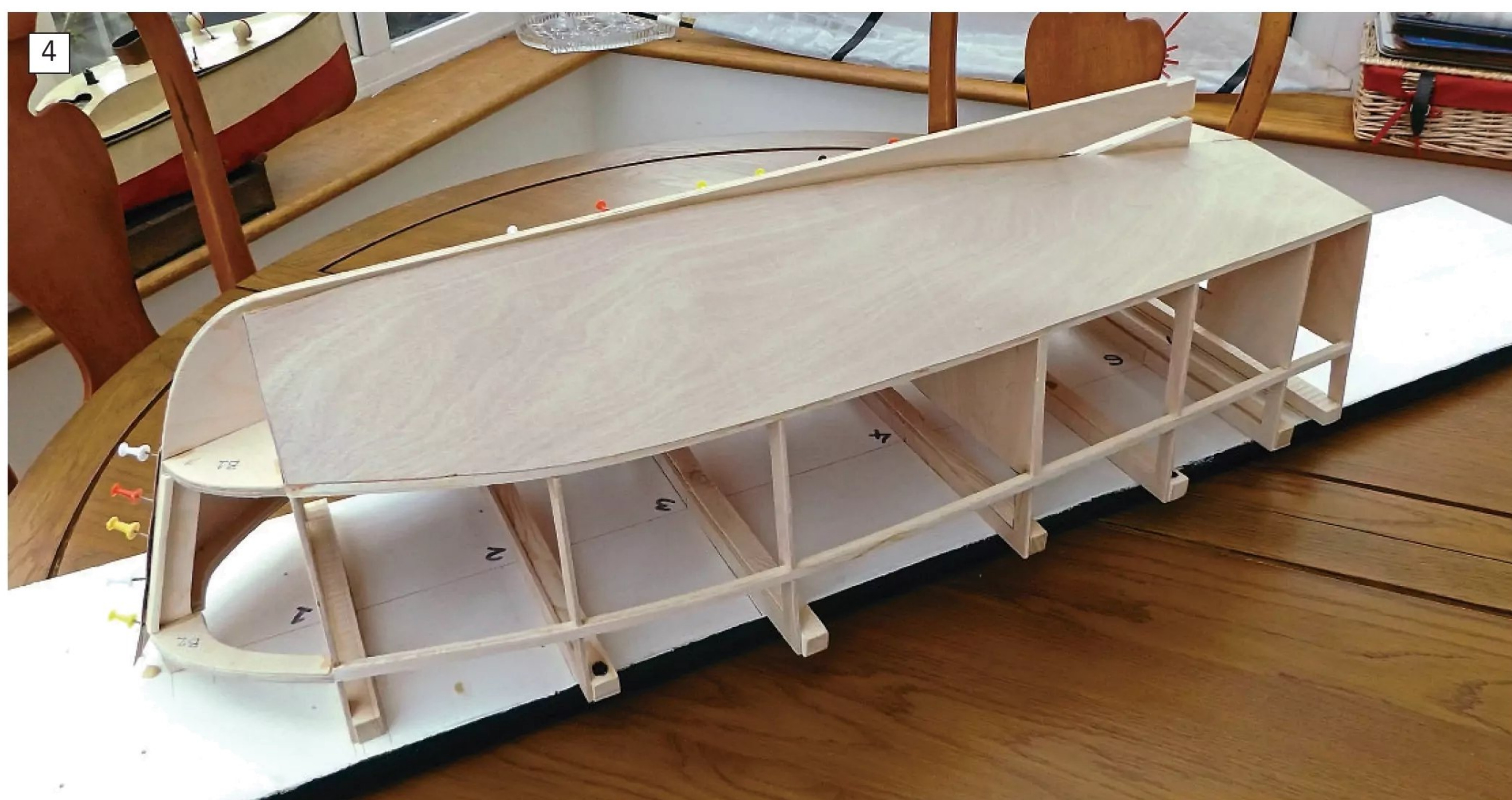
My bottom skins are \frac{1}{32} -inch ply, but you use \frac{1}{16} -inch if you prefer. I recommend cutting card templates for all the shapes before cutting your plywood, as it's quite expensive these days. Pins and clamps need to be used to hold the skin in position until your woodworking glue (I used Gorilla) has set. The pin holes will be filled at a later stage with a lightweight filler.
