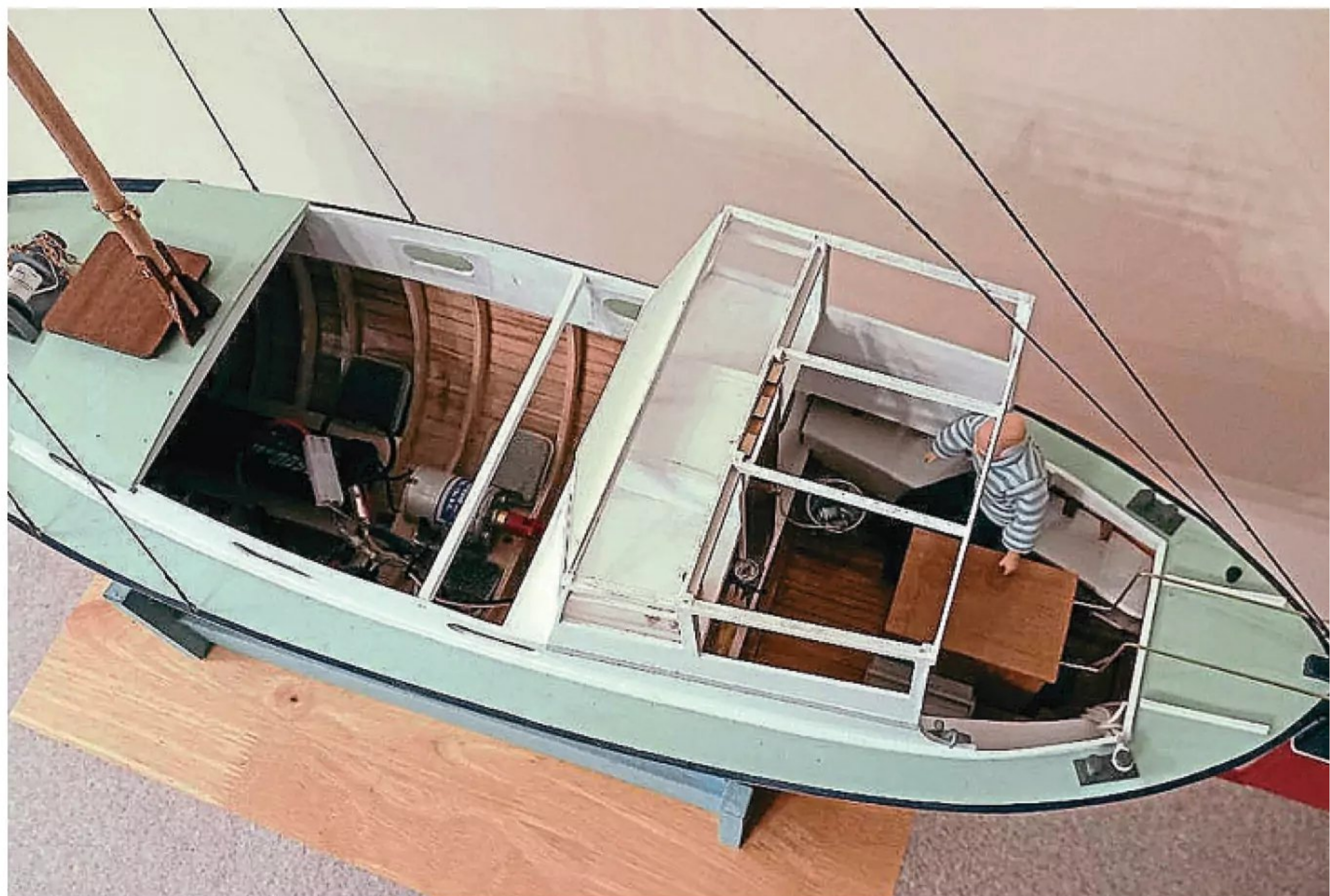
Cabin and wheelhouse exposed. Note the pump (the grey thing on the portside of the wheelhouse), which John and Mike had to rely on more than one occasion. First, however, it had to be primed, which meant adding more water to the boat before they could get any out!
