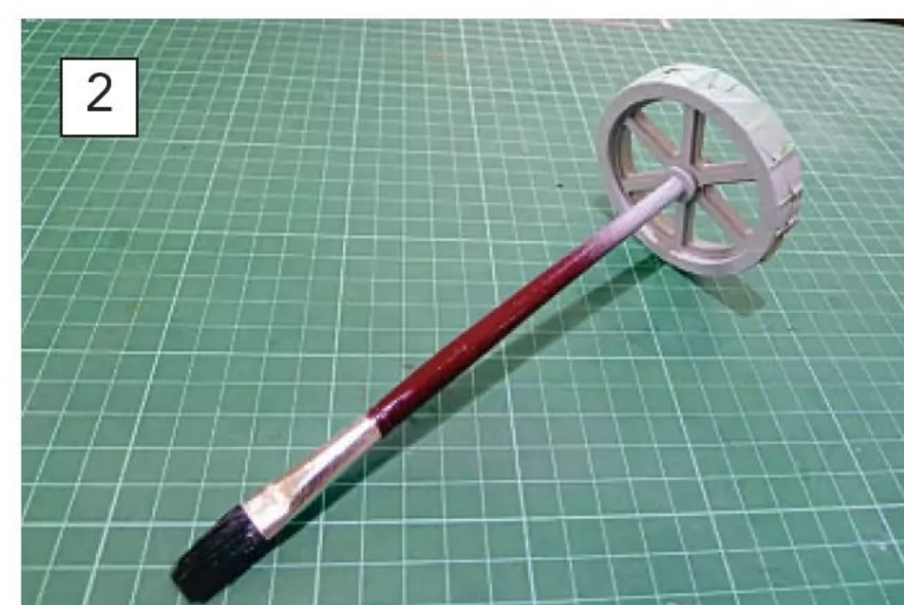
Richard's flywheel rim was polished before masking up with Frog Tape. Attaching it to a tapered spindle made handling and rattle can spraying as easy as it gets.
