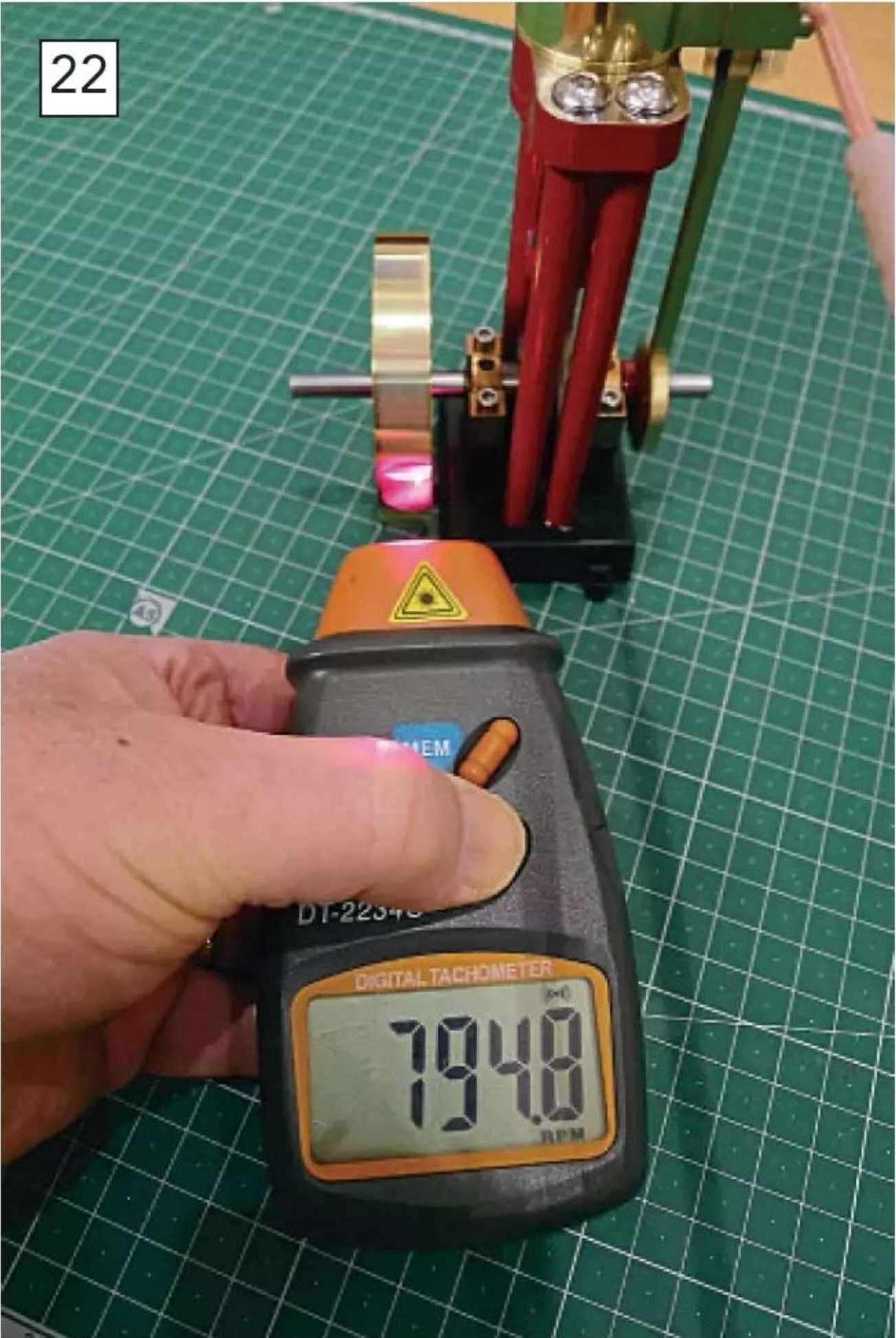
Interestingly, on only 5psi of compressed air, the Chiltern engine managed a healthy 795 rpm; and while under load the rpm would be significantly less, the boiler is capable of providing a lot more than 5 psi.
