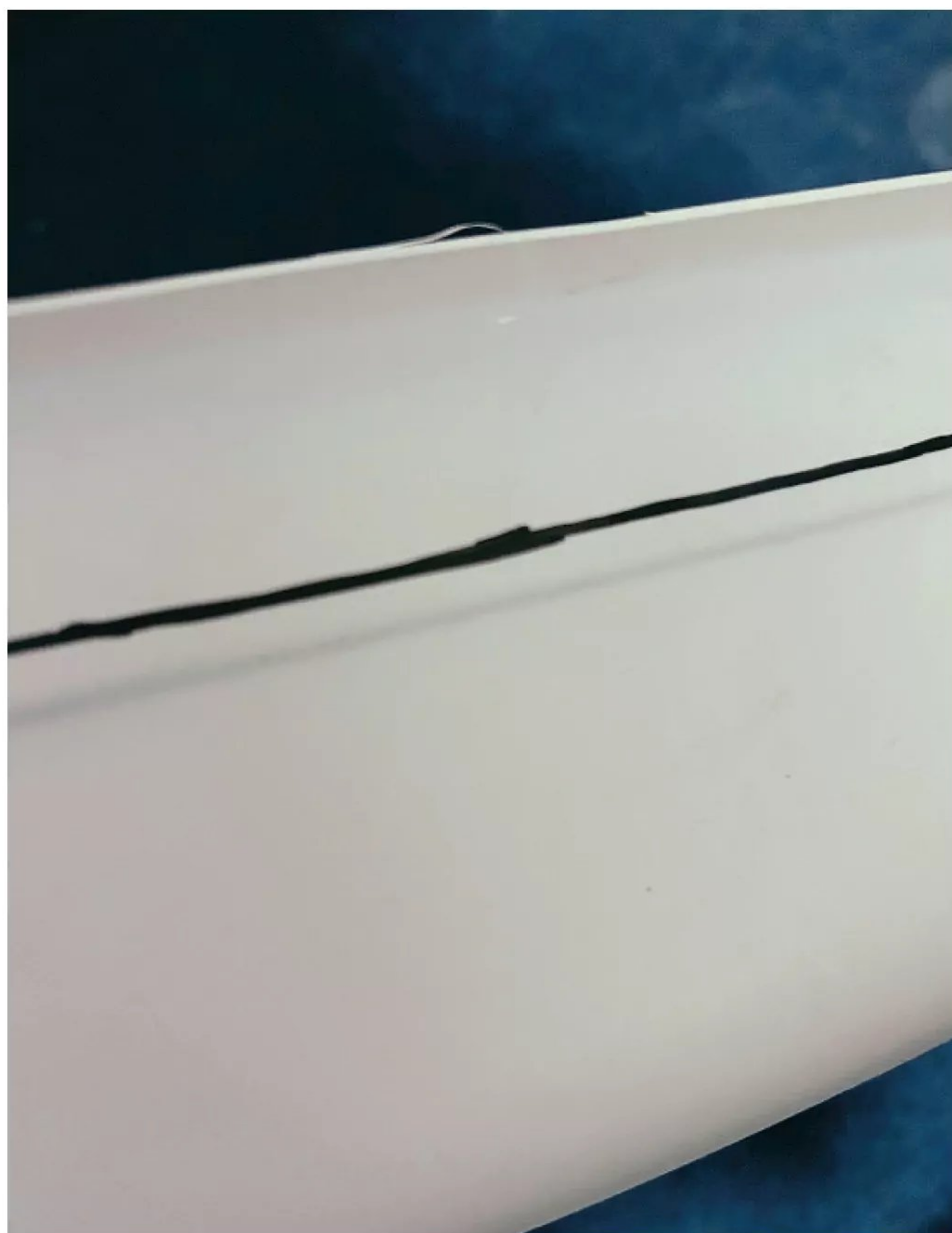
Nick marked the upper line with a Sharpie Pen to identify the correct line to cut to. NB failure to do so will result in the deck sitting proud of the hull.
