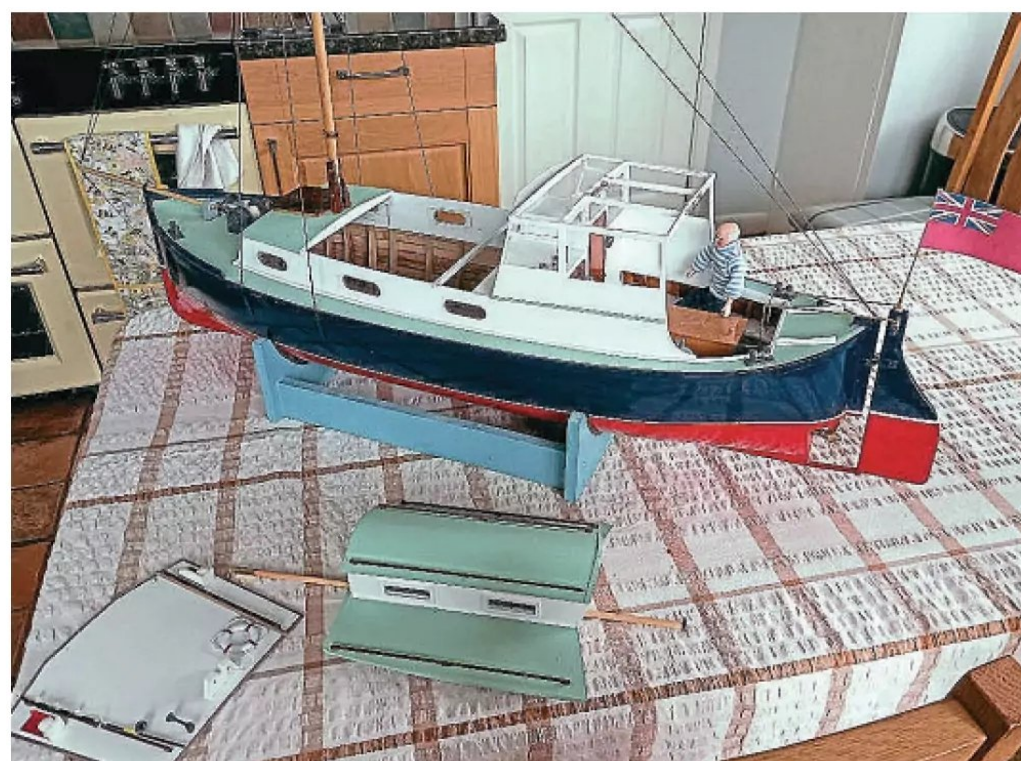
A view showing the cabin and wheelhouse exposed. The cabin roof is shown removed to give a better idea of its complicated structure.
