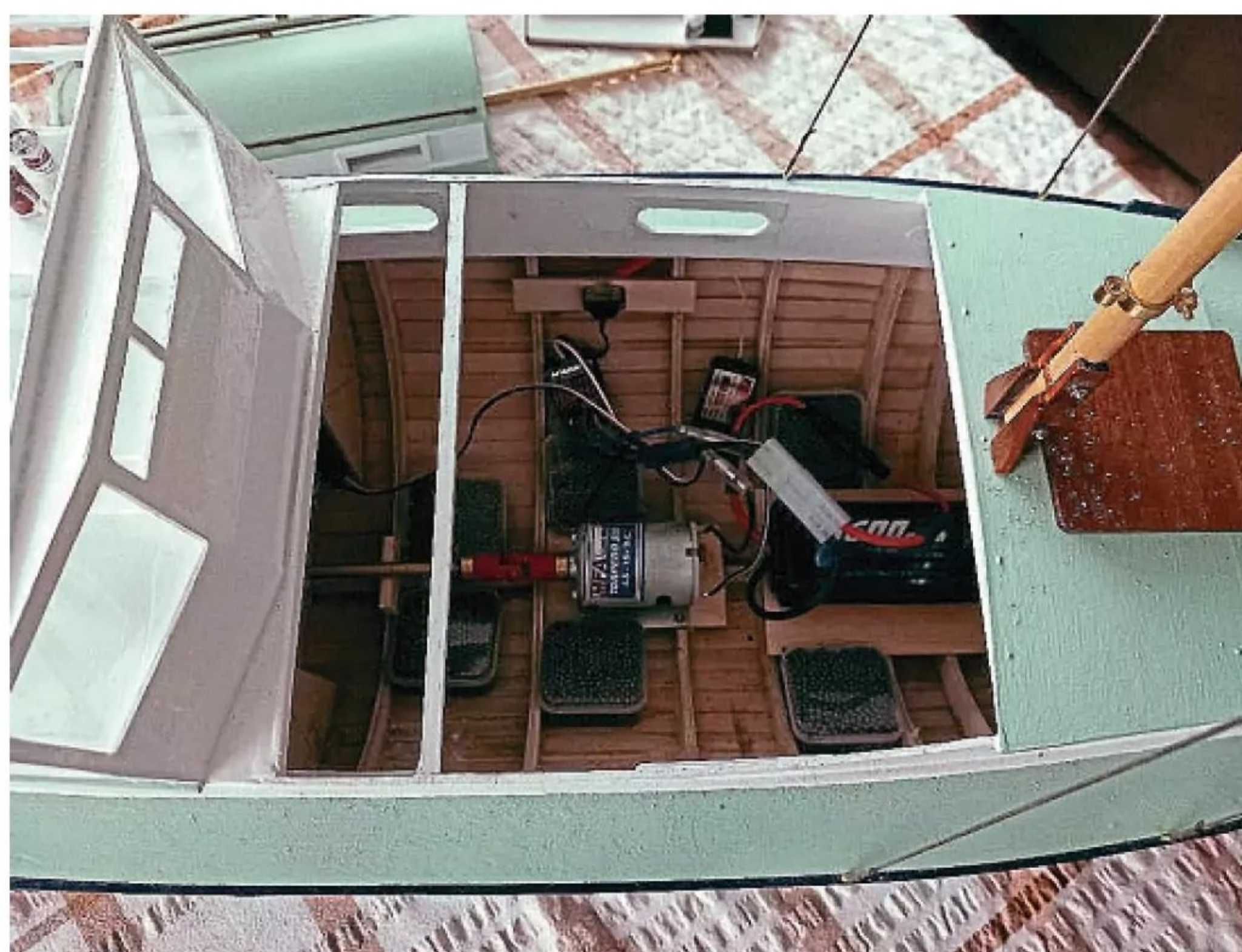
The front inner workings exposed, showing some of the ballast.
