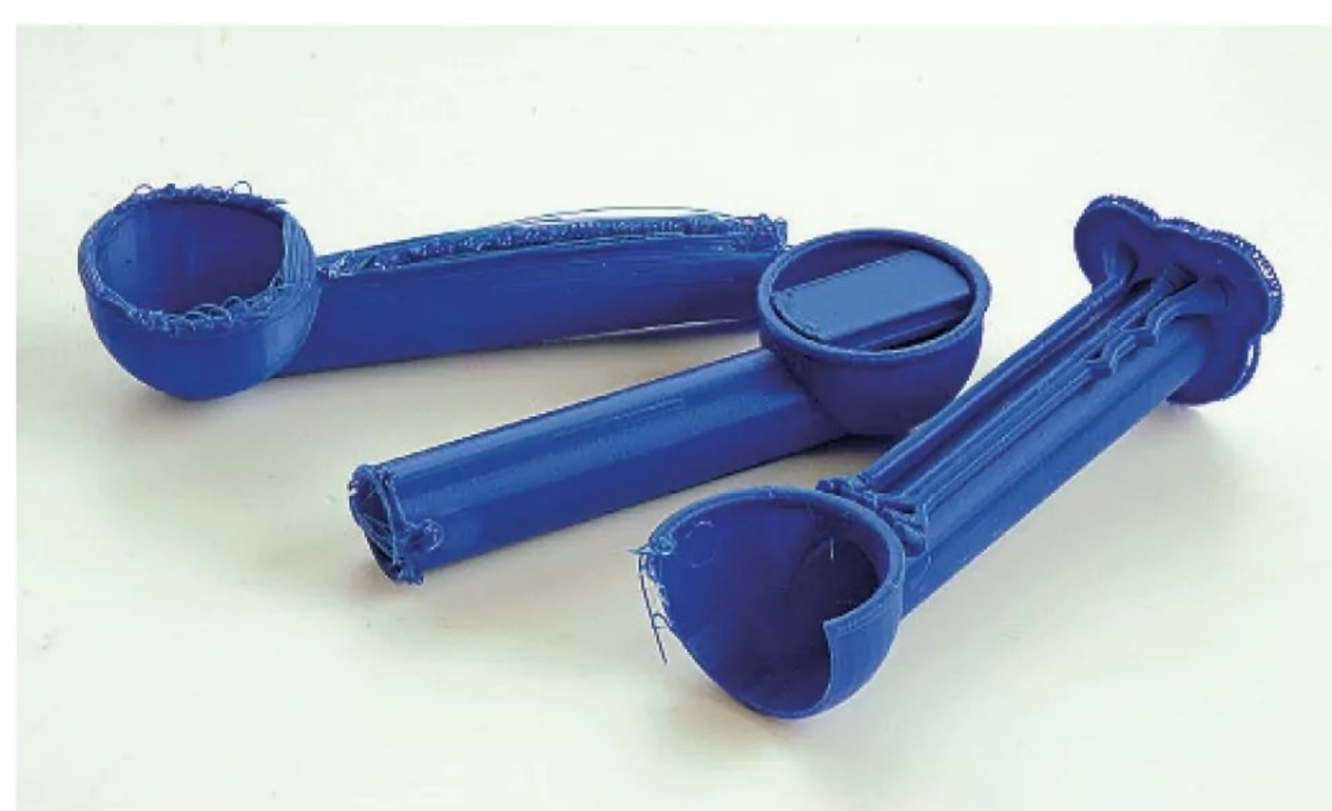
Three failed attempts at printing the cowl ventilator.
