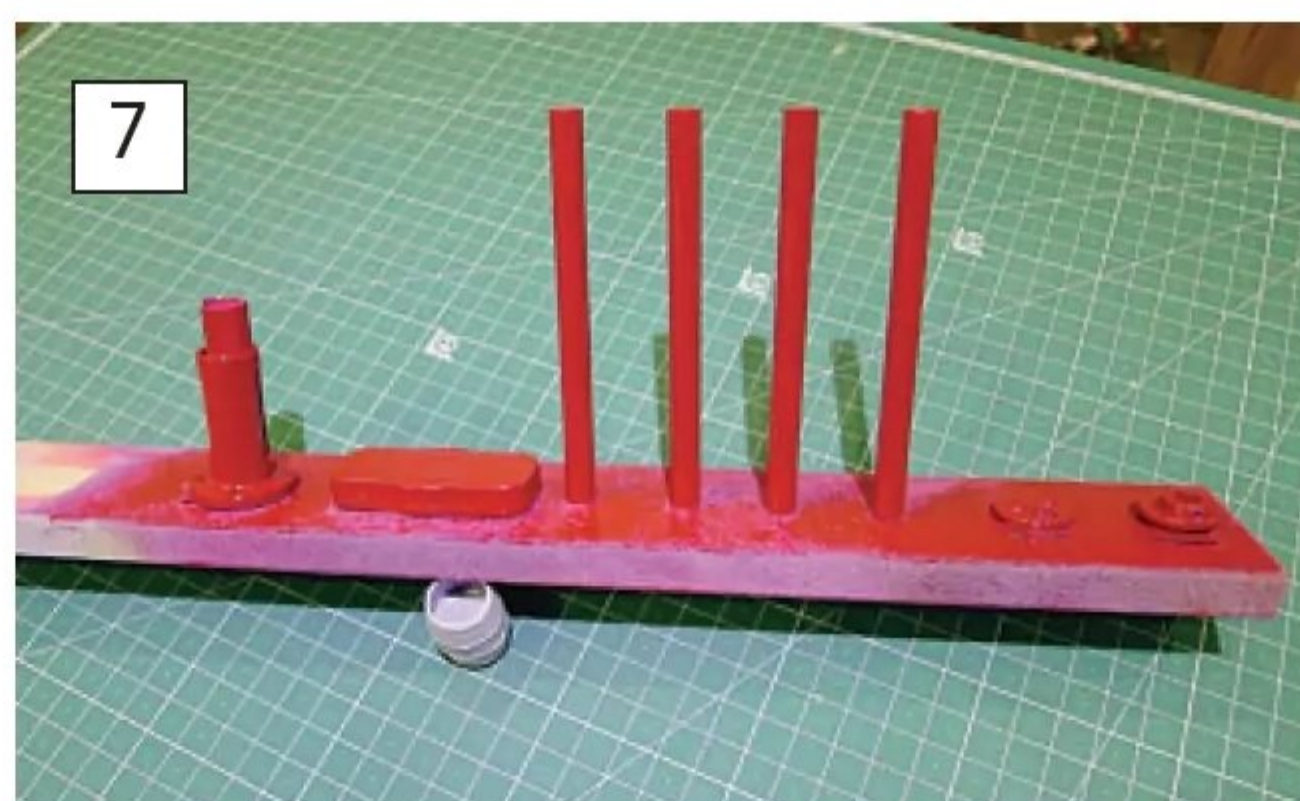
With its base removed, Richard's painting board, was given a light dusting spray followed with a heavier second coat of the gloss red, but not before the top plate had been masked with Frog tape and the crosshead guide masked internally with a roll of paper.
