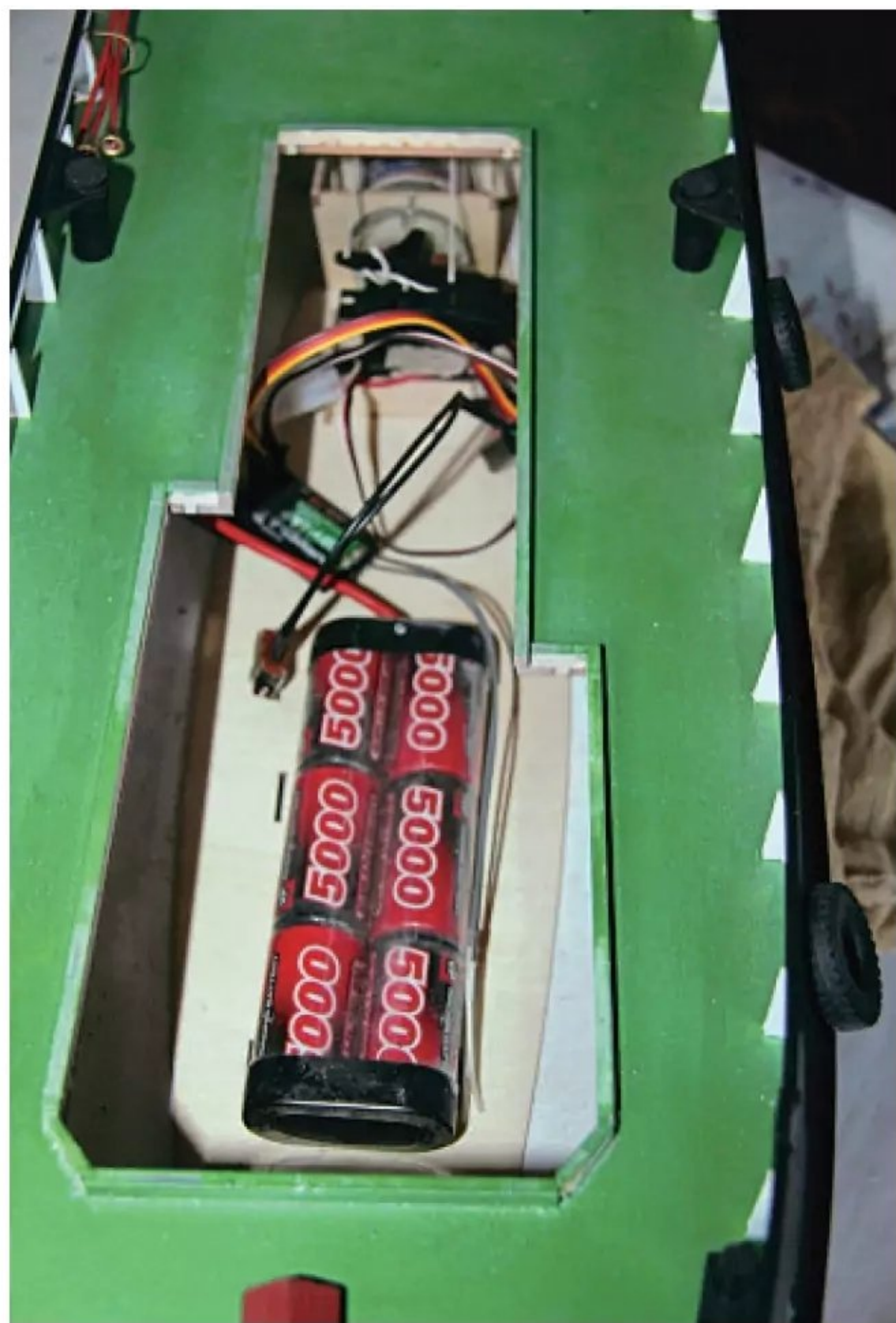
The internals fitted with an MFA Torpedo 500 motor, 20amp ESC, and Nick's 7.2v NiCad battery pack, a combination that proved to be more than adequate to propel the model.
