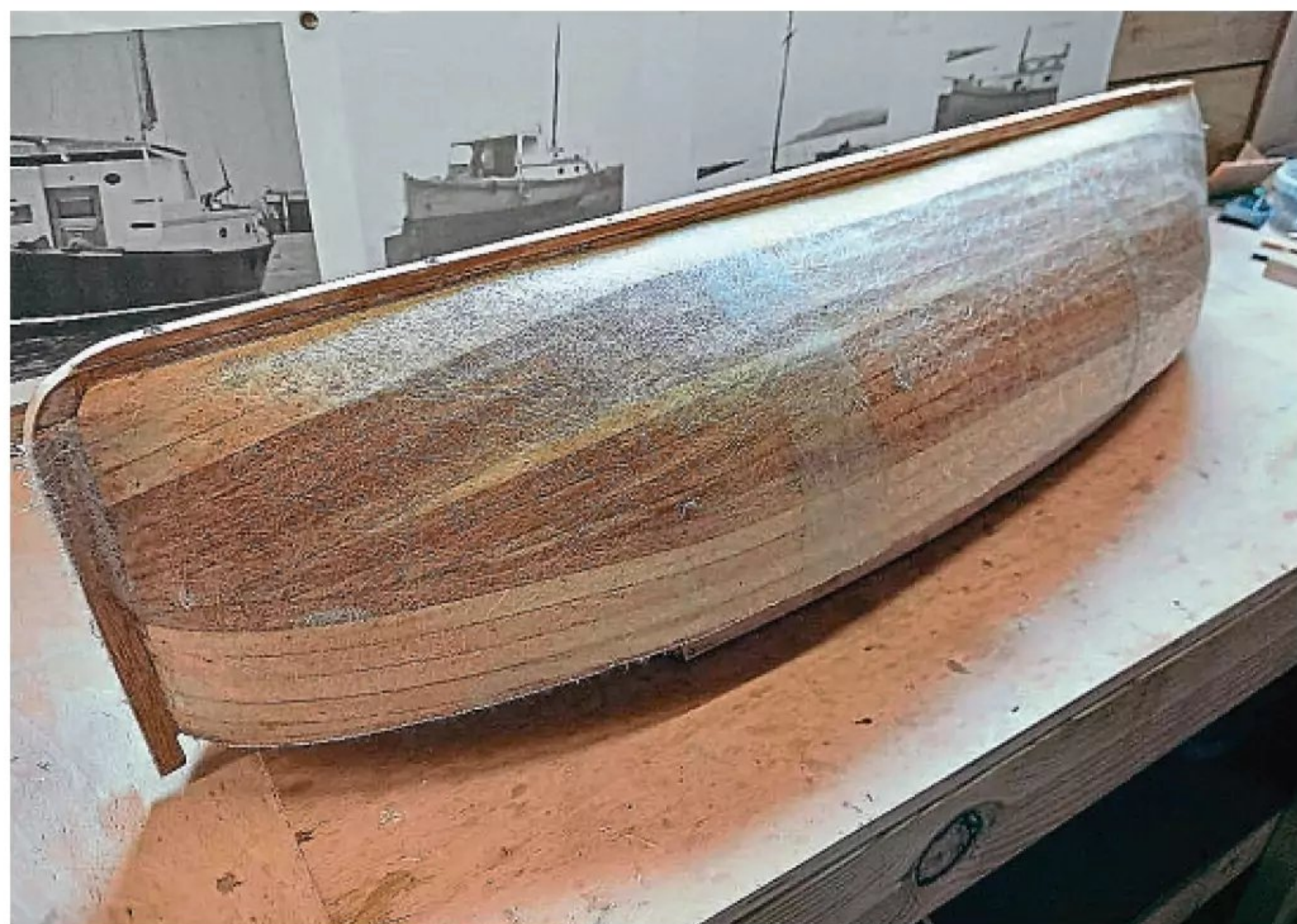
After spending many hours on the planking (including bending it shape and closing all the gaps), John then applied fibreglass matting and resin. He'd never attempted this before, but he got there!
