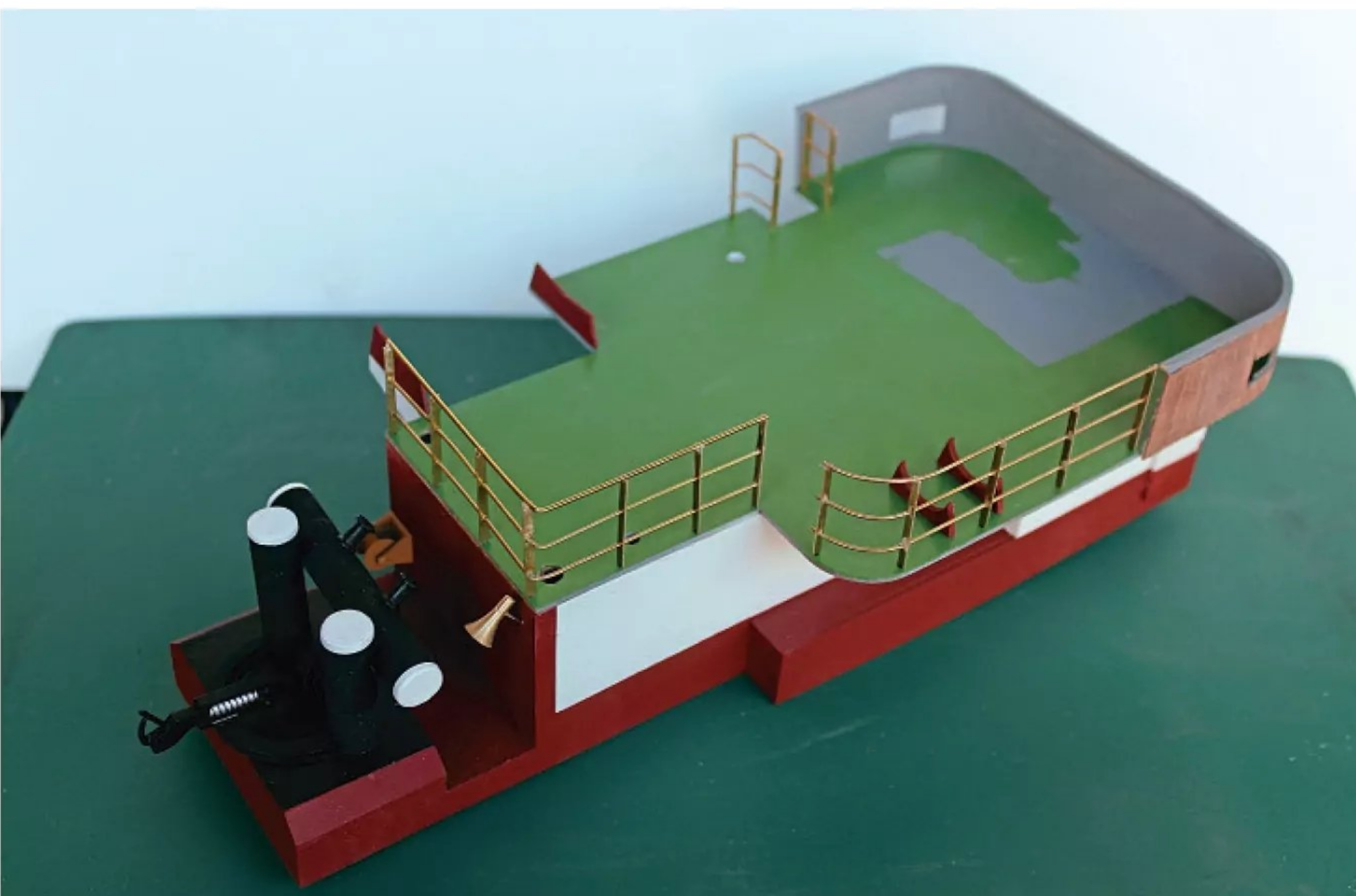
The brass stanchions are limited to the upper deck and are easily fitted thanks to the assistance of pre-cut holes in the deck. It's almost a shame to paint them!
