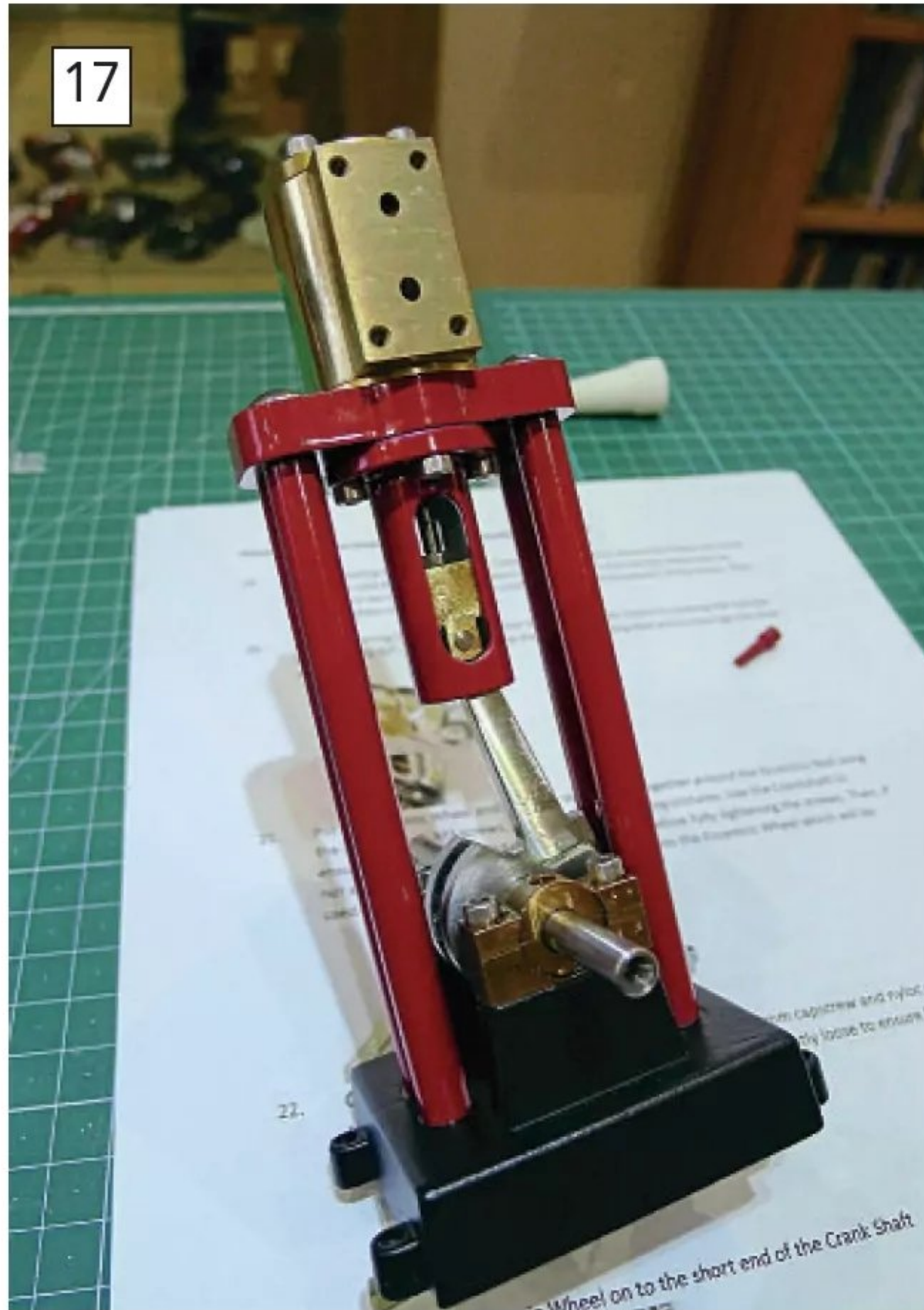
The cylinder base, piston, cylinder and cylinder cover all dropped in place, with some oil on the piston and the main four-cylinder screws fitted. Everything continues to rotate smoothly and easily.
