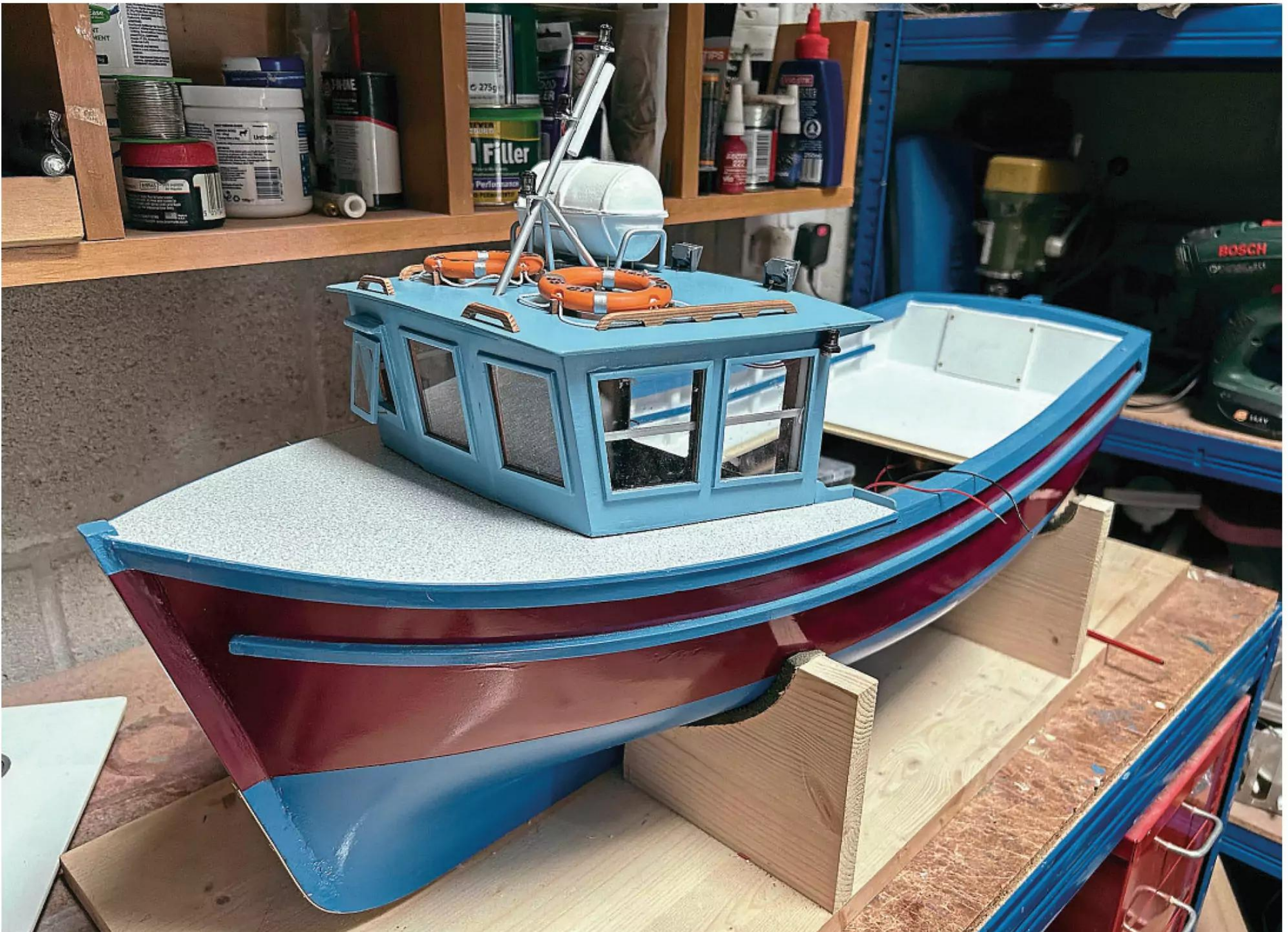
The finished wheelhouse with mast and life raft canister in place.
