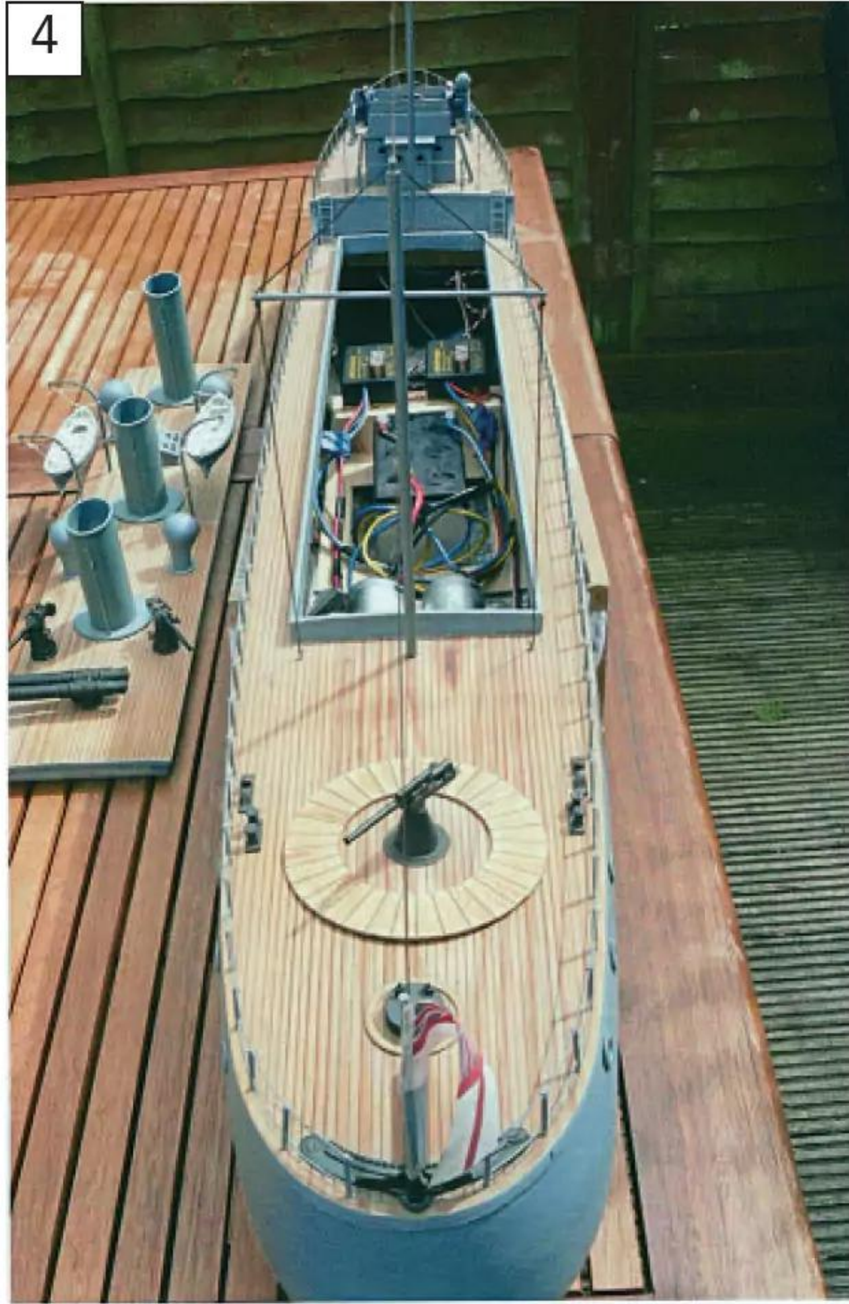
Unable to source a suitable vintage steam plant, Brian decided to instead fit electric motors and radio control gear in order to get his restored Torpedo Boat Destroyer on the water in time for its 100th anniversary in March 2016.
