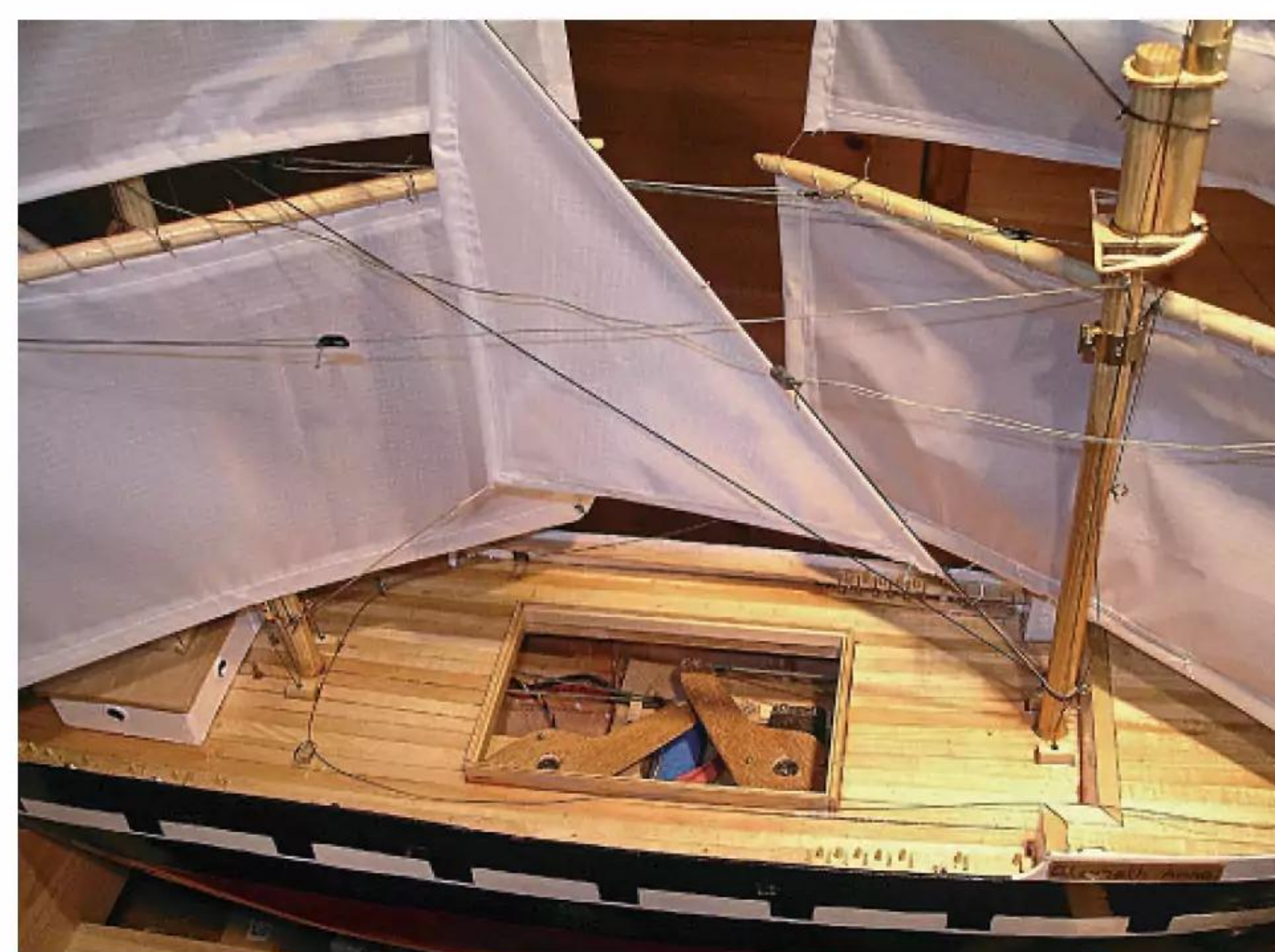
An actual brig, showing sail arms and the corresponding yard positions. Note that the sail arms are at different heights to prevent interference.
