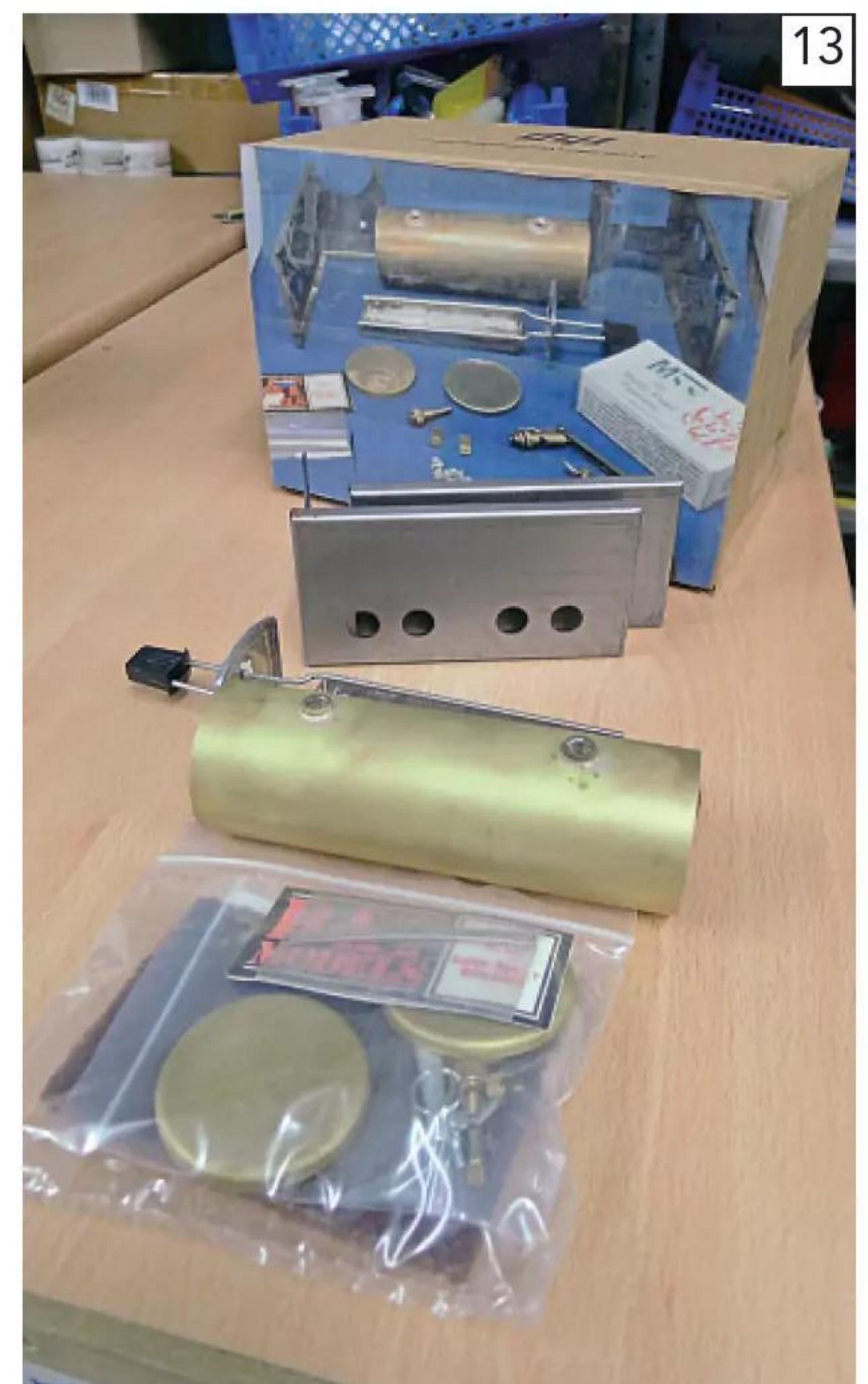
If you feel a little more adventurous, then have a go at making your own boiler from the Tony Green kit. Bushes are ready fitted, so the only remaining job is to silver solder the end plates on and assemble. It certainly adds to the sense of satisfaction in the finished build.
