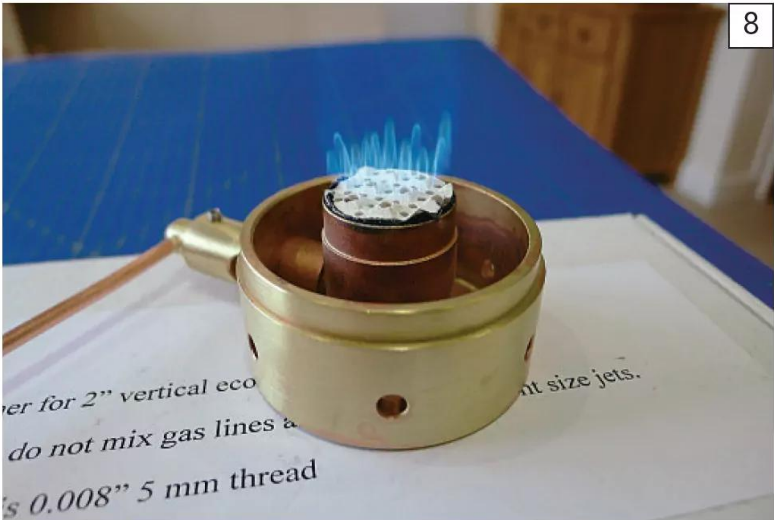
An evenly distributed efficient flame gives the most heat into the boiler, thereby maximizing endurance and minimising gas wastage.
