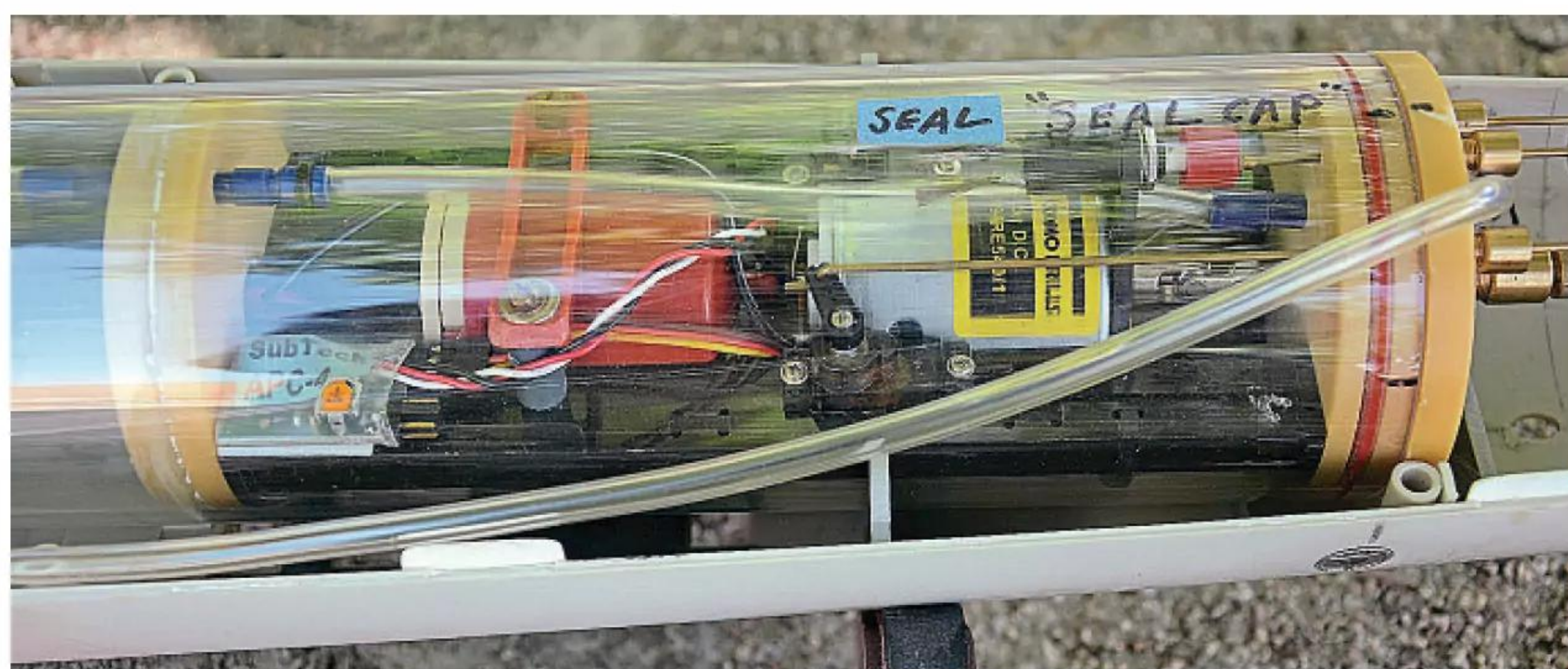
Rear of WTC, with drive motor, ballast pump, control servos and APC.
