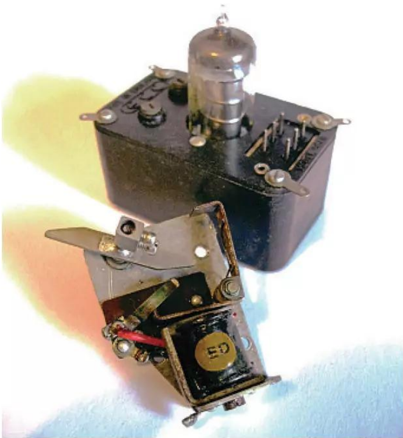
A suitable radio, circa 1960, could have been this valve receiver from ECC Ltd, shown here with a ED escapement.
