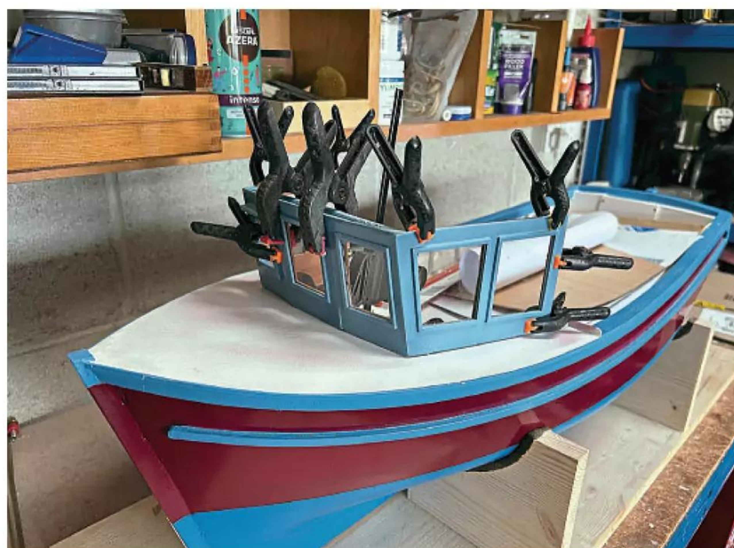
Glueing in the internal mahogany paneling before glazing.
