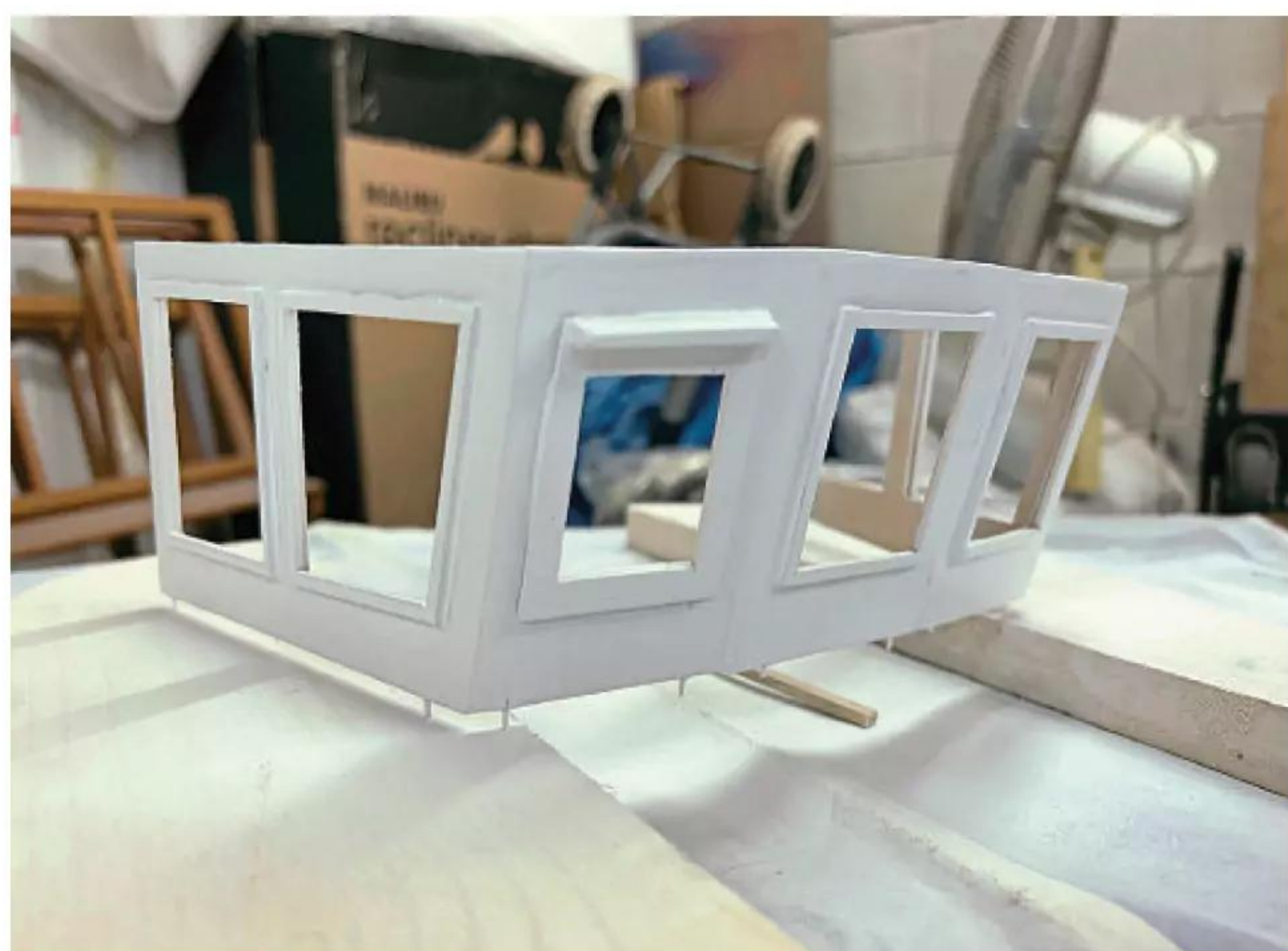
Angled front and side wheelhouse sections before attachment.
