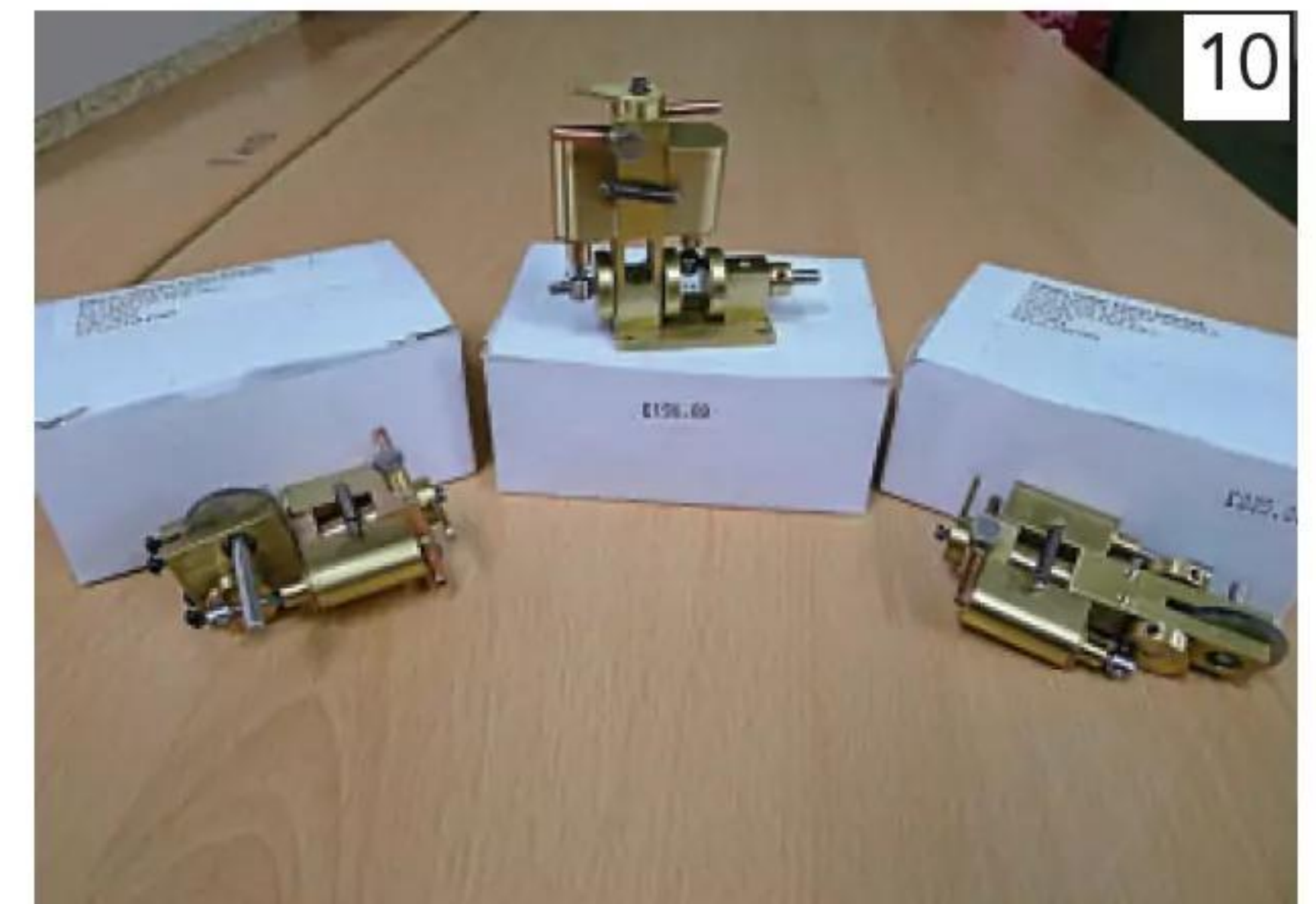
There is also a range of small twin cylinder, double acting oscillating engines in configurations to suit both model railway and marine applications. These engines are based on the old Stour Valley Steam, SVS, range of engines.
