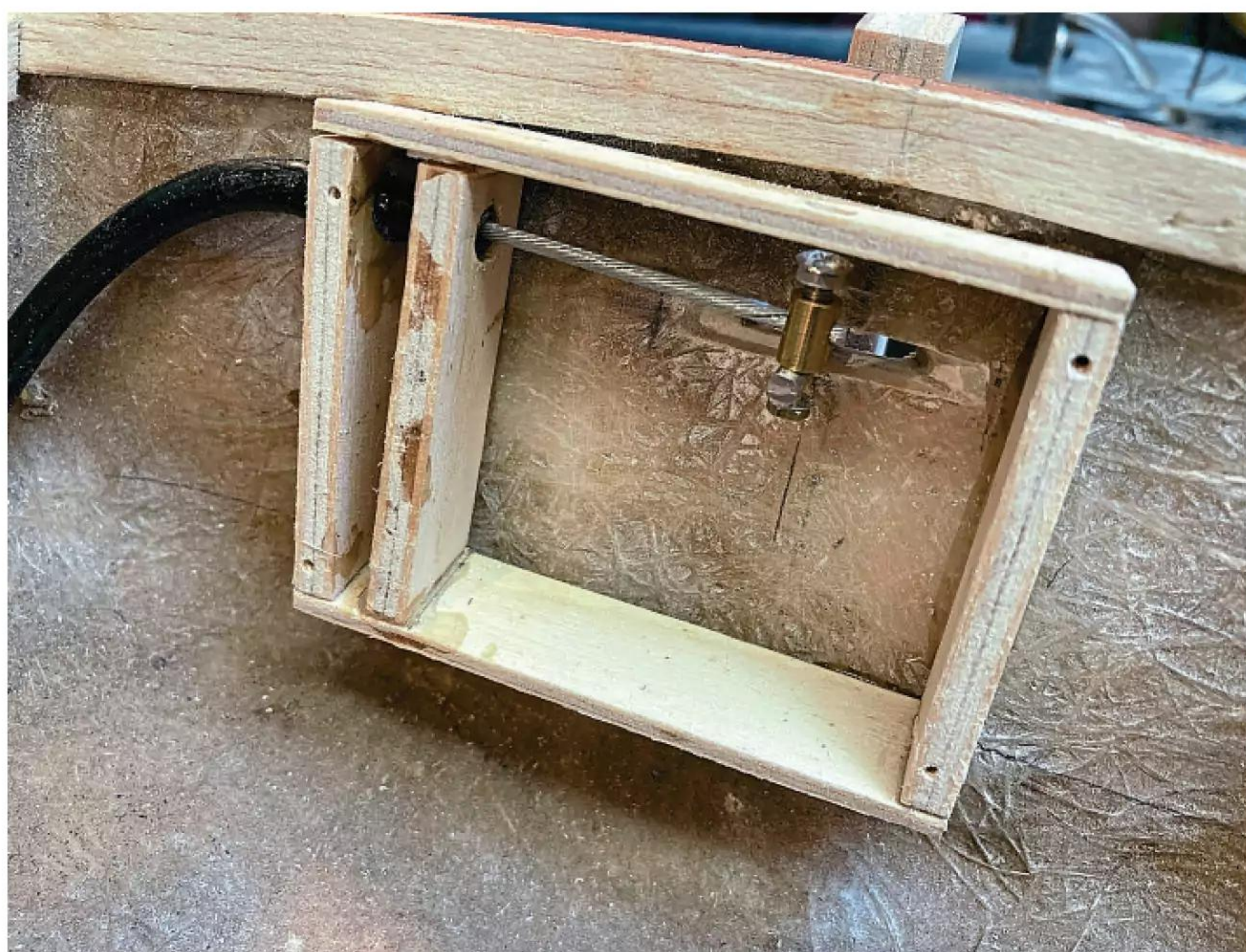
Inner cable attached to the tiller arm in enclosed cabinet.
