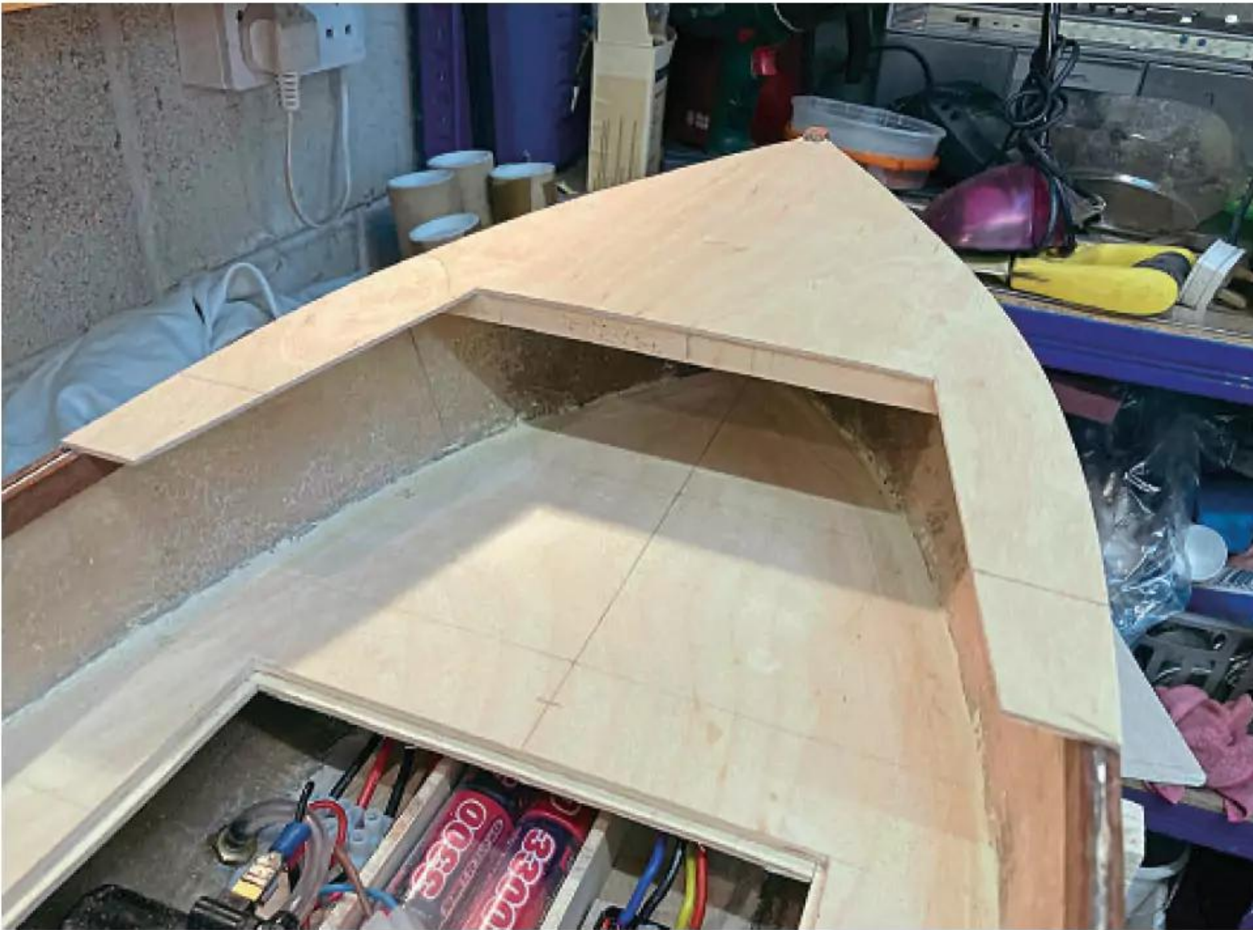
The forecastle deck in place.
