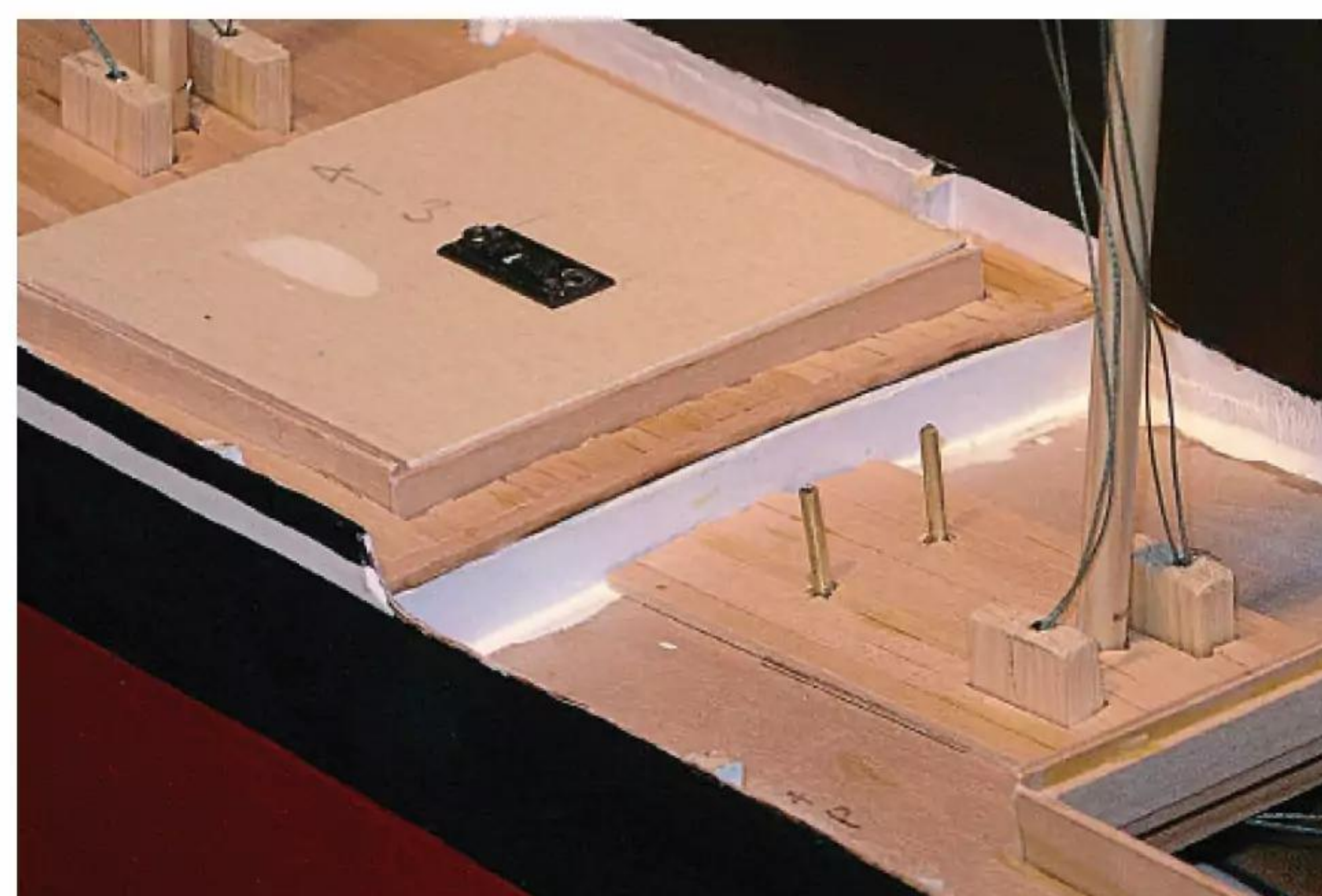
To save having to 'go below', here we see an on/off switch and the charging points above deck. Note the tops of the fairleads up, above deck level, out of reach (mostly) of water across the deck.
