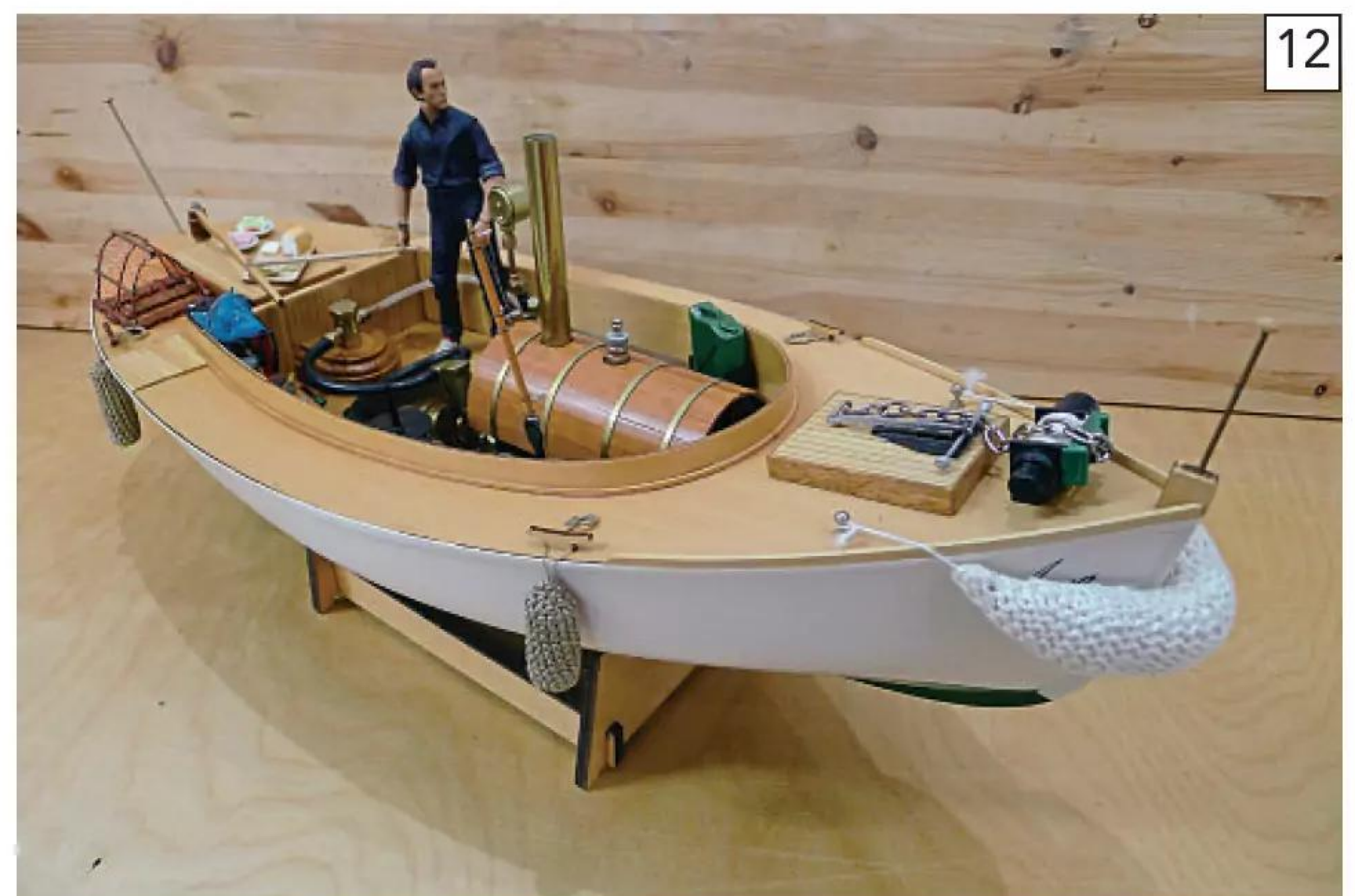
The boiler top cover simply lifts off and can be left with either a polished metal finish or, as here, can be clad to resemble an insulated boiler.
