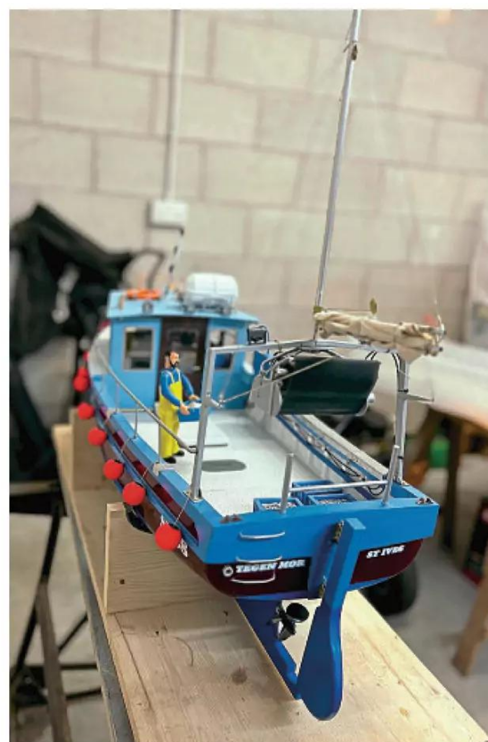
The aft gantry with mizzen mast, sail and net hauler in place.
