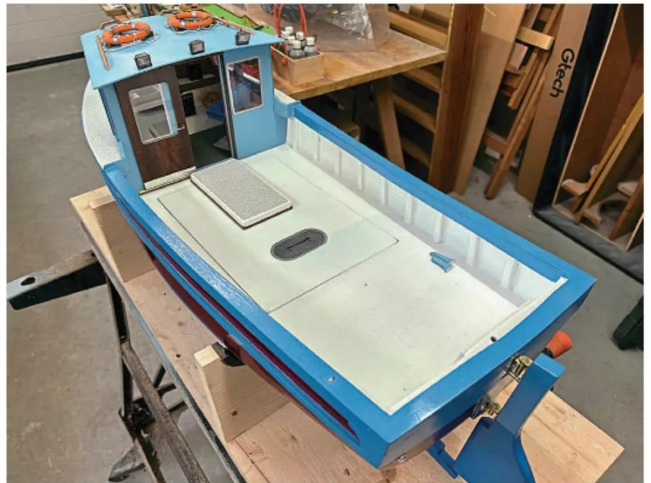
Timber frame uprights between deck and gunwales.
