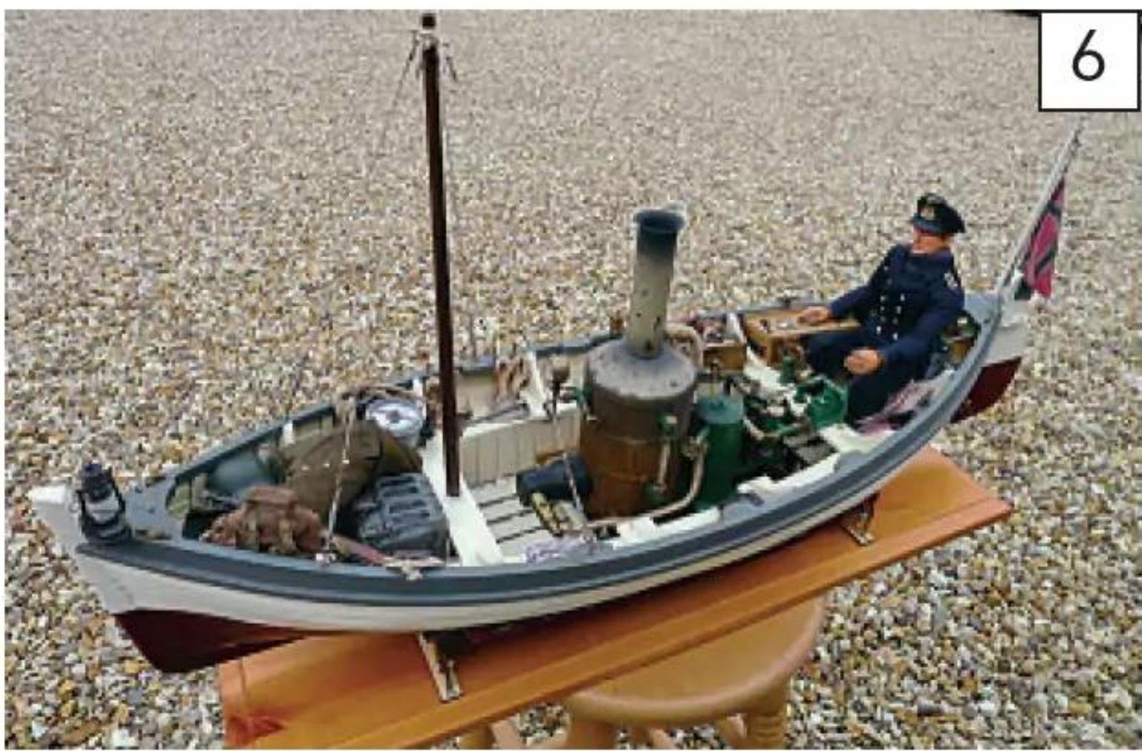
Keeping the plant on its common base makes for a very convenient to operate plant that can be removed and refitted into the model in a matter of minutes.
