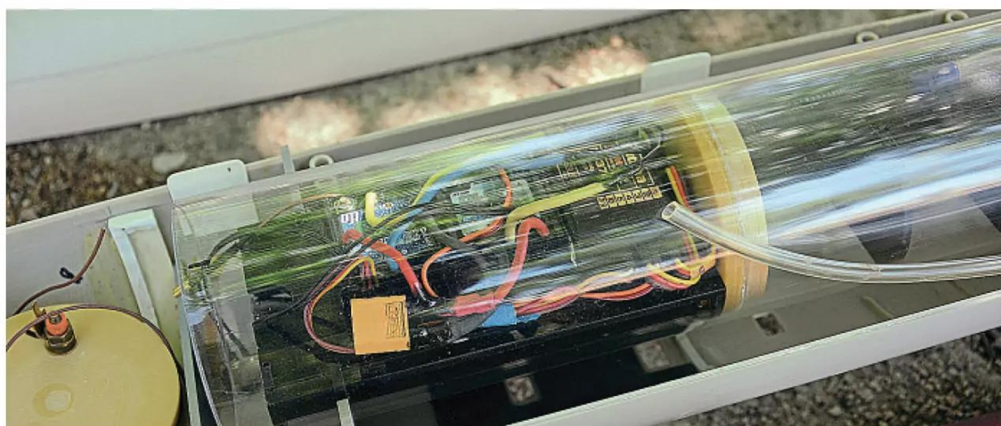
Forward end of WTC with receiver, ESCs for motor and pump and drive battery (under).
