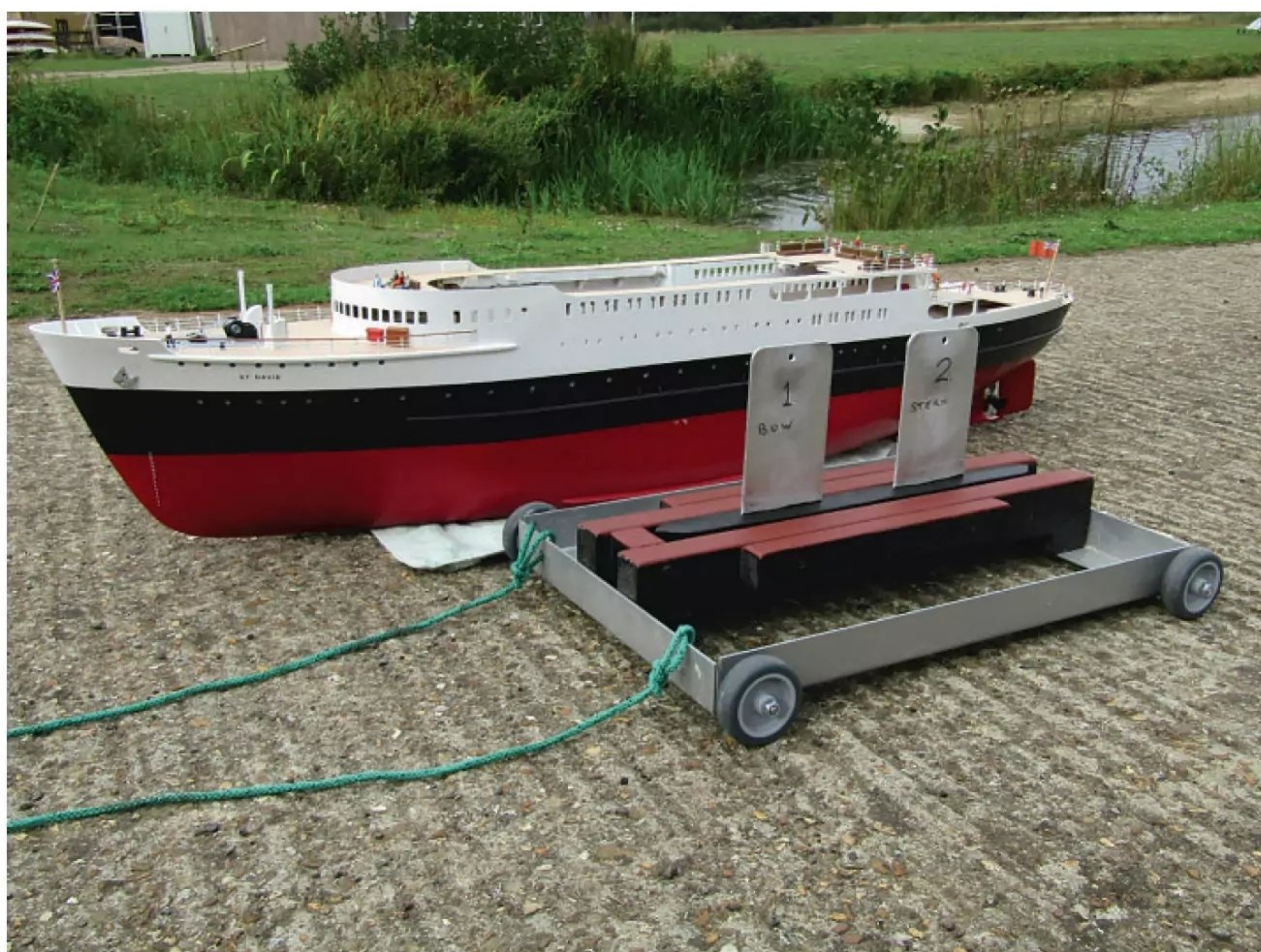
Barry's ingenious DIY trolley, designed to make launching and retrieving the weighty ferry struggle free.
