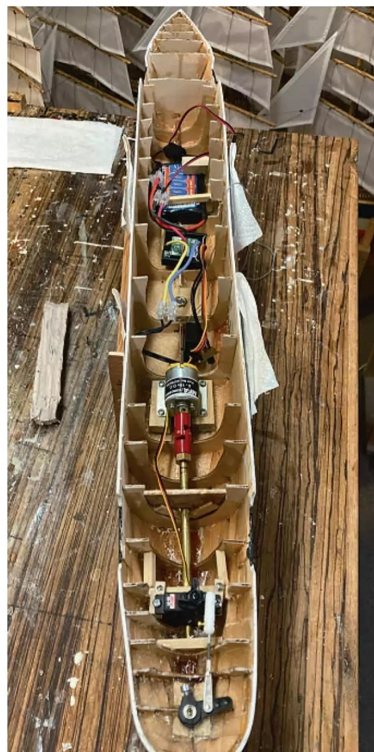
All the electrics in. The pale oblong to the left of the hull is the external keel.
