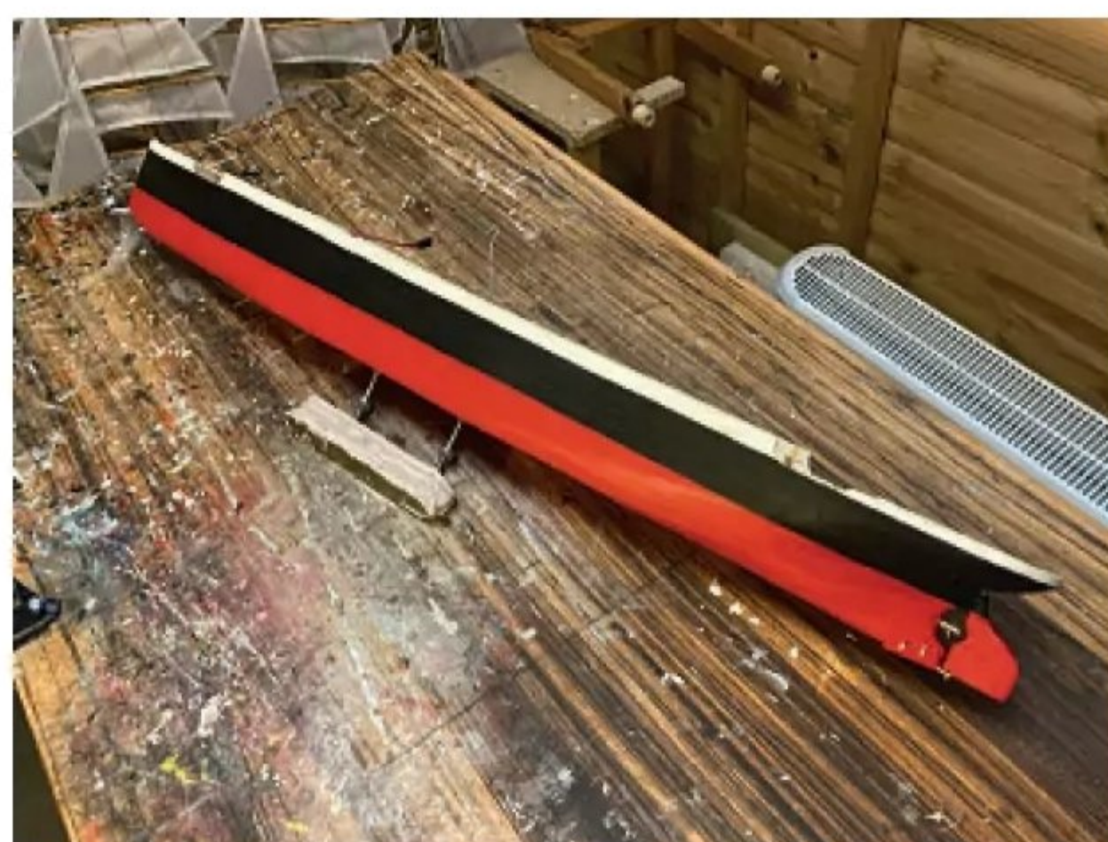
Preparing the keel for fitting to its bolts. The oversized rudder is apparent.
