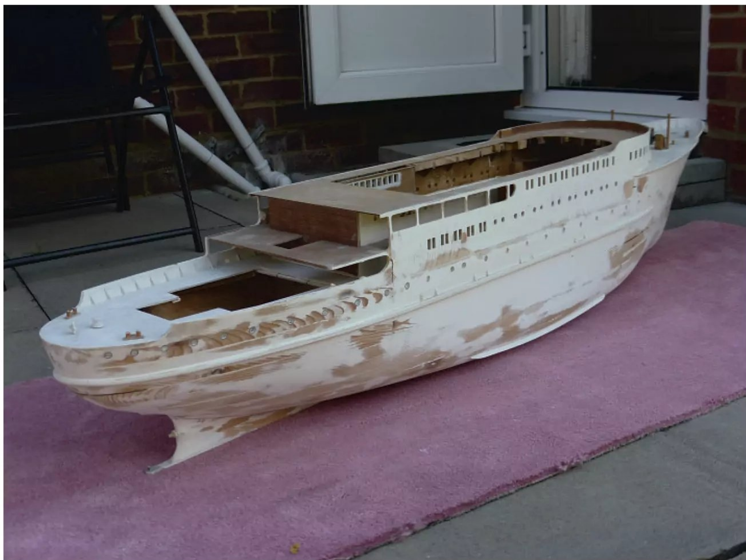
Giving the ferry a good sand, in order to assess the condition of the hull.
