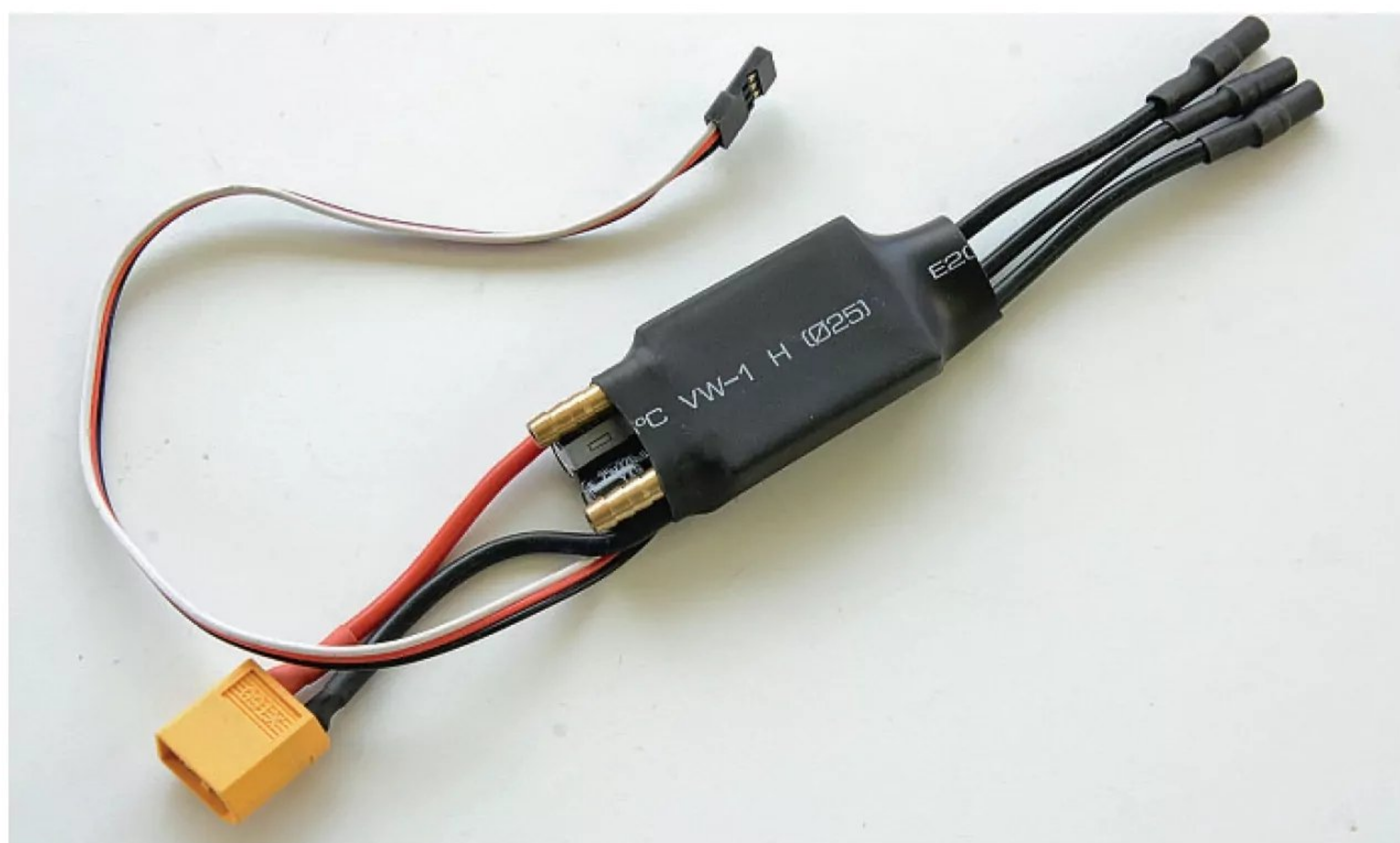
A modern water-cooled brushless speed controller.
