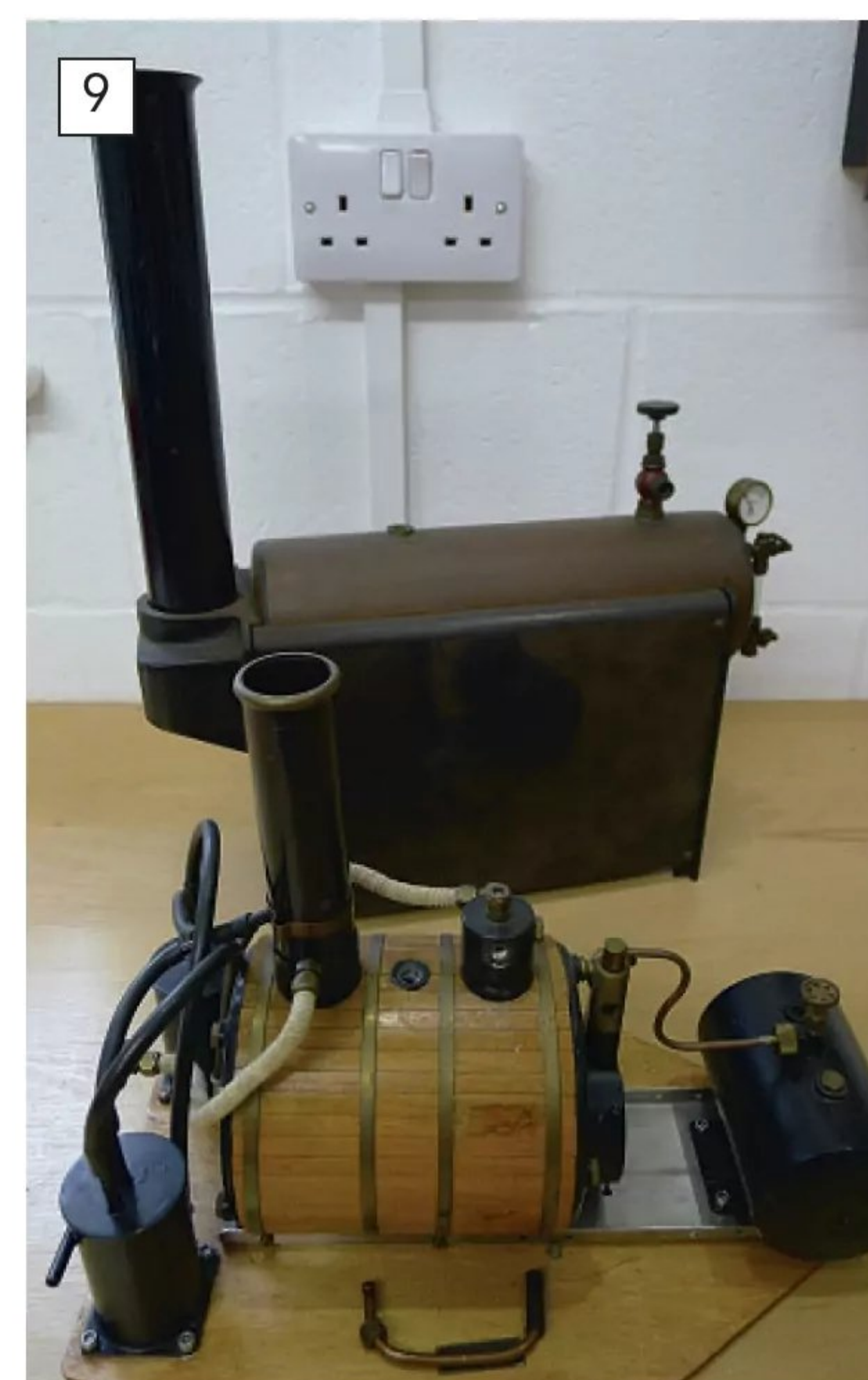
Examples of boilers above the 3 bar-litre limit: a 5" Cheddar boiler, produced to power two Puffin engines for a twin shaft model such as a tug, and the large Stuart Turner 504 boiler.
