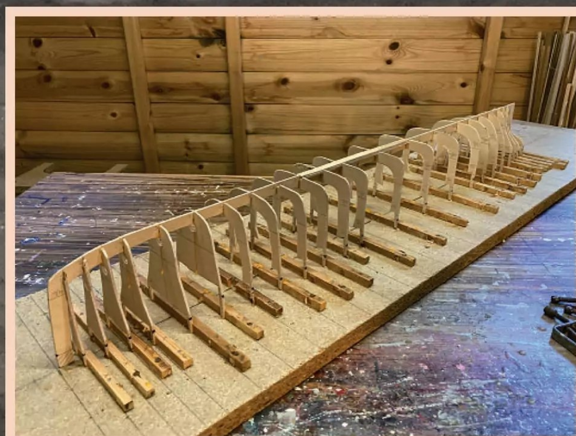
Titanic's frames on the building board.
