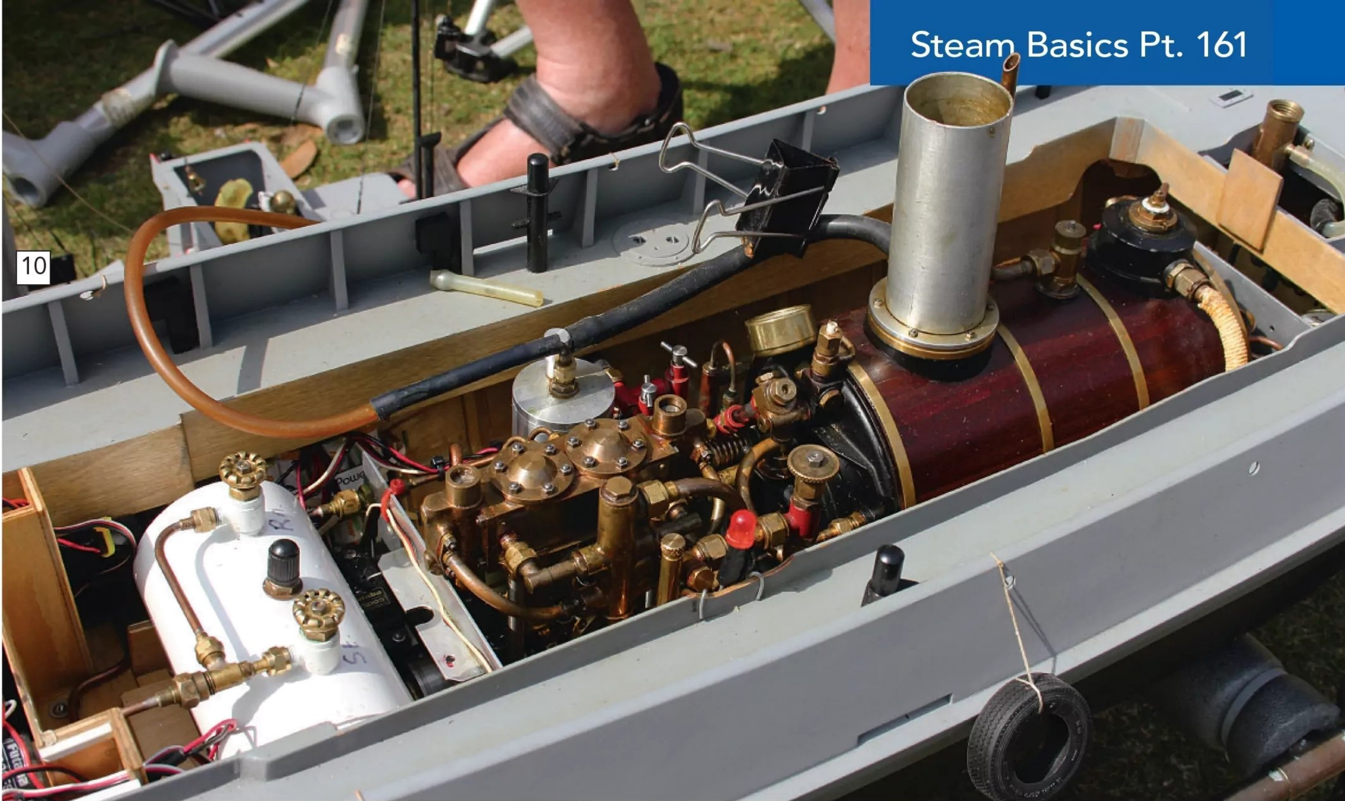
A typical larger than 3 bar-litres boiler in a large-scale tug. This will require removal for its four yearly hydraulic pressure tests, so the design of the plant must be done in such a way as to allow this.
