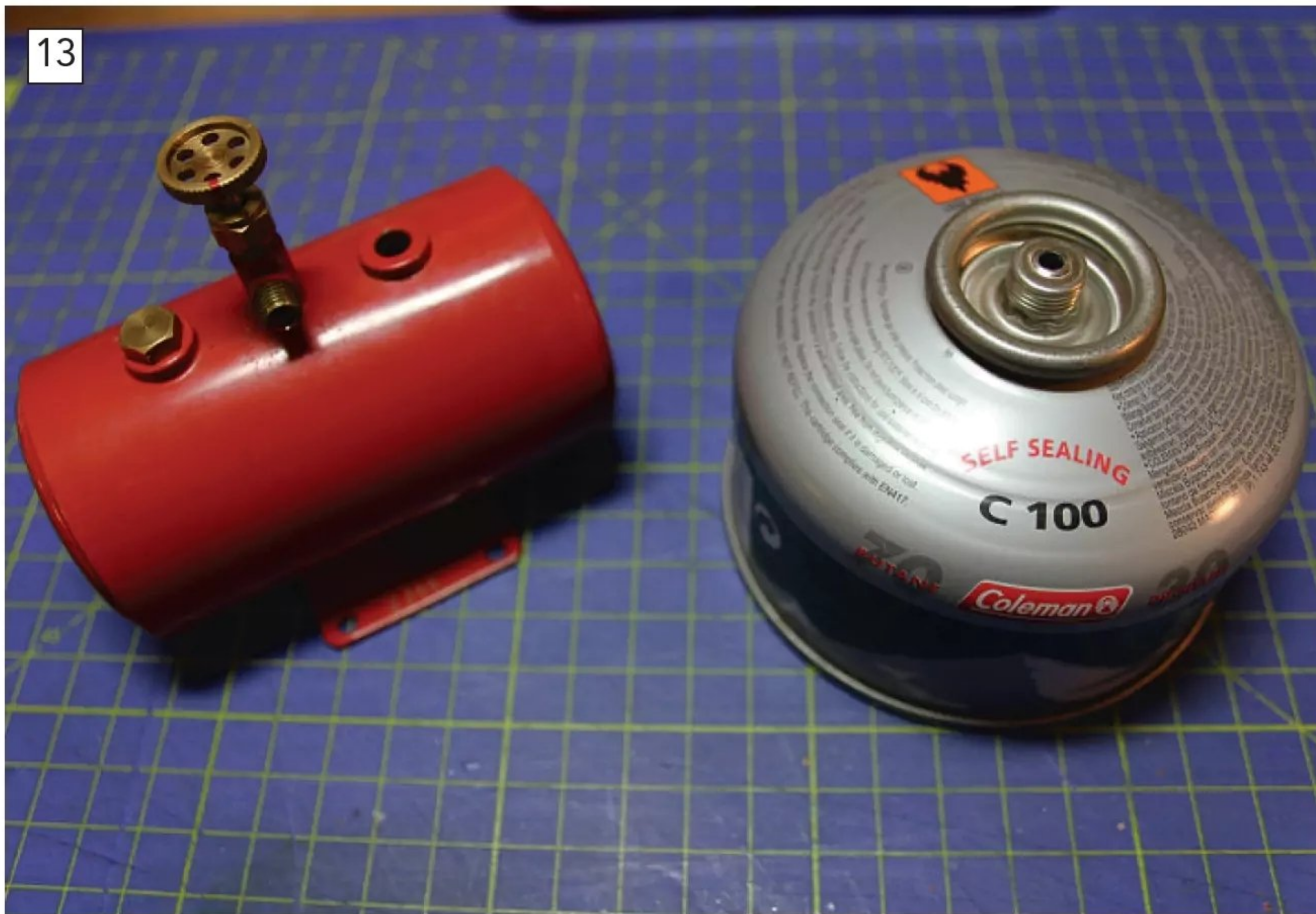
Volume 3 now covers the requirements for LPG tanks under 250ml. Most manufactured tanks with an initial pressure test certificate will not require further hydraulic pressure tests. They do require a safety check every five years though, so disposable tanks might be the easiest option.
