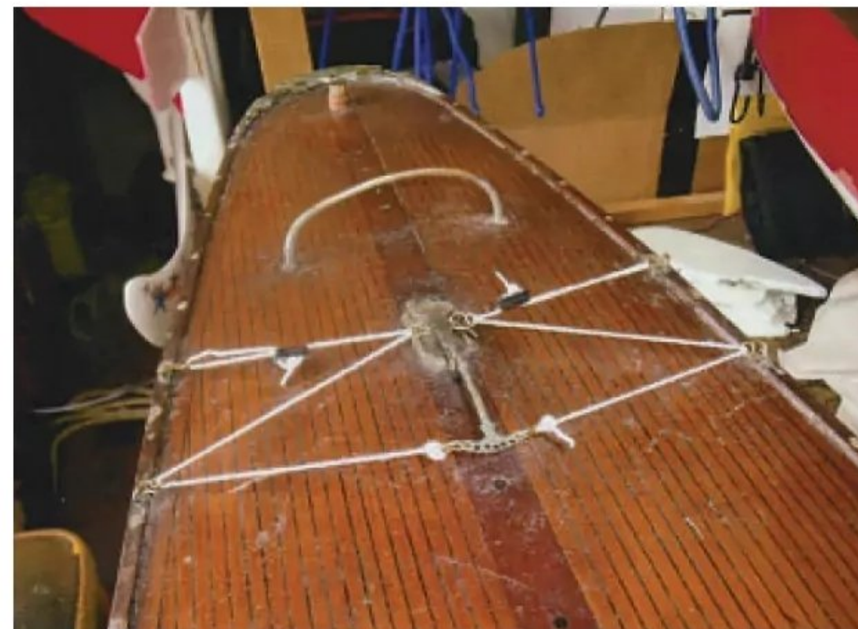
The 'adjustable' rudder steering on Fleetwing, as per original.
