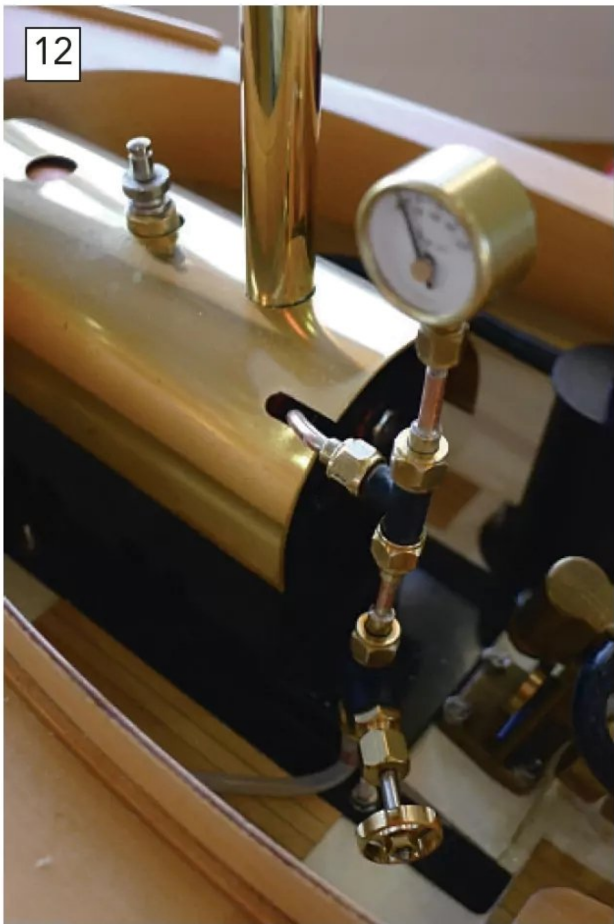
Small boilers are now classified as either LS or LO boilers. LO boilers have a steam outlet that is always open, but LS boilers can be shut off, as is the case with this Tony Green boiler with a steam isolating valve fitted.
