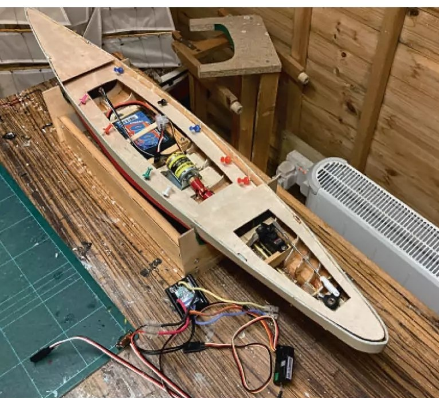
The fitting of 'false decks', made from thin ply, which will later be planked. The ESC is still outside the hull at this stage.
