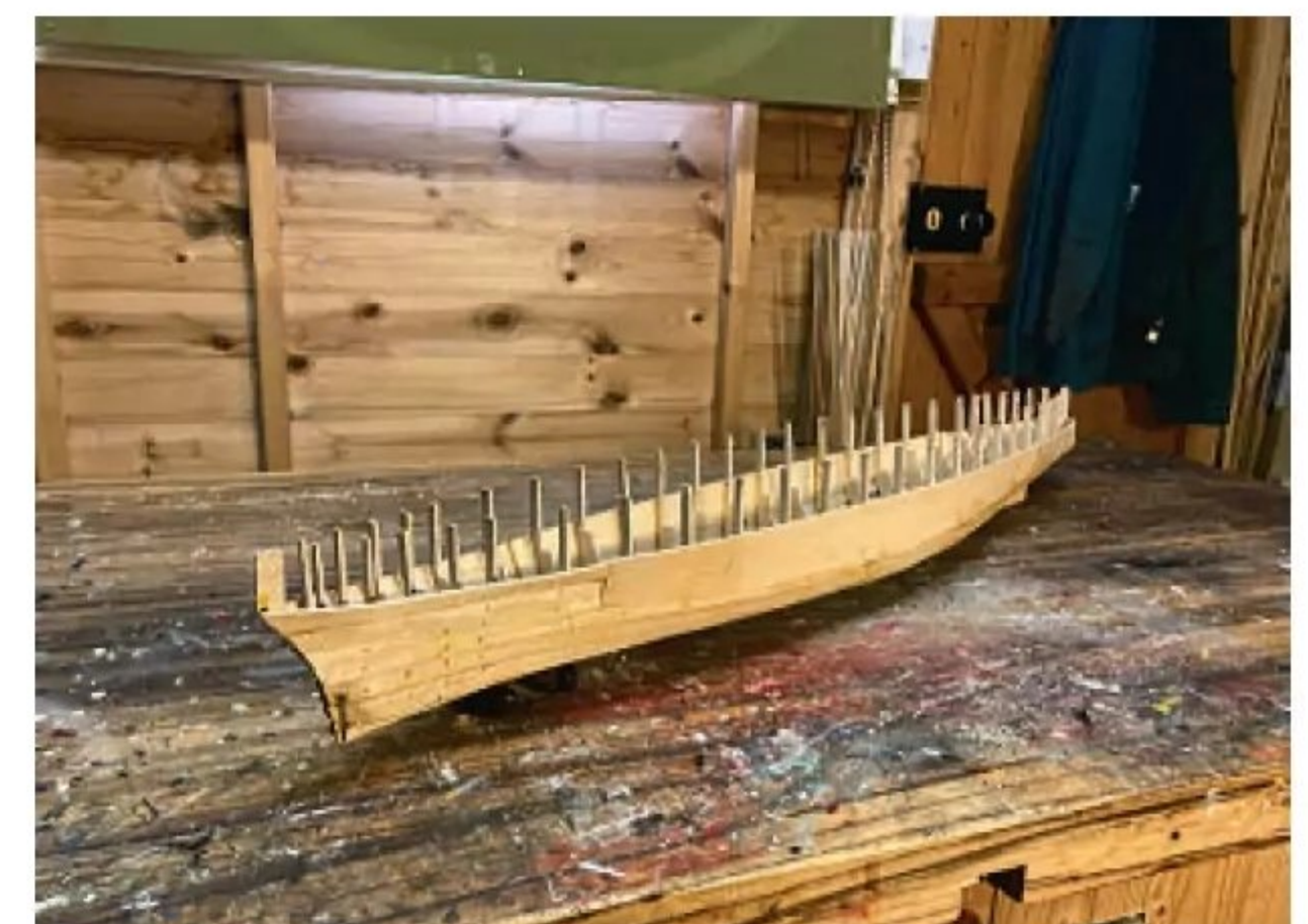
The hull released, but yet to be to cut off the uprights used to connect it to the board during building.
