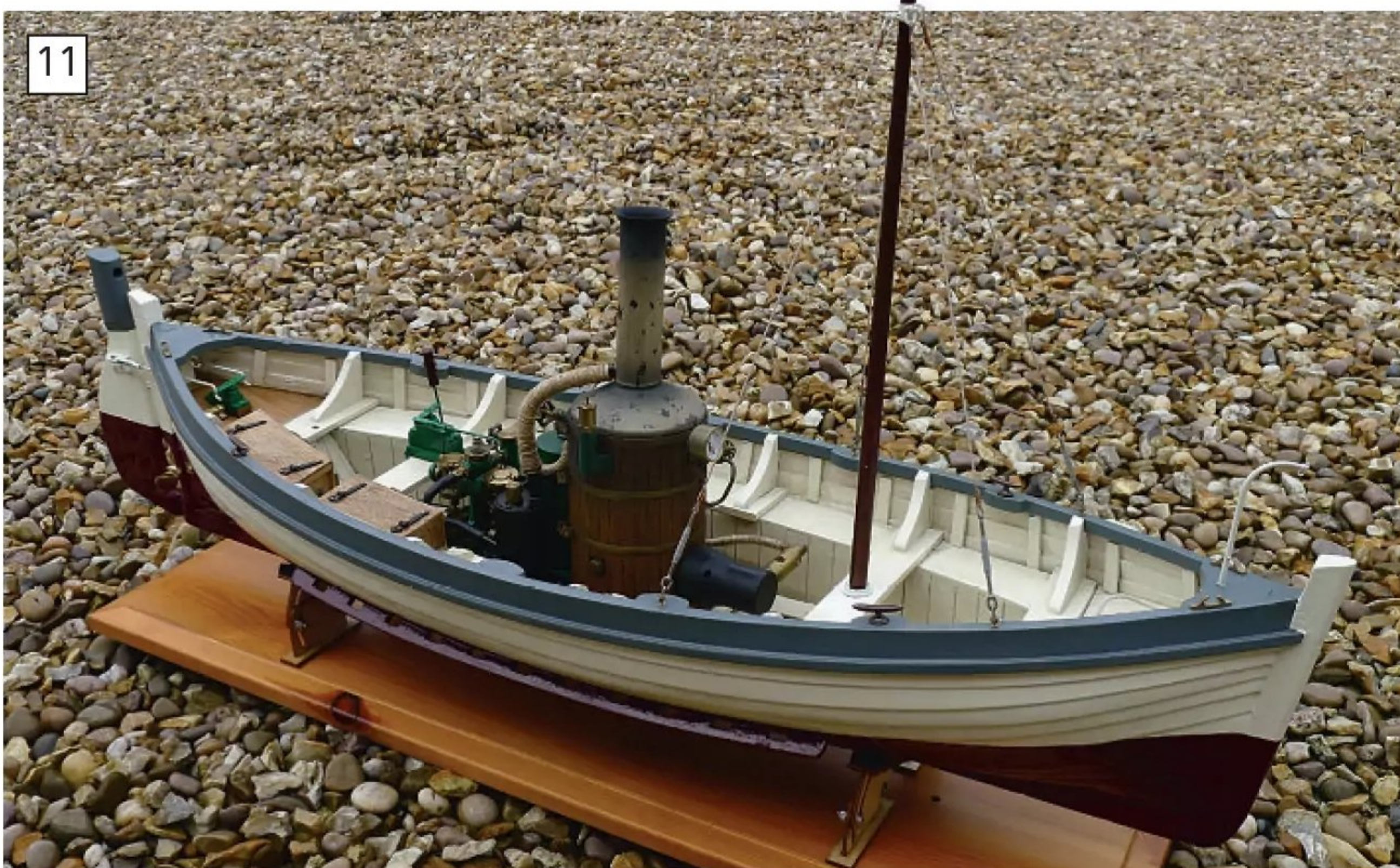
A very typical model boat with a pretty common boiler, a 3” vertical Miniature steam. This requires an initial hydraulic pressure test (which is good for life as long as no modifications or repairs are done) and then annual steaming tests.
