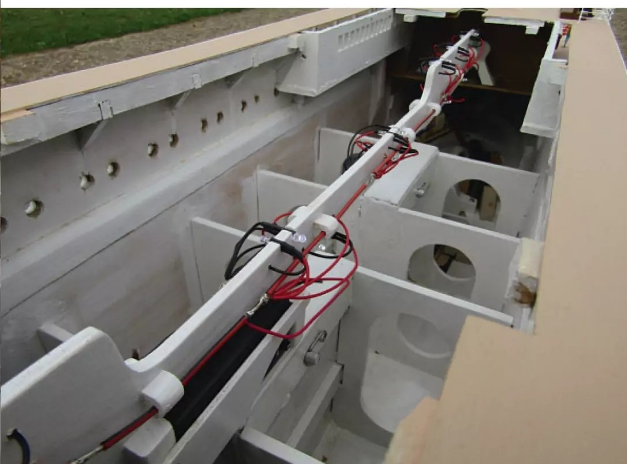
The light bar, and the bracing of the keel boxes.
