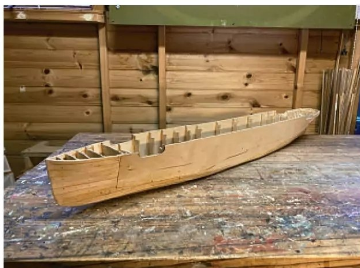
Titanic's hull off the building board. The sheerline has been cut to shape.
