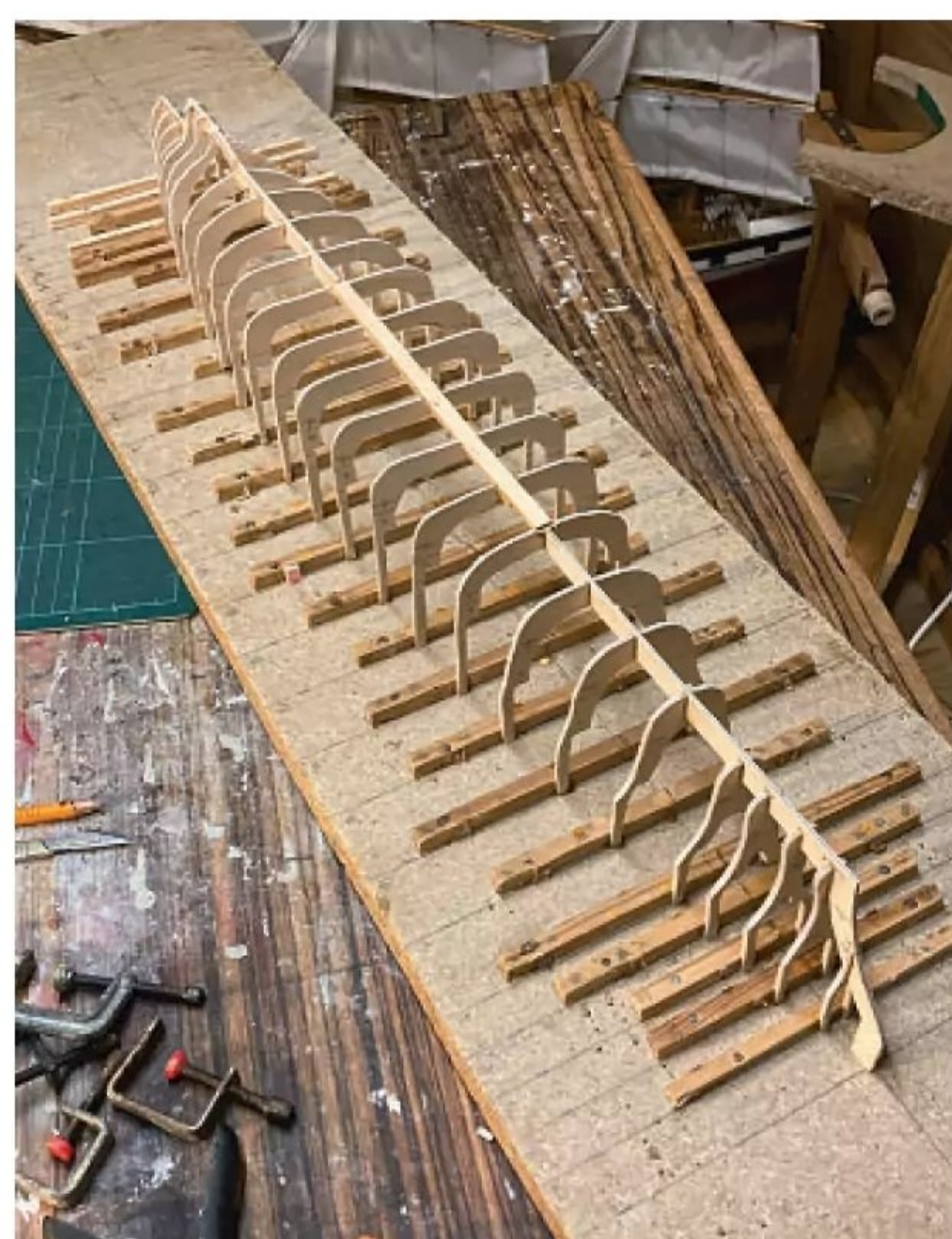
Bismarck's frames on the building board.
