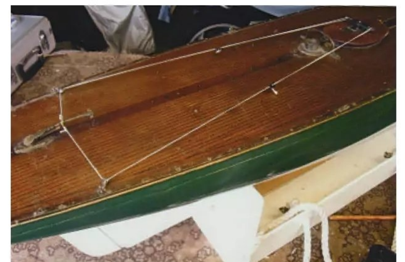
The R/C steering newly installed by Brian for the rudder. The servo for this is incorporated in a replacement hatch, while the battery and RX are attached underneath. The model, however, can easily be returned to former operation simply by swapping back to the retained original hatch.
