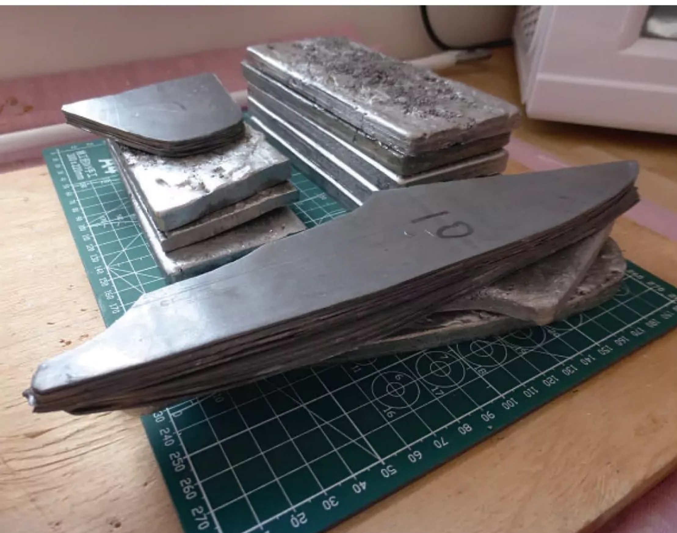
The 22lb of lead segments Barry initially decided to line the bottom of the hull’s interior with.
