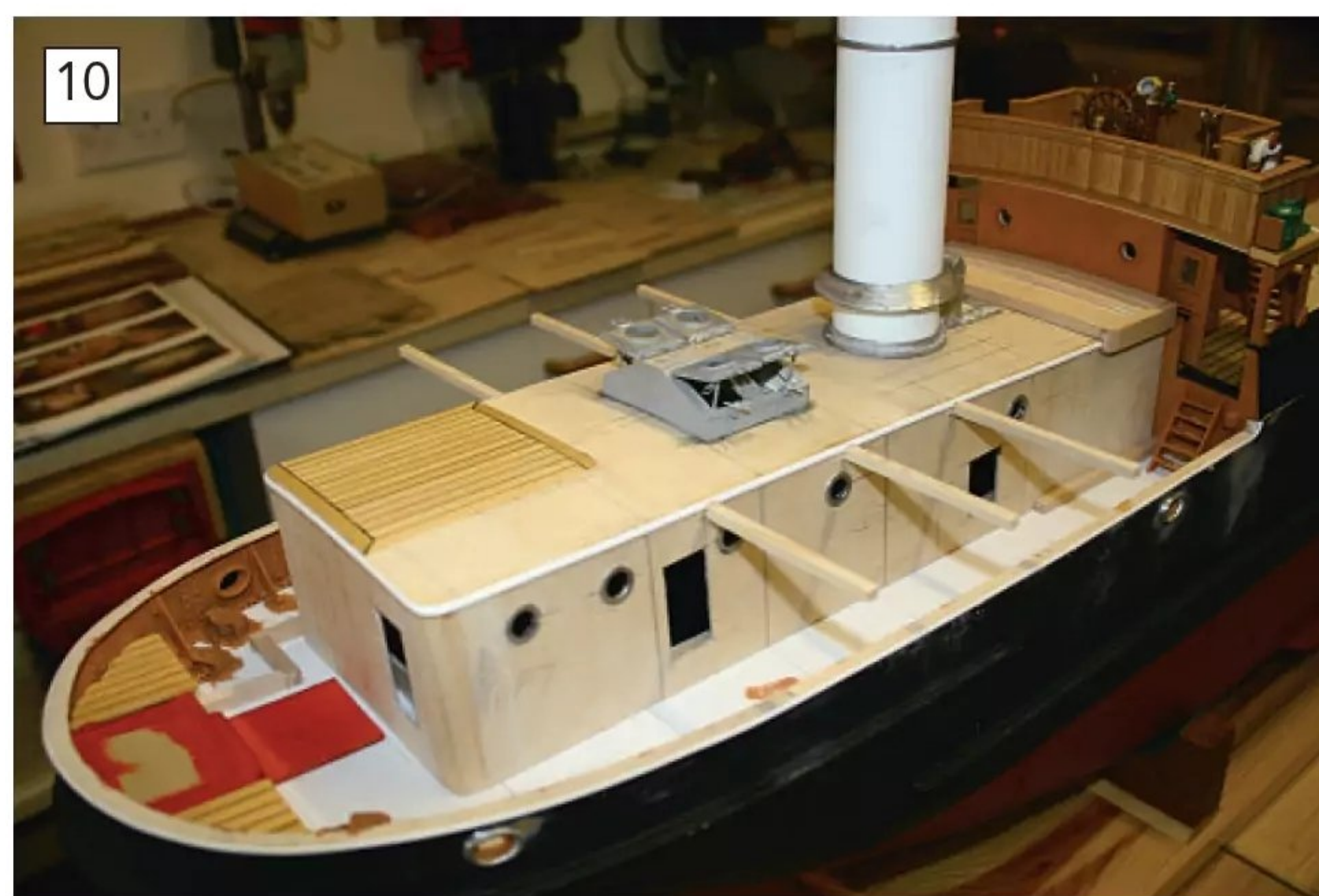
With the basic box complete, additional parts, such as the funnel with its details, the engine room skylight, the section of decking, the forward bunker and the beading around the top edge of the bulkheads, were added.
