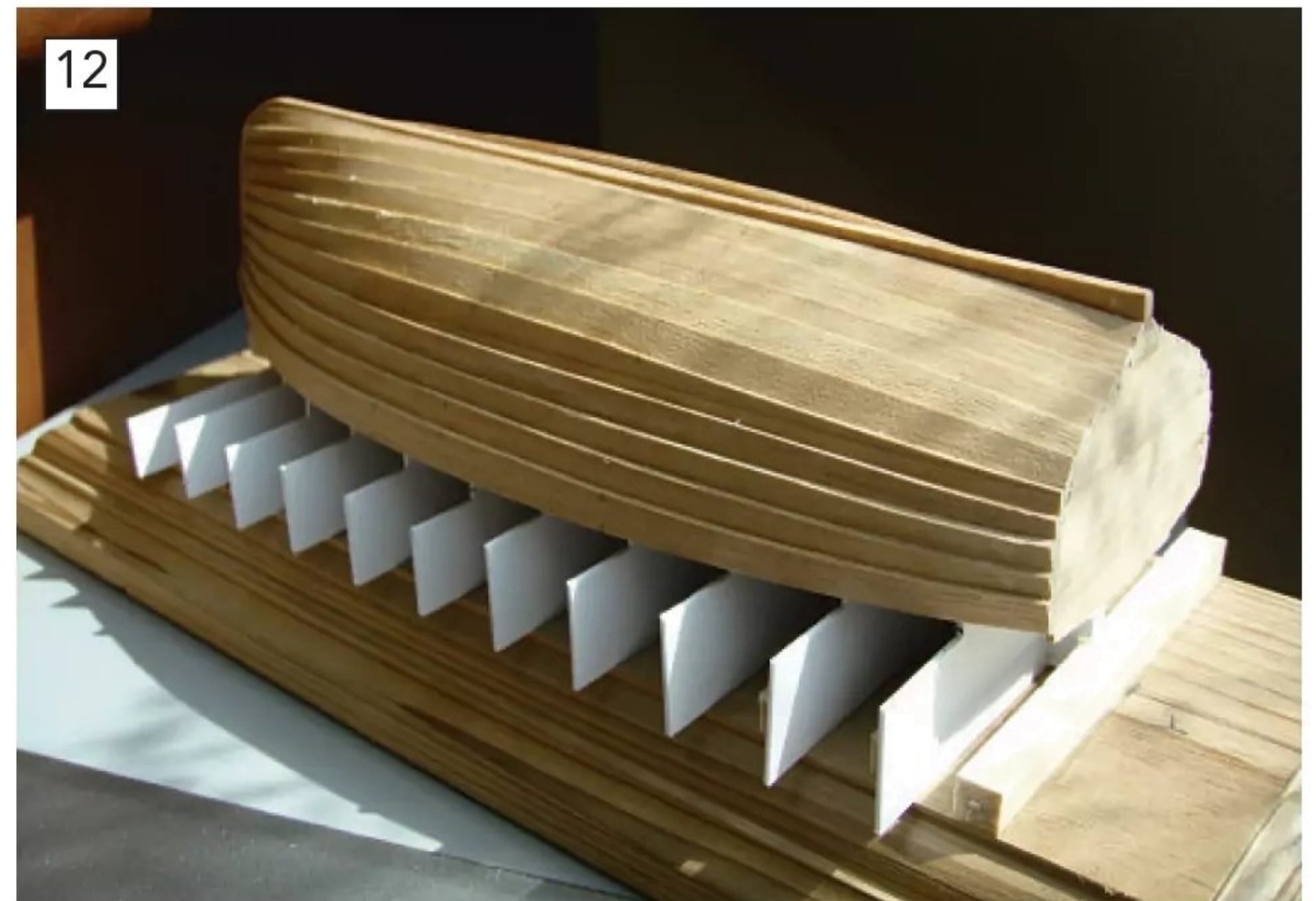
With all the planking complete around the hull sides, the familiar shape of a clinker-built ship's dingy emerged. Very pleasingly, the planking looked as good on the inside as it did on the outside, so a great foundation for a nicely detailed interior.
