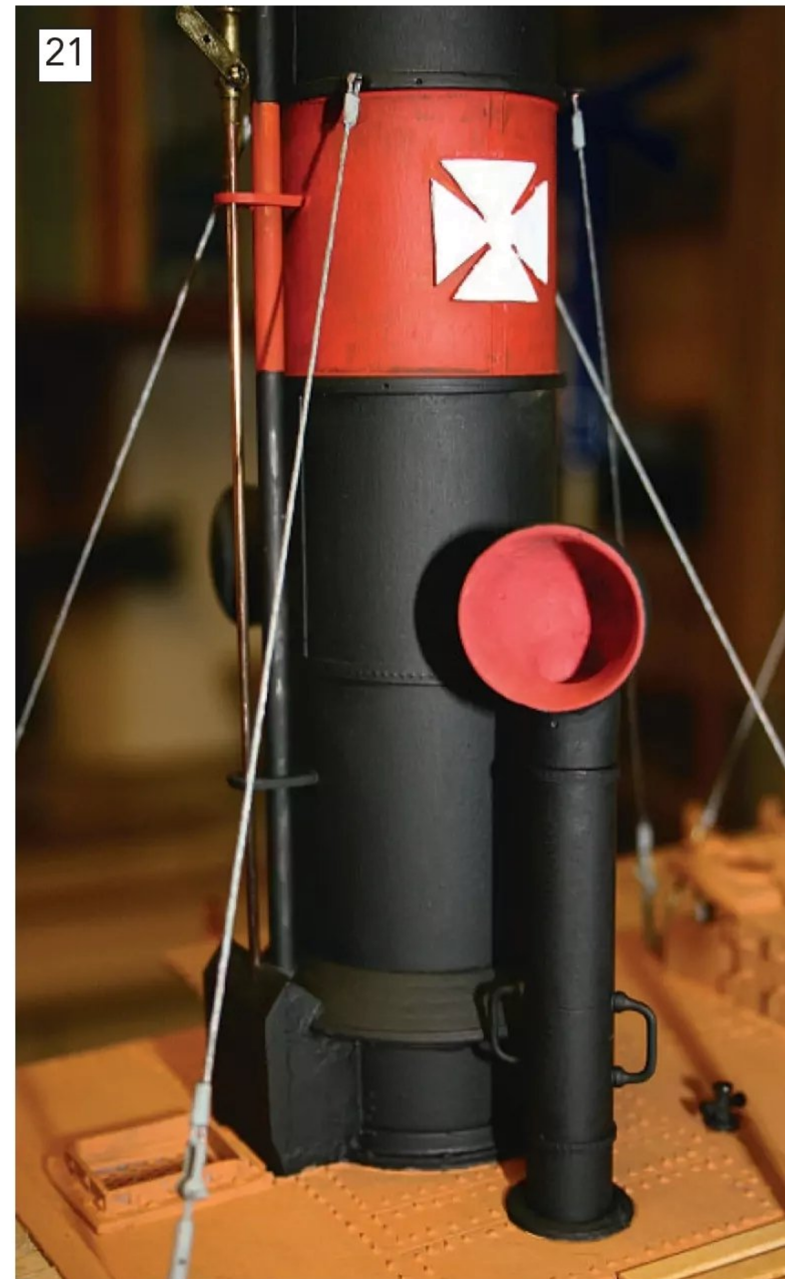
The vent cowls were machined out and fitted with copper tubes to enable as much ventilation into the hull as possible. Joints were enhanced with more riveted straps.
