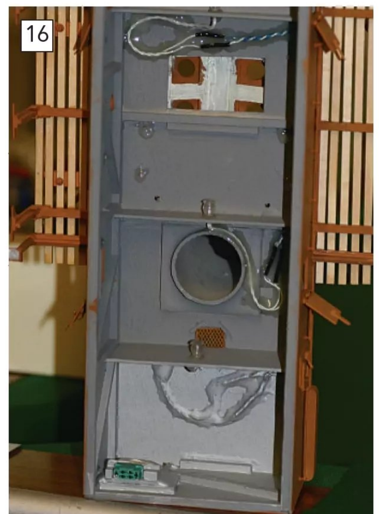
Internally, a light on each bulkhead and a stern light on the top deck were all wired into a plug fitting that located into a socket fitted to the inside of the coaming, thereby enabling the unit to be removed without the need to disconnect wires.
