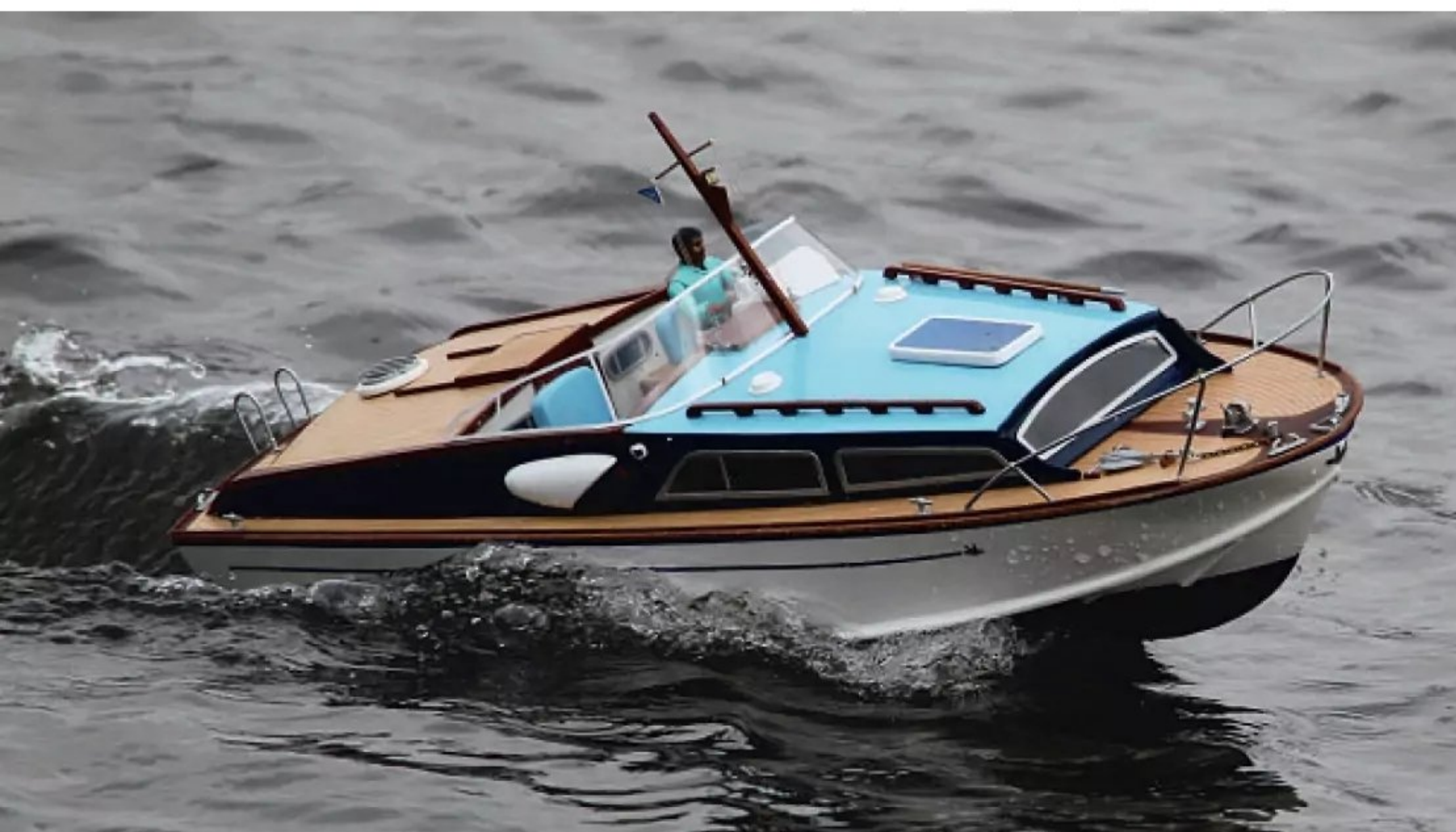
SLEC's Fairey Swordsman kit designed by the late Dave Milbourn is a very successful example of the use of laser cut Lite Ply for lightweight accurate hull construction.
