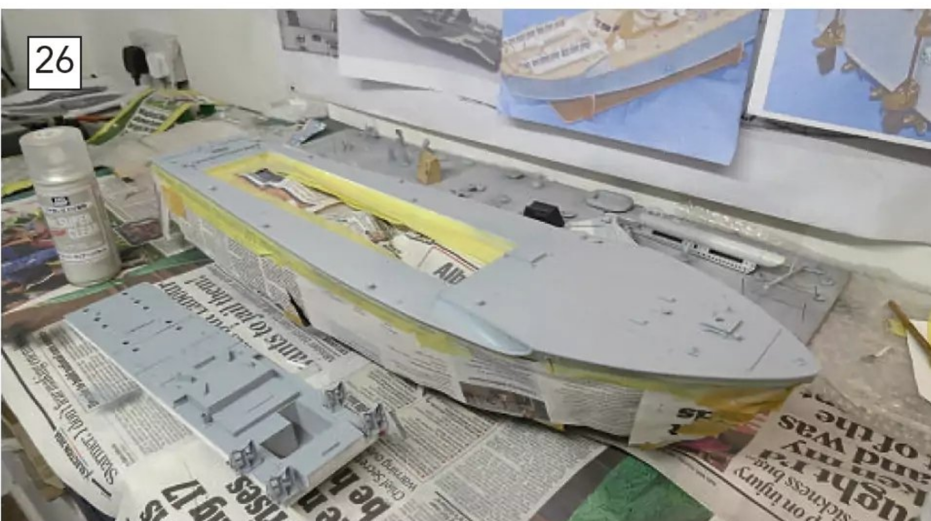
Preparing the deck and fittings for camouflage coatings.
