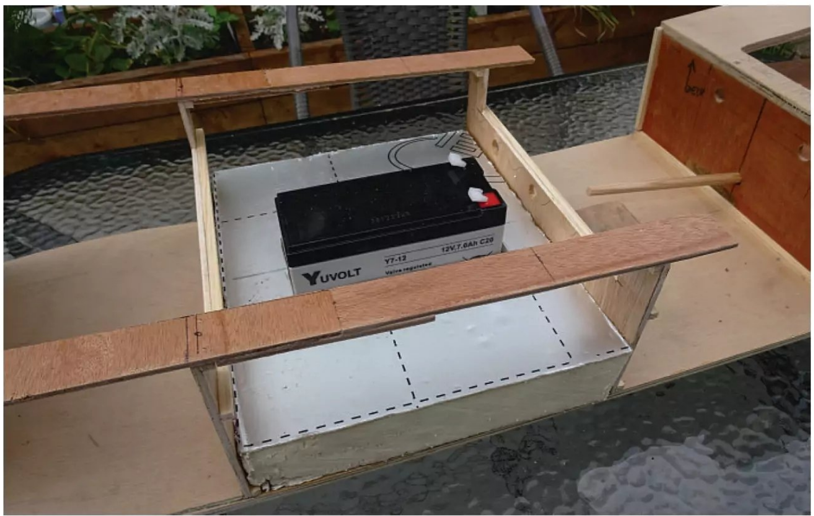
A piece of cavity wall insulation foam was used to add buoyancy and form the battery compartment.
