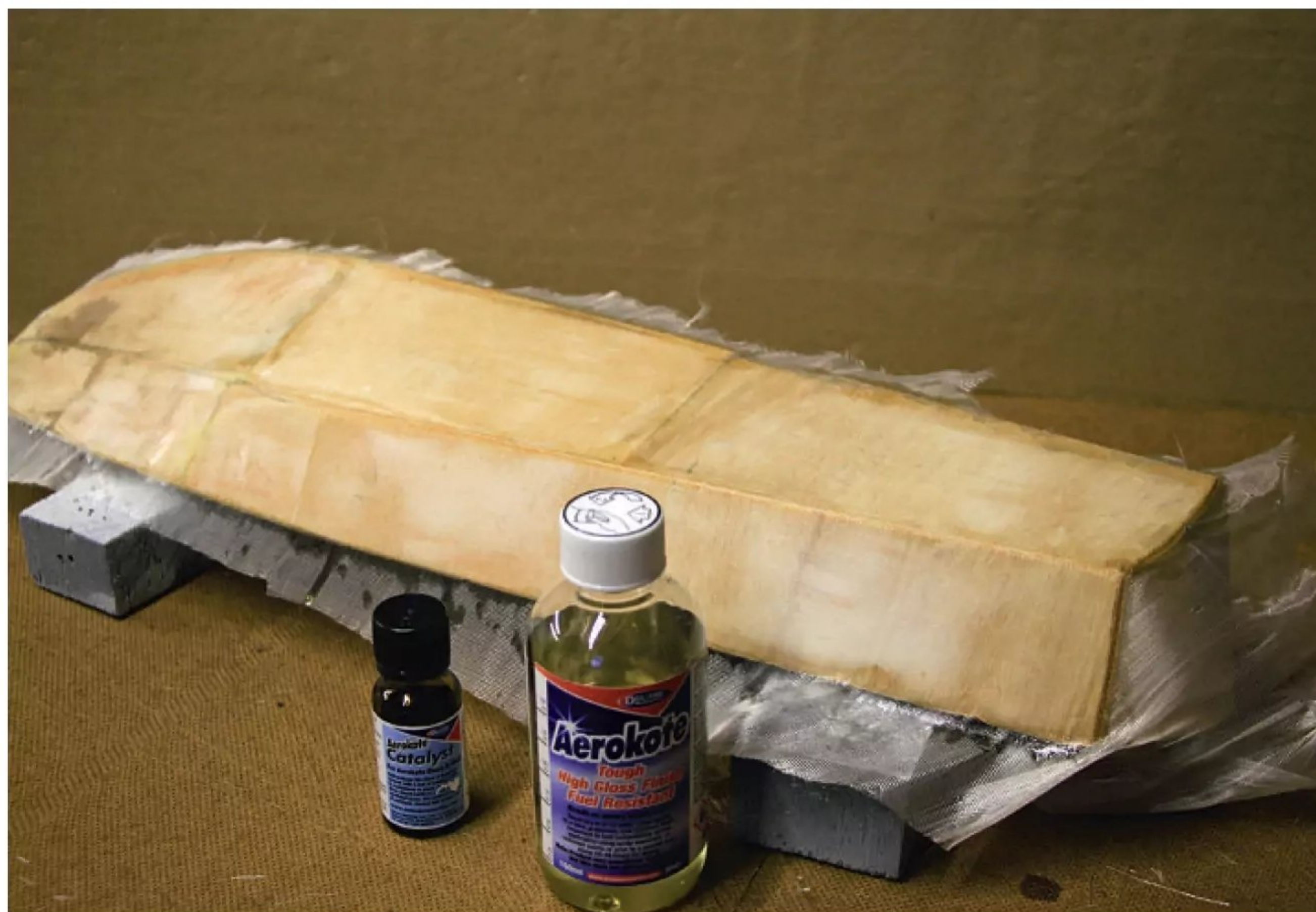
Application of glass cloth to the SLEC Fairey Huntsman kit to toughen the hull. Aerokote, finishing resin or Deluxe Materials Eze Kote can all be used.
