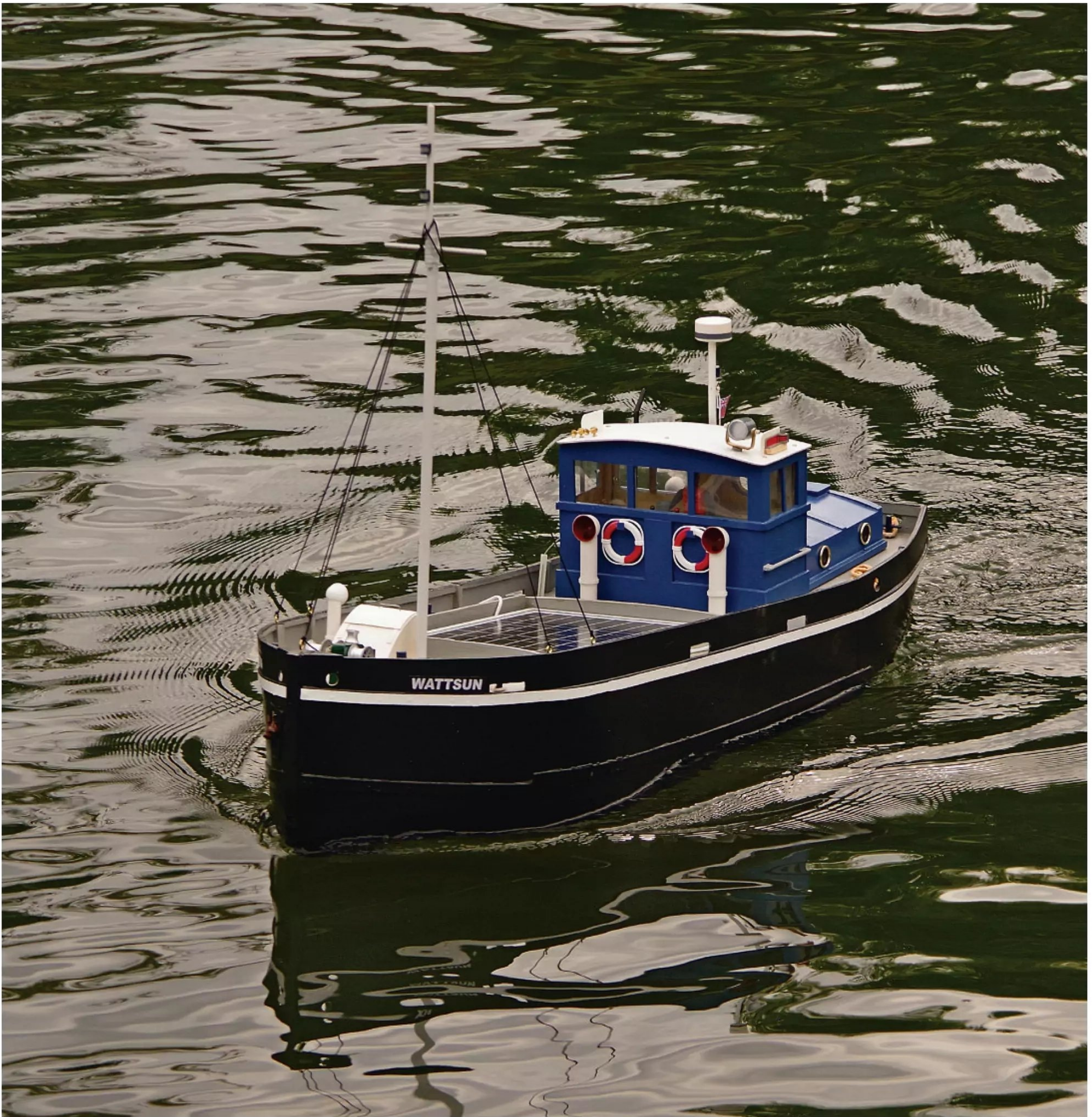
Adding a few fittings transformed a basic plywood box into a reasonable looking model boat. The only purchased items were the anchor, life rings and the working hollow ventilators.
