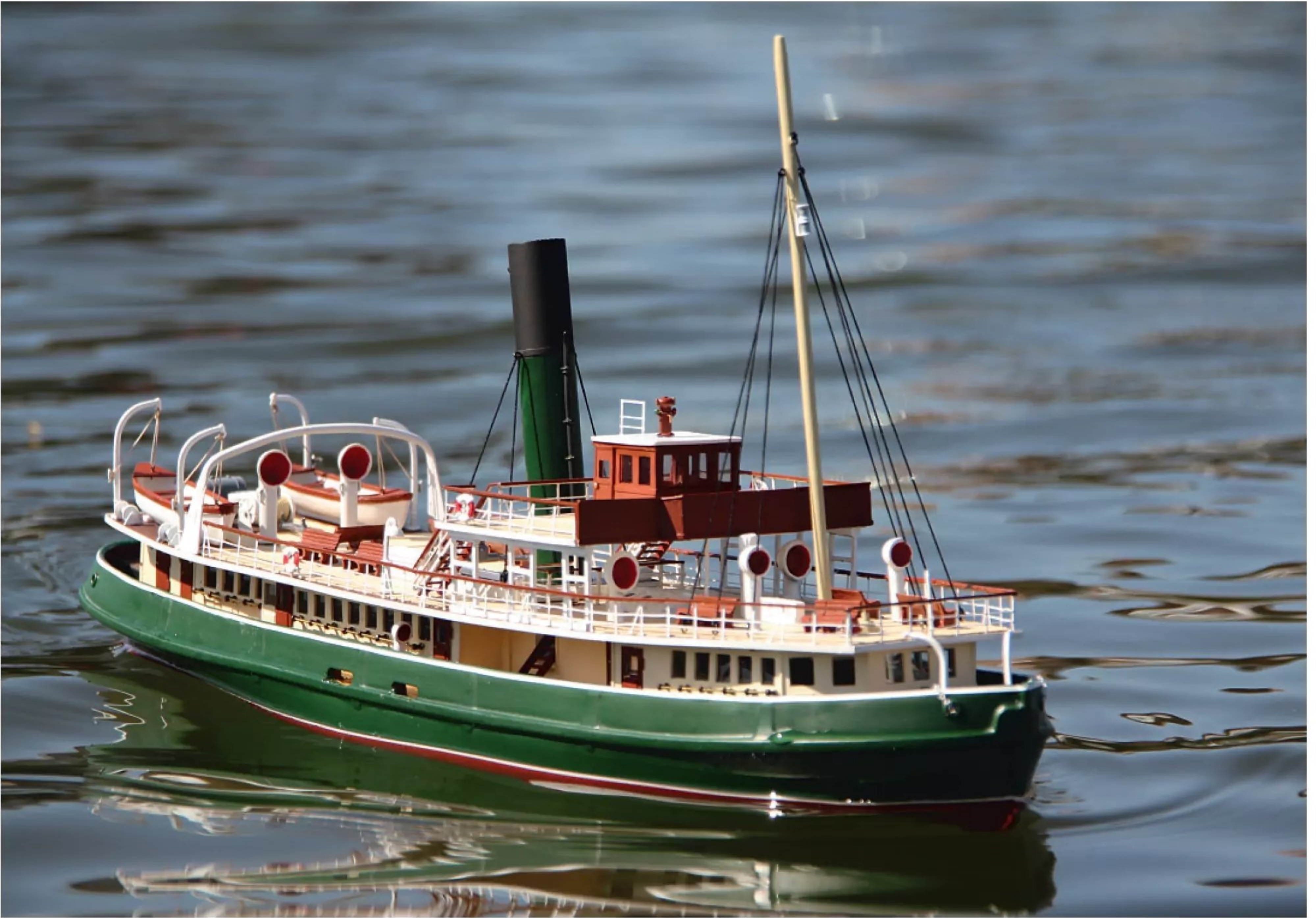
The Deans Marine Compact Kit of the tug tender Sir Francis Drake typically incorporates a GRP hull with plasticard decks, vacuum formed mouldings for the funnel and lifeboats, and a mixture of white metal and resin fittings.
