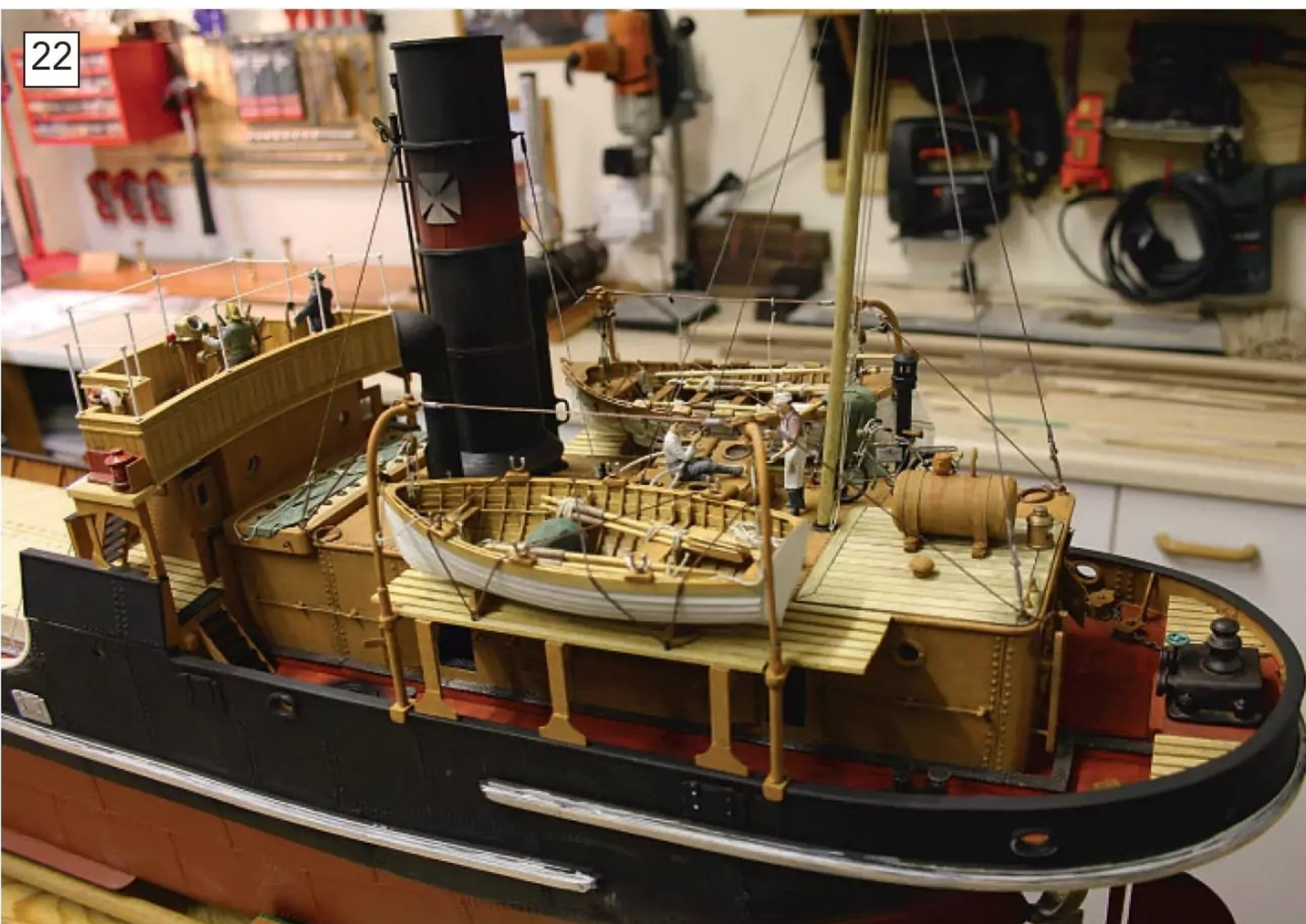
A pleasing look to the aft end of the model, with lots of added detail, and the camber, the fit and the plate detail all making the accommodation unit worth the additional effort.
