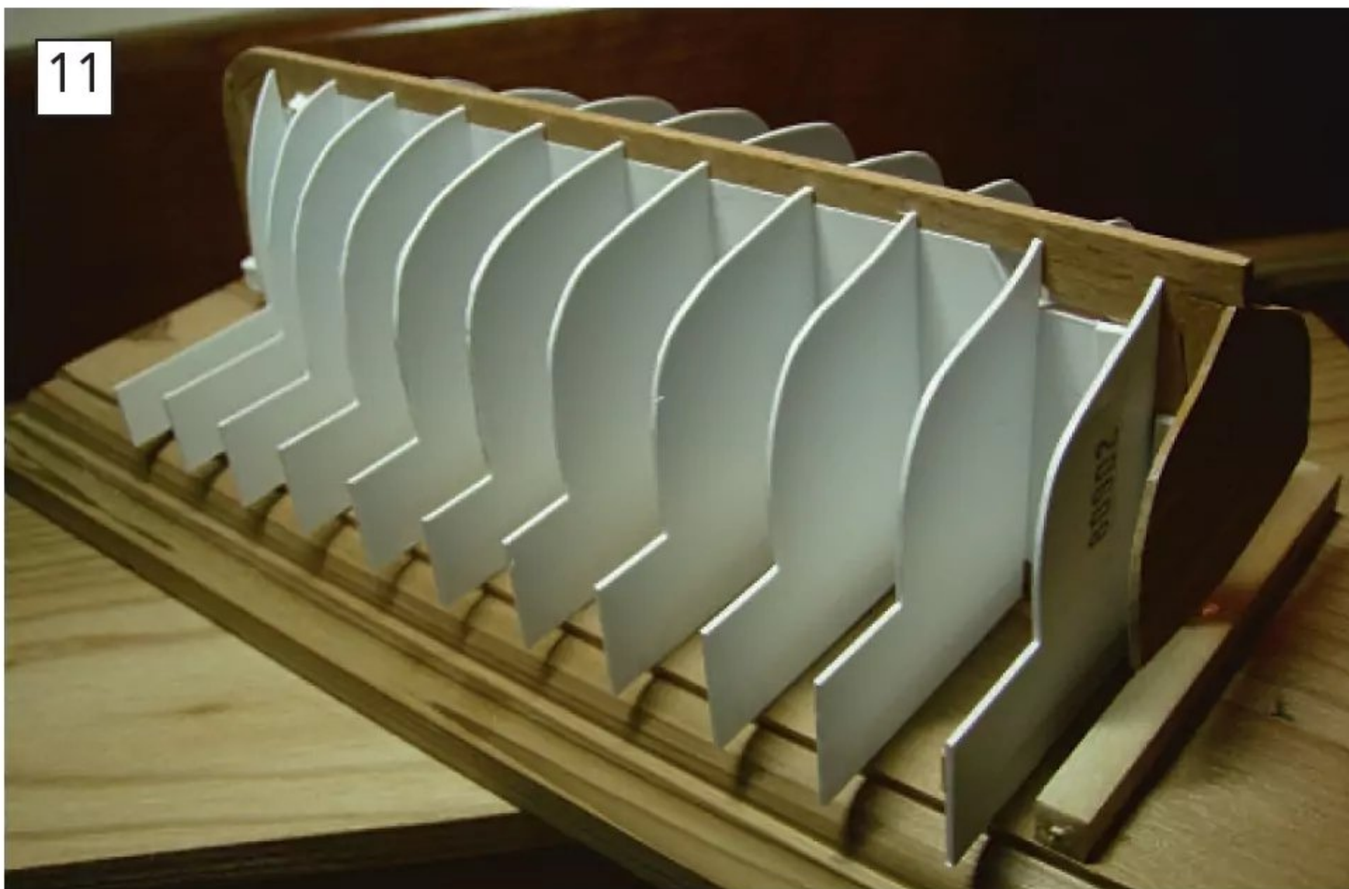
The plan was copied and adjusted dimensionally to give the appropriate length and width for the Ben Ain's dinghy. From this plan an inverted jig was made on which the model boat could be built. Being inverted, the first piece was the keel with transom and stem post that was laid across the top of the jig.
