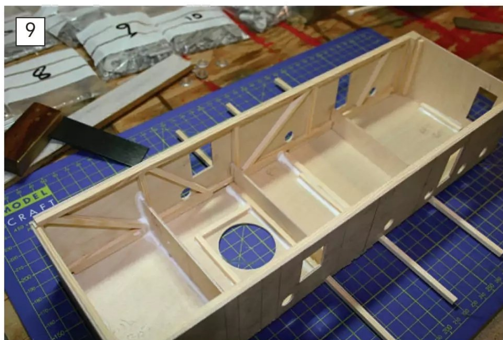
Internally a little additional bracing was added, and generous beads of glue were run along the edges of the framework to ensure the strongest possible joints and no possibility of the curved deck lifting.
