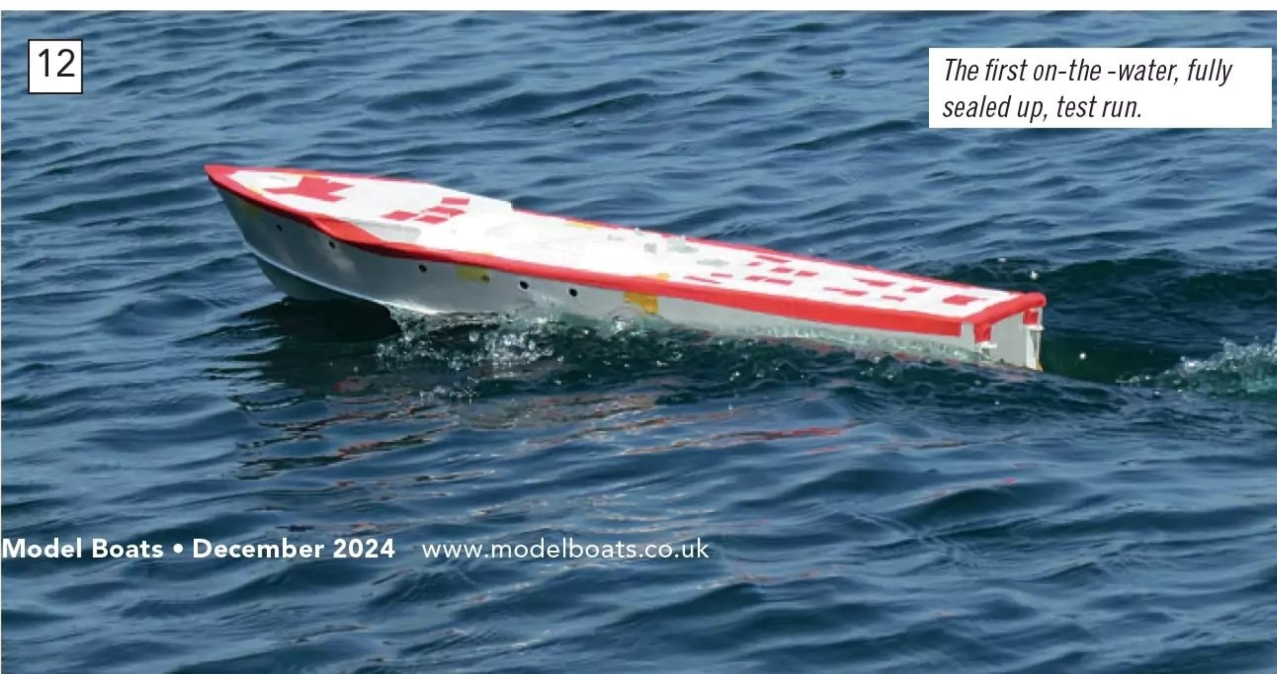
Dave realised that for a working model the spray strip from the kit would be inadequate, thus a length of 2mm square Evergreen strip was added.
