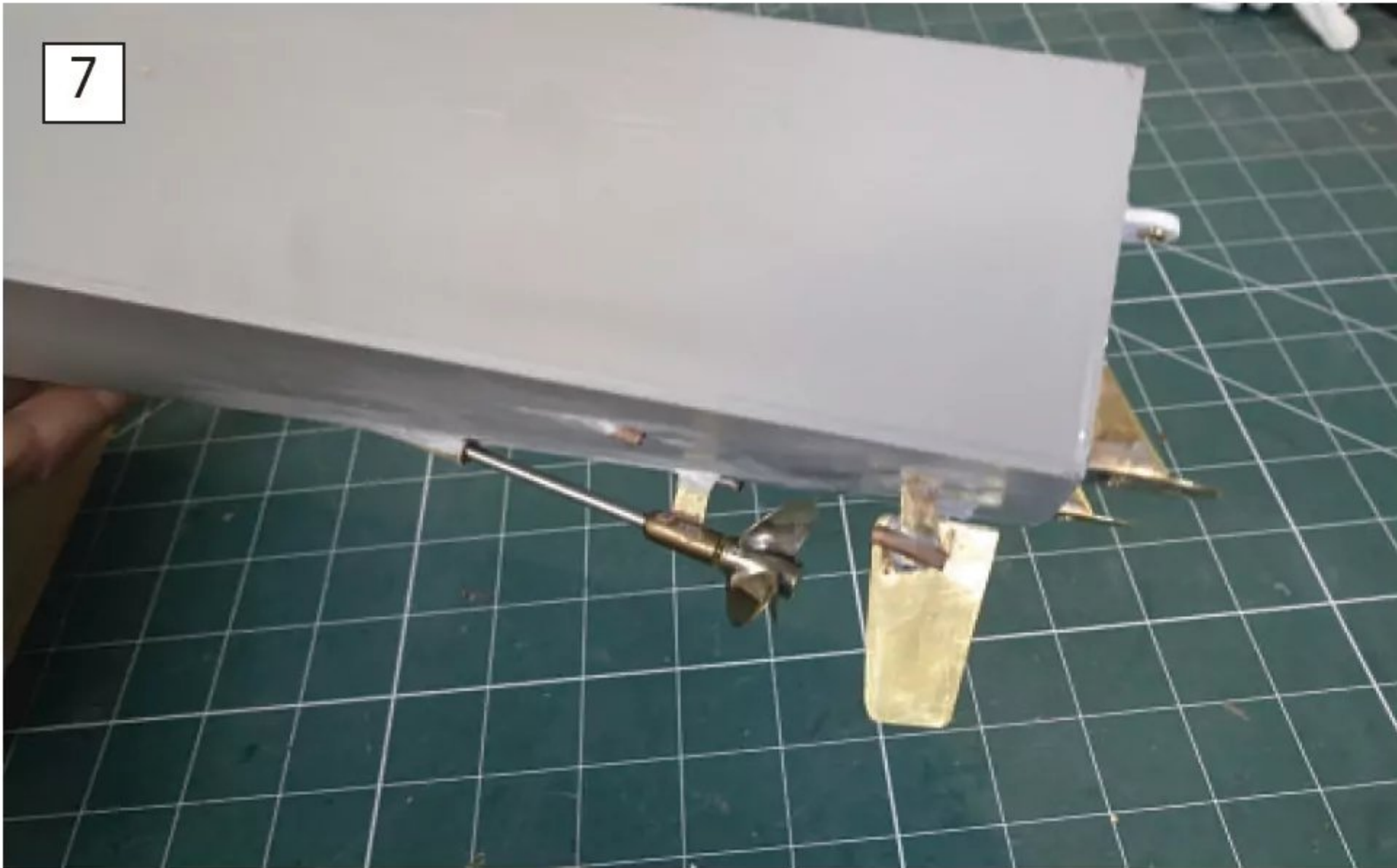
The centre drive shaft, functioning rudder and 25mm brass propeller.
