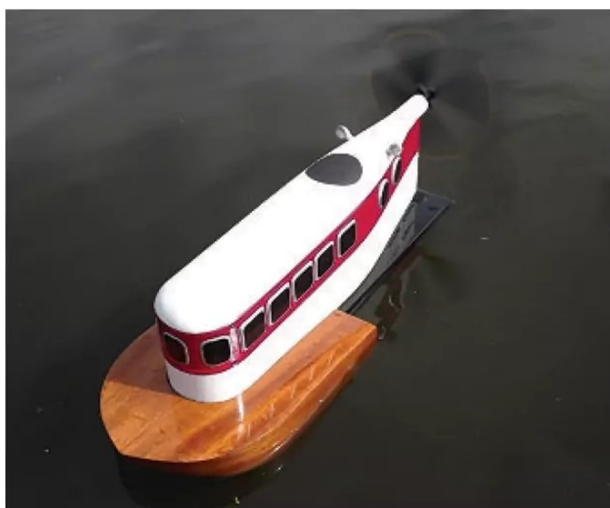
The 'wood' pontoon of Ashley's Farman Hydroglisseur is in fact veneered Styrofoam! Image courtesy of Ashley Needham.
