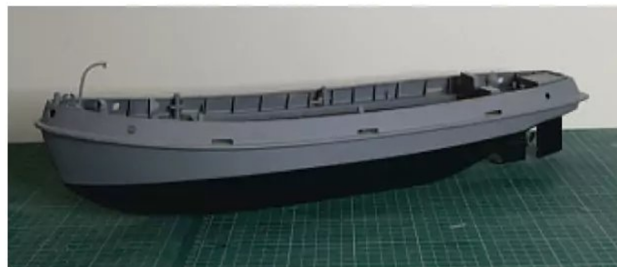
The Duplex TID Tug, an old kit but a fair representation of vac-form and plasticard construction. Humbrol's acrylic spray cans were used to create the base layers ready for weathering.
