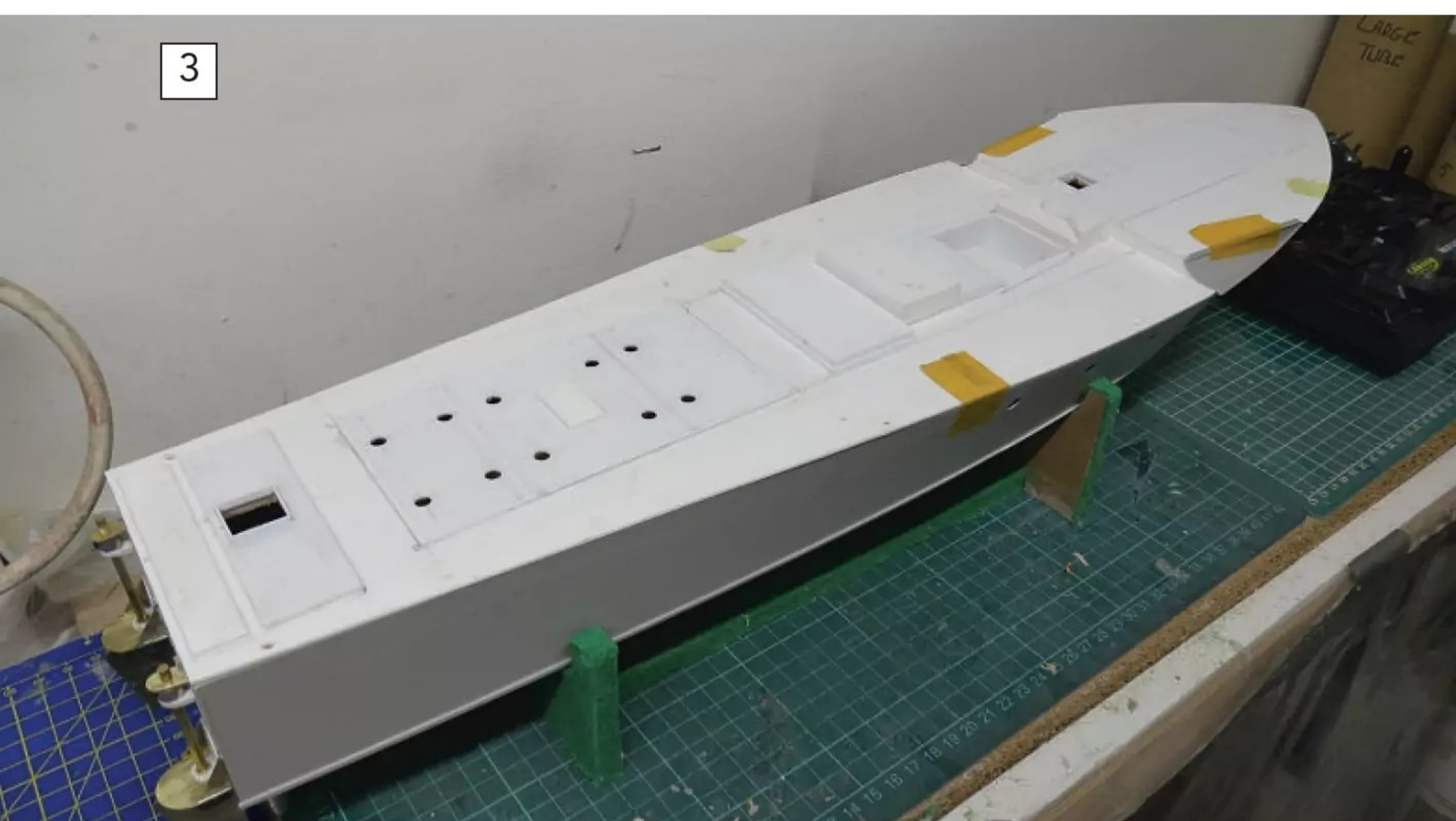
Dave's styrene deck fitted onto the hull.
