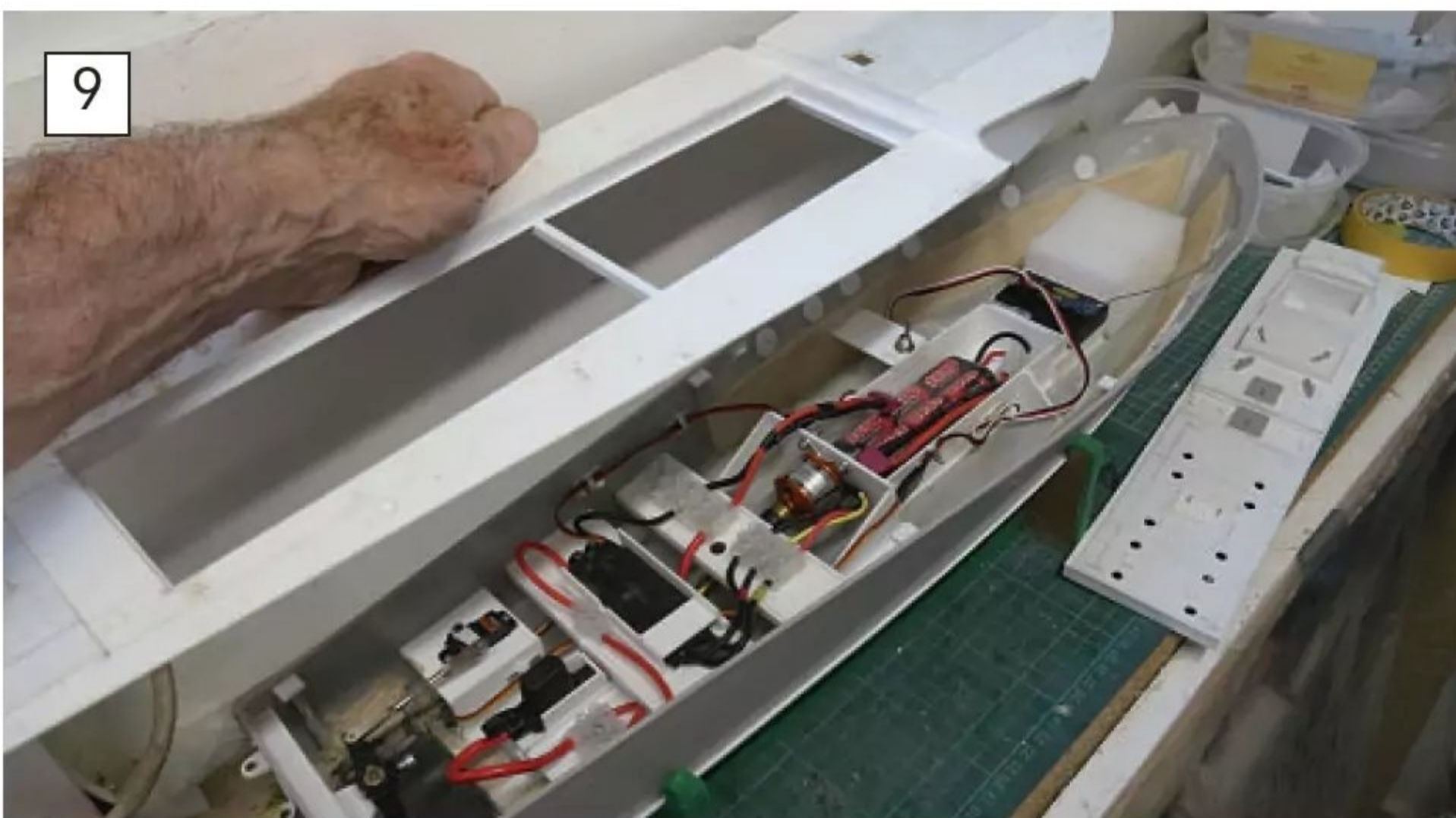
Fixing the replacement deck onto the prepared hull.
