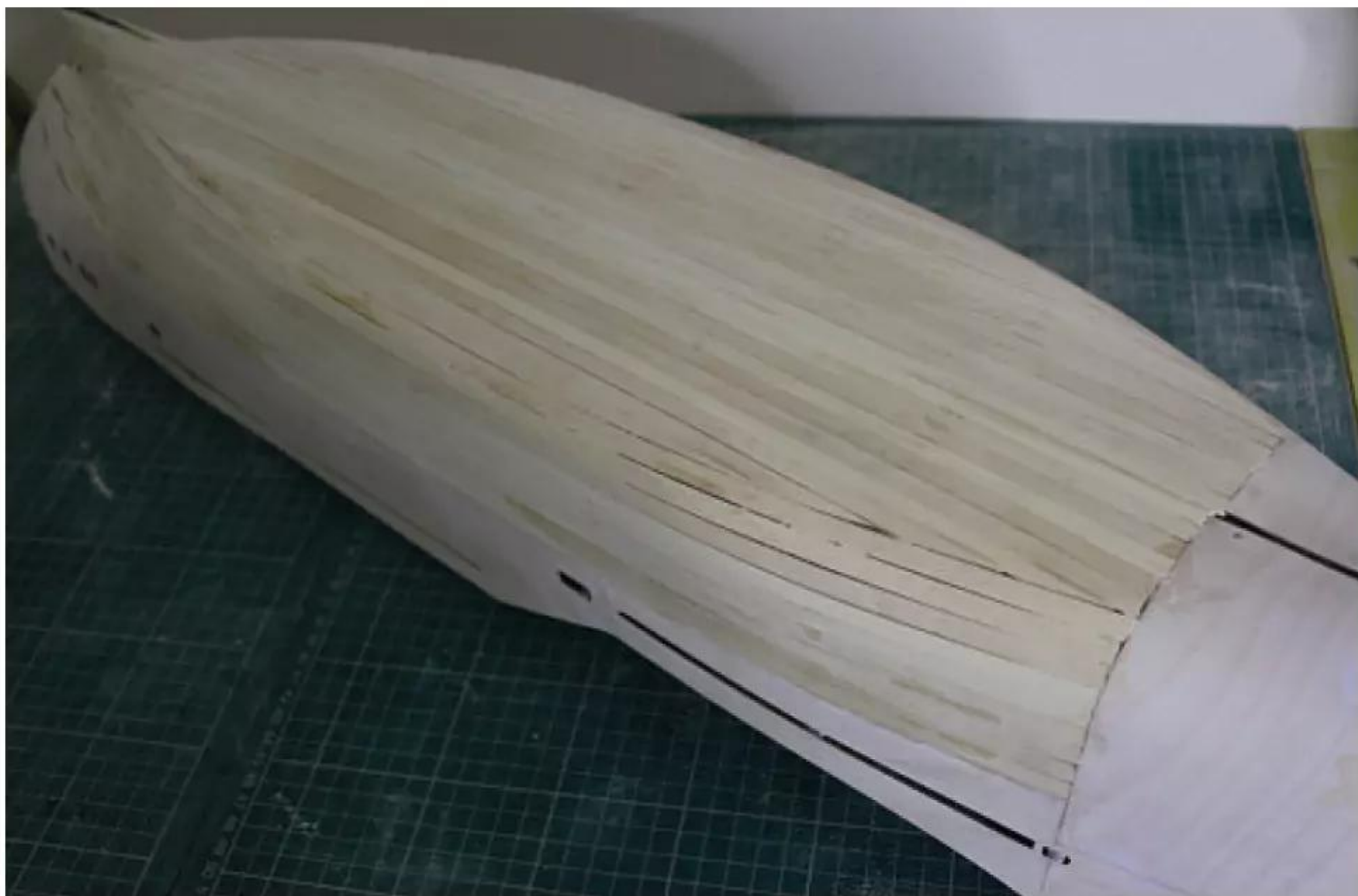
Planking is completed using the Obechi wood strip supplied. If you start below the plywood bulwark plates and continue towards the keel, you should have no problems, Nick points out.
