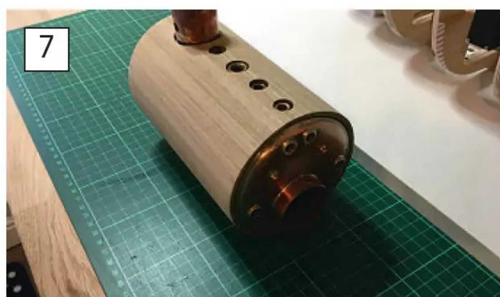
Here, Mr. Mark Tommy shows just how neat a homemade insulation job can be. Again, circular holes around the fittings and chamfering the internal edges to get the external edges perfectly mated together makes for a superb finish.
