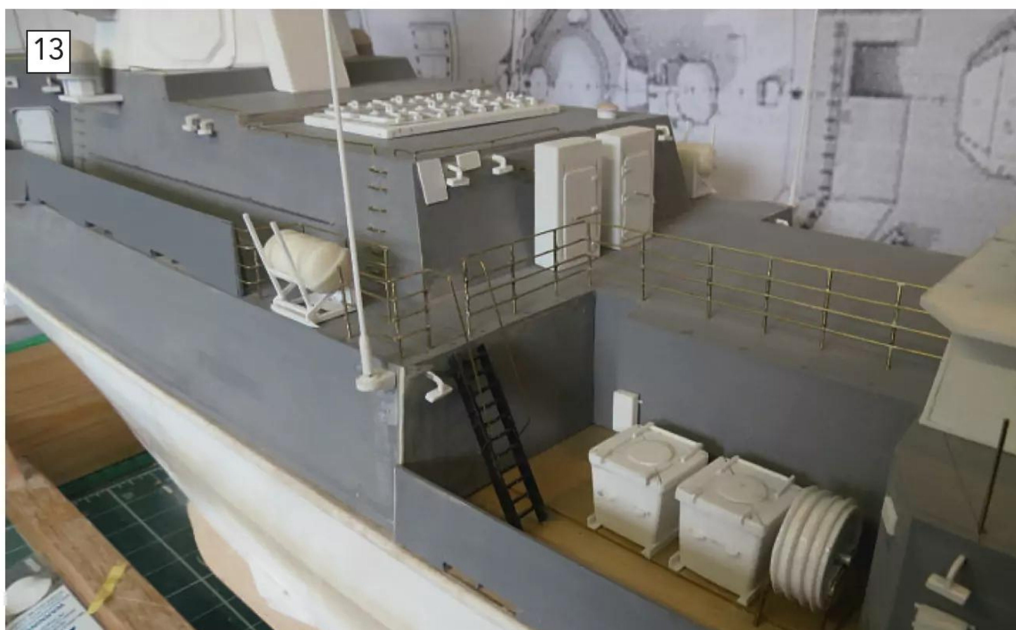
Locating part of the four-bar rail amidships to port.
