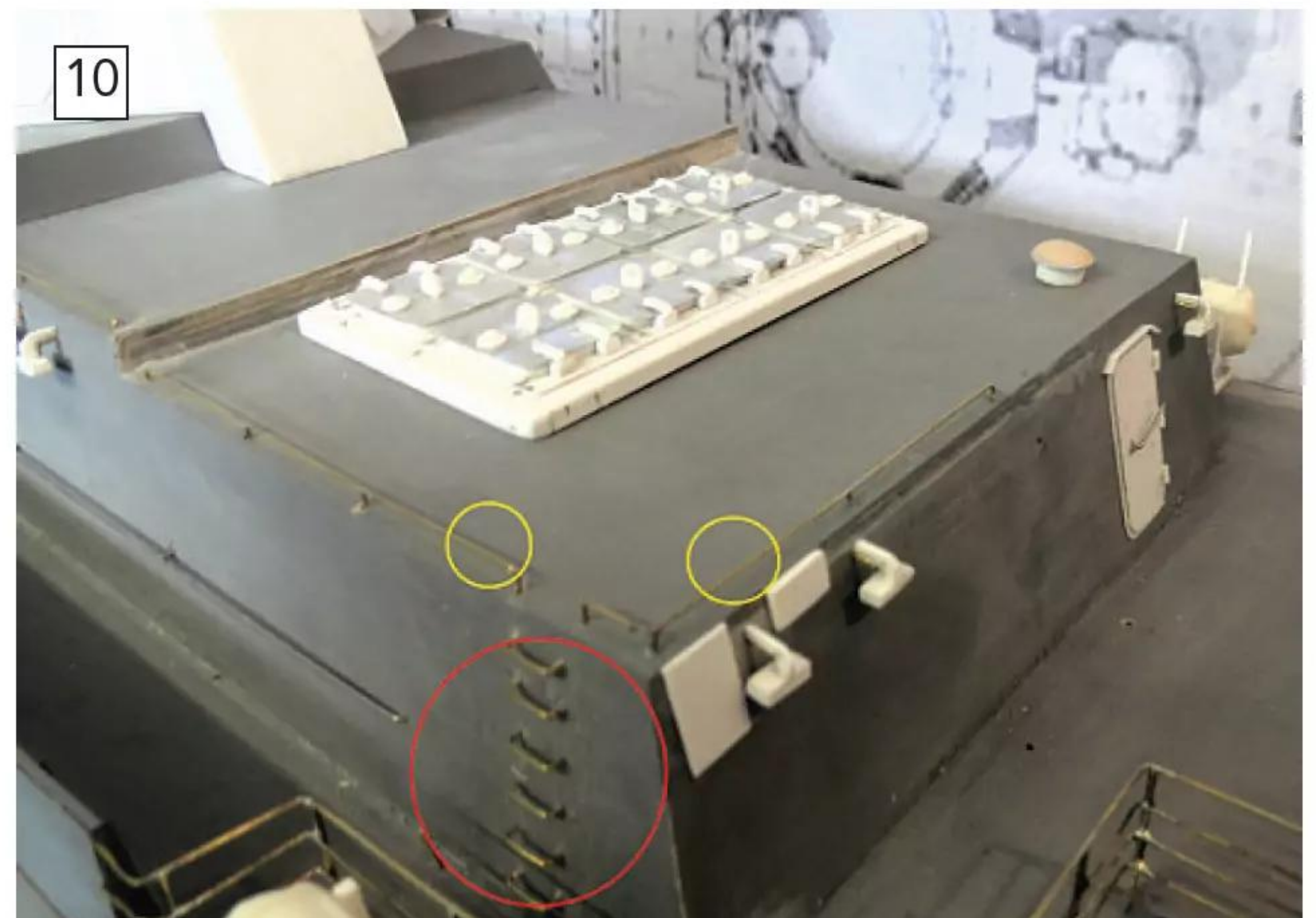
Rungs installed up the side of the VLS deck (ringed in red). To ensure consistency of depth on the deck safety rail while fixing into position, several gauges of the same thickness are placed between the wire and deck (marked in yellow).
