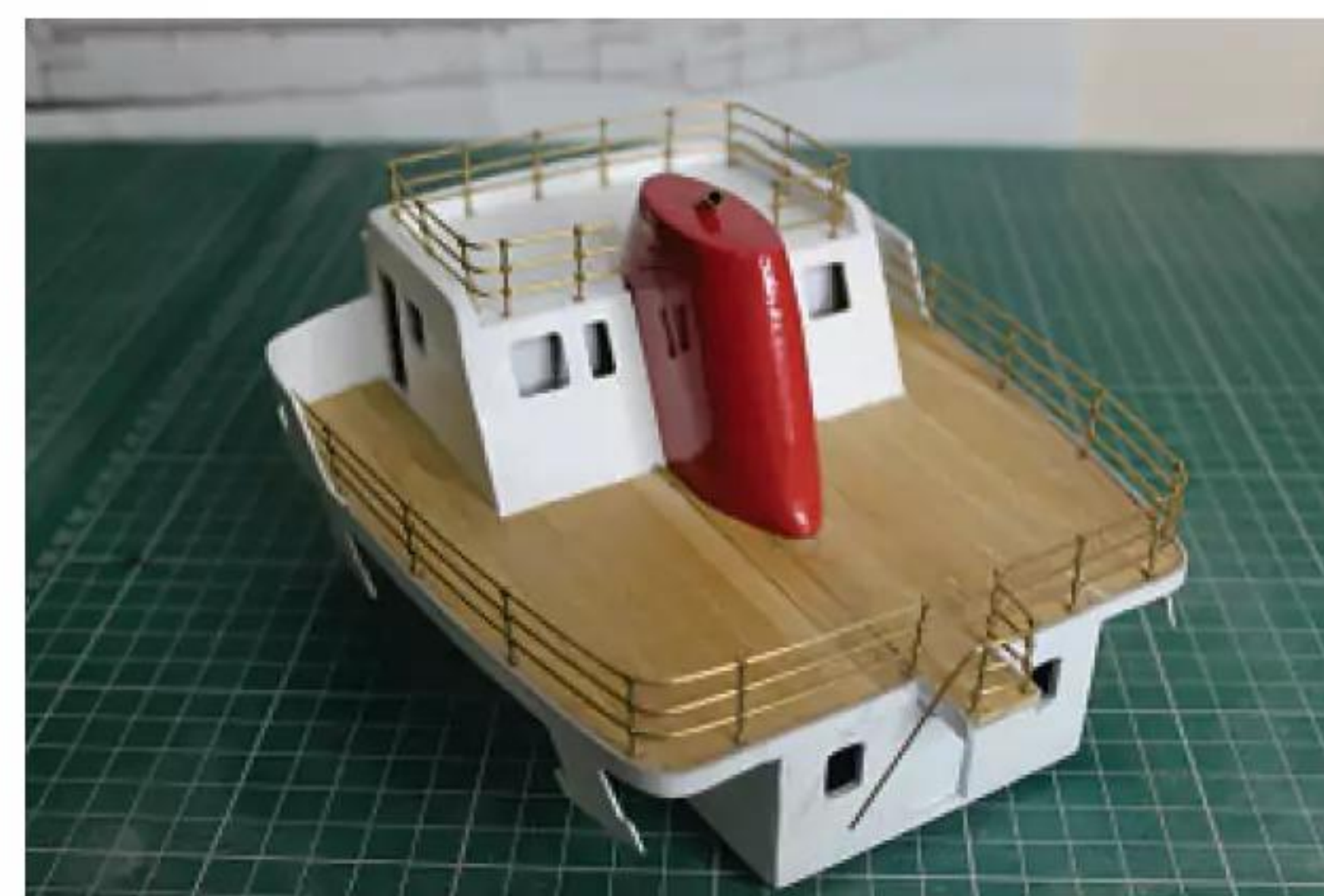
The basic structure of the bridge and funnel complete. Handrails are started to be fitted around the bridge wings and these add another layer of finesse.
