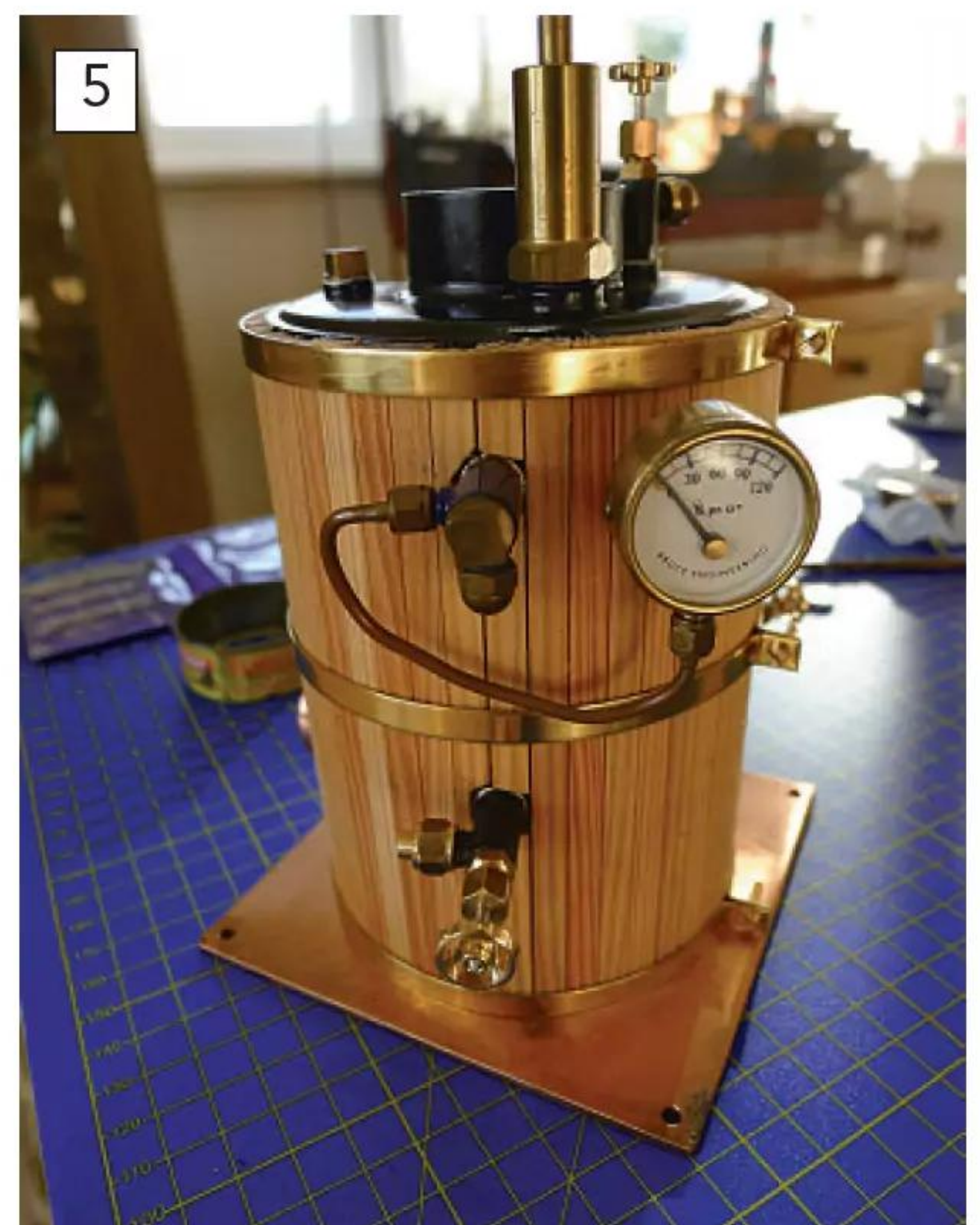
This Pendle boiler was clad with pine strip wood; a stash of which Richard keeps to hand for making frames and structures. With straight cuts around the fittings, this may not be the neatest of jobs, Richard concedes, but perfectly adequate for the job.
