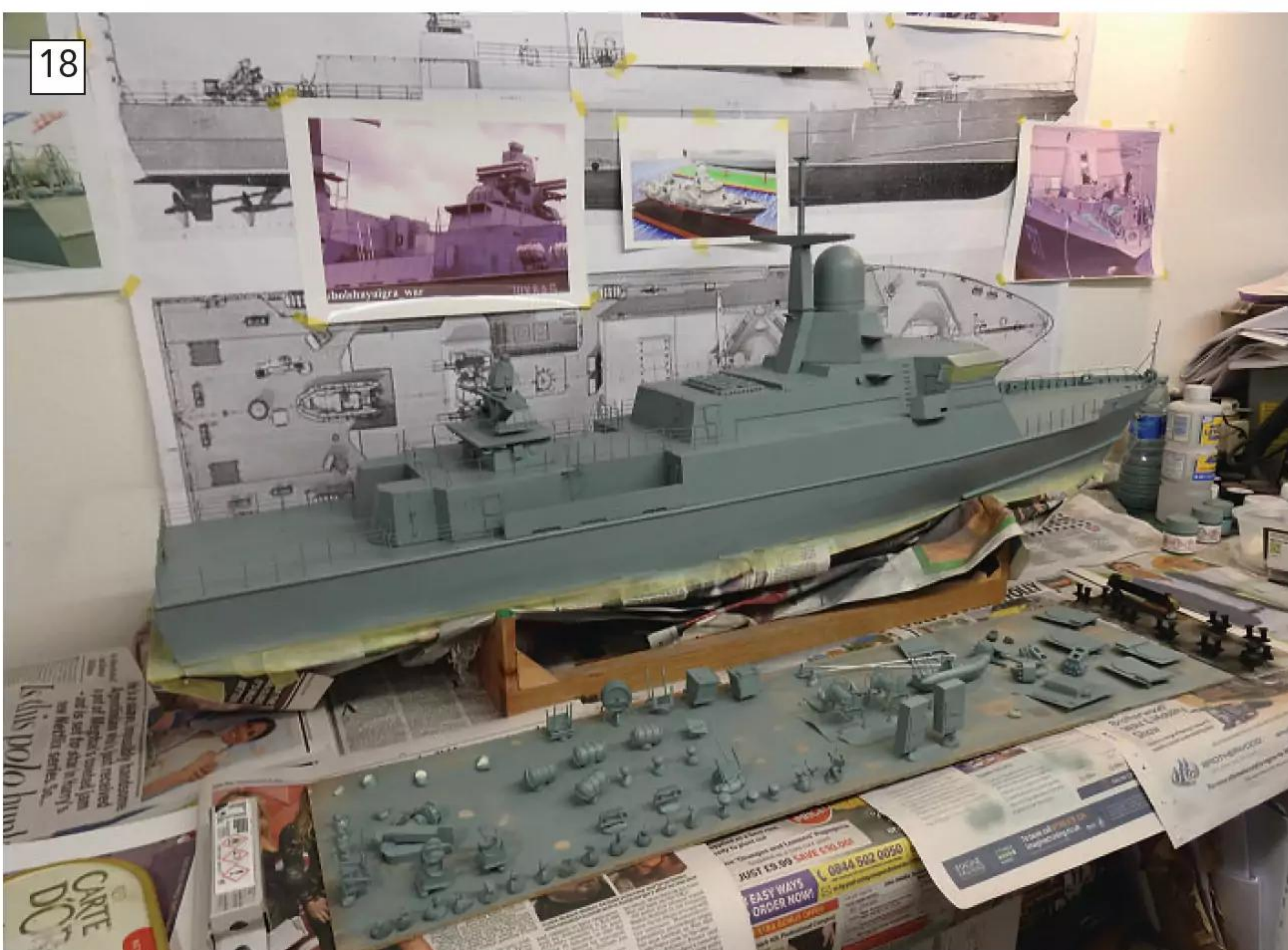
Applying the Mr Hobby 67 light grey basecoat to the superstructure, hull, and fittings.
