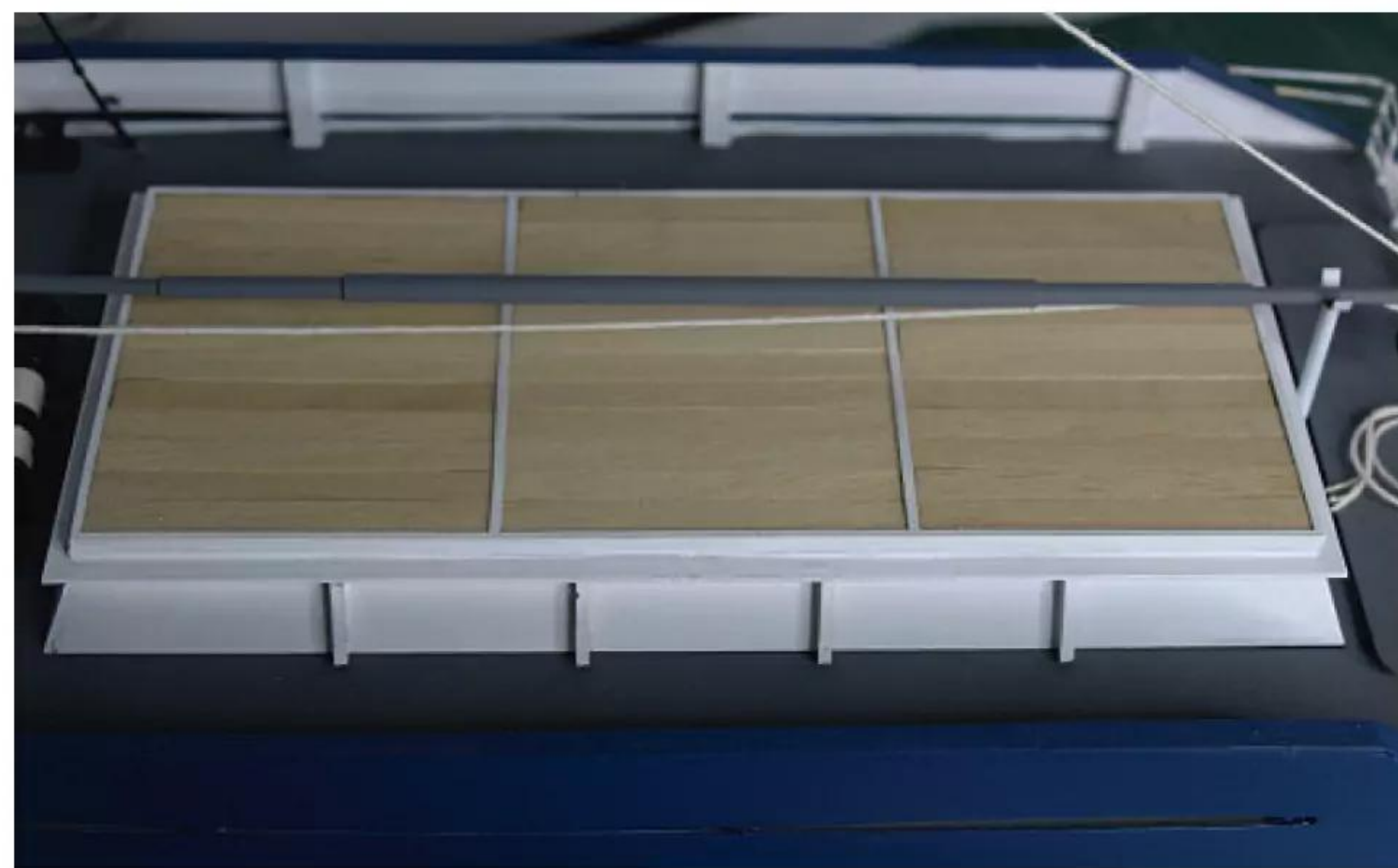
The cargo hatches, a key feature of this coaster freighter's design, are imaginatively created using laser-cut plywood to build up fantastically convincing replicas.
