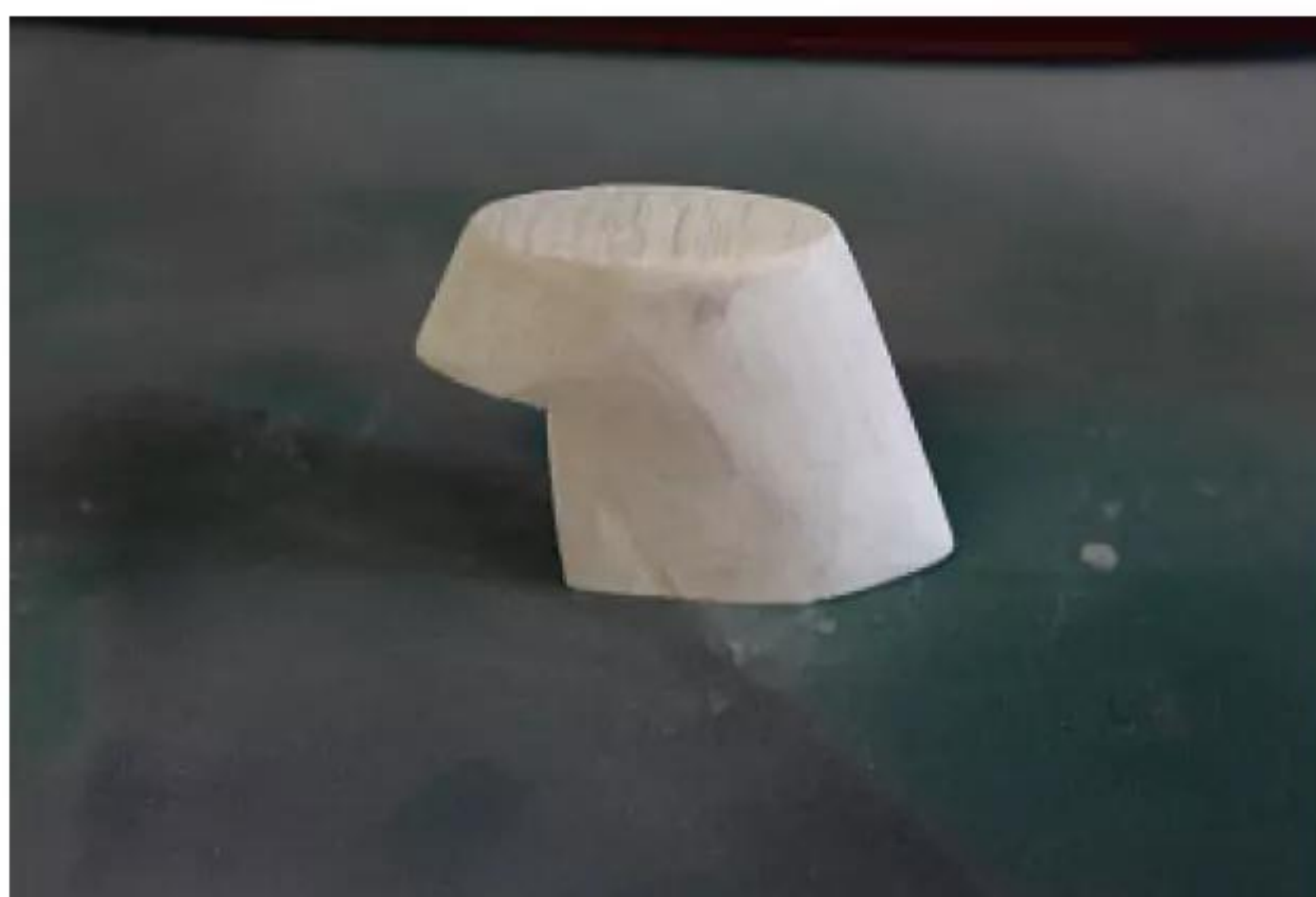
The funnel comes supplied as a balsa block that needs to be carved and filed to shape. There is a template in the manual to refer to, but Nick highly recommends using the plans as additional guidance.
