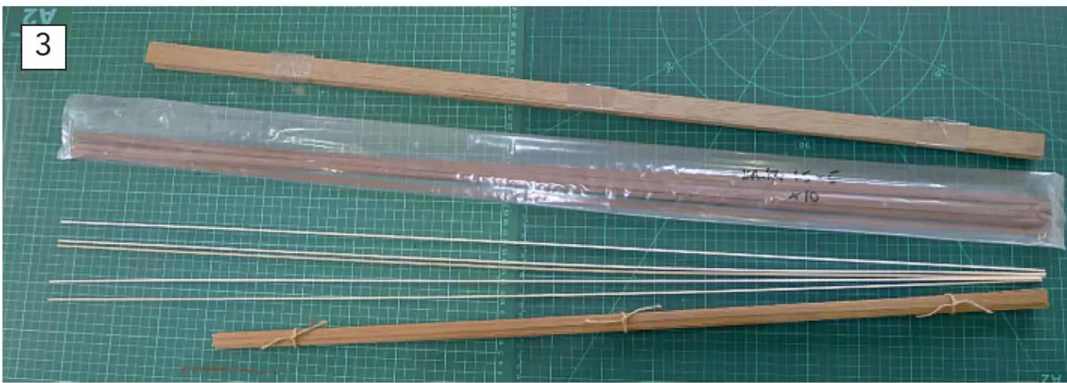
For cladding, any old wood will do, from purchased planking to simple modelling strip wood lengths. You will, however, probably want to take into account the overall appearance of the boiler once it's finished and how you want the complete model to look.
