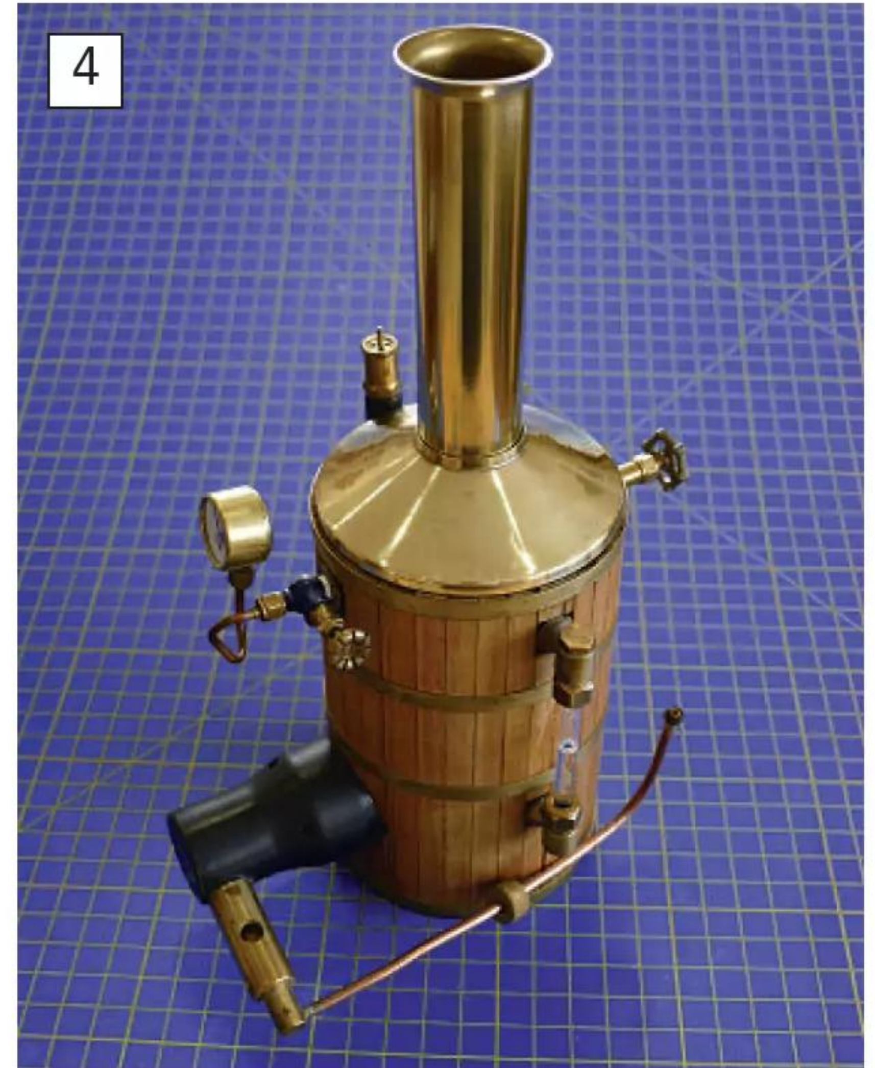
This Miniature Steam Models Clyde Boiler was clad with the kit supplied planking. The wood hasn't been treated at this point and could be varnished or waxed to bring out the darker colour.
