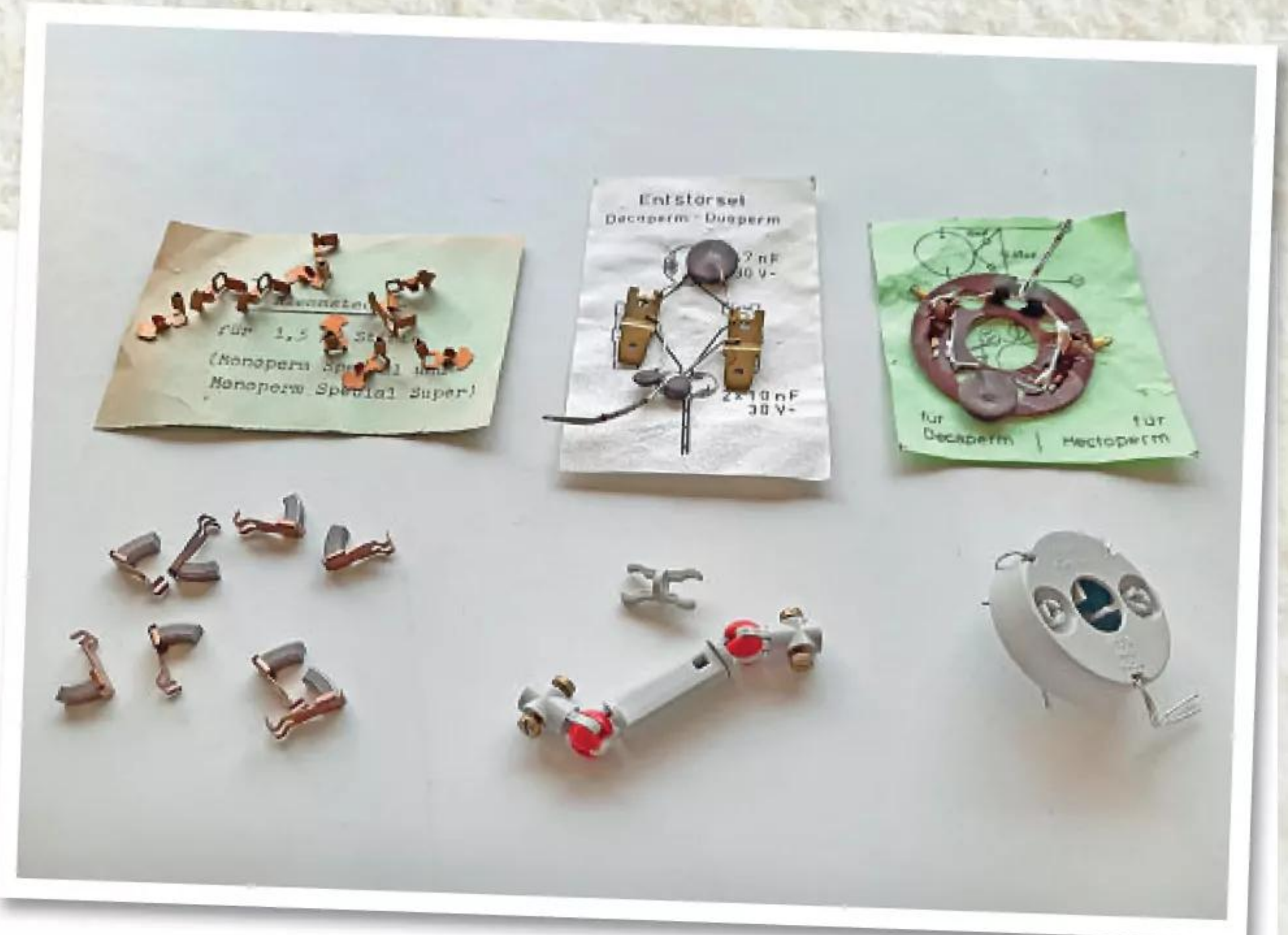
The range of Marx spares and accessories included brushes, a Cardan drive shaft, suppression gear and terminals.
