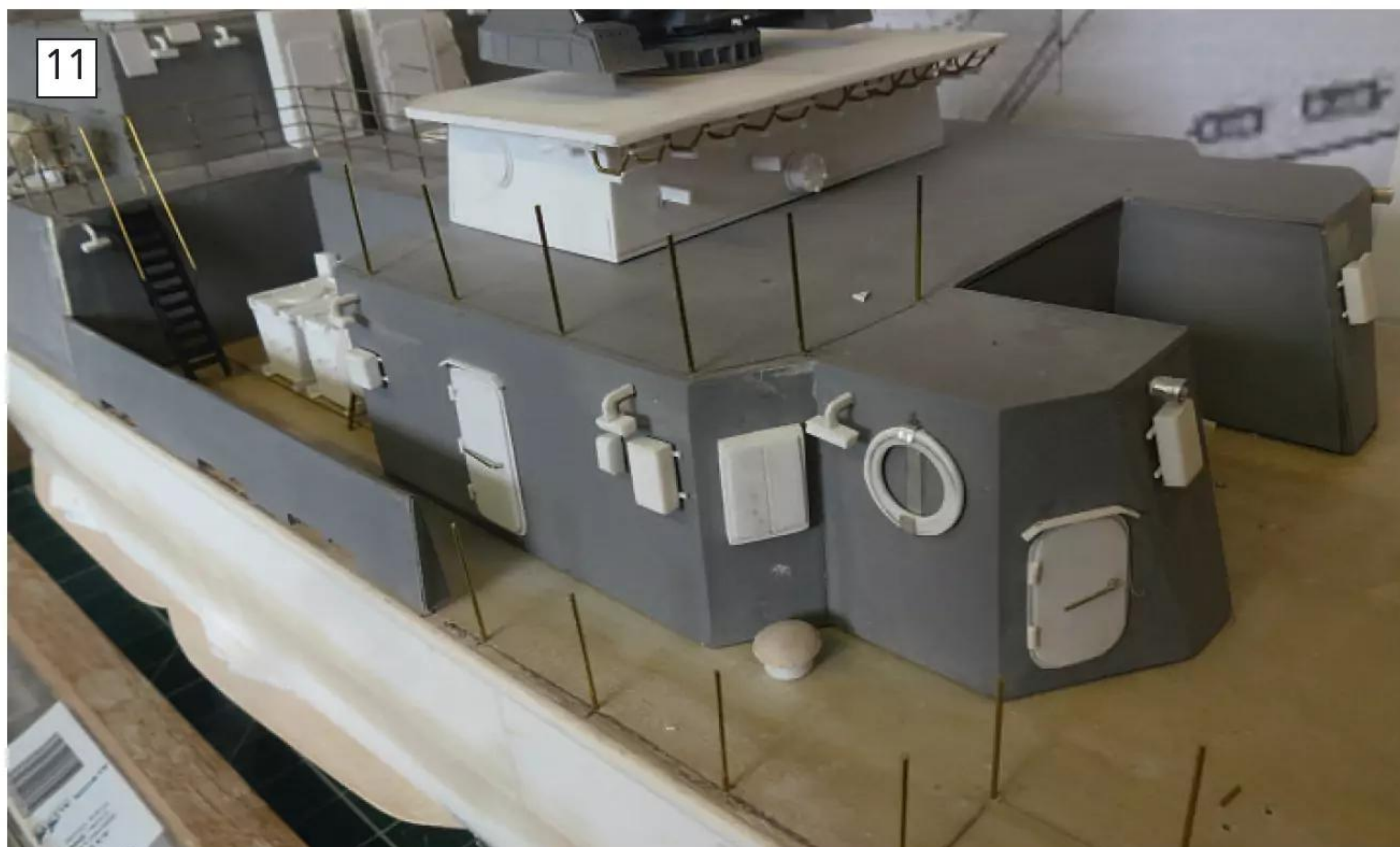
Stanchions of .8mm cut to size and located to the deck in preparation for being transferred to a jig for assembly of the four bars, each .4mm thickness.
