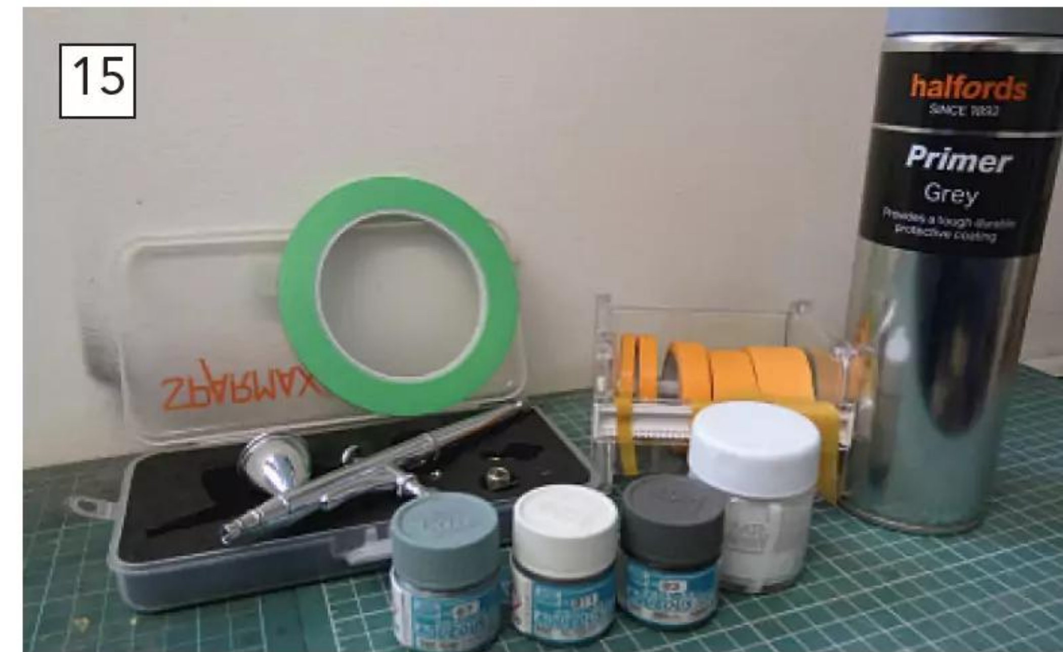
Some of the material used for creating the camouflage shapes. Dave found the tape dispenser particularly useful. The green coloured tape was not required here but is perfect for masking curves.
