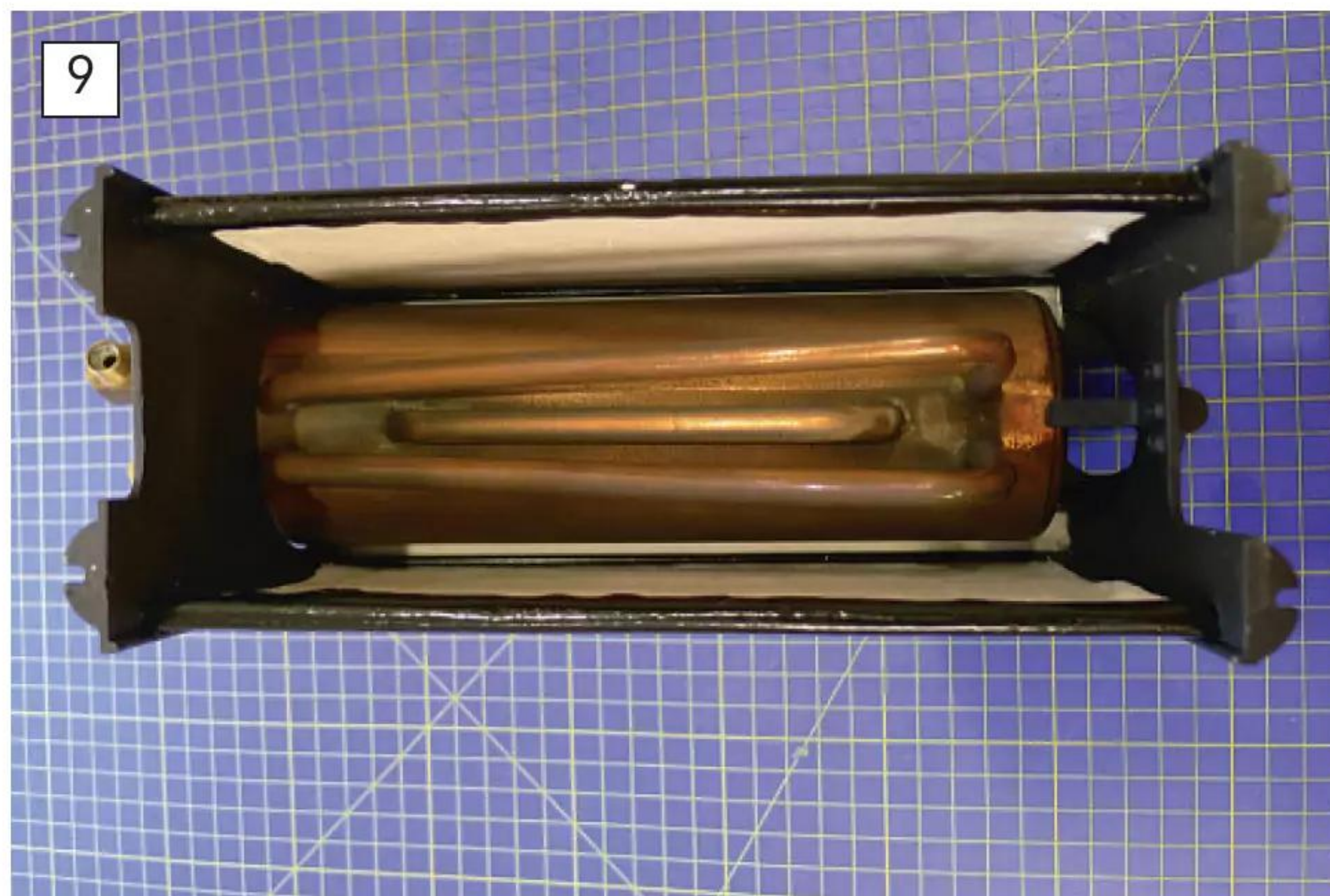
This Stuart Turner Type 500 boiler was stripped down for a complete restoration, during which the original casing lining was replaced with ceramic heat insulating cloth, this being simply glued in place with heat resistant adhesive.
