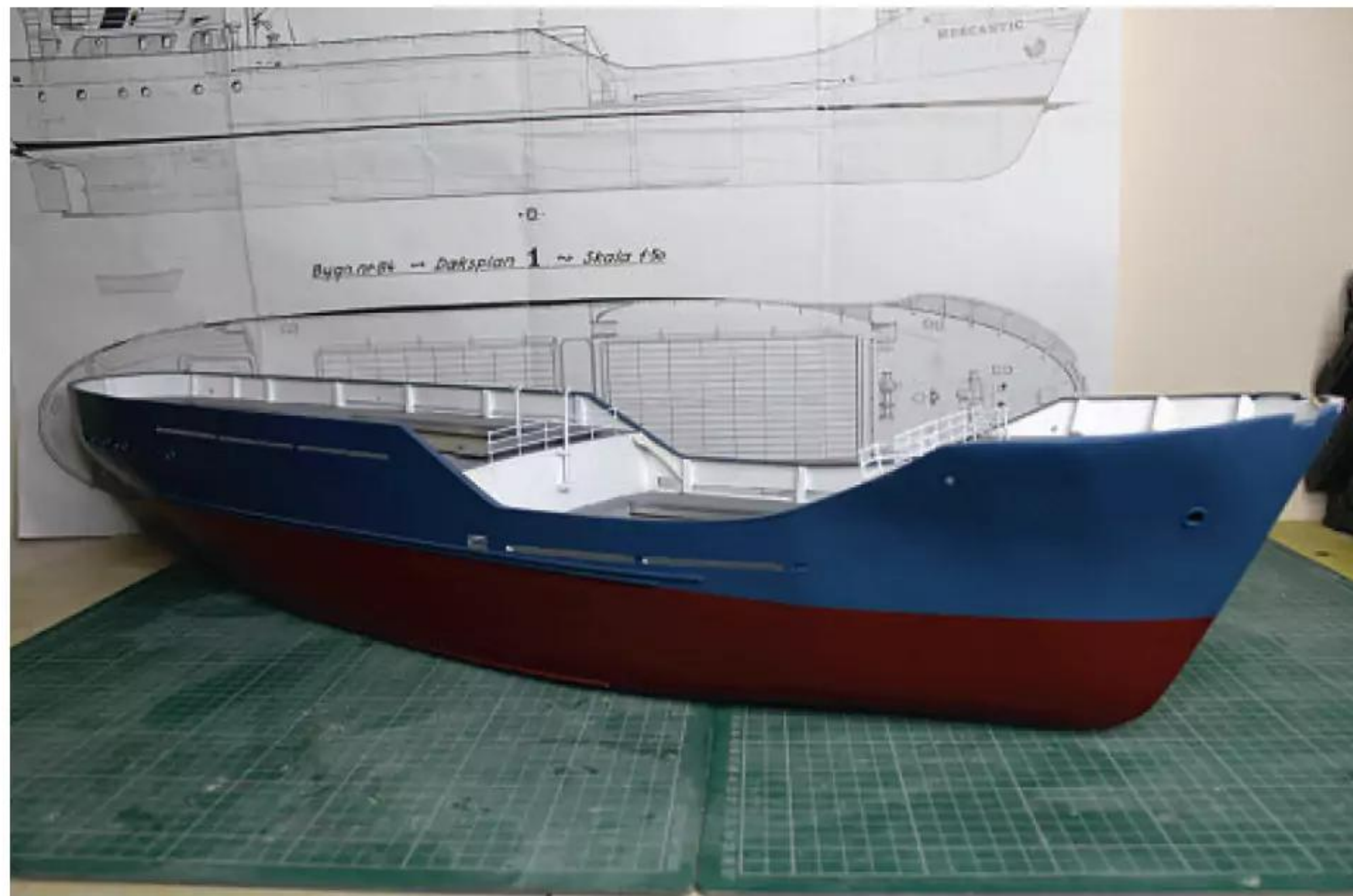
Success! Nick's second application of 'Mediterranean blue', courtesy of a Halford's rattle can. Unfortunately, his first 'finish' proved unexpectedly disastrous due to a nasty reaction between his original choice of paint and primer.
