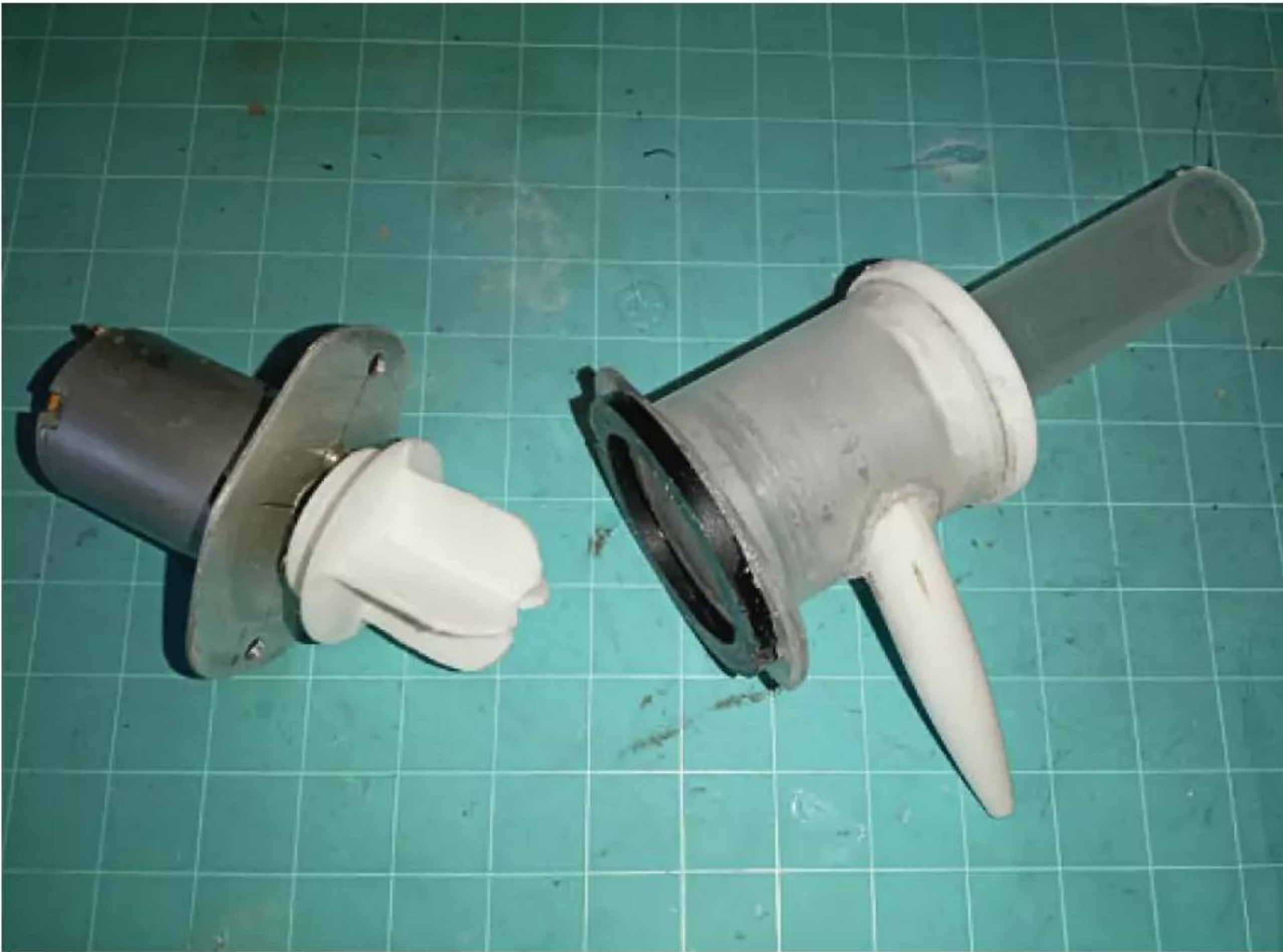
The pump before assembly showing the impeller, made from the syringe plunger.
