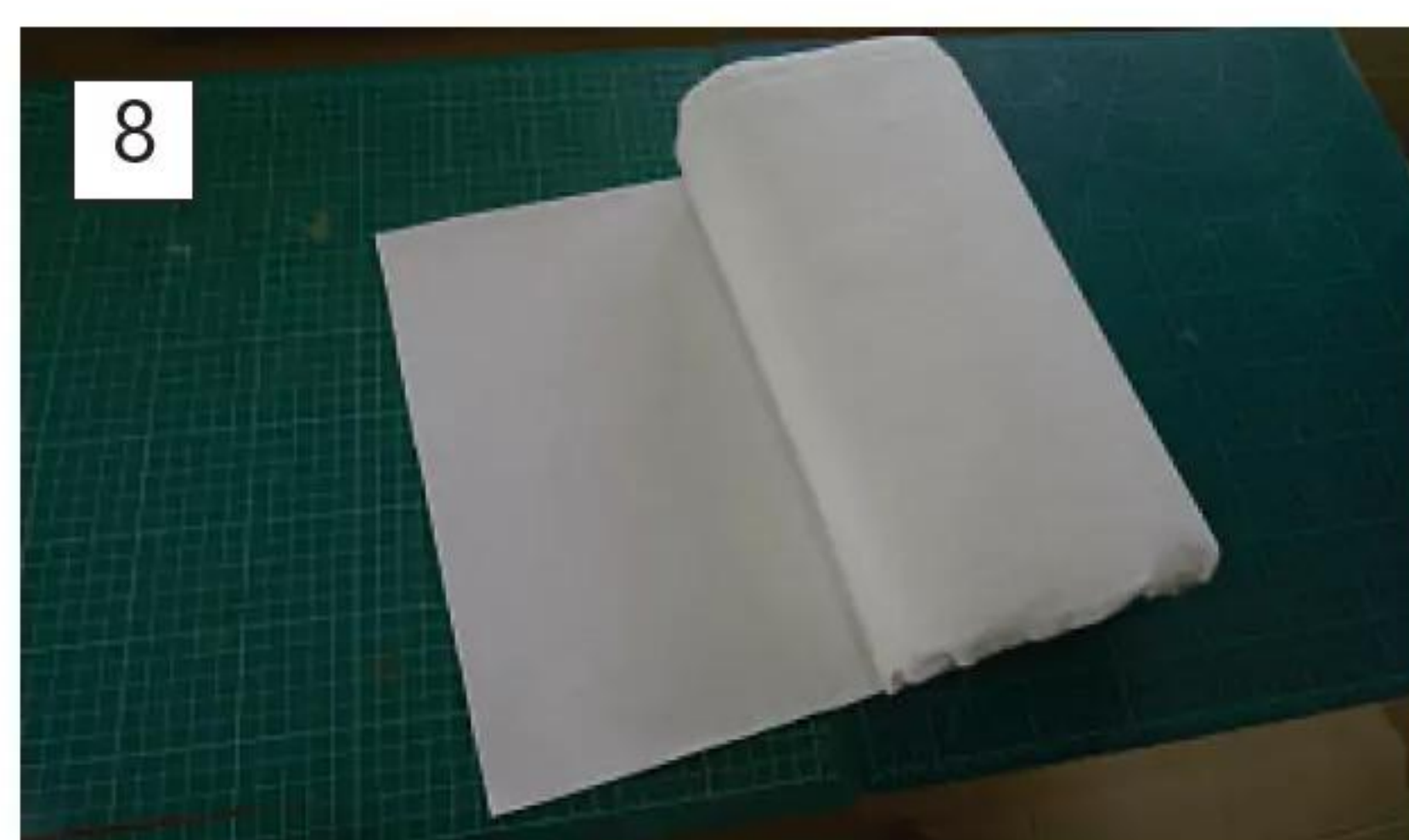
Ceramic cloth and paper are both readily available in a range of thicknesses. Used on their own, the guide of 1mm of insulation for every 1-inch of boiler diameter works well, but a thinner layer beneath a wood cladding is also the Rolls Royce of insulation jobs.
