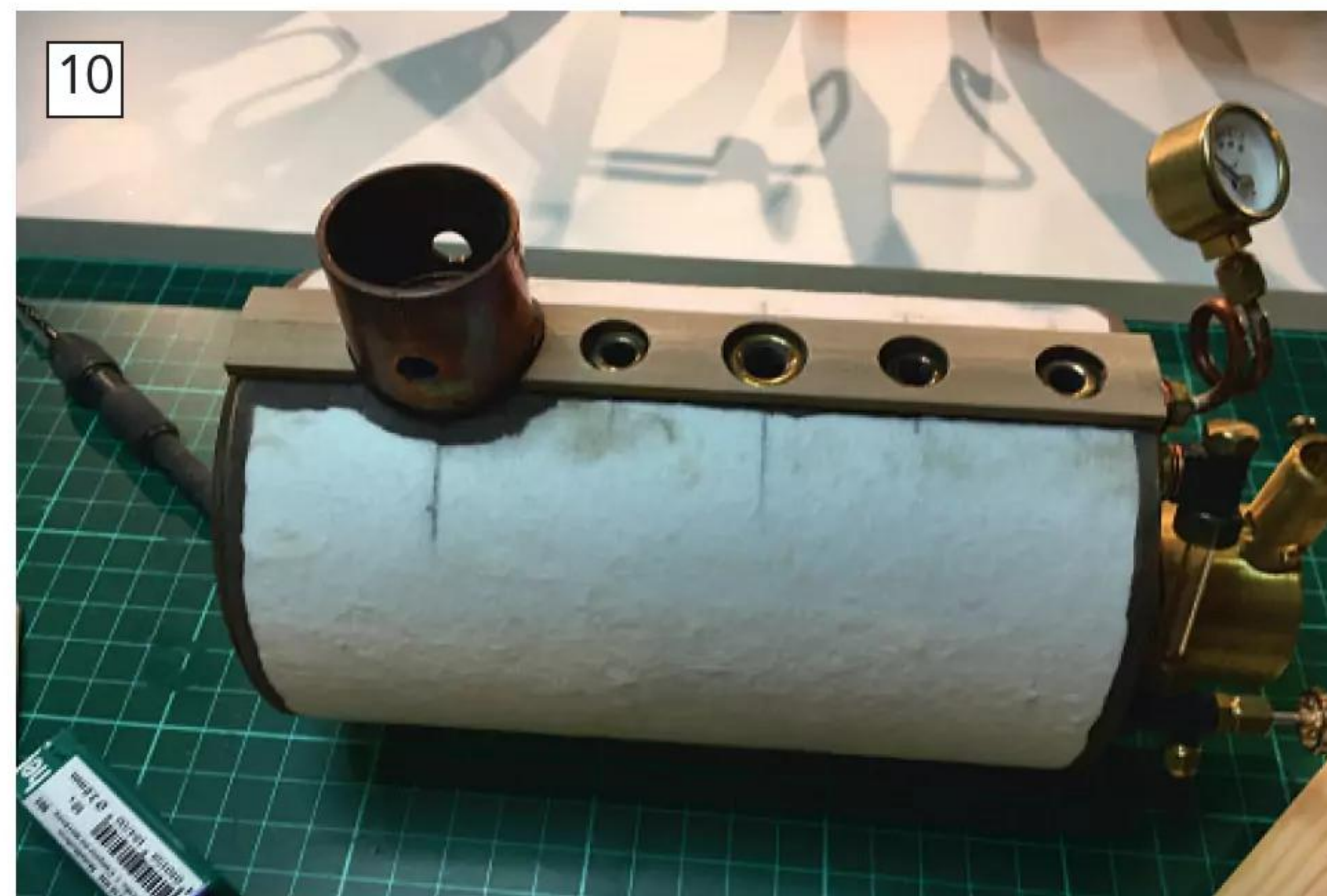
Again, the same boiler from Mark Tommy shows how ceramic paper glued to the boiler underneath the wooden staves gives not only a beautiful finish but also a very effective insulation system.
