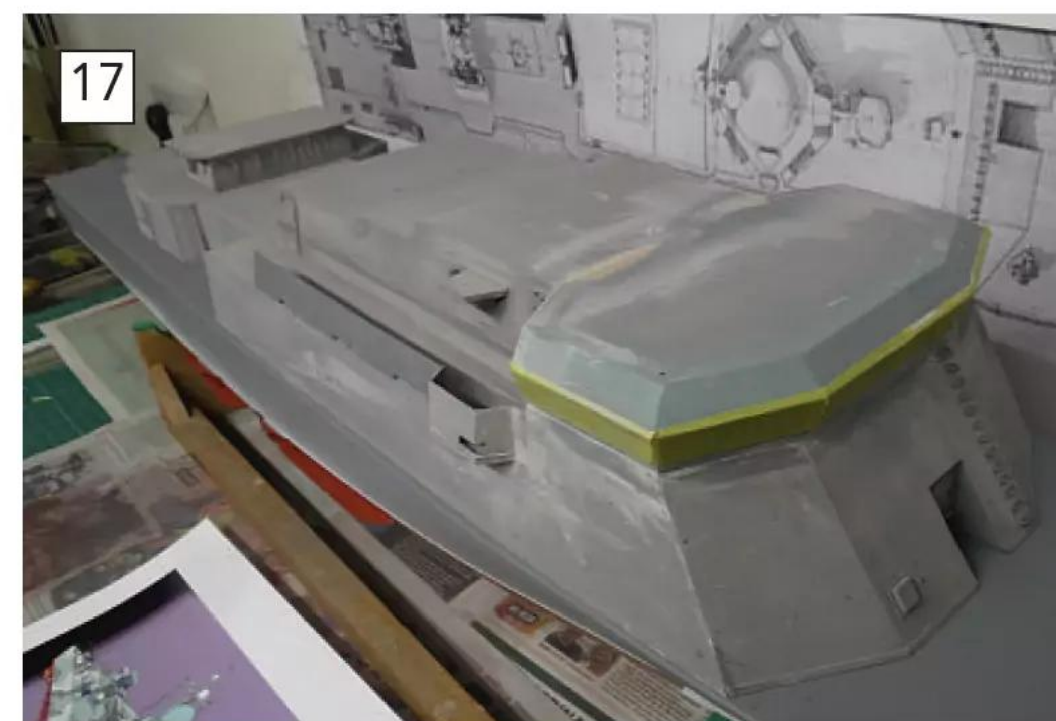
With the glazed bridge windows masked, the superstructure is also now prepared for its second coat of Halfords' grey primer.
