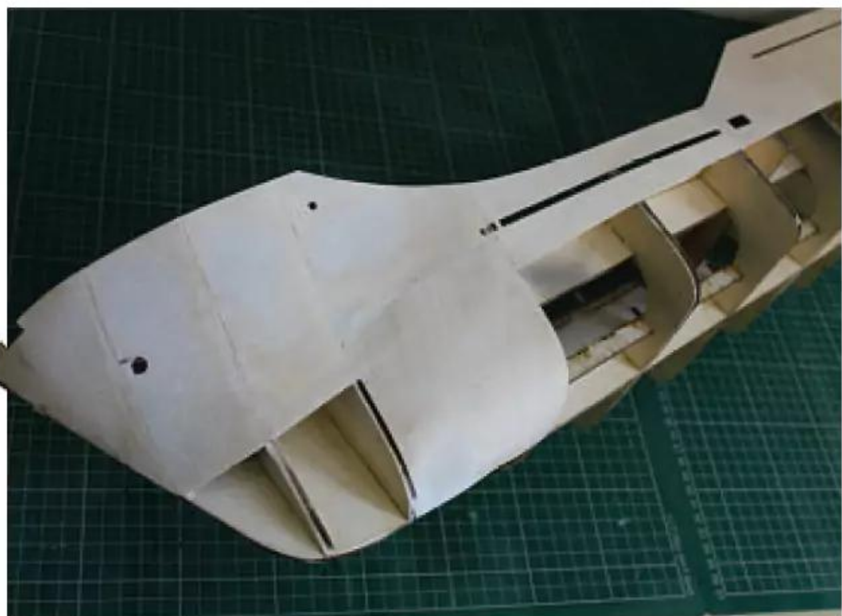
The forward hull plating requires virtually no modification to fit and incorporates the scuppers and anchor holes.
