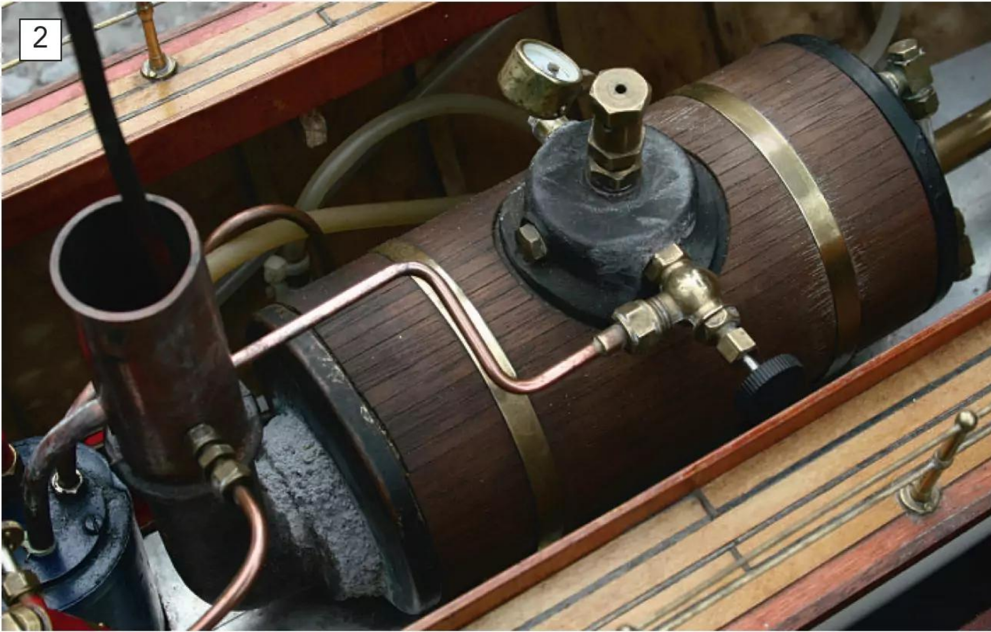
If insulation doesn't need to be removed for hydraulic testing, a neat approach is to use fire cement. Some old boilers use this system all over the shell, held in place with plating or wood cladding.
