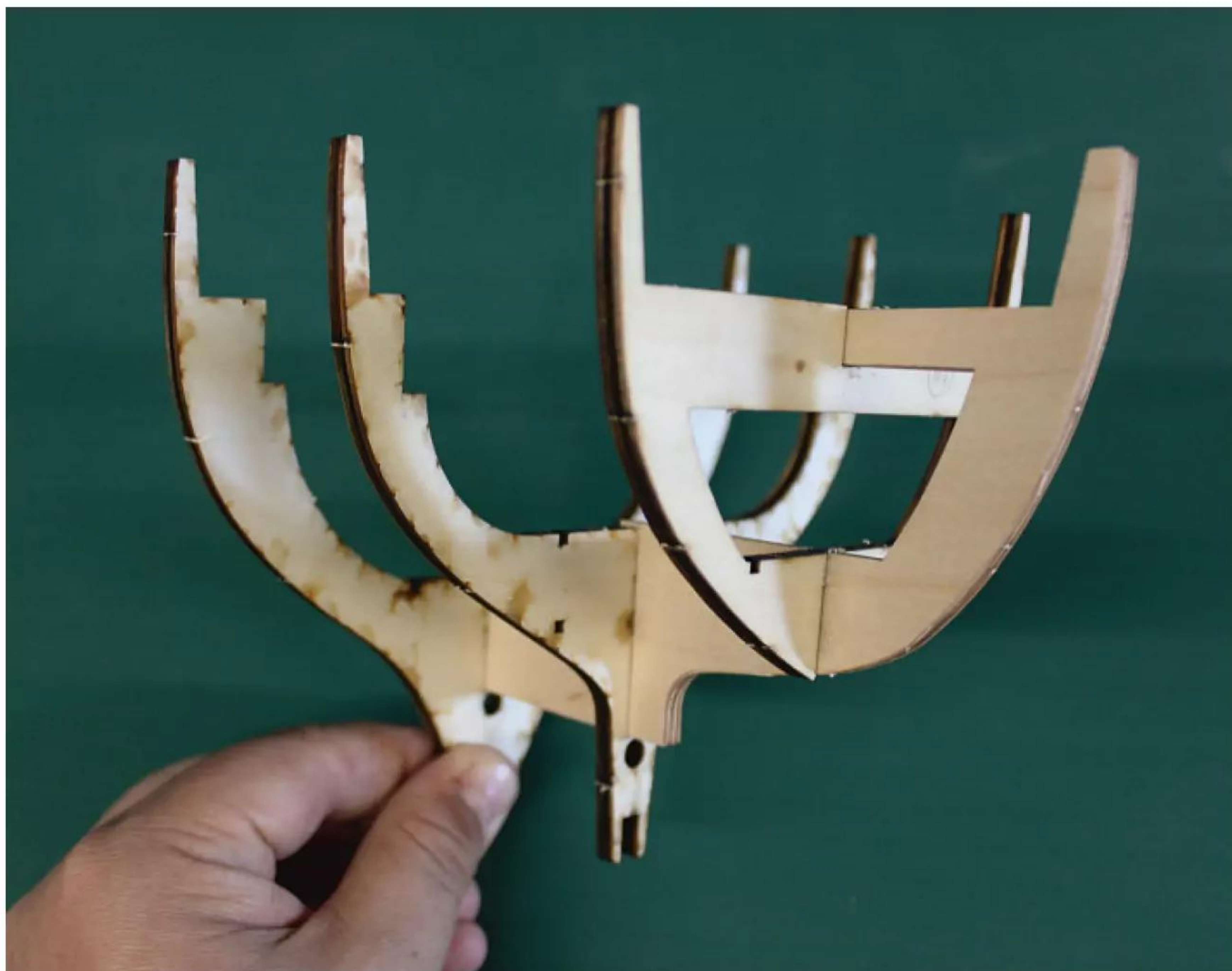
Assembly of the stern section requires a little more patience and care to be taken; the end result, however, serves as a good, strong support structure for the hull plates.
