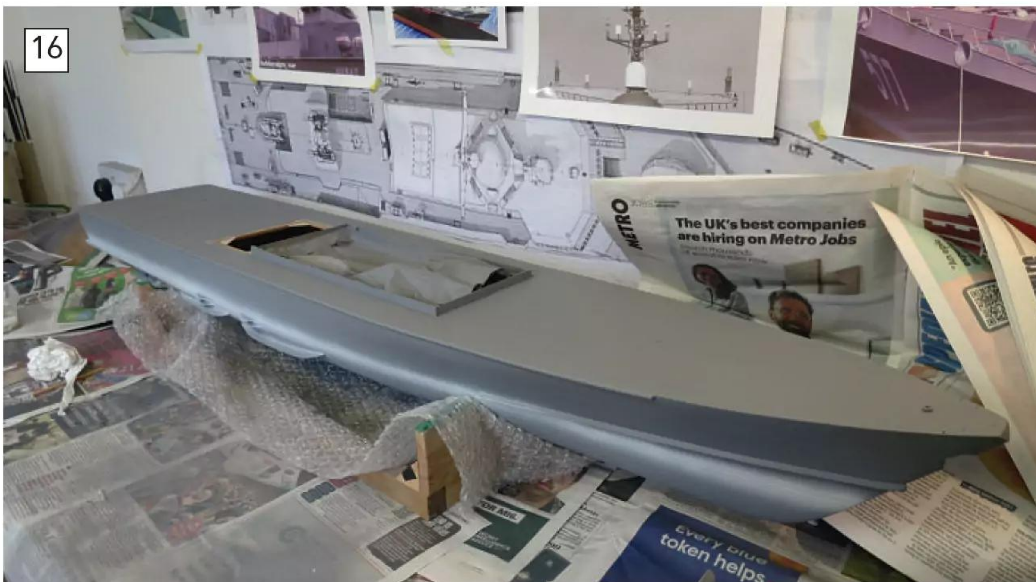
The hull and deck with the second of two coatings of Halfords acrylic grey primer applied.
