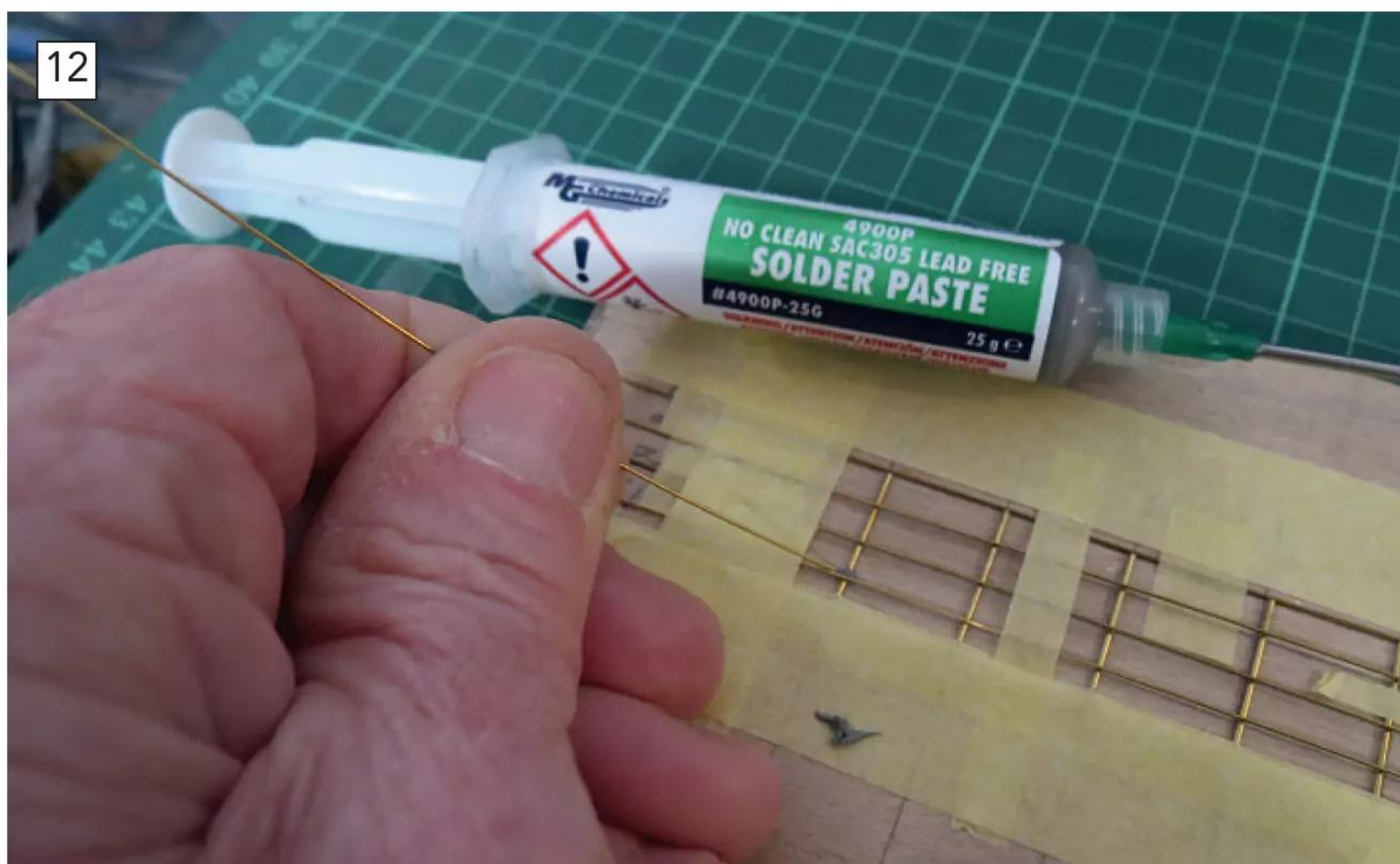
The use of a jig and solder paste to form the four bar rails.
