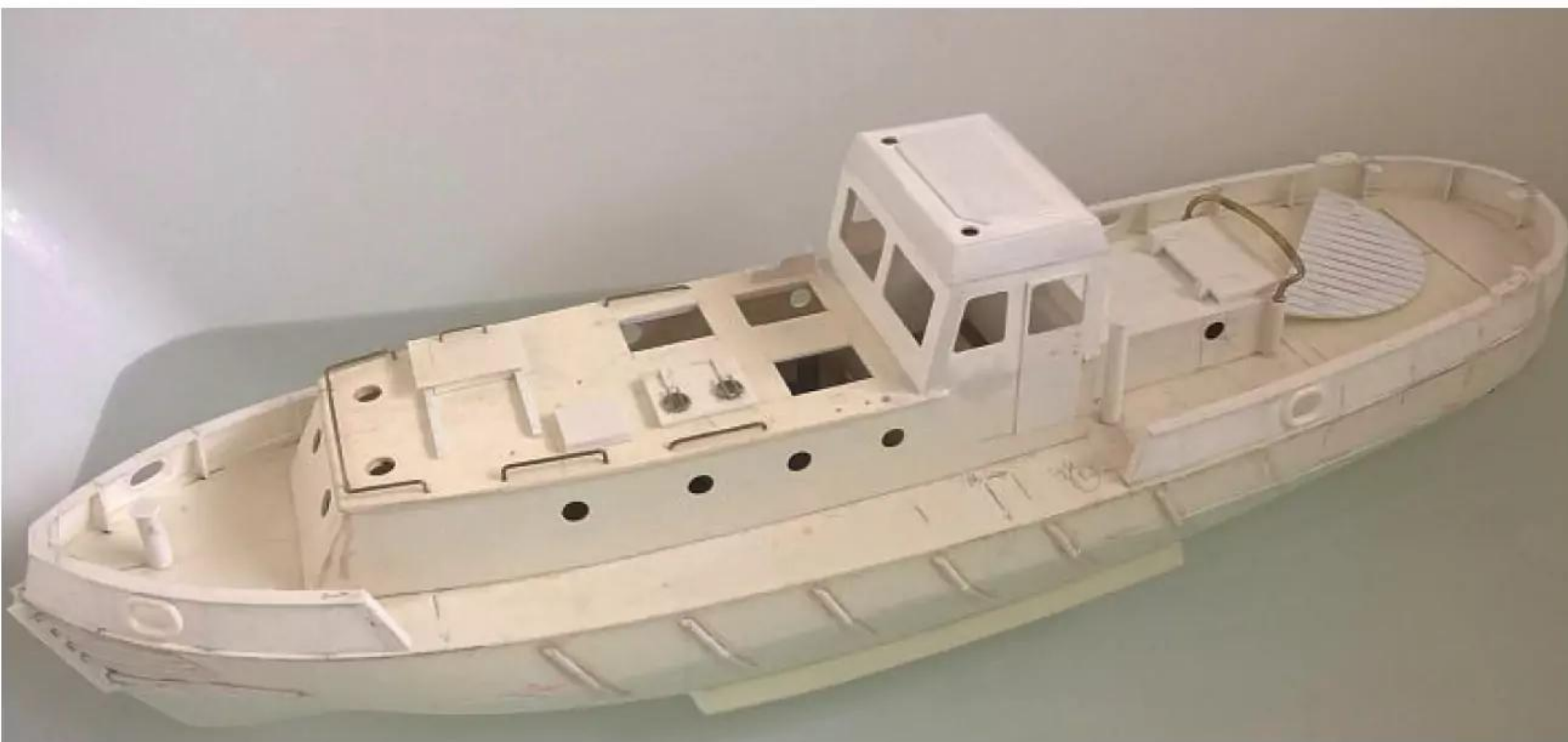
Working to Dave Metcalf's plans for the Thames tugboat Plaudit, David Marks added his own scratch-built superstructure to a vacuum formed styrene hull he purchased from Sarik Hobbies.
