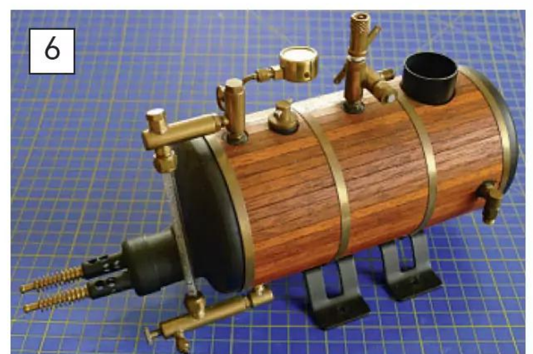
An old John Hemmens Caton boiler factory insulated with beautifully fitted mahogany planking. The circular holes cut around the fittings and the banding, hiding the ends of the planks, makes this as good an example of cladding as you are likely to see from any manufacturer.
