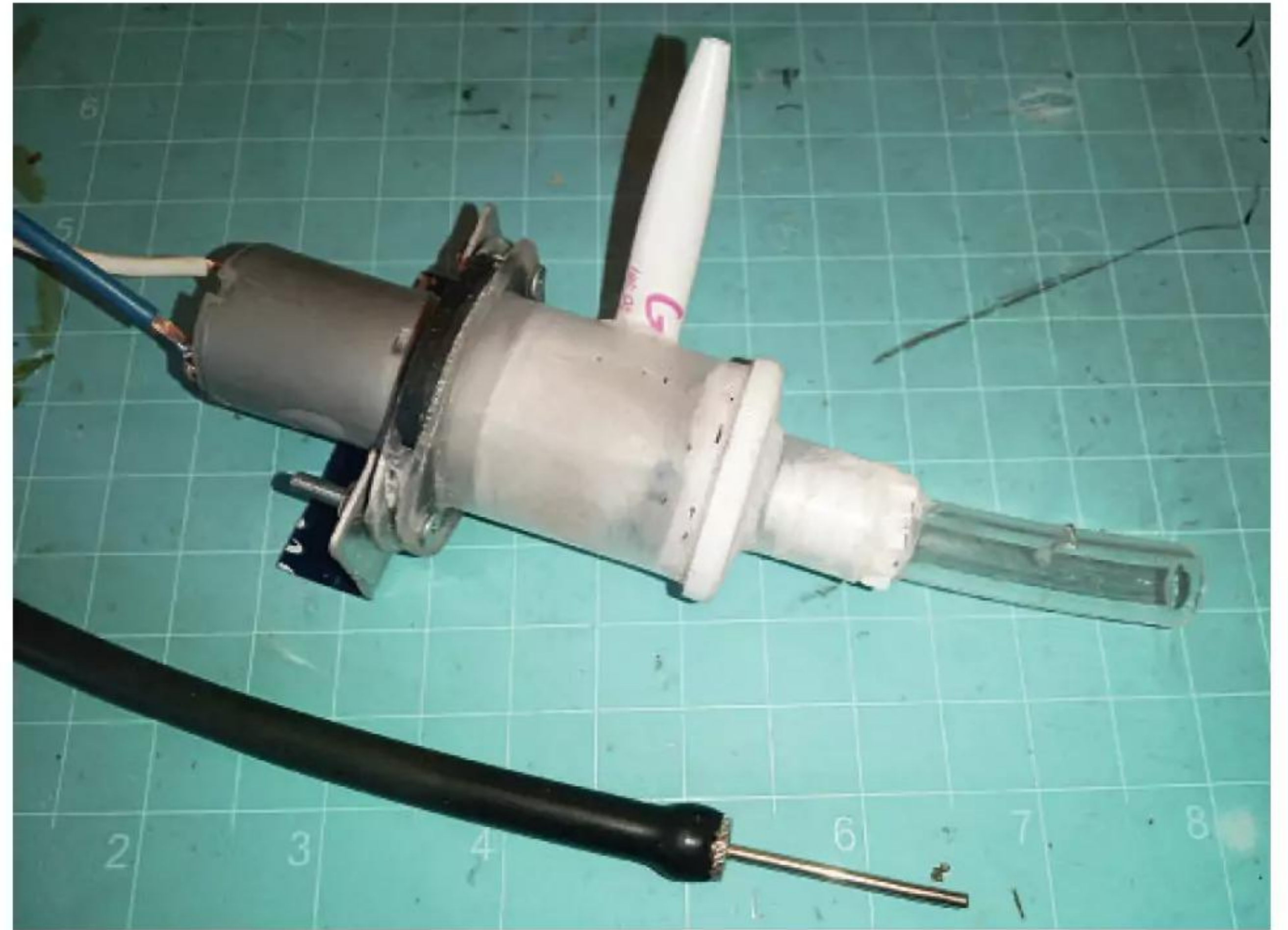
The assembled pump alongside the proposed hose & nozzle.
