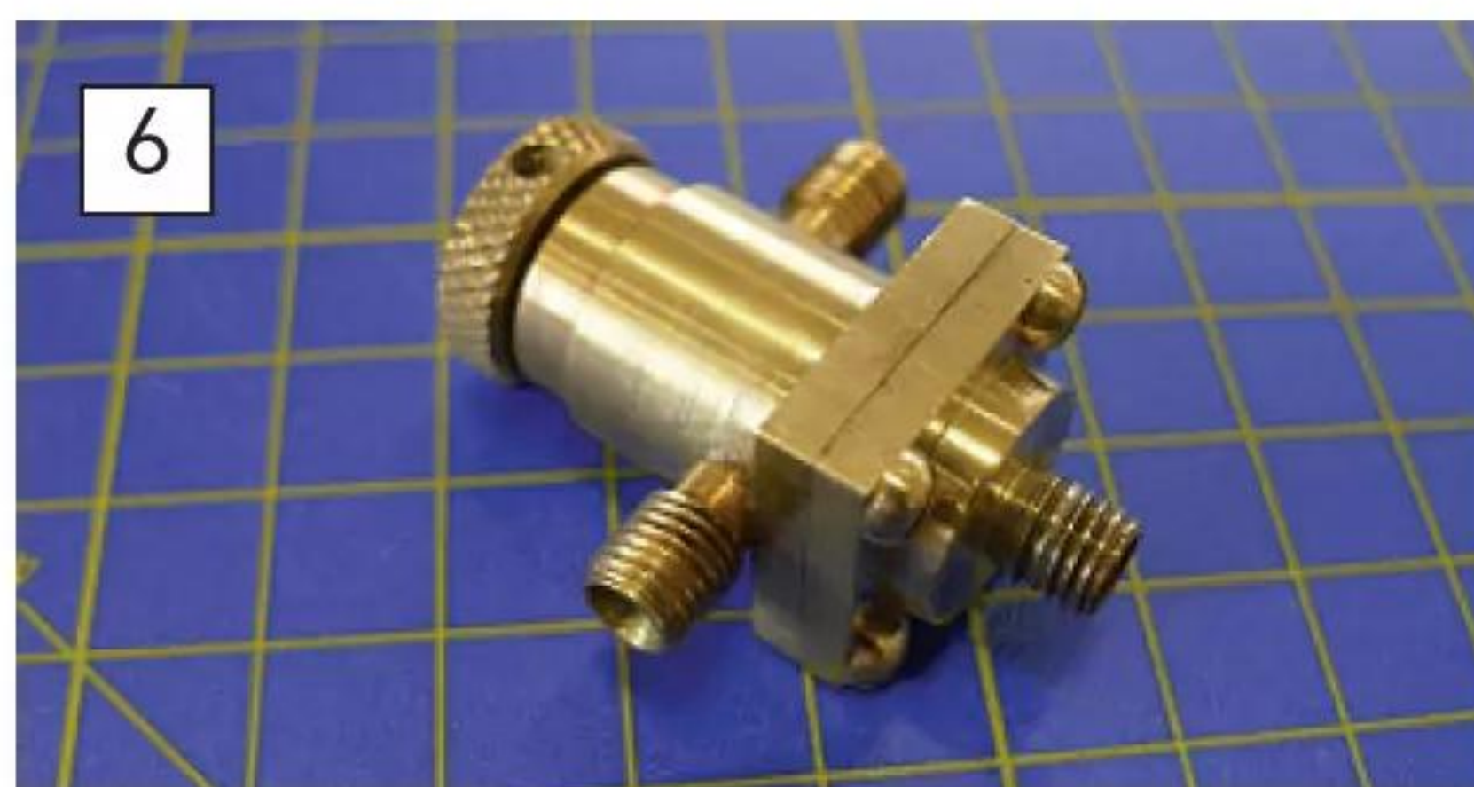
A mechanical attenuator valve can greatly extend the duration of your gas, as it averts the need to keep going at full speed to prevent the safety valve lifting. Bear in mind you don't fall foul of the requirement that the gas must be consumed before the available feed water in certain models.
