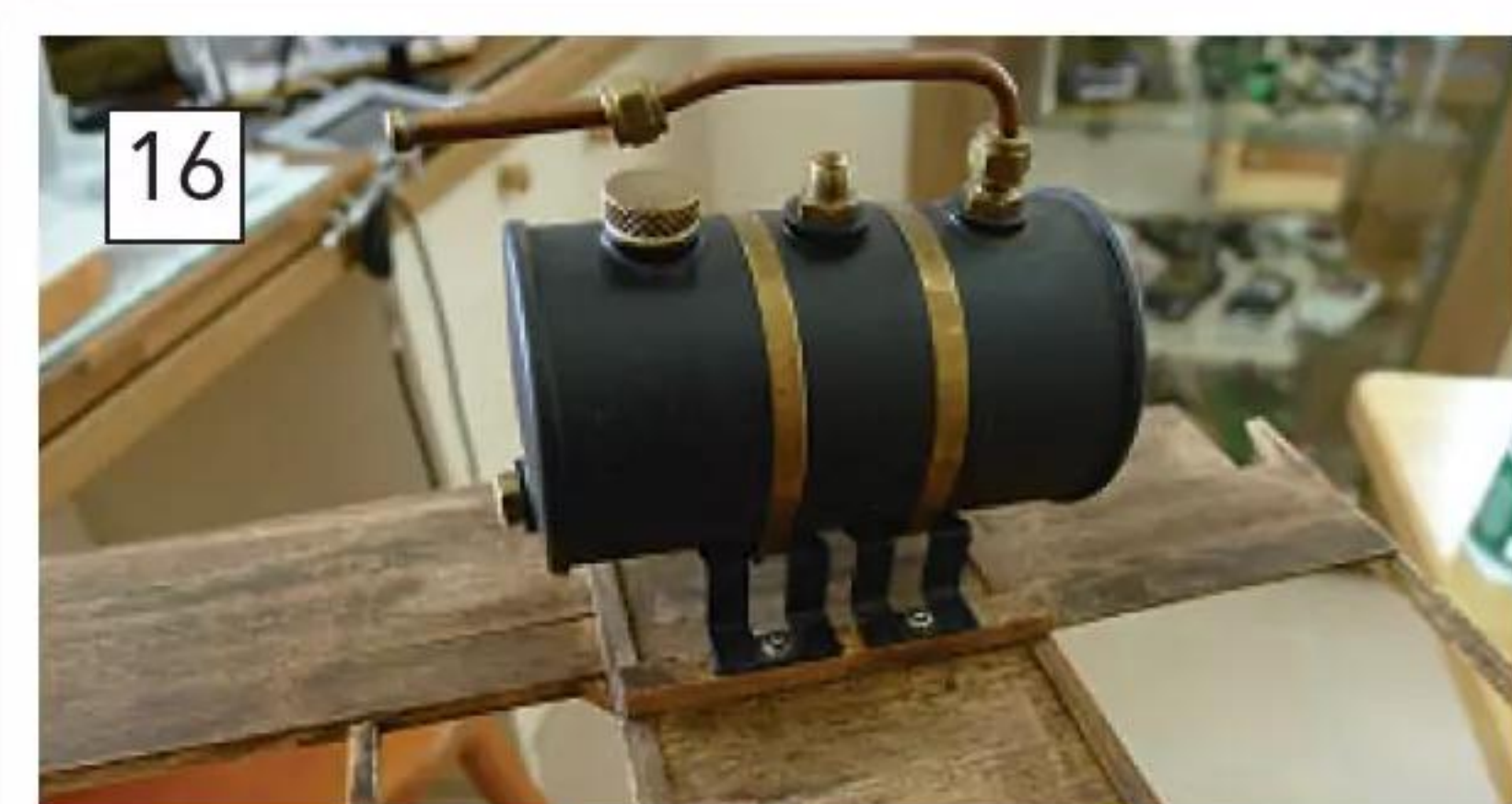
Using a syringe with a suitably large nozzle fitted also makes the separator tank quick and easy to attend to.
