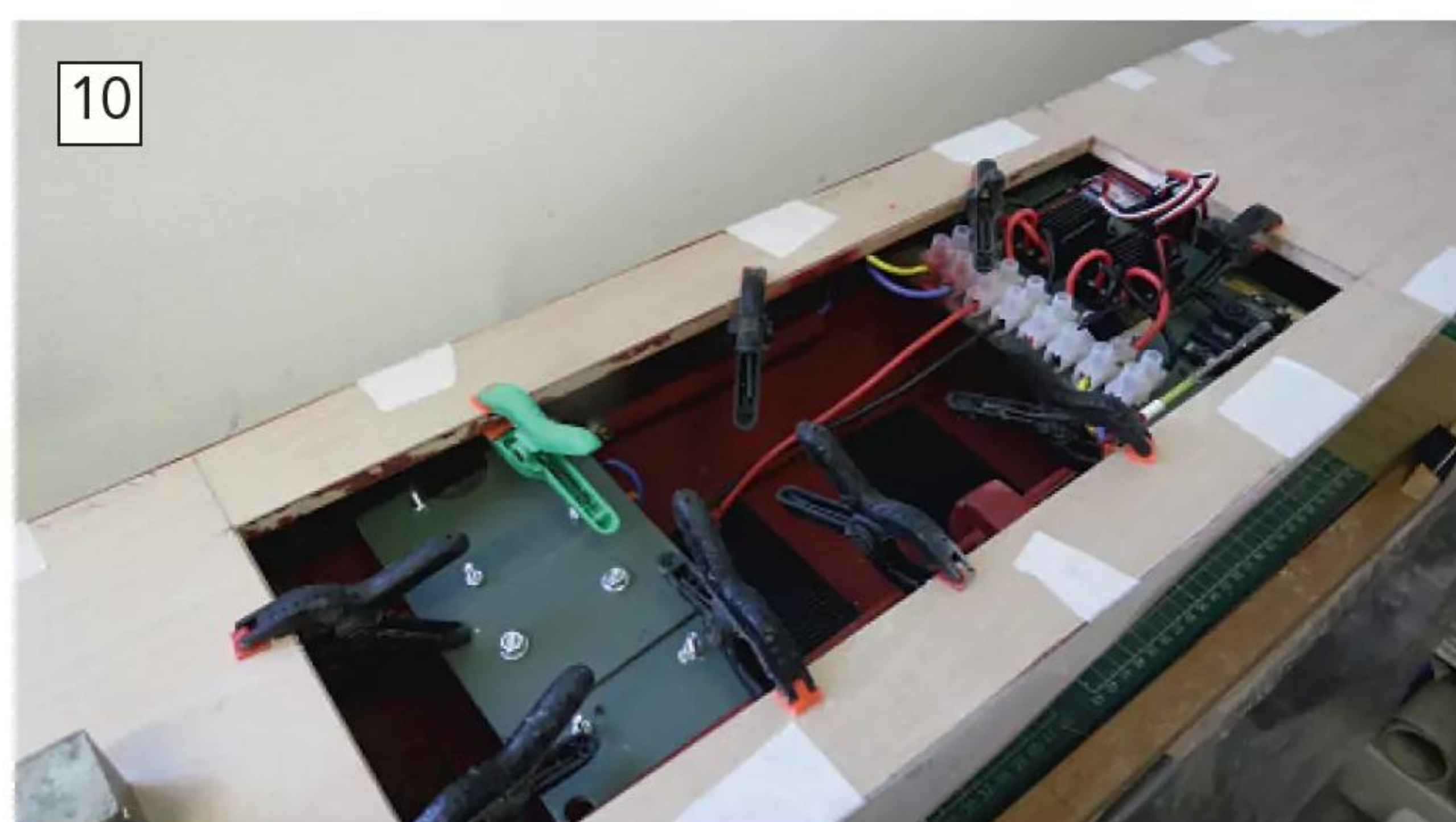
Having applied waterproof PVA, the inner edges to the openings are held firmly in place with plastic clips.
