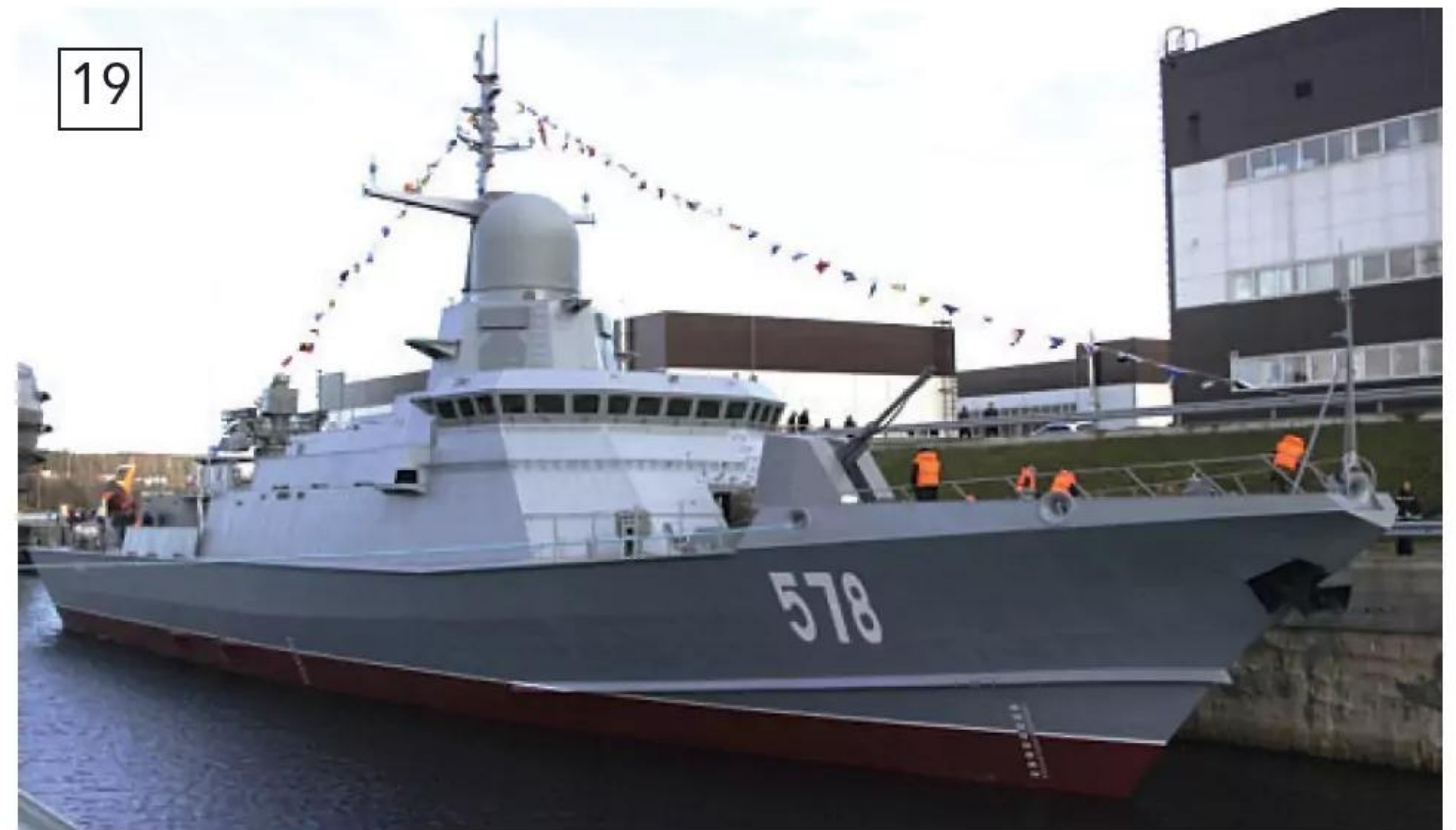
Each of the octagonal facets of the radar tower slope inwards, as evidenced by this image of the full-size vessel.
