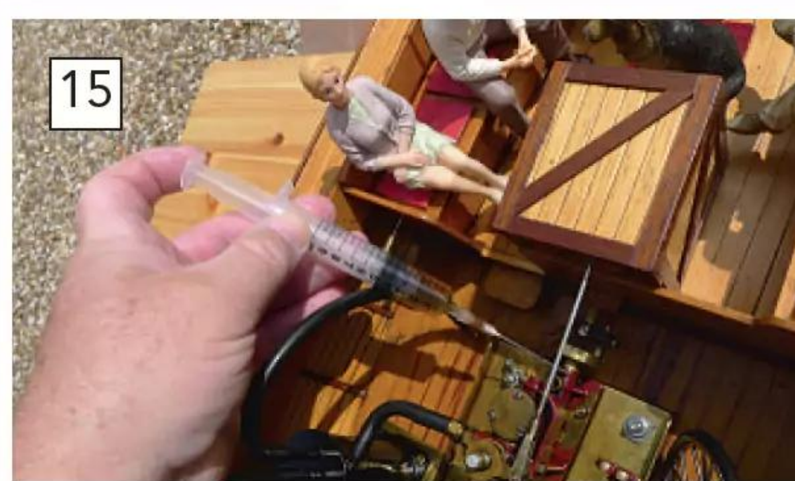
Again, a syringe with a fine tube fitted makes oiling the engine quick and easy, as well as minimizing mess.
