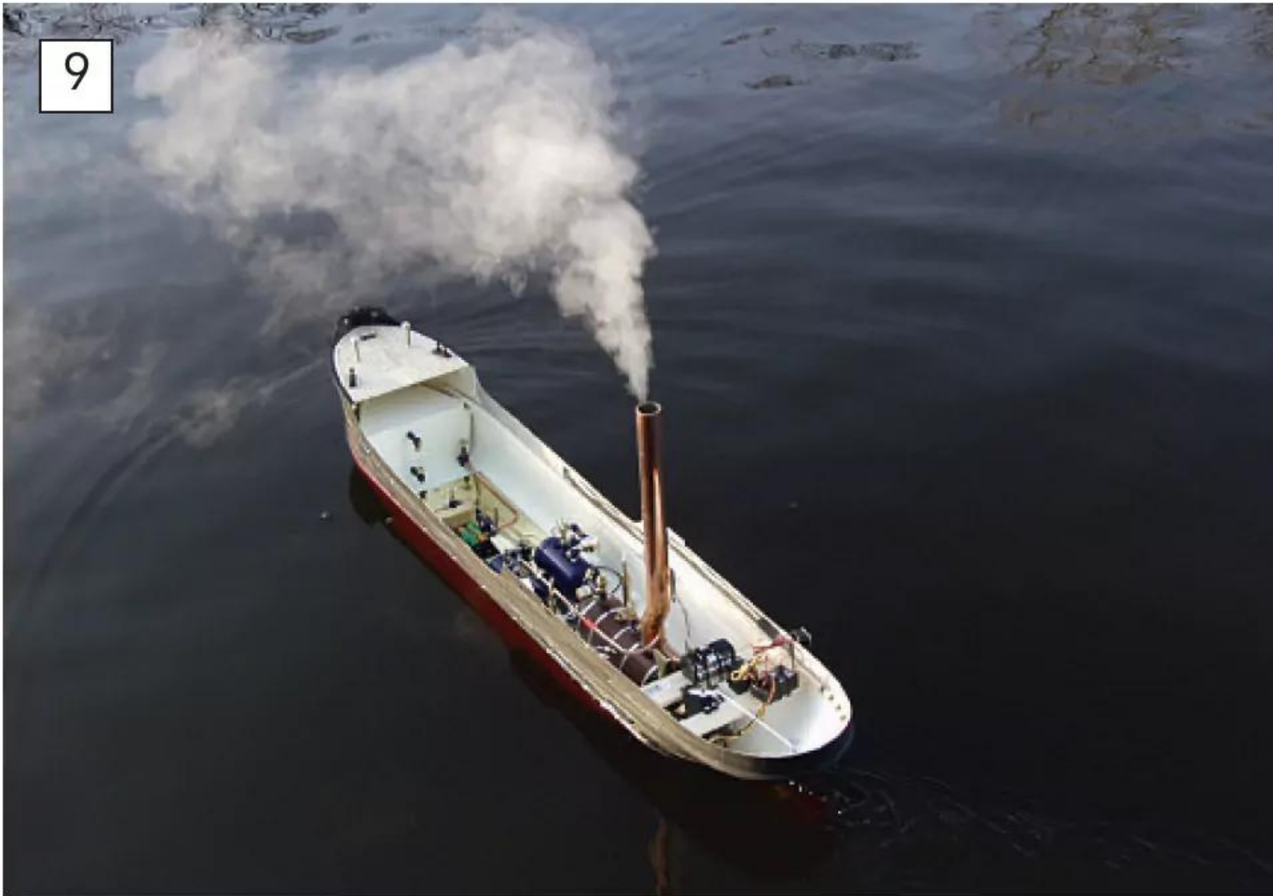
9 Never underestimate the value of sea trials. Best done without the decks fitted, this is the best chance you are going to get to see if everything works in harmony and is easy and convenient to operate.
