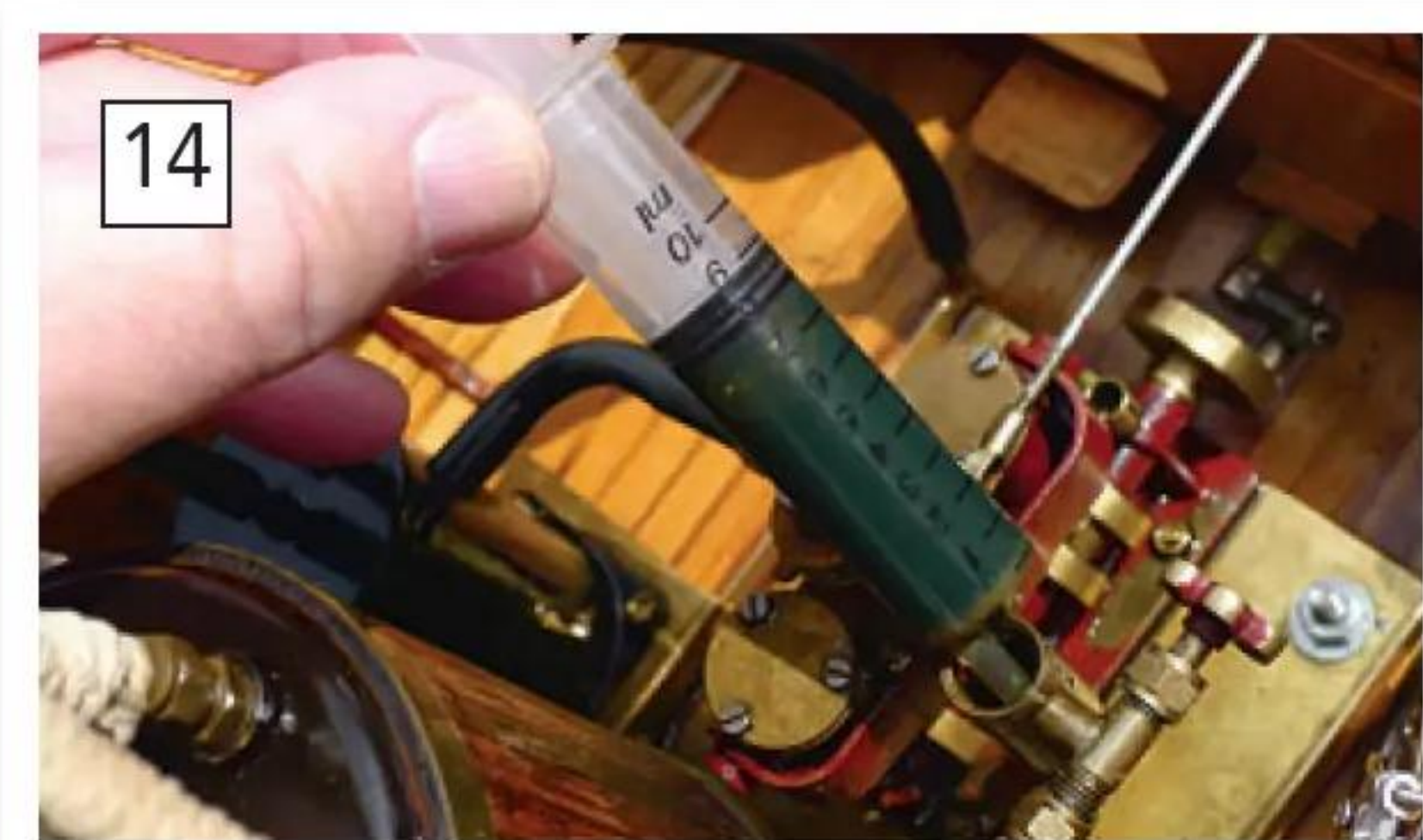
Using a syringe, rather than waiting for gravity to act on the thick steam oil, always speeds up filling the lubricator.
