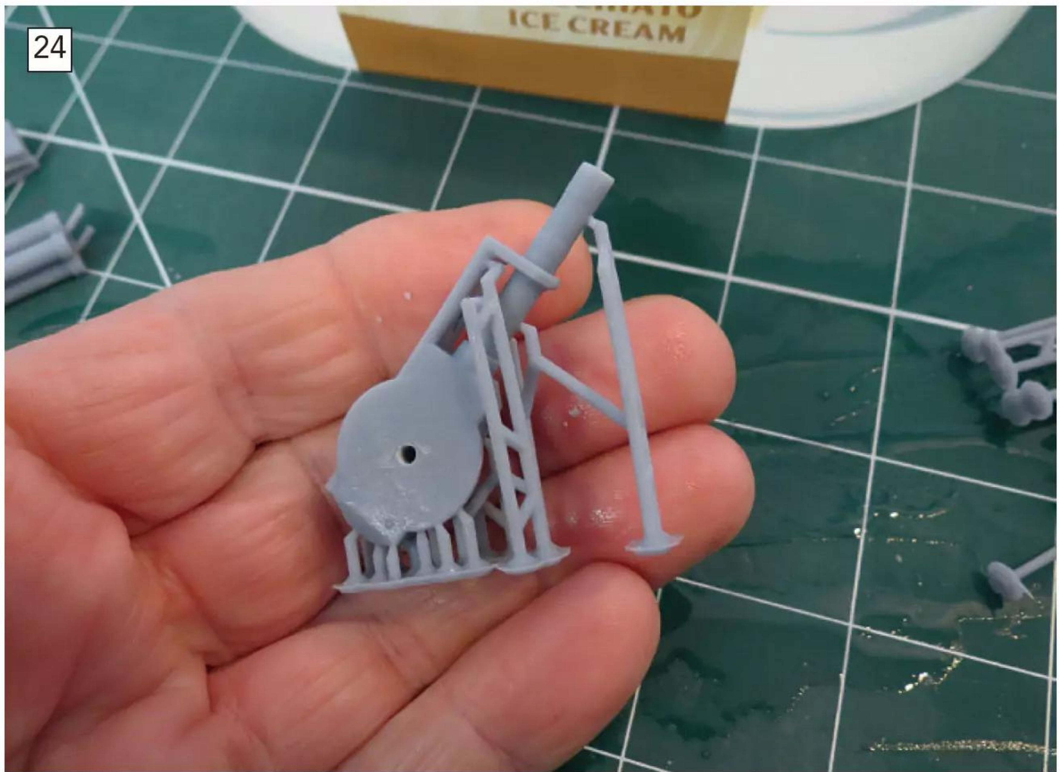
One of two 3D produced gatling type guns directly from the printer.
