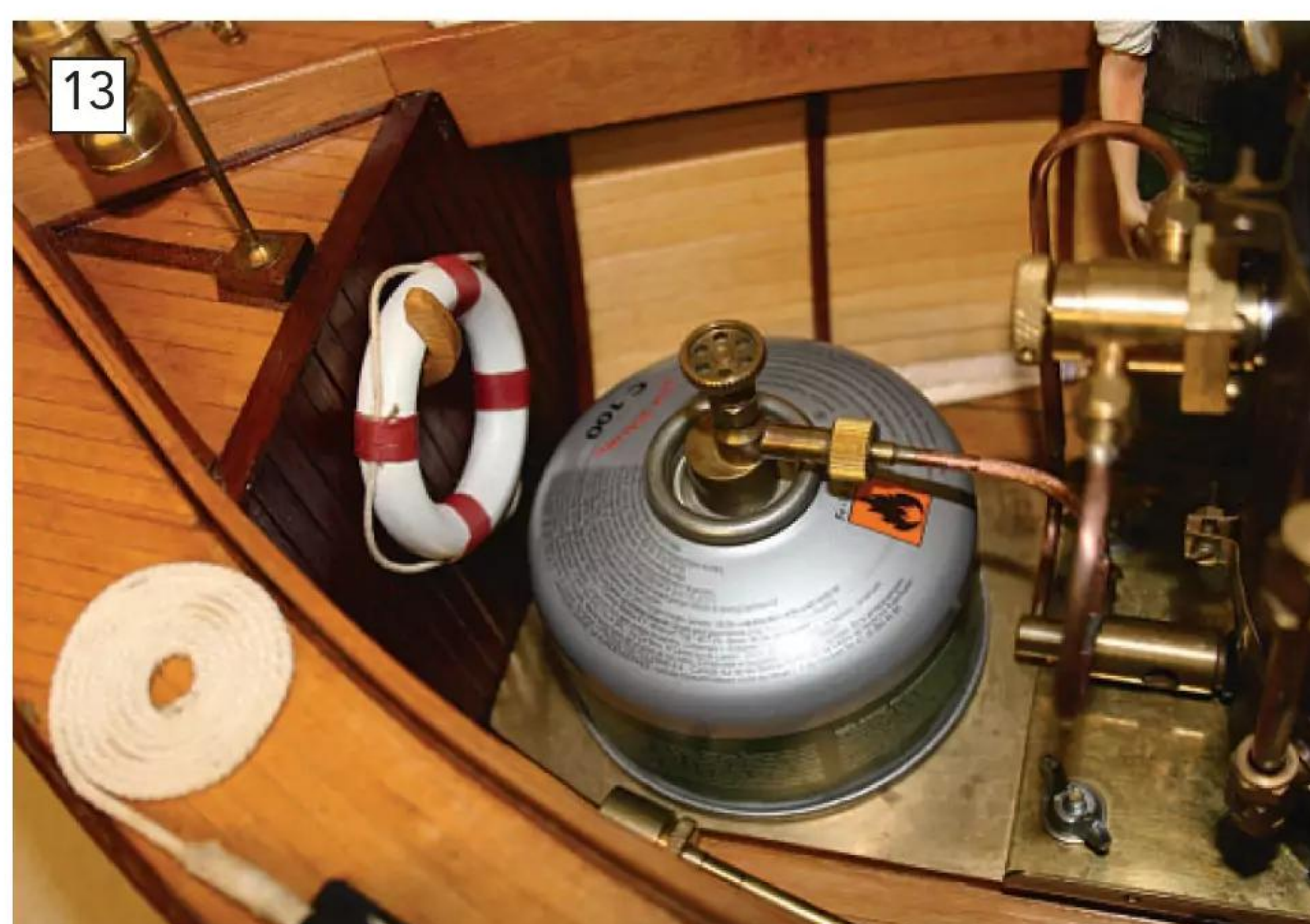
A disposable gas tank makes for a quick and easy tank change.
