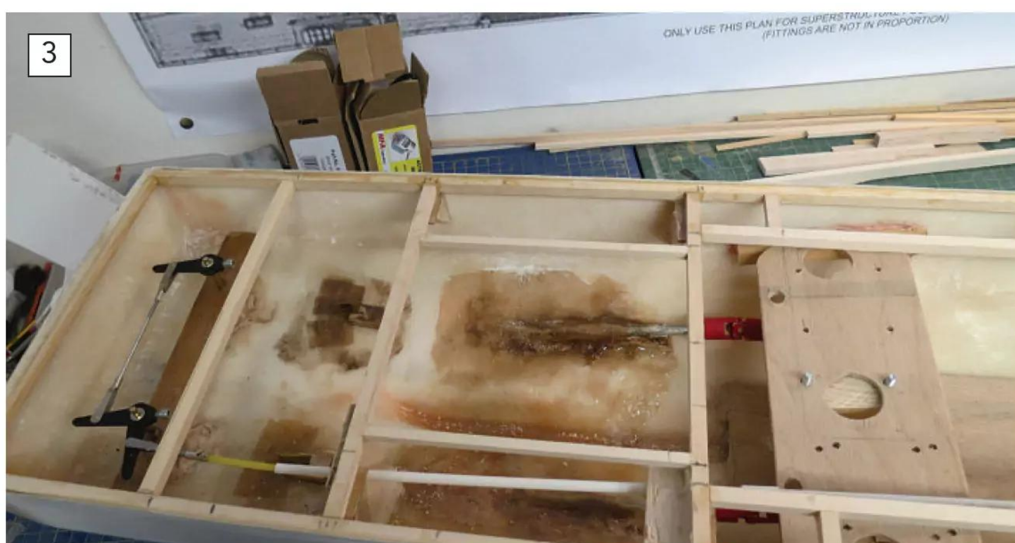
The dual rudder linkage and inverted engine mounting for two 540 motors.
