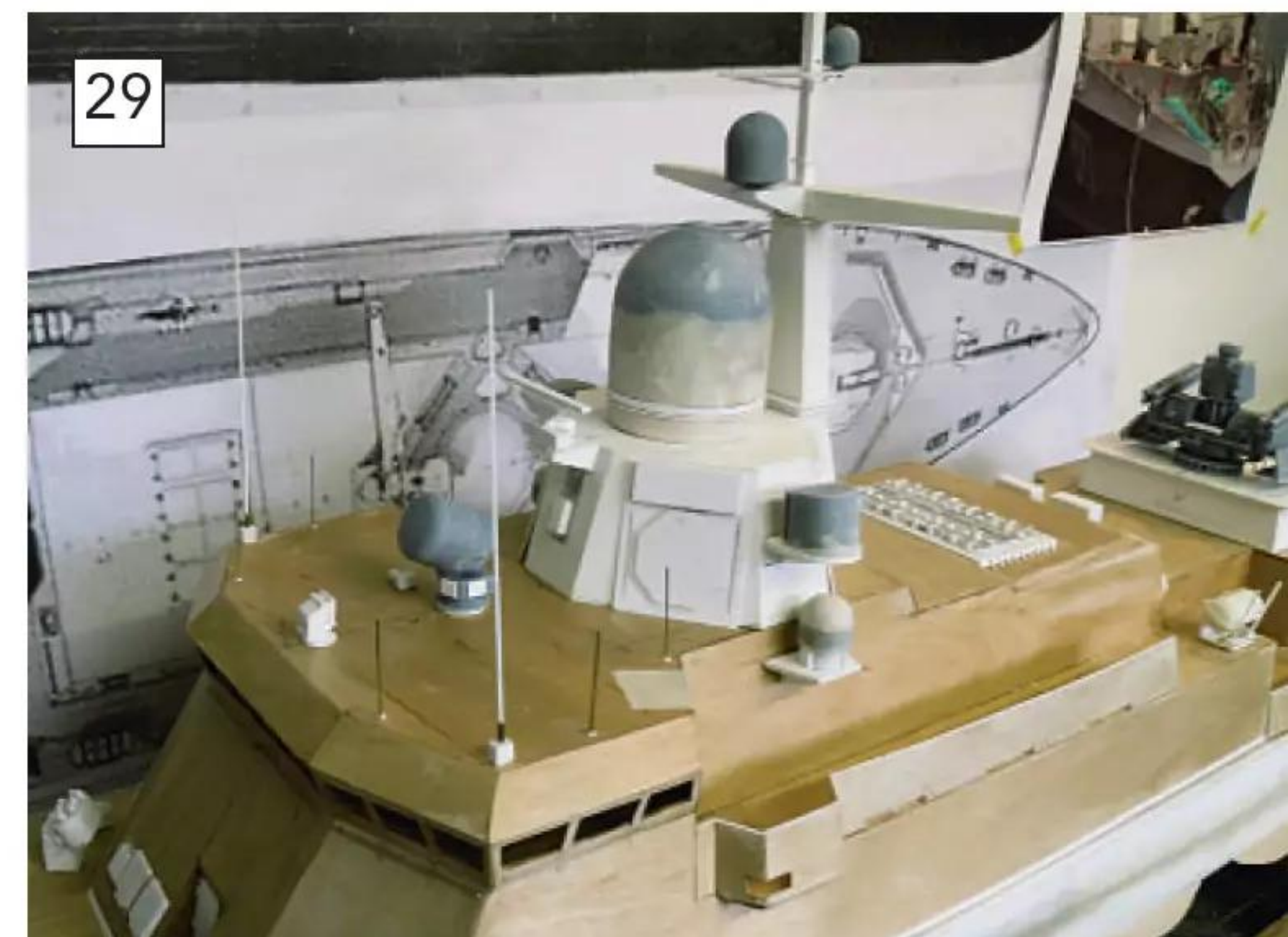
Locating the various fittings on the bridge roof.
