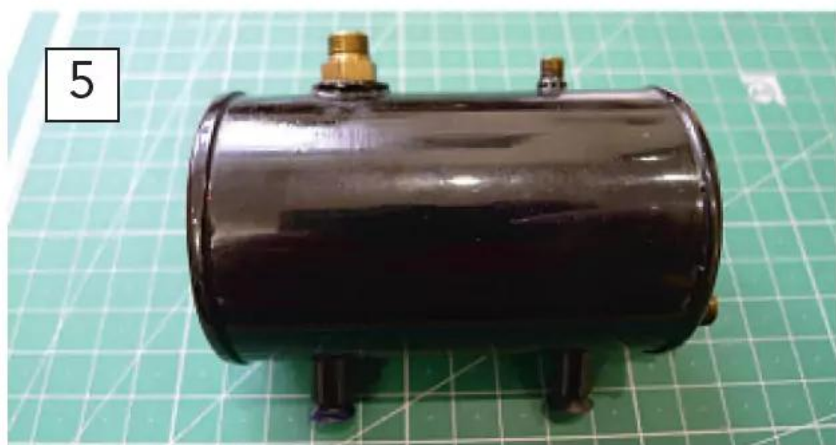
A typical horizontal type separator. If the exhaust steam remains fairly dry and the separator is mainly collecting oil, this unit could last well in excess of the 20 minutes.
