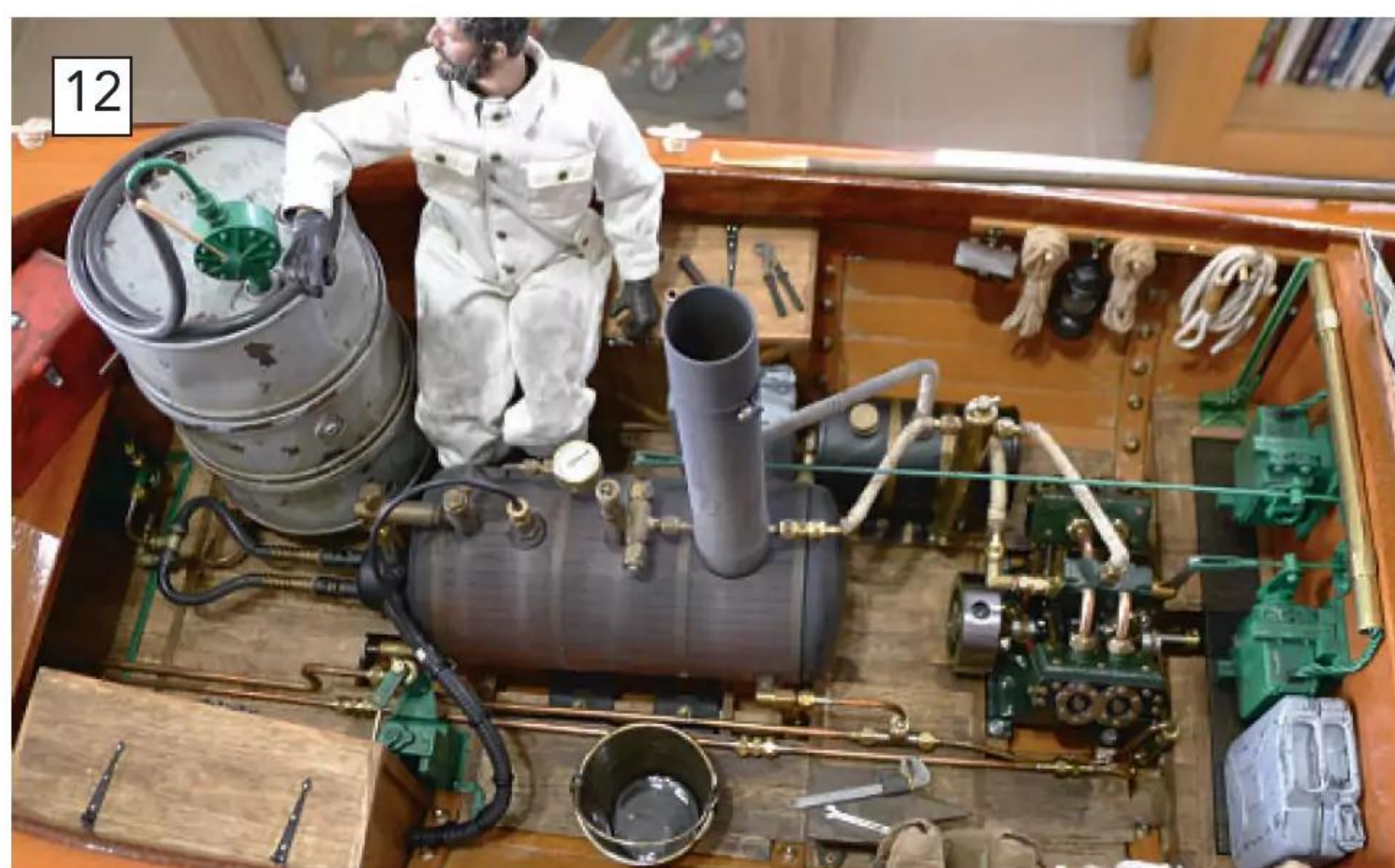
If you have a big open hull, you can take advantage of this to push the boundaries a little as far as endurance is concerned. This plant has an automated boiler water feed system, an automatic gas control valve and a larger than normal lubricator.
