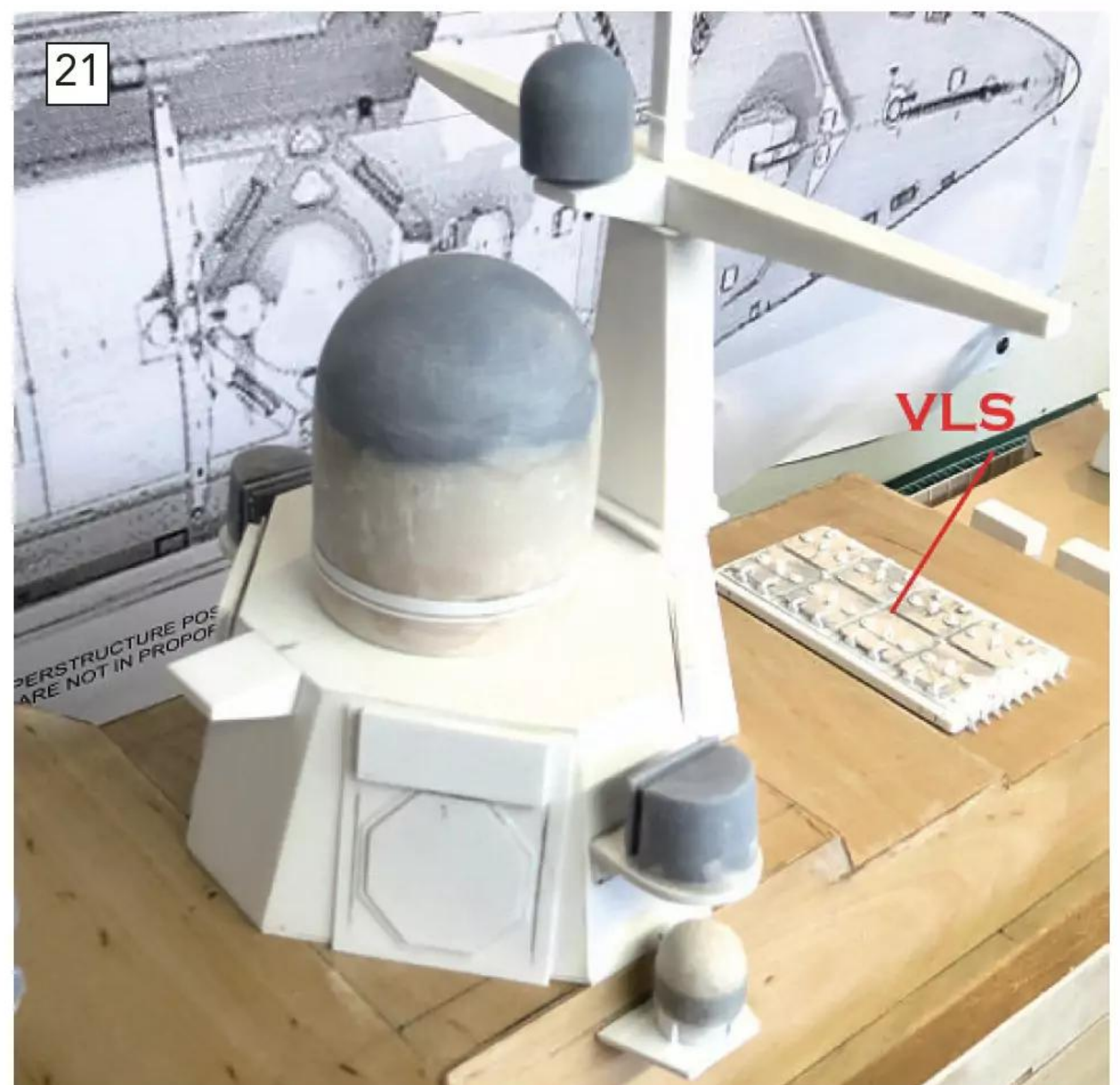
To the rear of the mast, at a slightly lower level, is the 8-cell VLS (Vertical Launch System).
