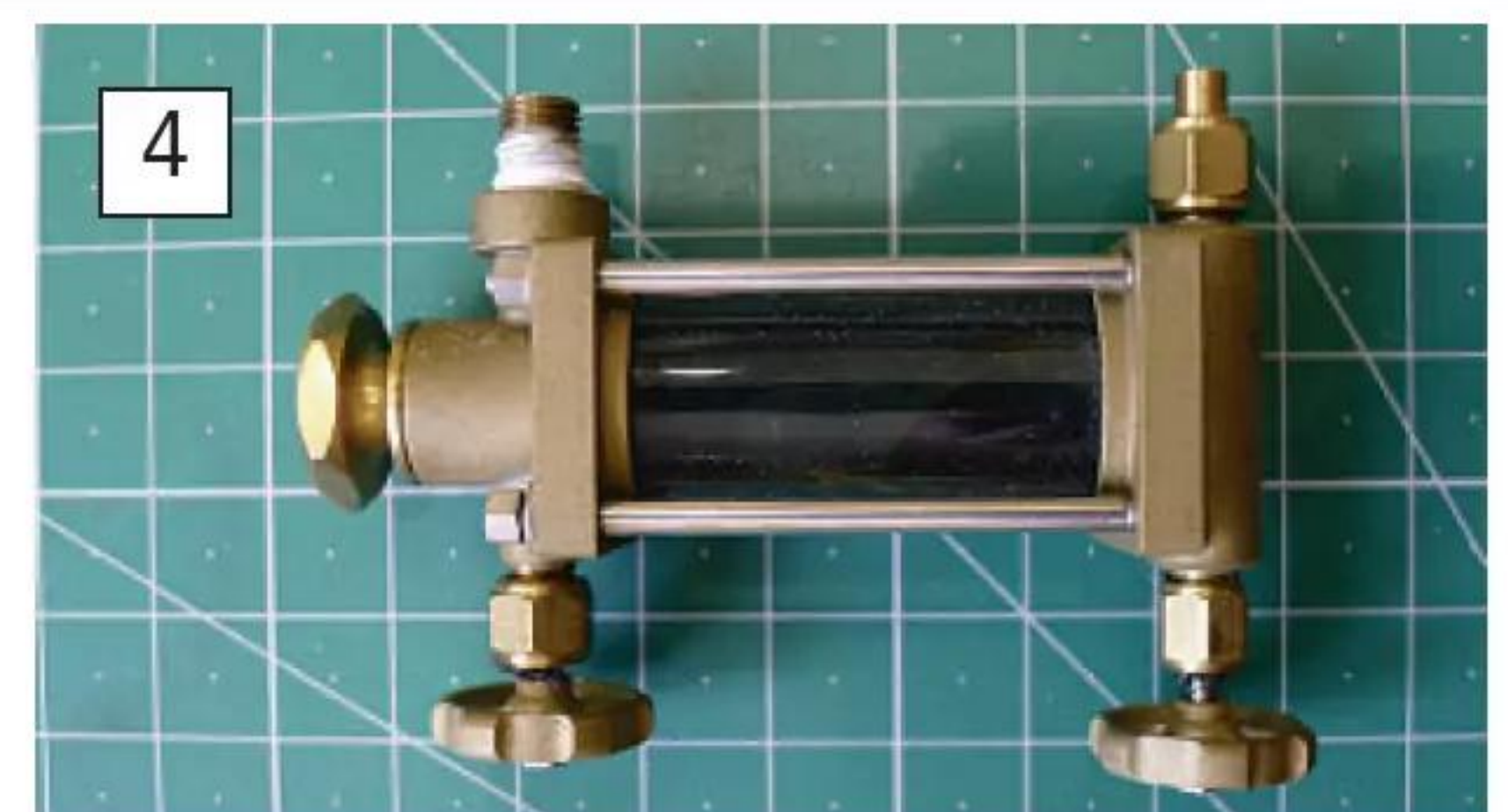
At the other end of the scale, a much higher capacity and a needle valve to control oil flow will give you a lubricator that could easily last up to an hour.
