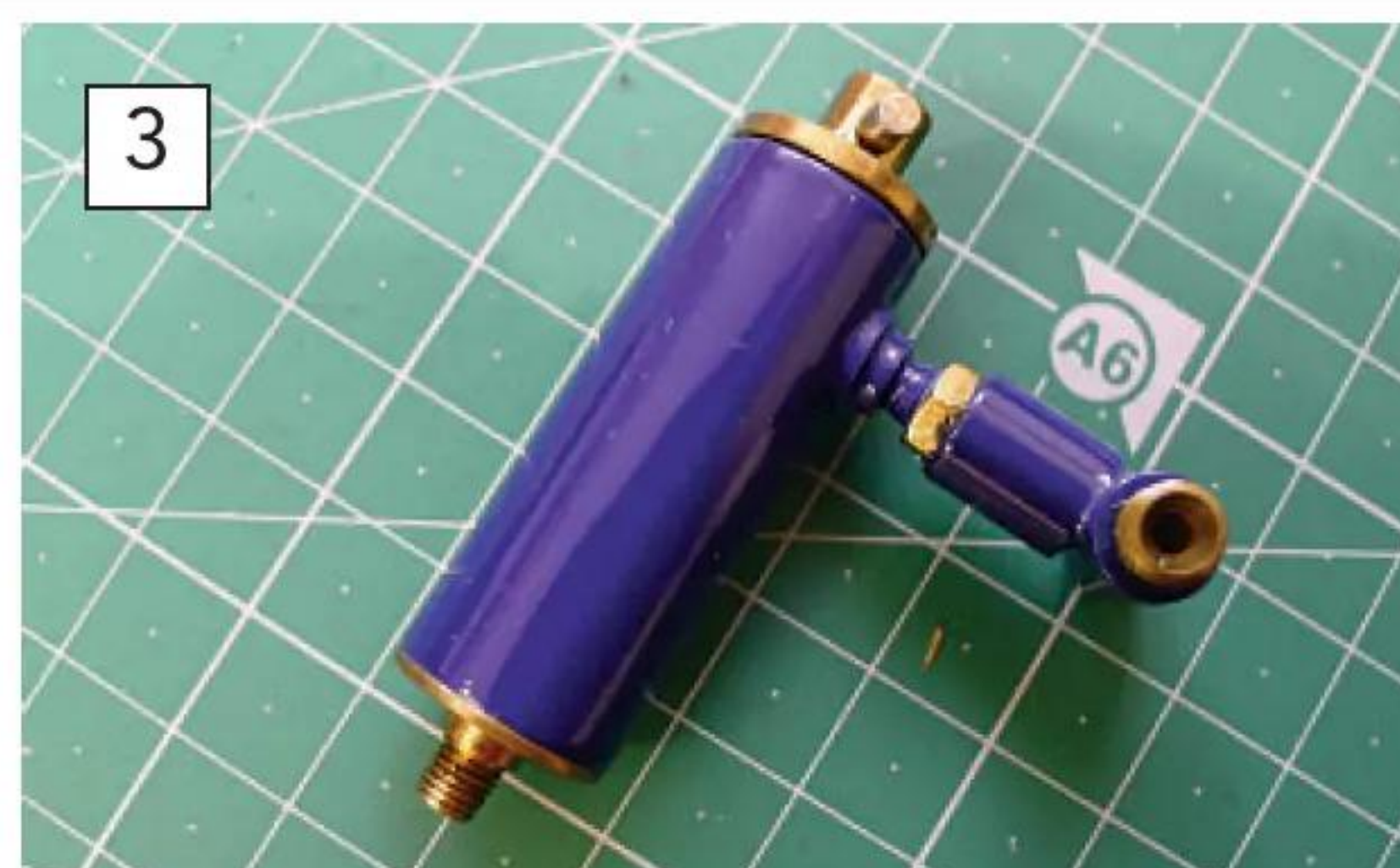
A standard Hemmens lubricator unit for a twin cylinder oscillator, complete with drain connection but no control.
