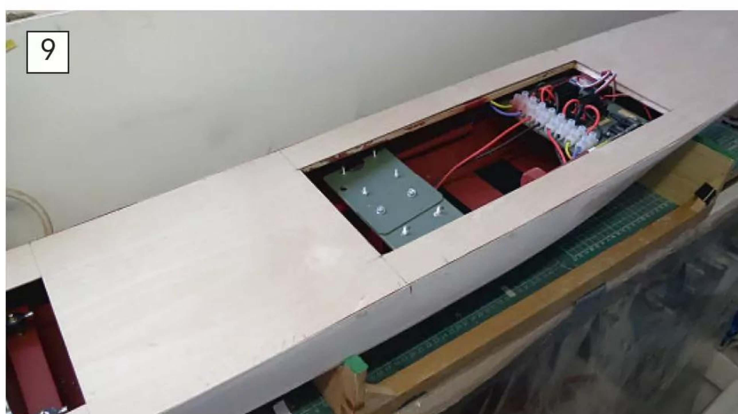
Satisfyingly, the deck openings match the inboard edge of the bearers so that a raised coaming can be added to the main access area.
