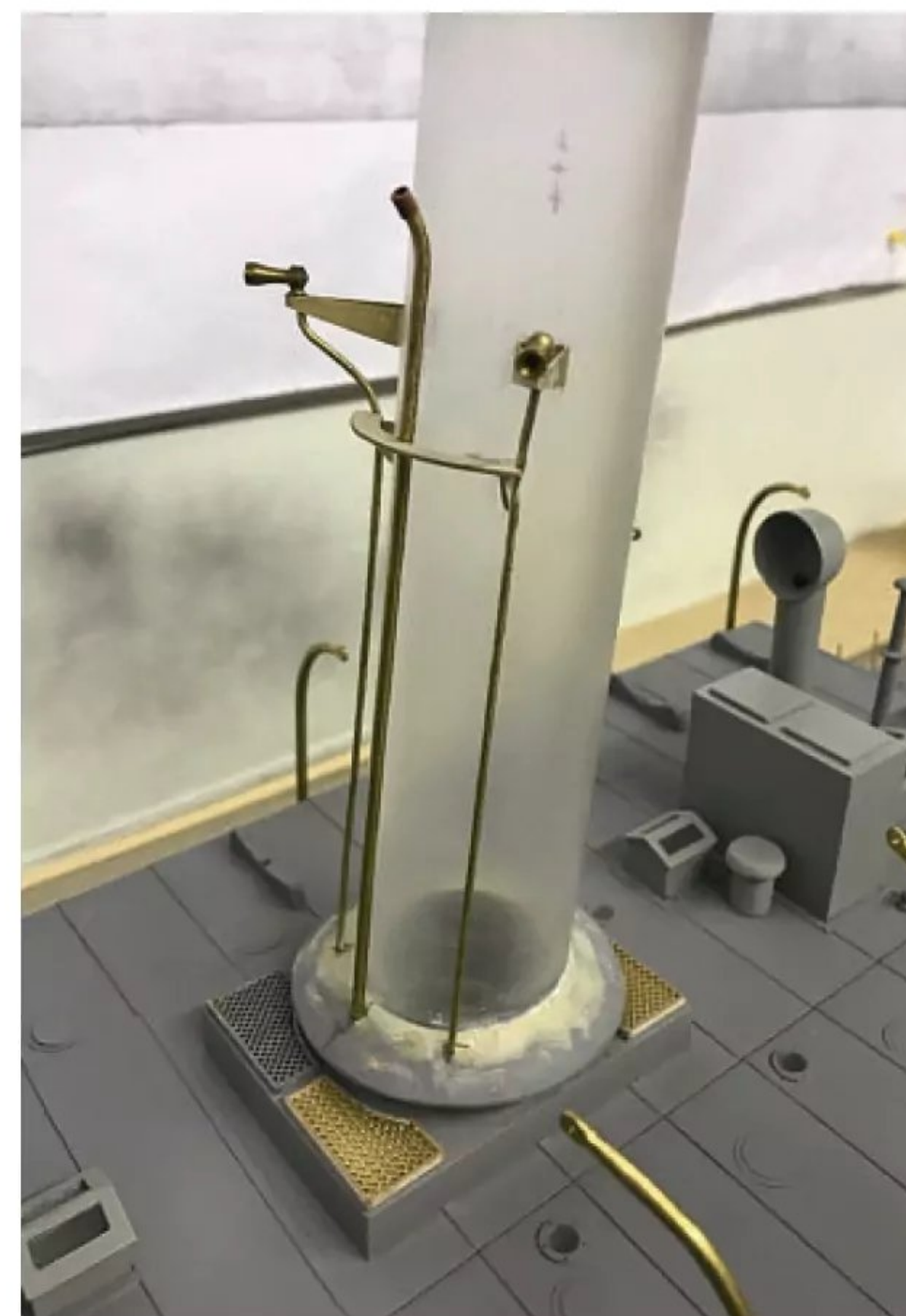
Acrylic tube, which, when detailed with fittings from the drawer that time forgot, was turned into a stylish funnel.
