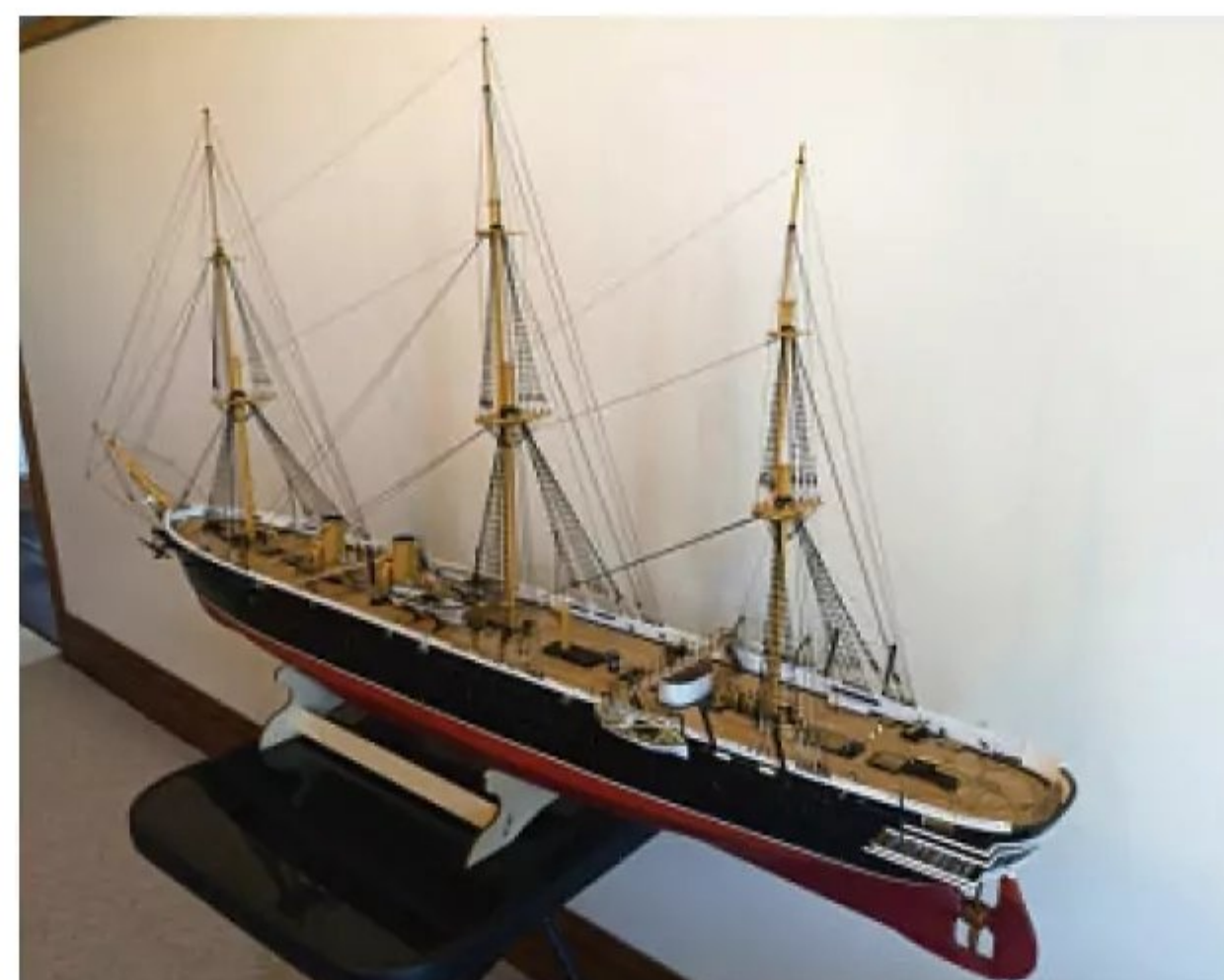
The standing rigging complete.
