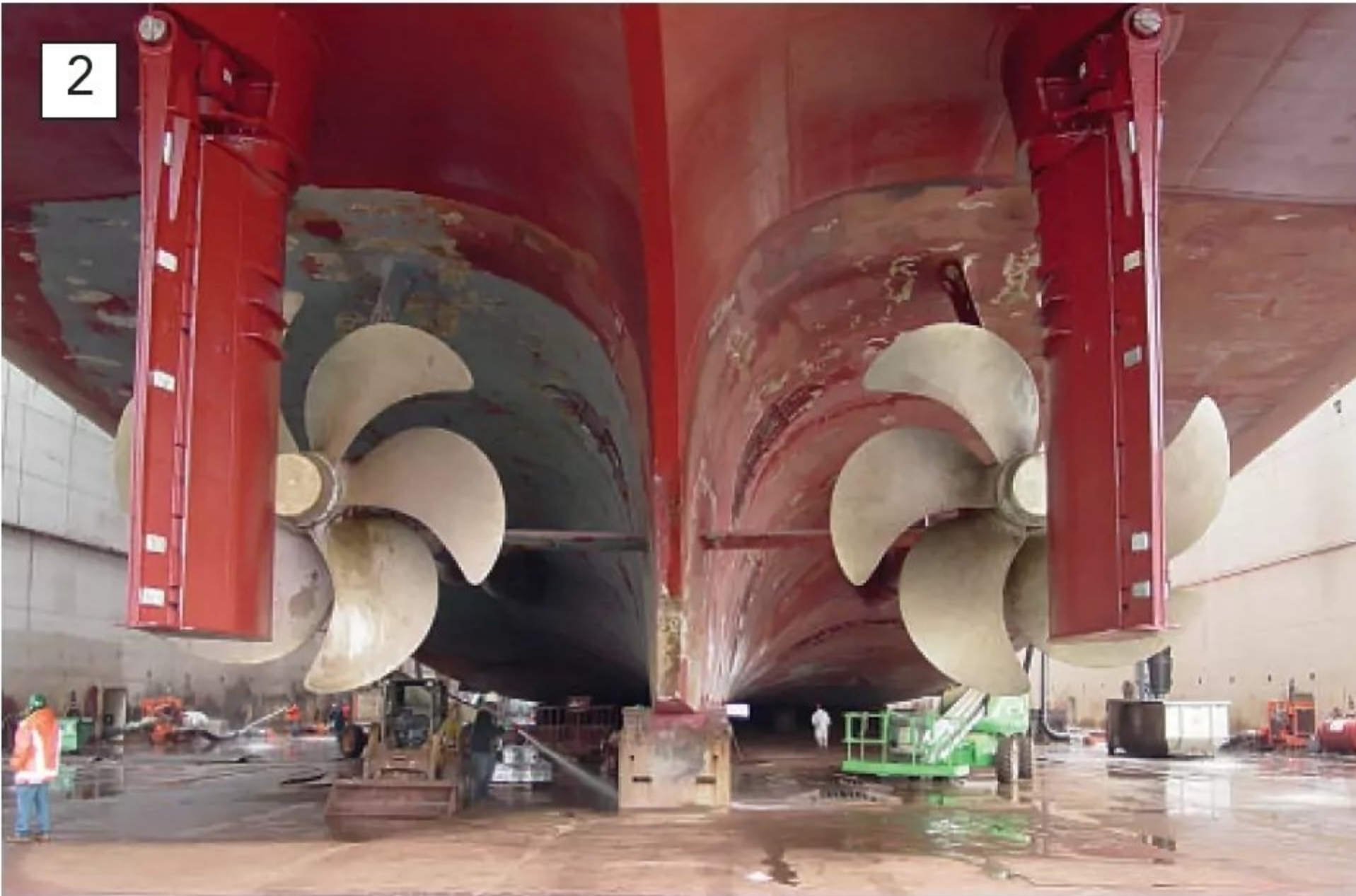
The two propellers on this vessel generate a significant amount of thrust to push a ship of this size through the water at speed. If this thrust wasn't transmitted directly into the ship's structure and isolated from the prime mover, it could cause significant damage.
