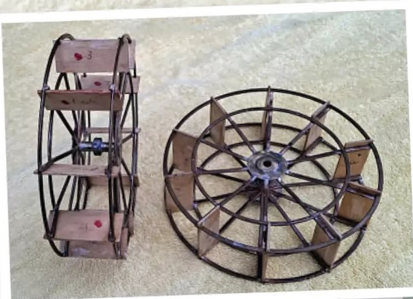
One method of paddle wheel construction from flattened and shaped copper wire, by M. Teese.
