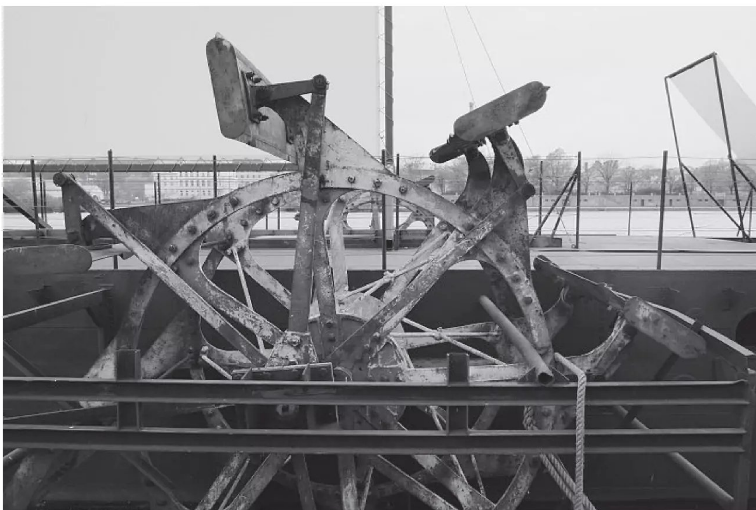
Feathering paddle wheel of an old paddle steamer in Prague (Wikipedia).
