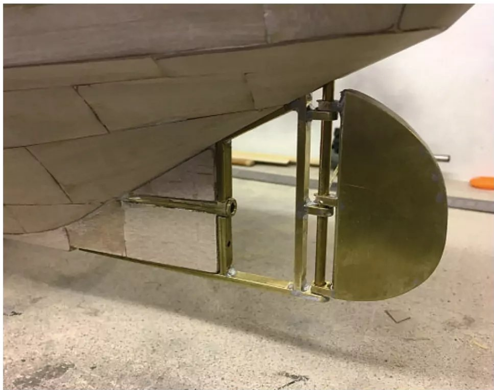
The rudder support framework is technically fully removable via hidden screws, but only in the most drastic of emergencies!
