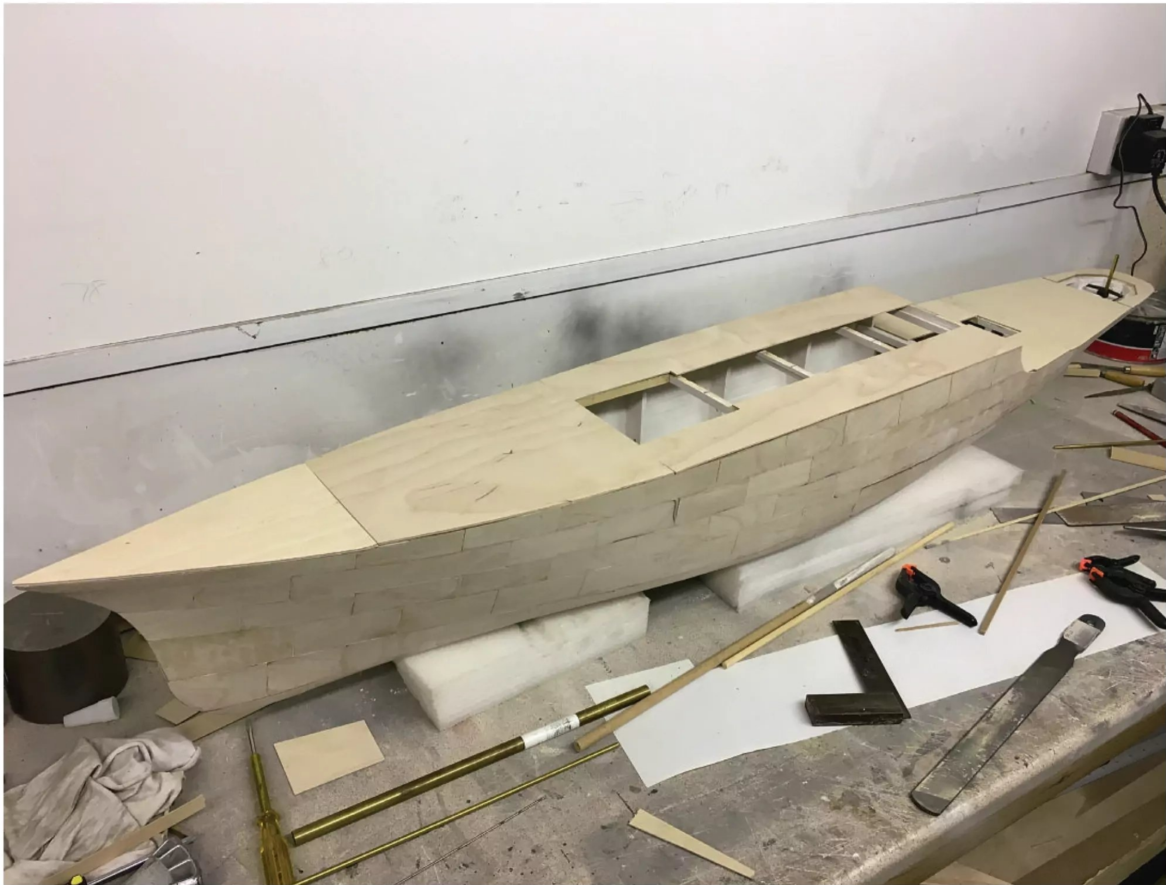
The application of the 1/32" plywood plating allows the shape of the hull to appear.
