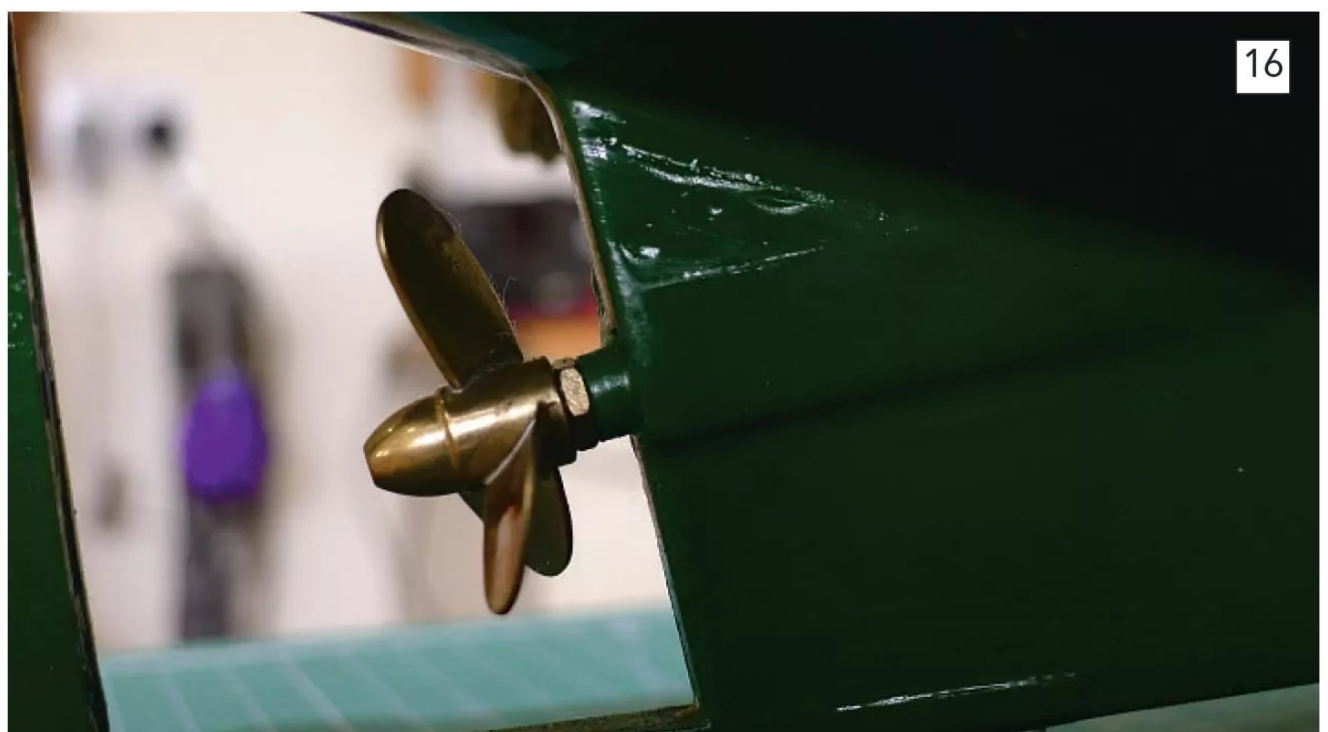
At the ‘business end’ you want to feel just the slightest amount of clearance when pushing the propeller backwards and forwards. When you do, you should see no movement at the motor or engine. Again, this set up uses a plastic bush with a built-in thrust face.
