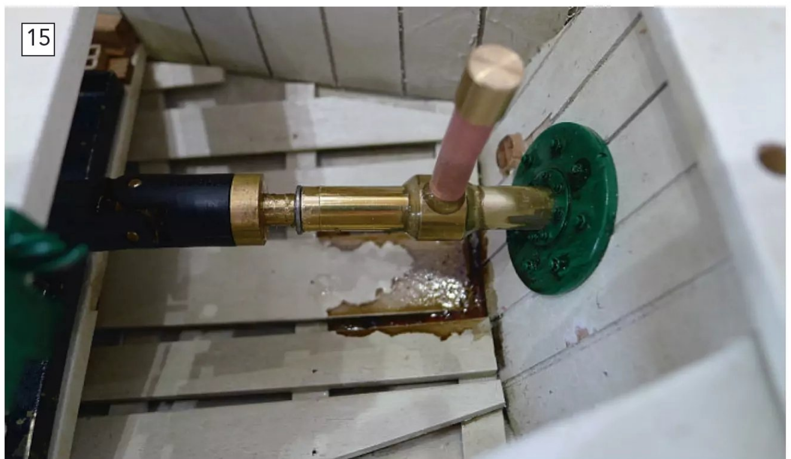
A simple spacer was made, and a thrust washer was fitted to accommodate the thrust in the shaft when going astern.
