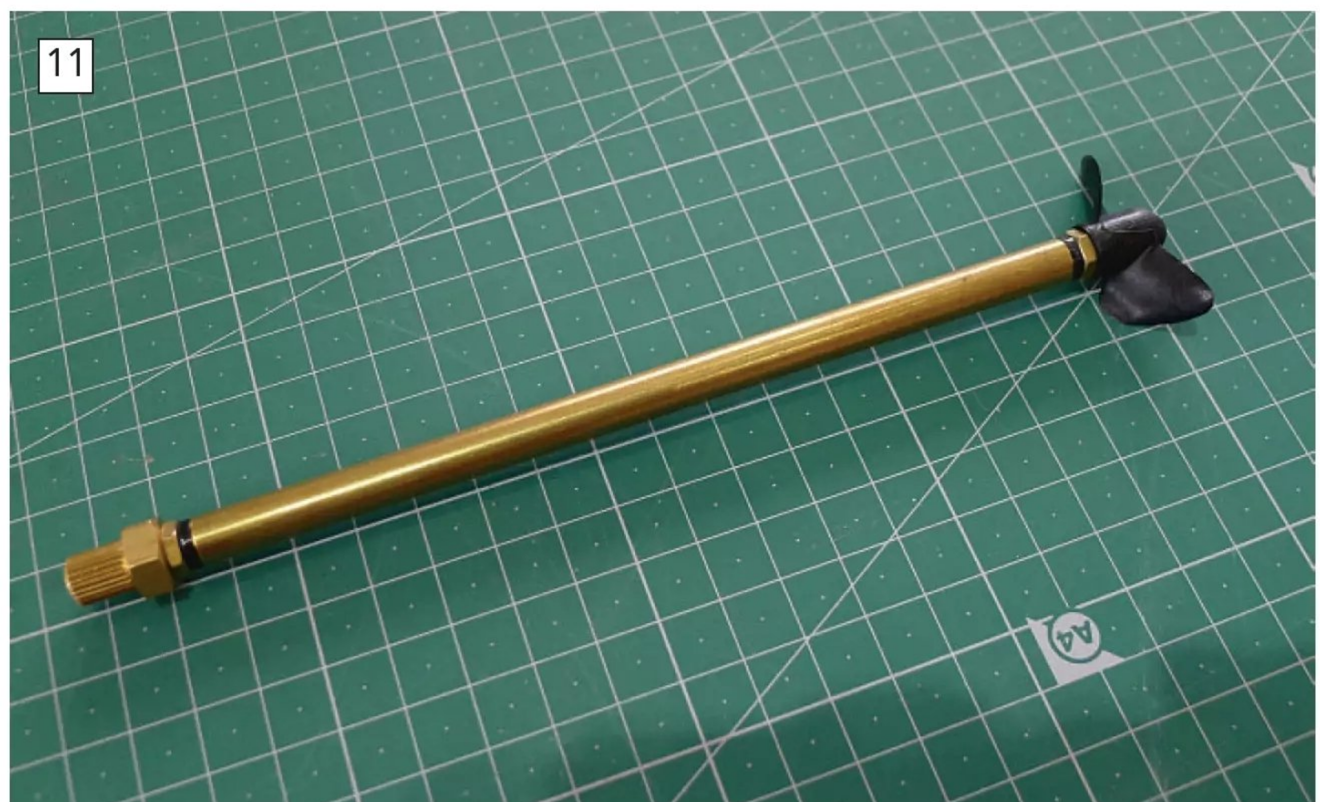
When the coupling is fitted, whether threaded with a locknut or simply a collar locked by a grub screw, the shaft should have a slight movement backwards and forwards to allow the ahead and astern thrust faces to do their job.
