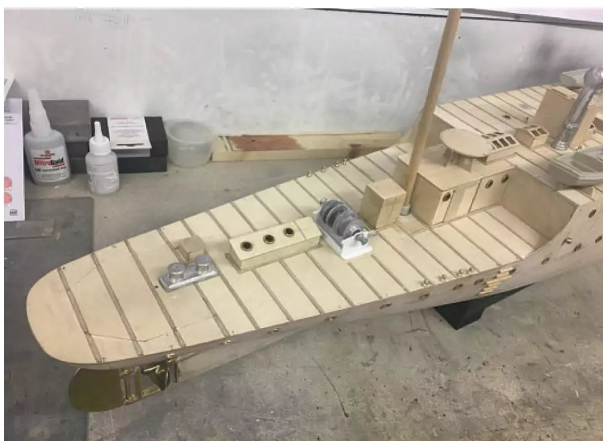
The initial details being added on the hull and deck using lithoplate sheet, brass and aluminium tube. The off-set access to the internals of the model can just be seen.
