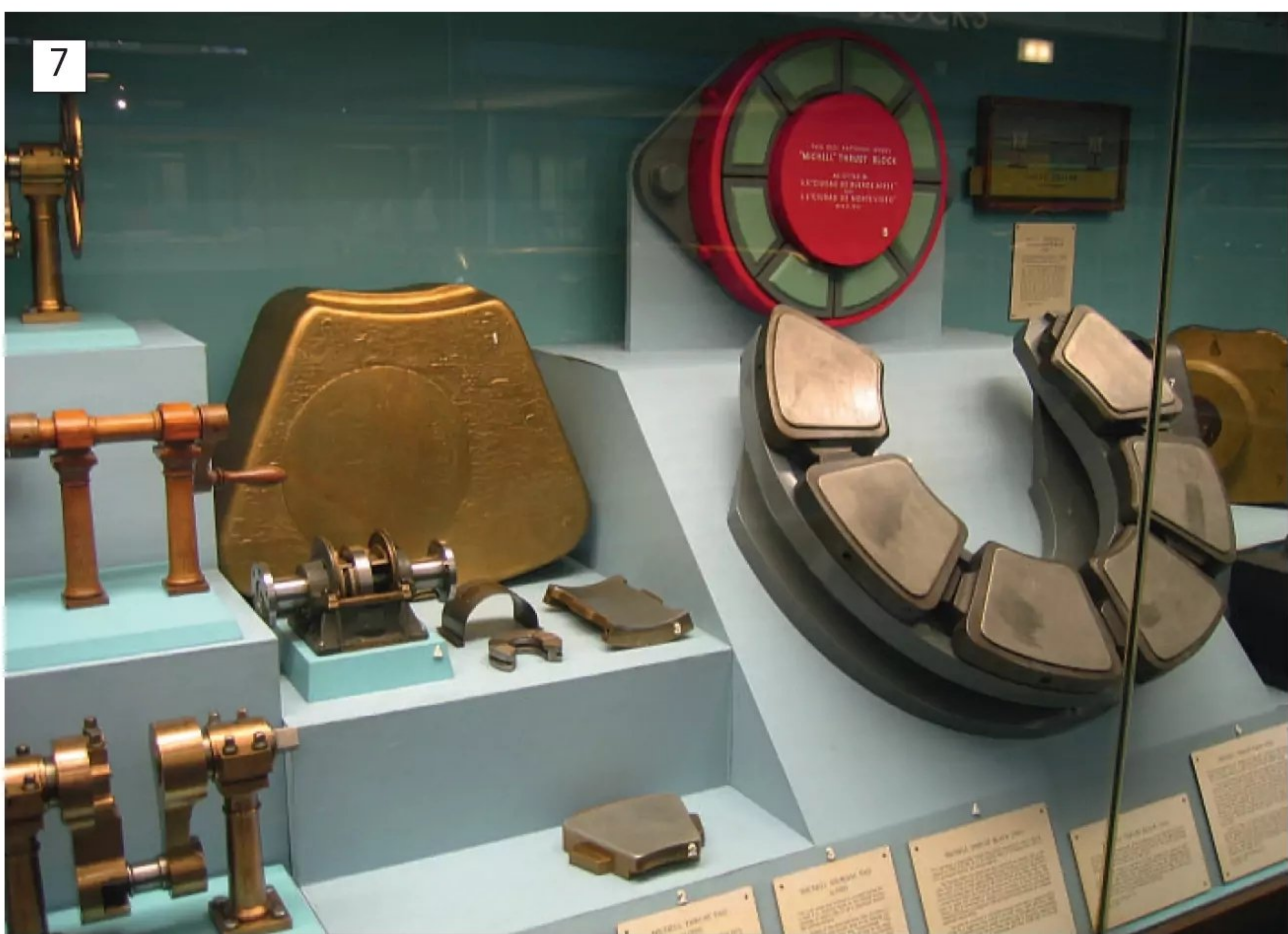
Nowadays a Michell type bearing arrangement is common. The bearing 'kidney' pieces are free to 'float' on a pivot, so form an oil wedge on the thrust face in exactly the same way as a rotating bearing does.
