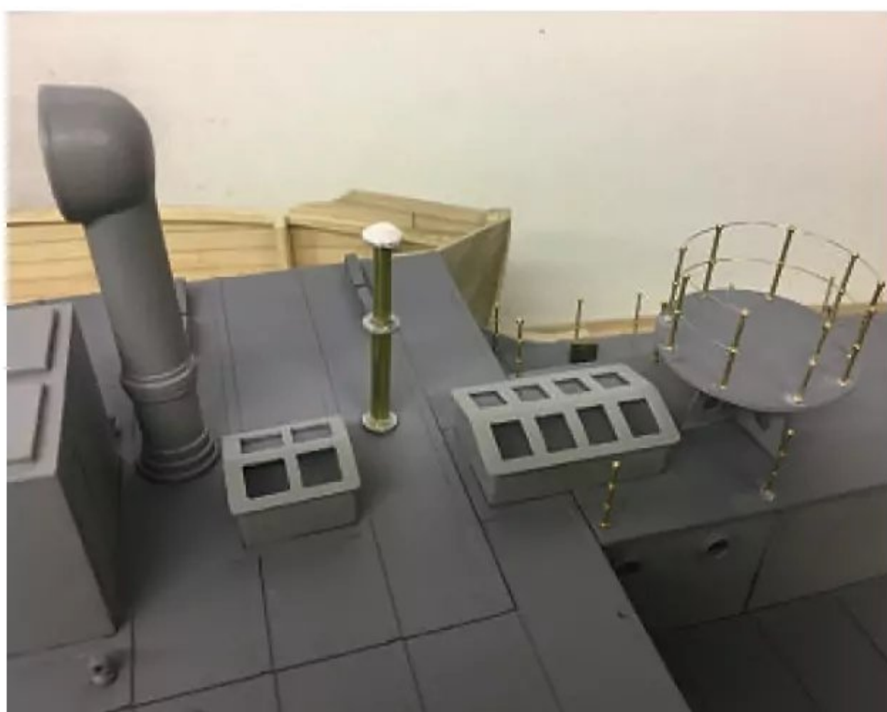
Further deck details being modelled from 1/32" plywood sheet. The deck was festooned with many decklights and skylights. The 3D-printed searchlight was from the Shapeways Shop 3D Boats.
