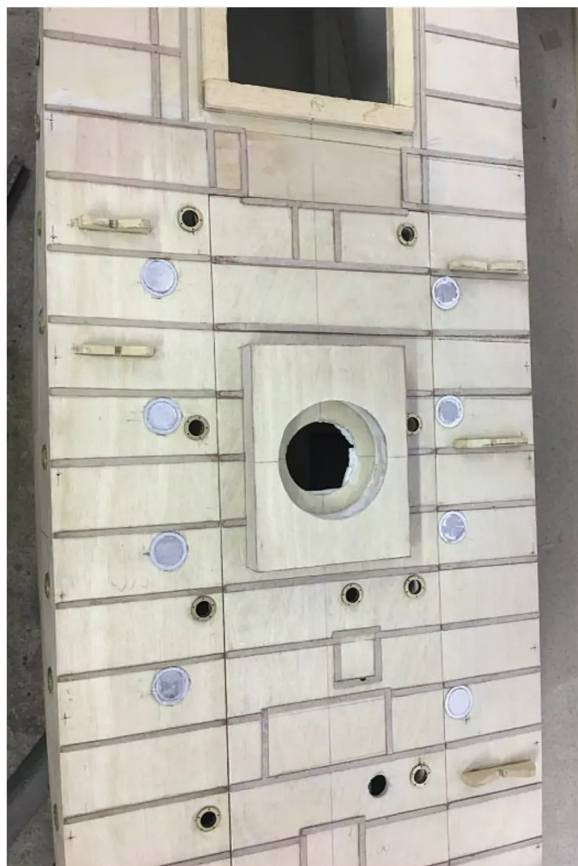
The initial details being added on the hull and deck using lithoplate sheet, brass and aluminium tube. The off-set access to the internals of the model can just be seen.
