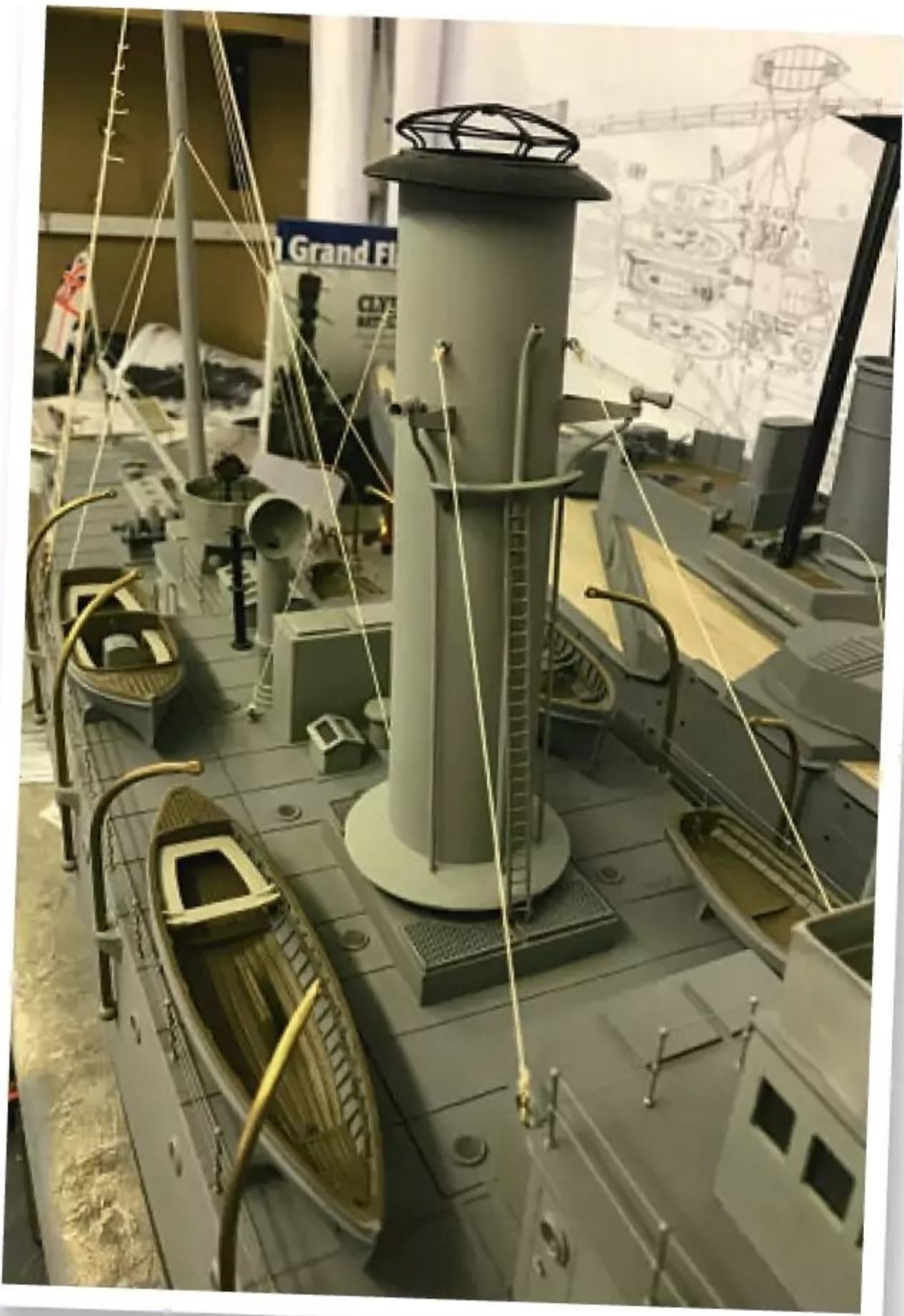
The ship's boats, sourced from Quaycraft, being fitted out, with the associated davits being made from brass tube bent to shape using a pipe bender.
