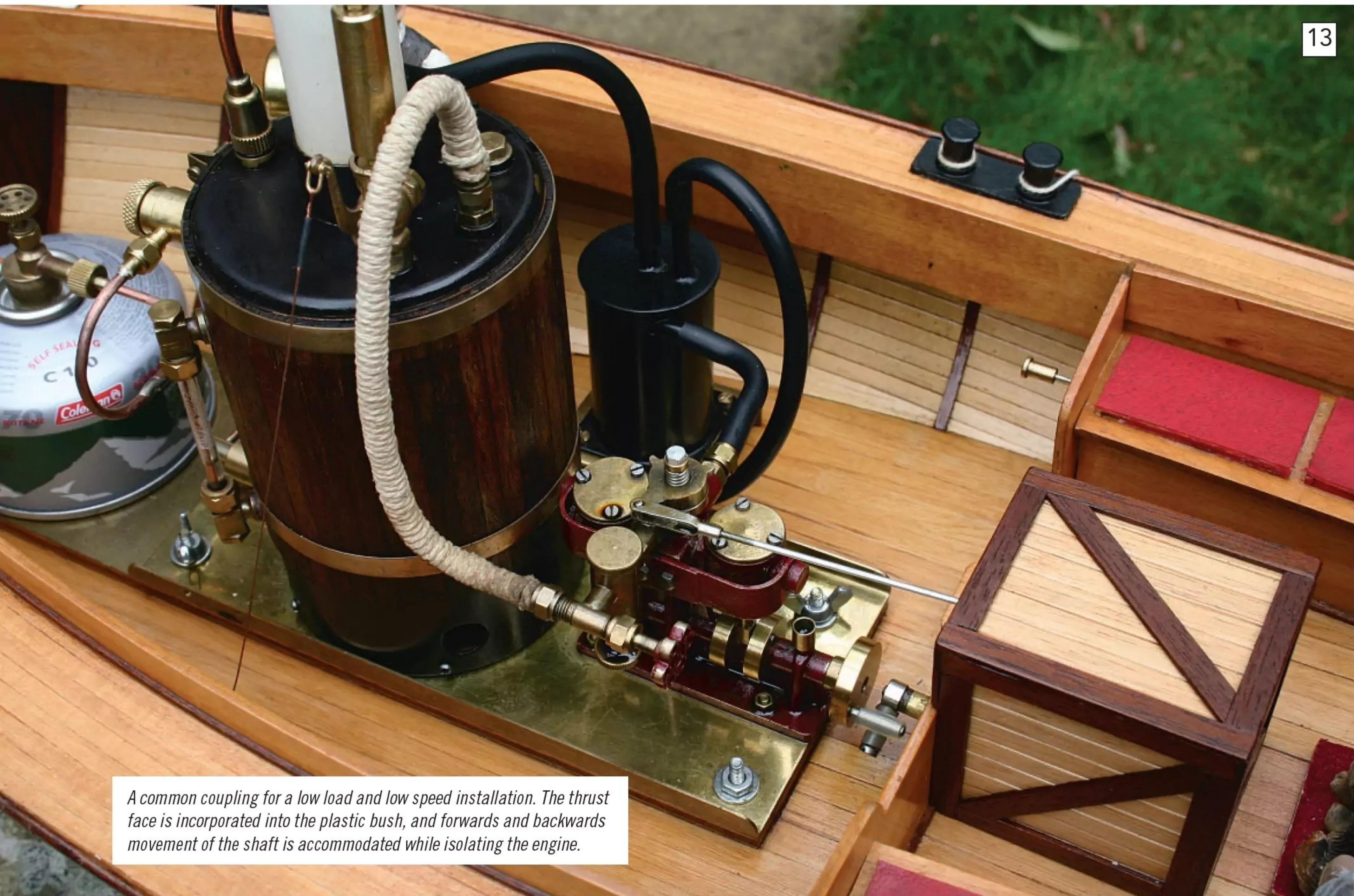
The most important aspect is that the coupling should allow free movement of the shaft backwards and forwards, while isolating this from the prime mover. Frequently, splines in this type of coupling are tight and so do not isolate the motor or engine from this movement.
