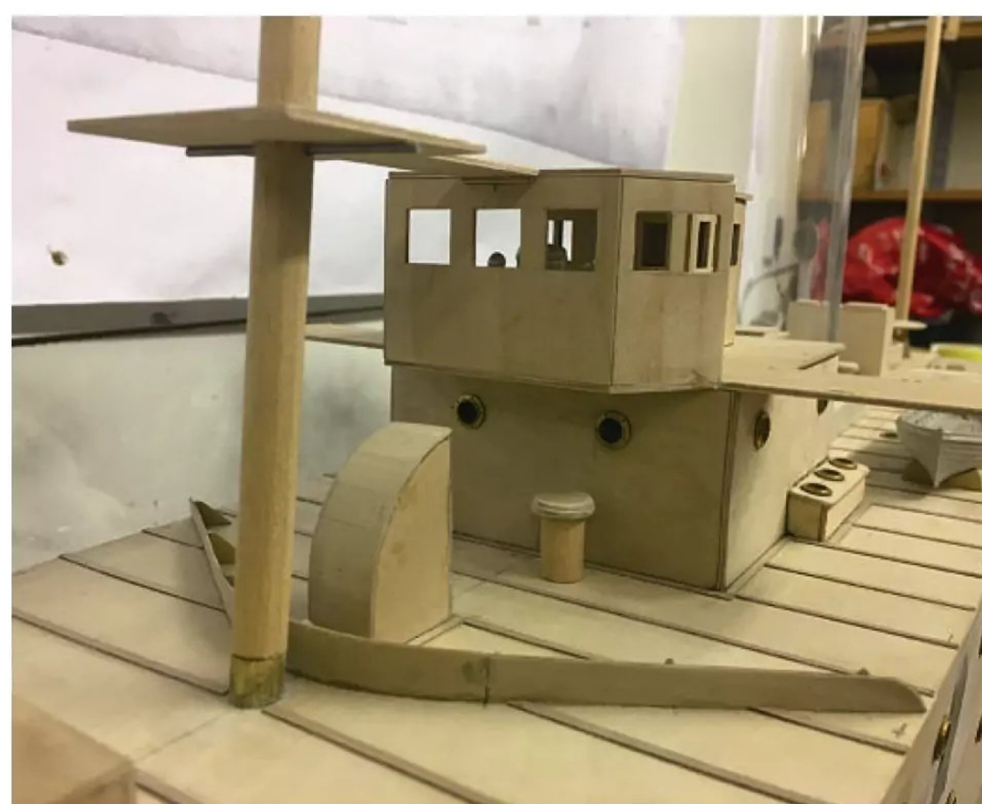
The initial details being added on the hull and deck using lithoplate sheet, brass and aluminium tube. The off-set access to the internals of the model can just be seen.
