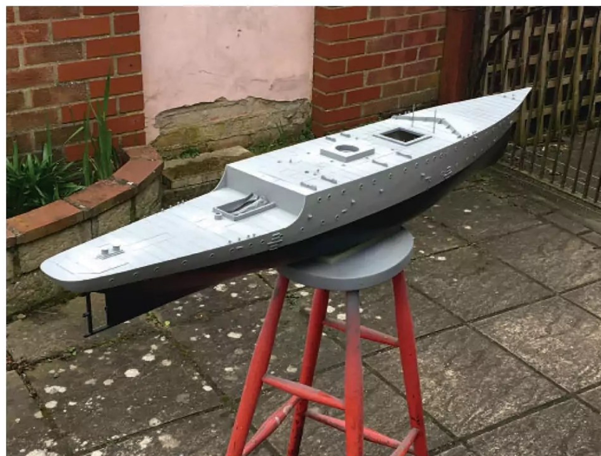
The hull spray painted in drab warship grey. Interestingly, the black waterline is not straight but actually tapers upwards at each end of the ship.
