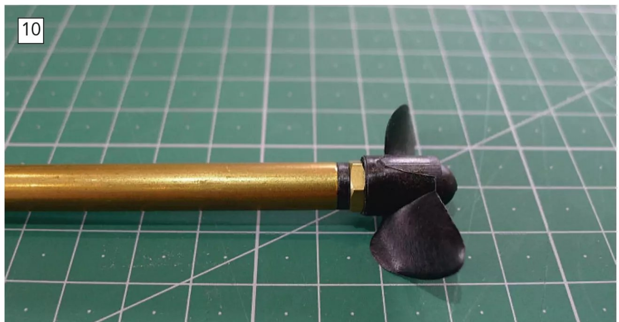
This then allows the lock nut to run on the aft thrust face of the shaft bearing, and hence transmit the thrust from the propeller into the stern tube, and therefore the model. If there is a clearance here when the propeller is pushed forwards, then something else is transmitting the thrust.
