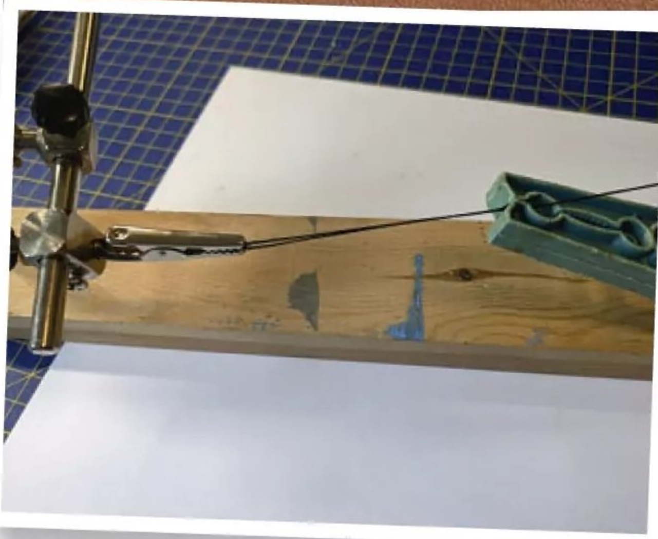
Seizing a deadeye onto the end of a shroud.
