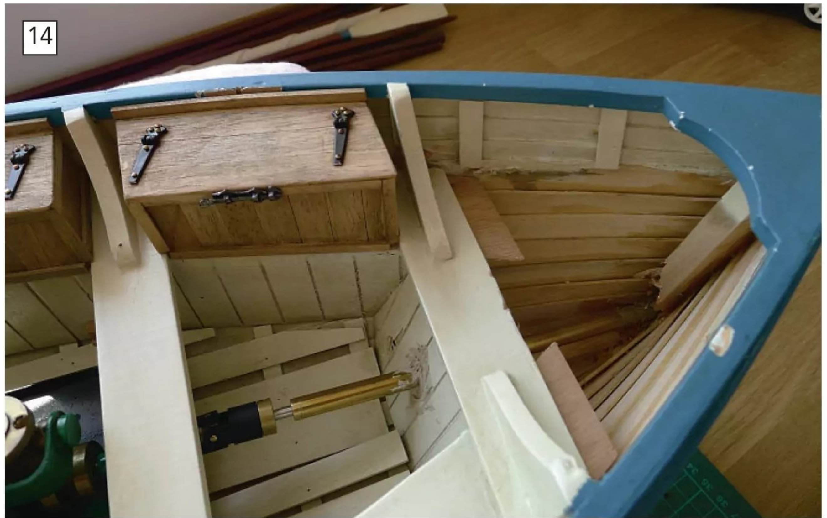
In this initial assembly it is easy to see that if the splines in the coupling are tight, forces will be transmitted into the engine. If the splines are slack, there’s too much movement of the shaft and you might get the propeller interfering with the rudder.
