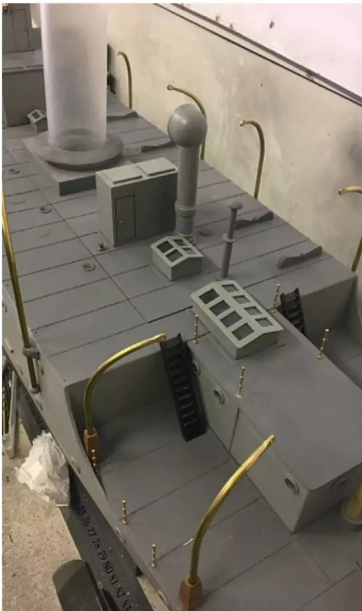
Further deck details being modelled from 1/32" plywood sheet. The deck was festooned with many decklights and skylights. The 3D-printed searchlight was from the Shapeways Shop 3D Boats.
