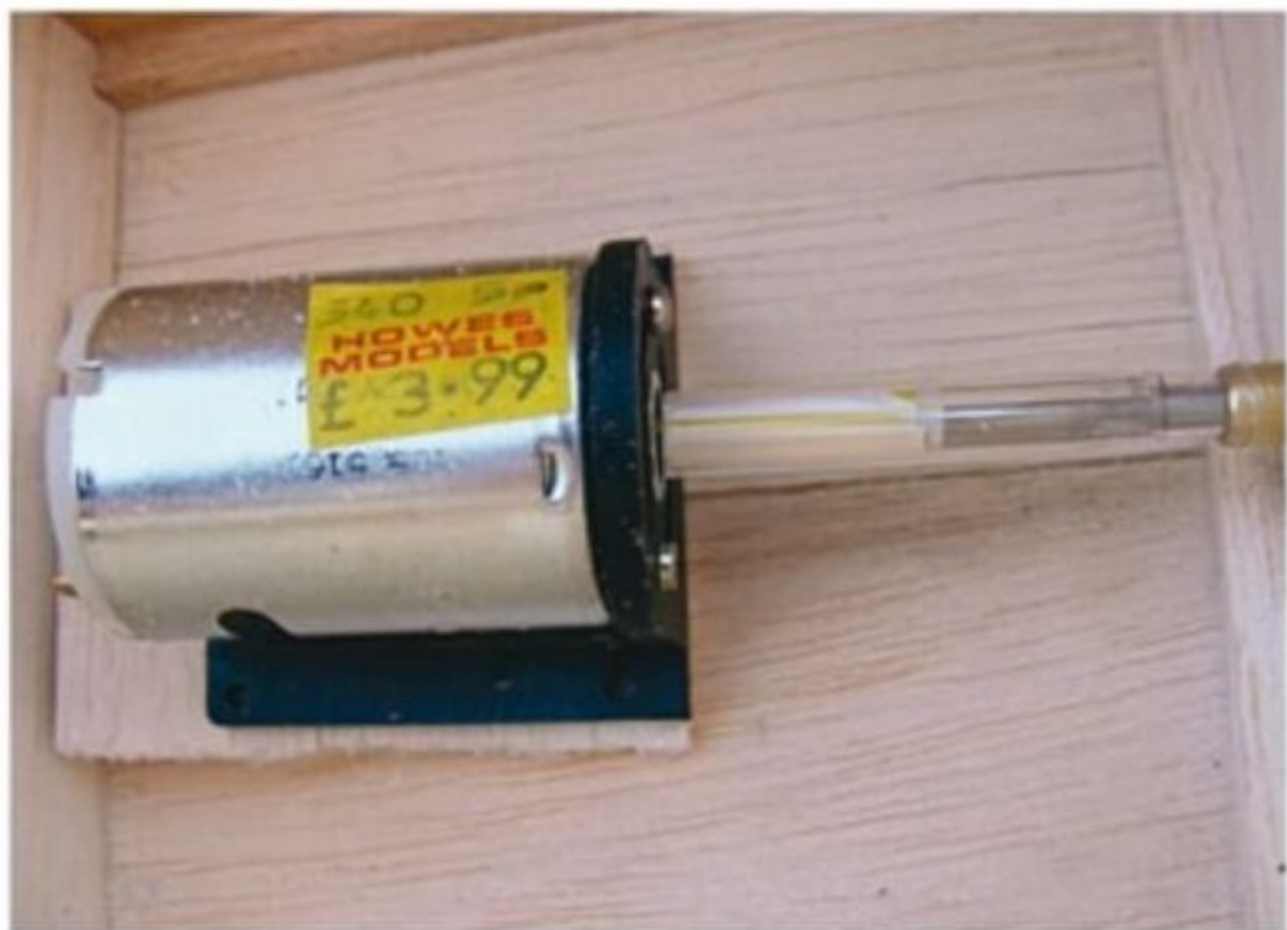
Getting shafts aligned with rigid close-fitting tube.
