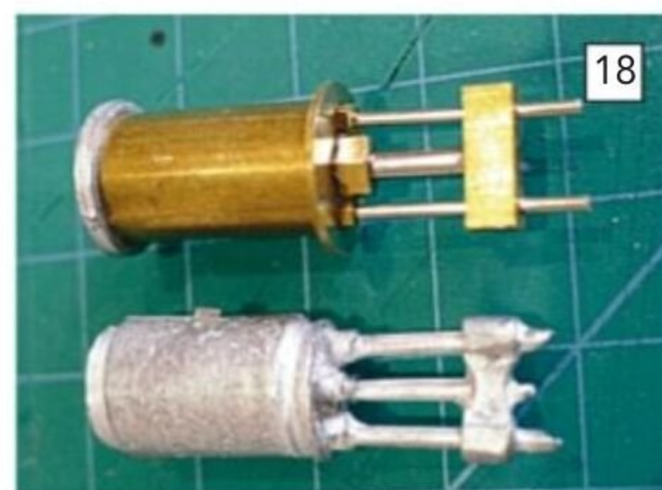
The kit-supplied cast white metal cylinder and Richard's own self-fabricated and much improved version.
