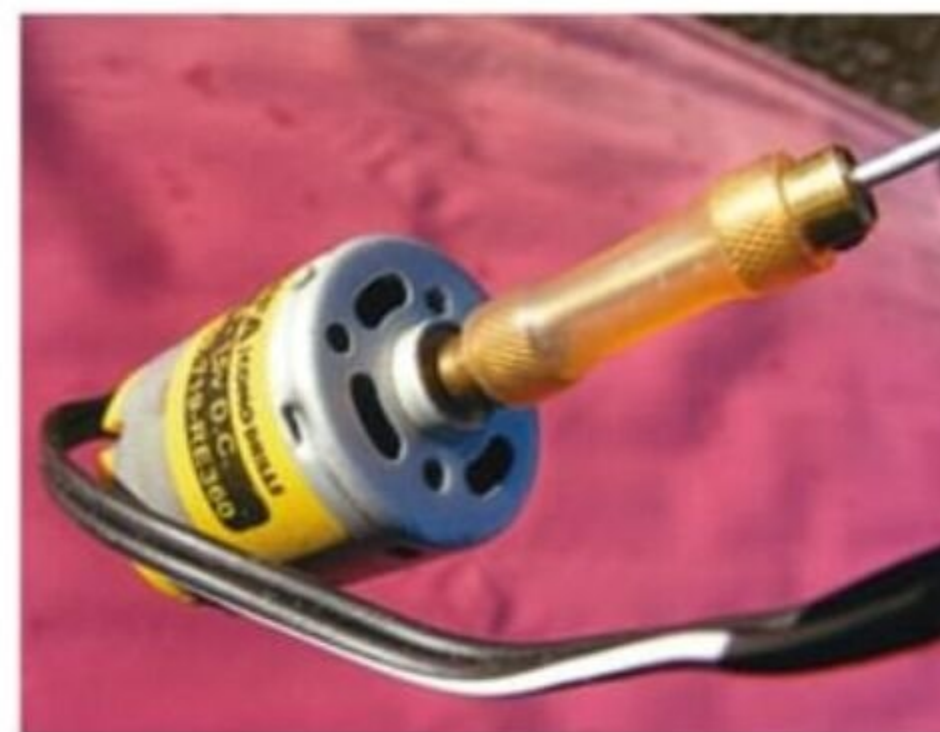
Silicone tube coupling with brass inserts.
