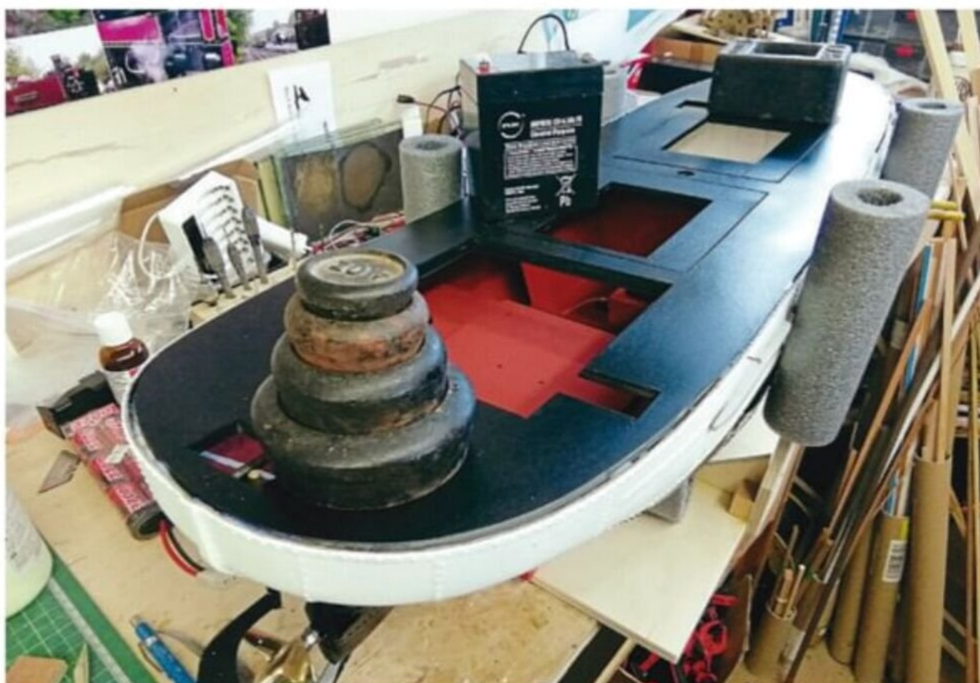
The deck, made from 6mm plywood, took some holding, down due to the curvature of the hull, while the glue set. It was painted black so it would better represent the caulking once the planking was added.
