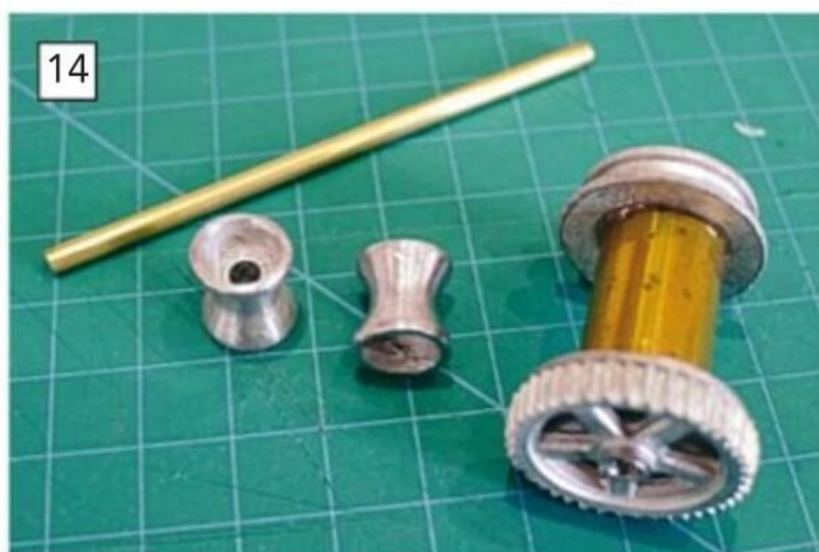
The plastic winch drum was replaced with another section of brass tube and the cross members were all created by repurposing various pieces of brass pipe and tube. The warping ends were dressed up but, by the time the finish was good enough, too much metal had been removed.
