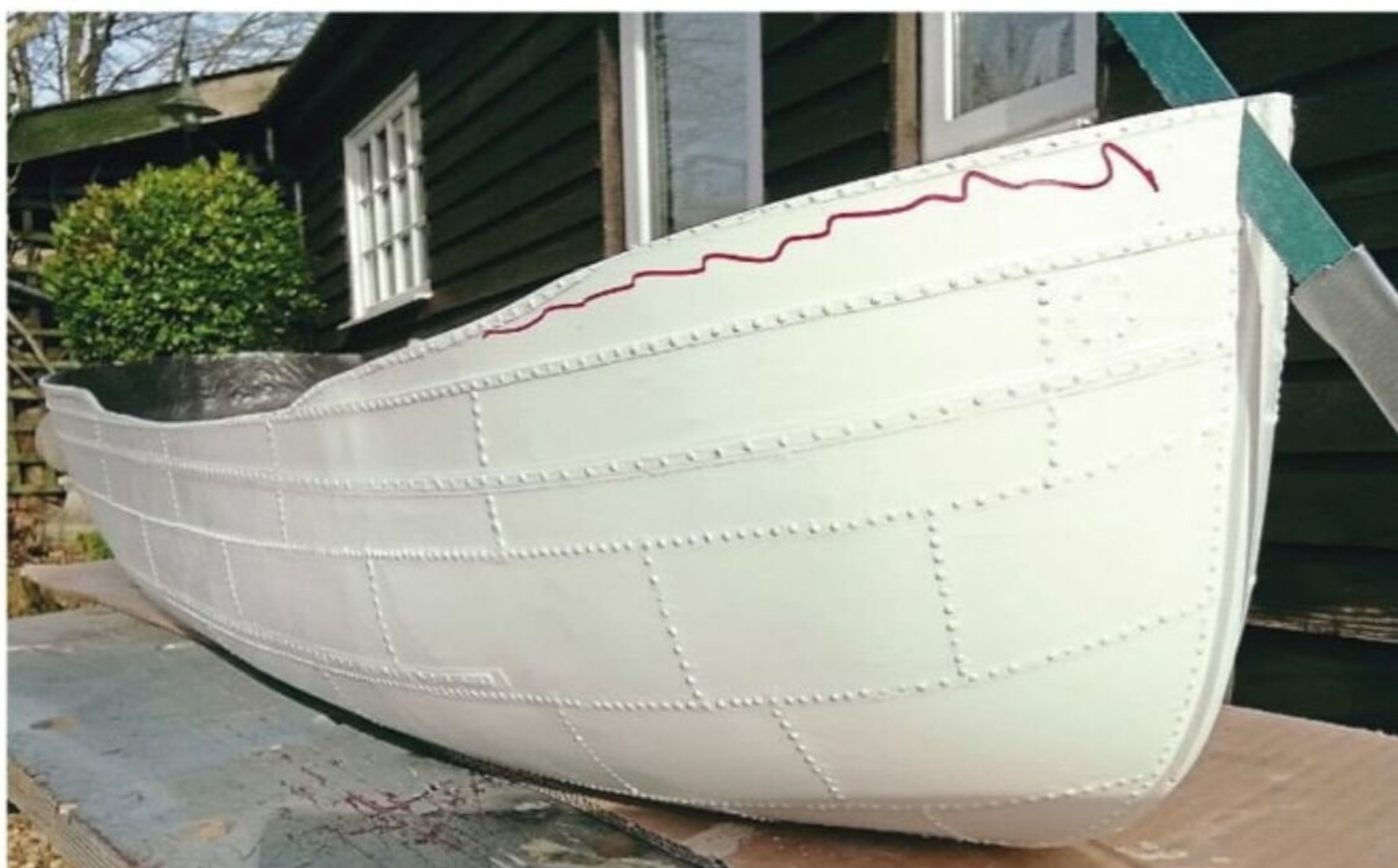
Orion Mouldings' superb Clyde Puffer fibreglass hull was drastically altered by removing the bulwarks at the bow and stern. This was carried out using a hacksaw blade.
