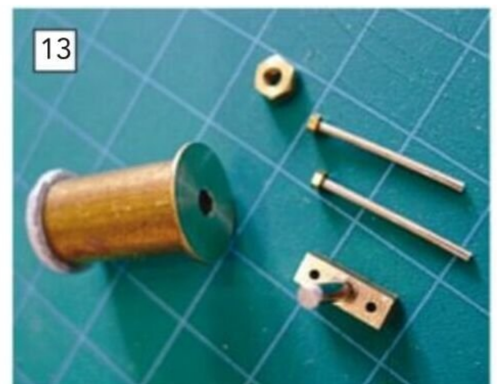
Identifying the best metal spare to use can often be identified by the shape of what you're trying to reproduce. Frequently there is little more than a bit of cutting and drilling required. The lathe makes square cutting tube very easy.
