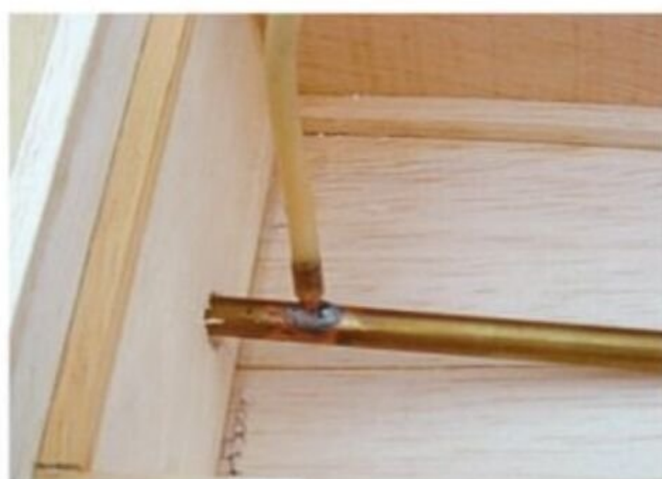
A prop tube oiler with flexible extension tube.
