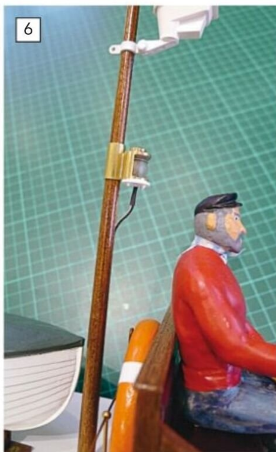
Brass tube can be used to make your own mast fittings and soft soldering the parts together makes for a good, strong fitting. The base and the nuts are plastic, just for a scale effect.
