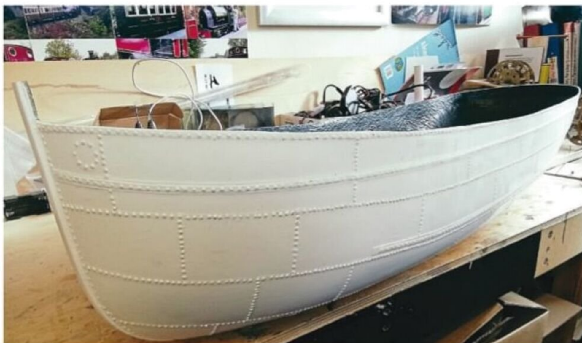
Having removed the bulwarks, the hull required further cutting back to create Raven's almost flat deck. John's 6mm plywood deck was cut but not fitted at this stage.
