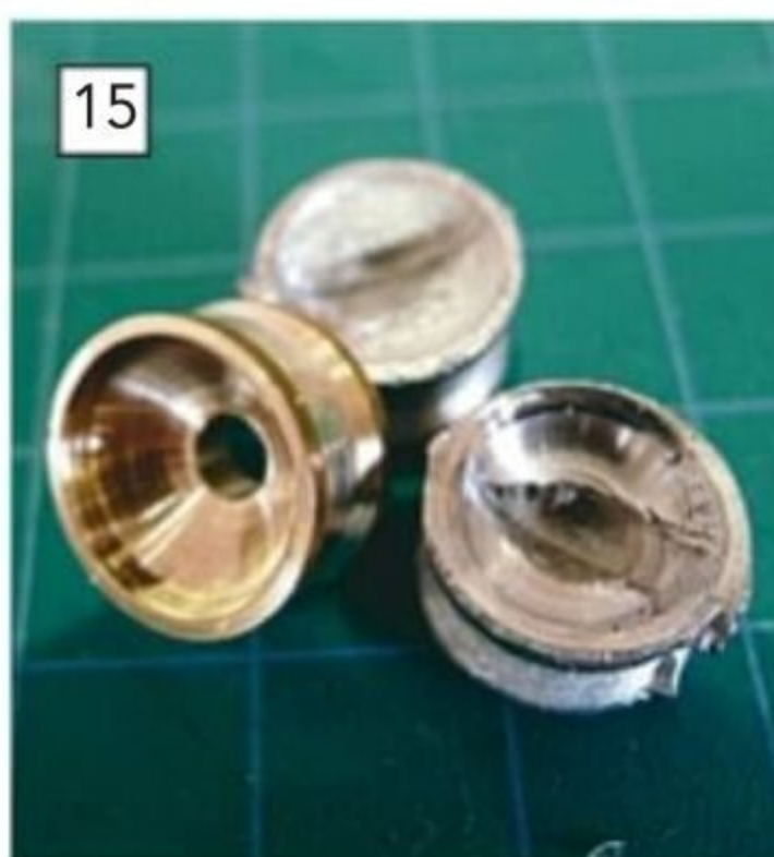
Consequently, the warping ends were made out of brass bar in the lathe; A fairly easy turning and drilling job that shouldn't take a great deal of time.
