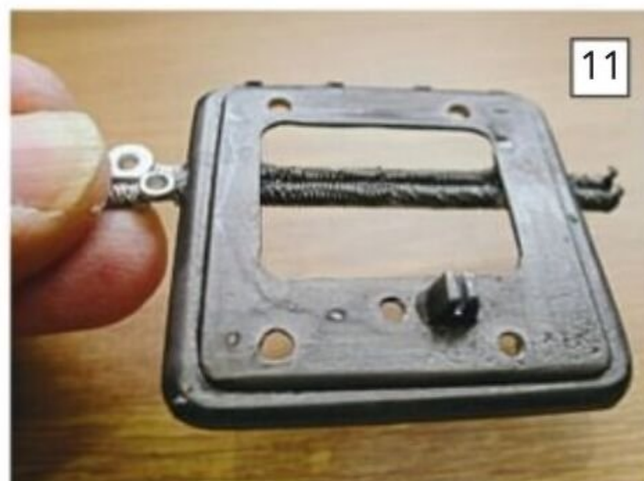
A coat of paint frequently shows up those areas that could do with improving. Richard decided to remake this part from a solid piece of aluminum plate to give a neater finish and a more regular shape.
