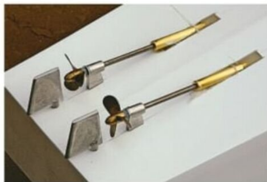
An external view of the Perkasa's running gear. In this case the thrust is taken by the substantial skegs built into the hull forward of the rudders.
