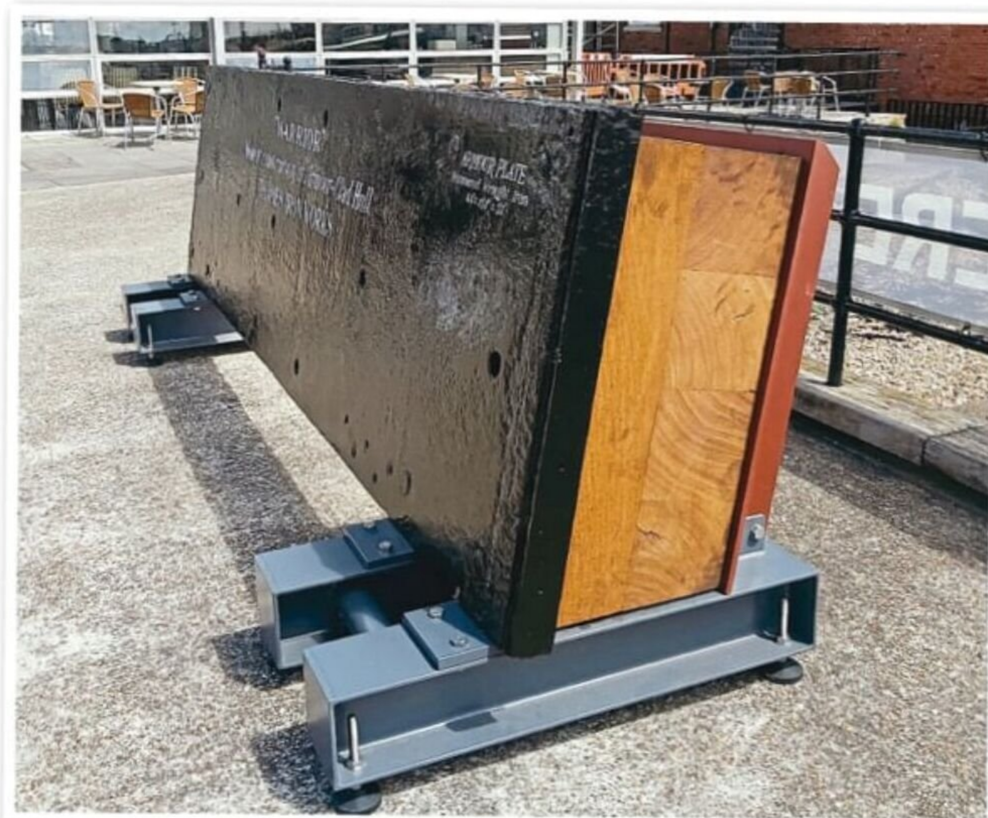
A section of Warrior's armour plating, showing the 18 inches of teak backing the 4½ inches of wrought iron. All of this overlies the ship's inner iron plating.
