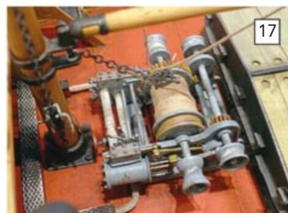
Some painting and weathering used alongside real metal finishes, some scale rope wrapped around the drum, and the fabrication of steam pipes from copper tube wrapped in cord insulation, all serve to make things look very life-like.
