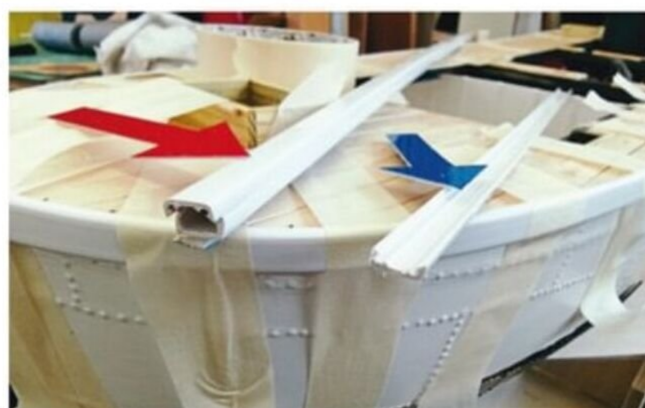
In the foreground the frame for the skylight, made from various brass sections silver and soft soldered together, can be seen. Behind this are some of the ladders that permitted access to the hold and engine room.
