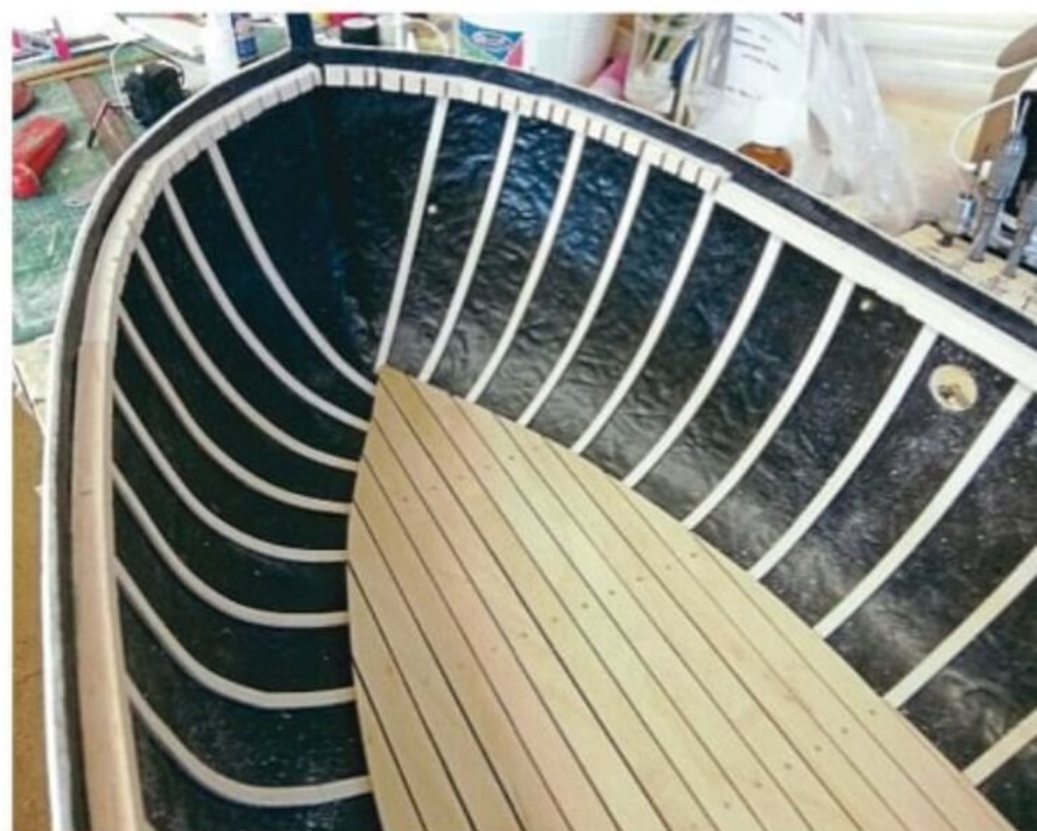
The bow section of the hold showing the 'mock' ribs in place. Both these and the decking were cut from plywood.
