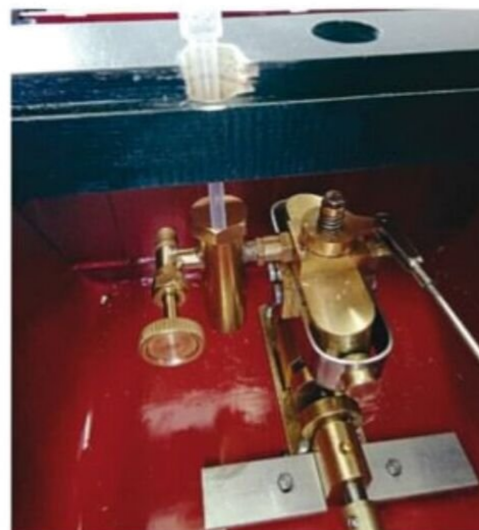
To remedy the problem with access, a hole was bored through the beam. Note the plastic syringe going through the hole and lining up with the oiler.
