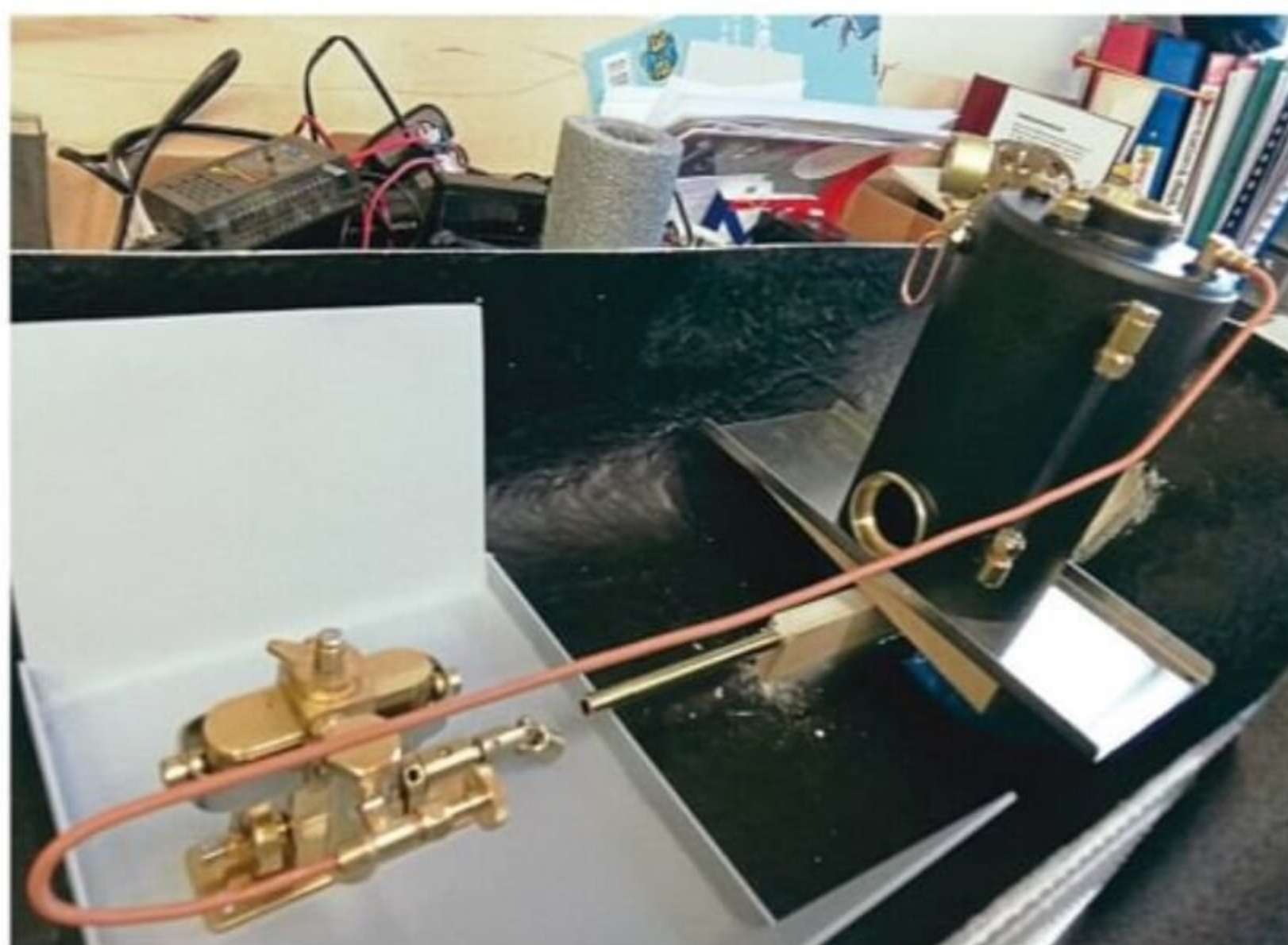
The trial setup to establish the position of the boiler and engine. The 14-inch prop shaft is located beneath the boiler.
