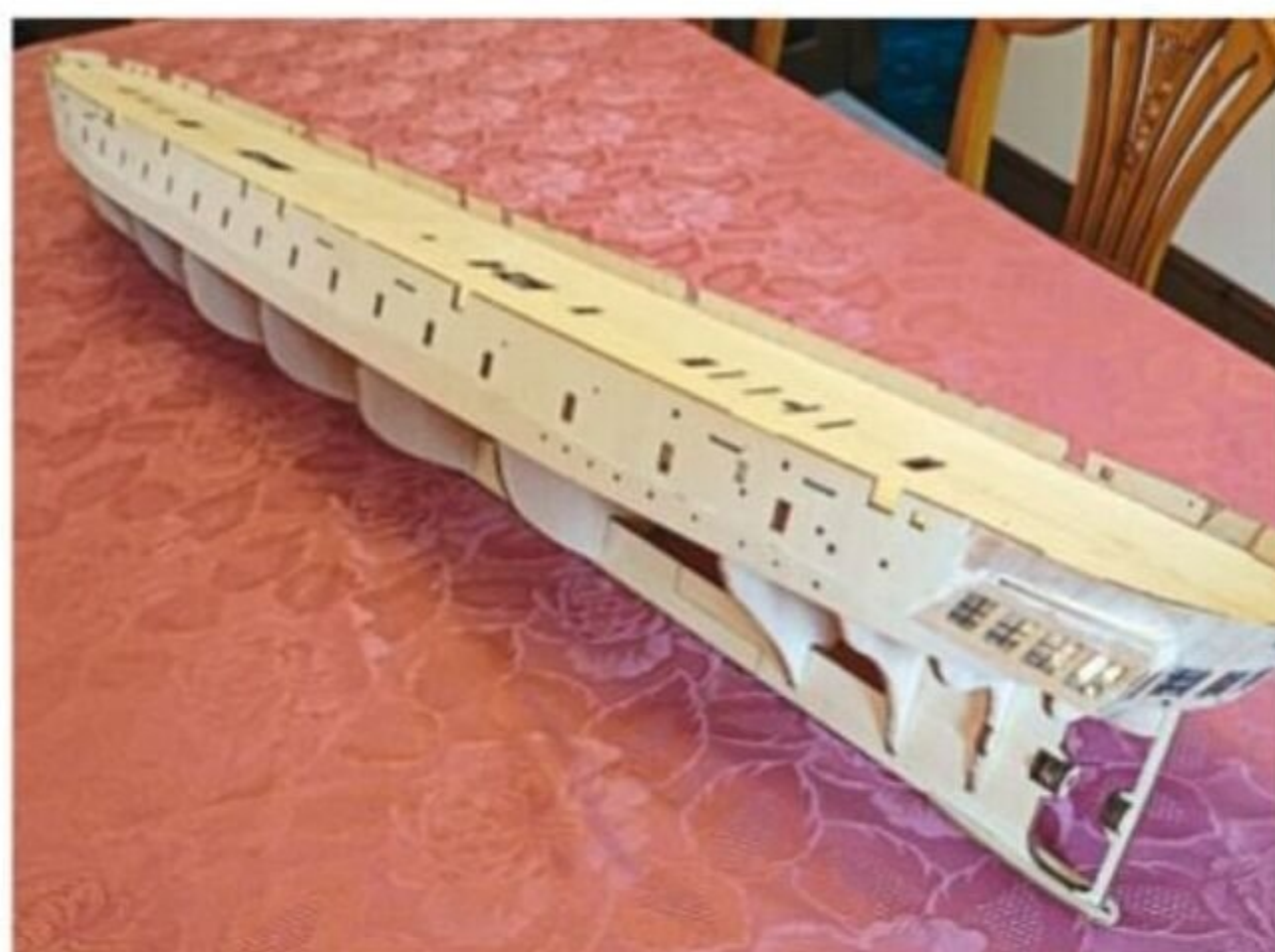
The deck ply substrate is in position at this point.
