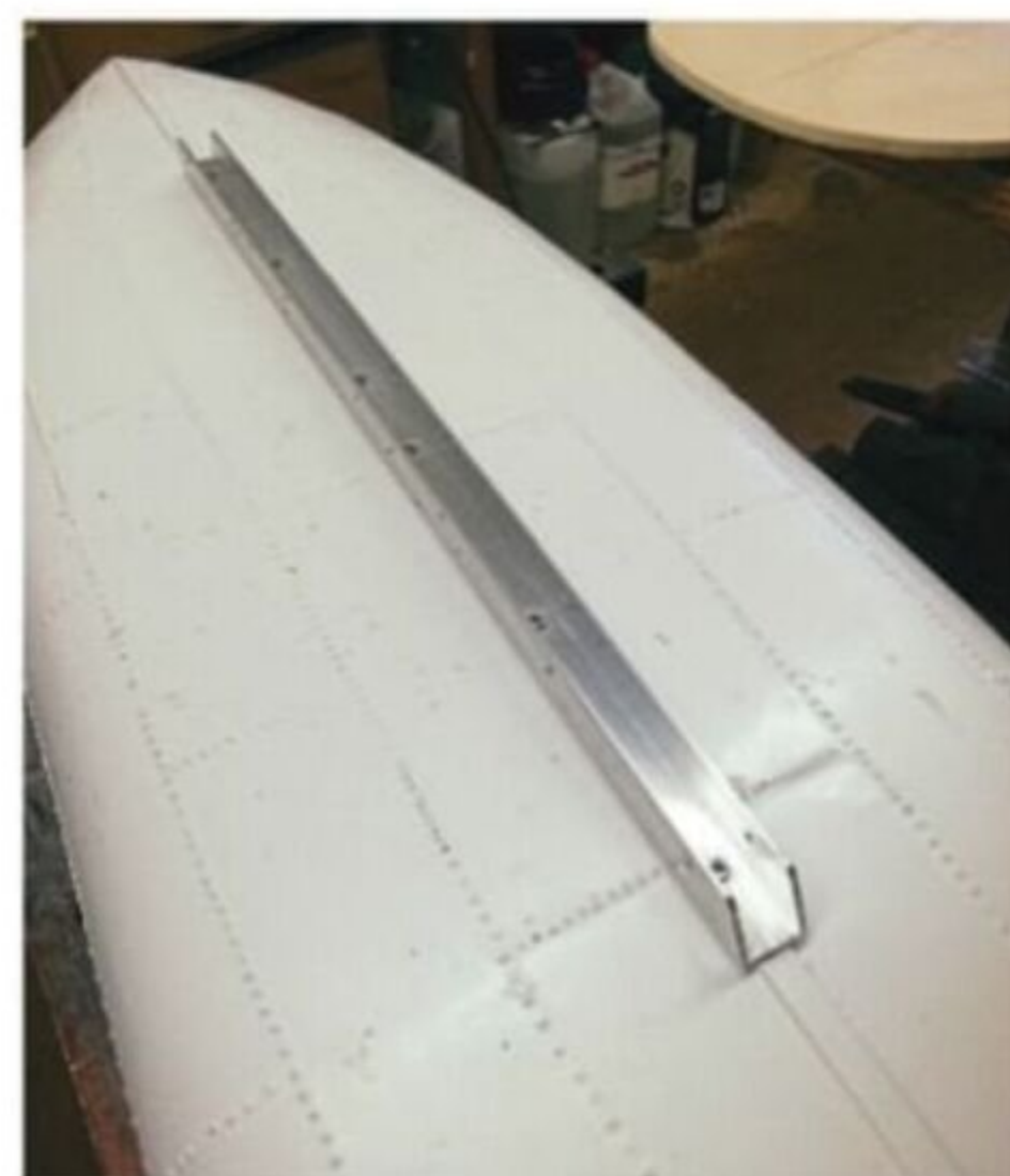
A keel was to be fitted to the hull. To this end, an aluminium channel was screwed to the underside of the hull. Into this a plastic keel could be slotted.
