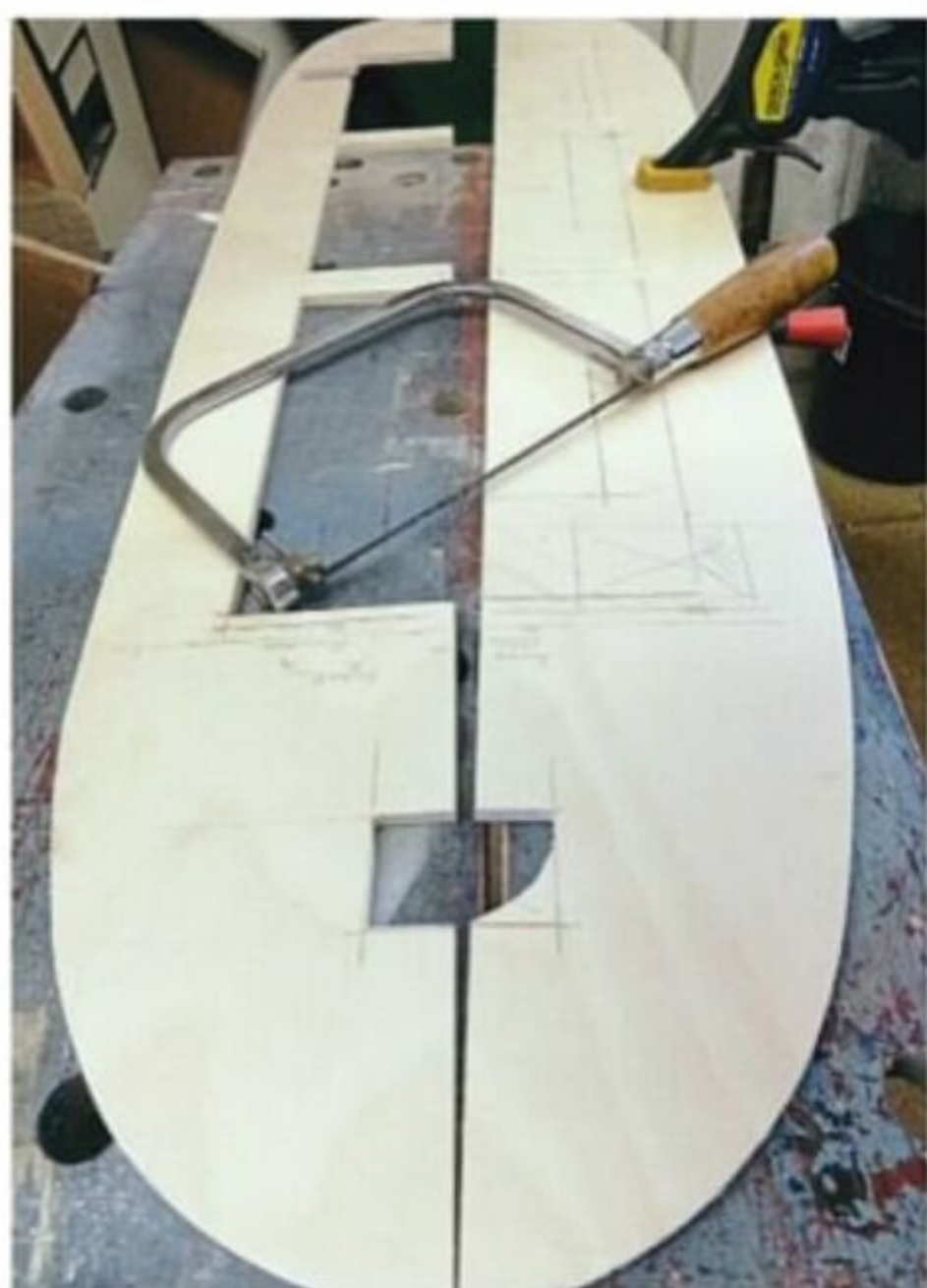
The deck, due to its size, was made in two halves. This involved a fair amount of work with a coping saw as it was too wide to fit onto John's bandsaw.
