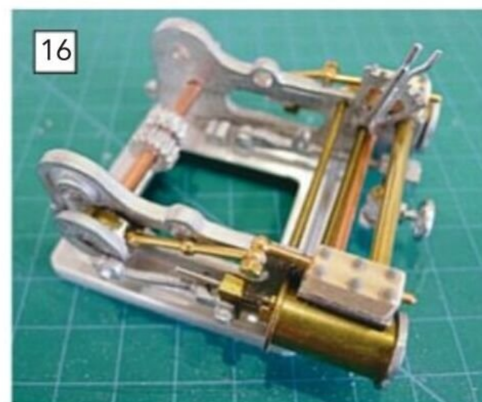
With a wooden valve chest, valve rods and cranks made from brass, BA brass nuts and bolts for crank pins, and plastic nuts on the valve chest, the cargo winch is looking much more realistic.
