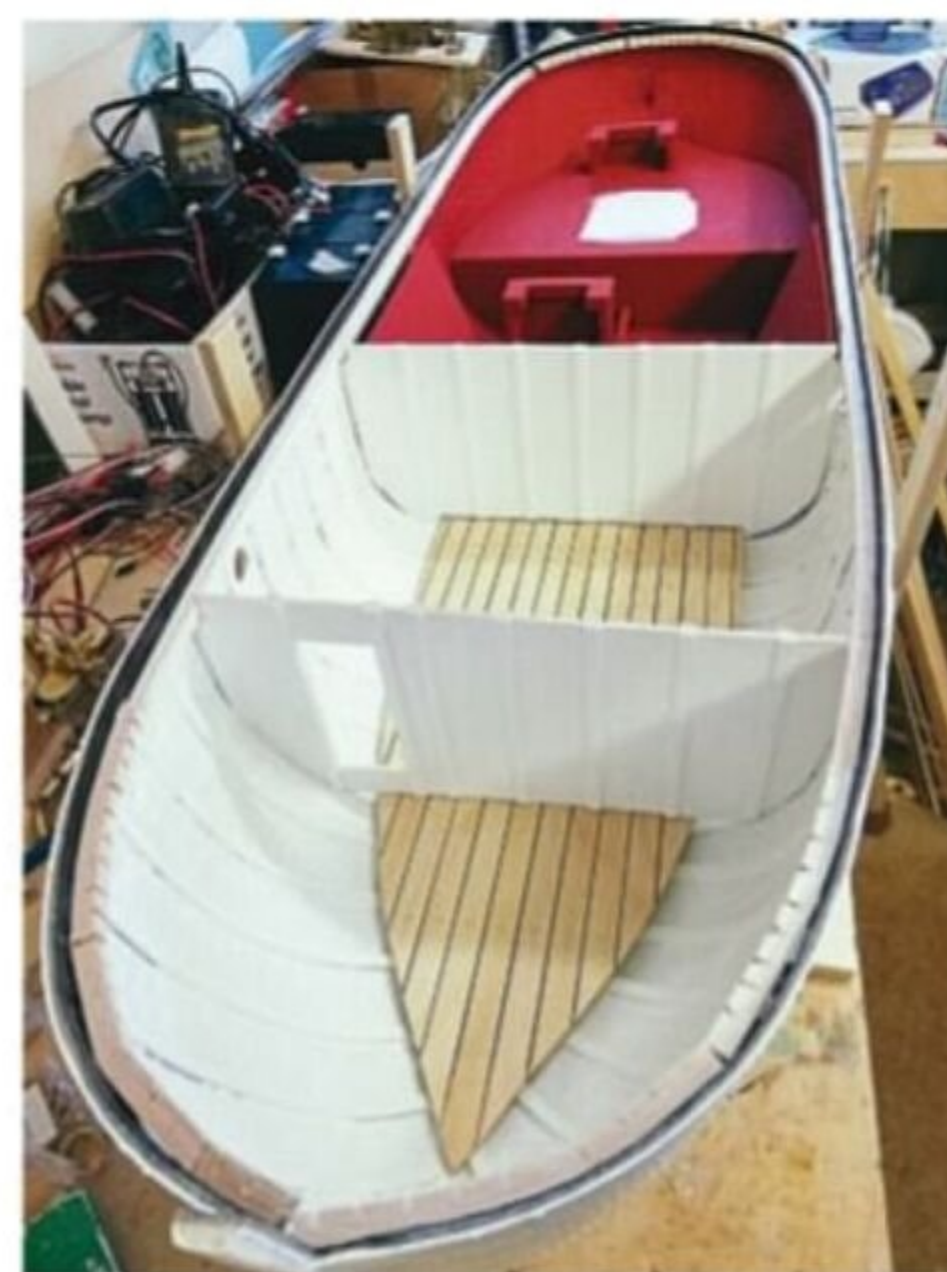
The interior of the hull virtually complete. The model's hold is considerably smaller than that of the full-sized vessel due to the fact that the engine will be located forward.
