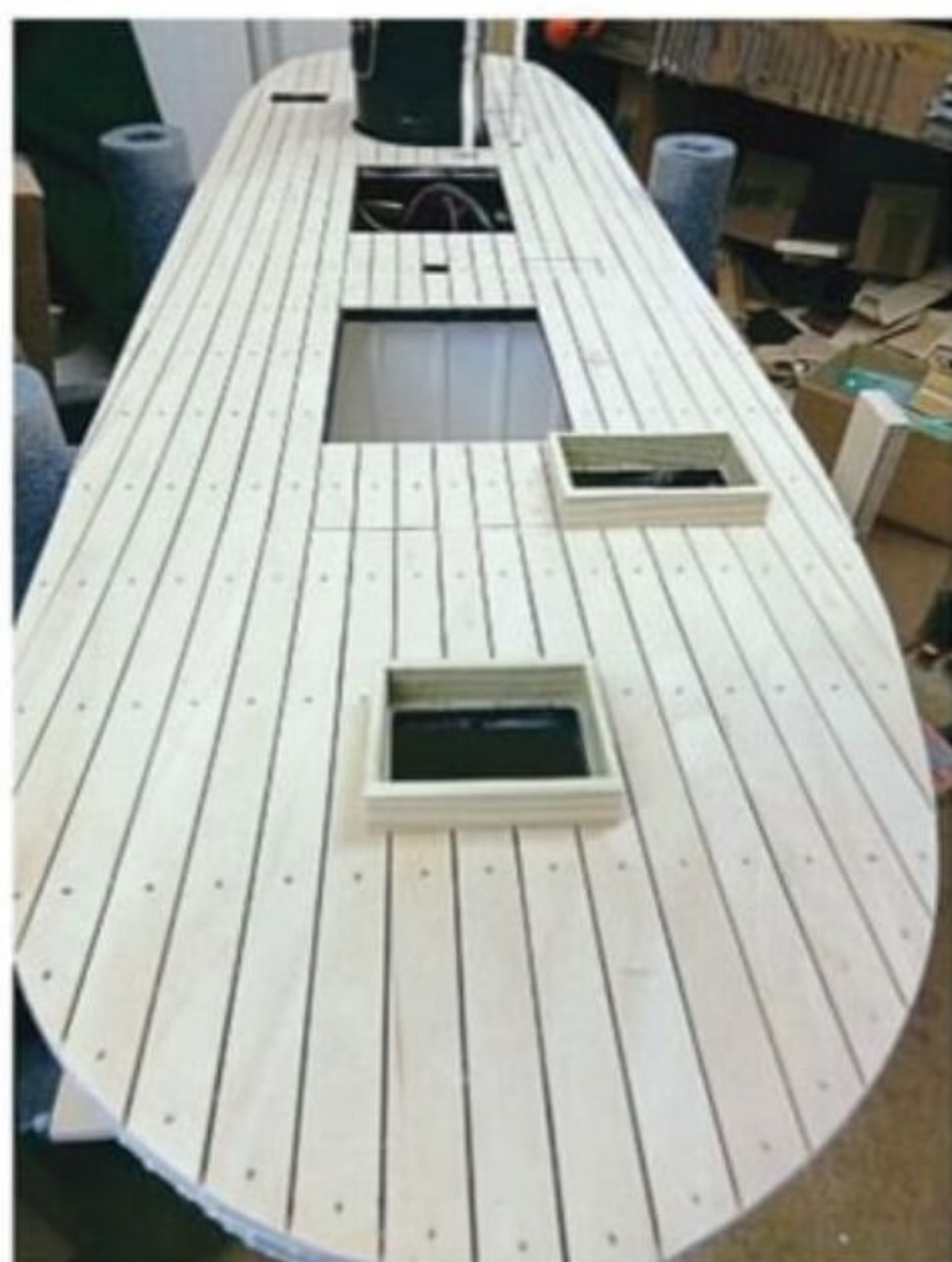
The deck planking complete. A gap of approximately 1mm was left between each plank, which allowed the black paint to show through, representing the caulking.
