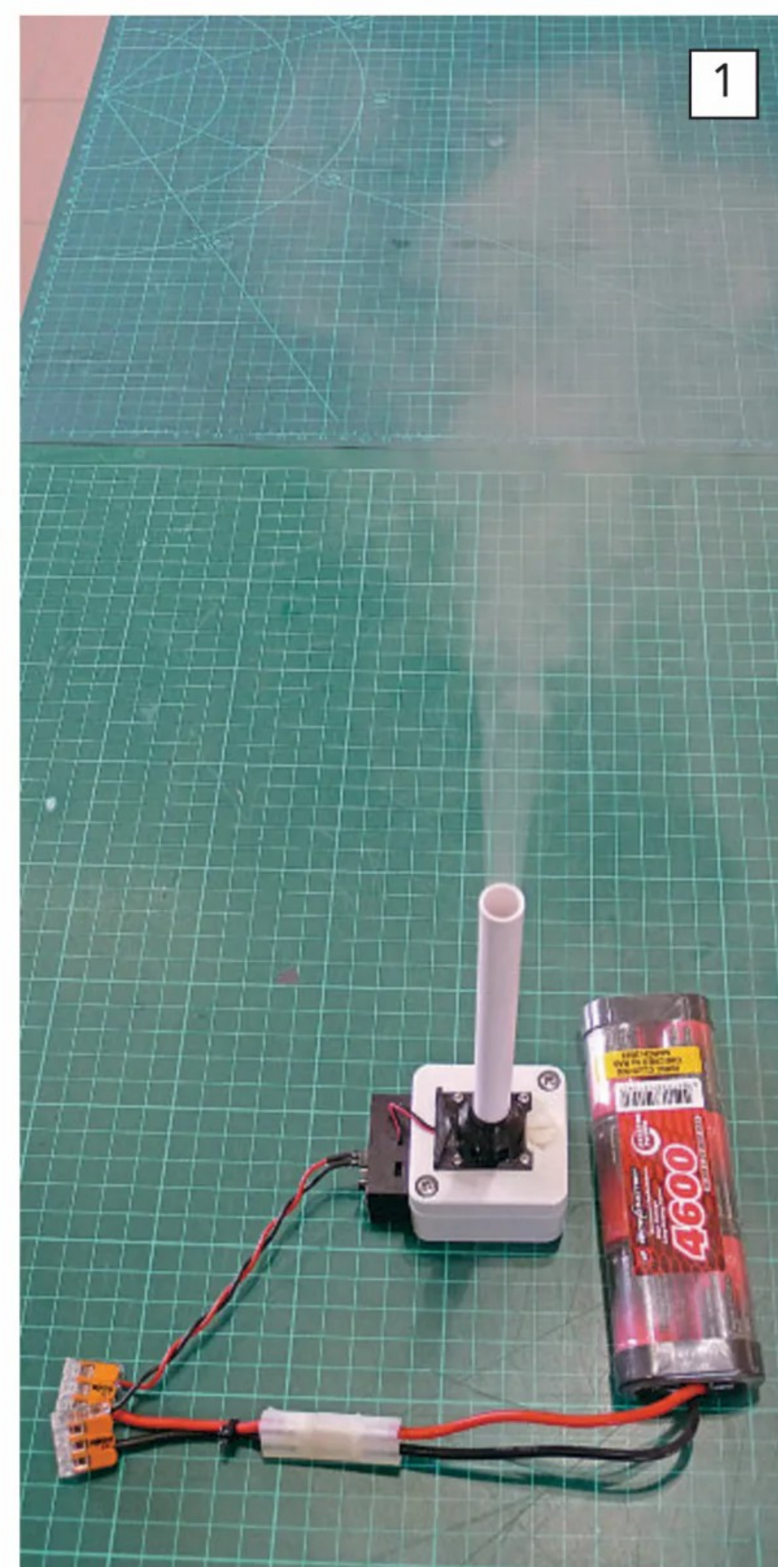
A new take on the nebuliser. Instead of a large unit submerged in the water reservoir, this vapour generator uses a small unit at the base of the funnel, fed from a wick below it.
