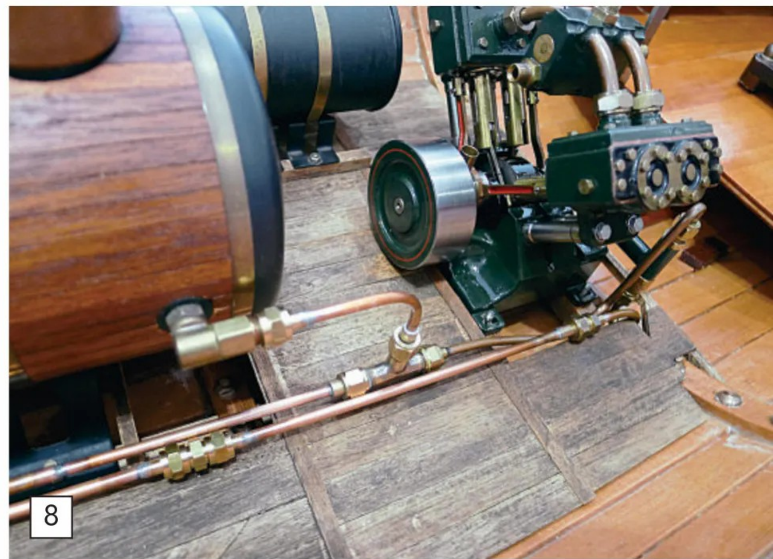
An engine driven pump can be neat and compact and, contrary to what some believe, doesn't actually use a lot of engine power.
