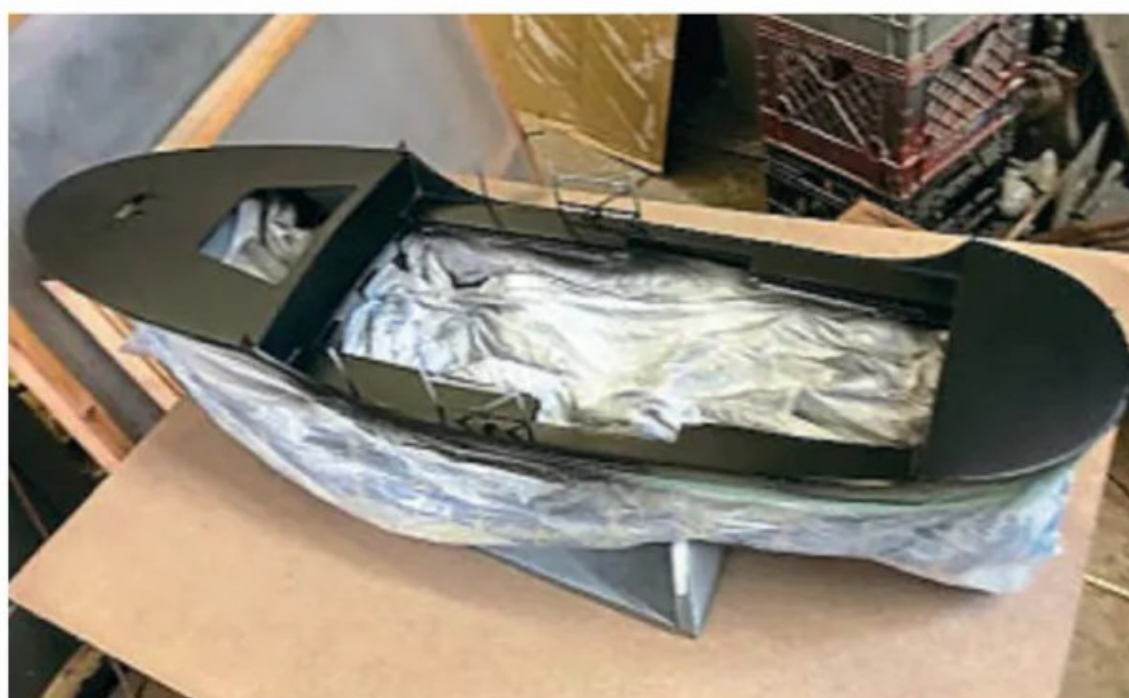
Painting in stages makes the process much easier. Here the deck is painted after careful masking and before fittings are installed.
