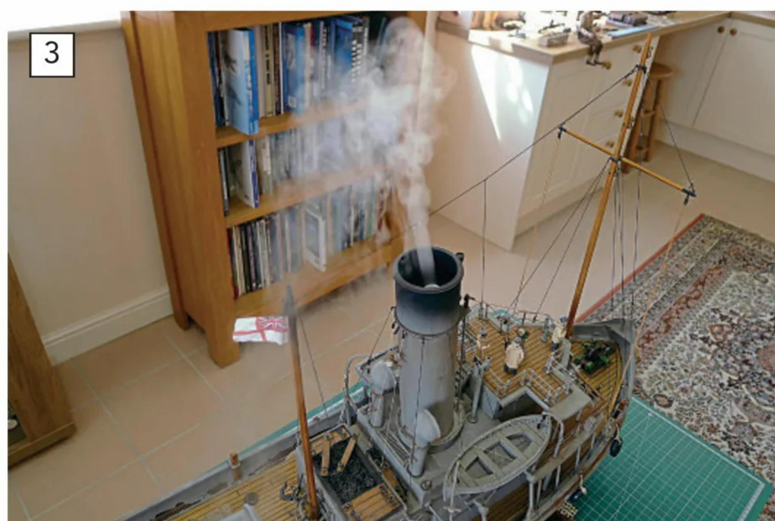
The vapour generated looked adequate for the scale of Richard's tug and followed the control of the main motor perfectly. Density and pulse rate are both adjustable.
