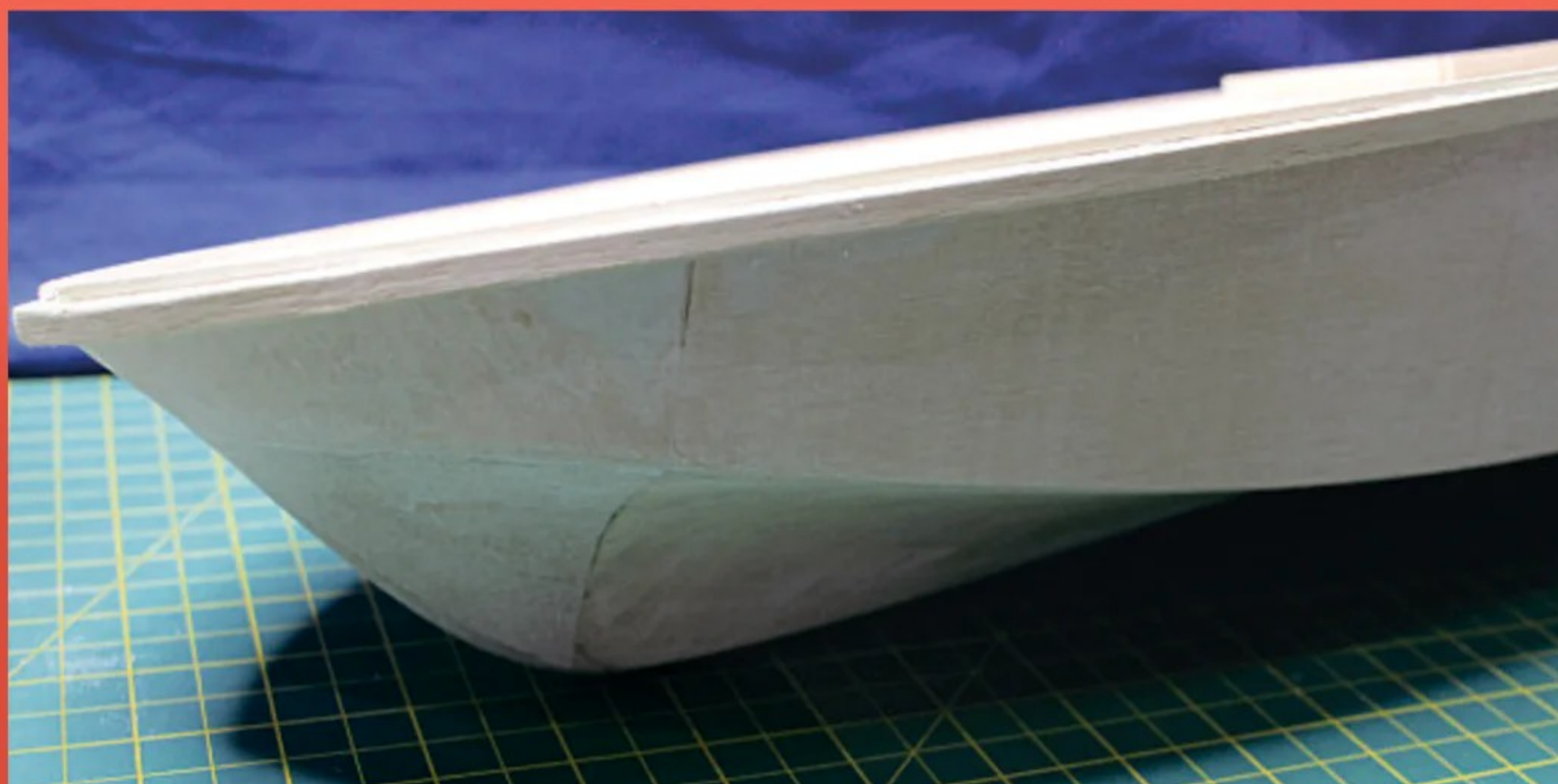
And now the completed bow. Doesn't look like anything special but that's the point! The entire hull has been coated in a layer of lightweight fibreglass cloth.
