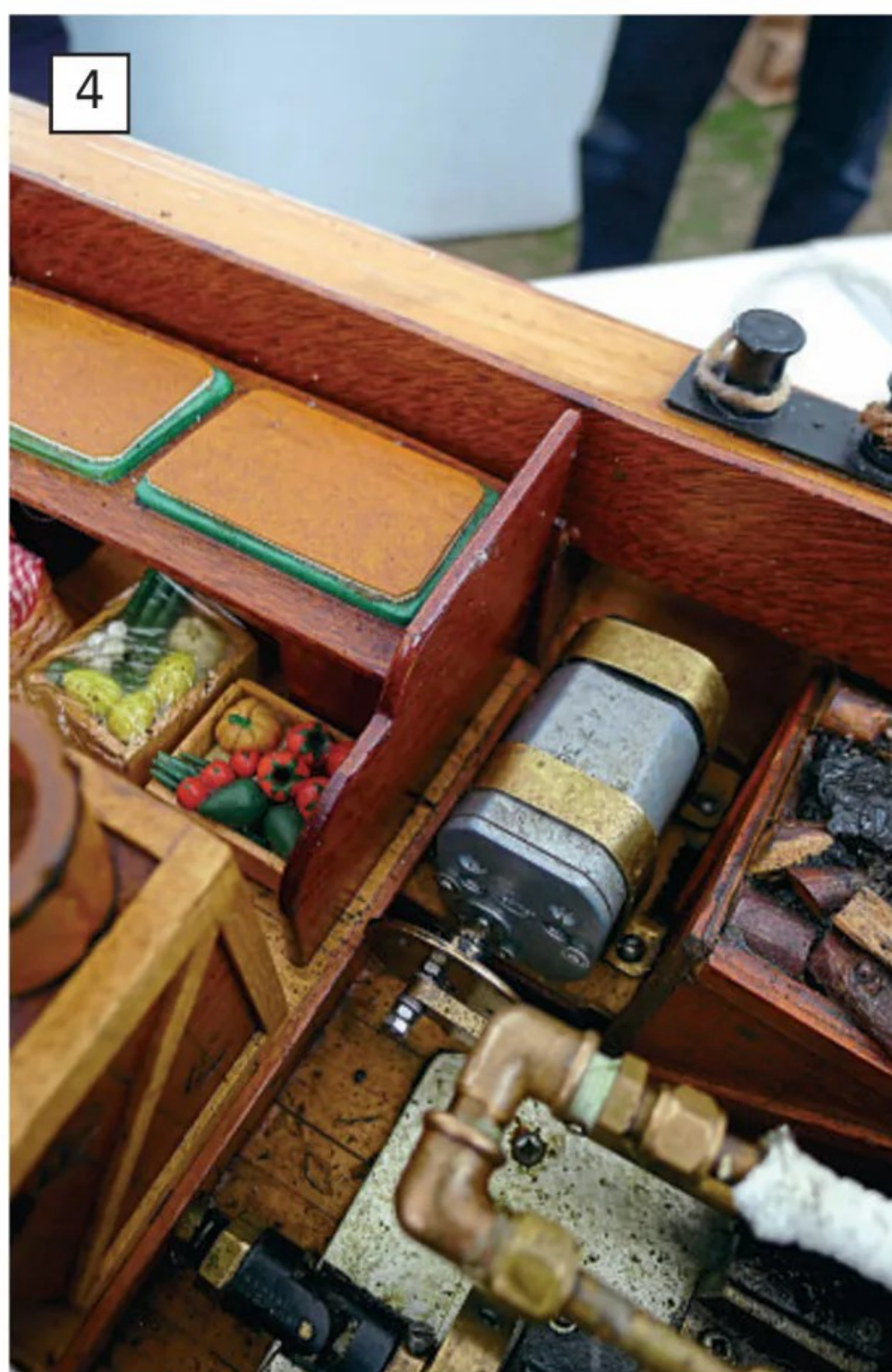
A motor and built-in gearbox can also be used to drive a piston pump via a simple disc crank.
