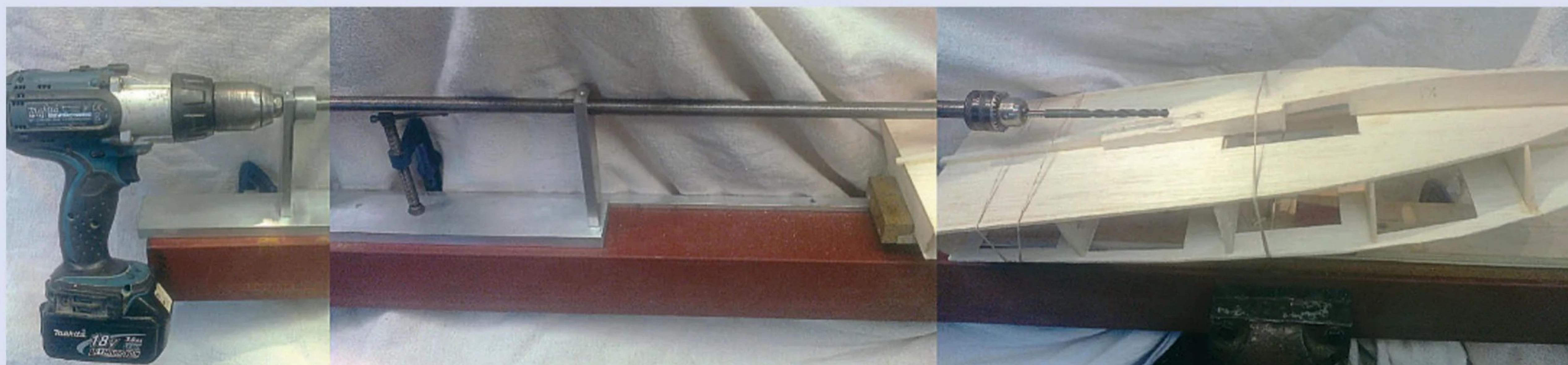
The ingenious solution Mike Joseph came up with for fearlessly drilling a prop shaft hole.
