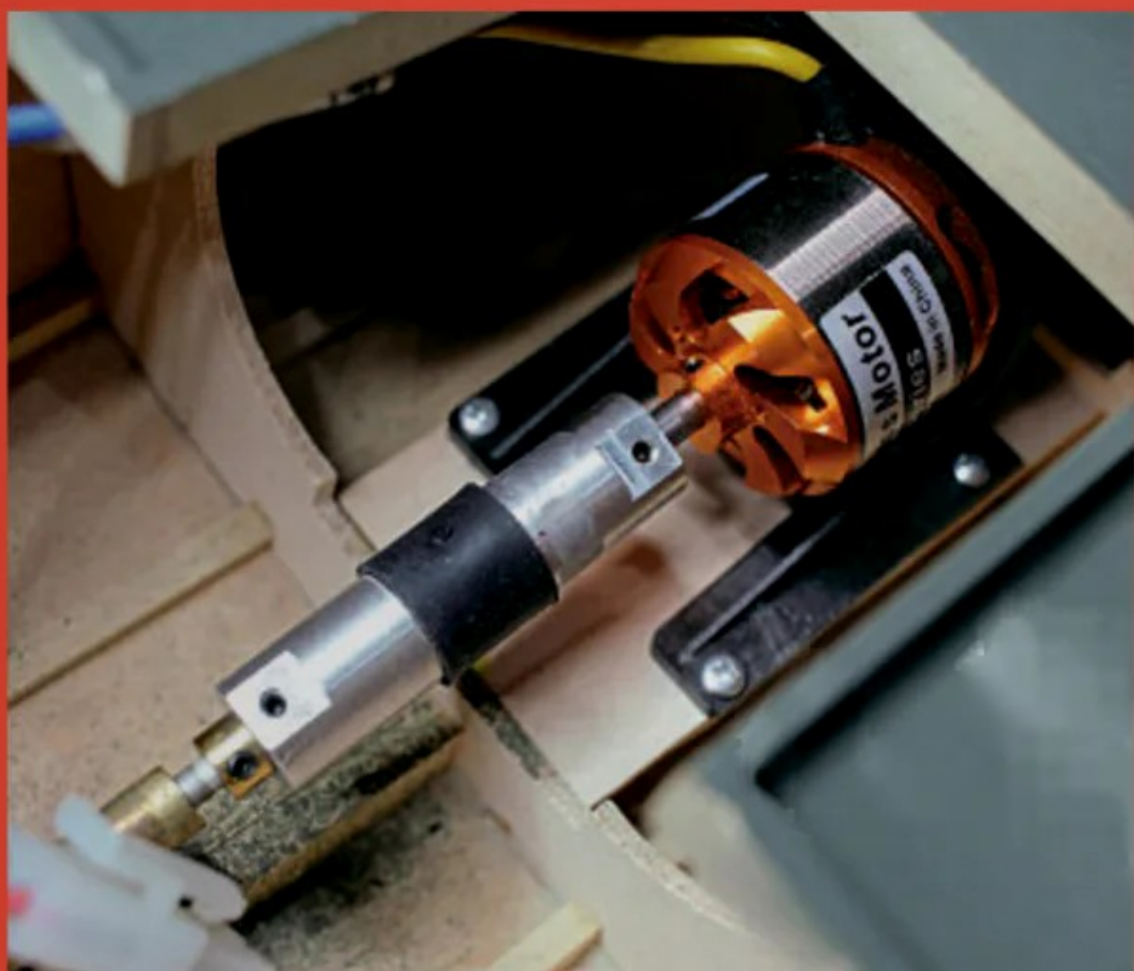
The brushless motor supplied by SLEC; this is more than powerful enough to propel this beauty through the water.
