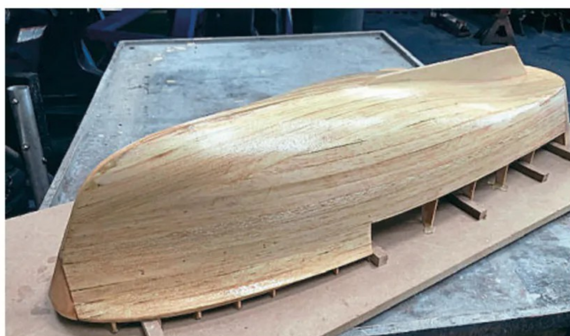
Planking completely smooth and ready for fibreglassing. Eliminating all flaws before applying the cloth and resin is essential.
