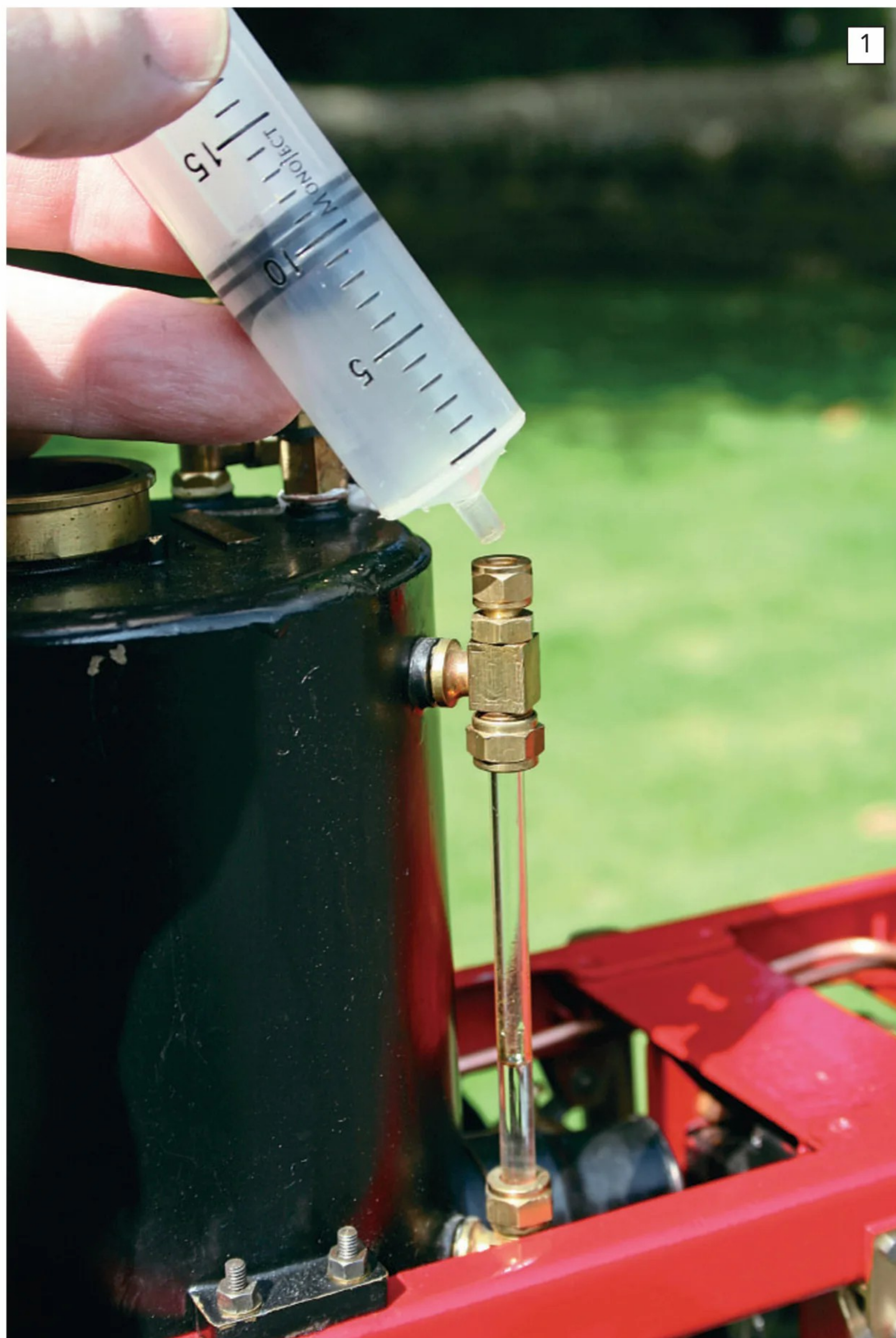
Simple but surprisingly effective: a syringe held against the nitrile ball and some water is injected. This takes a bit of practice, and you will get spat at a few times, so, Richard points out, you should wear gloves.
