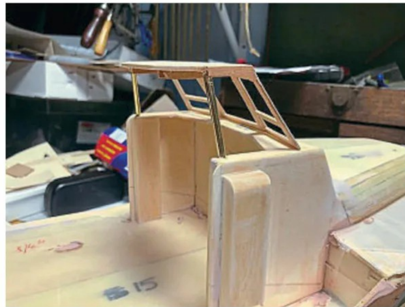
Wheelhouse window framing was scratch built to create a cabin strong enough to be lifted by the frame.
