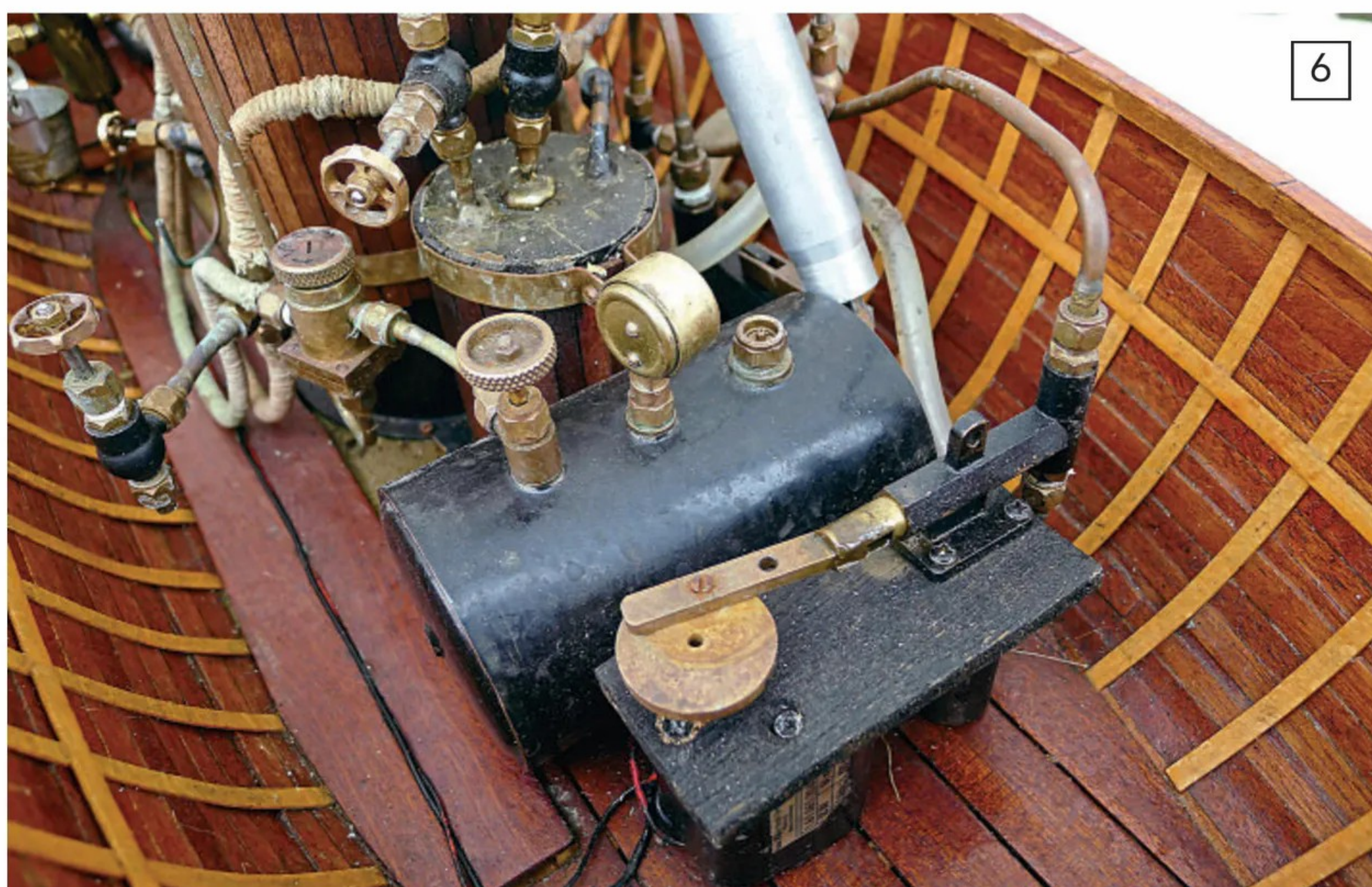
Another similar arrangement, again using a servo but with a disc crank. Using the servo motor makes speed control very convenient.
