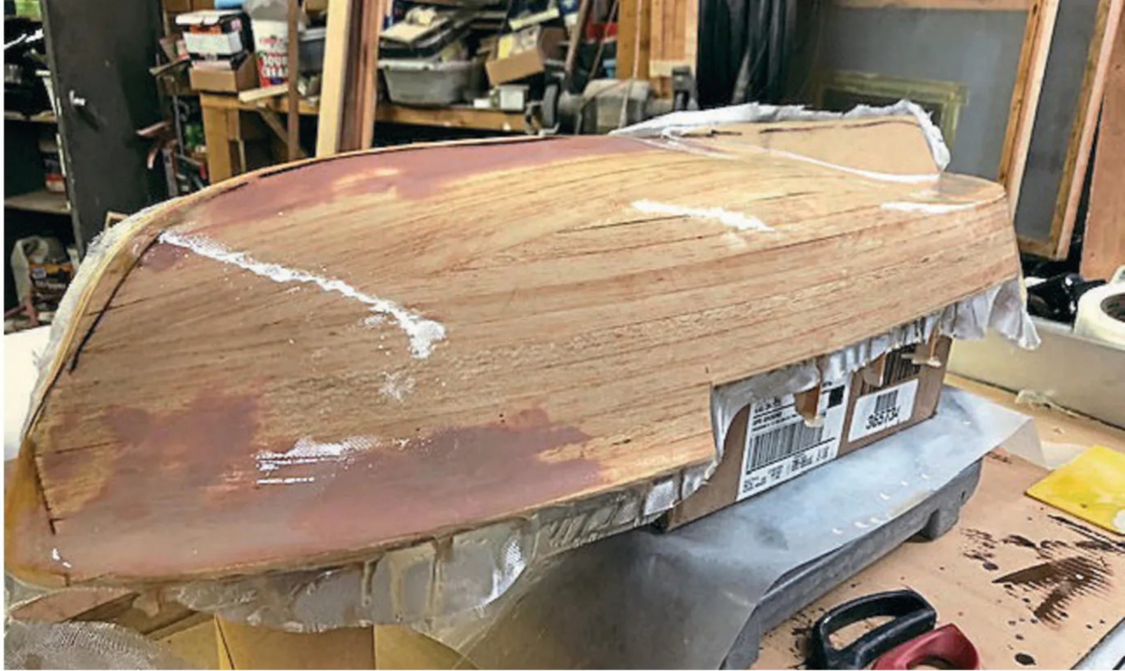
Fibreglass work completed, with no drips or runs. The hull is extremely durable at this stage.
