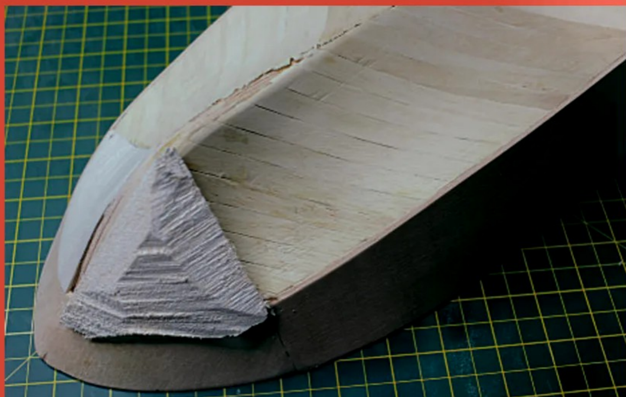
With the hull sides added it was time to create the beautiful, curved bow area using the balsa block.
