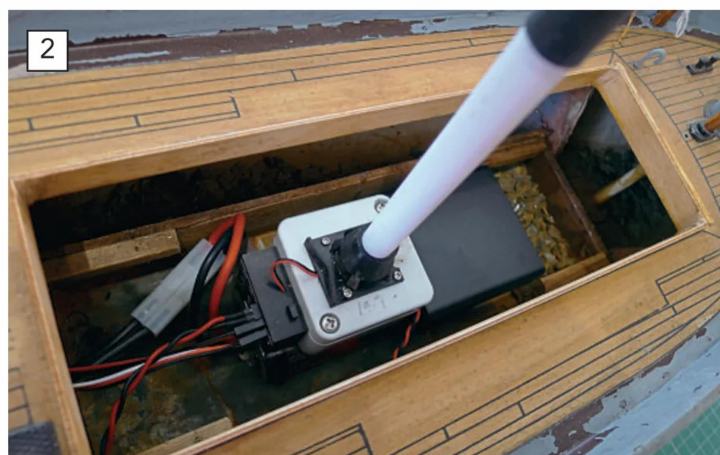
Being so much smaller, the Mini Smoker lends itself to applications where previously nebuliser units have not been suitable. This unit was simply sat on top of the main power battery with a dedicated battery next to it.
