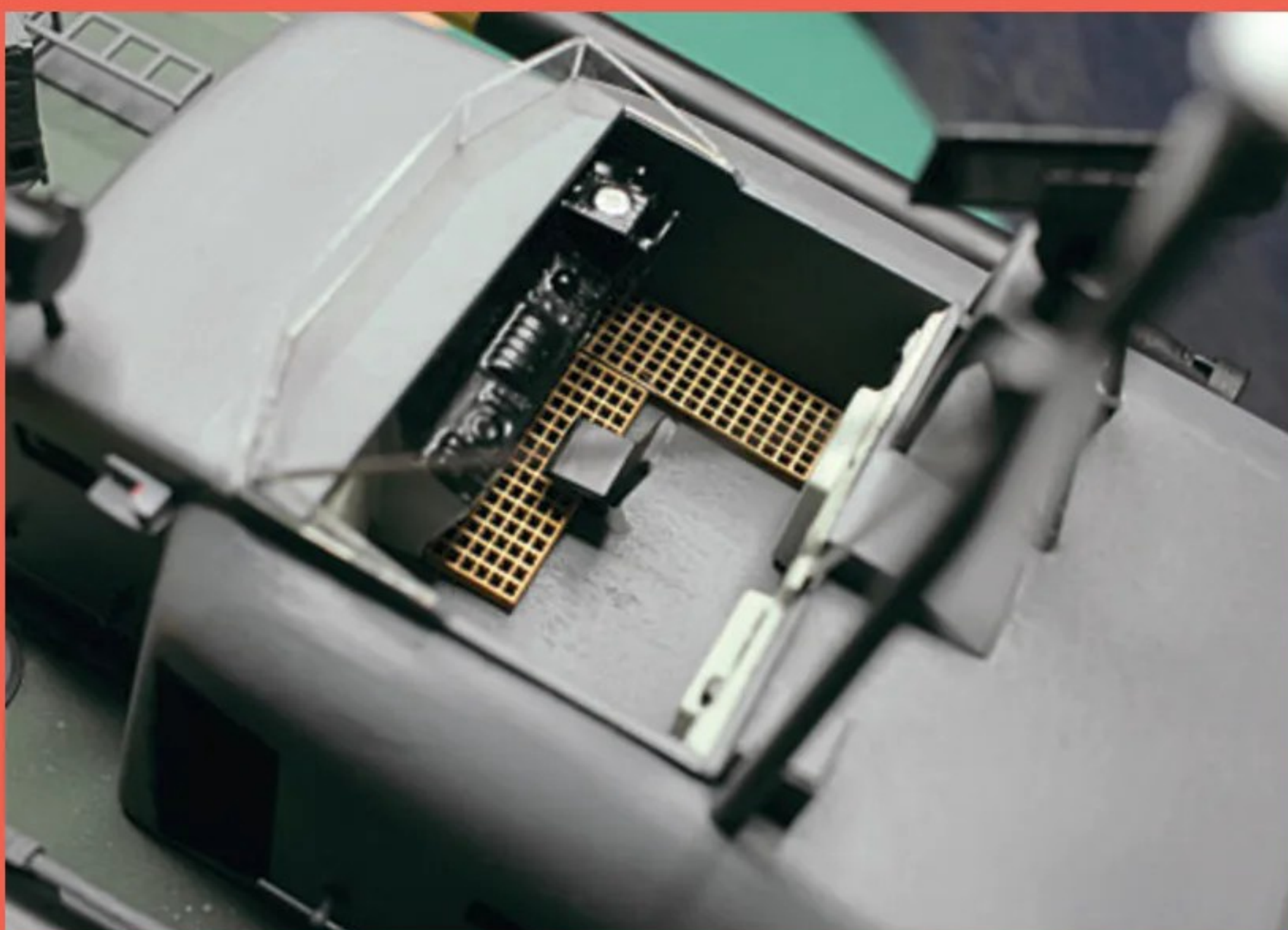
Above and left: The open bridge is suitably detailed with the vac-form console bulkheads, the floor gratings are a nice touch.
