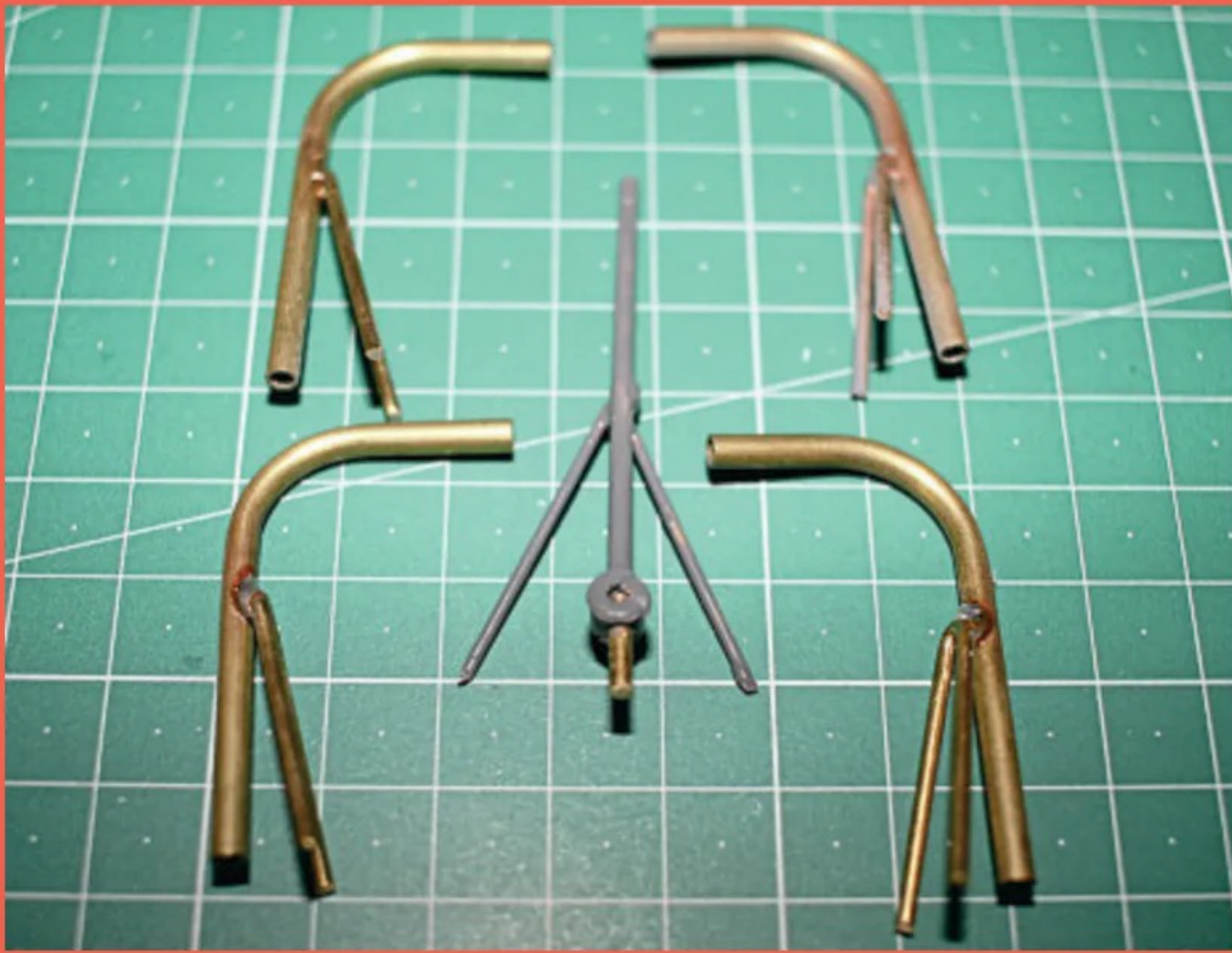
The torpedo davits are pre-curved and just need the support arms soldering to them. The jackstaff can be seen between them.
