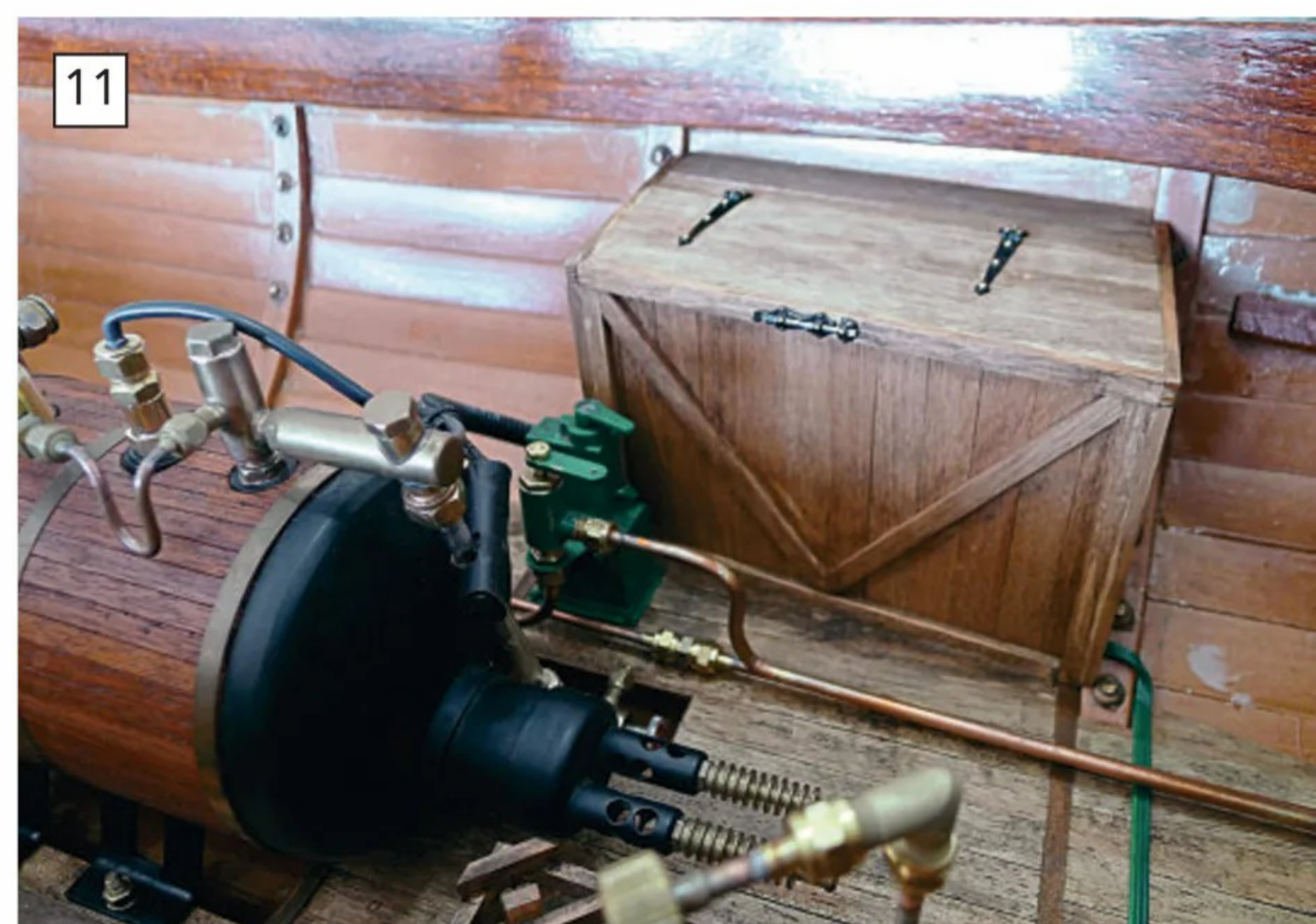
It then takes a bit of creativity to come up with a housing which allows easy access but completely disguises everything. This locker is only loosely sat in place, held by the lower frame piece, which is attached to the deck.
