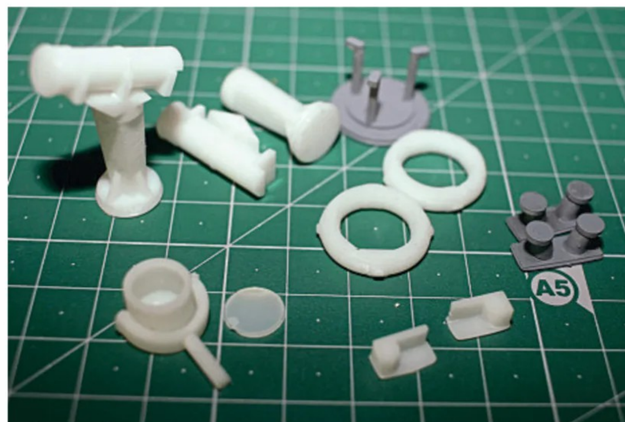
Some of the 3D printed parts provided in the kit which include the grenade launchers, life rings and searchlight.
