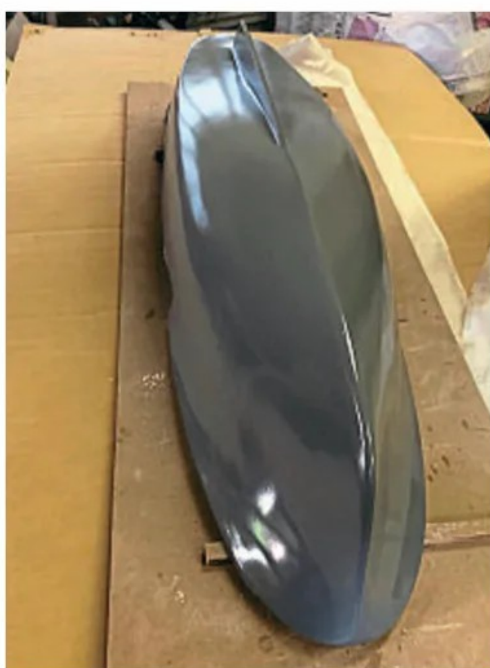
An industrial grade marine primer was used to prepare the hull for paint.
