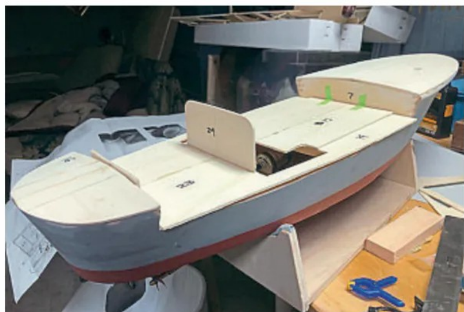
Deck pieces were fitted carefully and examined before final gluing in place.
