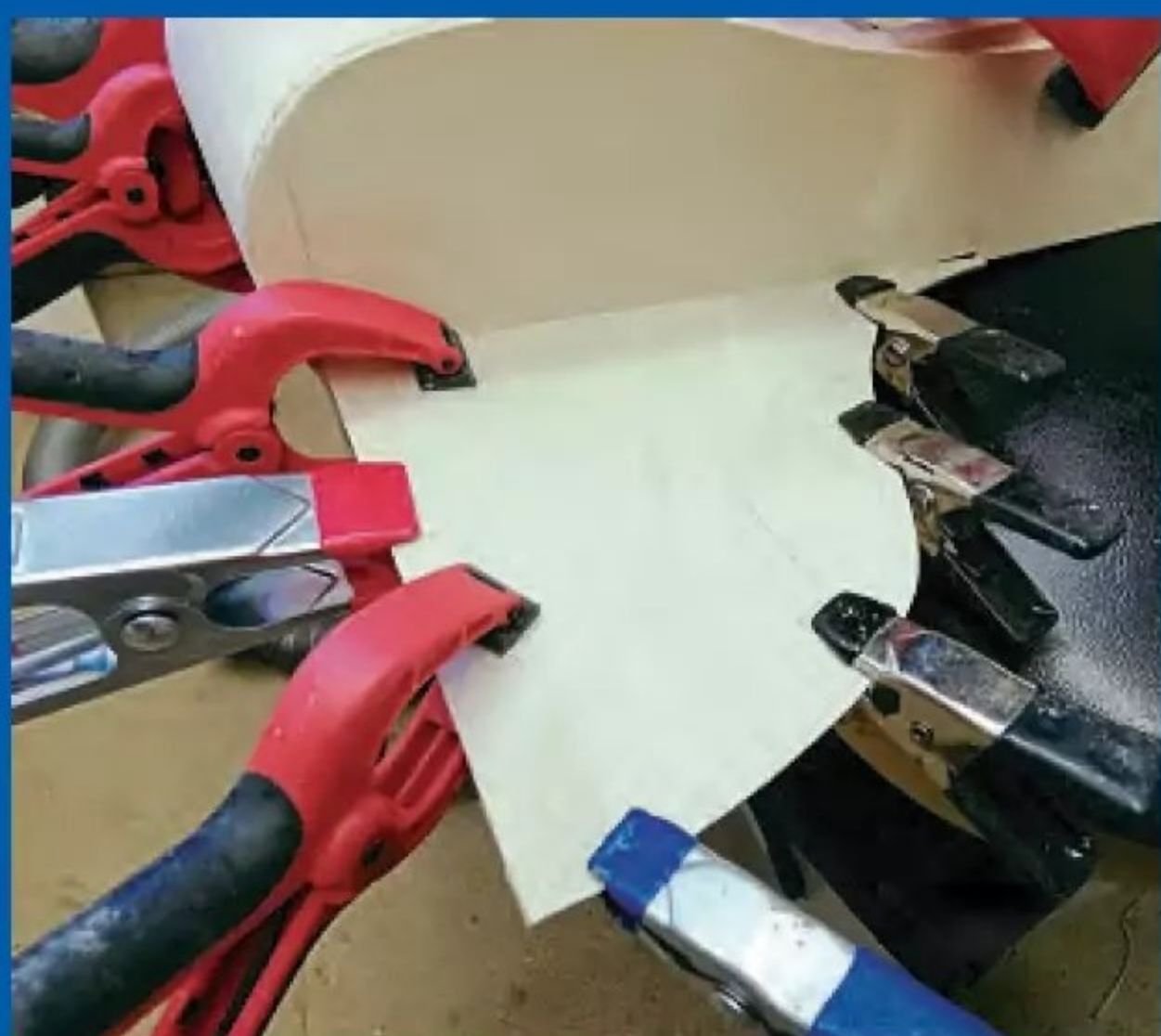
The 1mm thick outer skin being attached to the rear wing.
