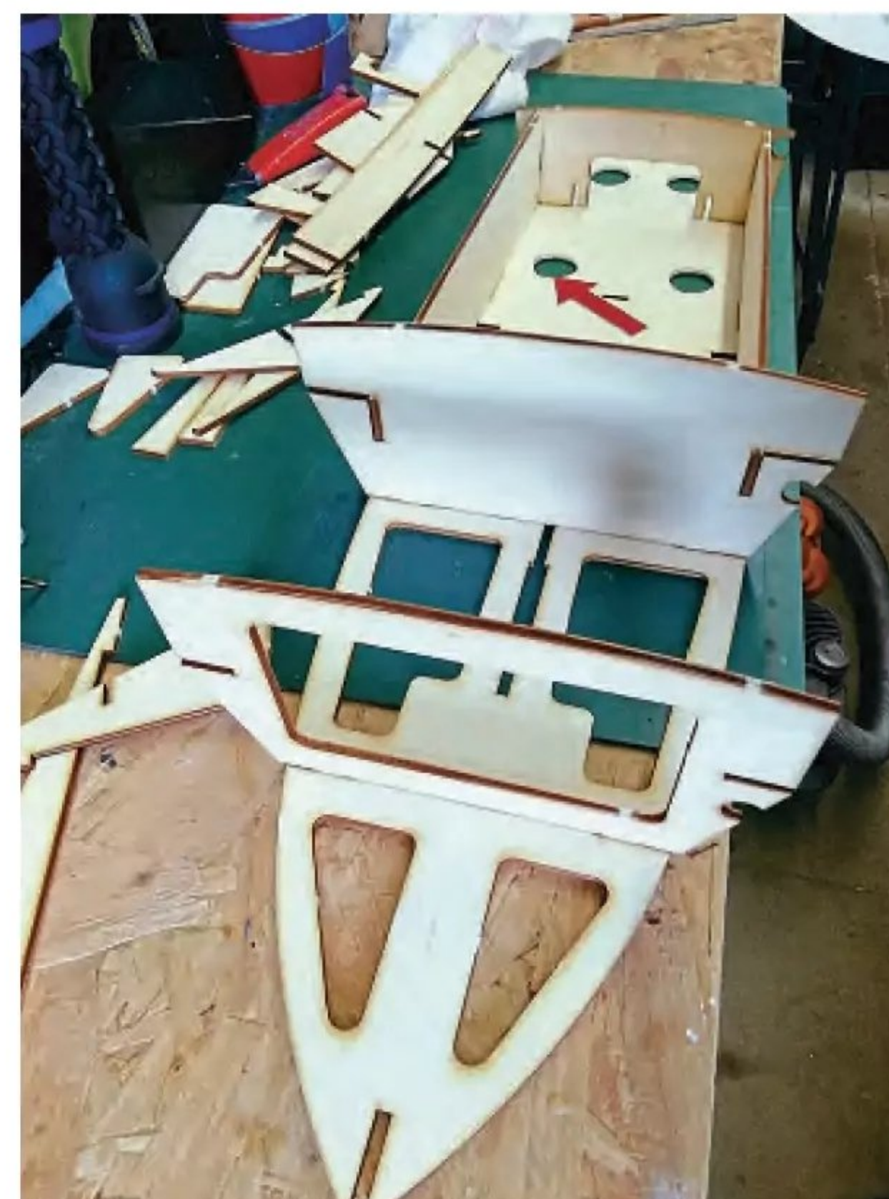
The construction is very basic, following the usual sequence of deck and bulkheads.
