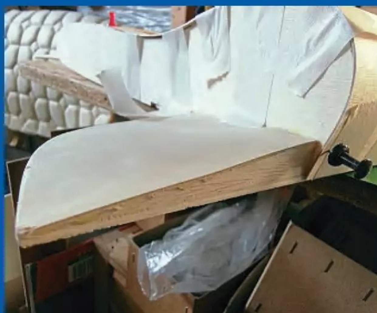
The 1.5 mm plywood top is glued on. This photo also shows the contoured rear fin.
