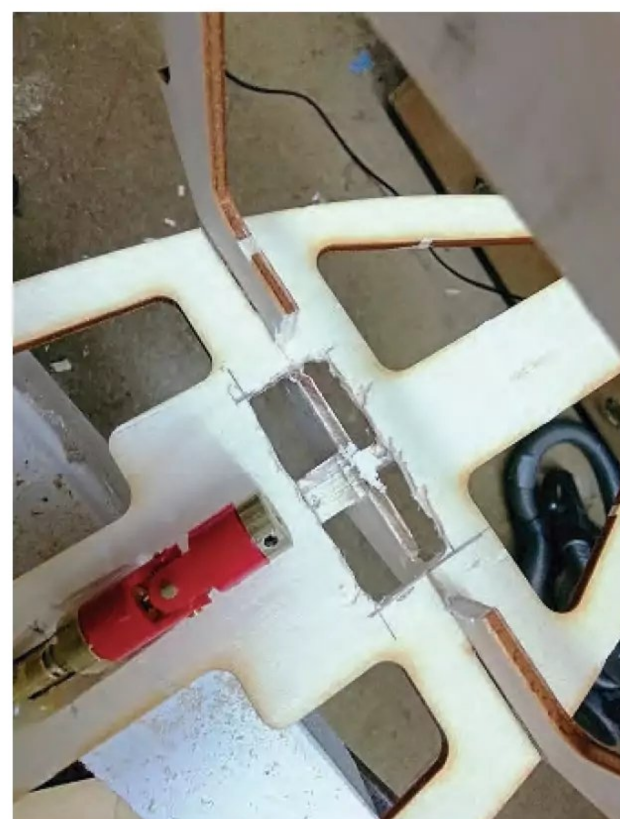
The hole cut in the deck for the motor to be dropped into.
