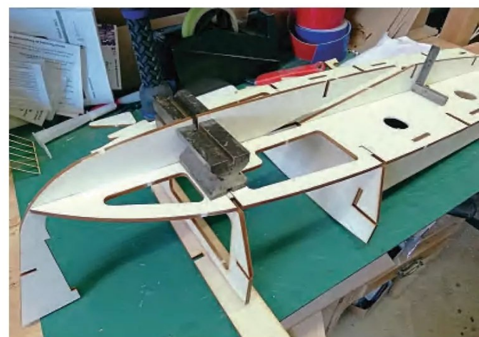
The keel fitted. John admits he made a big mistake not fitting the propellor shaft at this stage.
