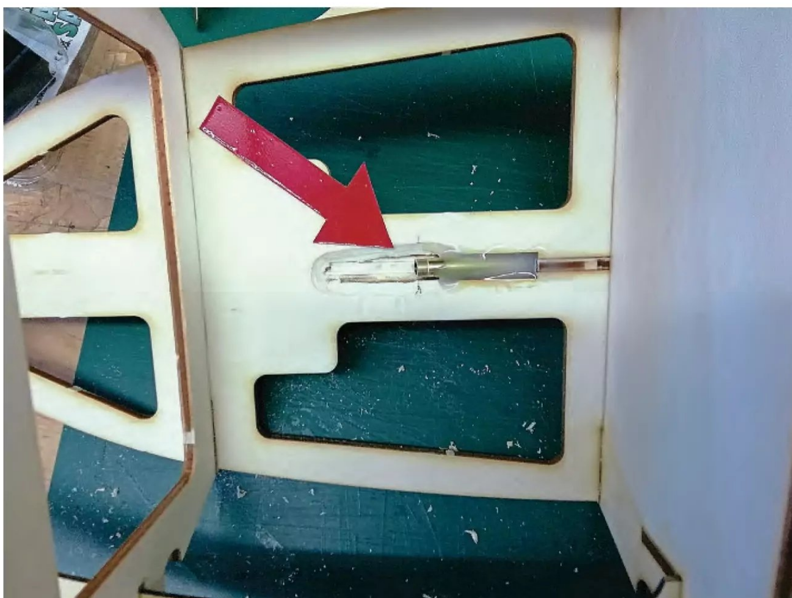
Where John's propellor shaft came through into the deck, a trough had to be gouged out to facilitate clearance for the universal joint.
