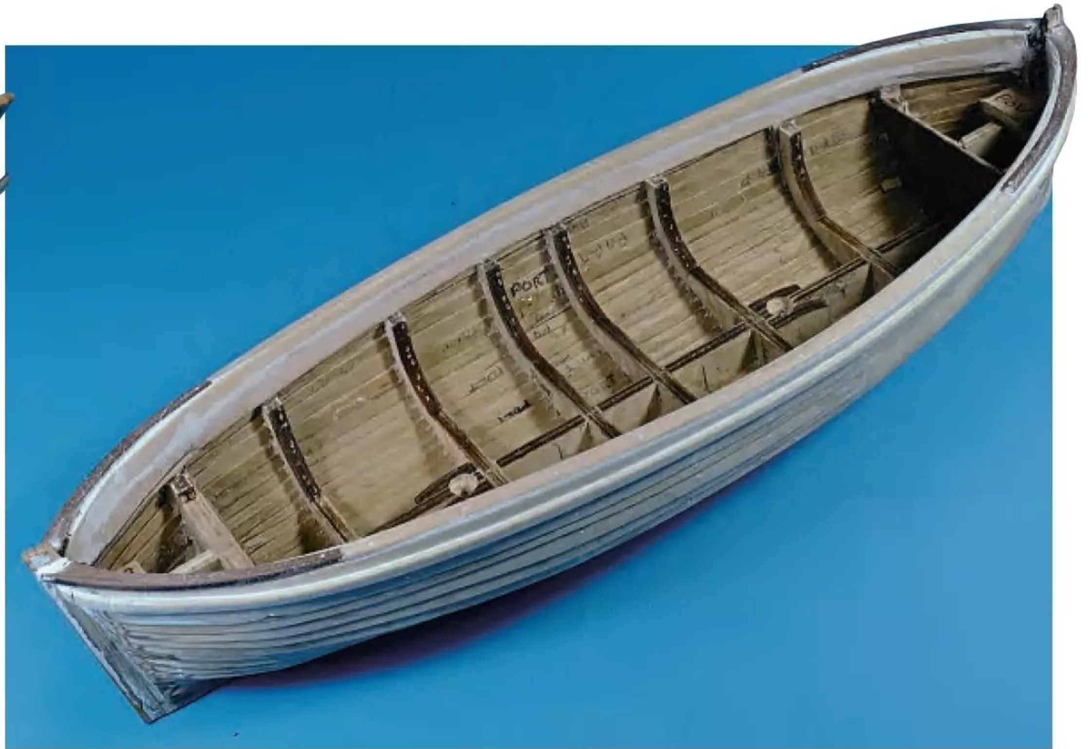
The clinker-plank fitting progressing and showing the pedestal screw fixing holes.
