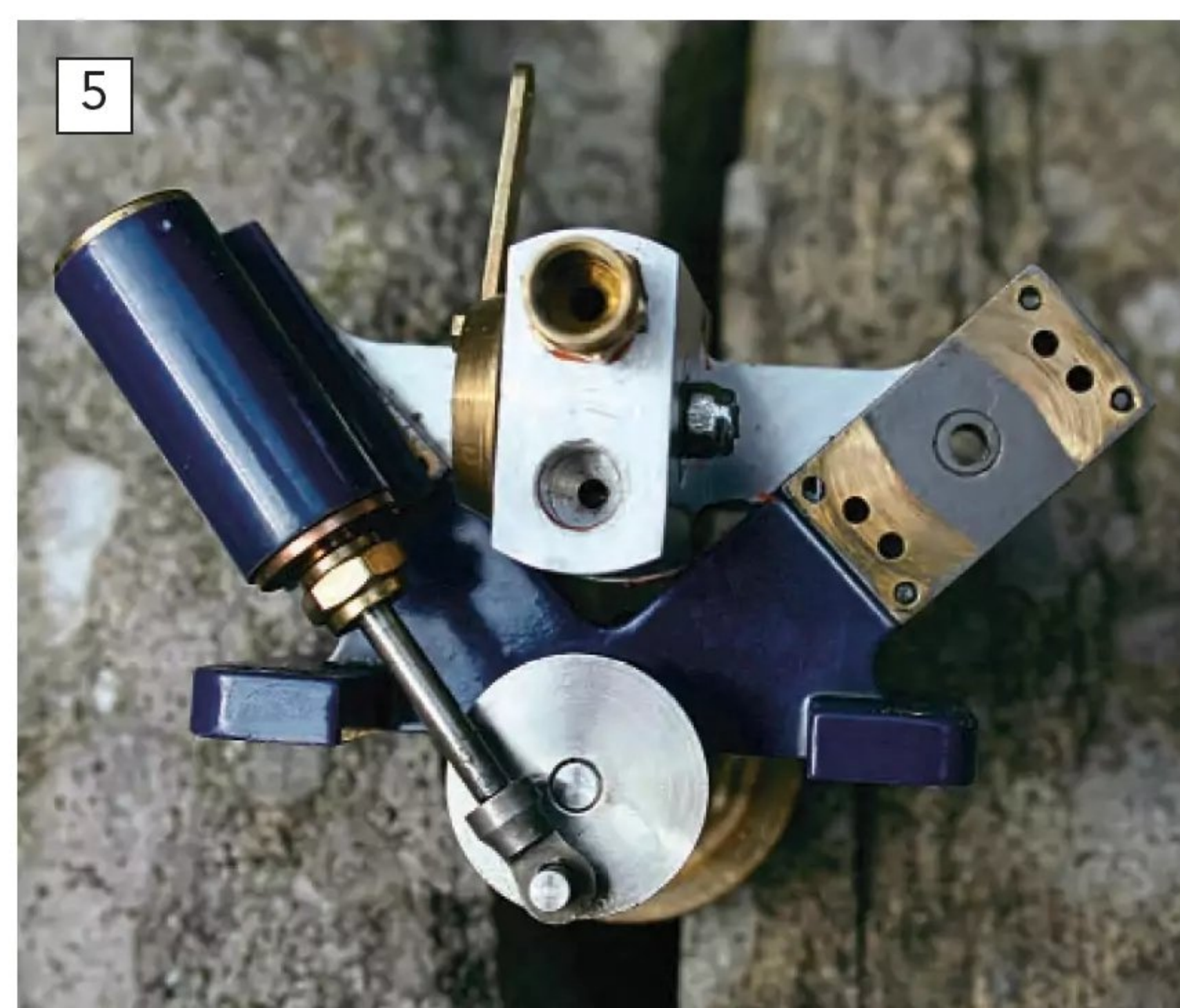
You can see from the port positionings here that there has to be a space between them, so timing is far from efficient, and both inlet and exhaust ports are of the same size. Everything about the oscillator is a compromise.
