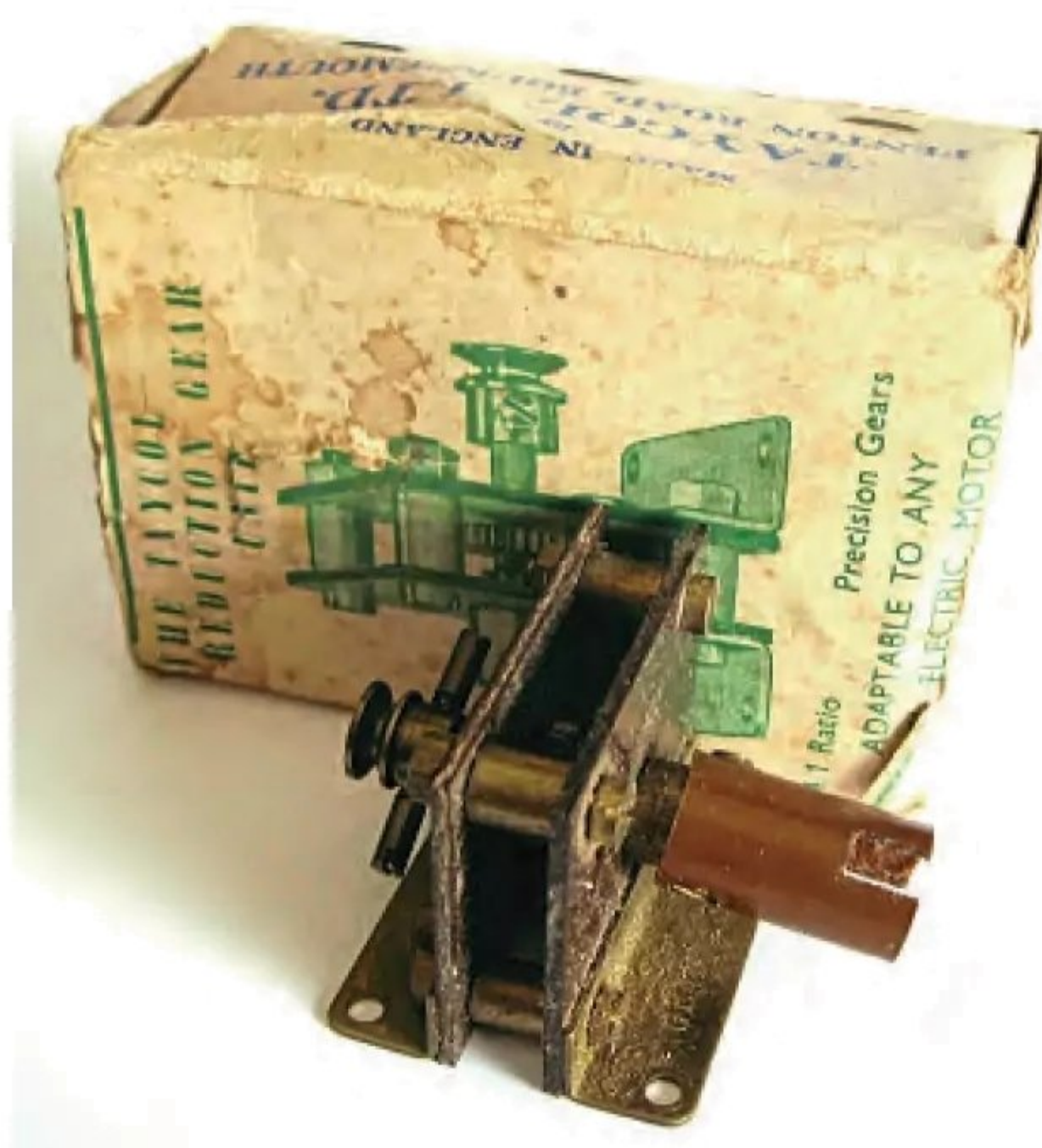
The Taycol reduction gear unit (for use on ungeared motors), which was originally priced 9 shillings and nine pence.
