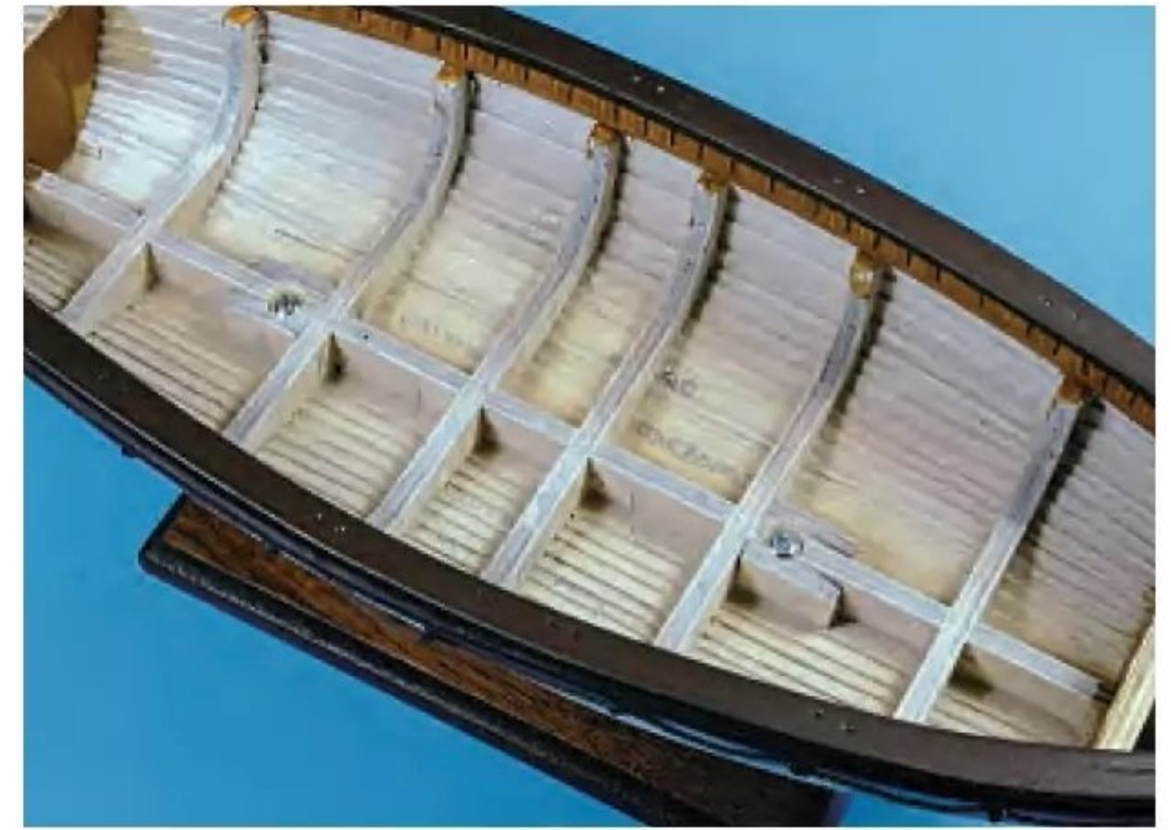
The screws fitted through the keel, brass pedestals and into the base.
