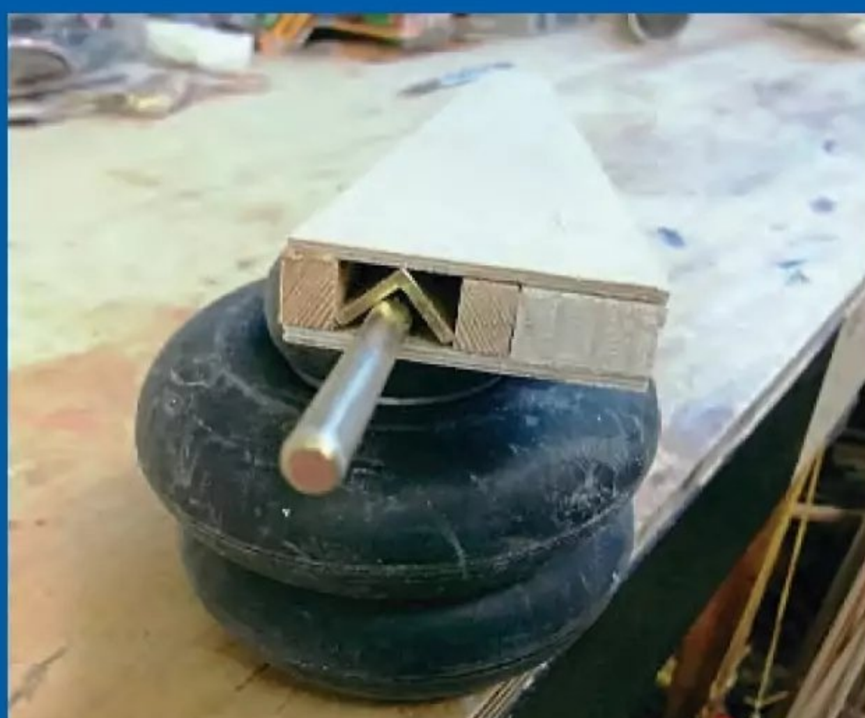
An end view of the axle showing the 'sandwich' design.
