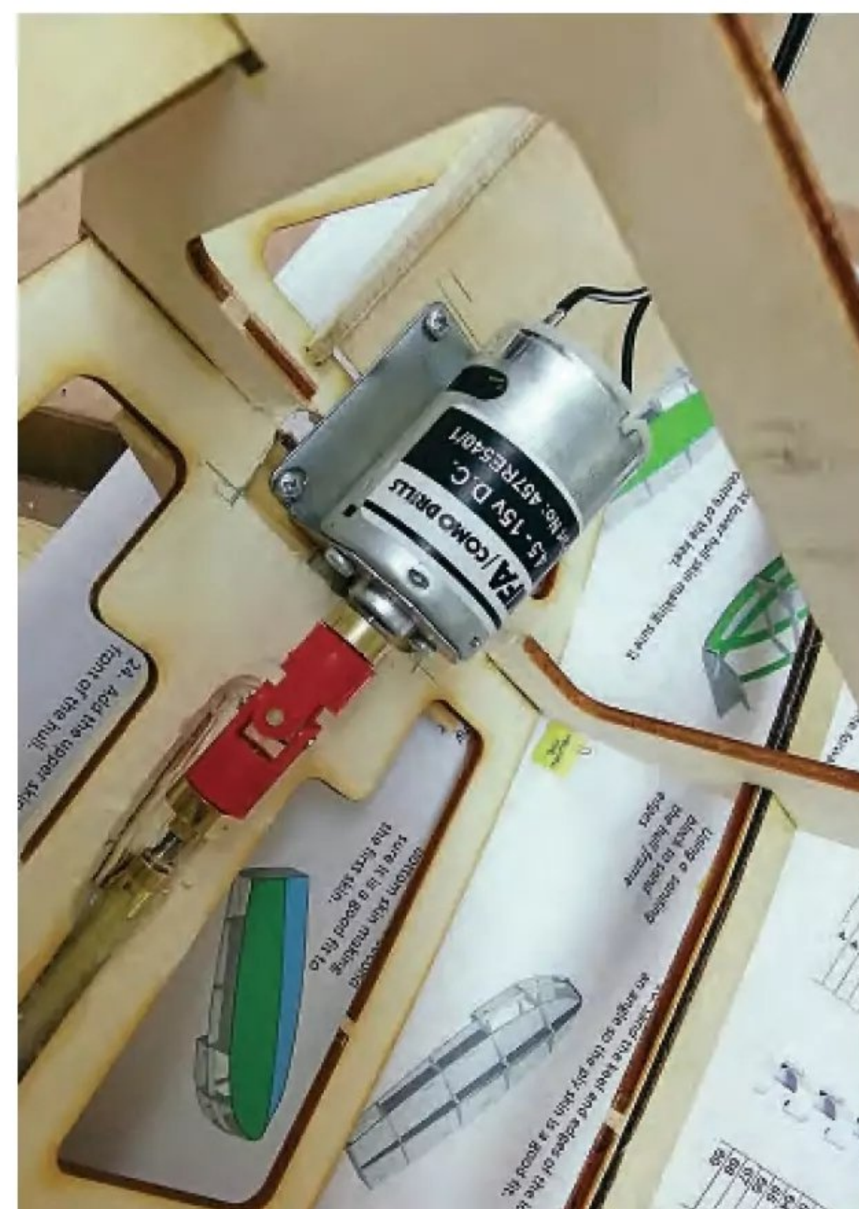
The motor dropped into the aperture and mounted on an angled block of plywood, allowing alignment with the prop shaft.
