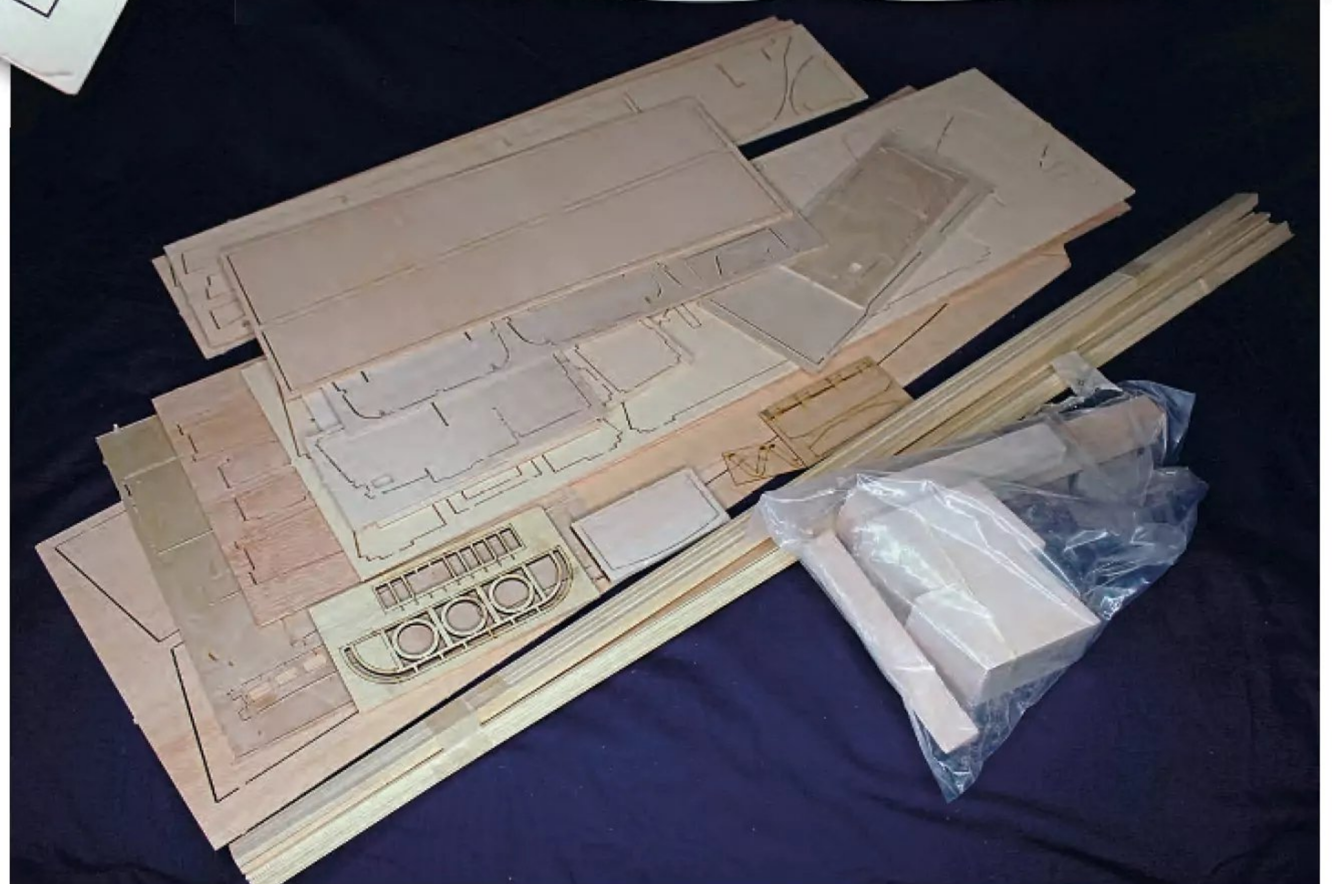
The entire hull and superstructure sections are constructed from a mixture of CNC cut plywood sheets, balsa blocks and hardwood strips.
