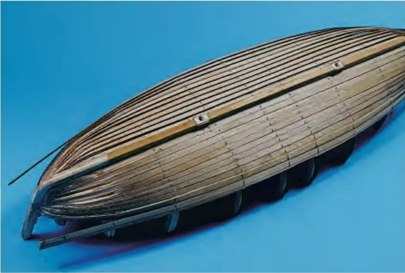
The clinker-plank fitting progressing and showing the pedestal screw fixing holes.
