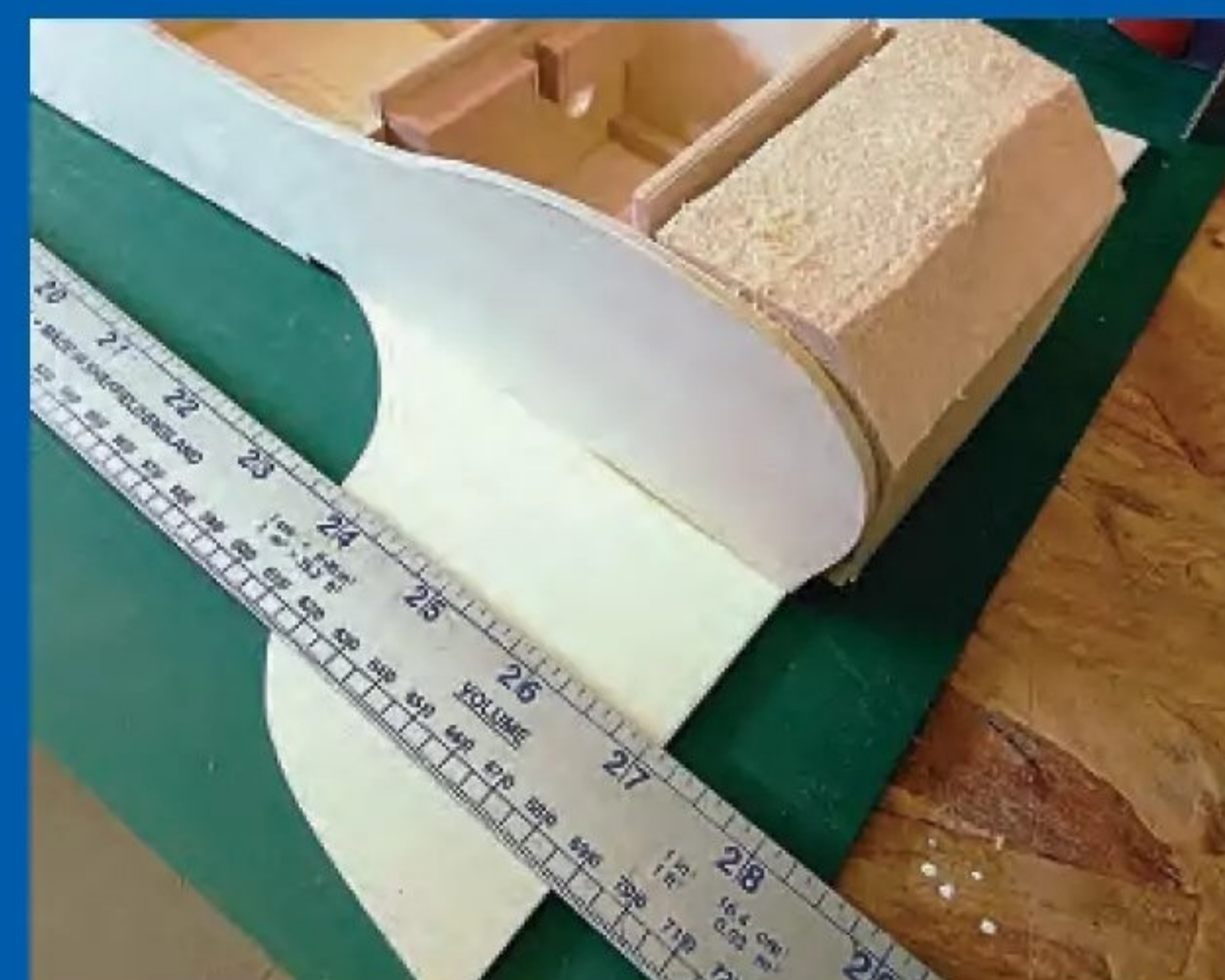
A chunk of balsa wood was glued in between the side panels at the rear of the yacht. This would be carved to shape in due course. The rule shows the length of the body.
