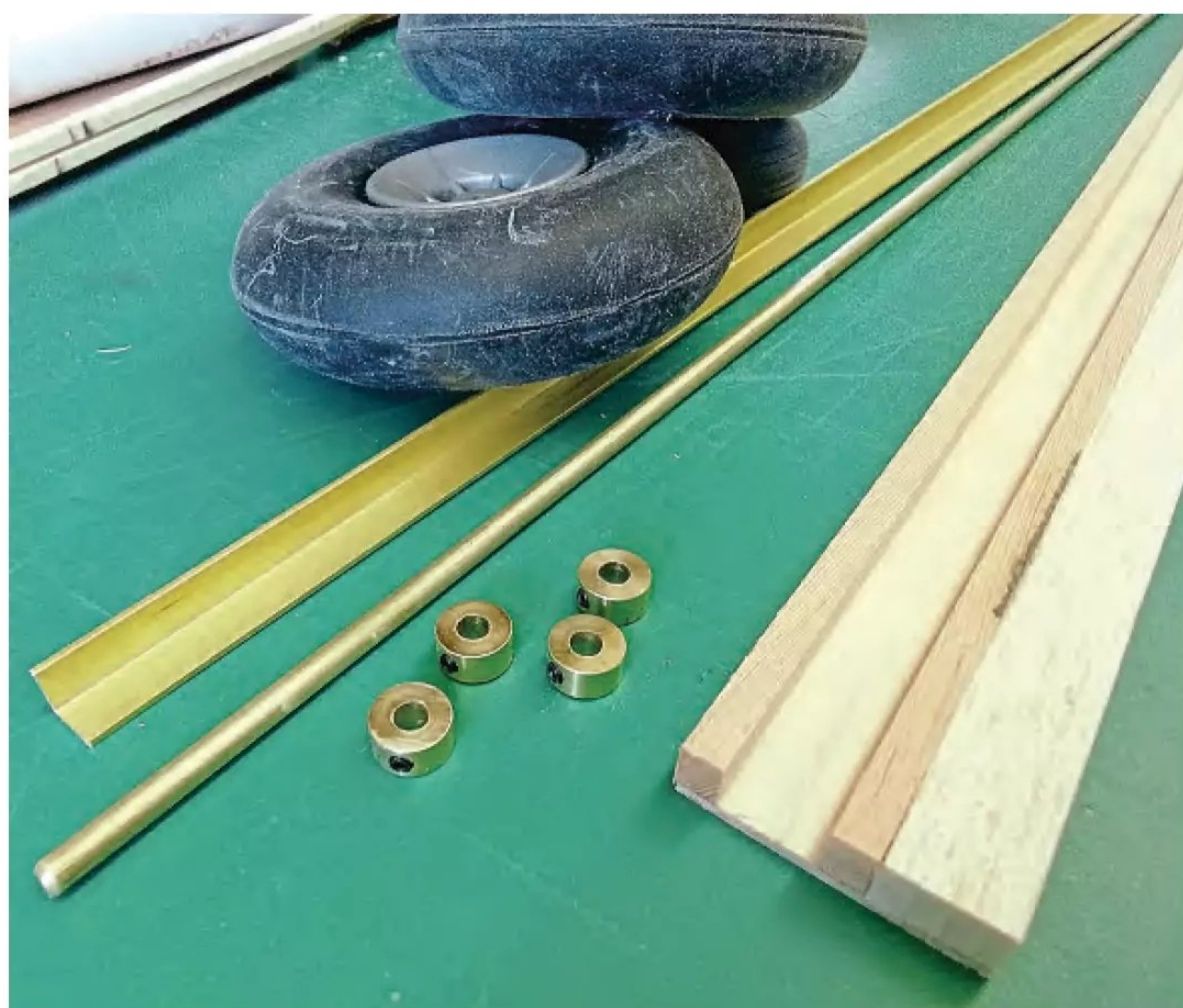
The components making up the rear axle. The brass angle gave additional rigidity to the brass axle shaft.
