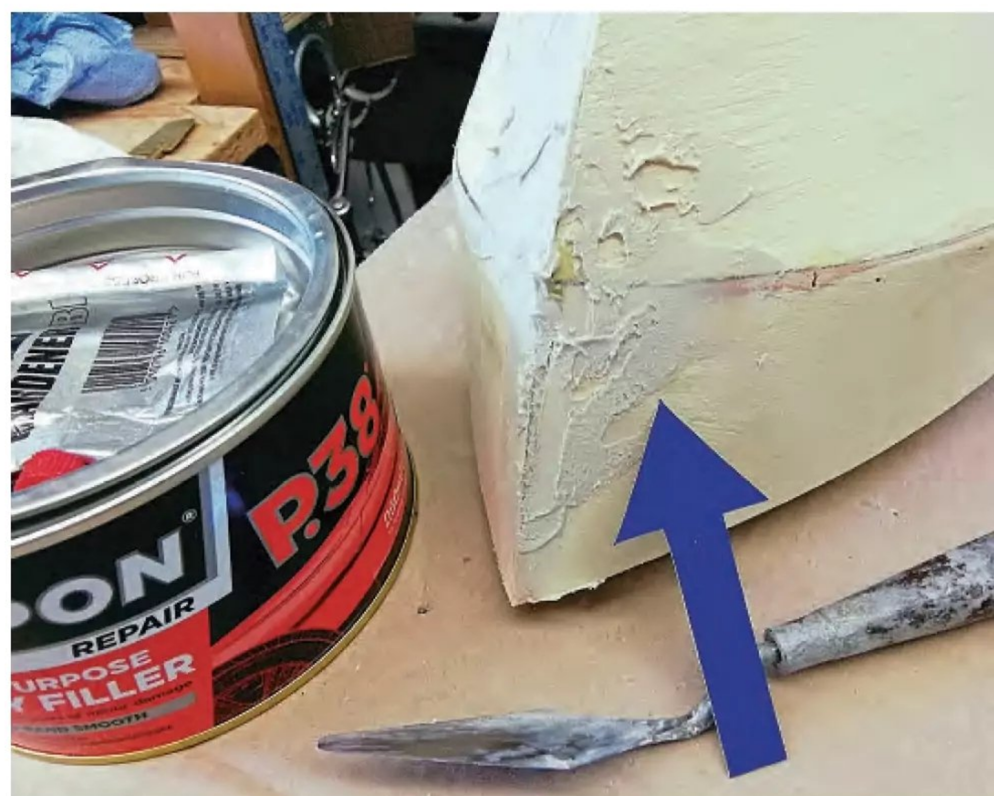
Once the outer skins have been fitted, any minor gaps and map pin holes can be filled with P 38 filler and sanded down.
