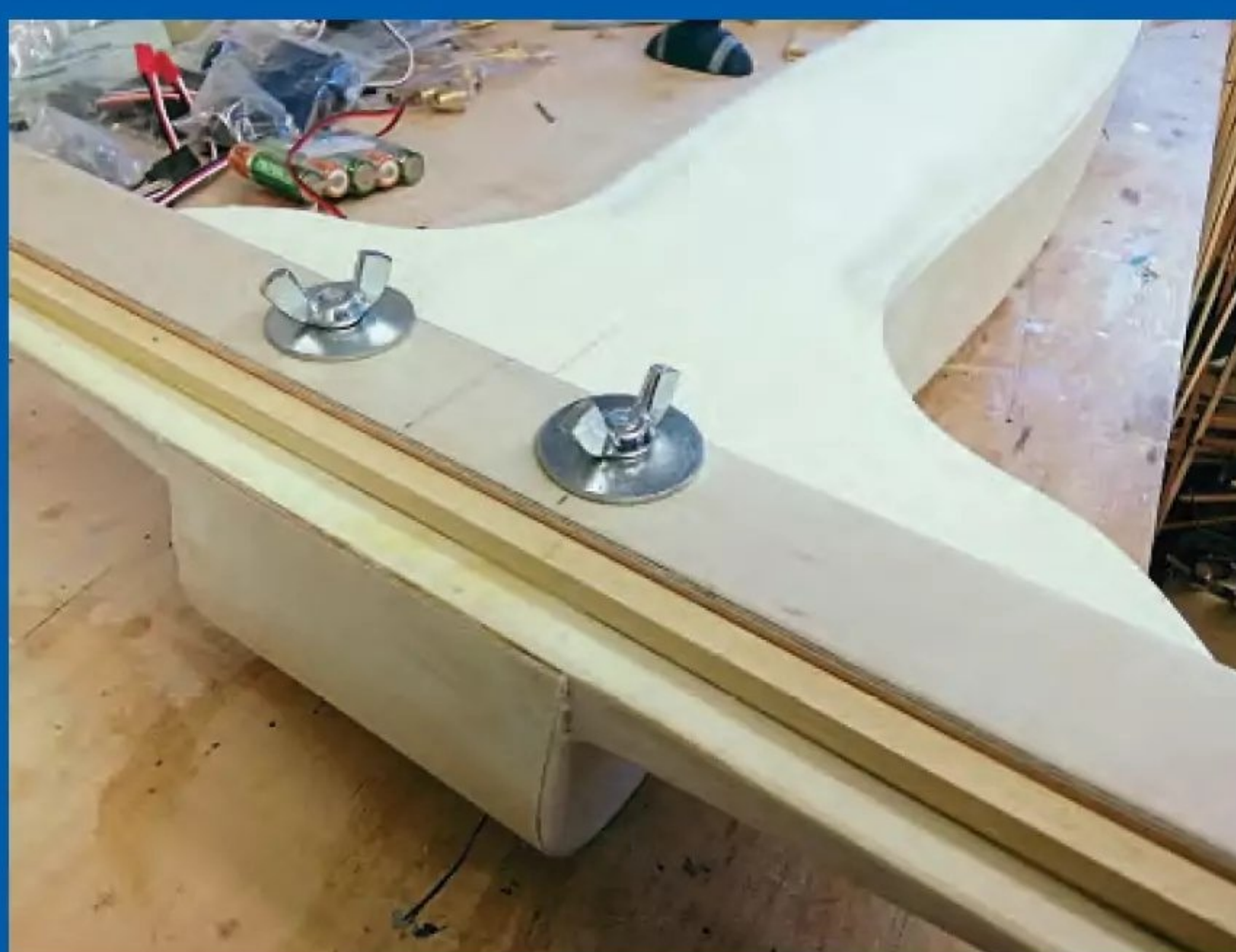
The rear wheels axle was required to be removable for ease of carriage and was held in position by two studs and wing nuts.
