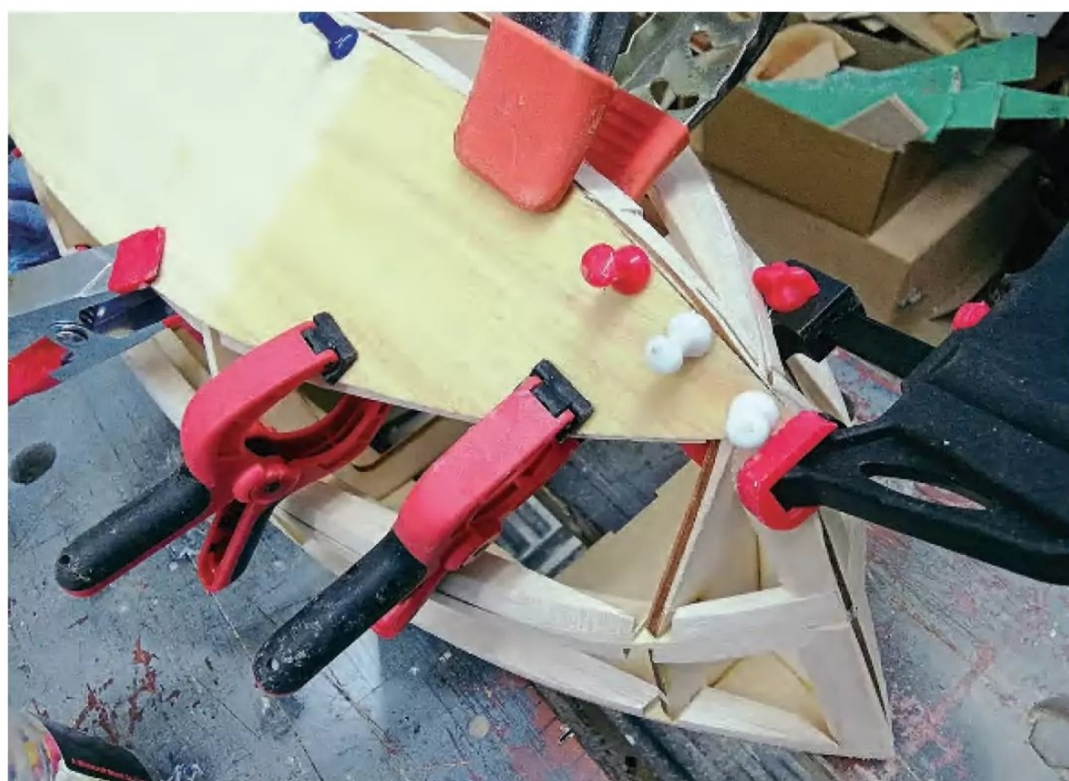
This is probably the most difficult task of the entire build: the outer skin needs to be glued onto the bow and held securely with tape, clamps and map pins.
