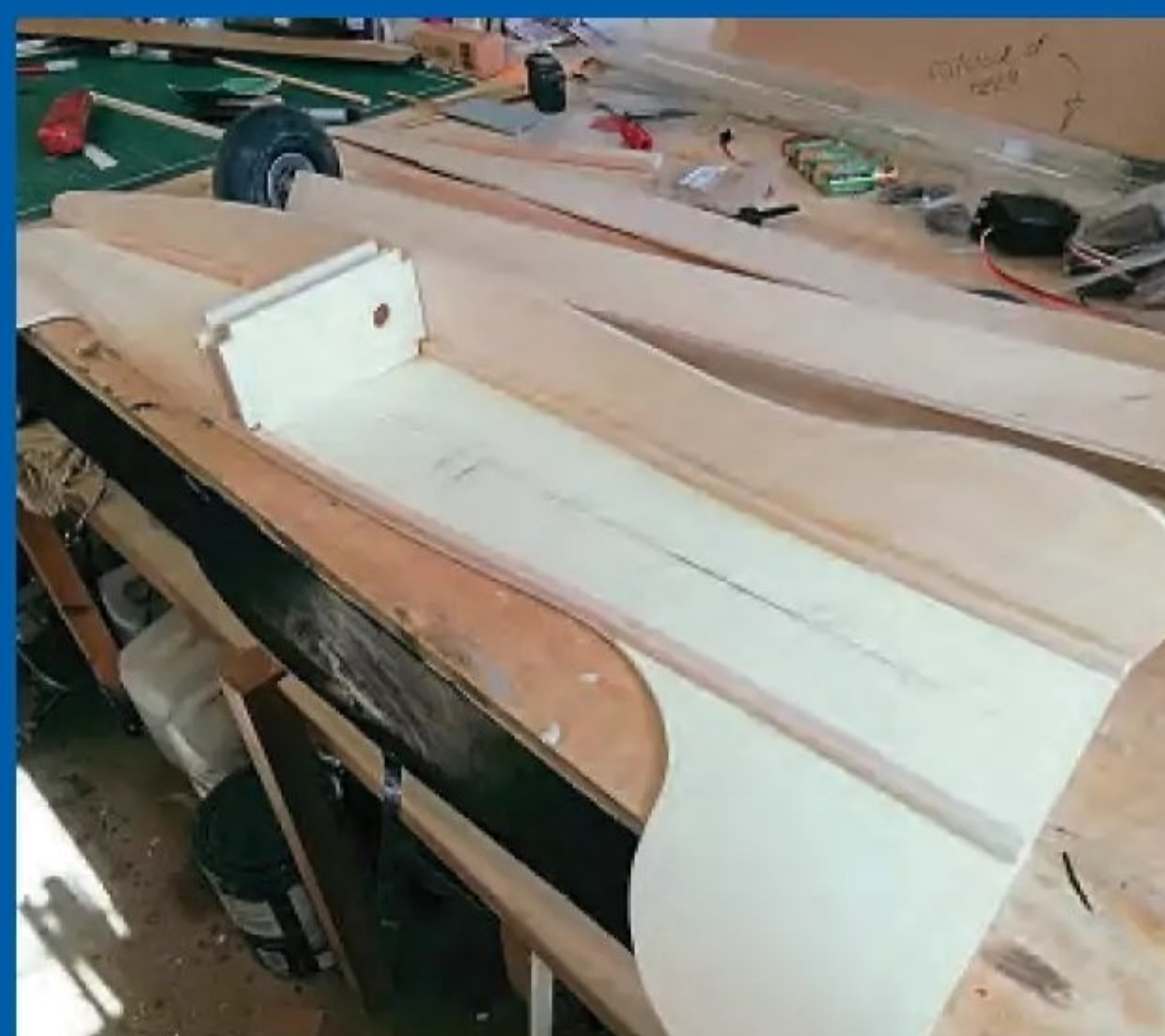
Left: The starting point for the body. The chassis was cut from 3mm plywood. Here we see the right-hand side panel, cut from 2mm plywood attached to the chassis. While John was loosely following a prescribed design, much as made up as he went along.
