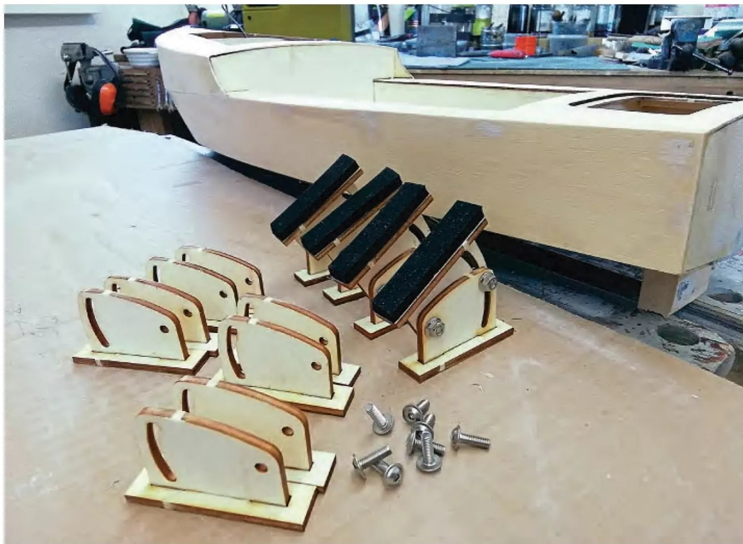
With the hull complete, a set of adjustable supports need to be made up and glued in place on a piece of plywood. These supports, made by H.A. Kits, are particularly useful when constructing any vessel.
