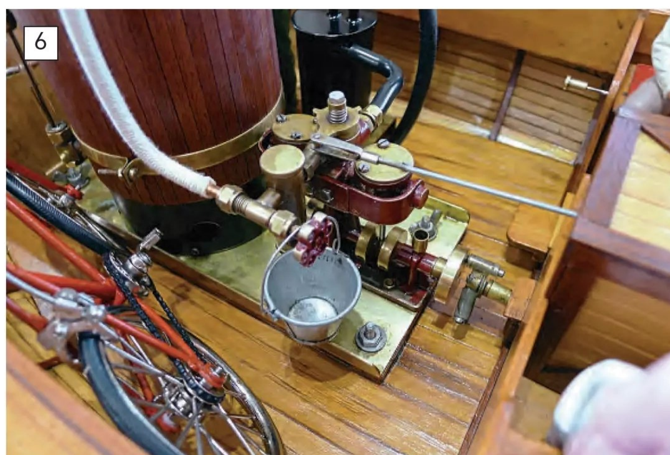
Where oscillators win out, though, is their simplicity and compactness of design and operation, which makes them ideal for small models that are convenient to carry around. Getting a valve operated engine into this same space would be a lot more challenging.
