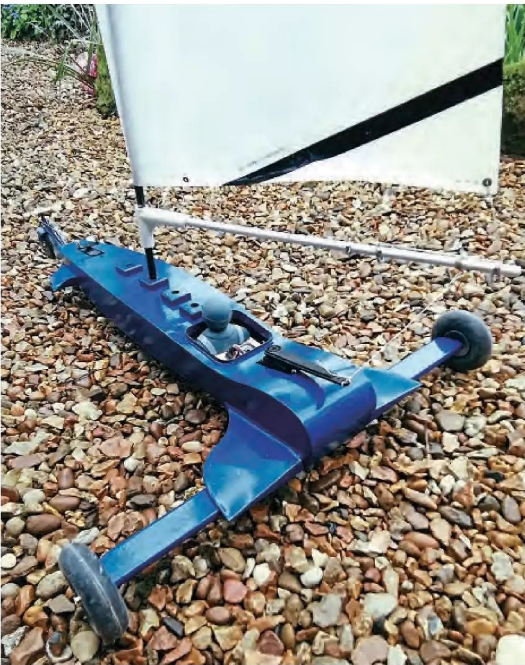
A view from the rear showing the long arm attached to the servo for the sail control. Control is somewhat limited and will probably require the attached nylon cord to be adjusted after testing.
