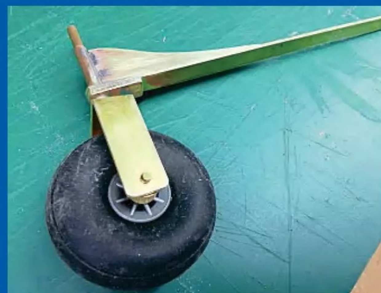
The front steering wheel was fabricated from scrap brass. After fitting, it was found to be too 'springy', and had to have an additional support added.
