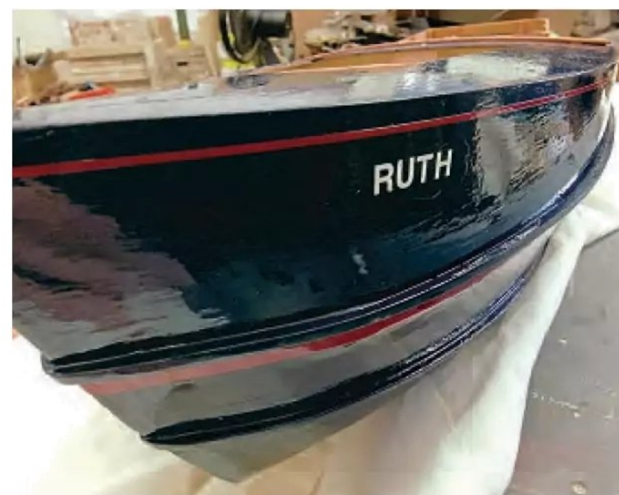
The hull exterior having received its final coat of enamel paint and with the name 'Ruth' added. The lining is Trimline self-adhesive tape, which has been applied and then given a coat of gloss varnish.
