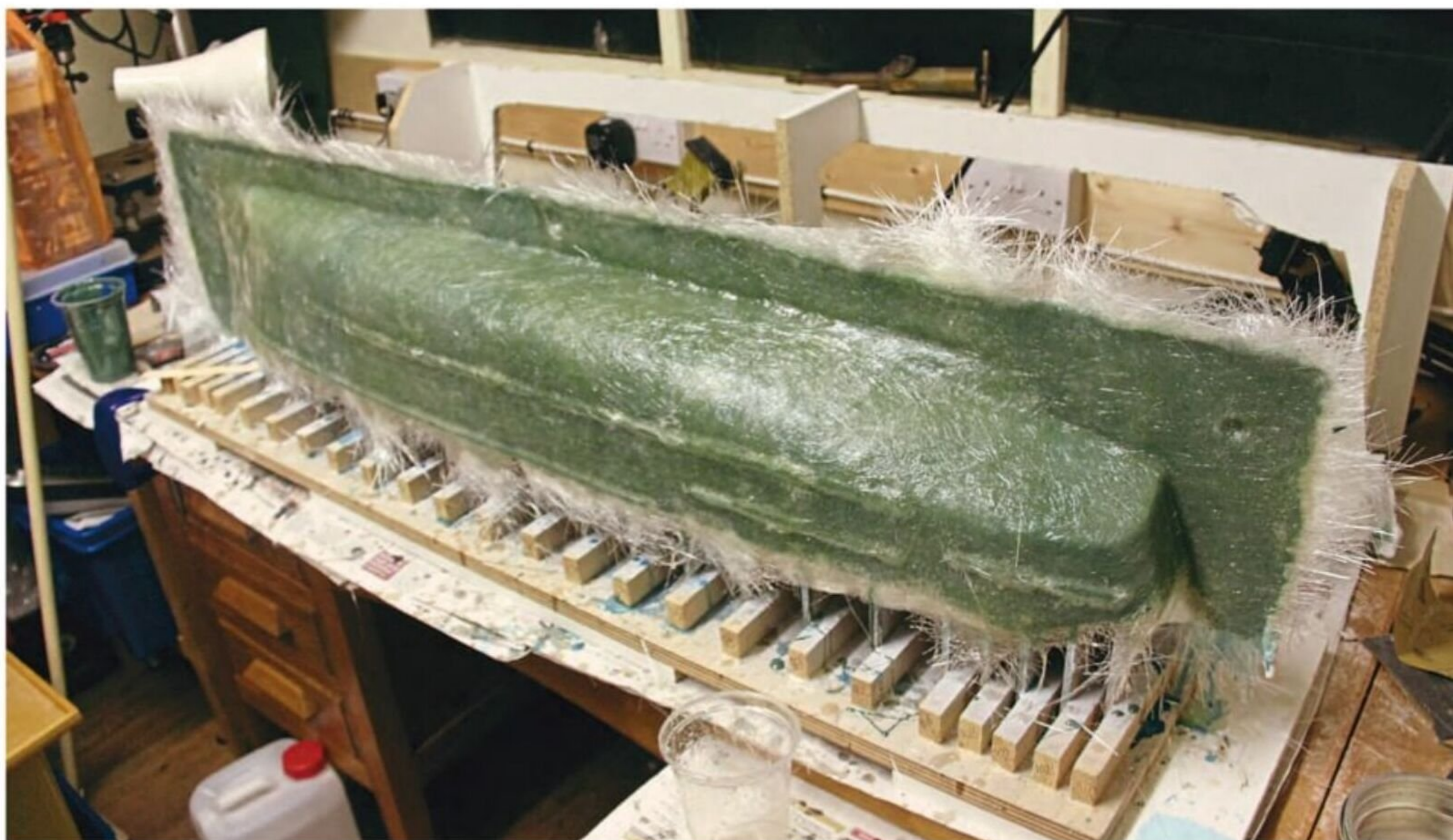
Making the mould in fibreglass.
