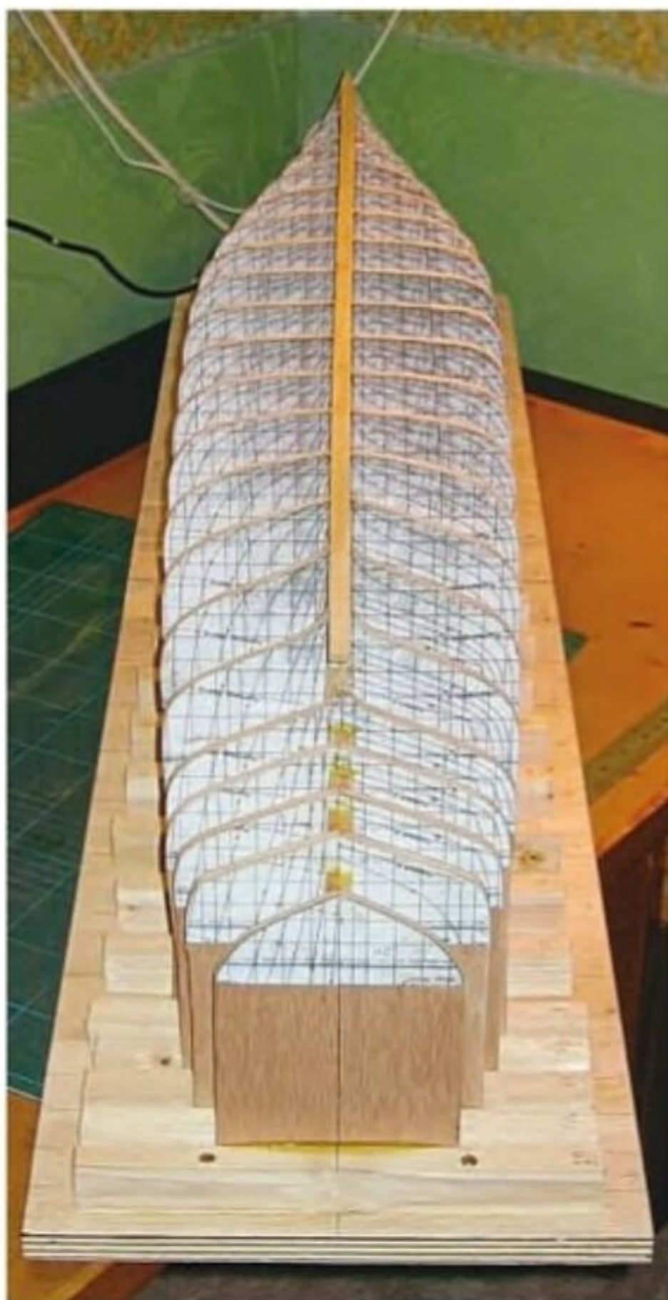
Making the plug. The individual bulkhead templates were produced and attached to ply, which was cut out and glued to the building board.
