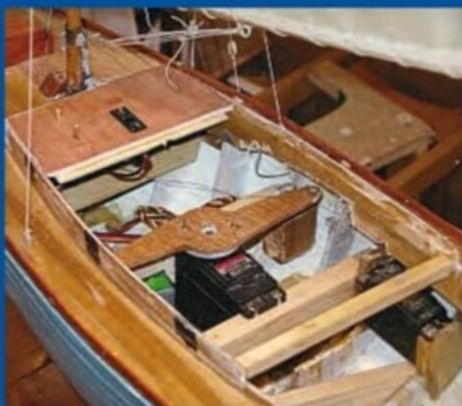
The deck forward has in it the on/off switch and the charging points.
