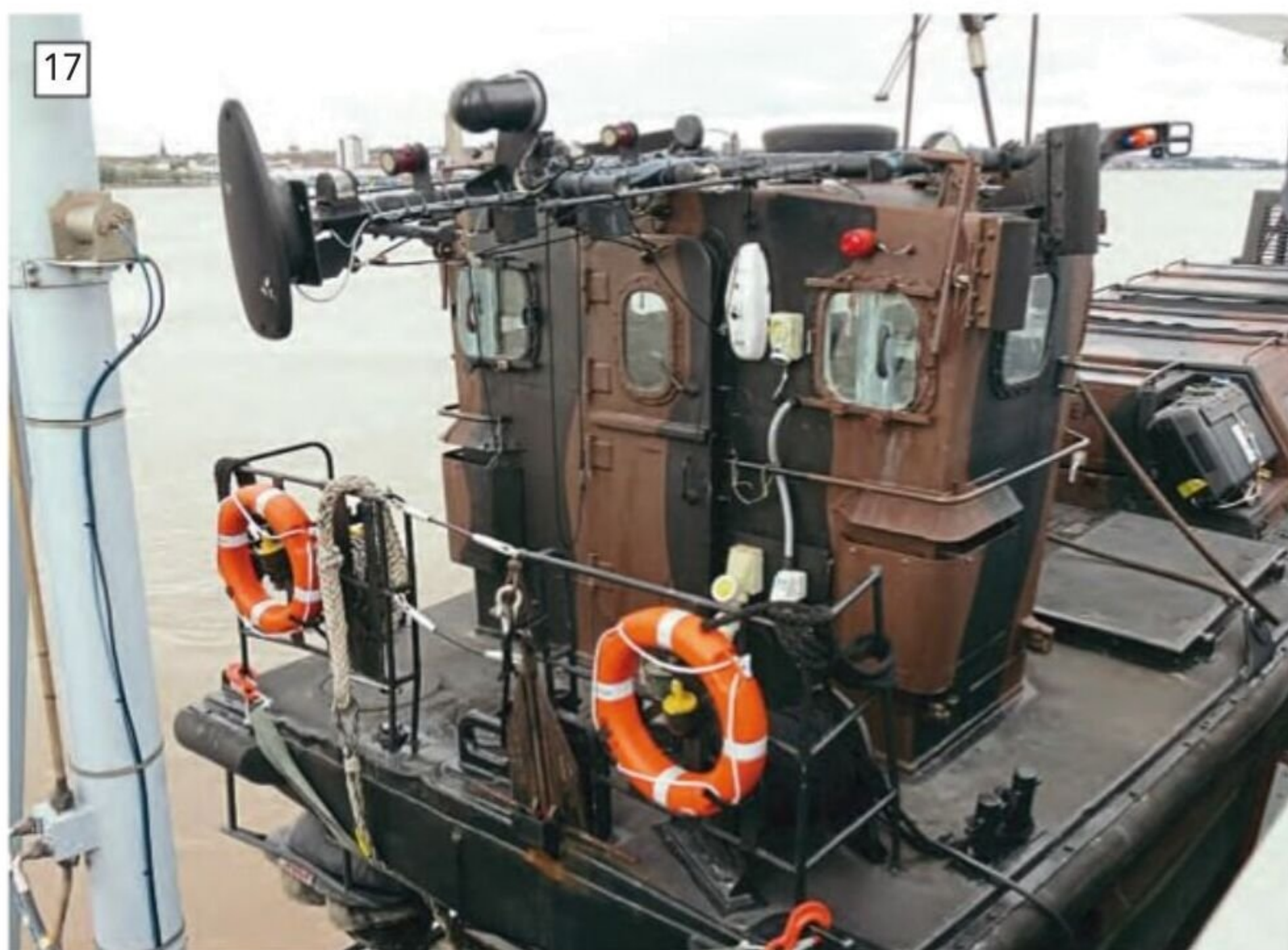
Wheelhouse after face with door.
