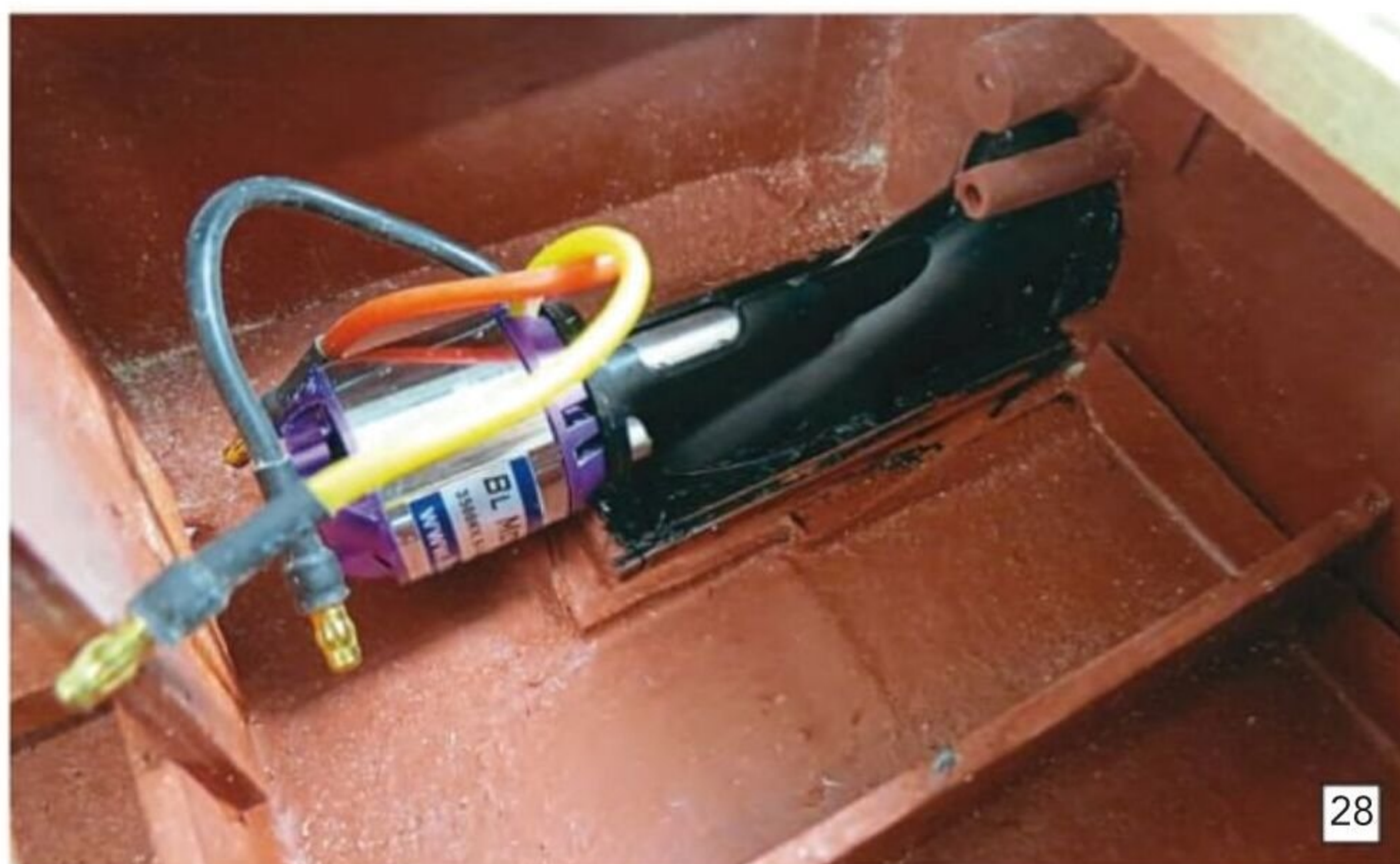
Each of the water jets sealed into the cofferdam and transom.
