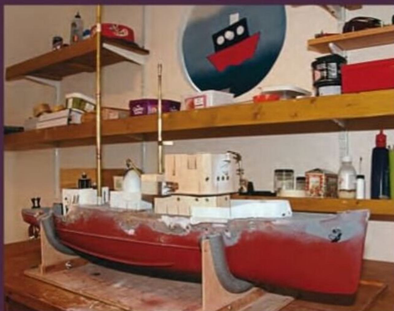
The front sea protection shroud was made from a strip of steel, bent and rolled to suit.
