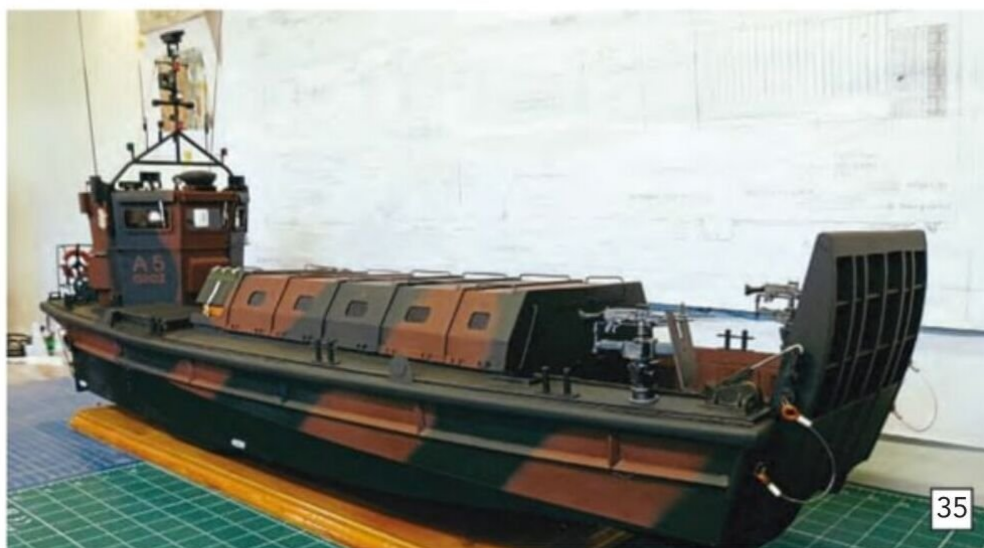
Either side forward are the two GPMG's 3D printed with brass barrels for added strength.
