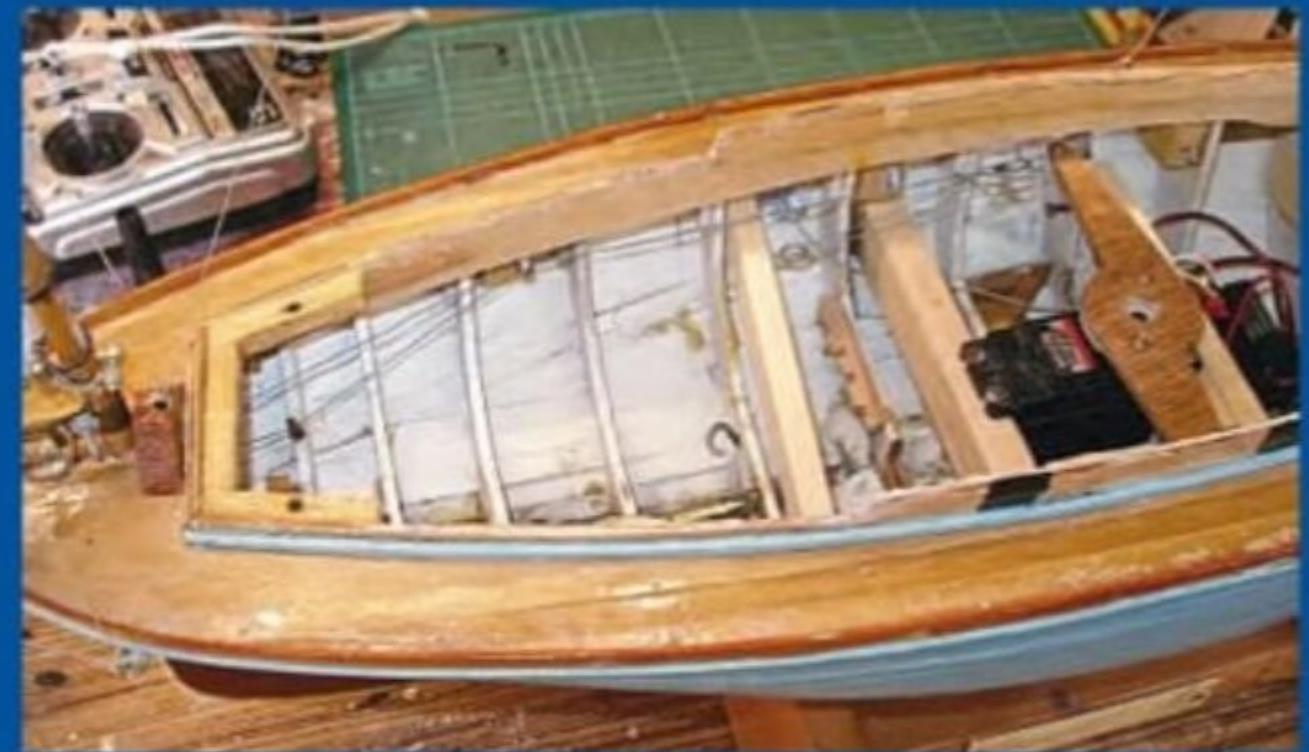
Here the boat's bows are to the right. The sail arm servo is now centrally mounted and has a centrally pivoted arm, while the sheets for the main and mizzen sails are seen on the port side. The sheet for the main sail goes through the multiplying pulleys, while that for the mizzen sail is a direct run, both from the port end of the servo arm.
