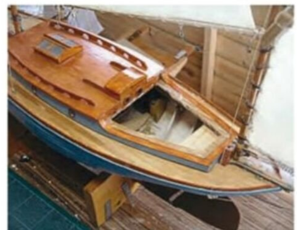
With the under-deck arrangements finalised, Nev cut out of the removable 'upper deck', creating the largest size cockpit opening that he could in order to understand what would be required below.
