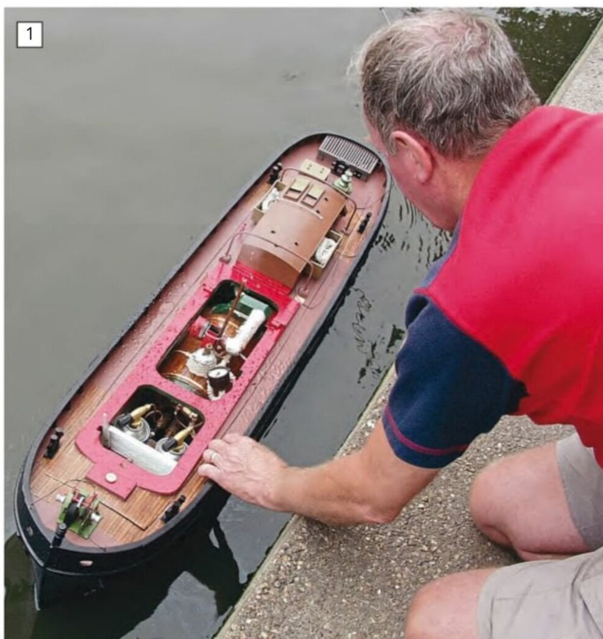
An unusual model built originally by Mr. John Goodyear's boss in his much younger days. A full strip down for a hydraulic pressure test and the model was able to be certificated.
