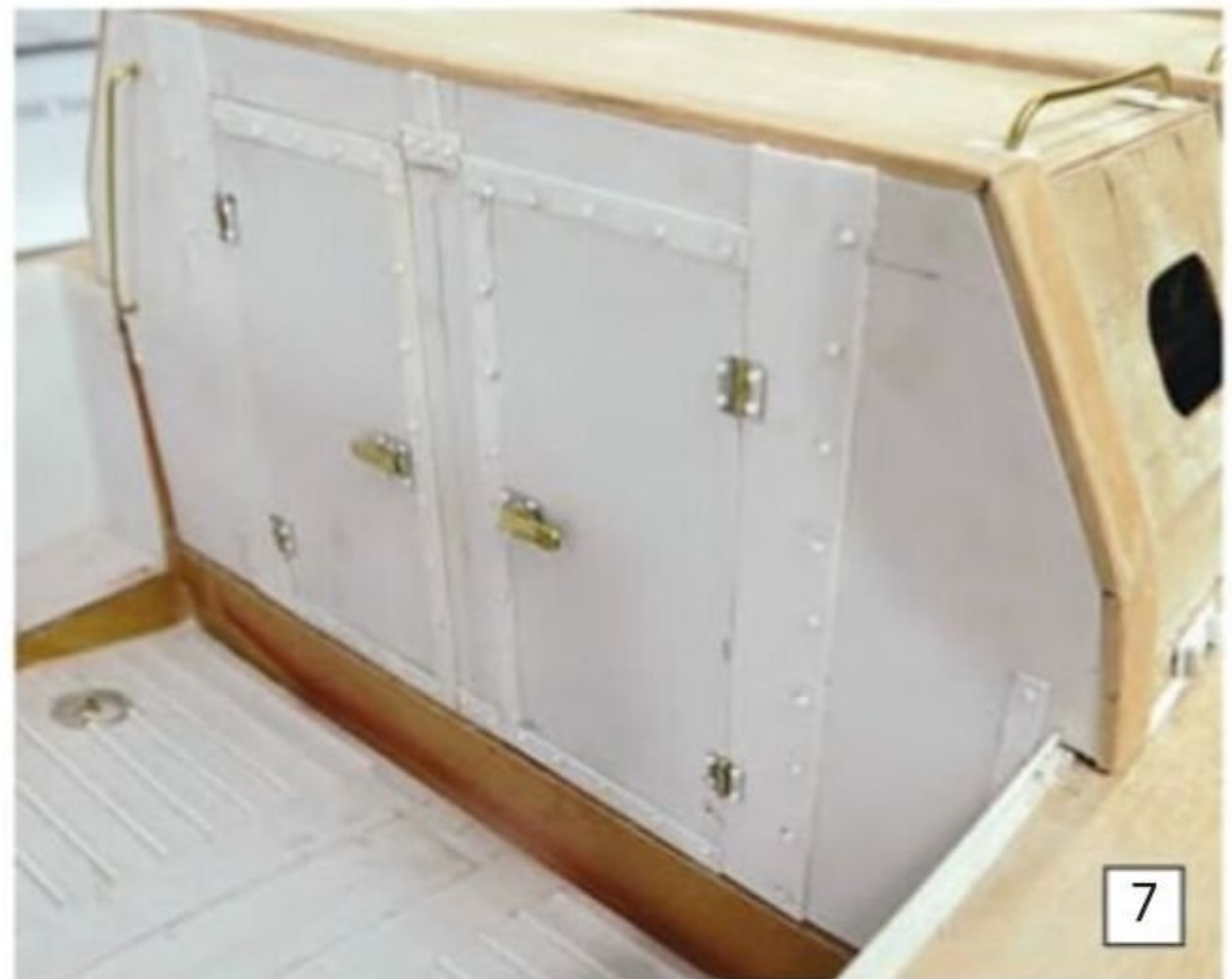
The arctic cover forward bulkhead door.
