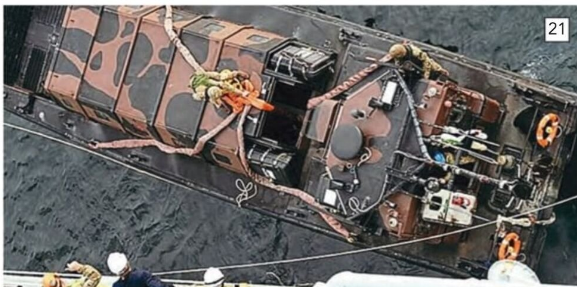
Wheelhouse roof and aft deck fittings and equipment on an actual LCVP Mk.5. Photo Crown Copyright.
