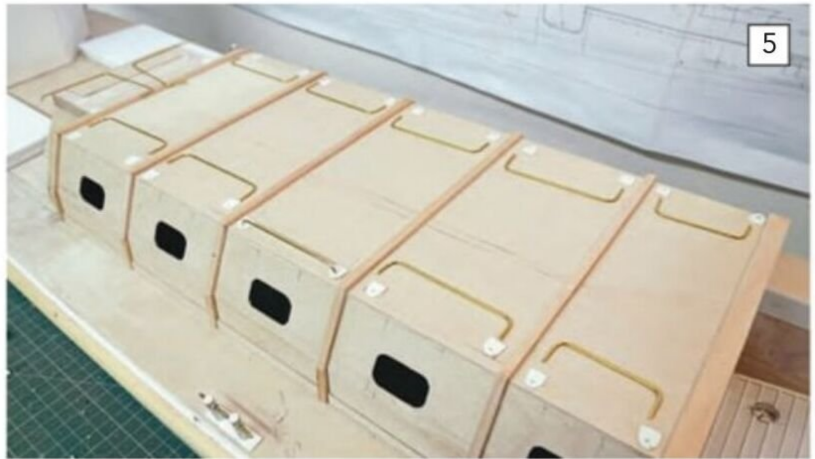
Handrails and their flanges ready to be fitted.
