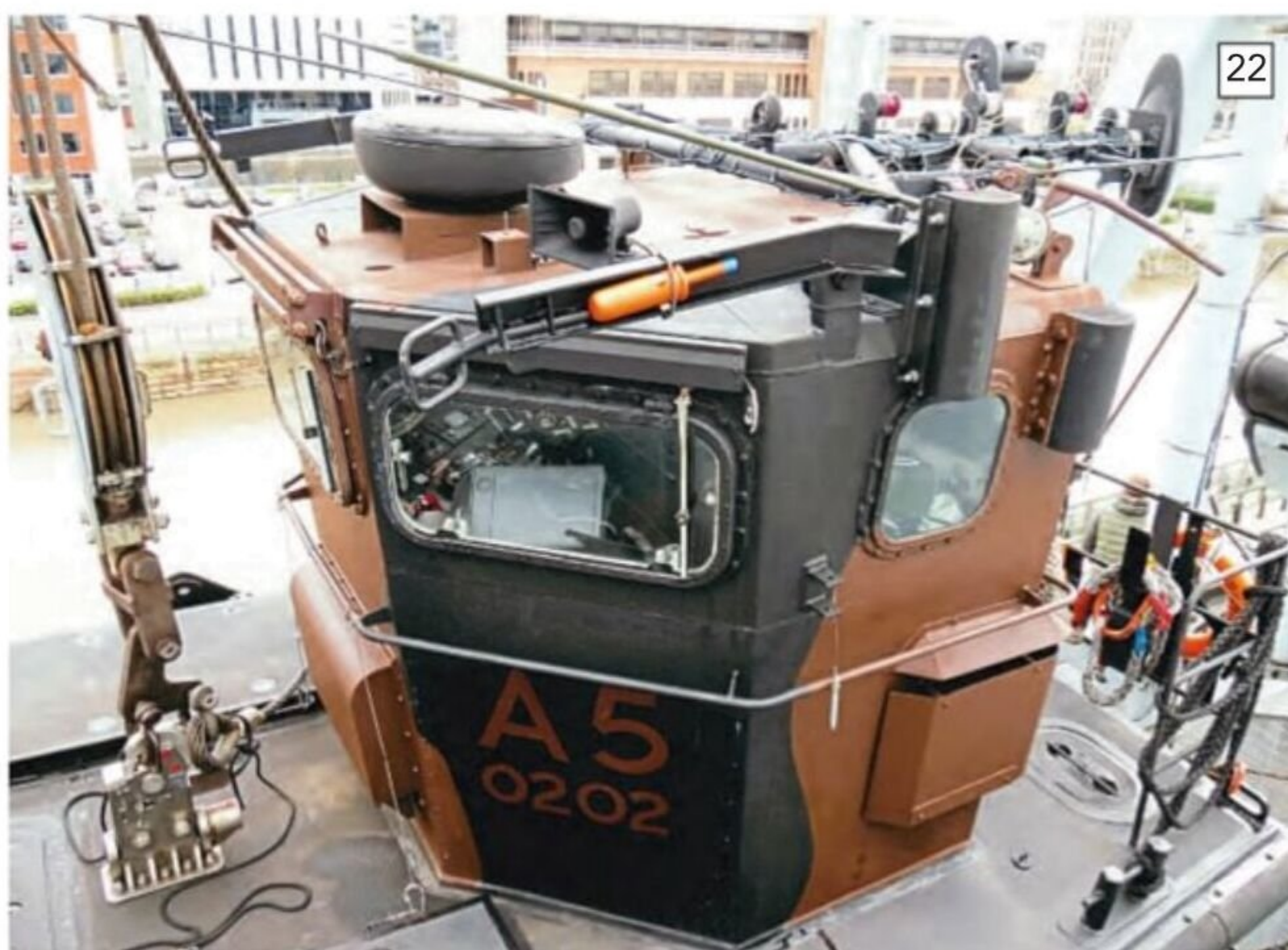
The mast can be lowered by removing locking pins on either side of the wheelhouse.
