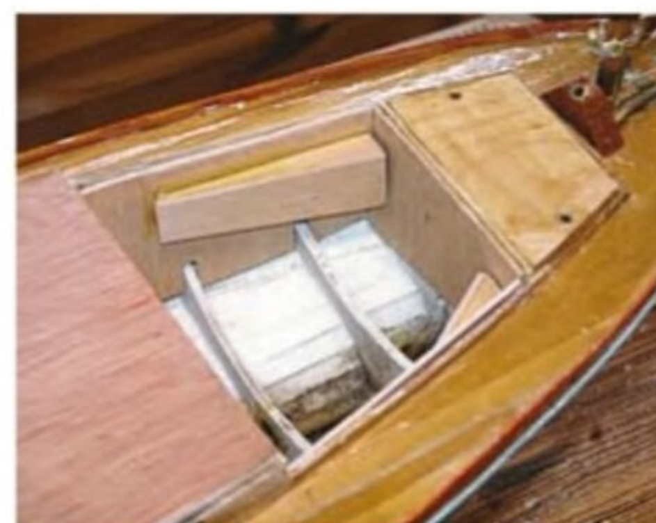
The rudder linkage on the starboard side and the main and mizzen sheets on the port side intrude into the cockpit area, so both had to be boxed in, for later waterproofing.
