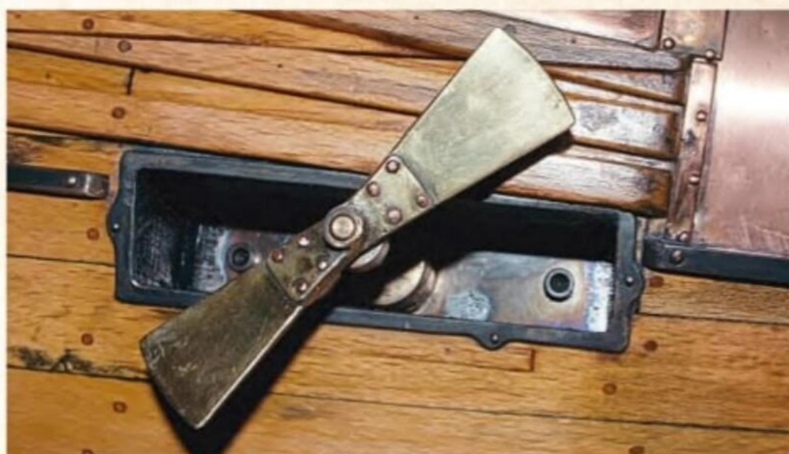
Close up of one of the retractable manoeuvring propellers.
