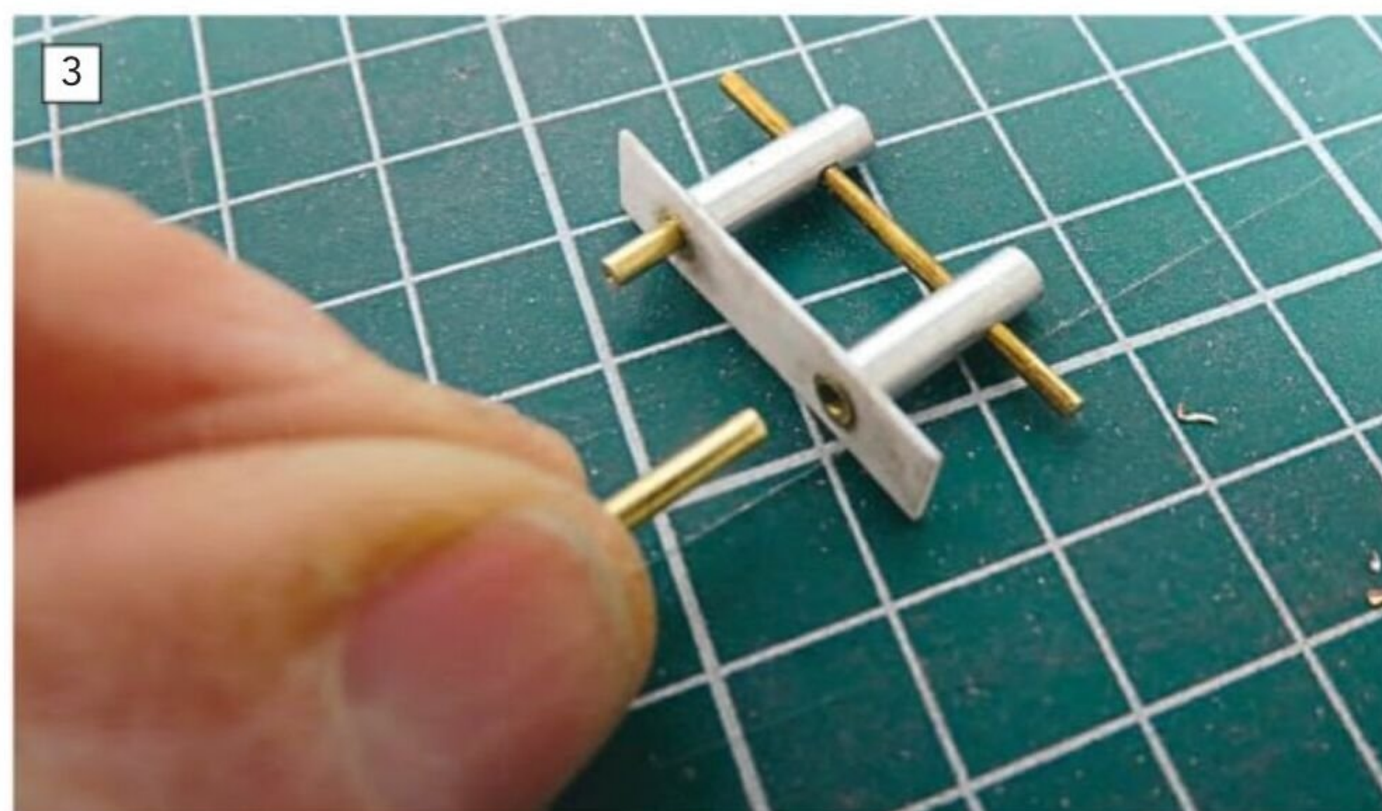
The bits are secured using brass pins inserted into the brass sleeves
