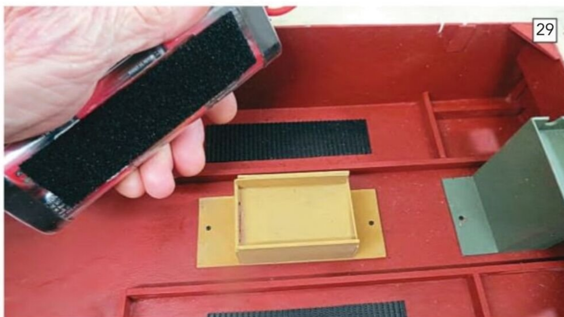
Velcro used to secure the batteries while permitting their movement when adjusting trim.
