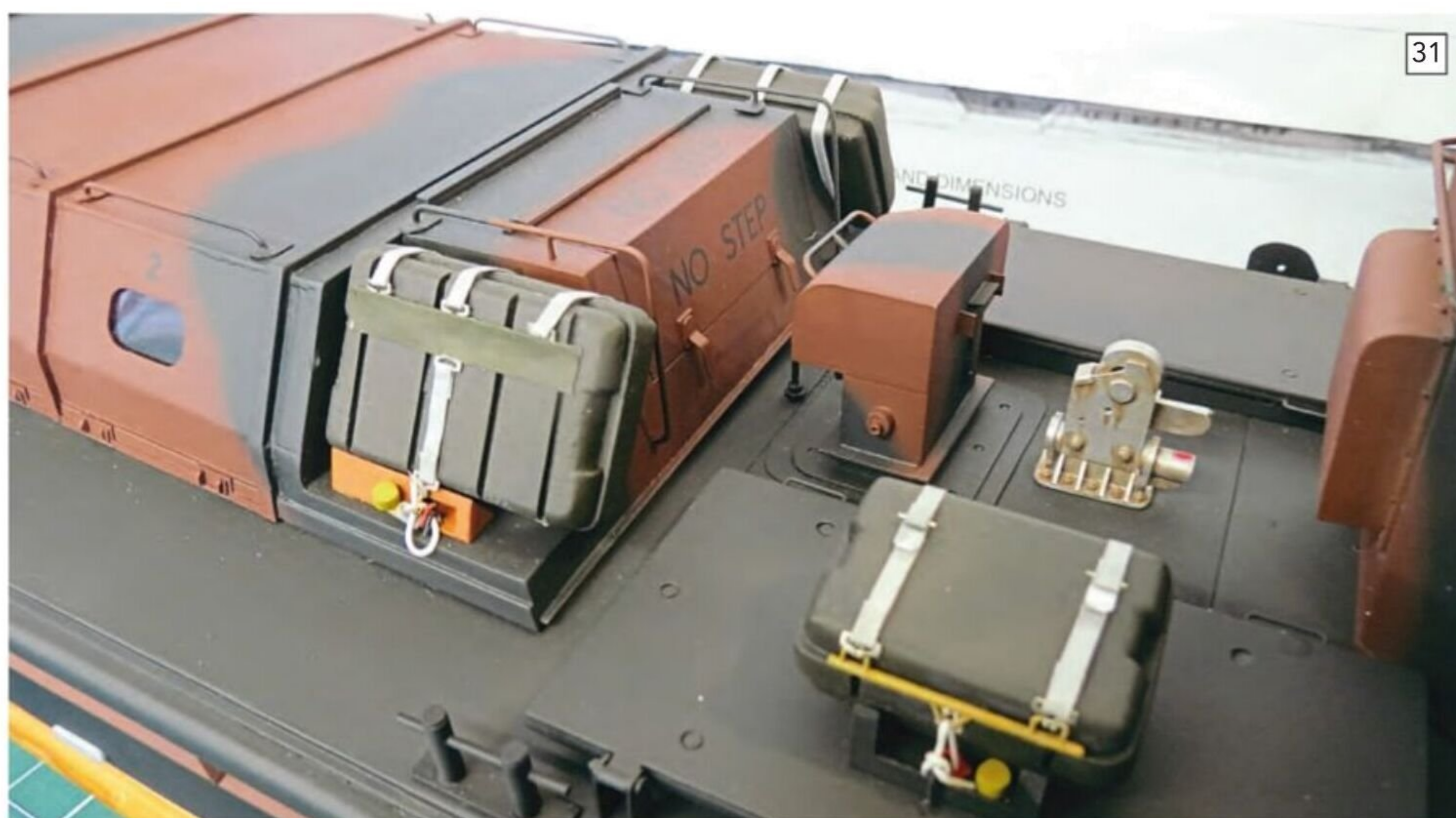
The 16-person inflatable life raft containers port and starboard, with a further 6-person raft container mounted on the engine access hatch to port, were formed from balsa.
