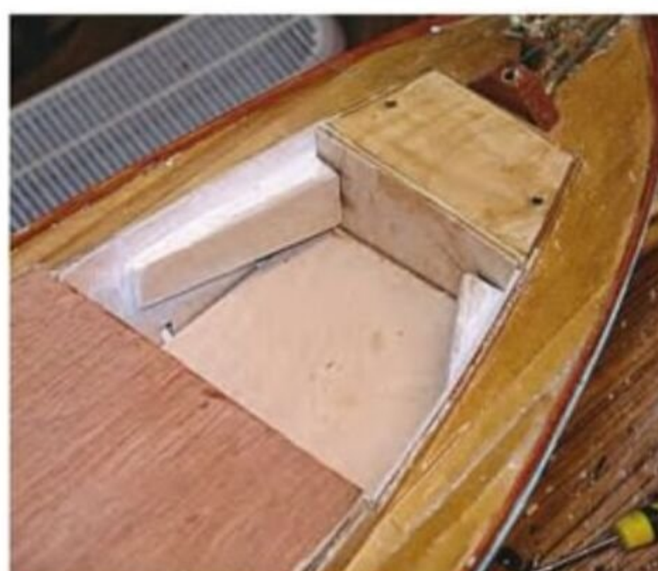
Decorators' caulk was used to start the water-proofing process.
