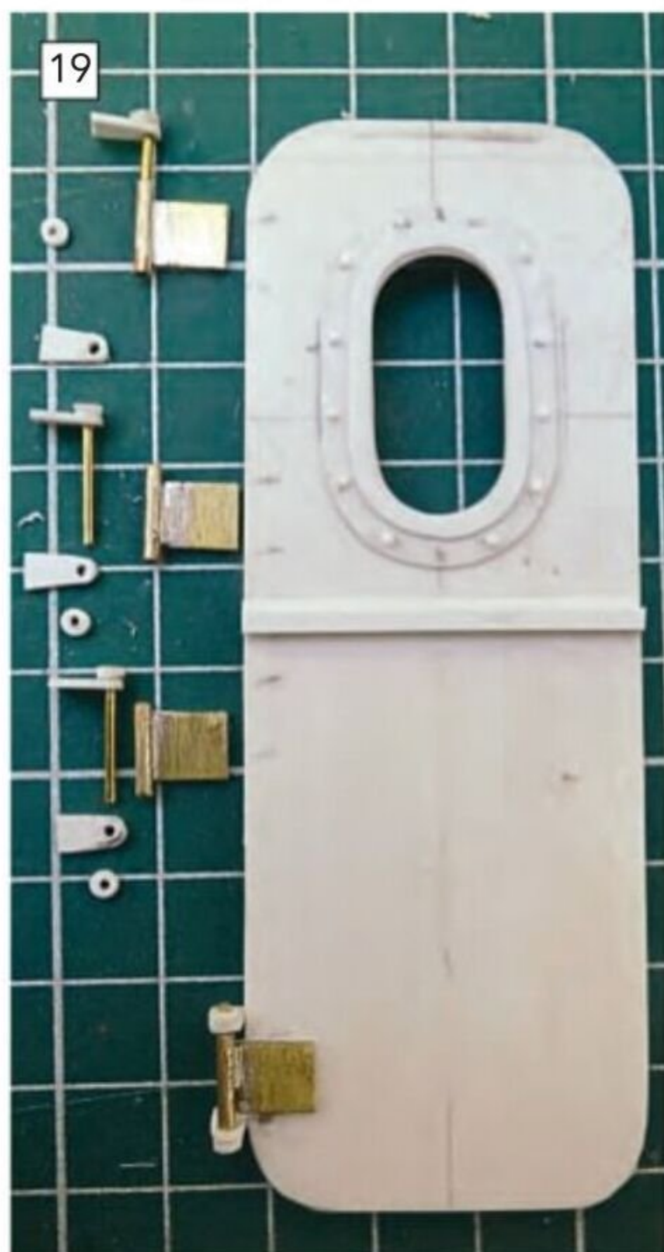
Adding the working hinges to the assembled door.
