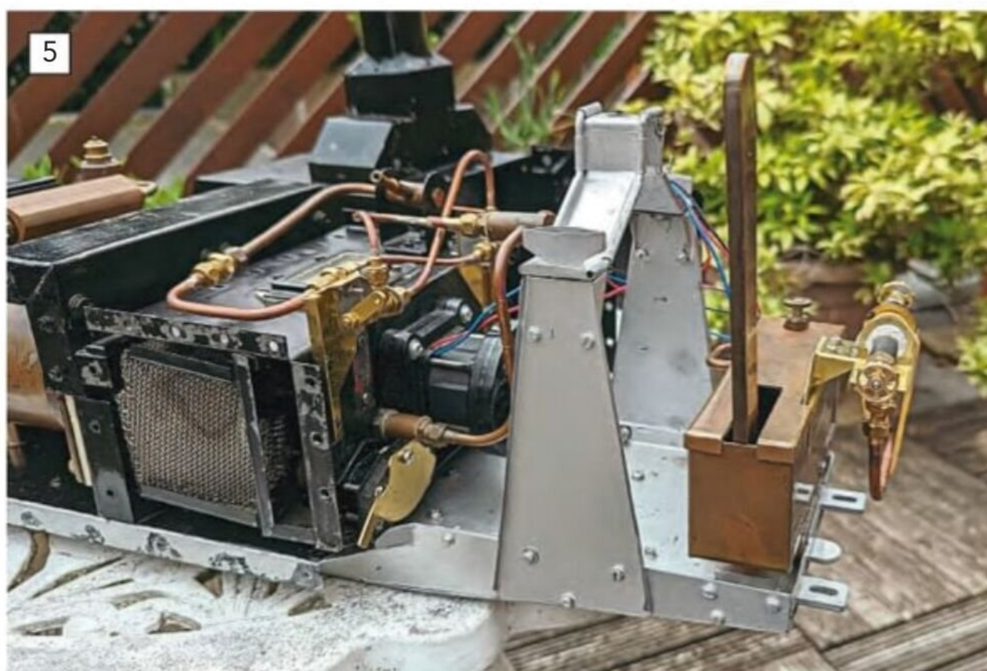
There is only a single water pump fitted, which is a manually operated pump, requiring the model to be brought to the bank for a top up of the boilers.
