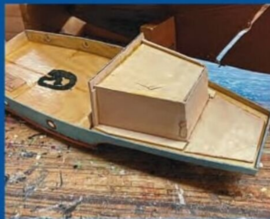
The cockpit shape completed.
