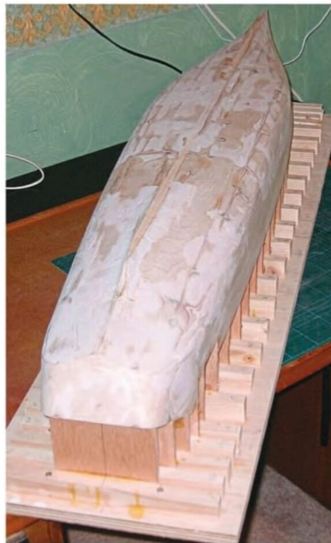
Having covered the bulkhead templates with thin ply, the whole was then smoothed over with filler.
