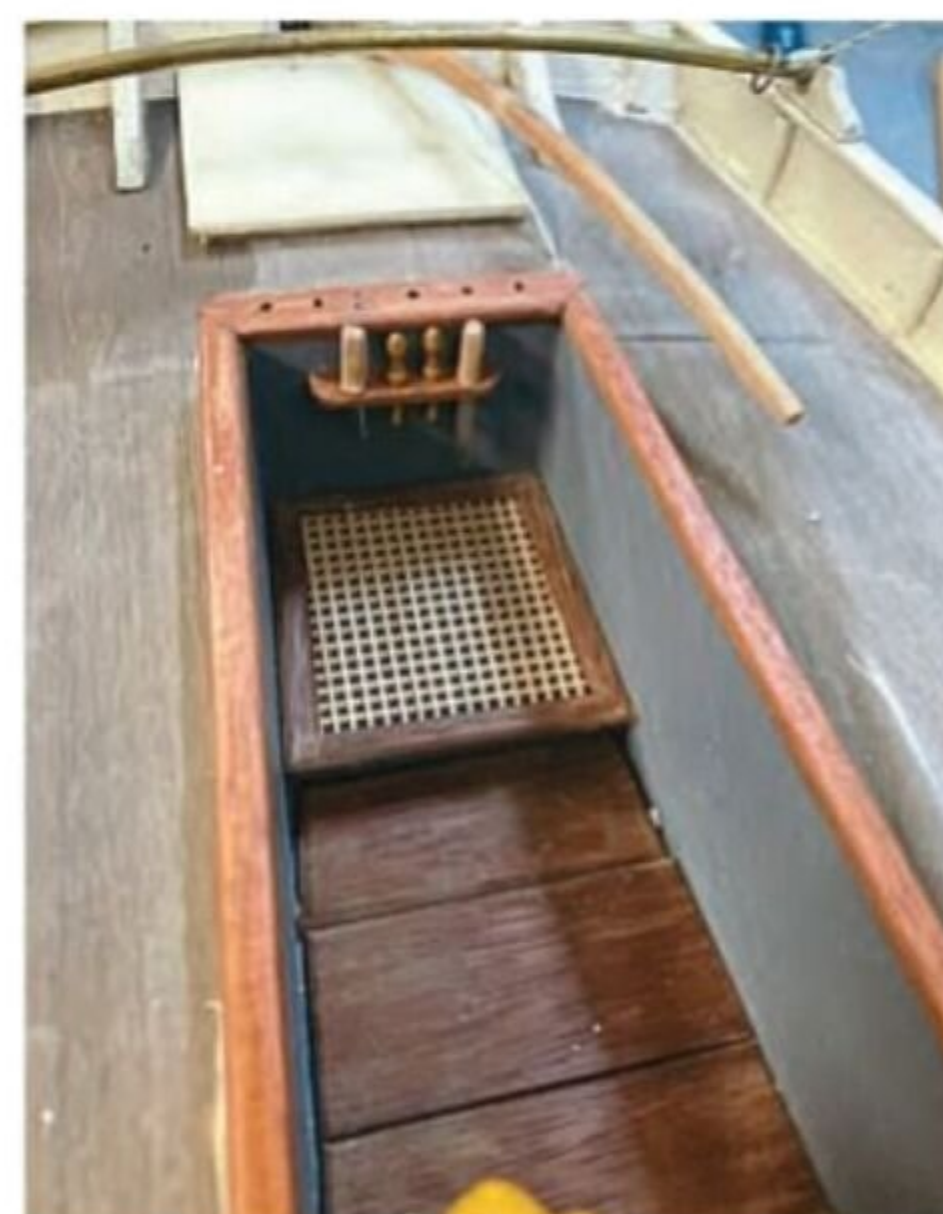
The pin rail on Peter's model: on the real vessels wooden pins could be dropped in either side of the tiller to keep the boat sailing on a steady course while the crew were busy working with the catch on deck.
