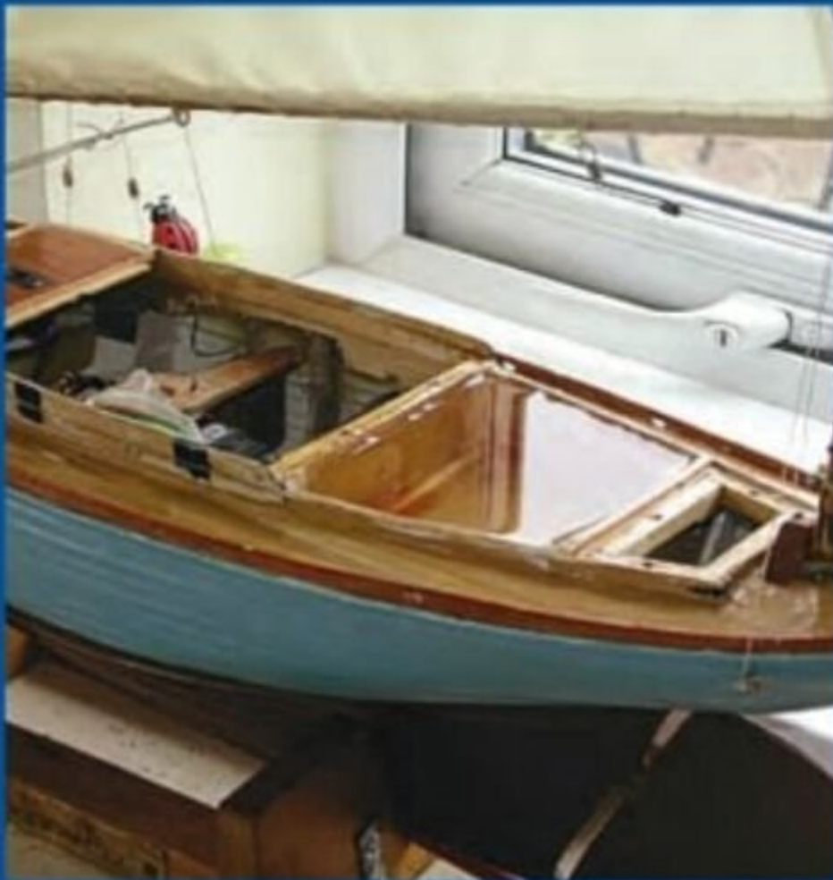
Testing the watertightness of the 'swimming pool'. Nev filled it full of water and left it for half an hour to see if the level dropped. It didn't!
