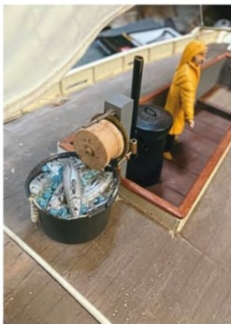
The 'wink', a hand-cranked device for hauling in the nets.
