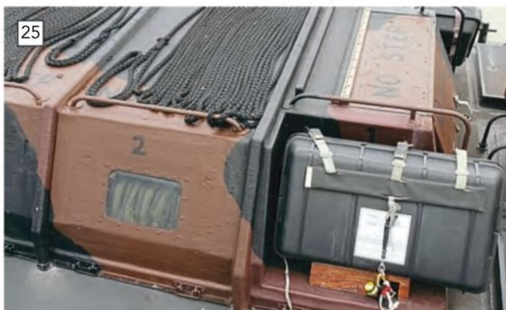
Fixed to the lower edge of each section of the arctic cover are two lifting handles.
