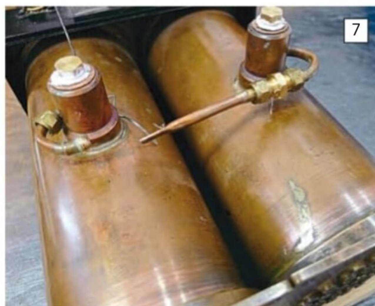
The boilers can actually be considered as separate from the feed side as there is an isolation valve to each boiler. The single pump is not an issue, but it does mean that Clause 11.7b of the 'Orange Book' must be complied with.
