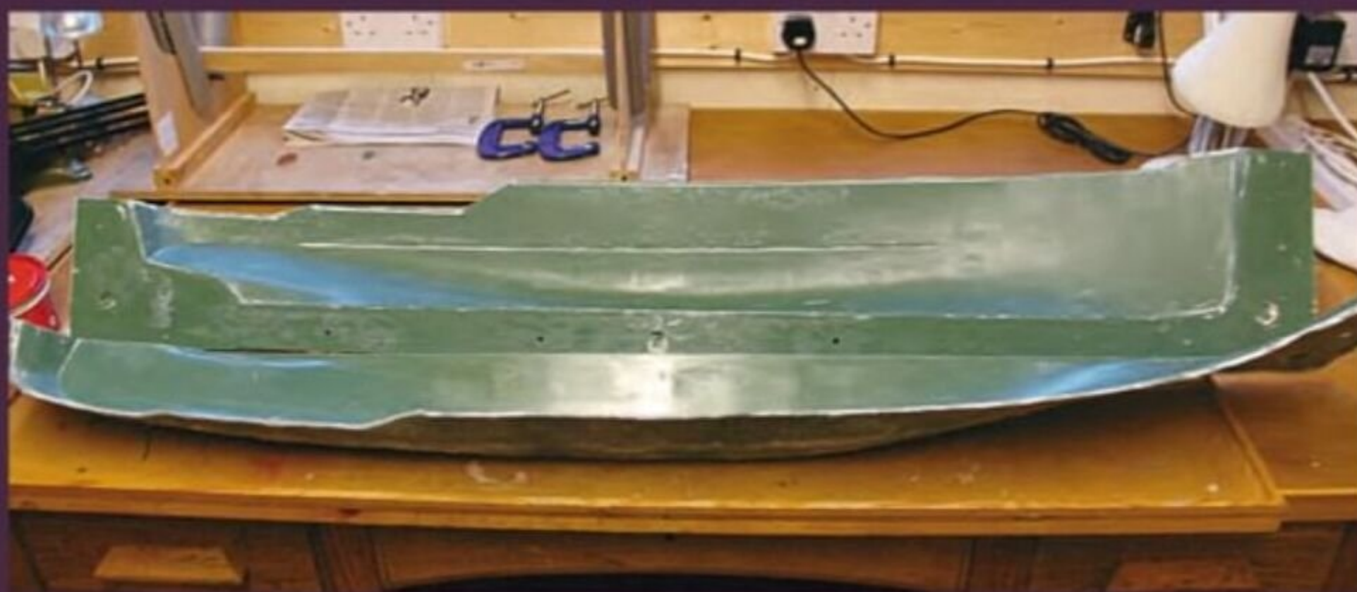
Because of the vertical inwards taper of the hull, the mould needed to be made in two halves bolted together that could later be split to release the hull.
