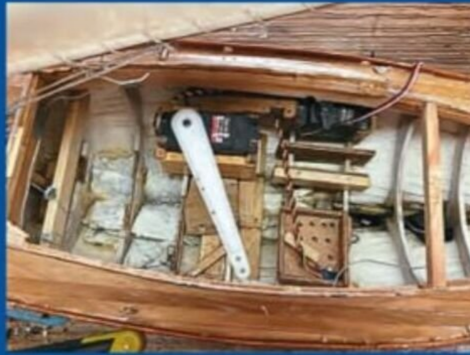
In 2021, the whole watertight 'upper deck' was cut off so that Nev could examine the possibilities. The original arrangement of the sail arm servo can be well seen in this shot.
