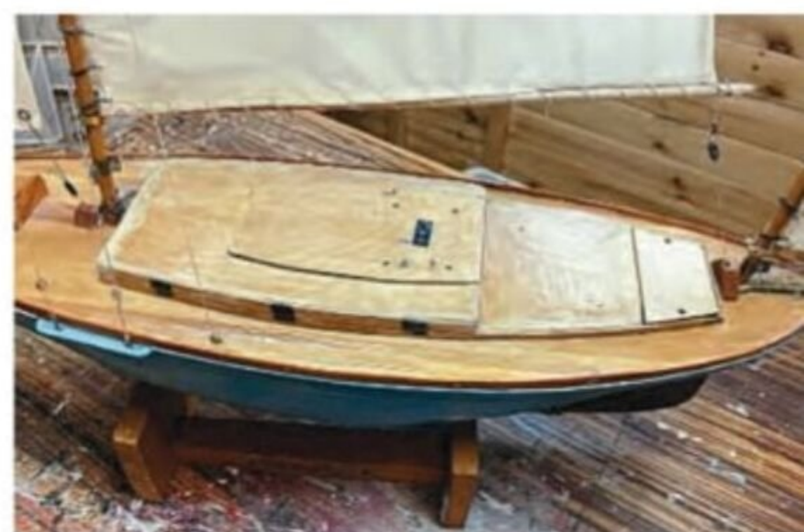
Back in 2006, Nev felt the solution to making the boat watertight was to enclose everything in as simple a way as possible.
