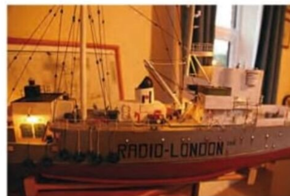
Nick used a mixture of LED and grain of wheat bulbs for lighting his model, but definitely favours LEDs due to the availability of bright or warm white as well as a good variety of colours.
