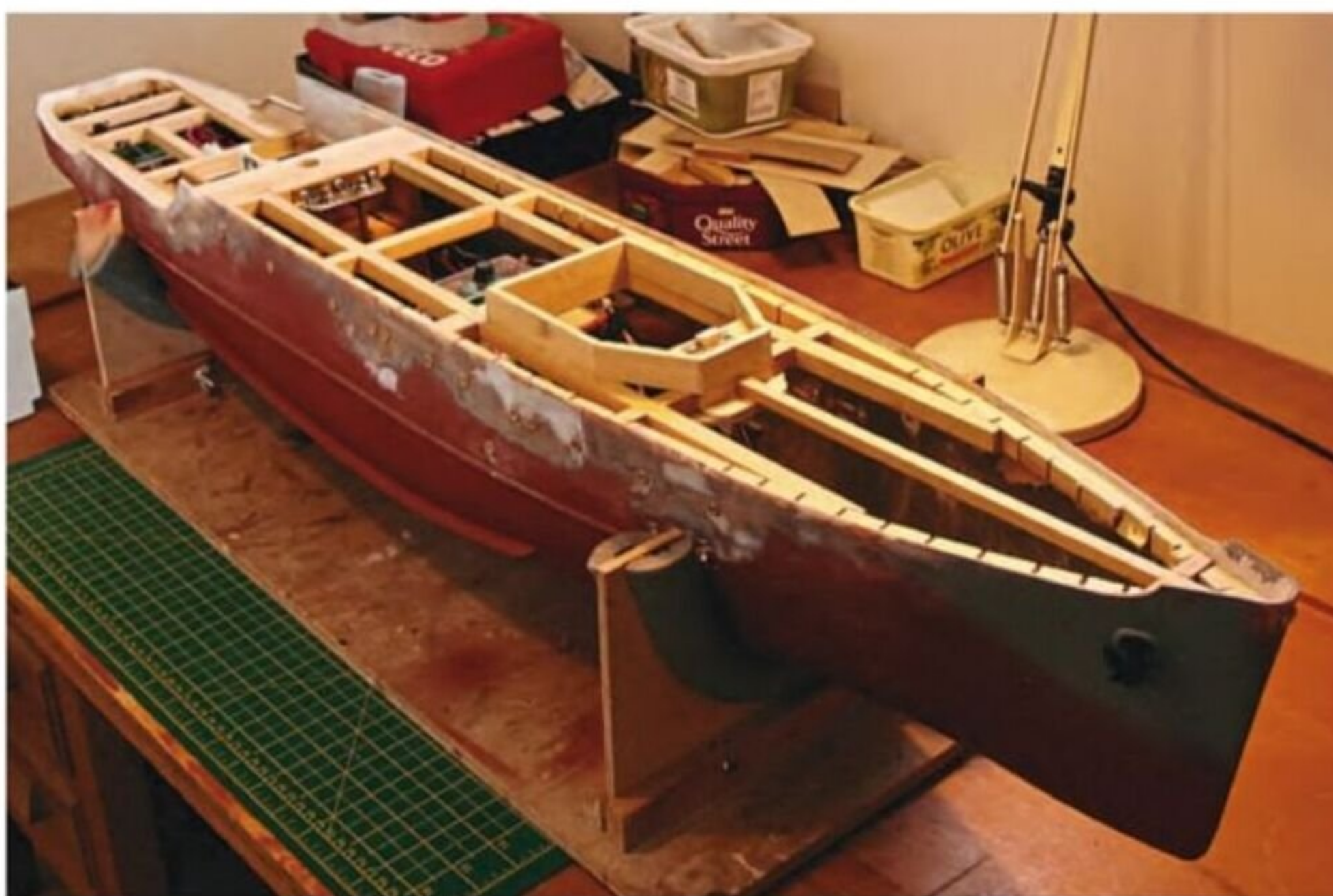
The deck supports were all made using 10mm square wood jointed to provide access points for the wiring, motors, etc. Below: The radio receiver, speed controller and power distribution board for the lighting circuits.
