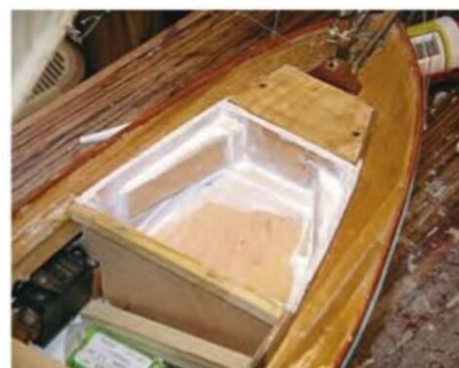
All the joints sealed with decorators' caulk. The next job would be to apply resin and then varnish to make this 'swimming pool' watertight.
