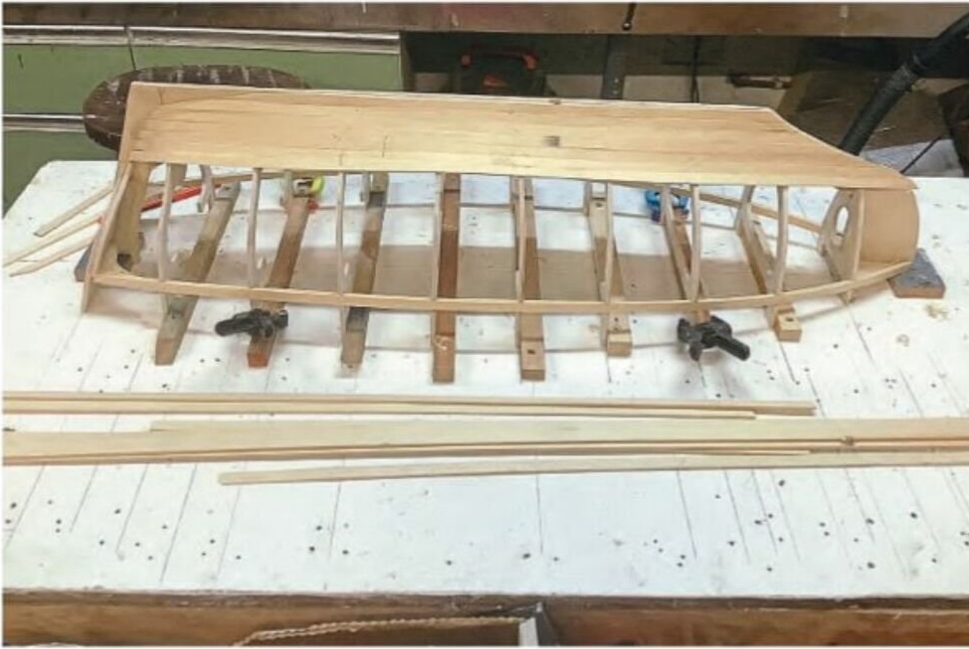
Set up on Peter's building board, with the first few planks fitted, work begins on the Mary Ellen .
