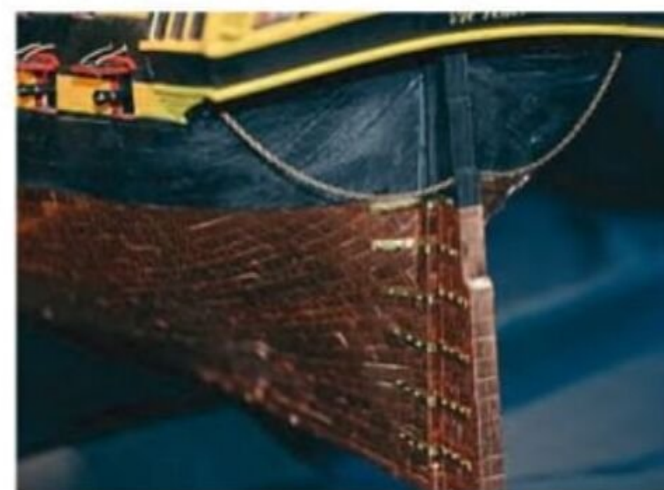
2,200 individual pieces of copper plate were painstakingly applied to the hull of John's Victory.
