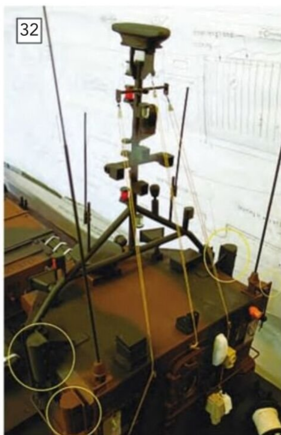
Atop the wheelhouse roof are various fittings clearly defined on the drawing, together with four buffers (all ringed in yellow), two on each wheelhouse side.
