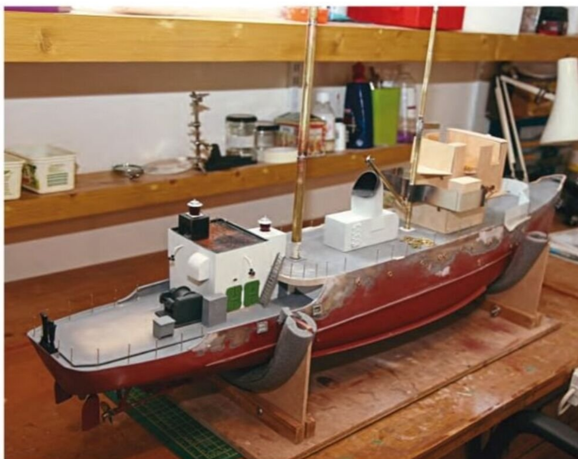
Superstructures in the process of being built, showing (stern to bow) the minesweeping winch, transmitter room, funnel and below decks access doors, main ship's mast and, lastly, the ship's main superstructure.
