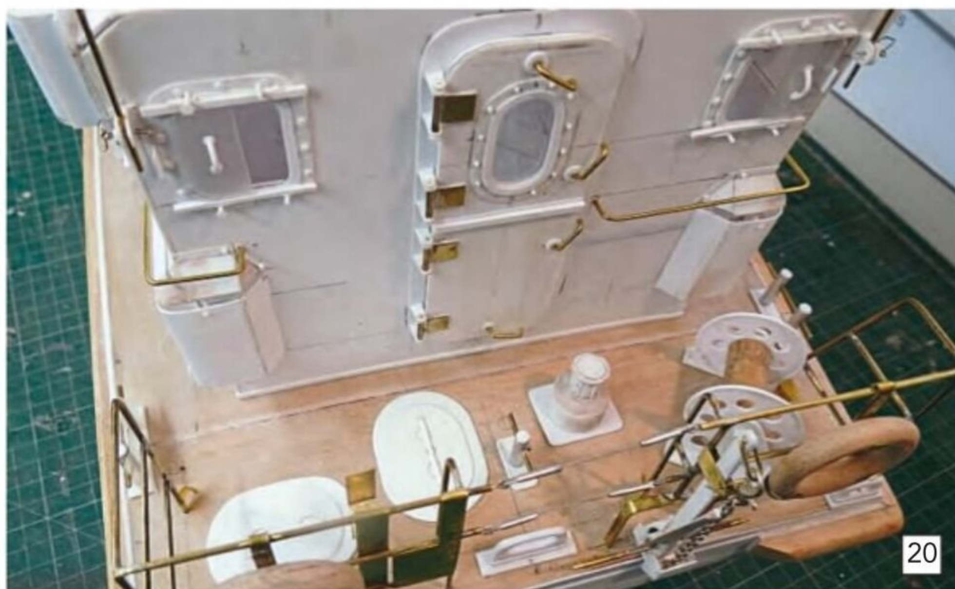
The wheelhouse door in place together with all the transom overhang deck fittings.
