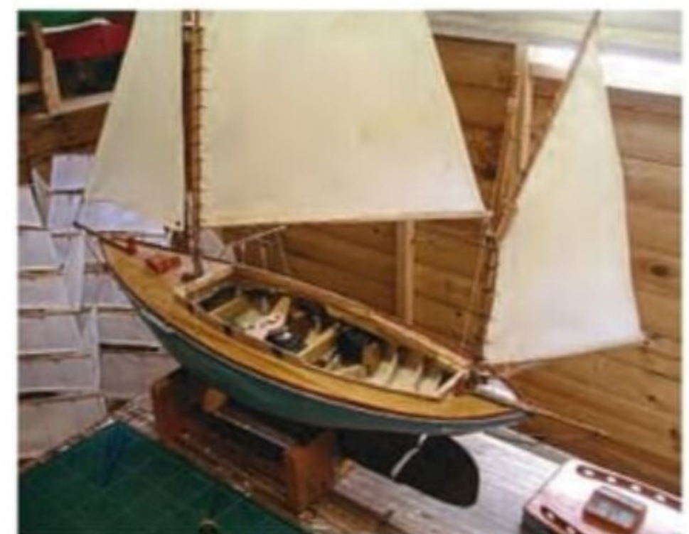
Work on the sheets complete. The fore sheet is visible running forward from the starboard end of the servo arm.
