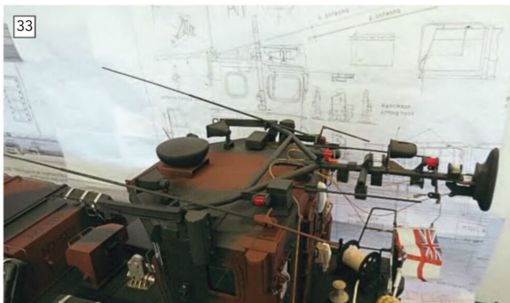
Just like the full-size LCVP Mk. 5, the mast and whip aerials drop down to lay on the roof.
