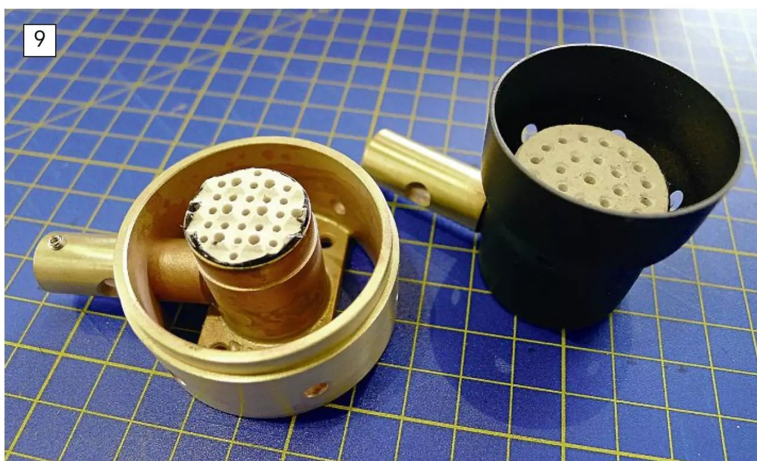
Typical ceramic disc gas burners, both by Miniature Steam for vertical boilers, the base mounted one on the left and the side mounted one on the right.
