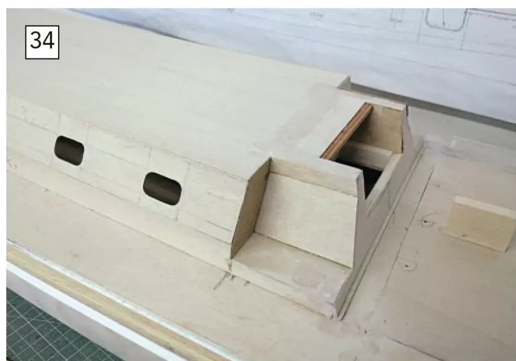
Cladding the arctic cover with .50mm marine ply and forming what will become the control box, as per the drawing.
