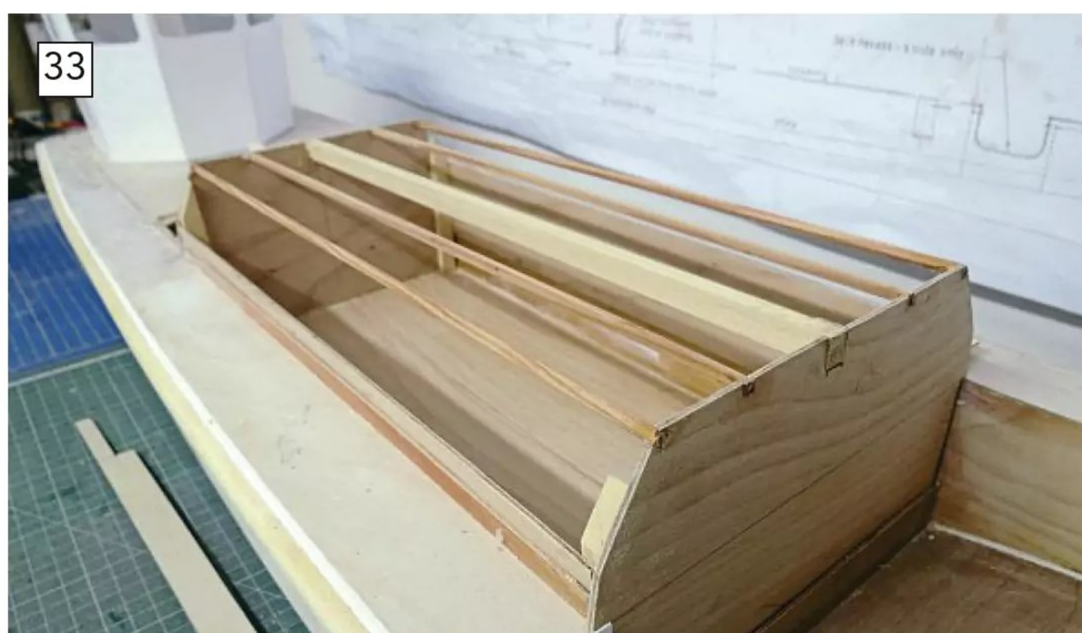
Forming a one-piece arctic cover to fit over the vehicle deck.
