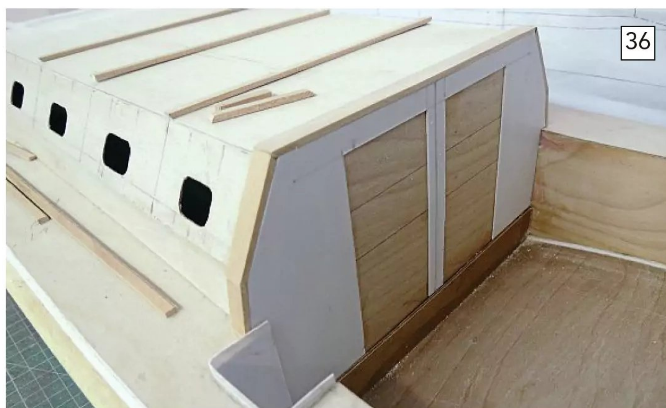
Preparing the arctic cover forward bulkhead with door openings.
