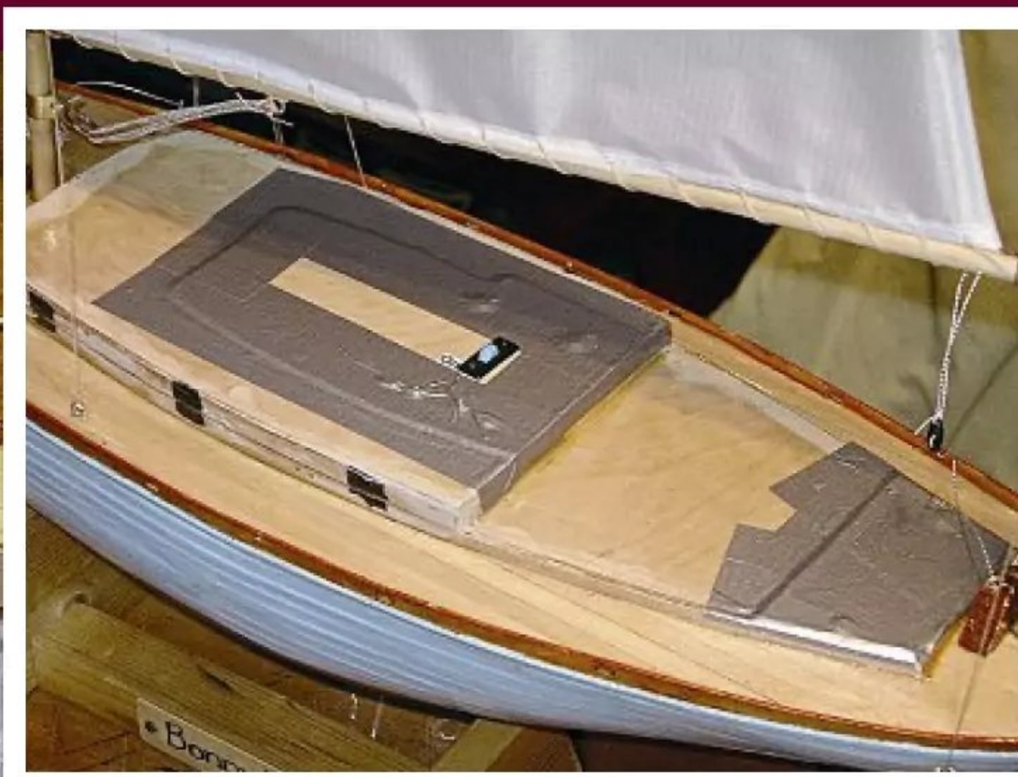
The final arrangement of the deck and its waterproofing. Now only the two taped hatches give access below deck.
