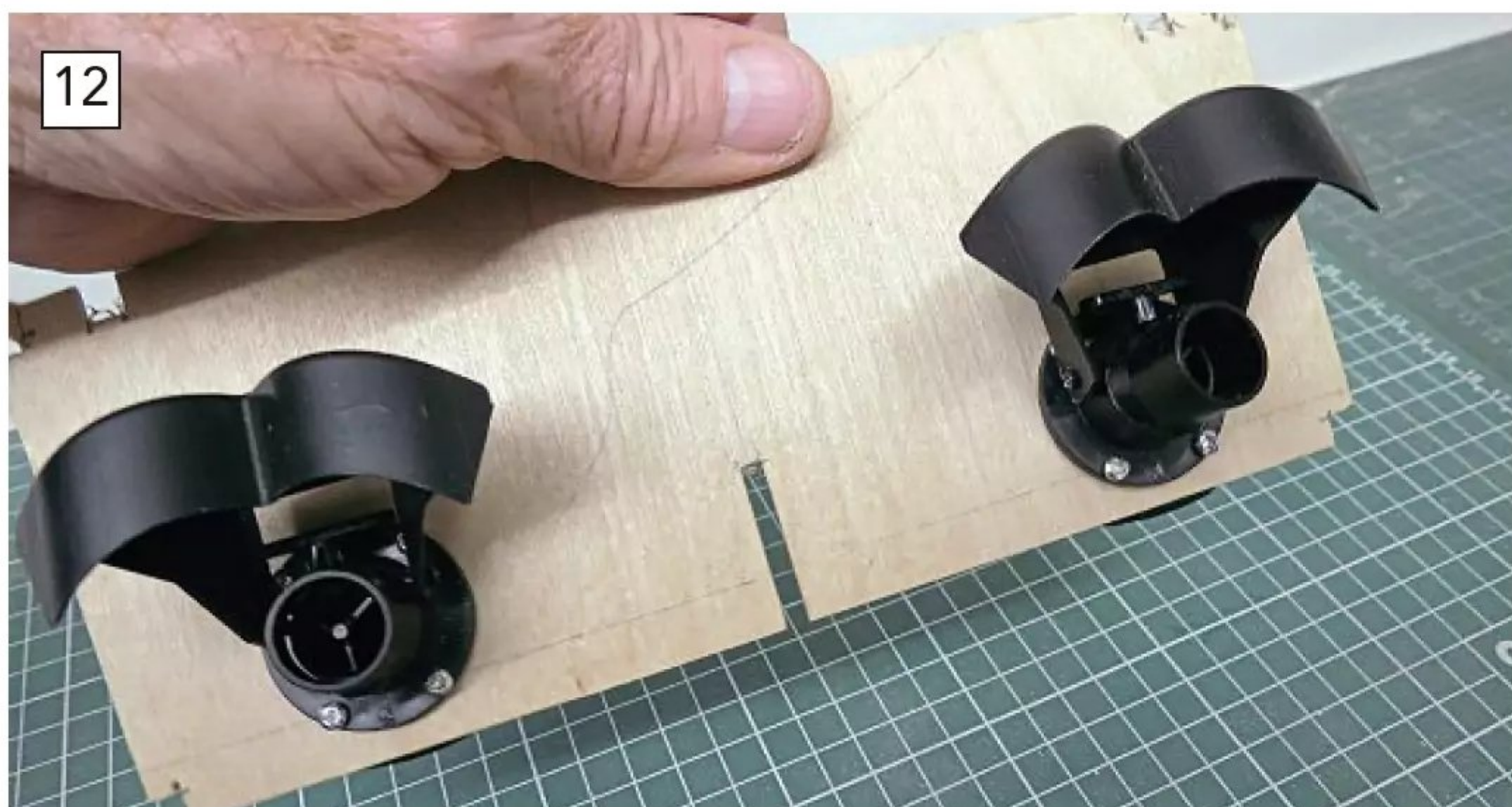
Water intake on the Bauer water jet unit.
