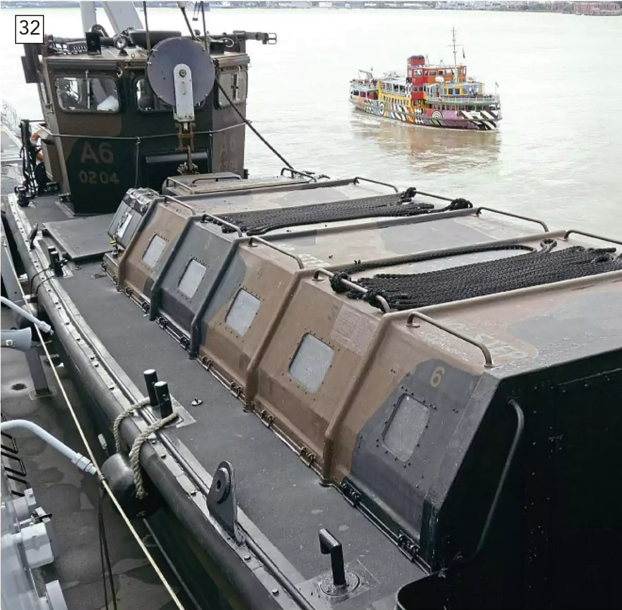
The arctic cover on an LCVP Mk 5 aboard HMS Albion looking aft.
