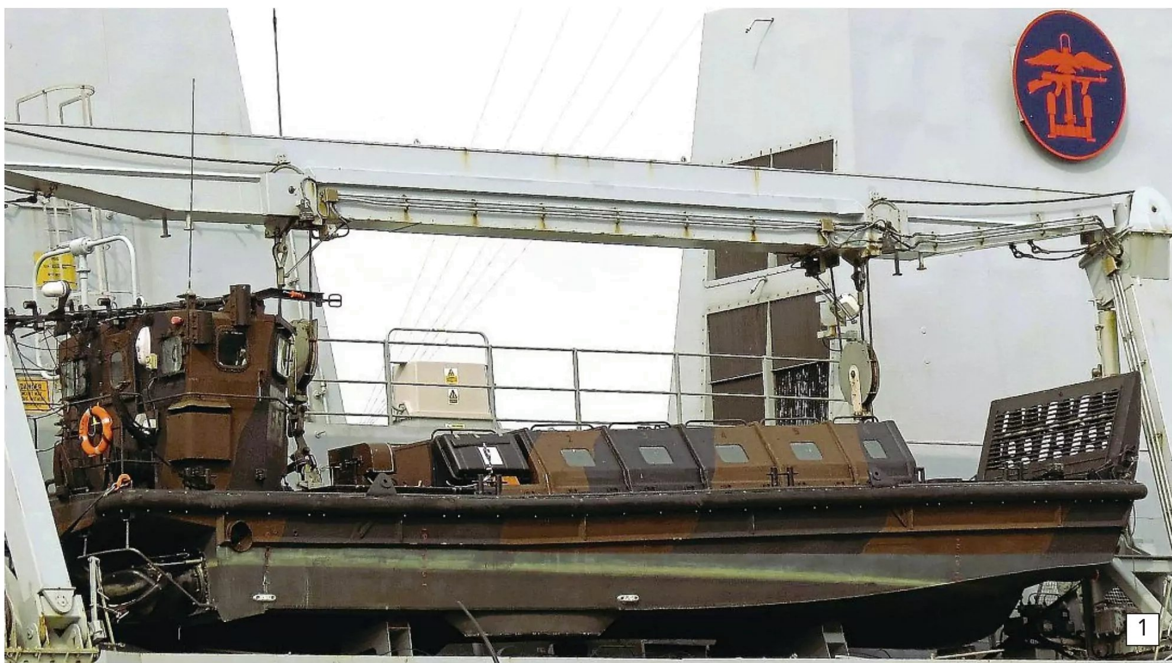
LCVP Mk.5 secured to its goal post davits aboard HMS Bulwark LPD (Landing Platform Dock) after a successful exercise.
