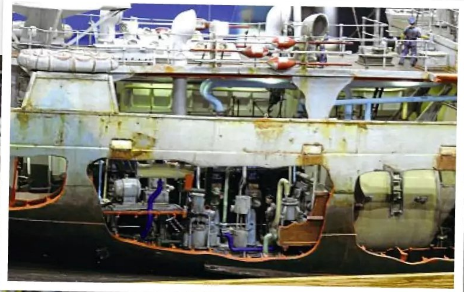
Left and above: Barry Sharman's 1:72 scale Flower class corvette HMCS Agassiz, cleverly designed and constructed to afford views of the internal fittings in the engine room, boiler room and radio room.
