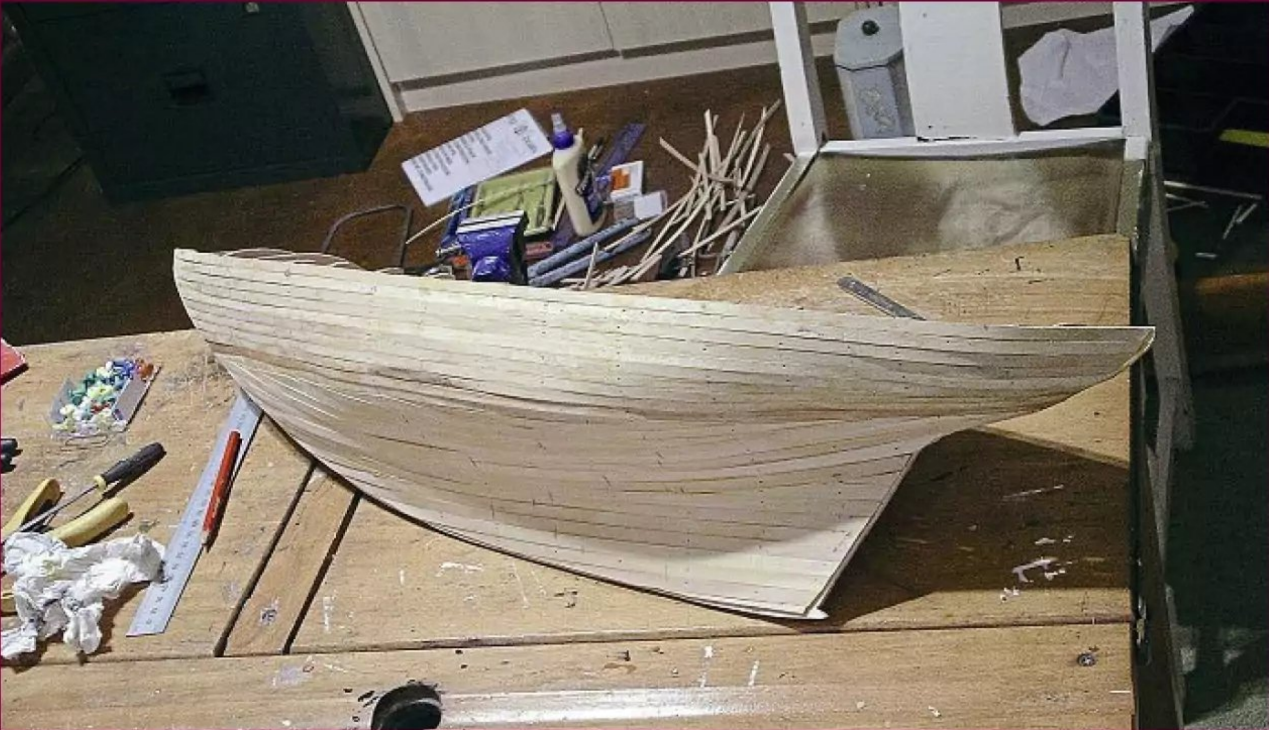
Bonny Lad after planking. While acknowledging he is no yacht expert, Nev believes she has what's known as a 'spoon' stern.
