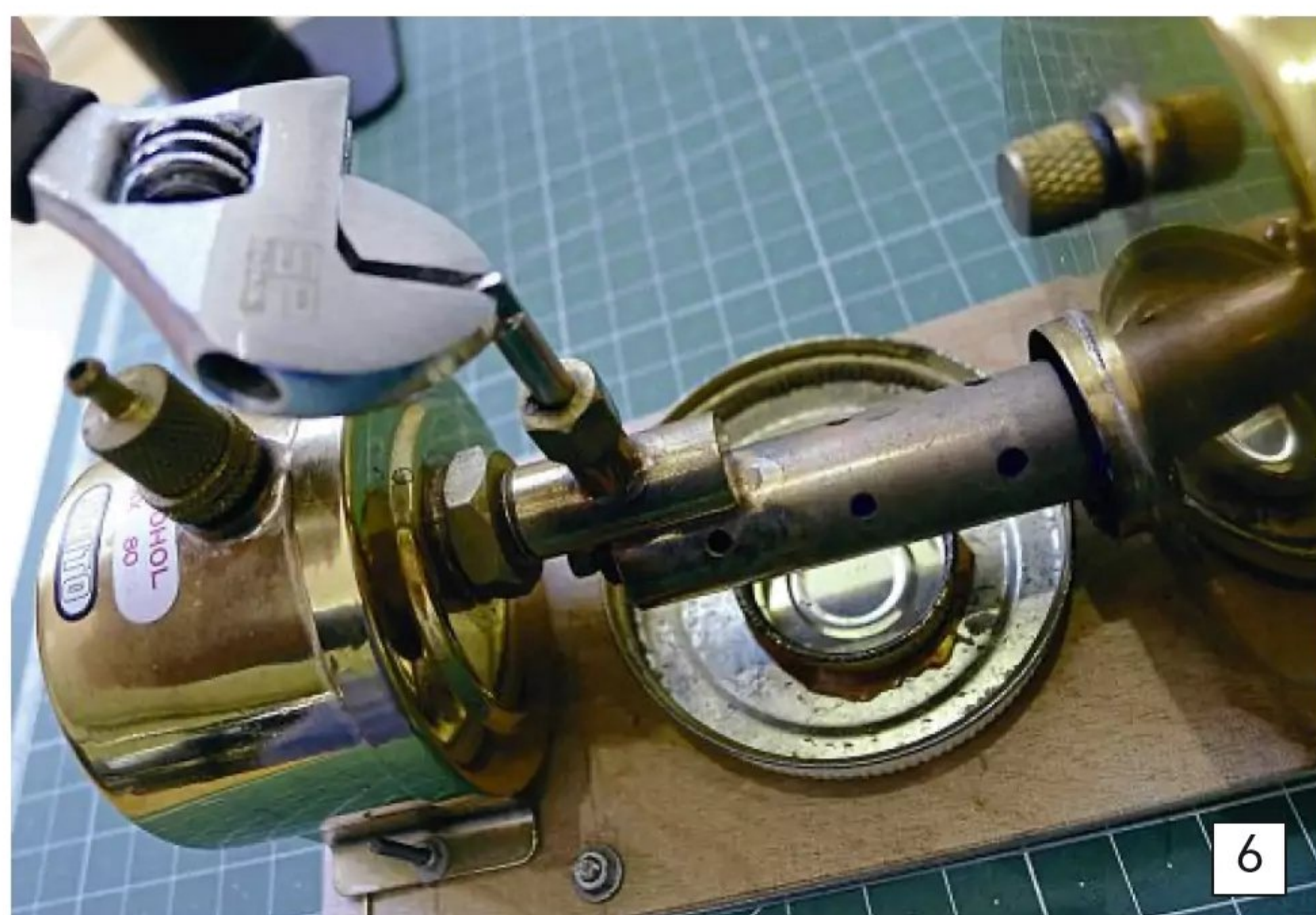
As soon as you crack open the metering valve the fuel should ignite in the burner, and you will hear a gentle roar. Only open the valve further as the burner continues to heat up and transfers heat to the tank. There will come a point where opening the valve further will have no effect.
