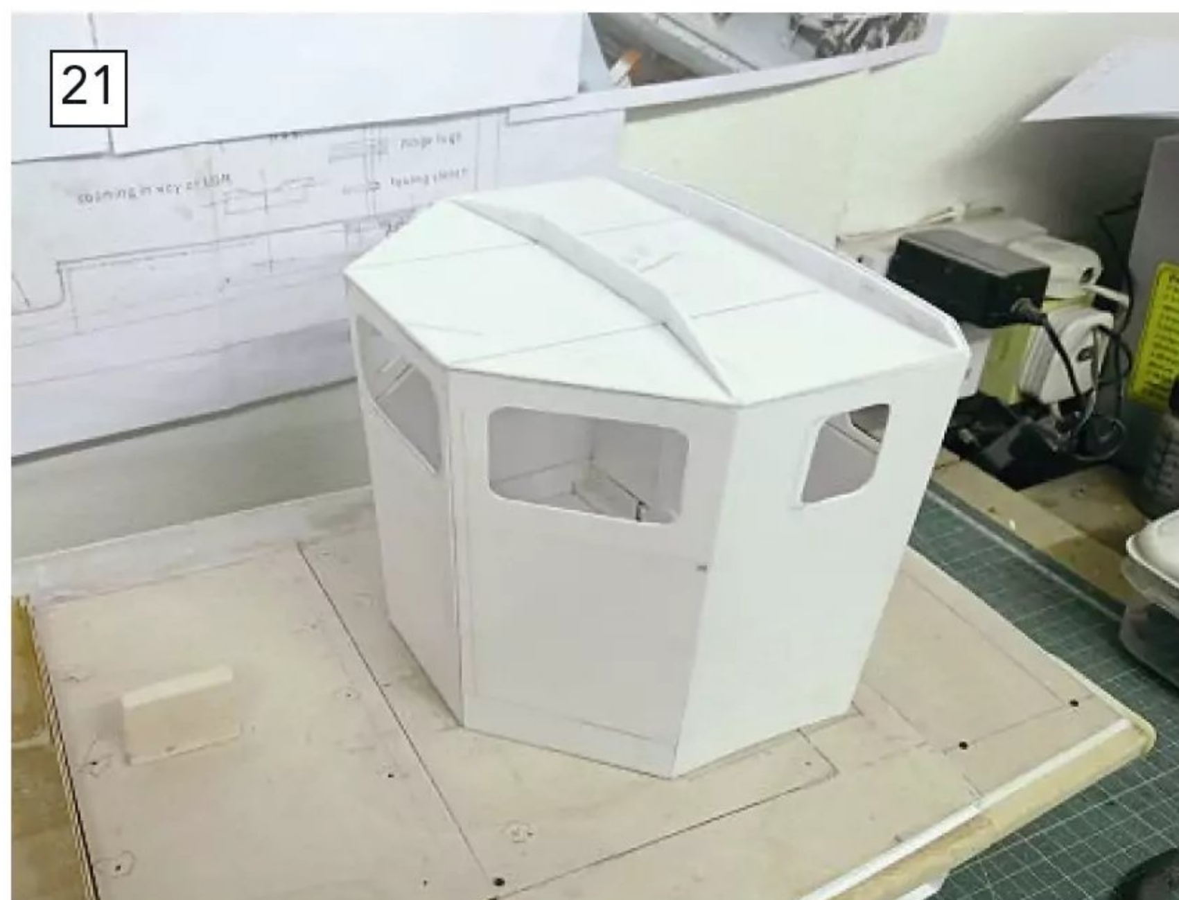
Forming the curved roof of the wheelhouse.
