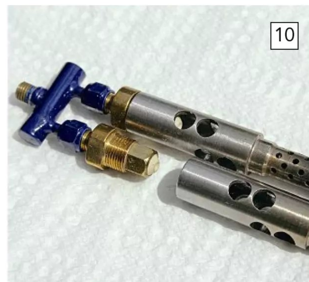
Another fairly typical gas burner arrangement is the poker burner. This one, actually fitted with ceramic tipped nozzles, is manufactured by Hemmens and used in its Ribbersdale horizontal boilers.
