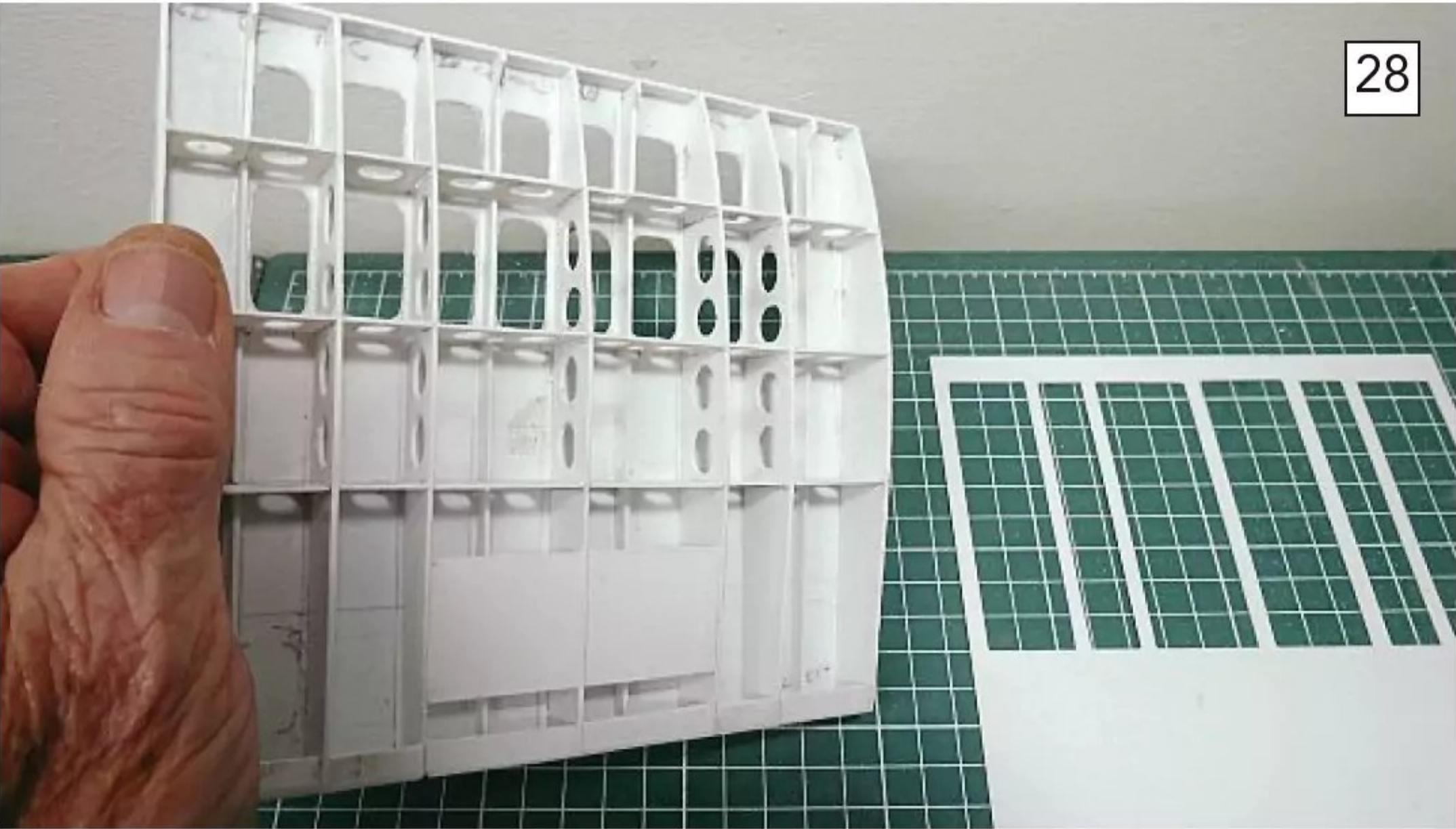
All the ribs and webs in place on the ramp floor.
