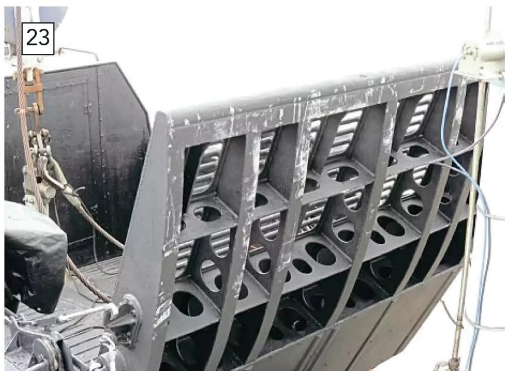
Honeycombed and light, the ramp as fitted to the LCVP 5.
