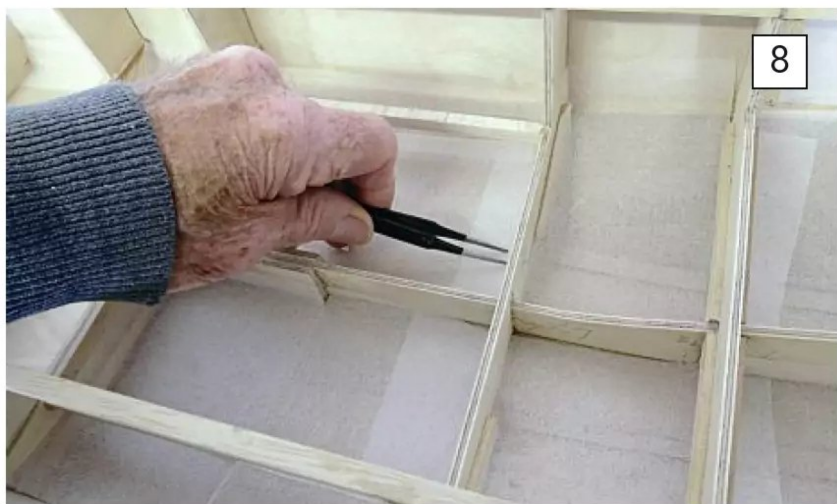
Glass fibre is applied to inside the hull and coated with GRP resin.
