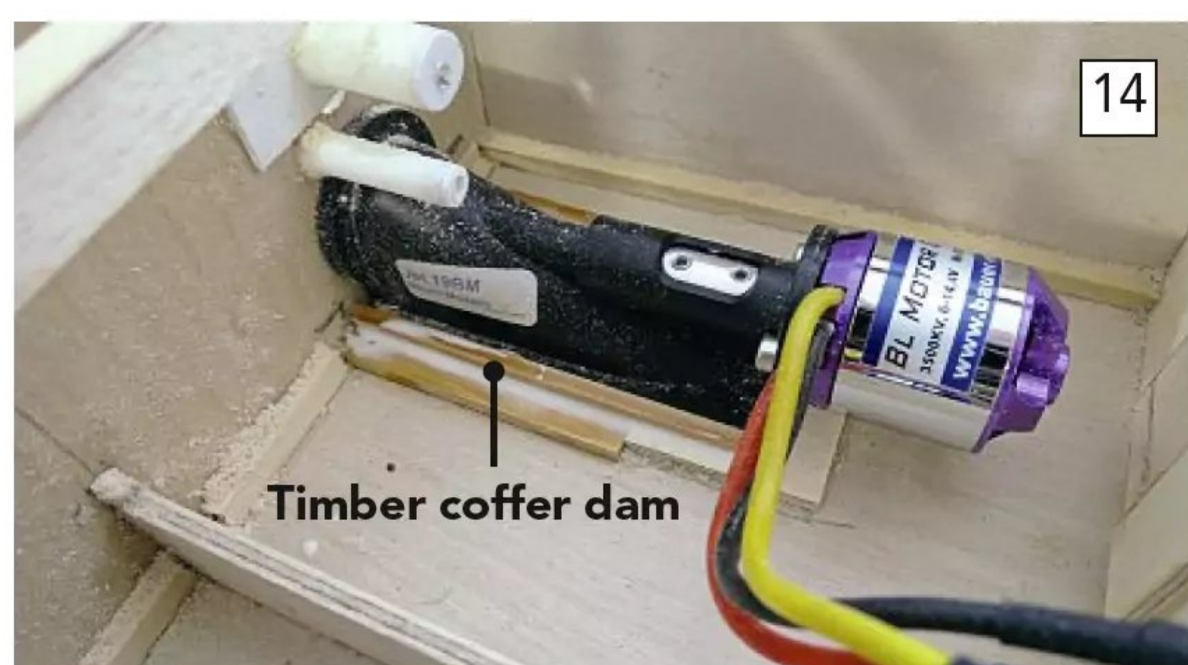
The water-jet unit and brushless motor fitted into the coffer dam to correspond with the inlet opening beneath the hull.
