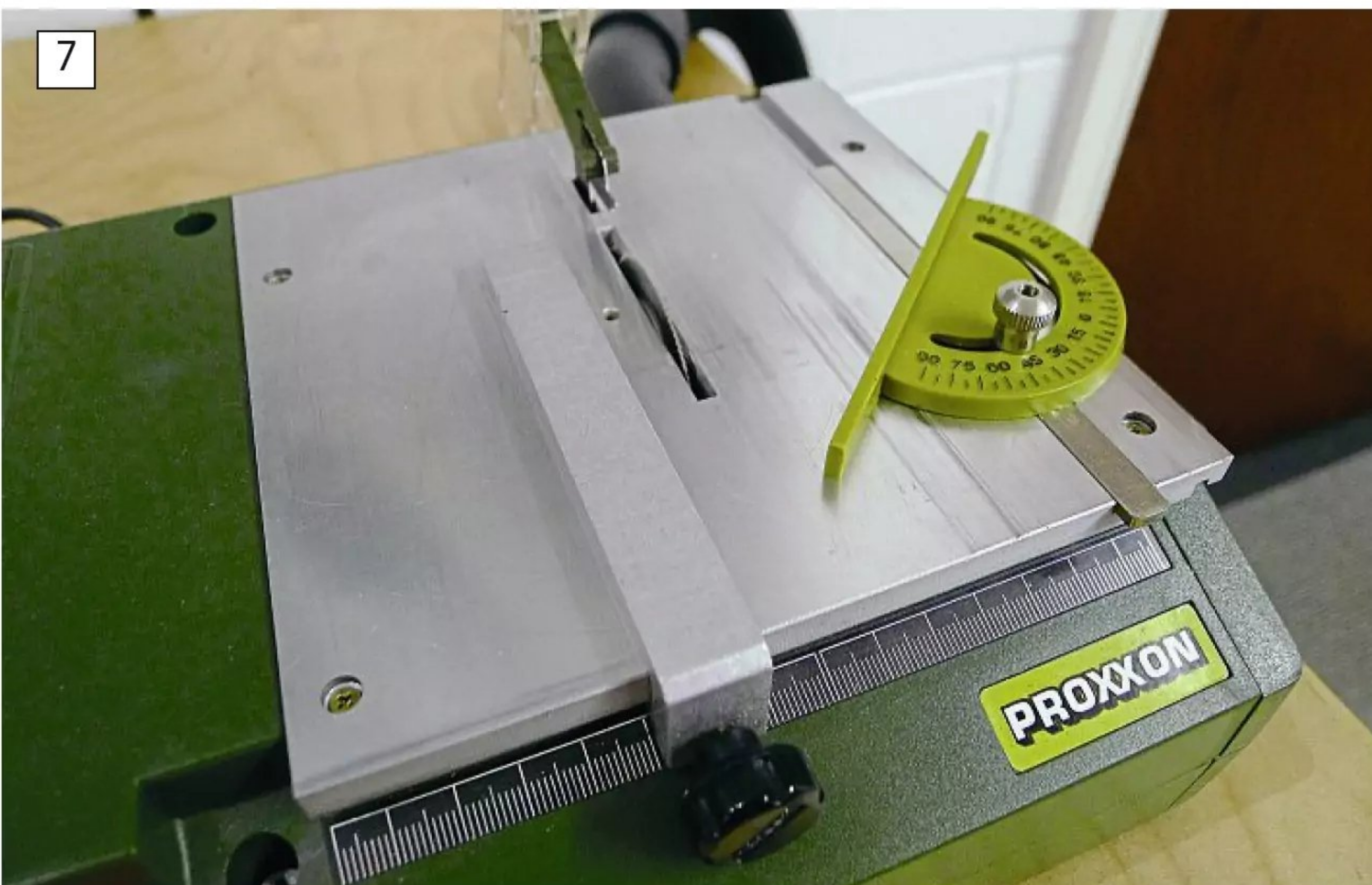
After changing the mitre setting a number of times, Richard decided it was worth another five pounds to buy a spare mitre and leave it set at 45 degrees. This means that framework corner braces can be cut in seconds and will fit perfectly.
