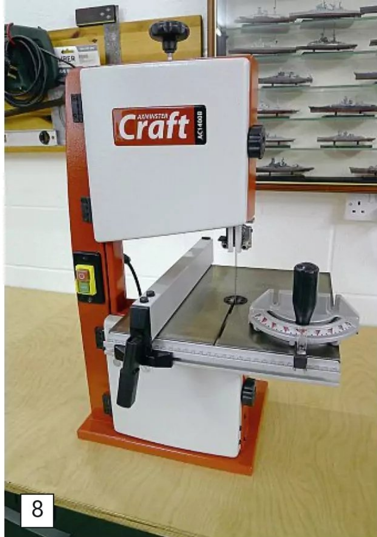
The band saw is bolted right through the 1-inch-thick benchtop with four 8mm bolts, making it very secure. Mounting it on a standard height workbench puts the table at a perfect height.
