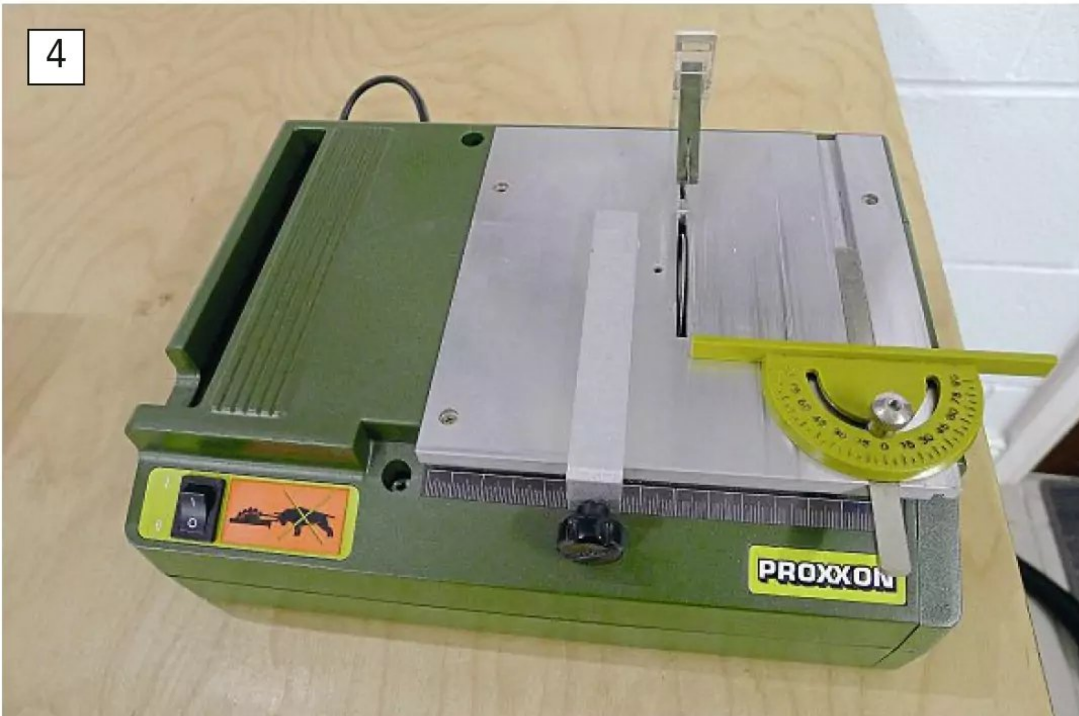
Richard settled on the Proxxon KS230 table saw. Small and compact, the blade does not tilt but the standard supplied blade cuts woods, plastics and non-ferrous metals without having to change it. Versatile, accurate and incredibly handy.
