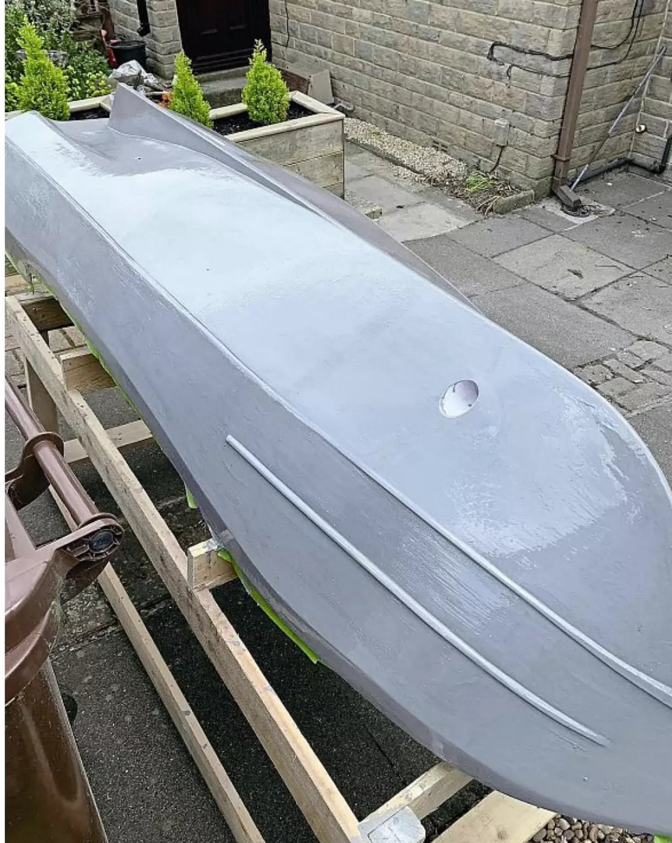
The inverted hull drying after wet sanding and a final coat of polyester resin having been applied.
