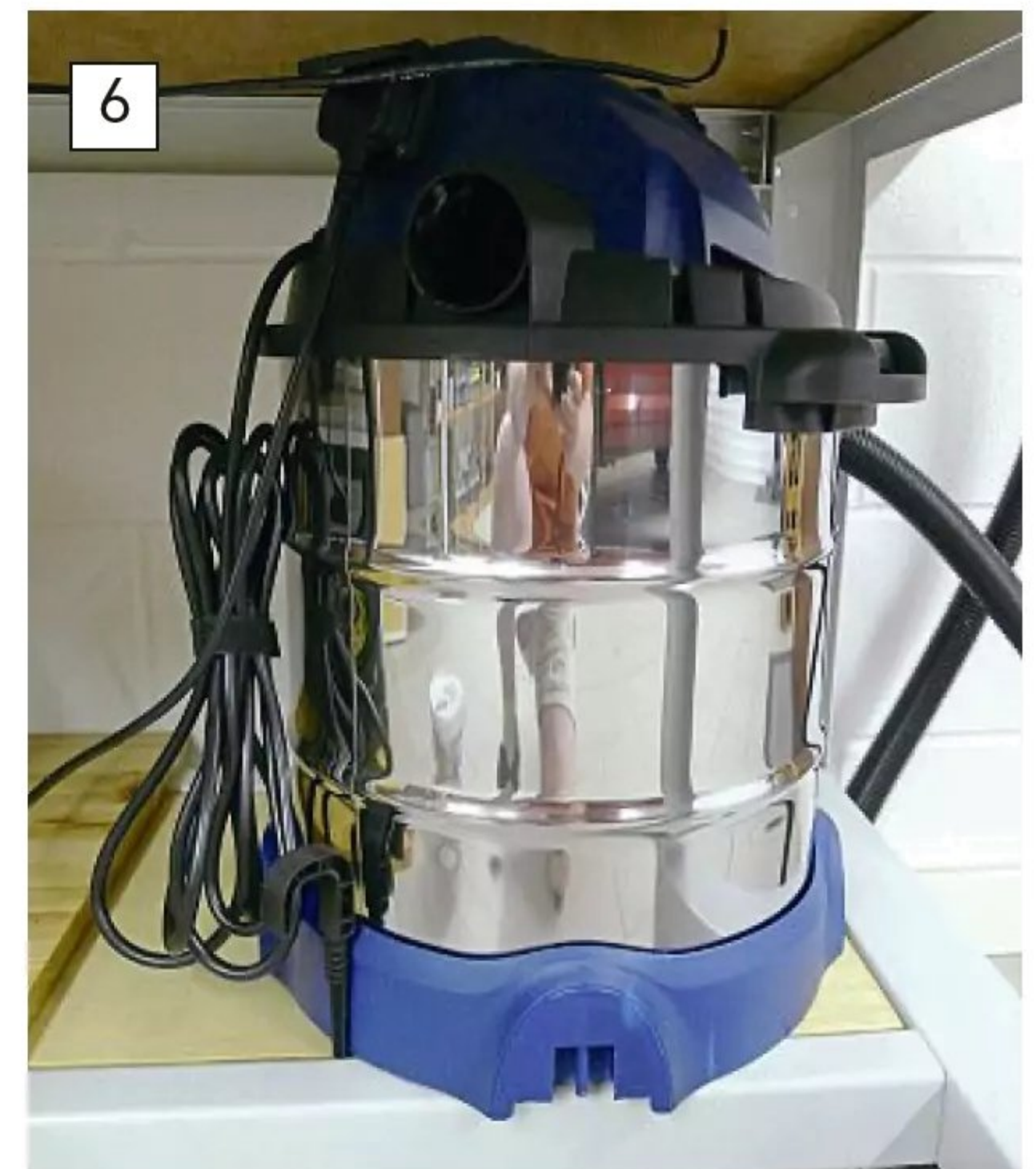
The Draper vacuum unit has a socket on the head to connect the saw into. This means that the vacuum unit becomes a slave to the power saw. It turns on immediately the saw is turned on and turns off just a few seconds after the saw is turned off.
