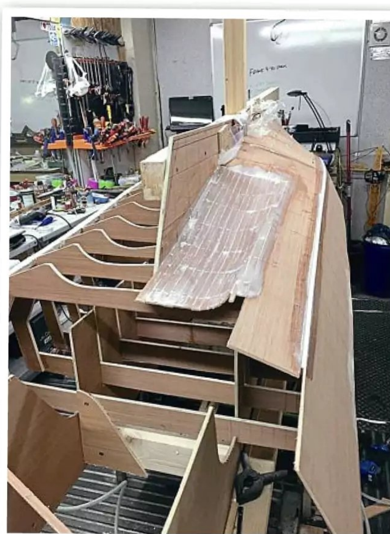
Fitting plywood sheeting to the hull frames.
