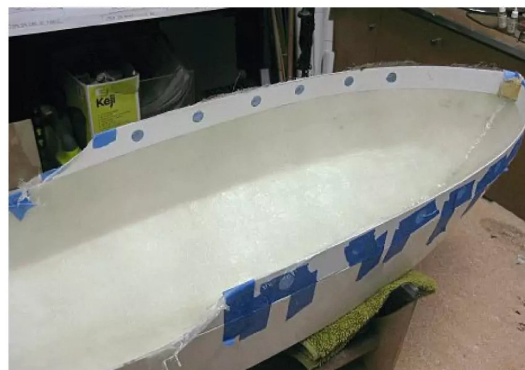
Above: Once the raised sides were glued in place and fibre-glassed from the inside, they ended up being 3mm thick – the same thickness as the hull.
