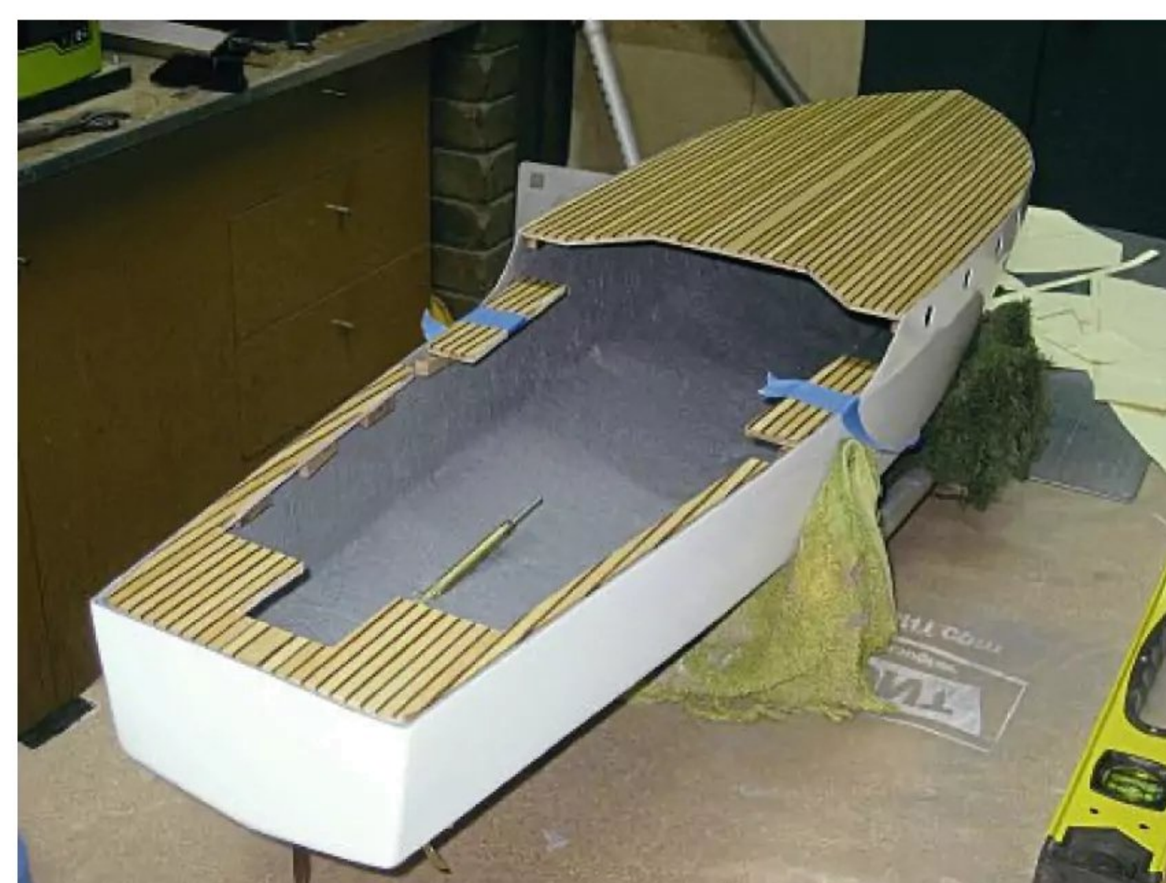
The top and lower deck installed and cut out for access to motors, batteries, radio, etc – fortunately, there was heaps of room. As Ian sells his models on (being a prolific builder but no longer able to sail his creations himself) he's installed the prop shafts and props and rudder only, leaving it up to the new owner to supply his/her own preferred gear.
