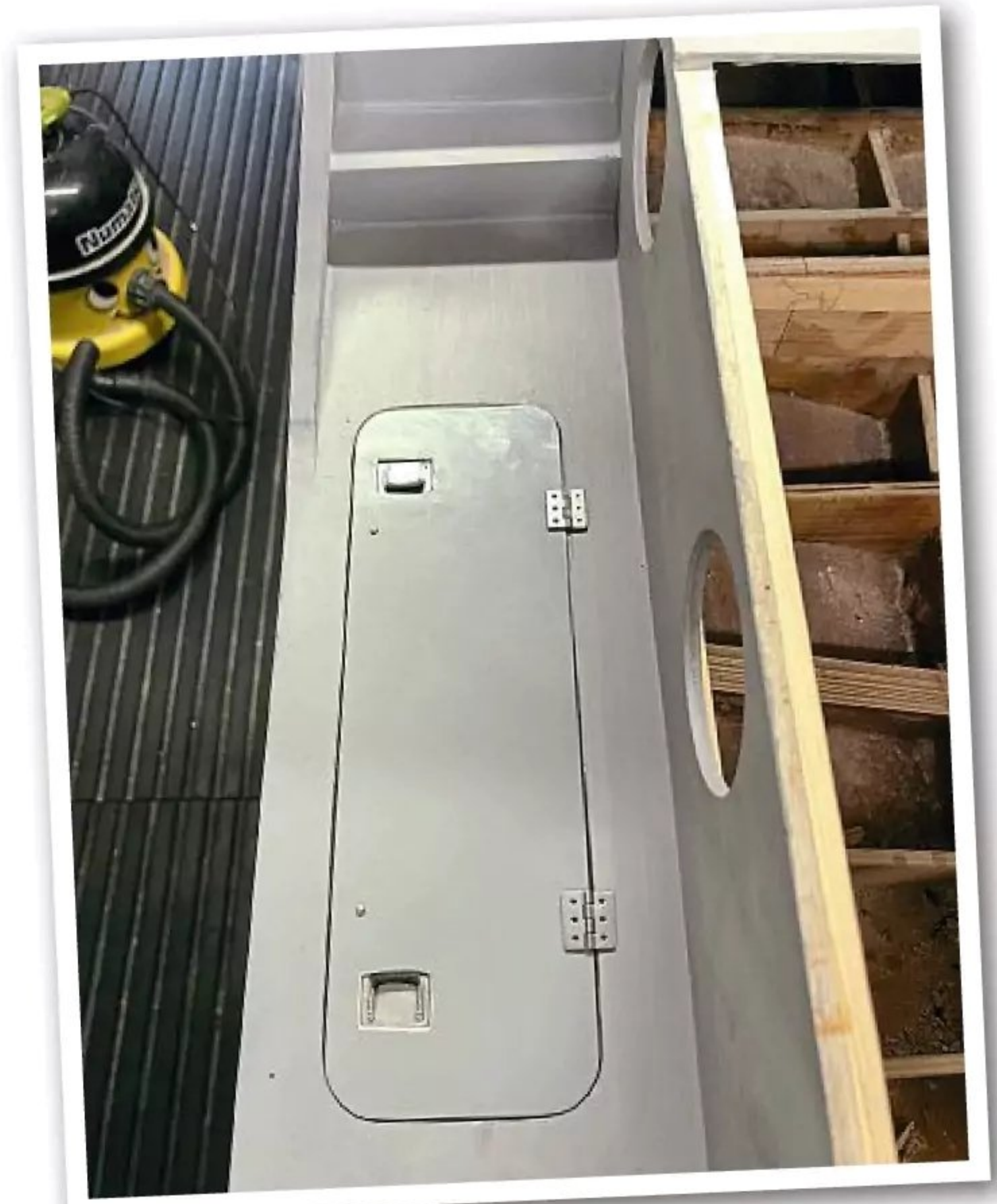
The neatly crafted lid to one of the lockers on the hull's decks.
