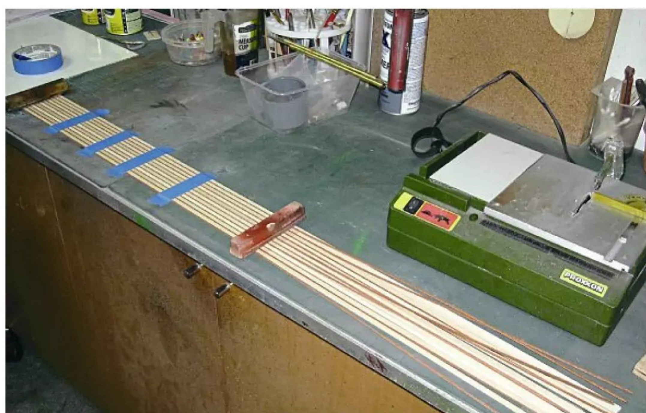
Ian laid the planks out in order on the workbench and with the aid of a sliding weight taped them together in about lots of twelve. He then brushed glue onto the decking support ply, laid the planks on this ply and weighed them down until dry. It took a few lots of taped planks to complete the deck, but the other than that the method proved quick and easy.
