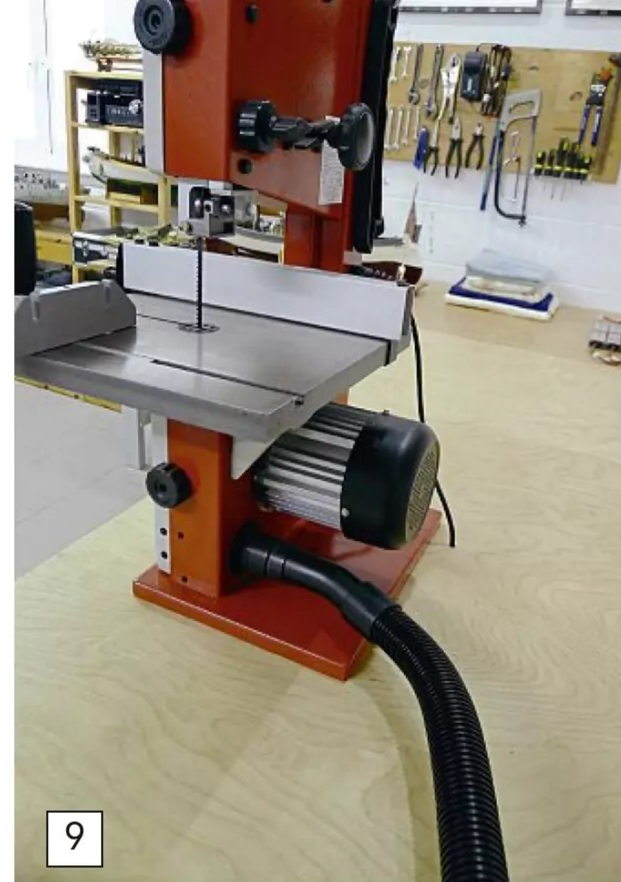
The same sized port on the back of the Axminster allows the hose from the vacuum unit to be simply pushed on when this saw is in use. Again, this keeps the workshop clean and free of any dust.
