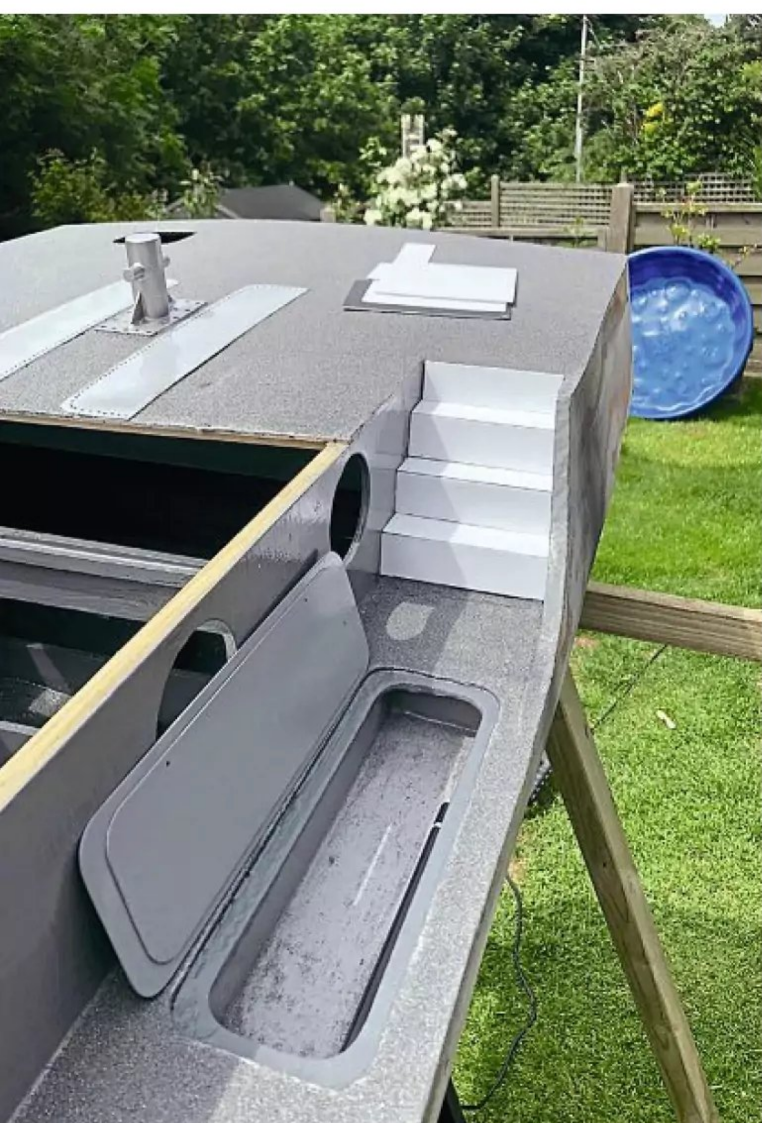
The rear decking with anti-slip texturing applied.
