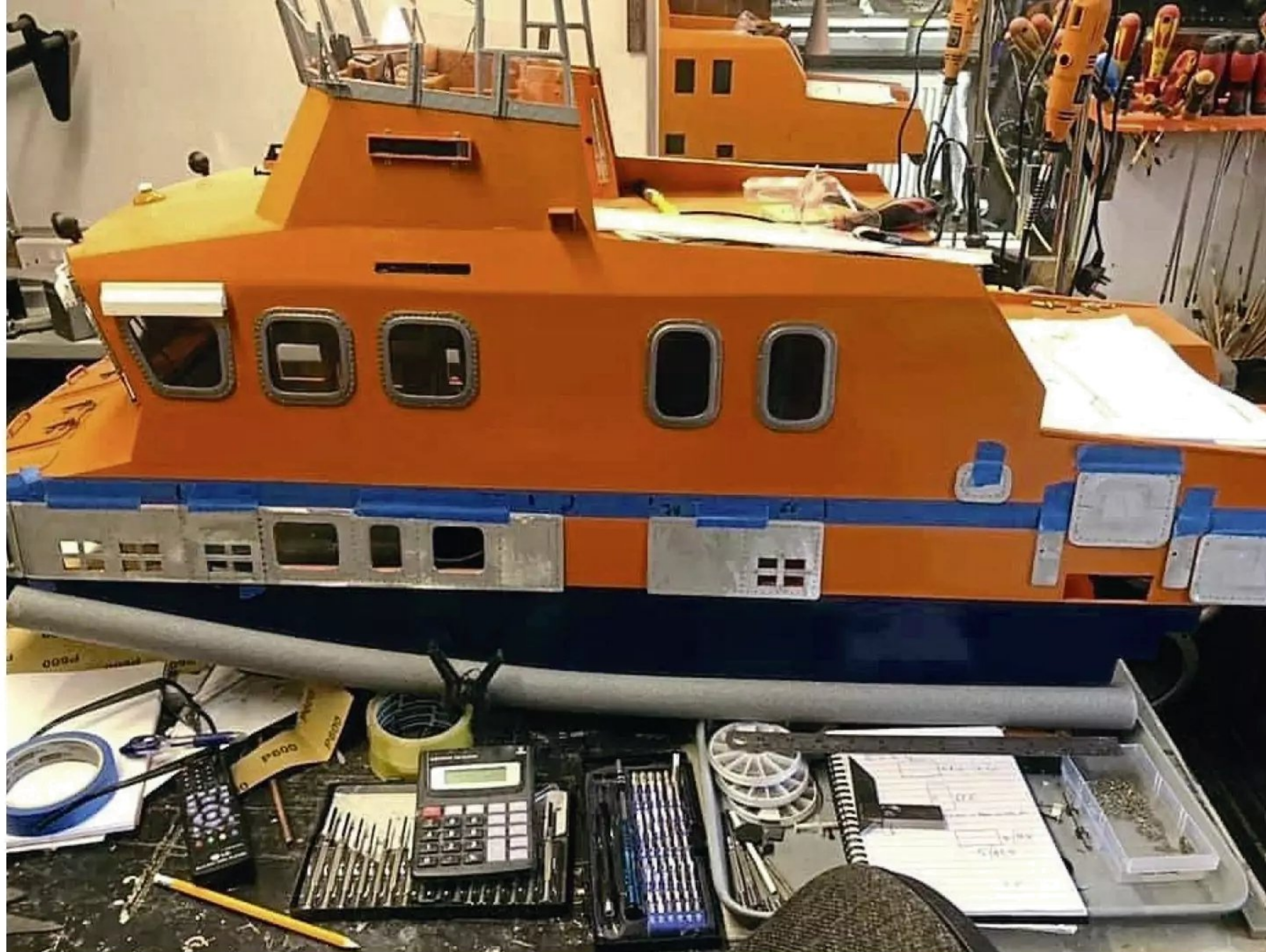
Fitting the aluminium panels to the port side.
