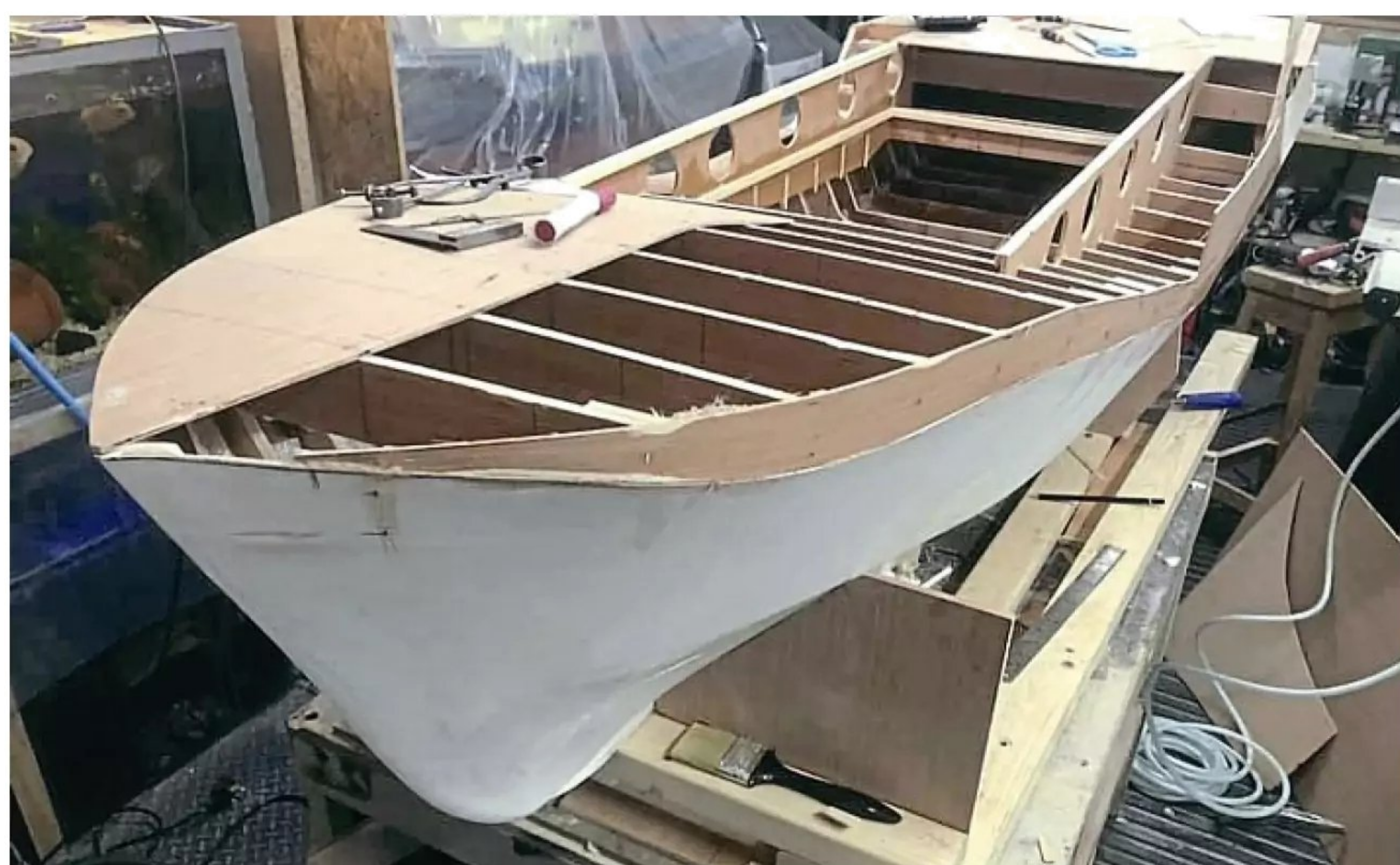
Starting to fit the decking.
