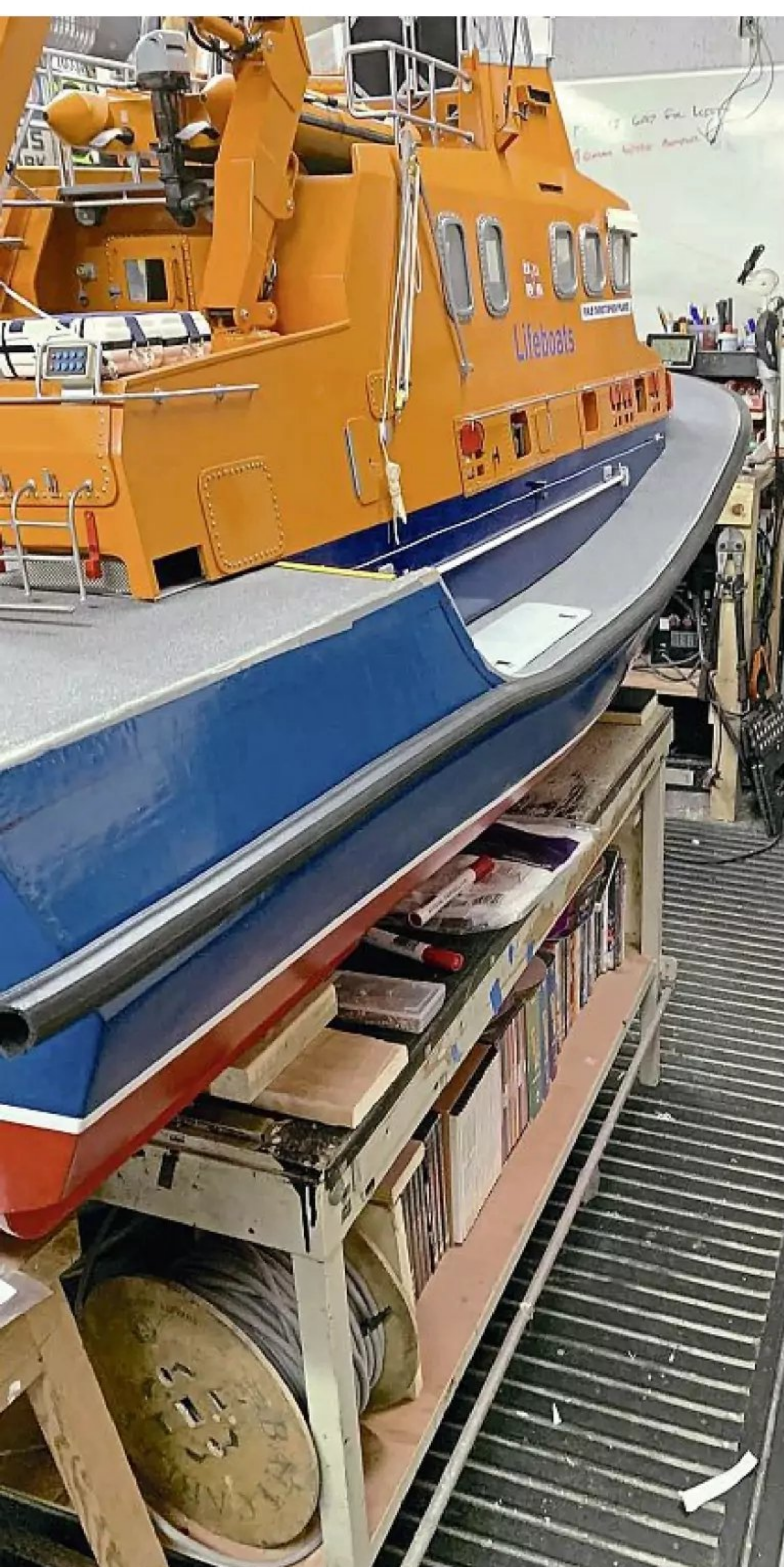
Starting to fit the rubber fender to the starboard side.
