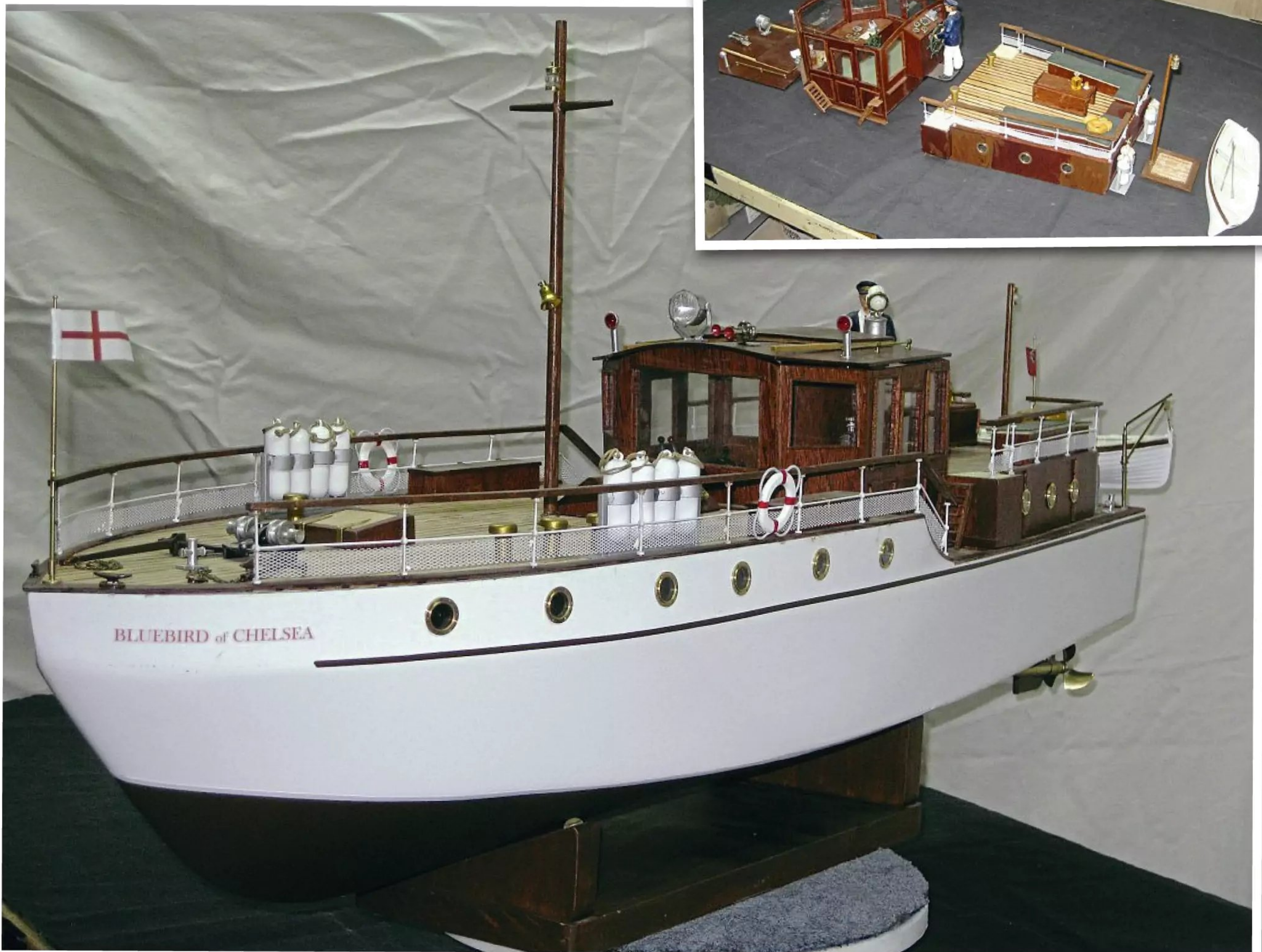
Main: The 3D-printed captain, lifeboat detail, life jackets, spotlights and horn, etc, on the cabin roof. You may also just be able to see the essential decanter of cognac – most befitting of a vessel such as this one! Inset: These components were kept removable to allow for full hull access, with everything lifting easily off.
