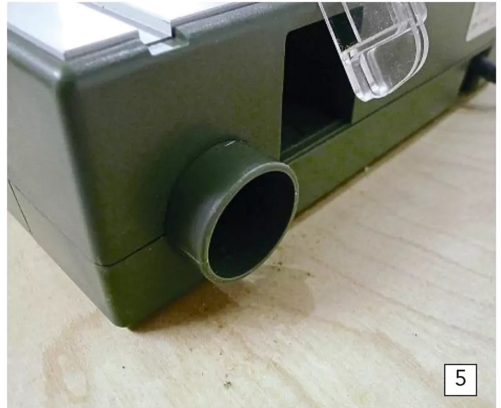
A standard size port is moulded into the body to enable an extraction unit to be fitted. This makes a huge difference to the cleanliness of the workshop.
