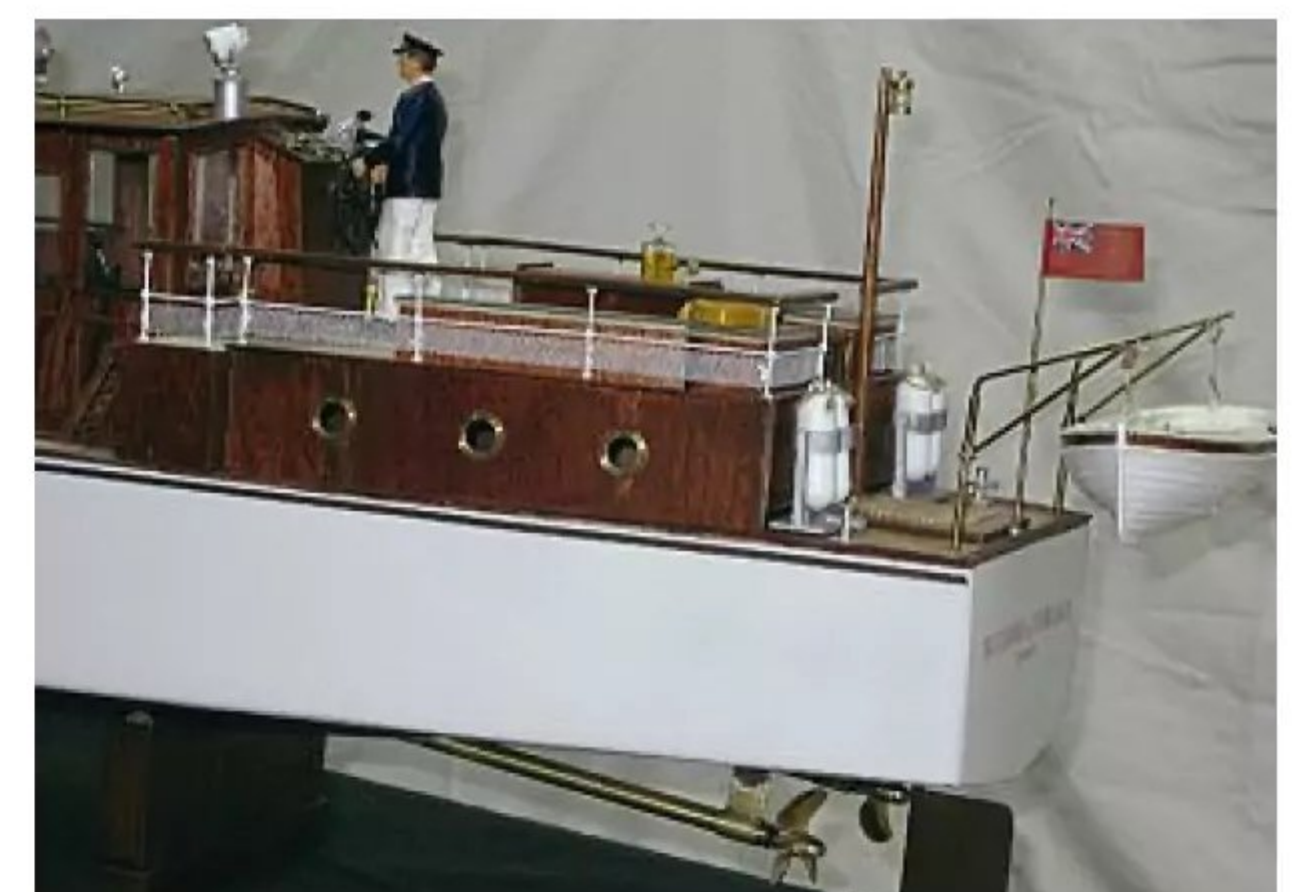
Twin motors need twin screws, and an interesting fact is that Bluebird only had one rudder.
