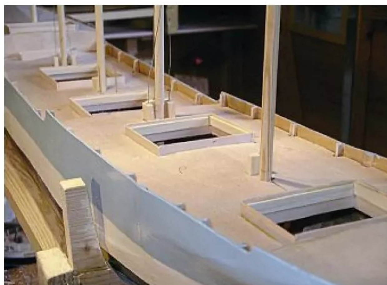
'False decks' and hatches fitted, a view looking forward from the stern.
