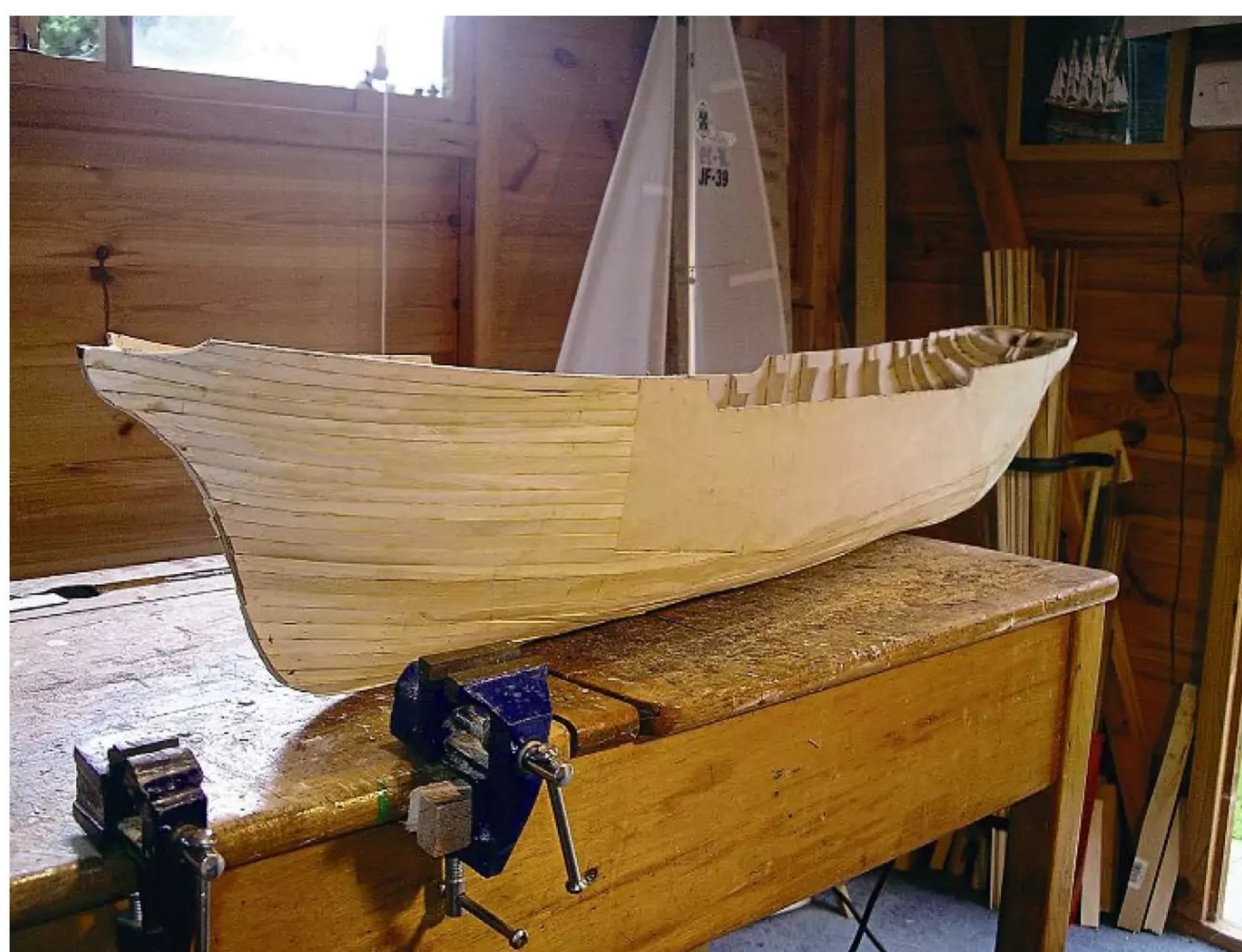
Off the building board, with the sheerline cut.
