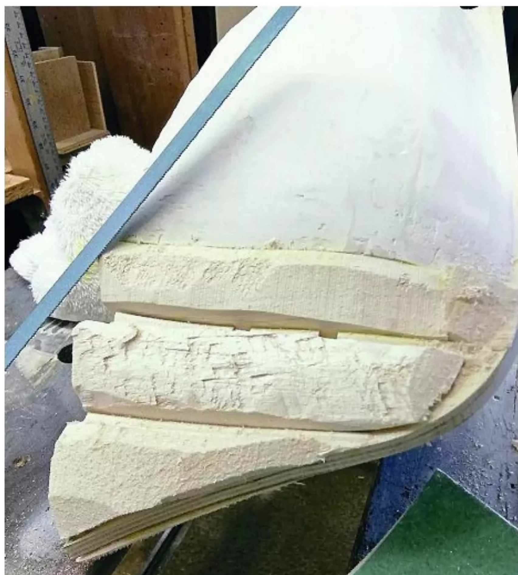
Blocks of balsa wood glued to the bow and stern. These were crudely cut to shape using a hacksaw blade. Not a pretty sight!
