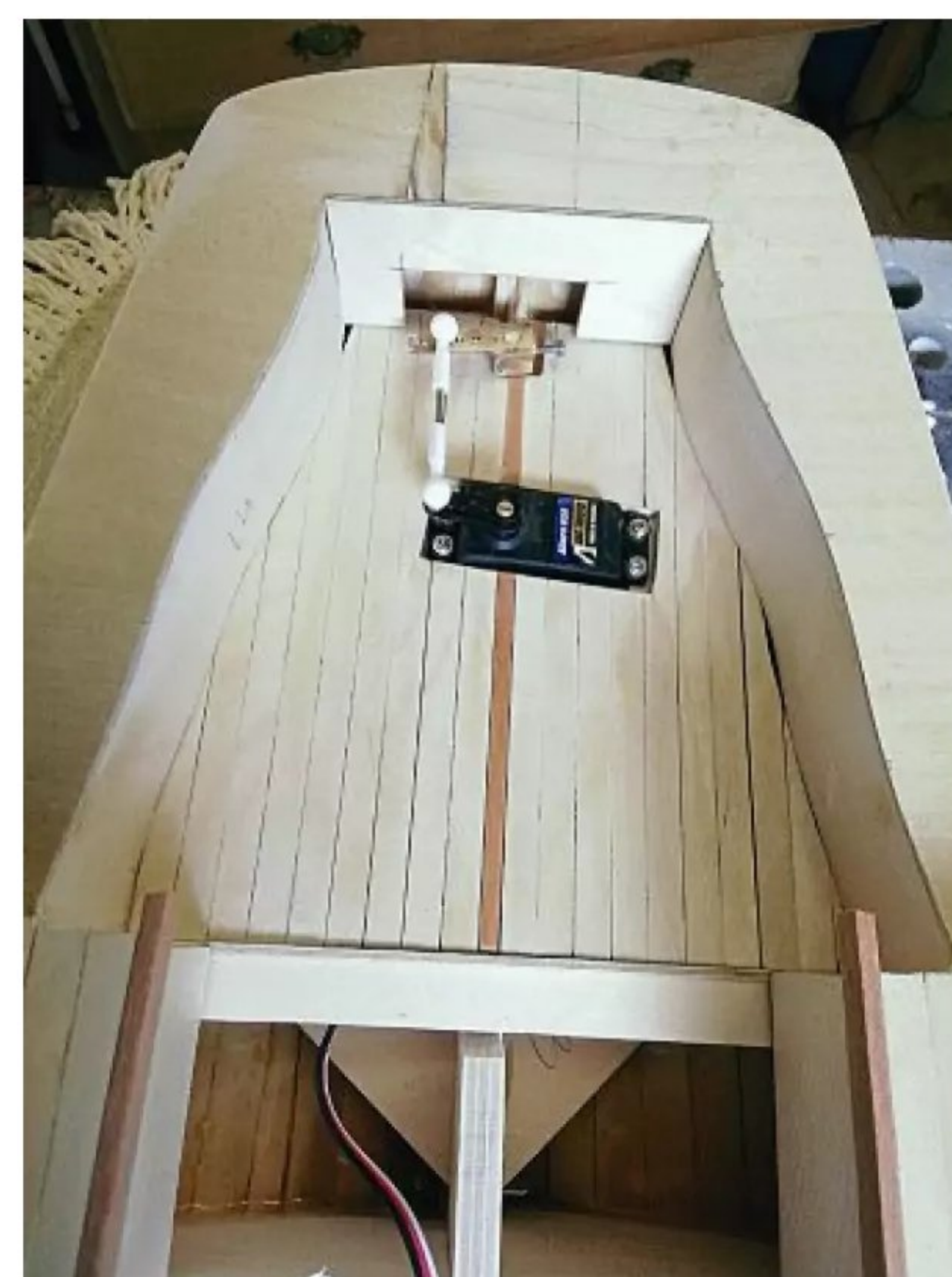
The rear and side decks in place. The side decks have a rather seductive curve to them. According to the plan they should have been parallel!
