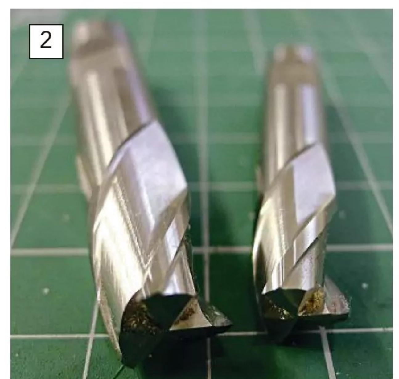
The details of a high-speed steel milling bit. Designed to cut on the bottom flat face as well as the sides, this tool is intended to move horizontally, thereby generating a finely machined flat surface.
