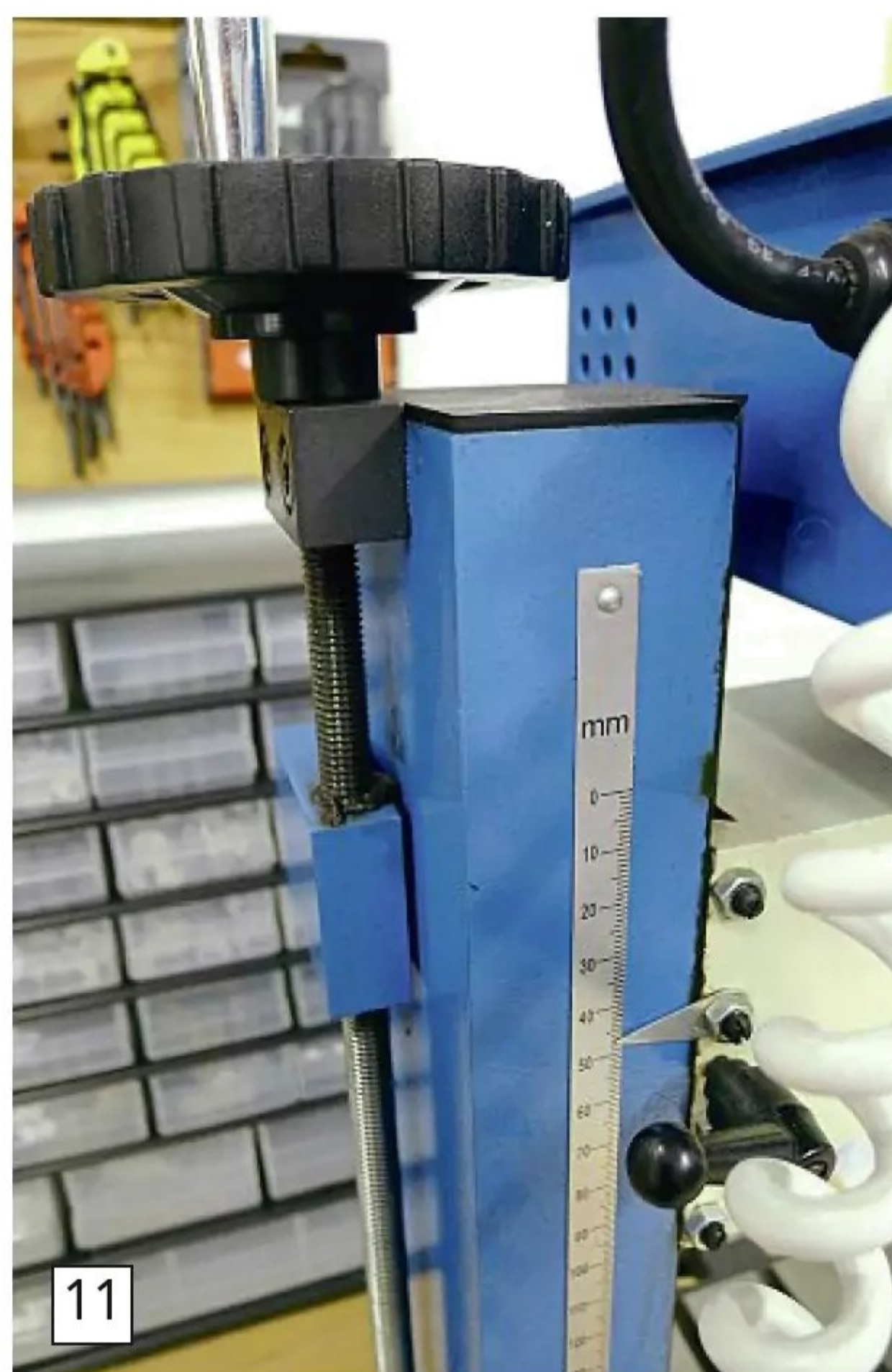
Head height is adjusted by another handwheel and a fine thread, making for very accurate positioning.
