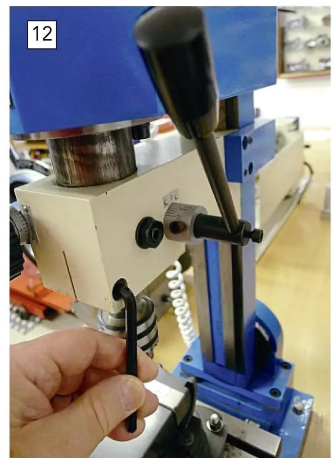
Once the head is at the height you want, it should be locked by the pinch bolt on the spindle. The side handle is for when you are using the machine as a pedestal drill, when the head remains unlocked.
