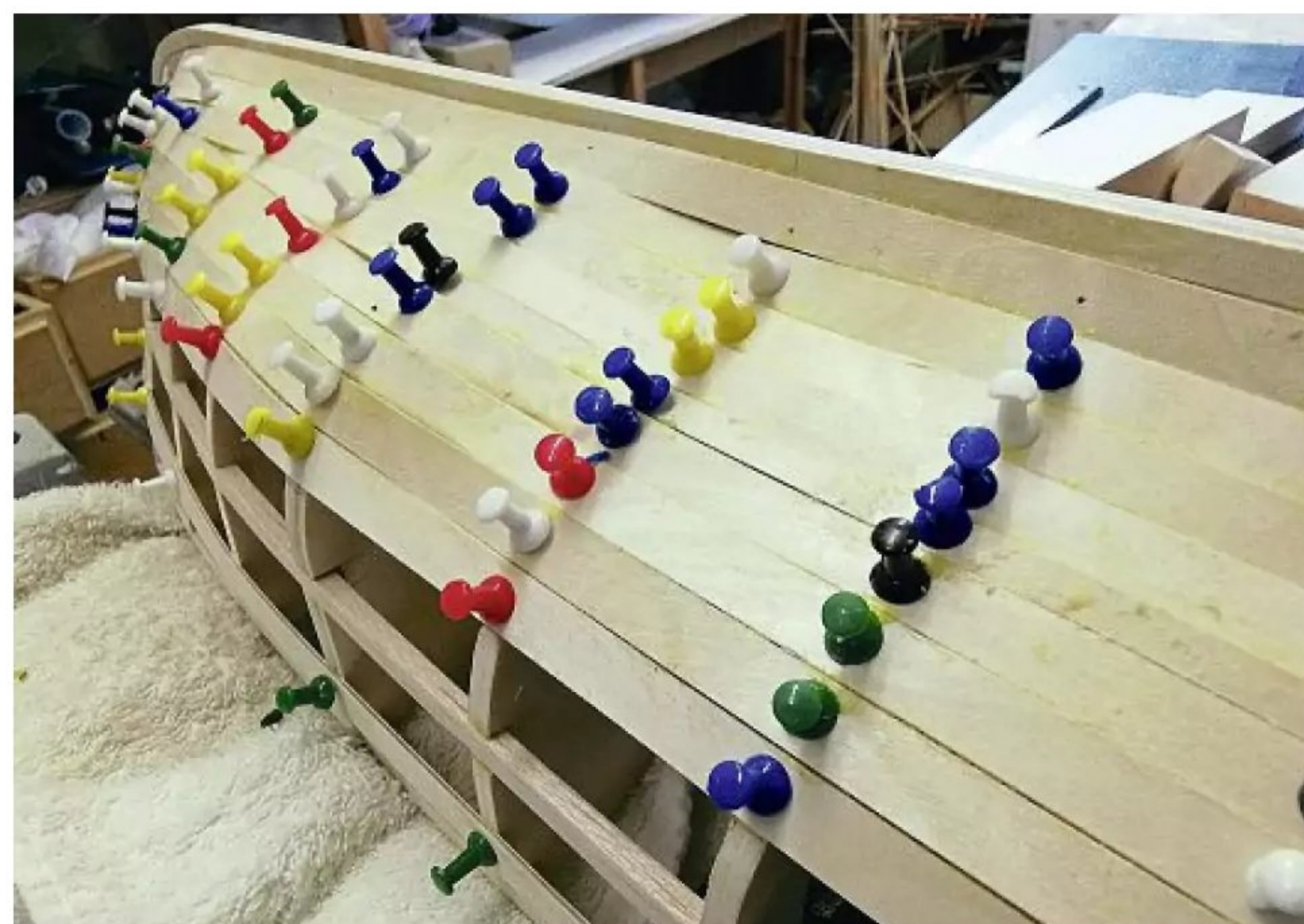
The planks for the ‘plank on frame’ construction, cut from 1.5 mm plywood.
