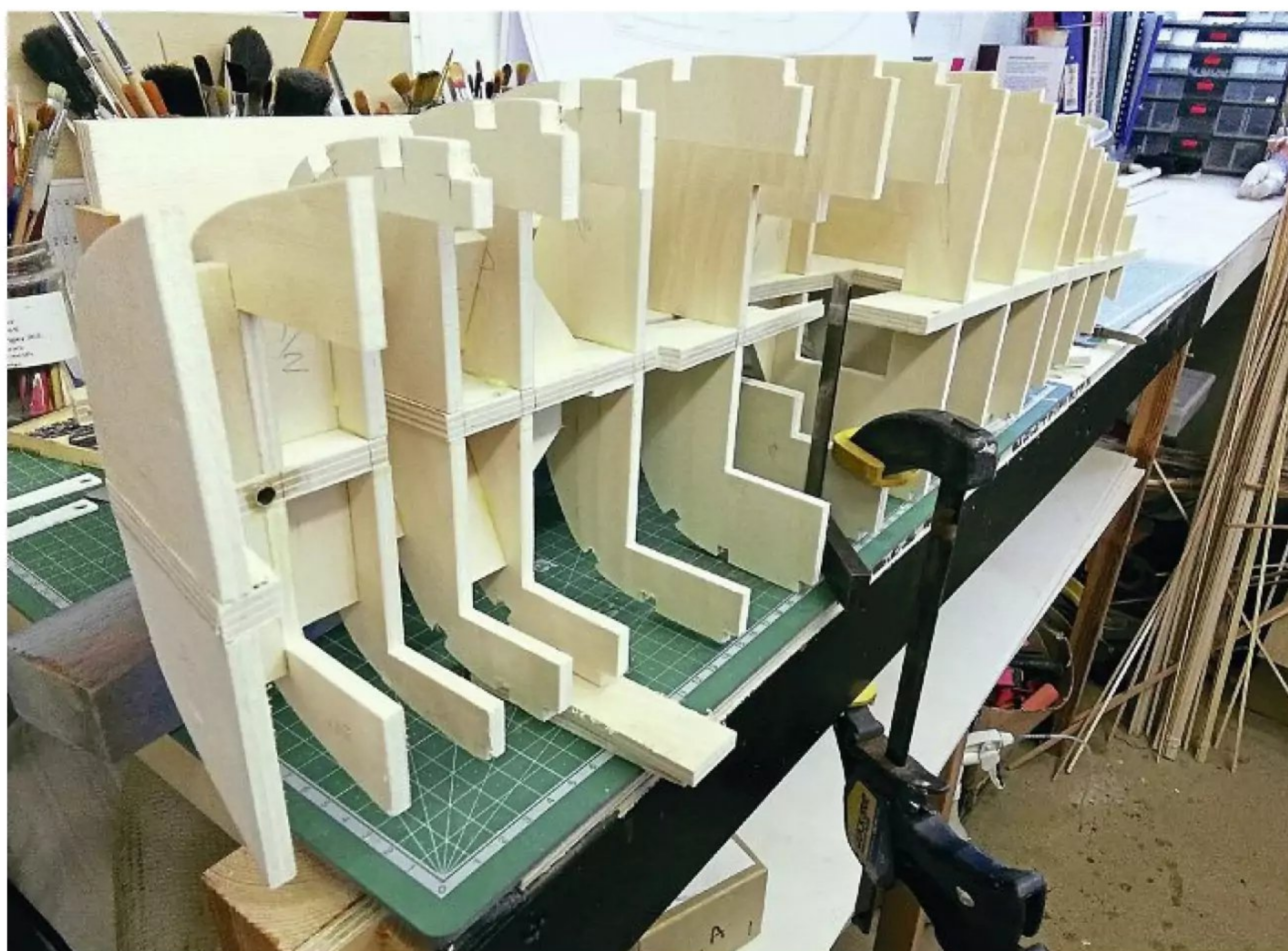
The completed keel with all the bulkheads attached.
