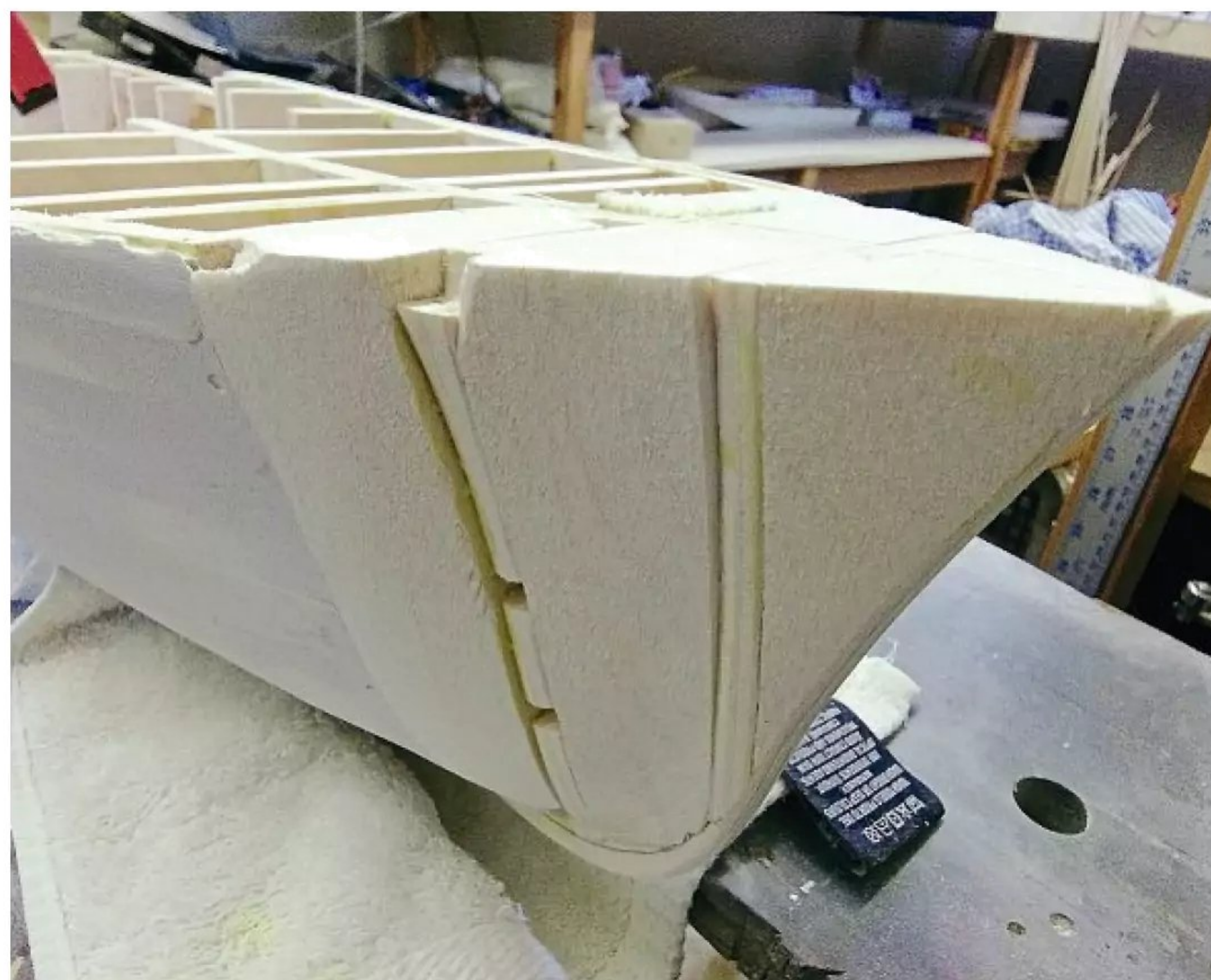
The bow having been roughed out prior to filling, and final shaping.
