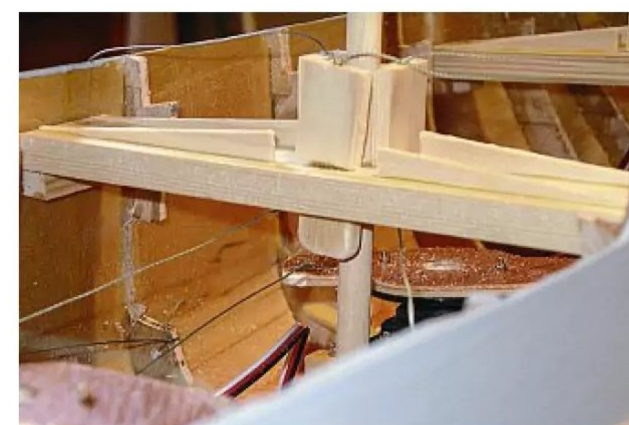
The extended fairlead for a sheet in front of the mast, and the two fairleads for braces on either side of it. The wooden cross-piece across the centre of the picture is the "thwart" that supports the deck and locates mast and fairleads.
