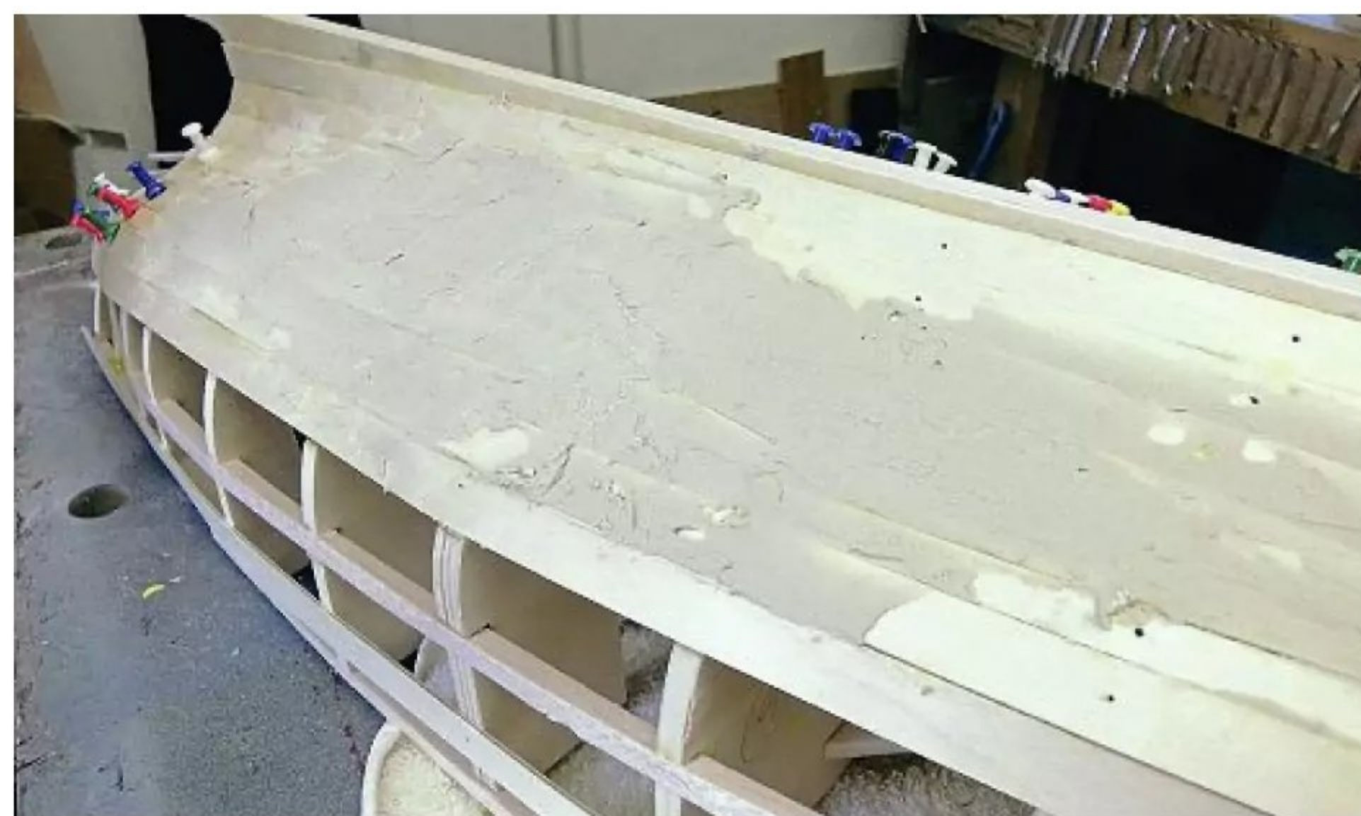
Lashings of P38 filler were spread over the outside of the lower half of the hull. The inner hull was then coated with a generous layer of resin to fill any cracks on the inside. It was easier to resin coat the lower half at this stage, as access would be limited when the remaining planks were added to the top half.
