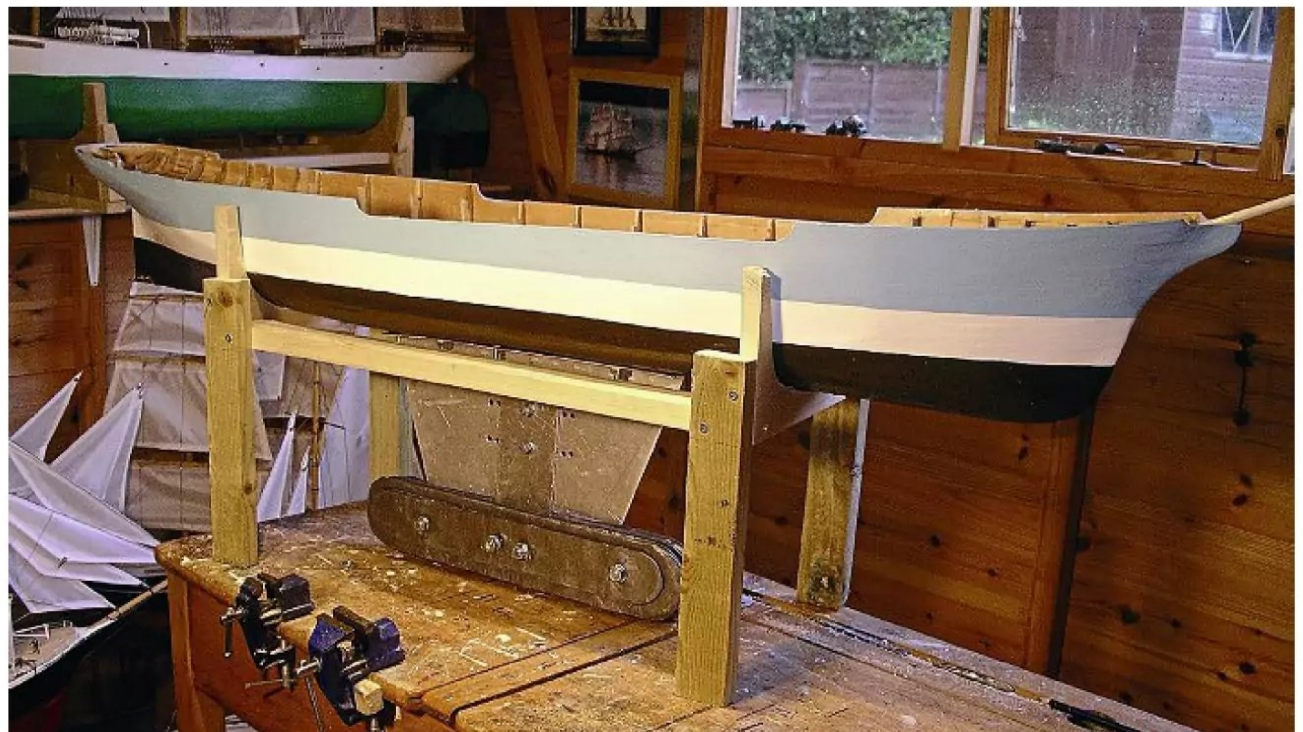
Painted and with the 8.2kgs sailing keel fitted.
