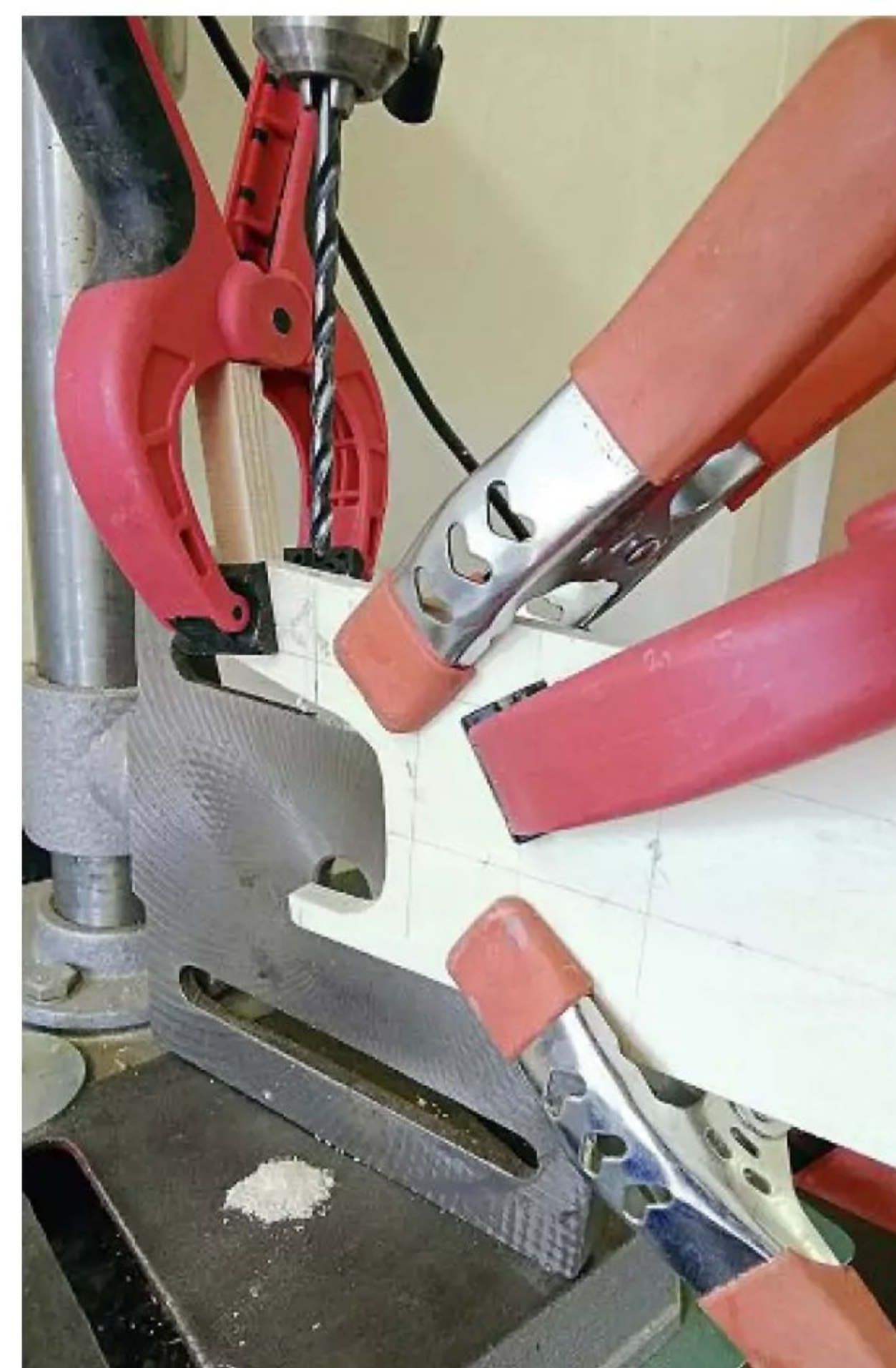
Drilling through the keel for the rudder shaft was a tricky job. The bed on the bench drill was turned through 90°, and the keel clamped to it.
