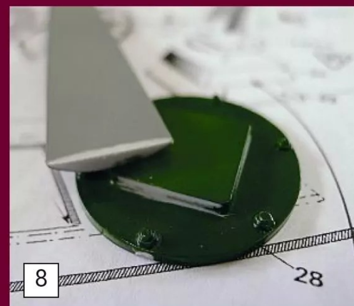
8 Standard plastic kit practice is to remove the paint where the parts are to be glued, otherwise the glue cannot dissolve the plastic in order to create a bond.
