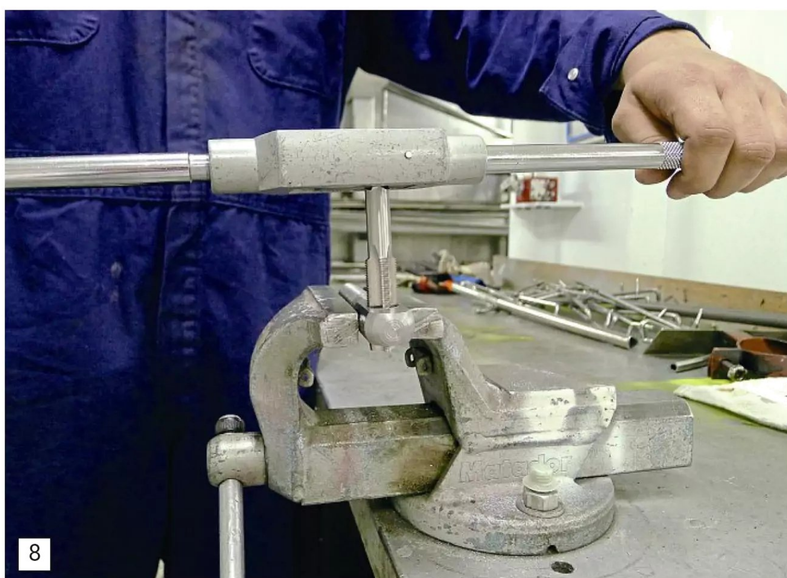
8 Manual tapping is a tricky operation that takes practice and skill. You will not get it right the first time and even the more experienced can get it wrong occasionally. Holding the tap perfectly perpendicular while looking down on it is not easy.
