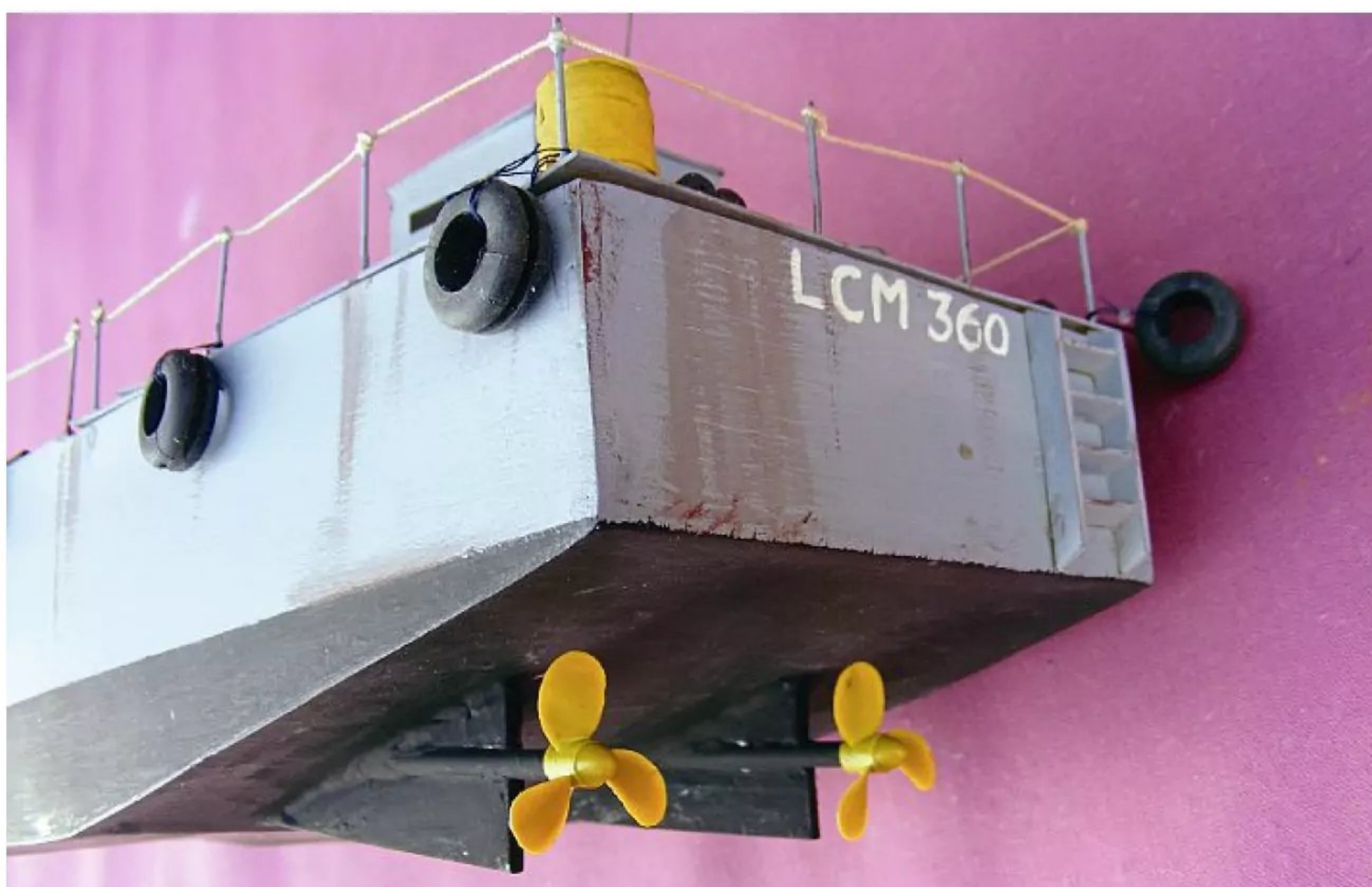
Glynn's propeller assemblies came from the bottom of his spares box, but modelling component specialist RadioActive offer a suitable alternative in the form of its one-inch (25 mm) diameter three-bladed propeller and shaft units.
