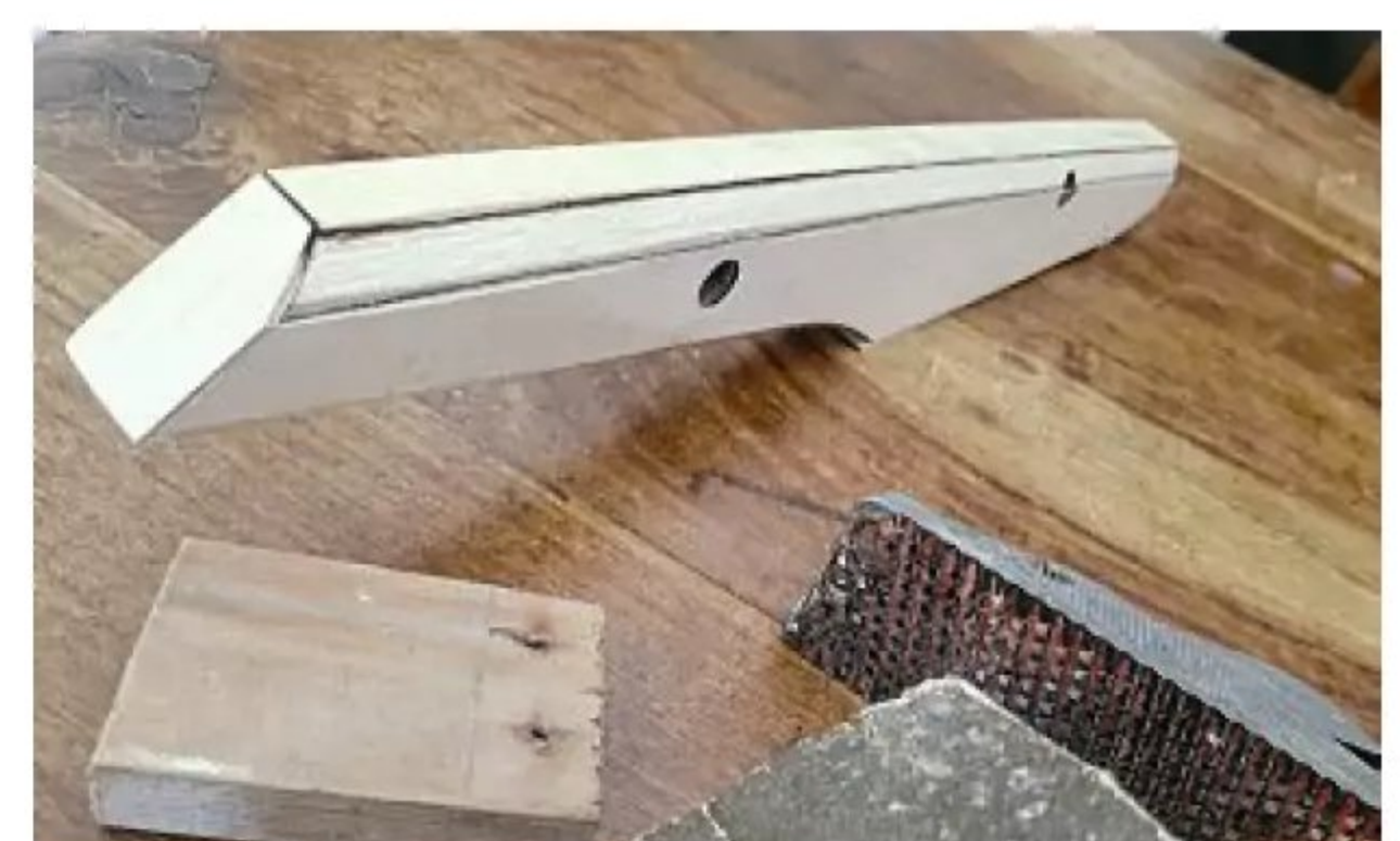
Using hand tools may be easier to obtain the top angle chamfer strip.
