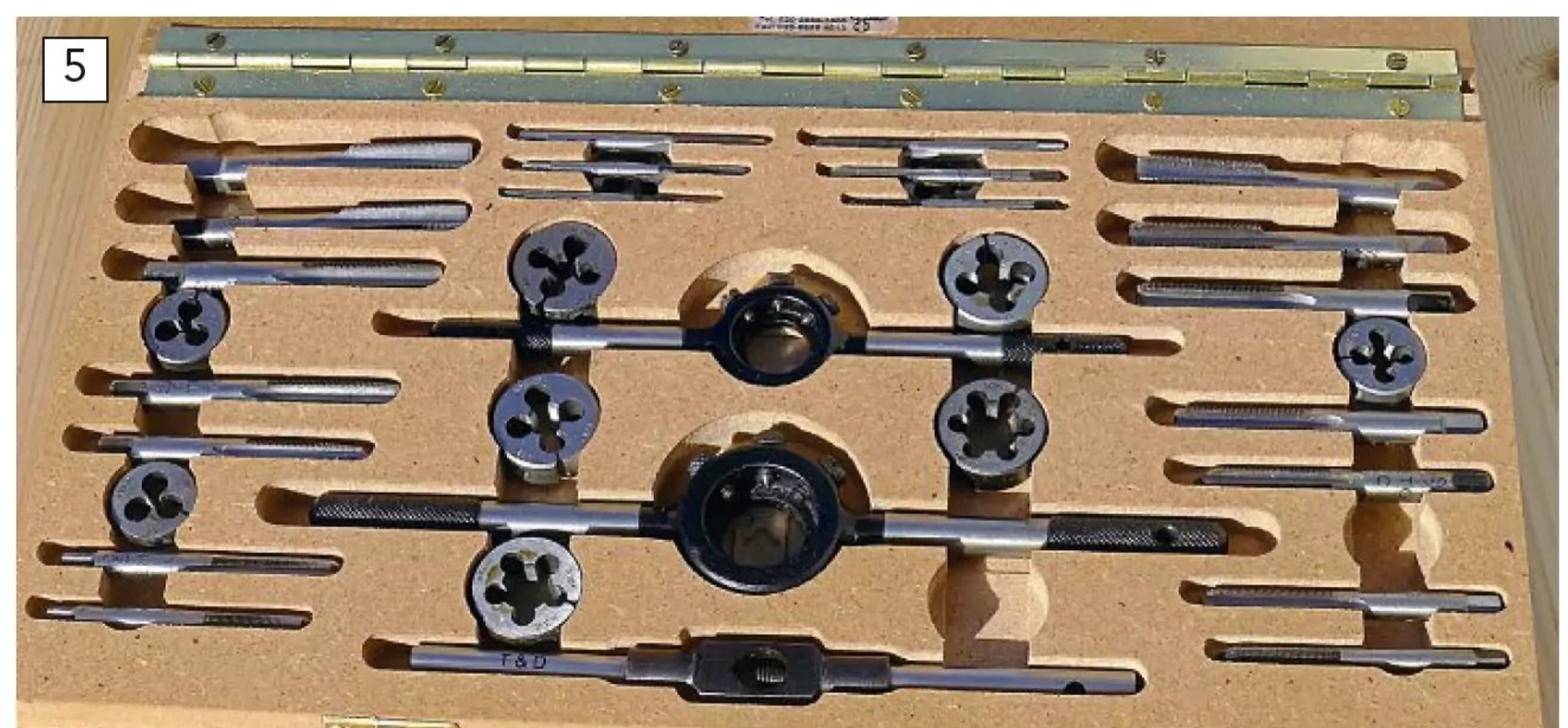
A Model Engineering (ME) set of taps and dies by the Tap and Die Company of London. ME threads are still found on a lot of older vintage steam models.
