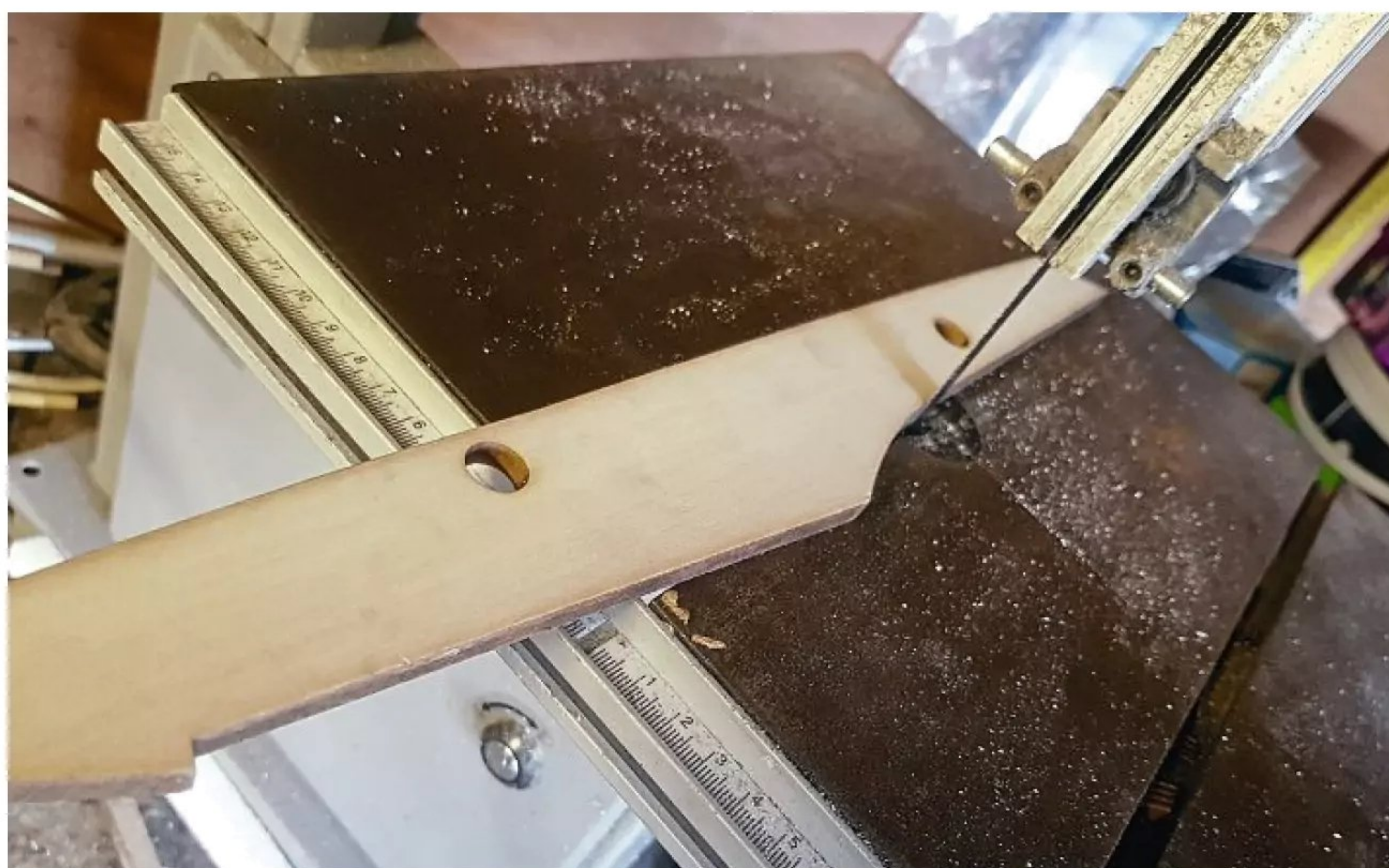
Cutting out shapes with a band saw.
