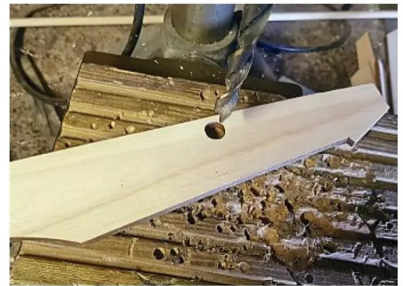
Drilling boom tube holes.
