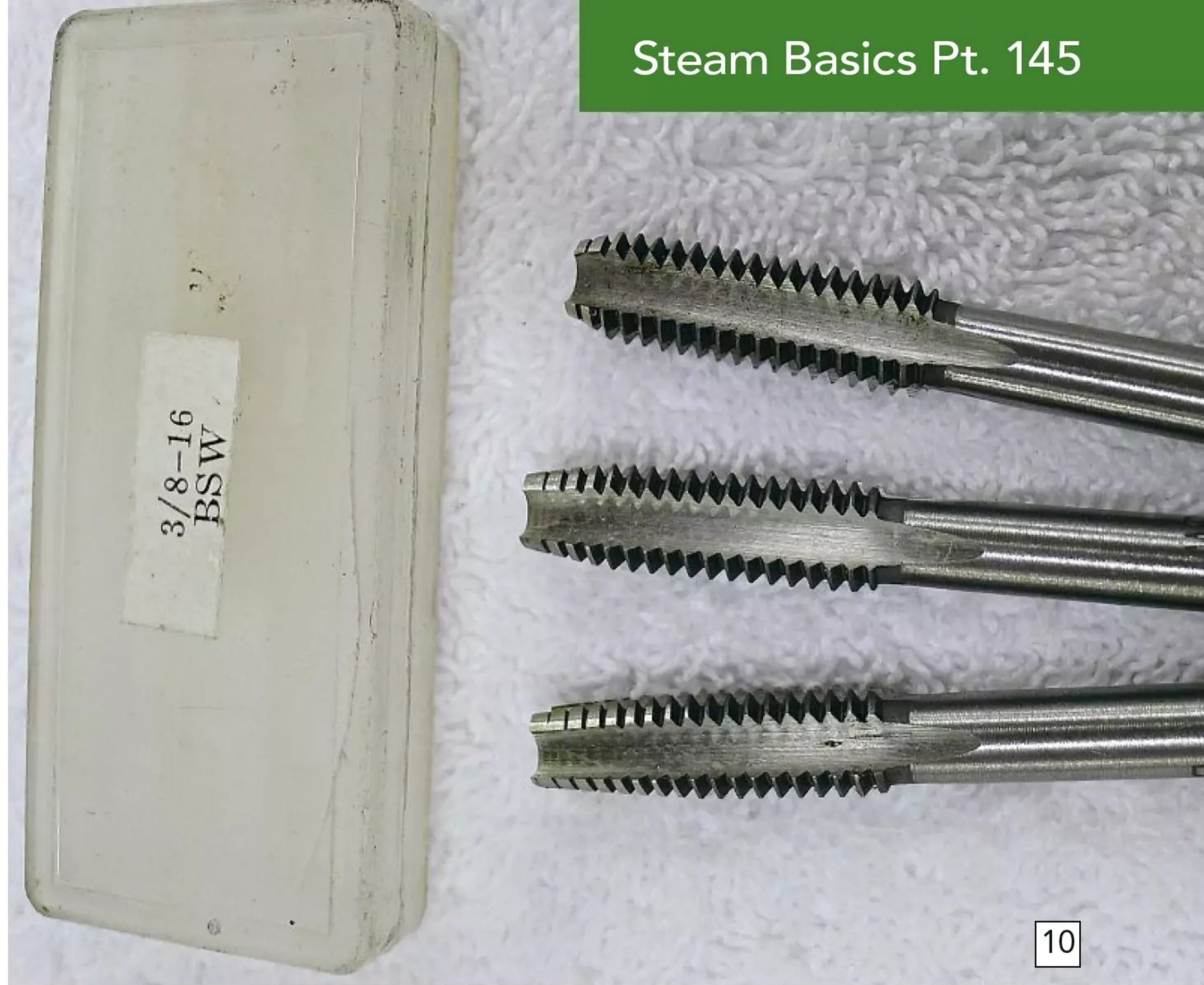
For a specific job you can buy a set of three taps of any specific thread, including Taper, Plug, and Bottoming taps.
