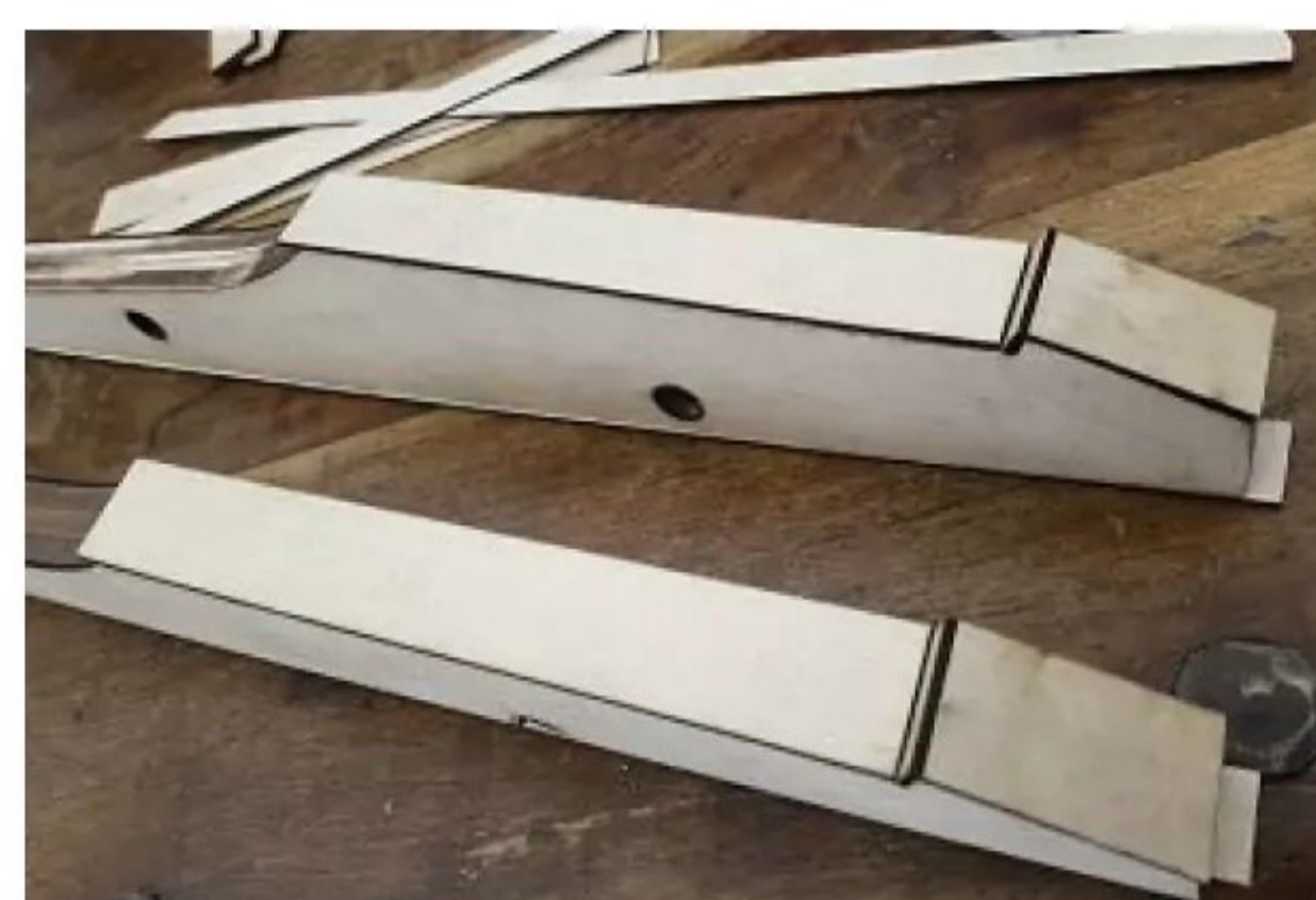
The ply side skins glued into place.
