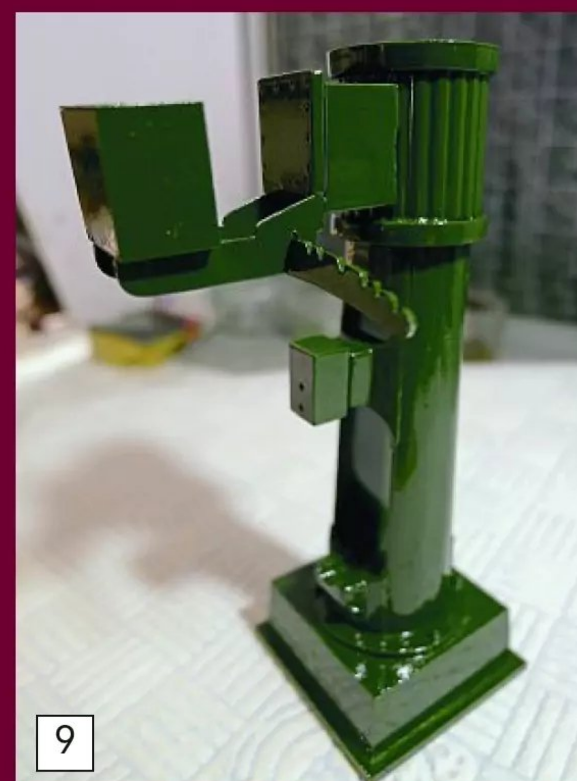
9 The completed engine entablature. The valve chest and other parts, along with the engine base, are laminated ply pieces and the cylinder cover is a supplied brass corrugated tube.
