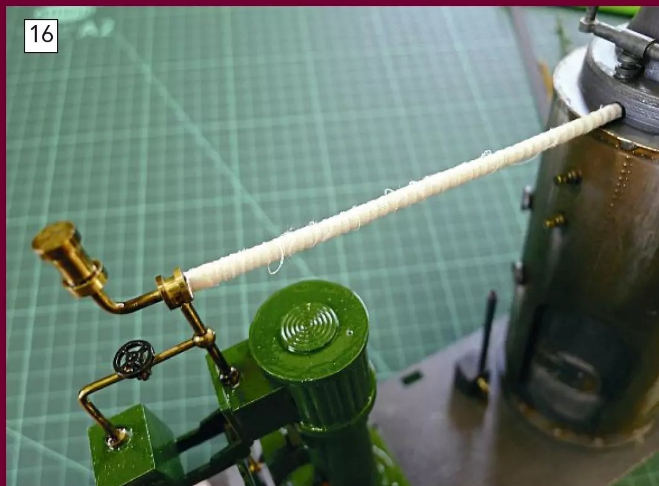
The cloth supplied for the lagging is a very loose weave so needs to be handled carefully to prevent excessive fraying. Care and patience paid off. Don't worry about the few stray strands at this stage.
