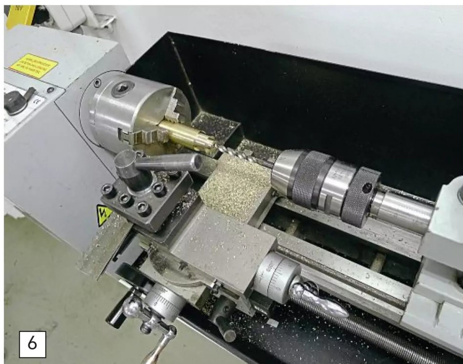
6 The great beauty of a lathe or a pedestal drill is that you can drill and tap without disturbing the job, thereby ensuring perfect alignment
