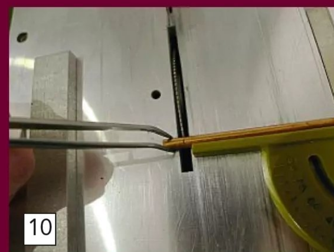
10 The best way to cut non-ferrous metal tubing to give a perfectly square cut and no burr is with a suitable blade in either a band saw or a circular saw. Richard's Proxxon KS230 did this job superbly.
