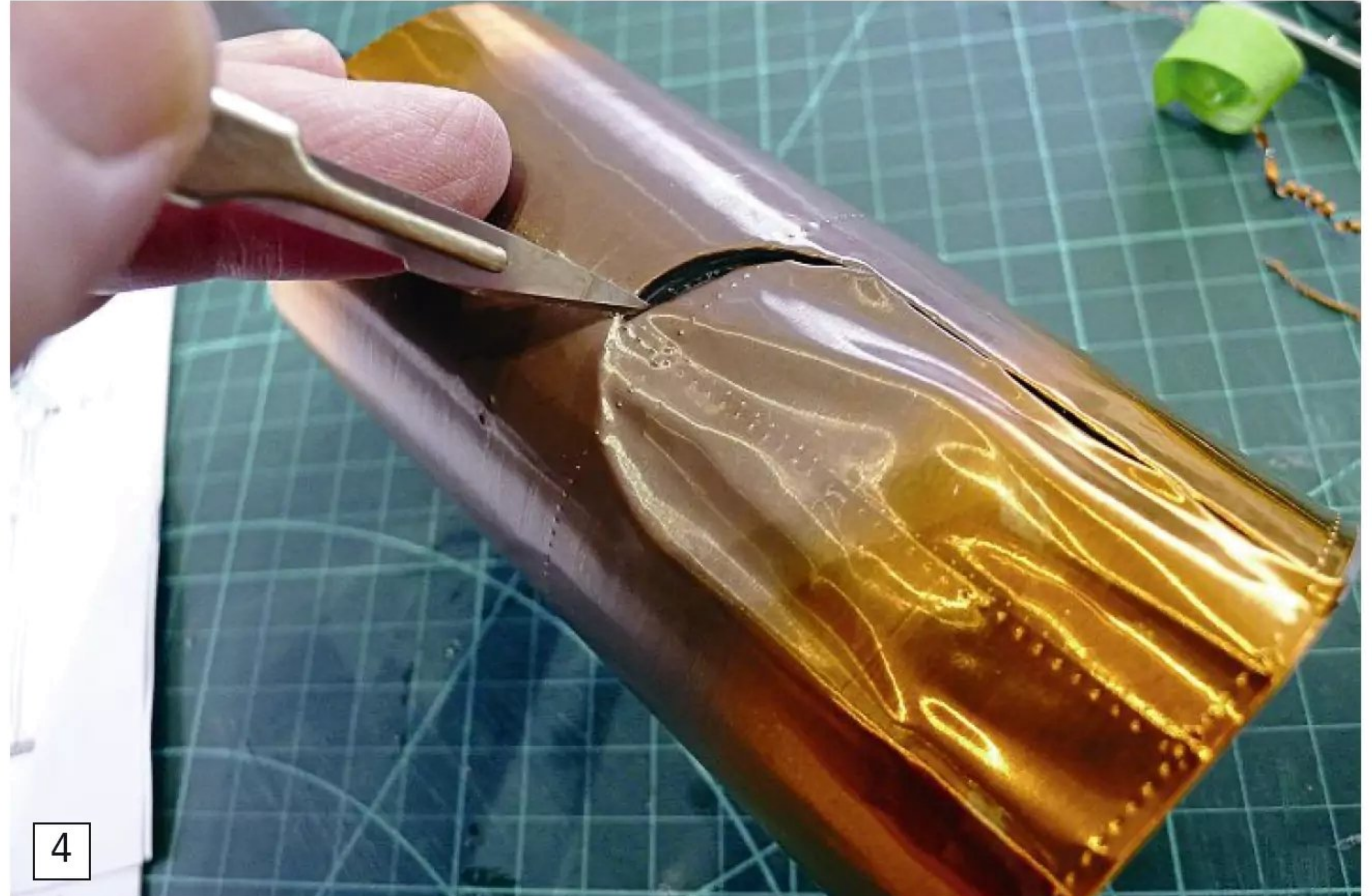
Once the copper cladding had been wrapped around the boiler and the epoxy cured, the recess could be carefully trimmed by running the blade along the edge of the plastic.
