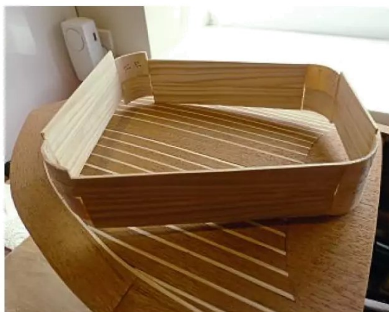
The deck openings, frames and seating.
