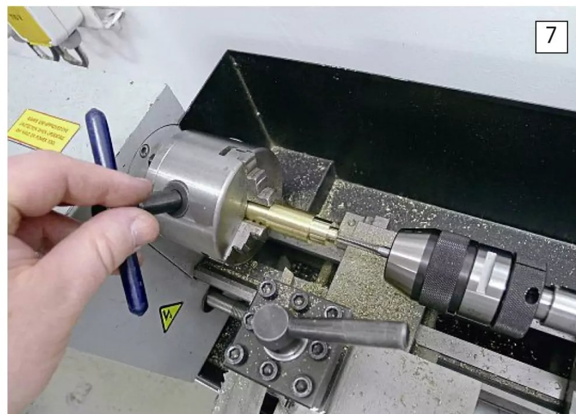
7 Rotate the chuck with the chuck key in a backwards and forwards motion to break the swarf. The tailstock will automatically be drawn into the job as the tap cuts, as long as you have taken the lock off!
