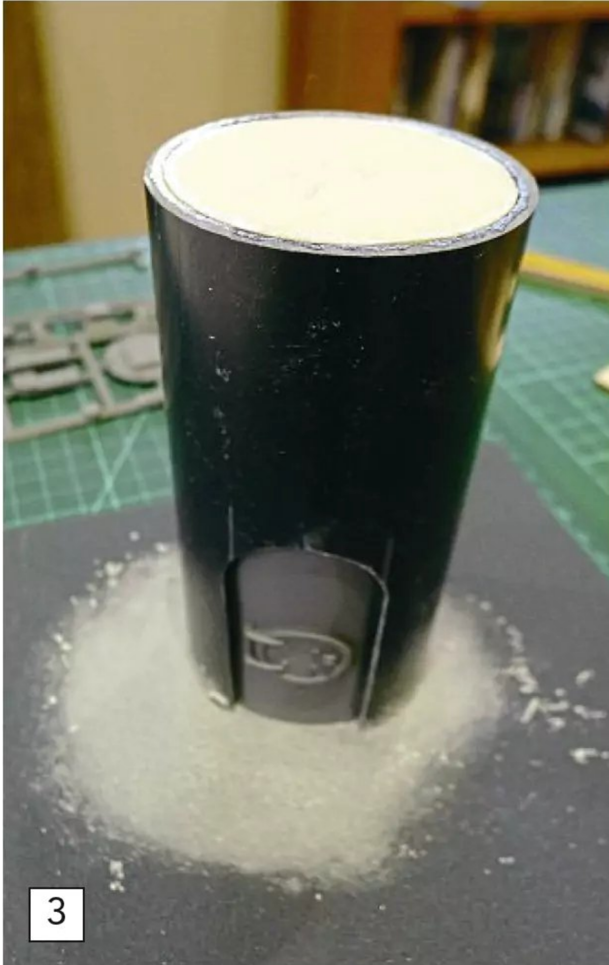
The ply inserts for the top and bottom needed a little reducing to get a good fit and they were dressed up when the glue had set. Two-part epoxy was used for these parts.
