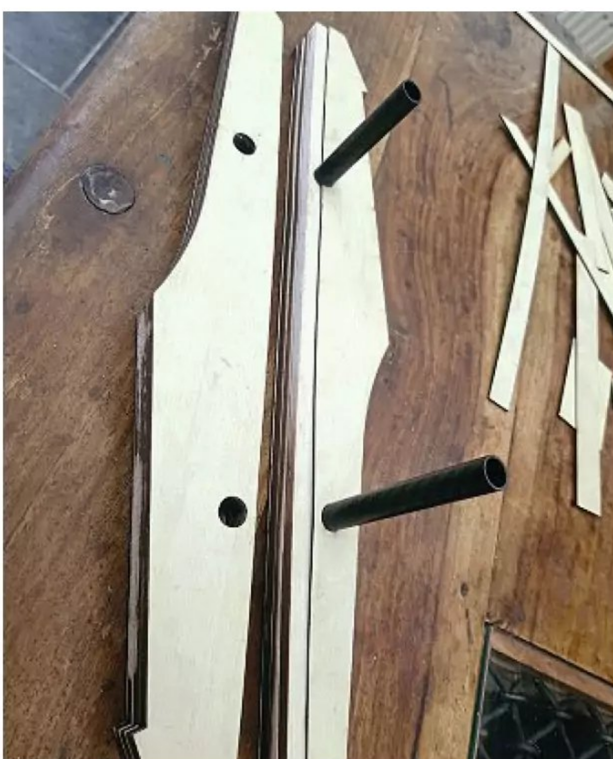
The scrap tubes used make sure everything lines up before gluing the core.
