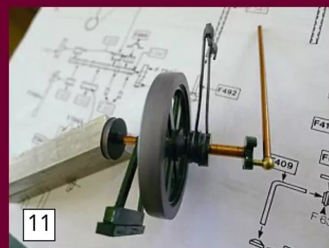
11 The completed running gear with flywheel, valve eccentrics, bearing and crank all assembled onto the crankshaft. The flywheel was dressed up in the lathe for a perfect surface.
