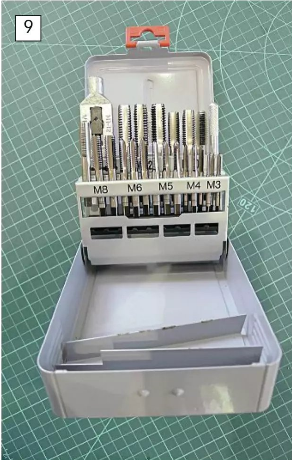
A very handy set of metric taps, with three of all the common smaller sizes.
