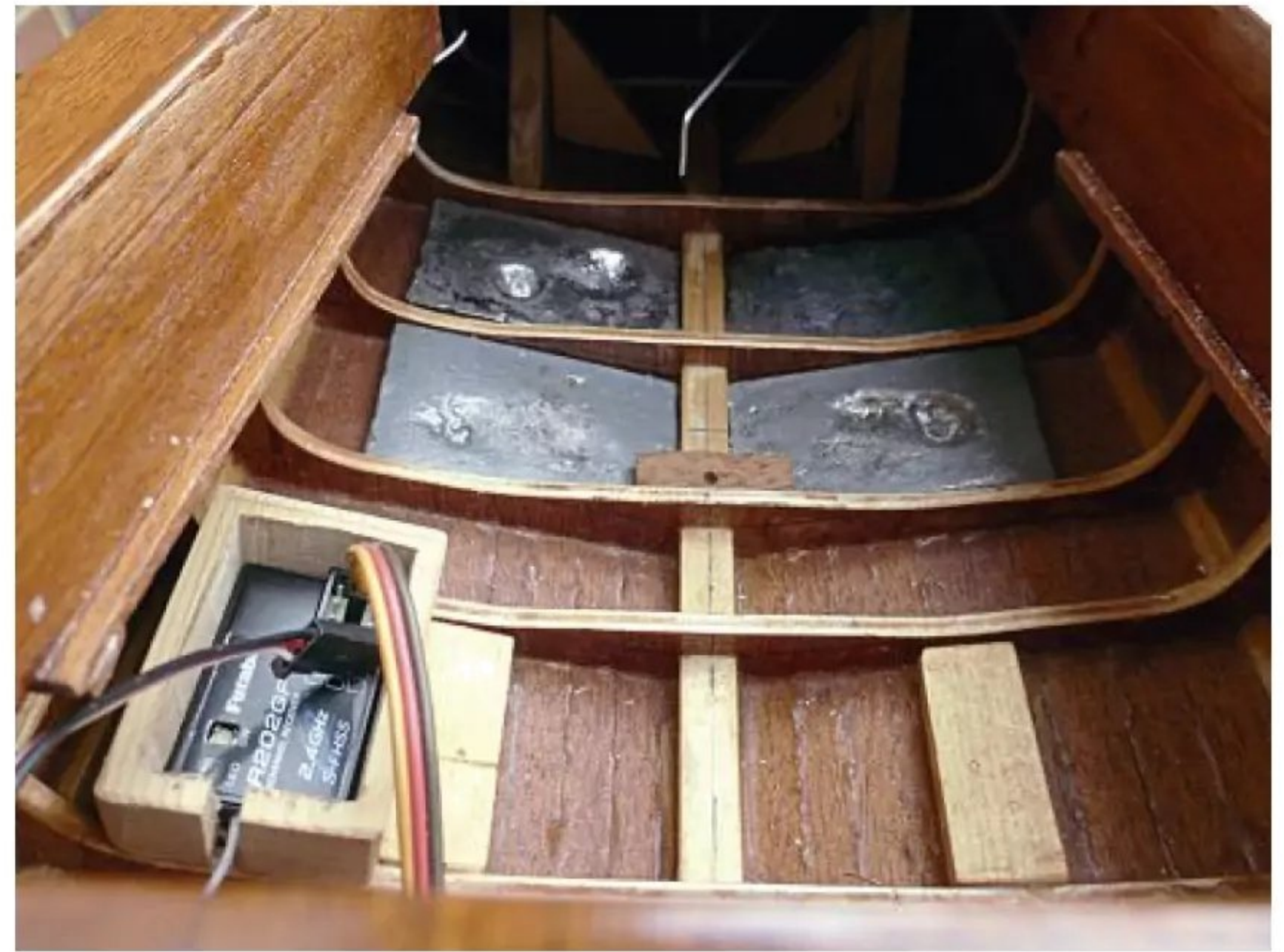
As the model sat slightly high at the stern, Barry cast four lead weights to fit between the frames slightly forward of the transom.
