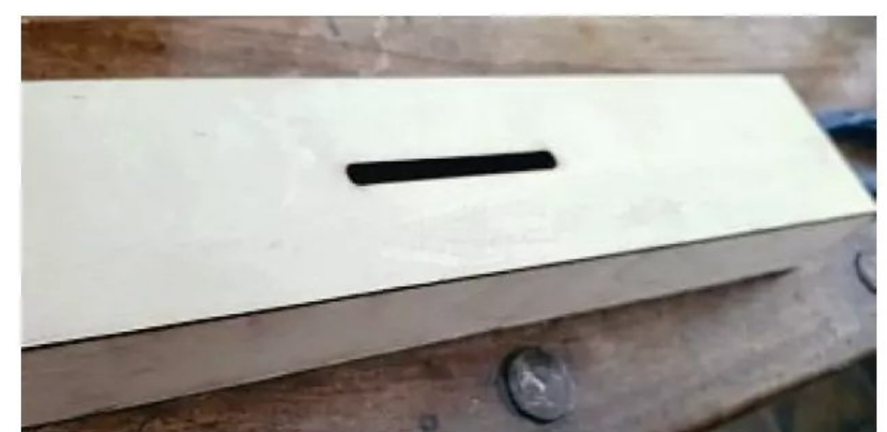
The underside ply skins also glued into place.
