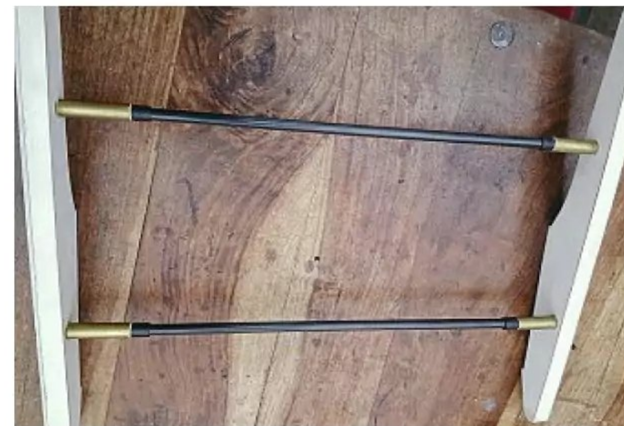
Use of the boom tubes to check sponsons are true to each other.
