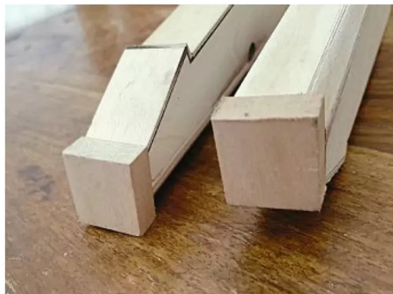
The hardwood nose blocks glued on, ready for shaping.
