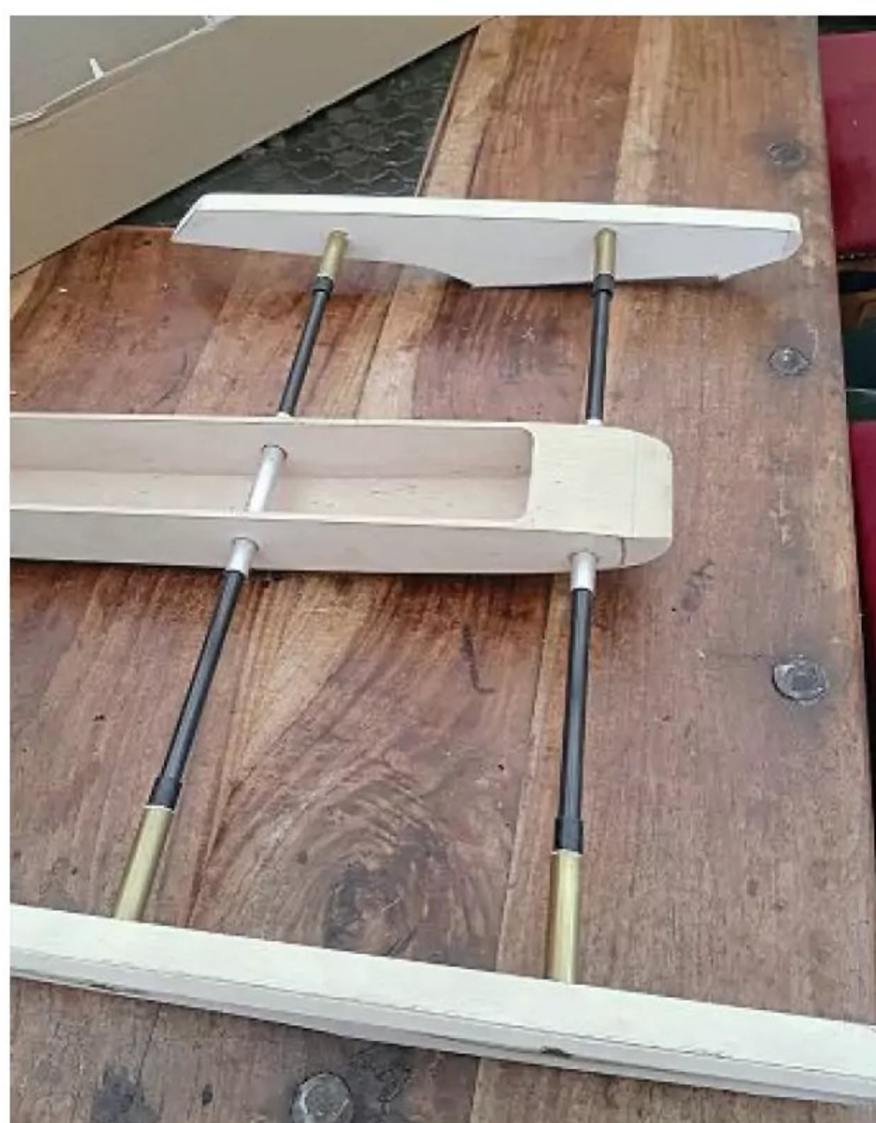
Using the tub to ensure sponsons align with the tub boom holes.
