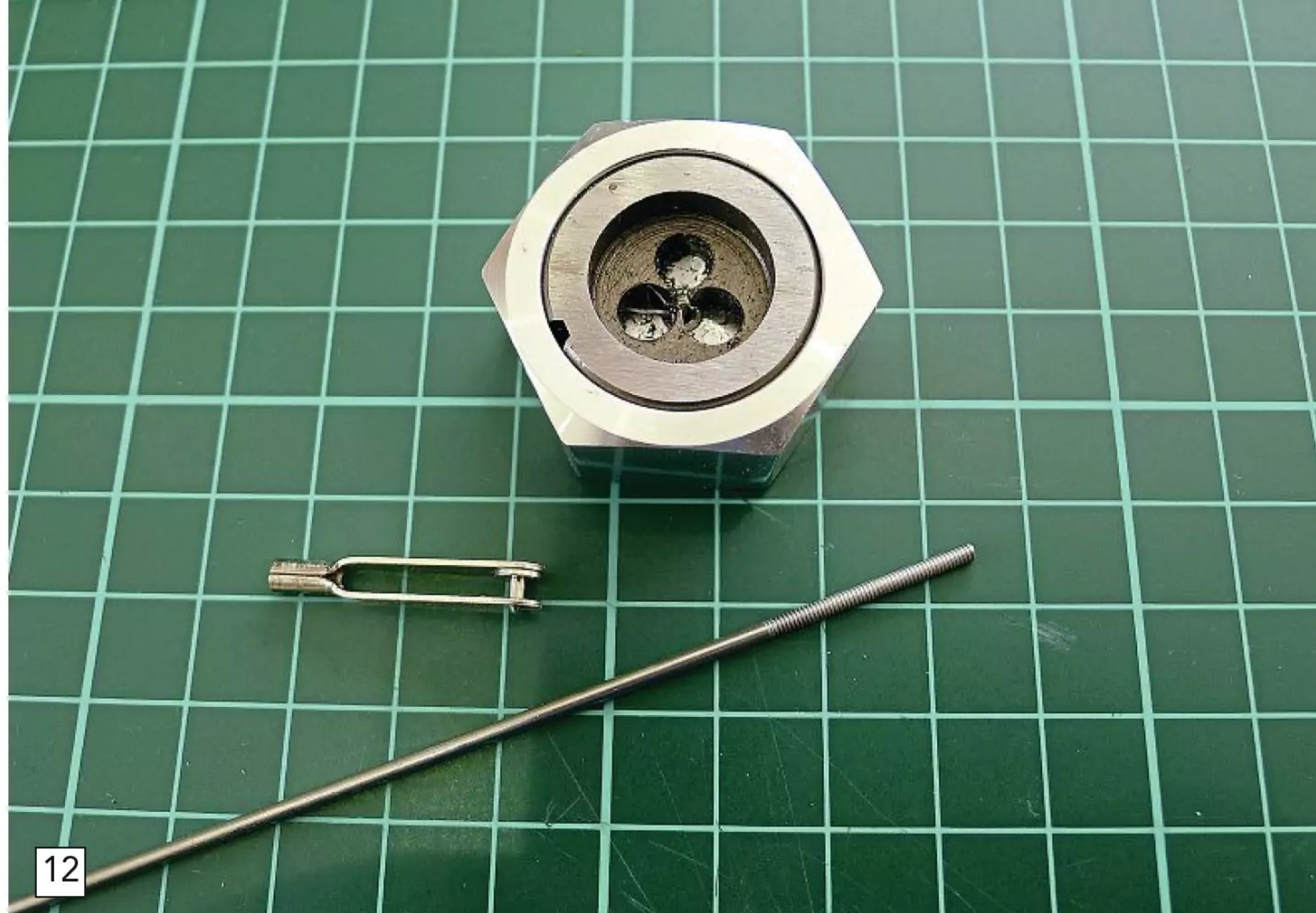
You can buy die nuts, but this is actually a circular die held in a hexagonal holder. The process of cutting the thread is exactly the same, but with a die, look closely at the two sides of it; one side will be tapered to start the thread, while the other side will be full thread for finishing.
