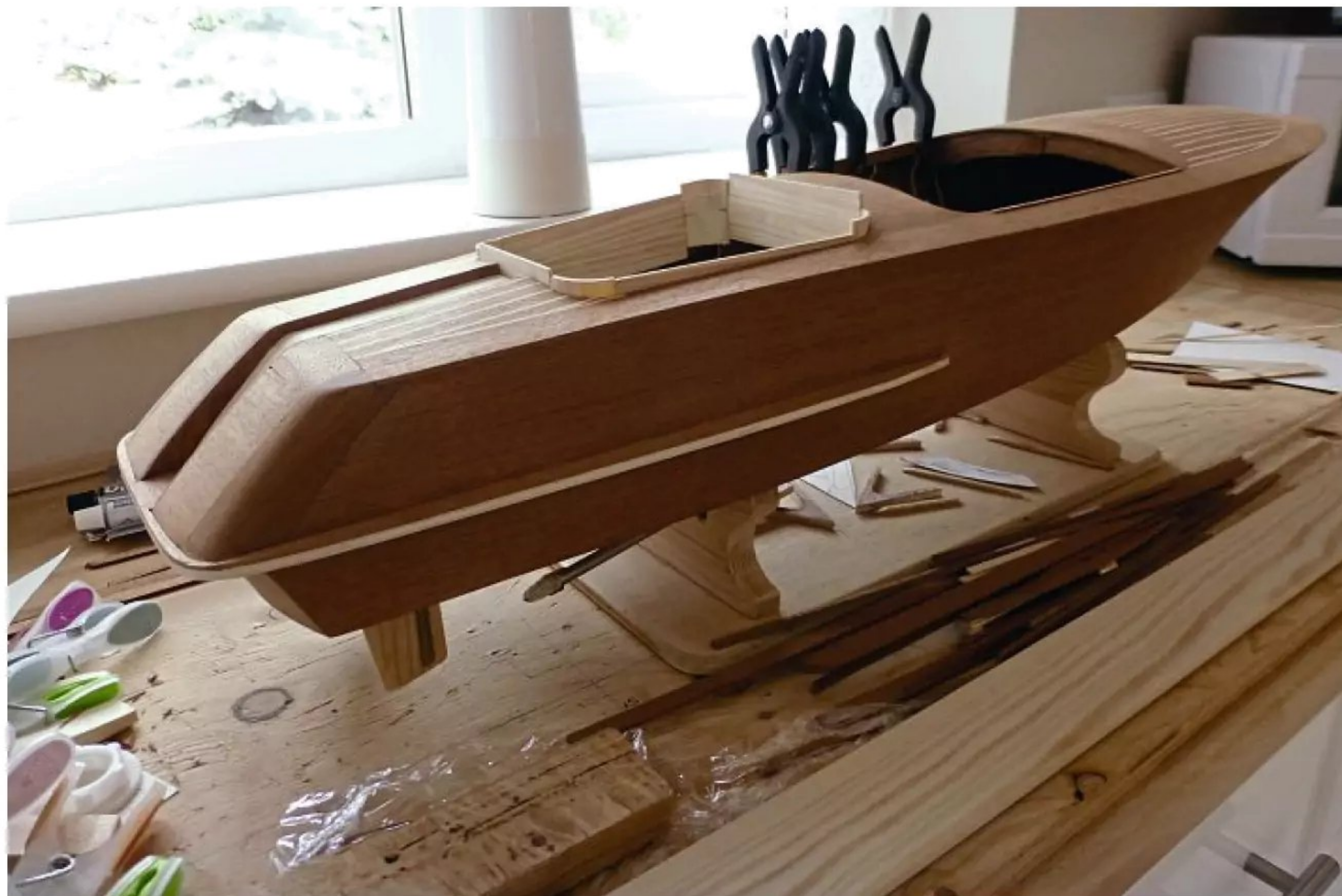
Blocks of teak were glued in to fill the stern quarters, then carved down and sanded to form a curve around the transom corners, so they blended into the side planking, rear decks, and walkway.
