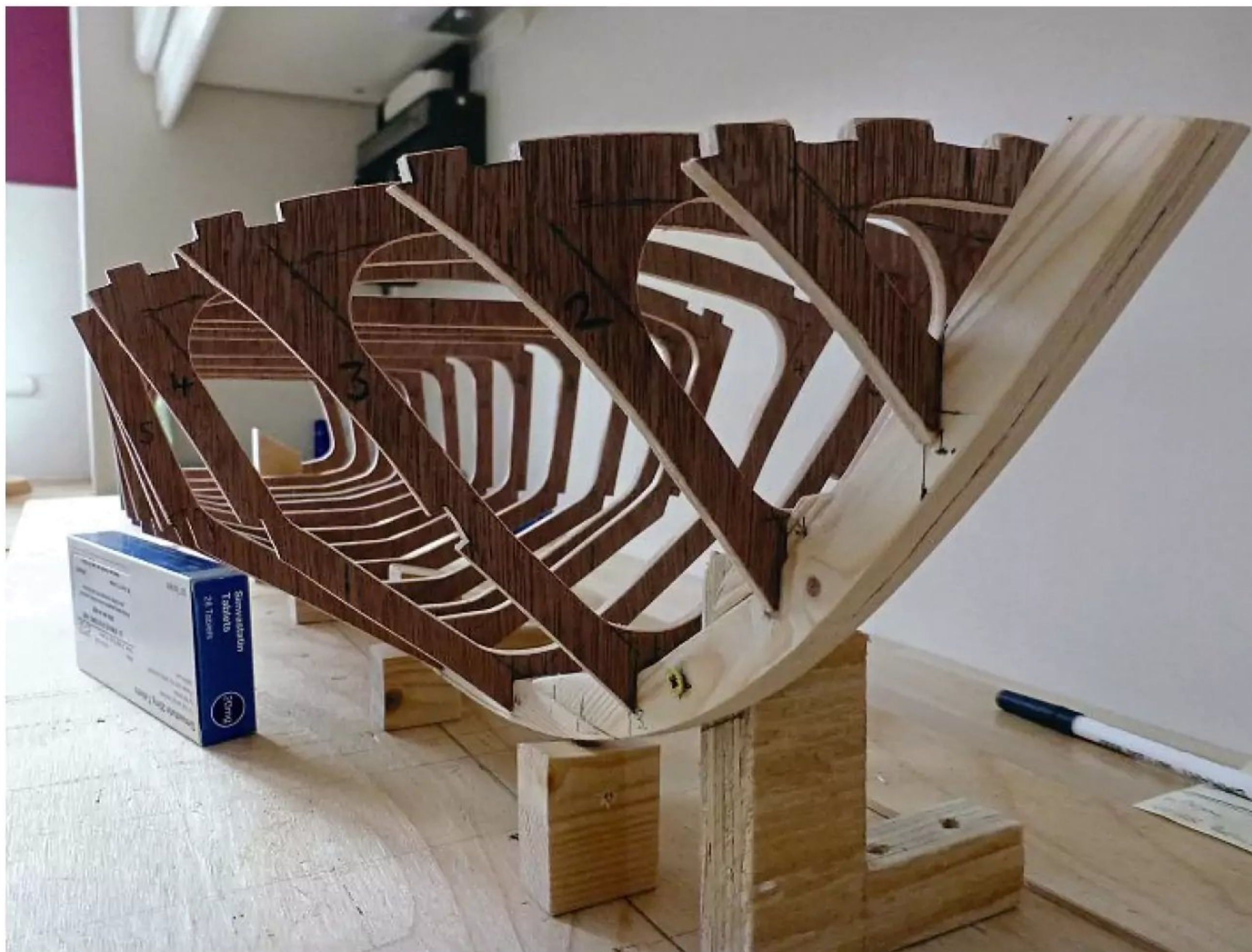
Laying of the keel and frames with the boat upright.
