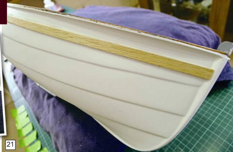
21 The rubbing strake could then be glued to the line, held in place with tape until the glue fully cured.
