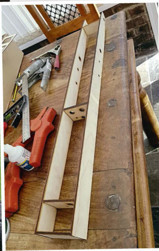
The bulkheads and sides glued in place.
