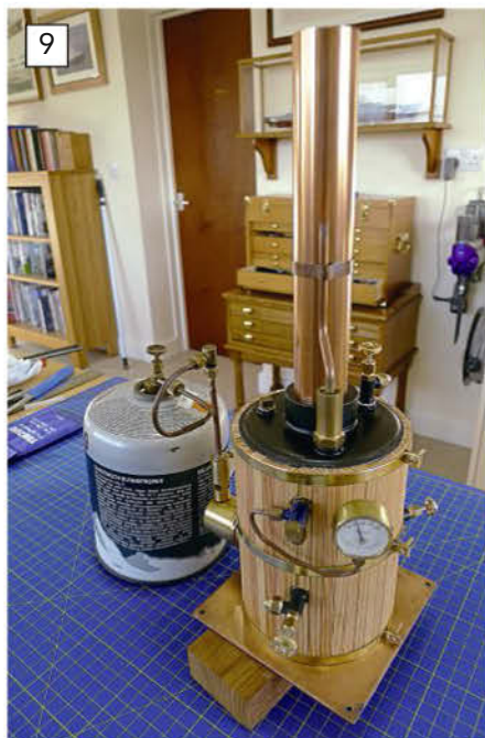
Most modern boilers are now fitted with externally adjustable safety valves, as illustrated by this Pendle vertical boiler.
