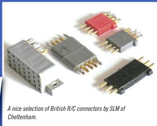
Often known as 'AEI' connectors, these c.1960s' silver and polythene devices were a big step up.
