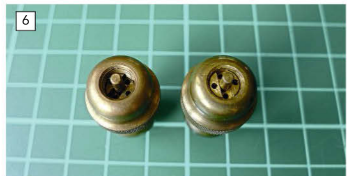
The valve on the left is set to lift at a high pressure and the valve on the right is set to lift at a low pressure. Never adjust the valve so it is hardened right down, as this effectively gags the valve and renders it inoperable.
