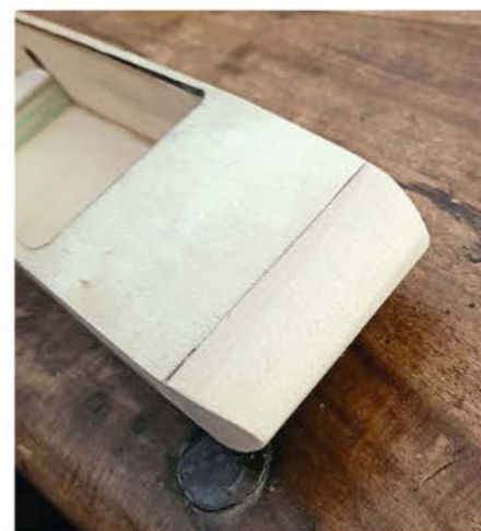
The front nose block in place, ready to be sanded to shape.
