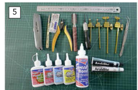
Basic tools and glues to start with. The Araldite was replaced with Stablit Express but most of the other items were as used. All paints were from the Humbrol UK range.
