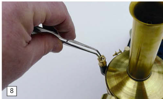
Over the years Richard has found the best tool to be angled nose tweezers. These locate easily but your hands are kept out of the way of any inadvertent release if you back off the disc when there's still residual pressure in the boiler.
