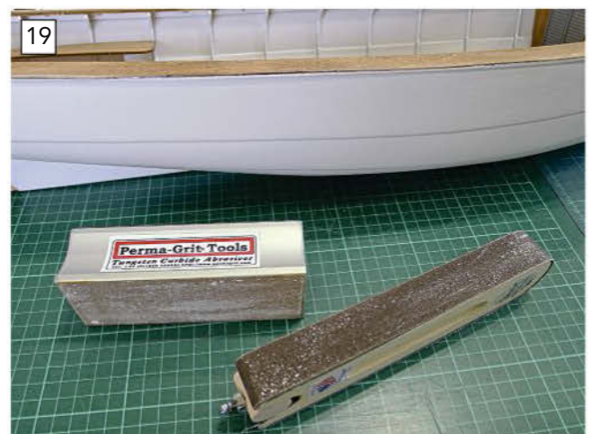
This was then trimmed back to the edge of the wooden deck with a coarse and a fine finishing abrasive.
