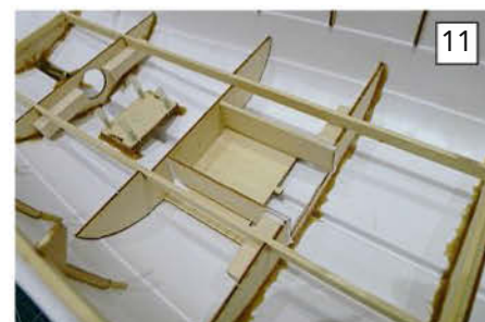
To get the battery fitted where I wanted it a frame required cutting so, to replace the strength, sides were added to the battery box.
