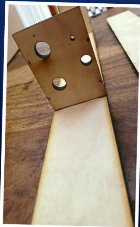
Holes pre-drilled in the bulkhead as the plan suggests.
