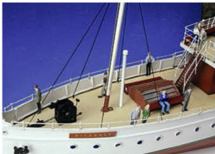
Foredeck detail. The pole behind the mast is the galley chimney.
