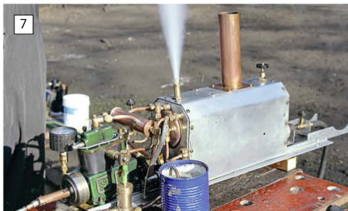
The first job is to lift at the correct pressure and vent steam. The second job is to vent enough steam to prevent the pressure building up by no more than 110% of working pressure.
