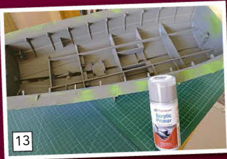
The first couple of coats of acrylic matt primer sealed the wood and showed up any imperfections. Note the threads of the motor mount screws masked by silicone tube.
