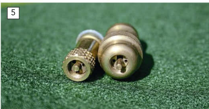
Two other types of externally adjusted safety valves. Both have vent holes in the disc for either pliers or tweezers, and the one on the right has a machined slot that can be used to adjust it.
