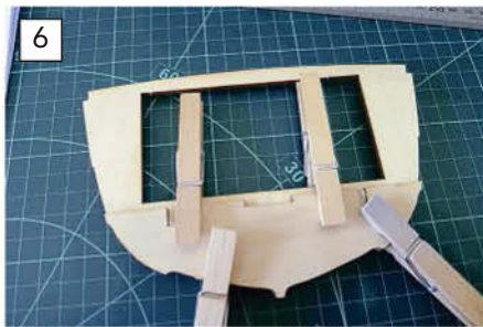
The forward bulkhead determines the position of the frames on the deck supports so it needs to go in first. Laminating the two parts is simply a white glue and pegs job.
