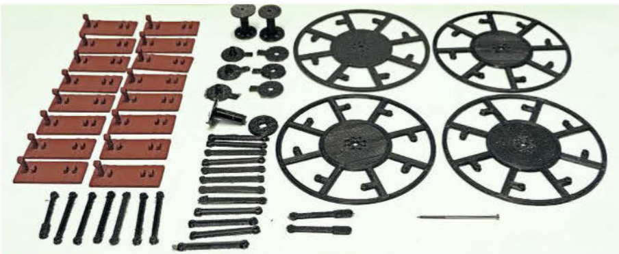
The next challenge! The 3D-printed components for feathering paddle wheels provided by Ron Rees.
