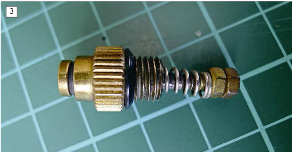
A very common valve found fitted to many older Cheddar boilers. These are simple yet effective, although with a rubber seat can start to leak after a while, meaning the rubber 'O' ring has to be replaced. Setting the valve could be quite a lengthy task though.
