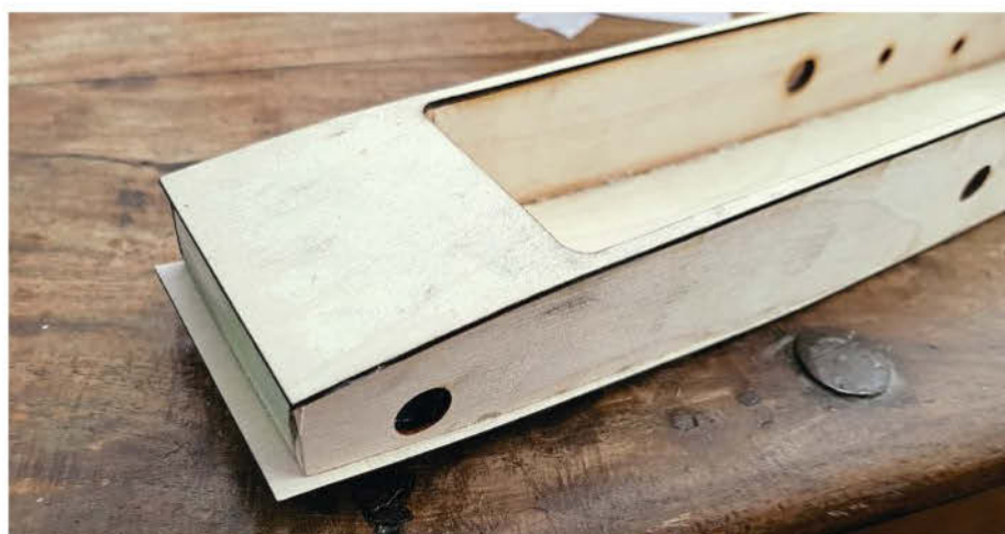
The top and bottom skins in place; note these have been left over-size and will be trimmed to fit later.
