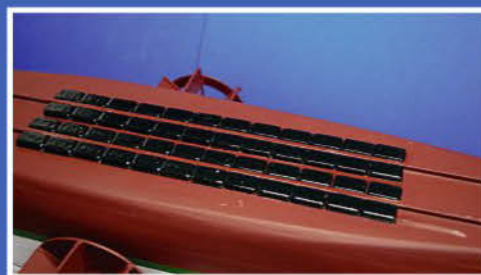
Additional ballast using motorcycle wheel weights (see text).
