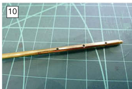
Simply gluing the rudder to the stock was never going to be strong enough so I pre-drilled the stock ready to take pins when it came time to fit the rudder.
