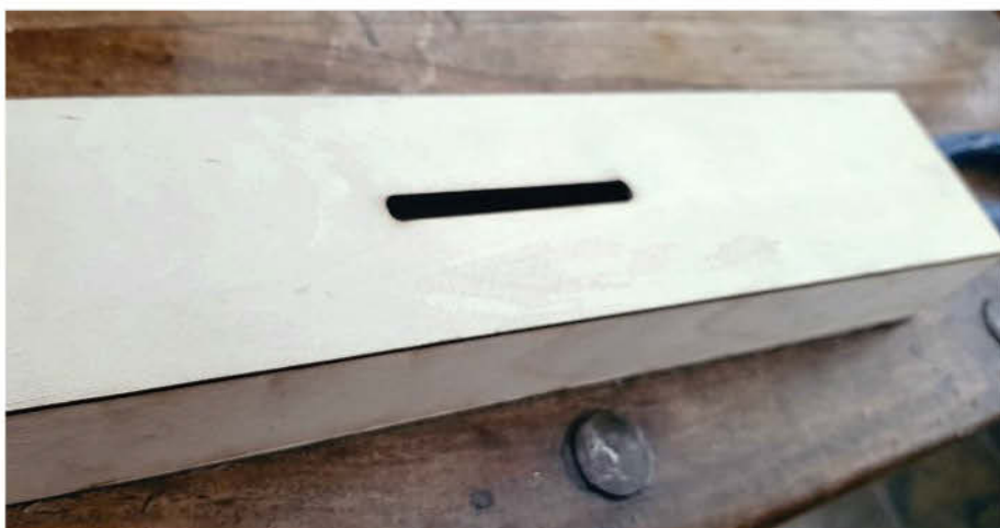
The bottom skin, showing the slot that's been cut for the prop shaft.
