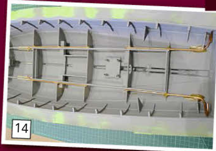
The space in the forward area of the frame had just enough room for the rudder servo but the connection needed to be fishing line led through copper tube.
