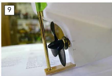
I replaced the keel extension with a piece of pine strip for strength and drilled for the rudder stock at the correct angle. You can see how little clearance there is for the propeller.
