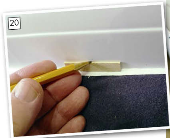
20 Marking out for the position of the rubbing strake with a spacer and pencil.
