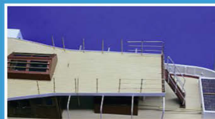
Railings under construction, as described in the text. A joint using sleeves and covered by a lifebelt will be used between stanchions.
