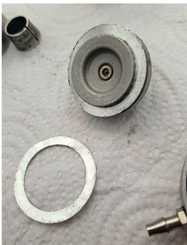
The head button with spacer shim.
