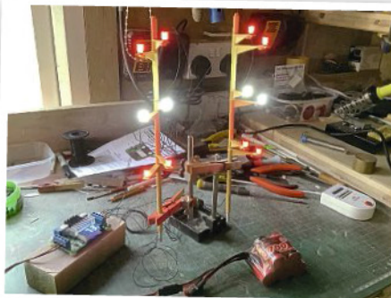
No resistors: lights running on 6-volt battery using voltage booster.
