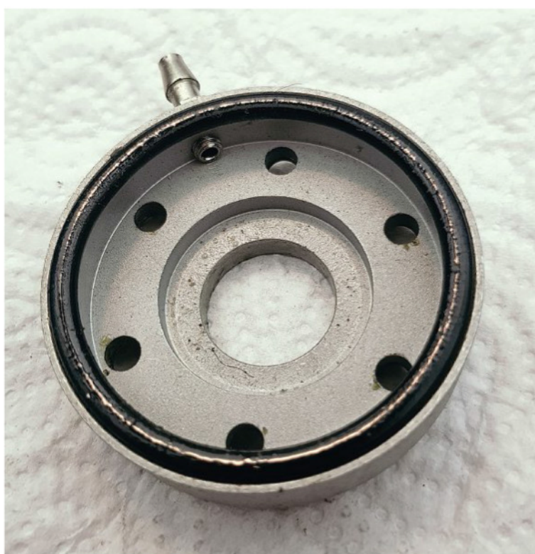
The water jacket with O ring seal.
