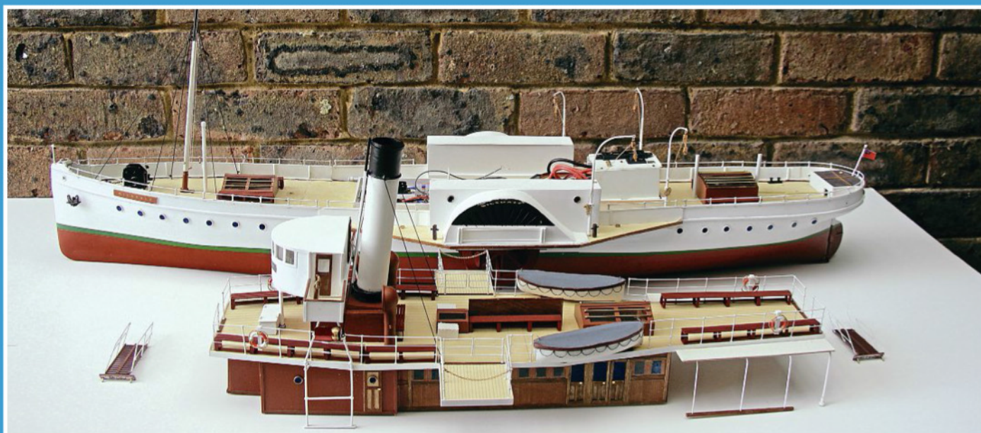
The promenade deck can be removed once the fore and aft stairs are unplugged and the lifeboat falls unhooked.
