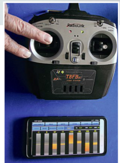
The clever Radiolink eight-channel TX can be programmed via an easy to use smartphone app.
