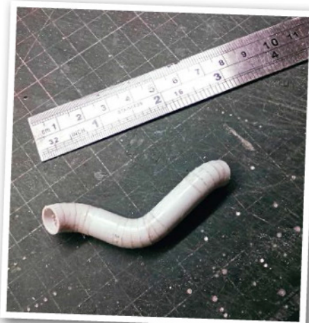
Shaping plastic tube into bends.
