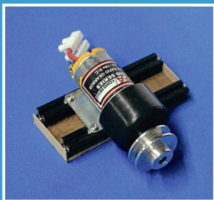
The geared MFA motor fitted to the adjustable Maker Beam mounting. The motor can be slid along the tracks and secured to adjust belt tension.
