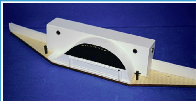
The completed paddlebox is held on by two bolts to brackets on the hull side. The portholes are for the lavatories, entered from the upper deck and which discharge into the paddle wash!
