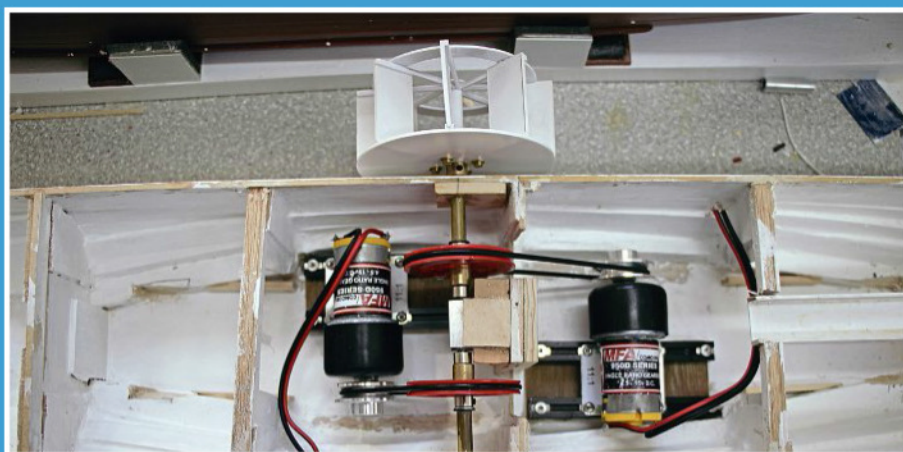
The two motors and final drive take up a lot of room in the central hull.
