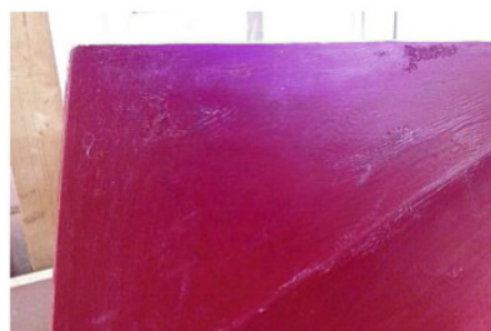
The hull after removal from mould; lots of sanding and filling were needed!
