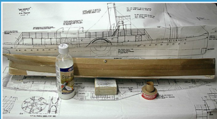
The hull being 'plated' with gumstrip paper and sealed with acrylic resin.
