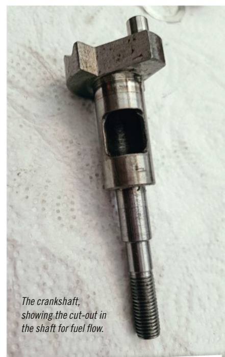
The crankshaft with its crank pin and fuel flow outlet web.
