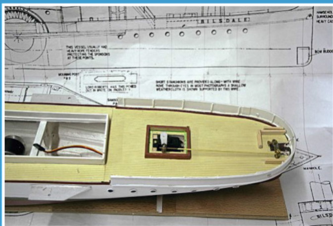
The cross-deck steering linkage (see text)
