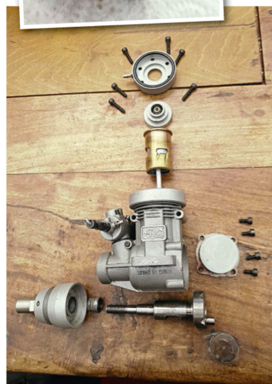
Right: Ready to be reassembled, following a light coat of after-run oil.
