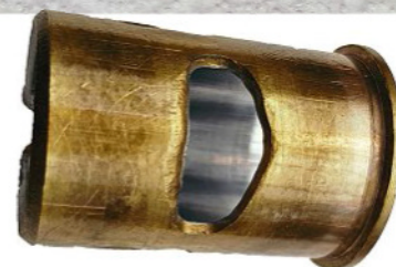
The brass sleeve, showing the exhaust port.
