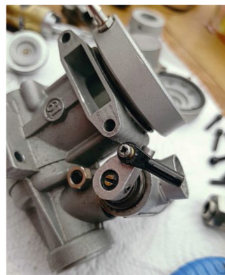
Small brass low end needle on the carburettor.
