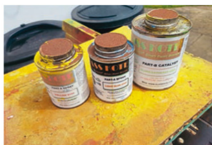
Typical products, including 2k primer, paint, hardener, clear lacquer and epoxy resin finishing resin used in conjunction with isopropyl alcohol.
