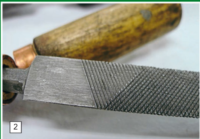
2 The surface of a flat file is quite interesting – although getting caught studying one might generate odd comments! You can, however, clearly see how the cut is coarser when the file is pushed lengthways and finer when it is drawn across the work.
