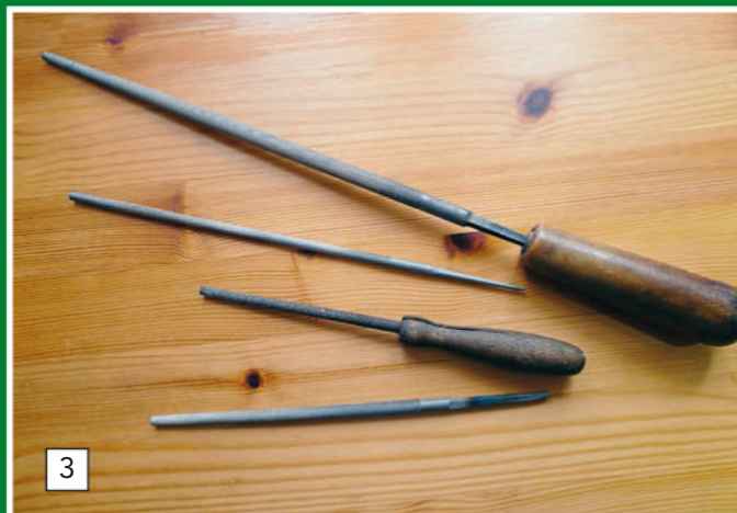
3 A selection of different size and grades of round file. Round files are designed to be used by hand, not put in a drill and used to open holes out! Note the ones that currently do not have handles fitted.
