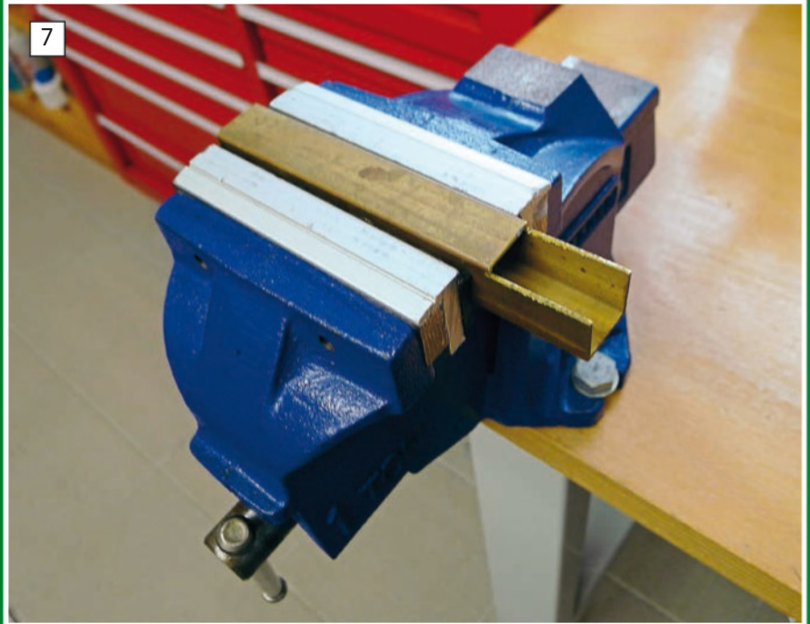
One of the first things you should fit out your home workshop with is an engineer's vice. The degree of ease this adds to a task (compared to holding something by hand) will make you wonder why anyone would even consider doing something without one. There again, there's always the 'G' clamp on the dining room table!
