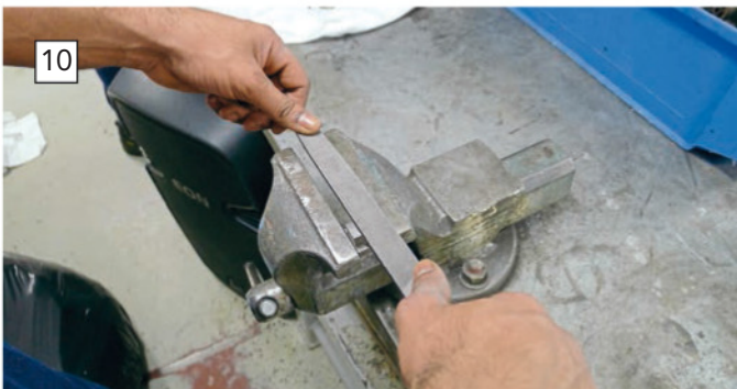
Final fine dressing up can be done by draw filing, using the file across the length. This technique is not as easy to control, so is usually kept to a few light strokes to smooth off the surface. If the file is used in this way for any length of time, the surface will frequently end up less than flat.
