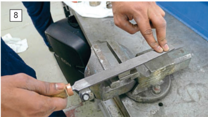
The standard filing stance. Control with the handle and apply pressure on the front of the file. Lighter pressure can be applied by just using a couple of fingers for finishing cuts and simple dressing up.
