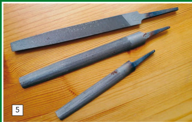
5 Another commonly found file configuration is the half round. Flat on one side but convex on the other, this is a handy configuration when dressing up internal curved surfaces. The flat face can also be used to draw file as it's cut in exactly the same way as a standard flat file.
