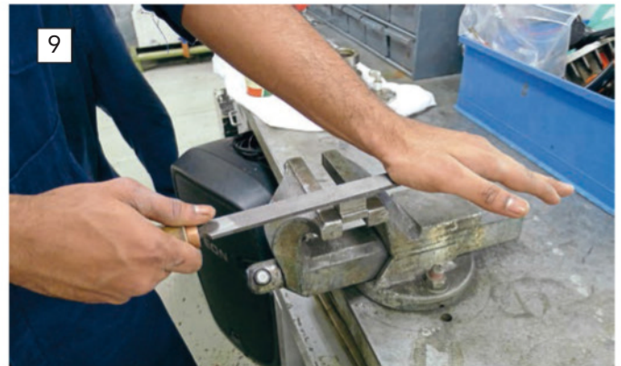
Pressure can easily be increased by using the heel of your hand, but control still remains with the handle.
