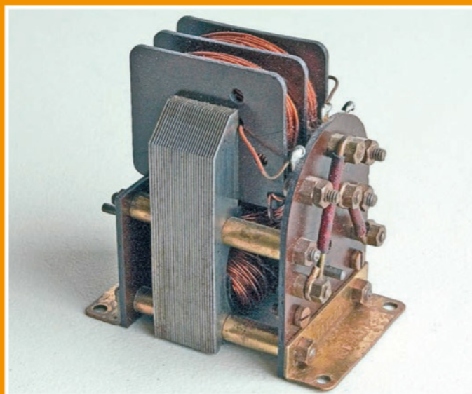
Early Torpedo with split field winding and wire links, rear view.
