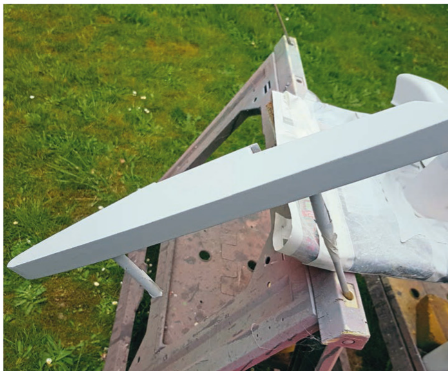
Parts being masked, prepped, primed and painted, finally resulting, after being lacquered, in this beauty
