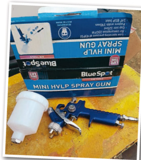
A typical small paint gun such as this one can be used for more intricate work.
