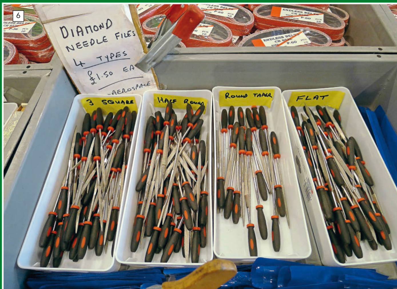
Richard tends to think of carborundum or diamond files as simply abrasive surfaces rather than files. They cut equally in any direction and tend to be available only in small sizes.
