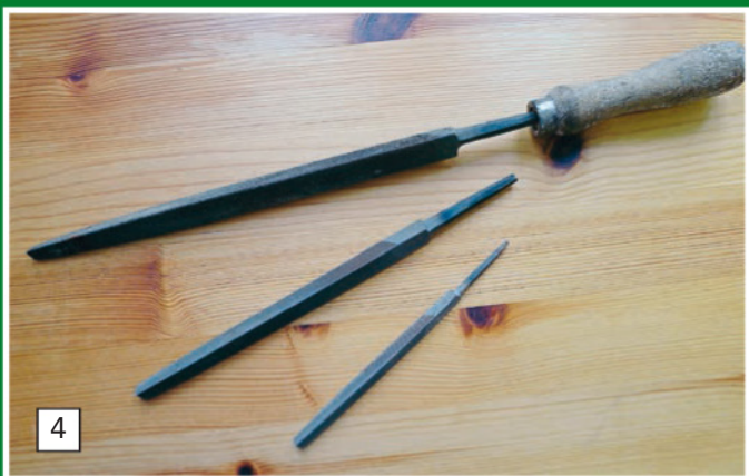
4 A selection of triangular files. These are very useful for dressing up traditional wood saw blades and cleaning out damaged screw threads.
