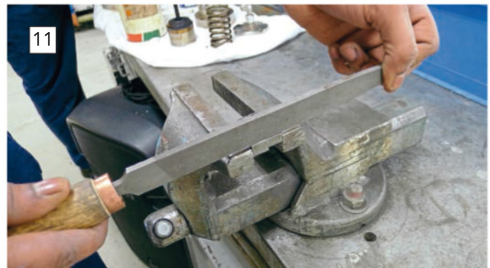
When filing an internal corner, always bear in mind where the cutting edge and the plain edges are. This will help prevent damage to the adjacent face that may then take a lot of correcting.
