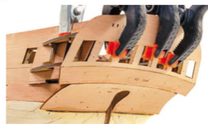
Getting the stern parts properly aligned can be tricky. The secret is to start at the top and work downwards so no gaps appear later.
