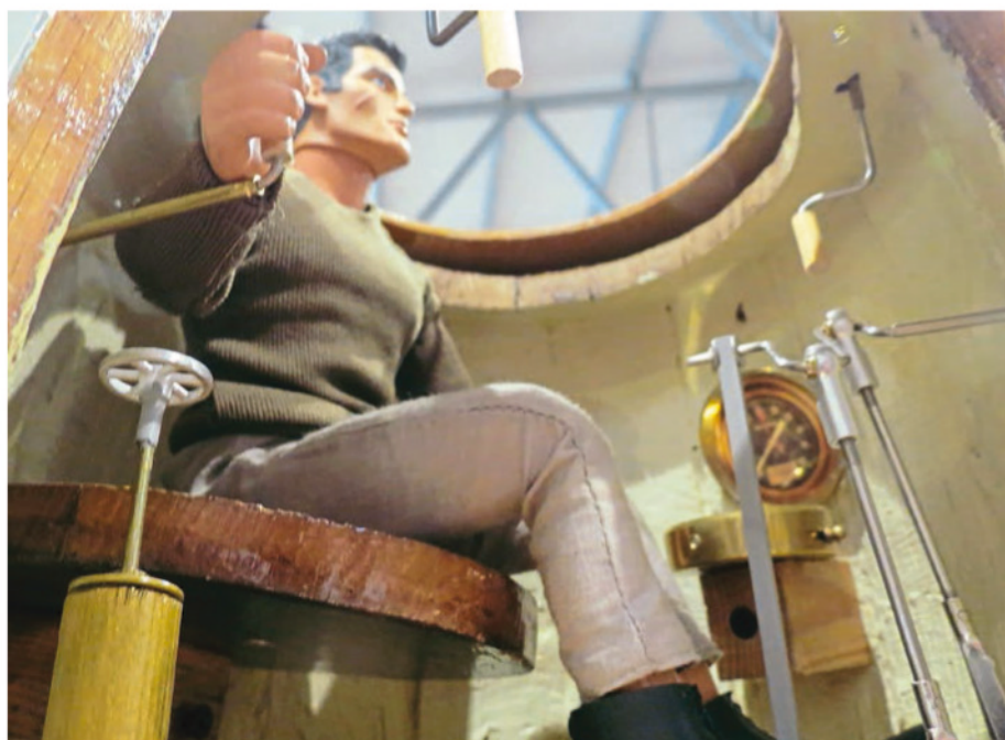
Lionel Broadbent's 1:12 scale model of Bushnell's historically fascinating covert attack submarine Turtle (as featured in the February 2023 issue of Model Boats ), complete with hand cranked propeller. If you look closely, you'll note the hand cranked auger for drilling holes in wooden hulls.
