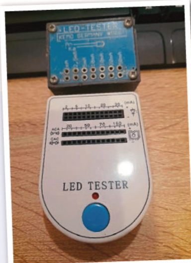
LED testers save so much time when installing LED lighting.
