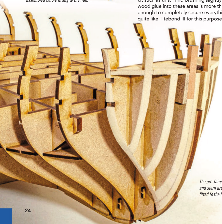
To aid the ease of fairing the hull, the bow and stern bulkheads are glued and assembled before fitting to the hull.
