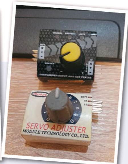
Servo testers allow you to easily assess performance ahead of rigging up your radio system.
