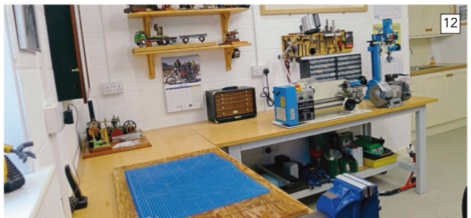
Richard's work bench today, with machine tools and workbenches that have followed him around for many years. A thick ply board protects the workbench top, and a cutting mat protects that.
