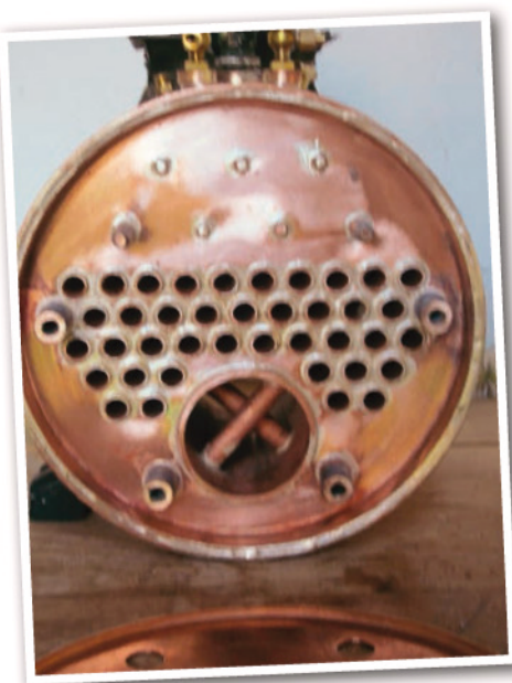
Alasdaair's new boiler with its end plate removed, showing fire tubes and firebox cross bracing.
