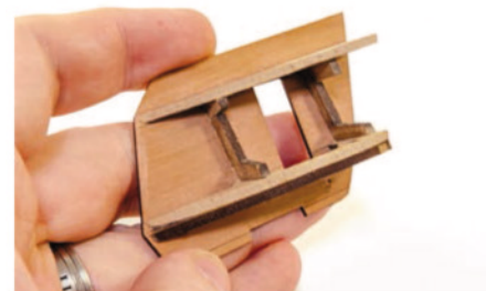
The quarter galleries start out as simple skeletal assemblies, including the hole for the 'seat of ease'.
