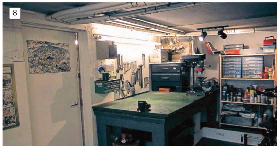
Richard's first real metalworking bench: nothing more than a pedestal drill, a grinding wheel, a vice, shadow board and suitable tool storage. This work bench was where he learnt the basic workshop skills, using mostly hand tools. That huge bench cost him just £30 from a carpenter's shop clearance.
