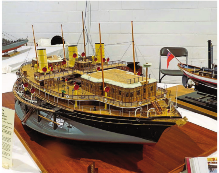
Built to original plans at 1:48 scale, John Hollis's scratch built live steam-powered replica of the circular Imperial Russian Royal Yacht Lavadia.
