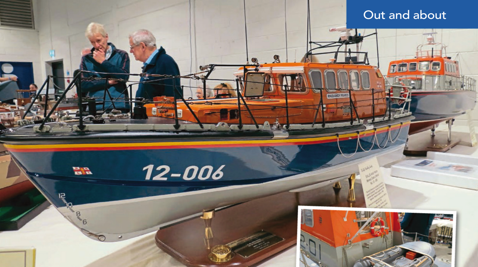
This award winning 1:12 scale model of the Mersey class RNLI lifeboat RNLB Andy Pearce is almost an exact copy of the full-size vessel and could be considered the benchmark for model lifeboat construction.
