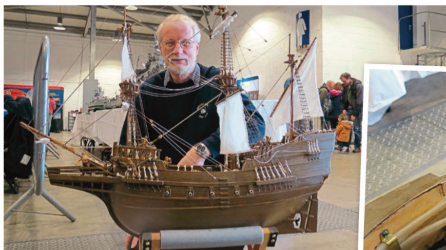
The fully working model of a 17th century man-of-war developed and built from scratch by David Moss. Each one of the brass cylinders fitted contain a smoke charge for each of the cannons, which on the model can be operated as a single shot or as a rolling broadside.
