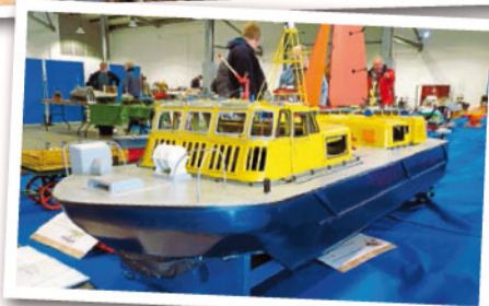
Hovercrafts also formed part of the displays, such as this 1:16 side wall HM2 built from balsa and light ply and using a single brushless motor for lift and two for thrust.
