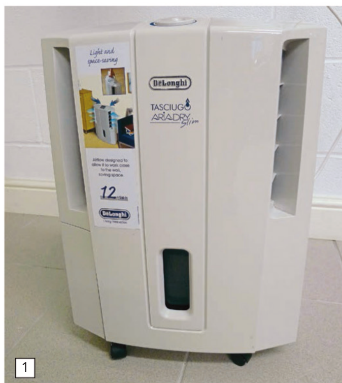
Running a dehumidifier (these are not expensive to buy and don't use a great deal of energy when used continuously) may be worth considering to prevent tools developing a film of rust.
