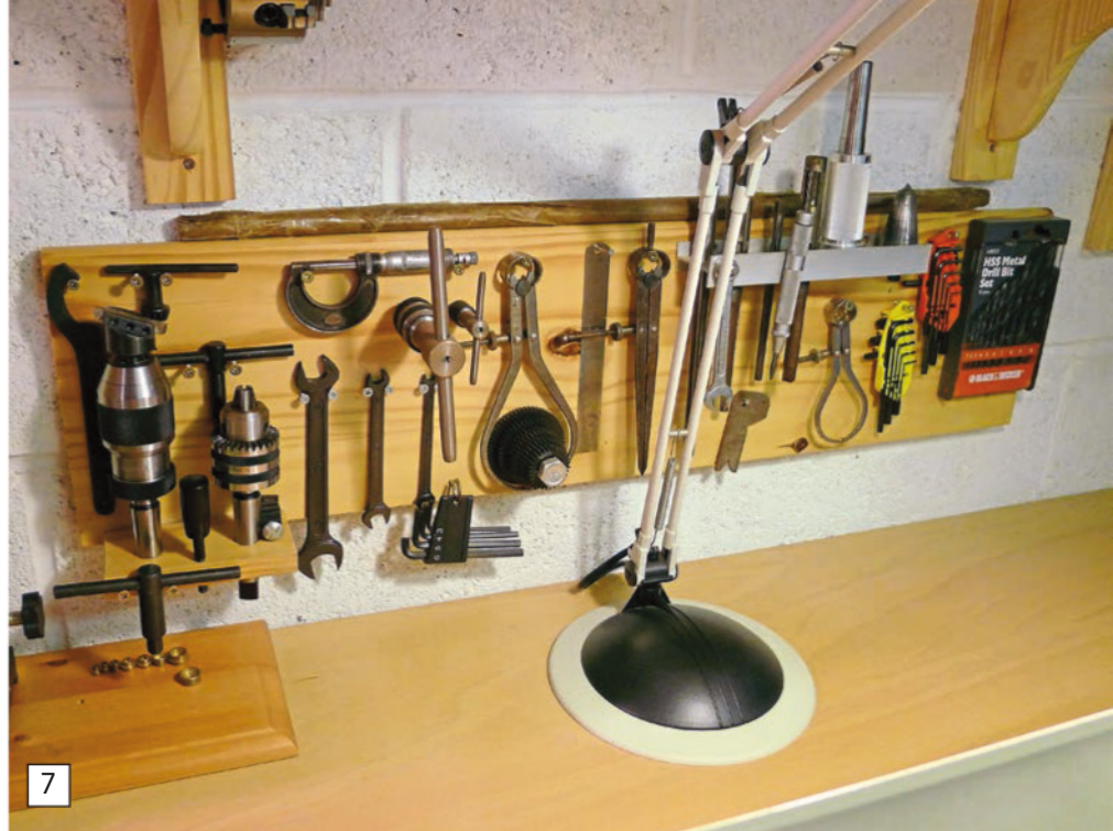
Shadow boards, Richard explains, are a throwback to his seagoing days and he's put them to good use in his own workshop. They allow everything to be immediately accessible; the only discipline required, in order to keep things ship shape, is that you remember to put anything used back on the board at the end of the day.
