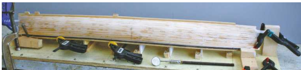
ABOVE: The construction stages of a plank on frame hull. (Image courtesy of Brian King)
