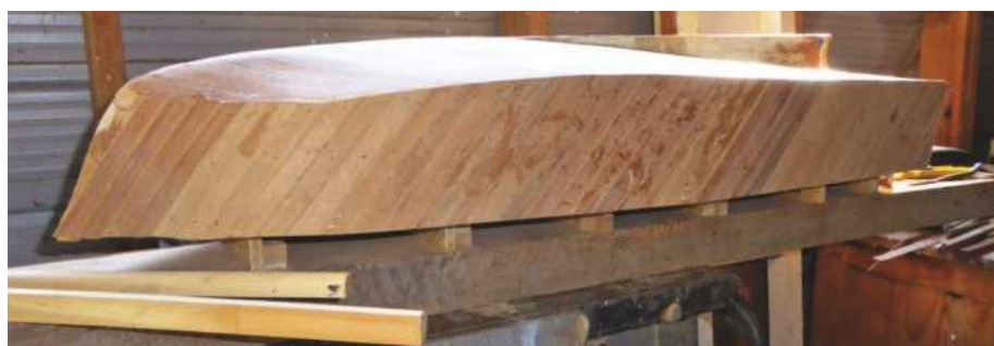
The outer diagonal planking coupled with an inner skin not only makes for an attractive finish but a structurally sound one too!
