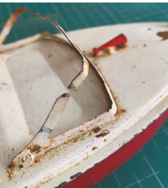
ABOVE: Rust had eaten clean through this old tin toy's windscreen strut.
