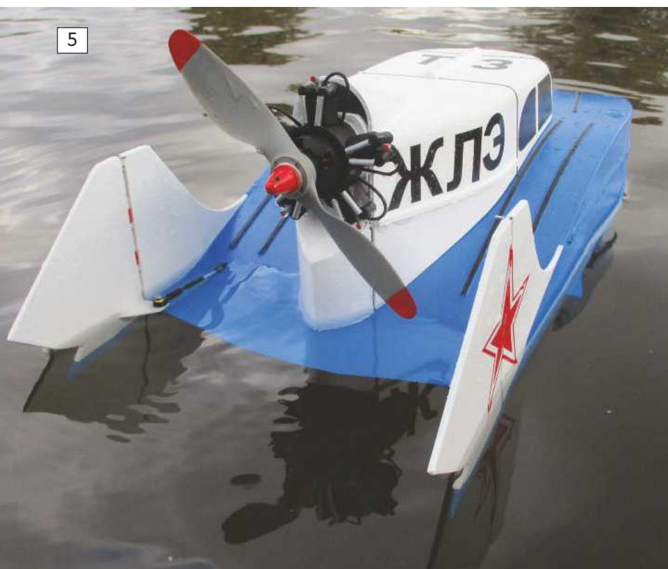
ABOVE: The tail fins showing Ashley's plywood lamination, and the brass strip and hinges incorporated. BELOW: In this view of the cylinder engine sported by Ashley's Tup, notice the water just over the rear shelf; this clears as soon as the boat moves forward.
