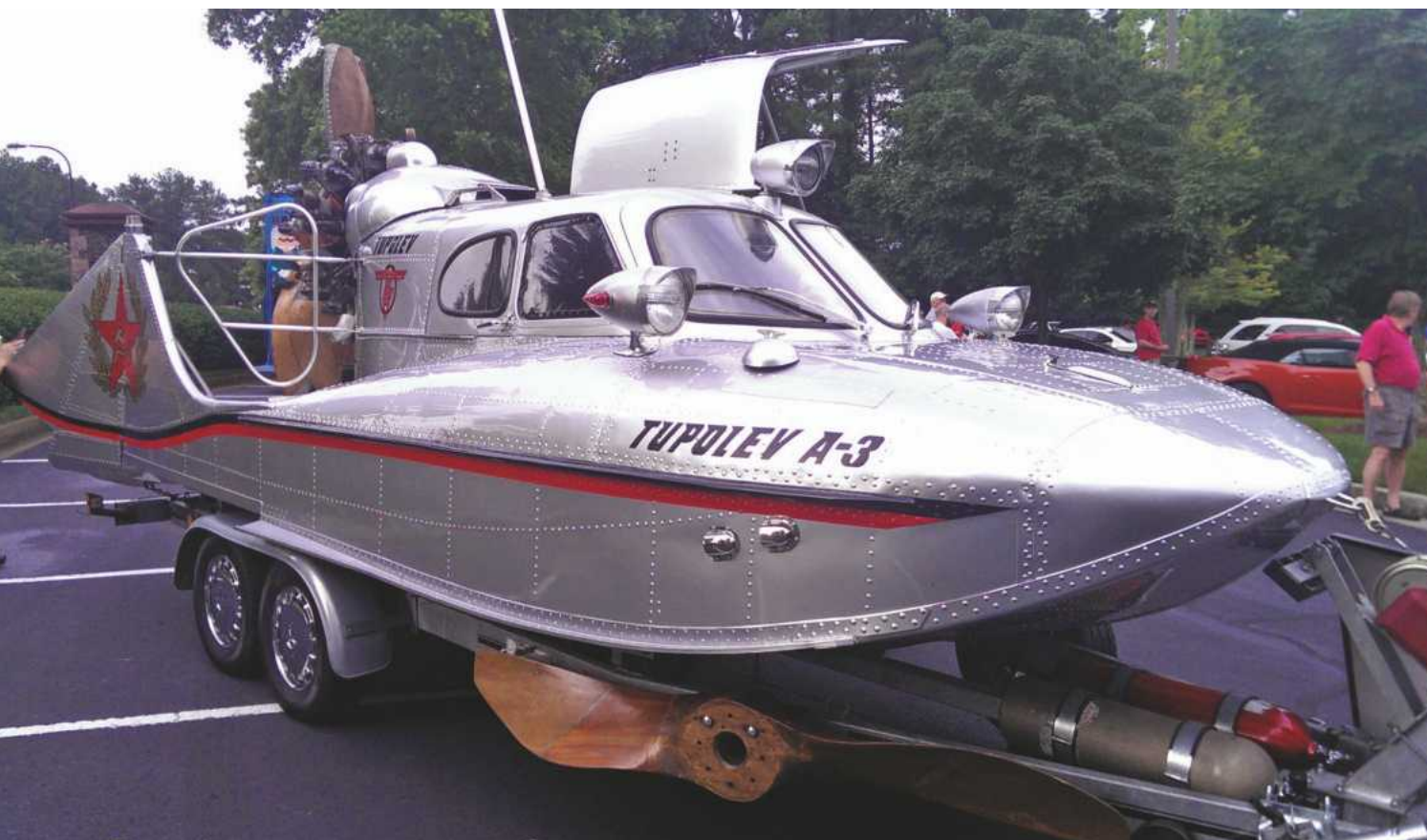
The very futuristic-looking Tupolev A-3 Aerosledge: an all-metal amphibious aerosledge designed to transport passengers and light freight in remote areas of the Soviet Union. Officially known as the A-3 'Hope' ('Nadezhda' in Russian), it uses a single pusher propeller mounted behind the enclosed cabin to propel the craft over snow, ice or water. Image courtesy of Brandon Adams.
