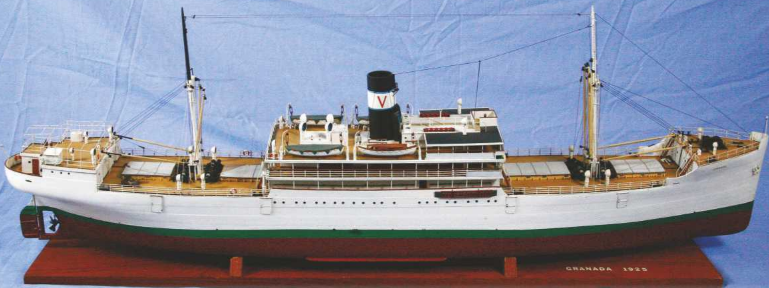
ABOVE: Colin's SS Granada built in 1979 was a classic 'scratch-built' model, with the anchor chain being the only commercial fitting. BELOW LEFT: Repurposing 1: the cargo winches on Granada incorporated eyelets and wheels from Airfix tank kits. BELOW RIGHT: Repurposing 2: the fire buckets on the wheelhouse roof are in fact toy pistol 'caps'.
