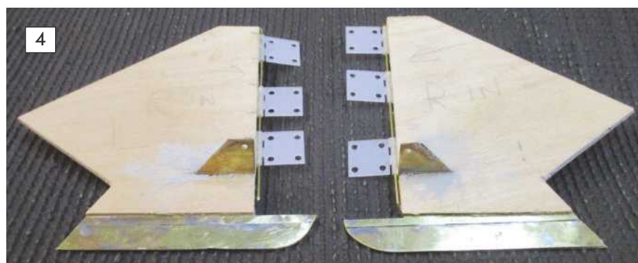
ABOVE: The tail fins showing Ashley's plywood lamination, and the brass strip and hinges incorporated. BELOW: In this view of the cylinder engine sported by Ashley's Tup, notice the water just over the rear shelf; this clears as soon as the boat moves forward.
