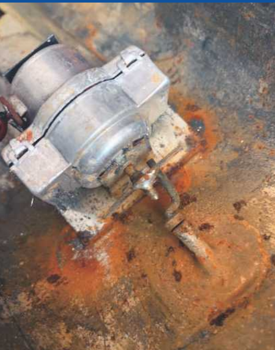
ABOVE: Although the motor, an early Mabuchi-style Japanese 2x permanent magnet, did run, it would need removing and replacing.
