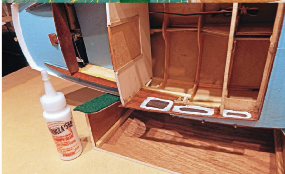
ABOVE: Acetate cabin window glazing, with canopy glue, which dries clear.
