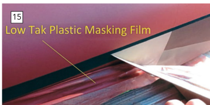
ABOVE LEFT: The arms of the upper platforms were also masked. ABOVE RIGHT: Using Ultra mask as an alternative to masking tape improved both performance and results. BELOW LEFT: Applying wide area low tack plastic masking film for masking the hull prior to airbrushing the boot topping. BELOW RIGHT: Here the low tack tape is combined with a plastic sheet.
