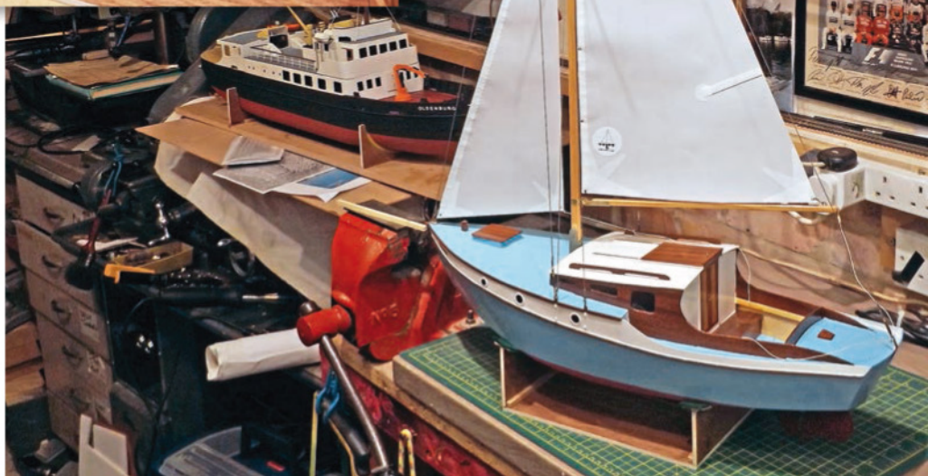
ABOVE: Acetate cabin window glazing, with canopy glue, which dries clear.
