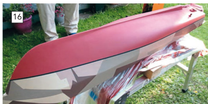
ABOVE LEFT: The arms of the upper platforms were also masked. ABOVE RIGHT: Using Ultra mask as an alternative to masking tape improved both performance and results. BELOW LEFT: Applying wide area low tack plastic masking film for masking the hull prior to airbrushing the boot topping. BELOW RIGHT: Here the low tack tape is combined with a plastic sheet.
