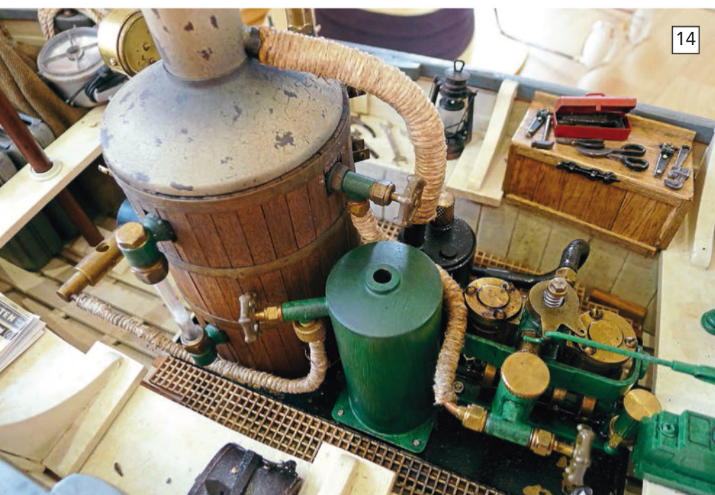
Even a very simple compact plant with only a couple of pipes can be elevated by the use of some lagging and a bit of weathering to make a much more realistic looking steam set up. Richard has found this also seems to attract more comment than a highly polished example.
