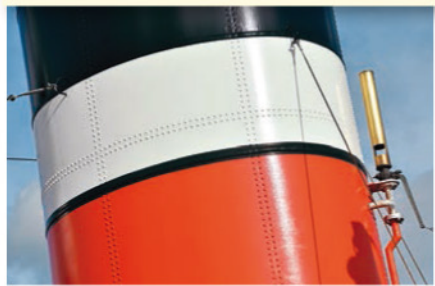
ABOVE: Waverley's steam whistle mounted on the fore stack.
