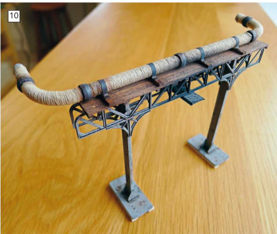
While admittedly for model railway use, the lagging, fittings and weathering are all on a piece of bent copper pipe from Richard's steam spares box and could just as easily be used, minus the plastic gantry of course, in a model boat.
