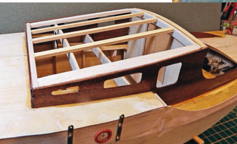
ABOVE: The cabin roof balsa frame built to fit with obeche support rails.
