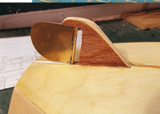
ABOVE: The completed hull removed from the building board and sitting on the building stand. LEFT A close up of the brass rudder blade soft soldered to the stock.
