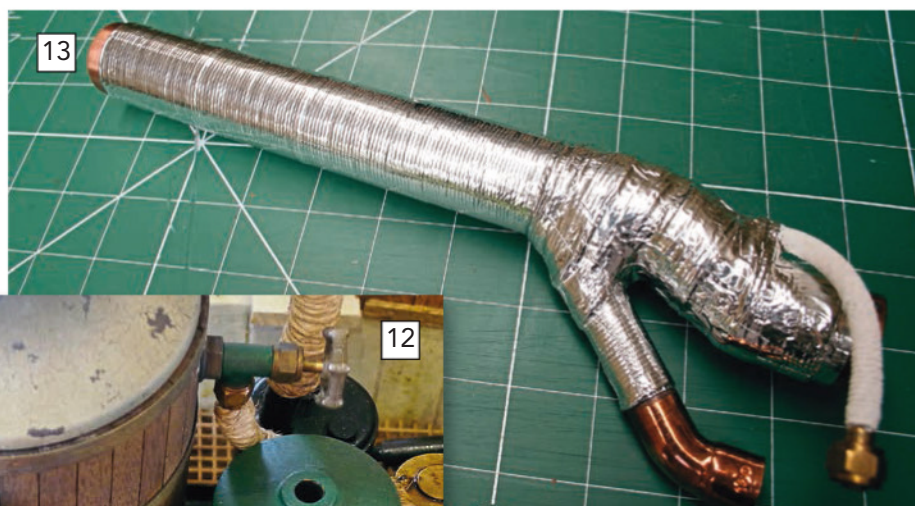
ABOVE: A complex boiler flue Richard made a few years ago to fit a steam coaster model. The engine steam exhaust was initially painted; however, realizing the error of his ways, Richard later applied lagging and foil covering. Insulating the boiler flue might be worth doing in an enclosed model.
