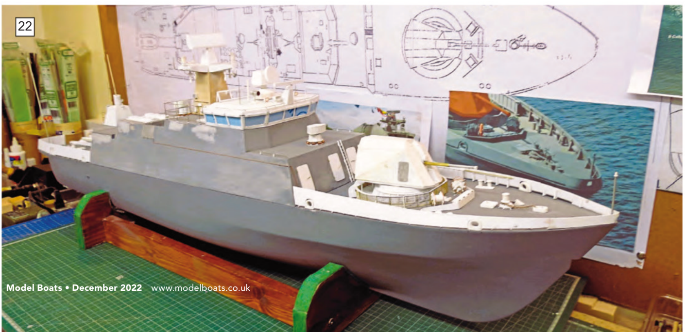
BELOW: A full 'dry run' of all the fittings, which will reveal and allow you to rectify any potential problems prior to air brushing.
