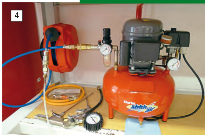
ABOVE LEFT: Running in by using a lathe to turn the engine is a perfectly acceptable method of doing things, provided a longer engine is supported at both ends of the crank shaft and the paintwork is protected from damage. ABOVE RIGHT: A typical 9-litre reservoir home workshop compressor fitted with a drier ensures you're not putting moisture through your engine during the running in, and a pressure regulator will enable accurate speed control.
