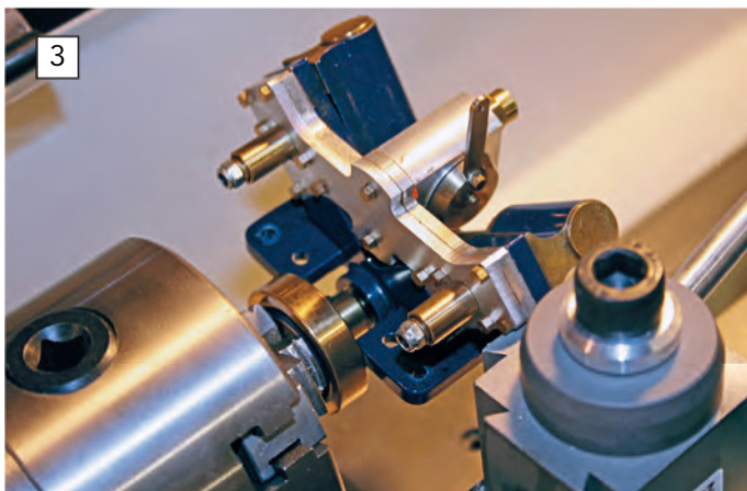
ABOVE LEFT: Running in by using a lathe to turn the engine is a perfectly acceptable method of doing things, provided a longer engine is supported at both ends of the crank shaft and the paintwork is protected from damage. ABOVE RIGHT: A typical 9-litre reservoir home workshop compressor fitted with a drier ensures you're not putting moisture through your engine during the running in, and a pressure regulator will enable accurate speed control.
