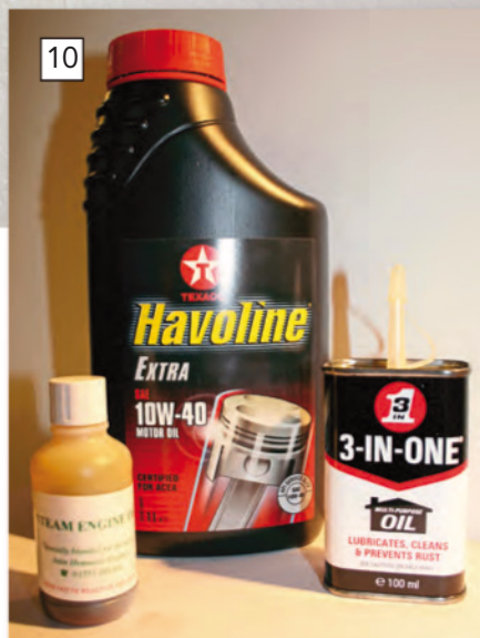
10 Steam oil is way too thick when cold, while household light oil is way too thin. Common or garden engine oil is fine for both the internal surfaces and the external surfaces of your engine during the running in process.
