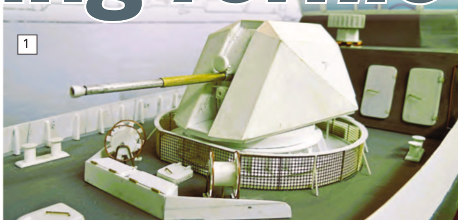
Installing the fittings for a so-called 'dry run', which includes the cordage reels.
