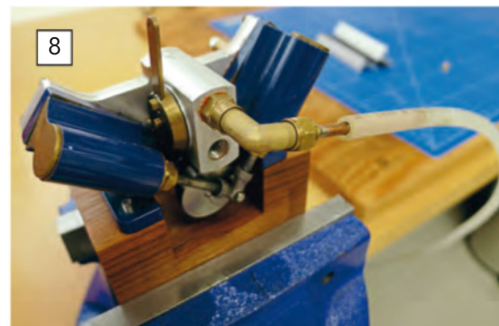
Here the air line is fitted and ready to go. In this case a hard flexible tube has been used, meaning the fitting will need disconnecting to add some oil to the engine, which can be a bit of a chore. You only need low pressures to run in, though, so even pushed on silicone tubing will do the job.
