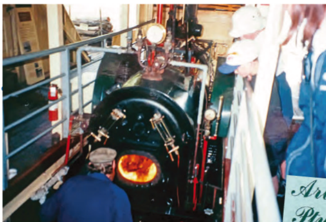
ABOVE: The Alexander Arbuthnot's wood-fired boiler. INSET RIGHT: John's ticket for his trip on the Alexander Arbuthnot, now a 24-year-old memento.
