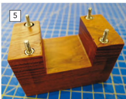
Making up a block of wood to hold your engine is not a difficult task and makes maintenance in the future that little bit easier. The screws here are simply tapped into close fitting holes with two-part epoxy around them.
