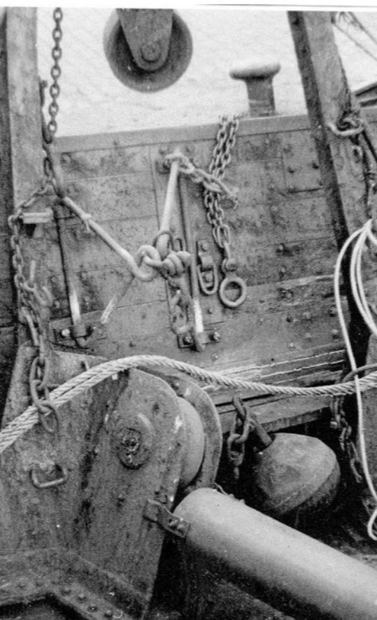
ABOVE: Forward gallows on starboard side, with trawl door outboard and angled sheave at base of gallows.
