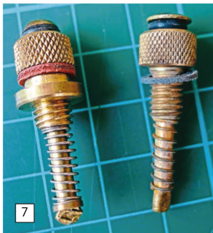
Some smaller and older types of safety valve consist of a spring held by a crimped shaft; this is nonadjustable, and the 'O' ring sealing face is not easily replaced – even if you did replace it, you wouldn't be able to set the valve to working pressure. These are, therefore, best swapped out.
