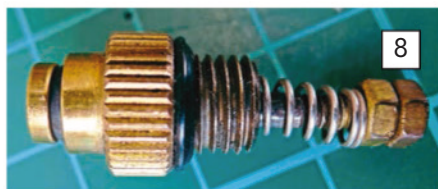
At least the old Cheddar type of valve can be adjusted, and the seat can be replaced. The challenge is that it has to be removed from the boiler.
