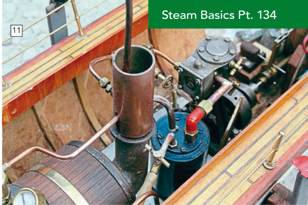
Checking for play in a plant that's already fitted into a model can be challenging. Excessive play in bearings though, can potentially be very time consuming and expensive to correct, so you really need to try and get your hands on the crankshaft.
