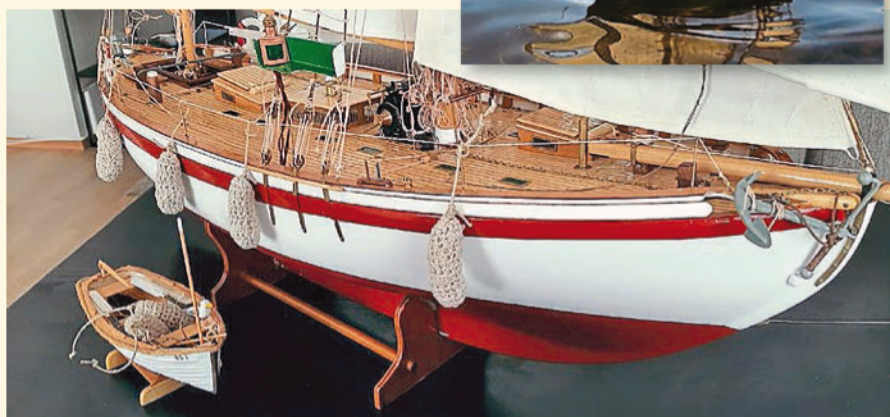
Built from a Billing Boats kit, George has added both R/C equipment and some astonishing detail to his model of the Colin Archer RS1, including a perfectly matched to the original and illuminated interior. A hull purchased from Sarik Hobbies formed the basis for the charming little Nordlandsjolle dinghy.
