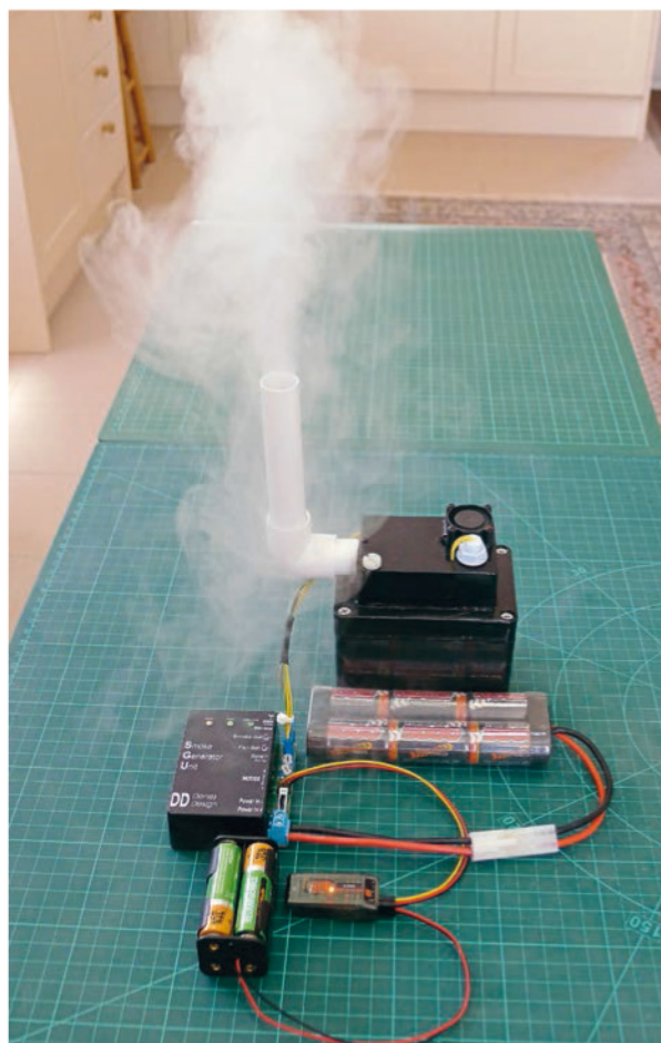
ABOVE LEFT: The prototype unit as supplied. Note, on top of the tank, the level switch and the fan unit with the pre-fitted stub for the exhaust. Controls include smoke quantity, fan speed and one of four different modes. ABOVE RIGHT: A quick test on the bench demonstrates the impressive quantity of smoke generated. A 7.2-volt battery was used for this test, demonstrating the voltage flexibility. The smoke follows the throttle signal closely.
