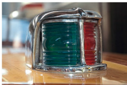
ABOVE: Capri runabout running light detail.
