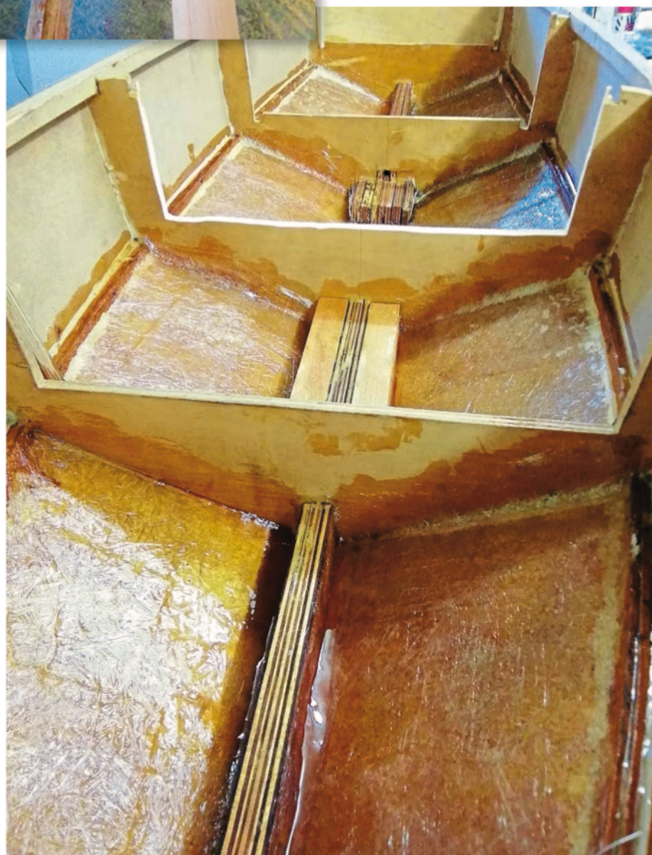
The lower panels of the dinghy were strengthened with fibreglass matt and resin. The inner sides were kept free of the resin as John planned to stick plywood planks onto these surfaces.
