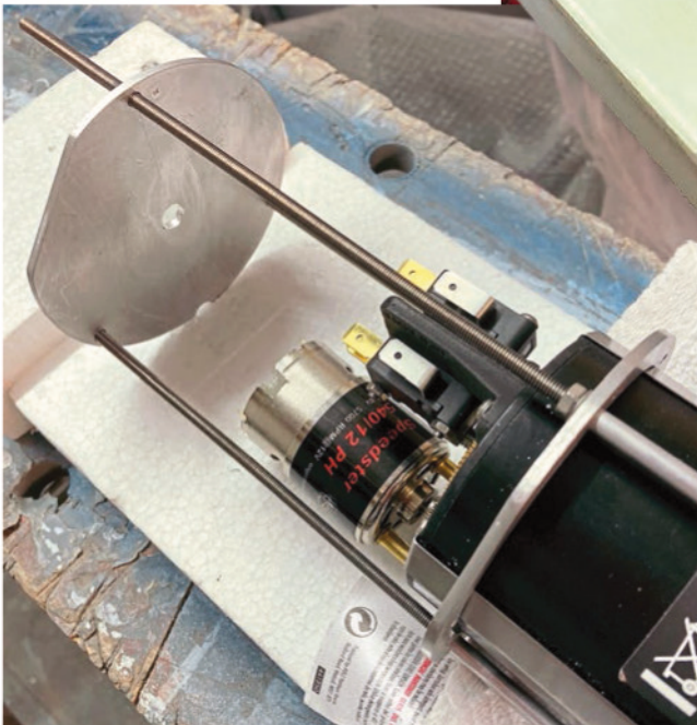
ABOVE: The aluminium discs that can be seen here cut from 3mm aluminium sheet, and then trued up on the lathe. These discs can be cut for you by Lazermaster ( www.lazermaster.co.uk ) if you're unable to tackle the task yourself. Note the 4mm studding and aluminium tubes that form the spacers between the aluminium discs.
