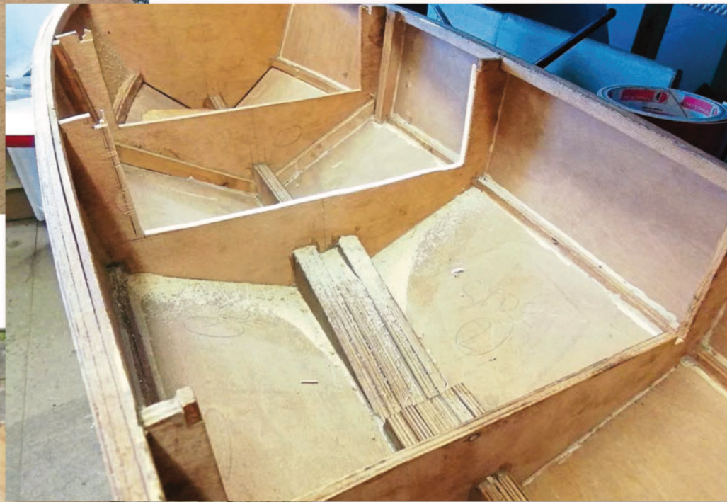
ABOVE: The hole in the underside plywood skin was repaired with a patch of plywood on the inside, and a skim of filler on the outside. RIGHT: Using a coping saw, the original cabin end wall was removed. The boat now resembled a rowing boat.
