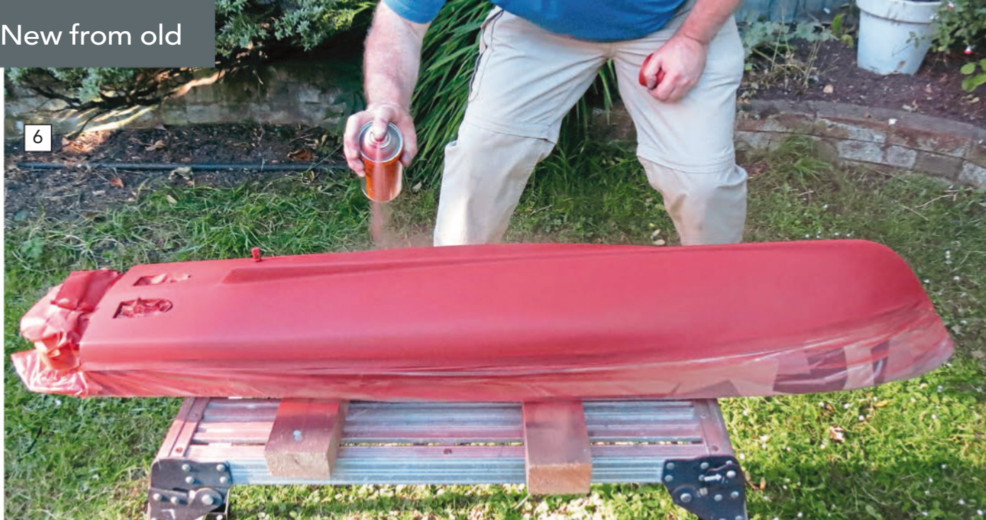
ABOVE: Spraying red anti-foul with a Halfords spray can, a task seen performed here out in the open on a calm, warm day. BELOW: Job done!
