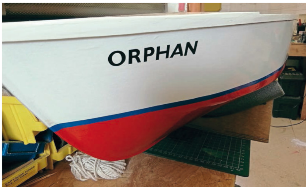
The hull was brush painted using Phoenix enamel paints. Brush painting saves an enormous amount of time masking off and cleaning up. The paint can be 'laid' on with the brush, giving a very durable finish.
