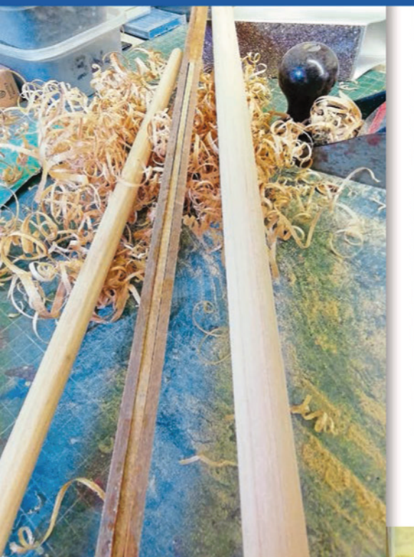
ABOVE: The cause of all John's problems and the ingredients for disaster! LEFT: The mast and boom, etc, were planed up. Each was formed by gluing a series of strips of wood together. At this stage they were made longer than necessary in order that they could be cut to length when fitted to the dinghy.
