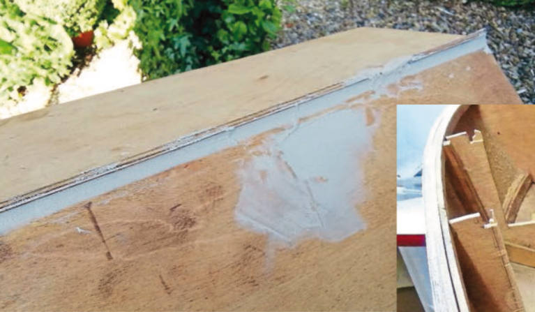
ABOVE: The hole in the underside plywood skin was repaired with a patch of plywood on the inside, and a skim of filler on the outside. RIGHT: Using a coping saw, the original cabin end wall was removed. The boat now resembled a rowing boat.
