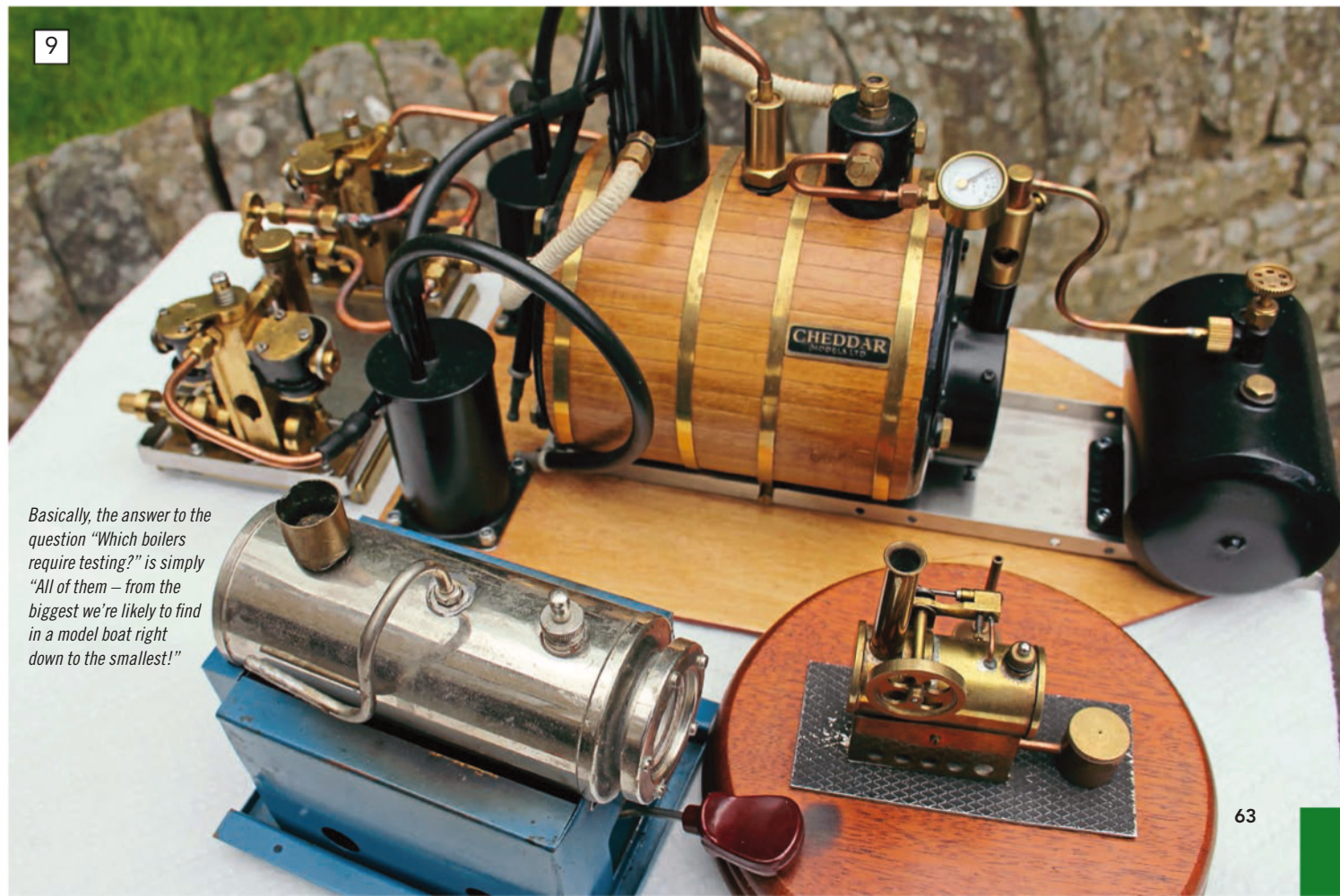
Richard made up a branch consisting of a stop valve, to assist in raising pressure, and a pressure gauge to see what was actually going on inside this boiler, instead of simply 'flying blind'.
