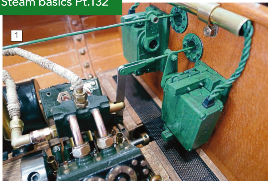
1 ABOVE: The position of the two engine control valves lent themselves perfectly to allowing an extension of the levers into the cockpit area. The operating rods were simply passed through bulkhead penetrations and located on the servo arms by swivel pins. BELOW: A 90-degree bend and the extension by brass tubes gave a credible look to the cockpit side, particularly when finished off with a couple of turned wooden handles at an appropriate height for the figure.
