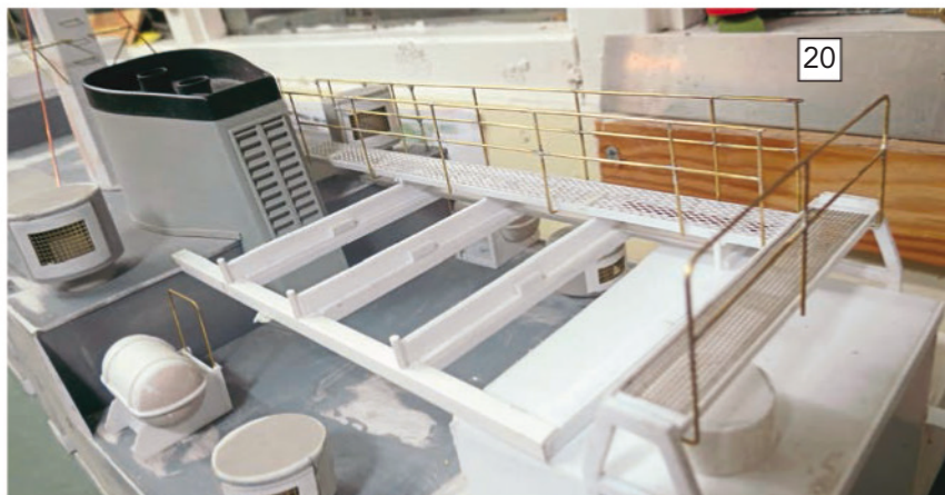
ABOVE LEFT: The starboard side walkway slotted onto the platform. ABOVE RIGHT: Both starboard side and after walkway in place.
