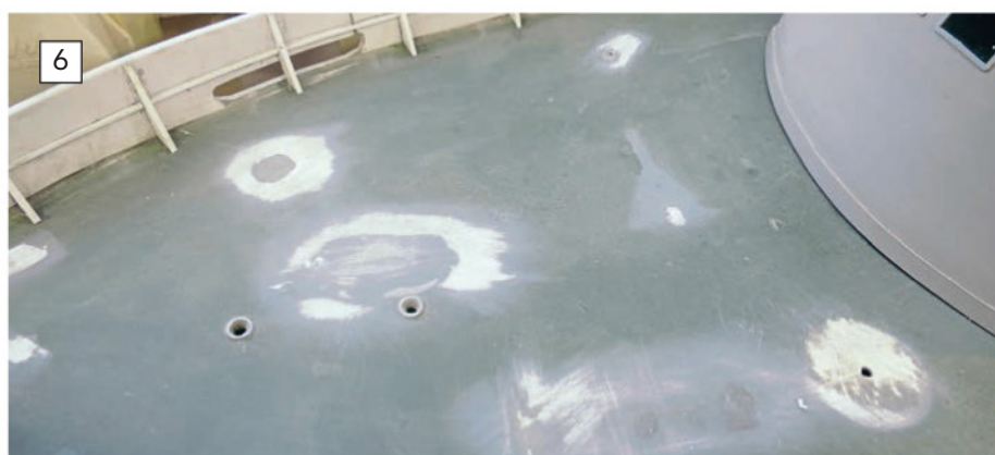
ABOVE: Removing the original fittings from the styrene deck required a level of care. BELOW: The exterior of the original hull completely stripped in preparation for the re-build.
