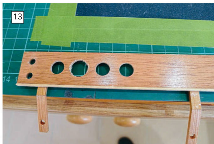
ABOVE LEFT: A softwood frame and a piece of a wooden kitchen venetian blind provided the base for Richard's gauge panel. ABOVE RIGHT: Holes were first drilled between two blocks of wood, then carefully reamed out to the right size for the the port holes.
