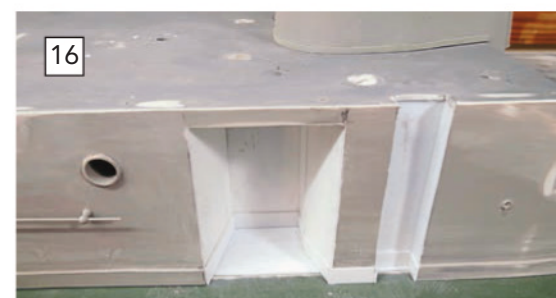
BELOW: The new openings created in the port side amidships.
