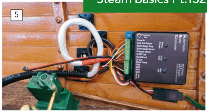
ABOVE LEFT: The starboard side electronics package consists of the Engine Control Unit and the receiver, complete with their own dedicated battery. The battery is mounted inside the wooden box to enable easy charging. ABOVE RIGHT: The Automatic Boiler Control unit sits in the port side locker to give the most convenient access to the two control valves and the two boiler sensors.
