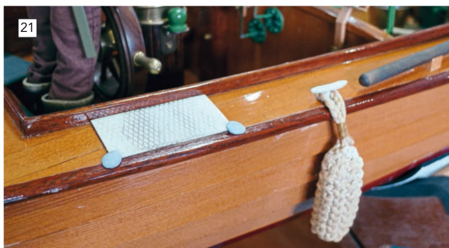
The metal cast fittings were sourced from a marine model supplier, which Richard painted with etching primer and enamel. The fenders are bespoke items from a supplier who was happy to create them to Richard's own design and dimensions, while the step was fashioned from a piece of aluminium chequer plate, which Richard painted and then 'scuffed' with some fine wet and dry.
