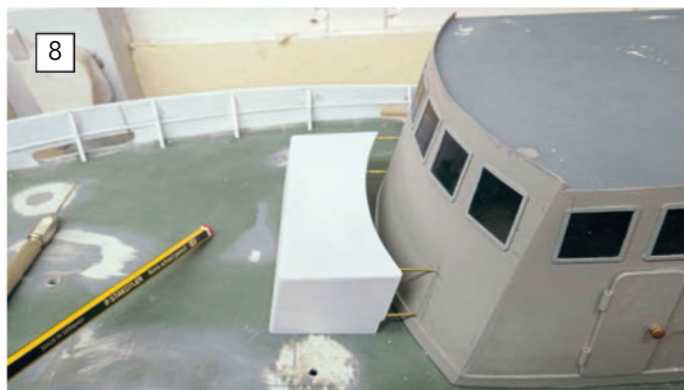
ABOVE LEFT: A forward extension to the original deck housing. ABOVE RIGHT: Adding a new roof and upper bridge area.
