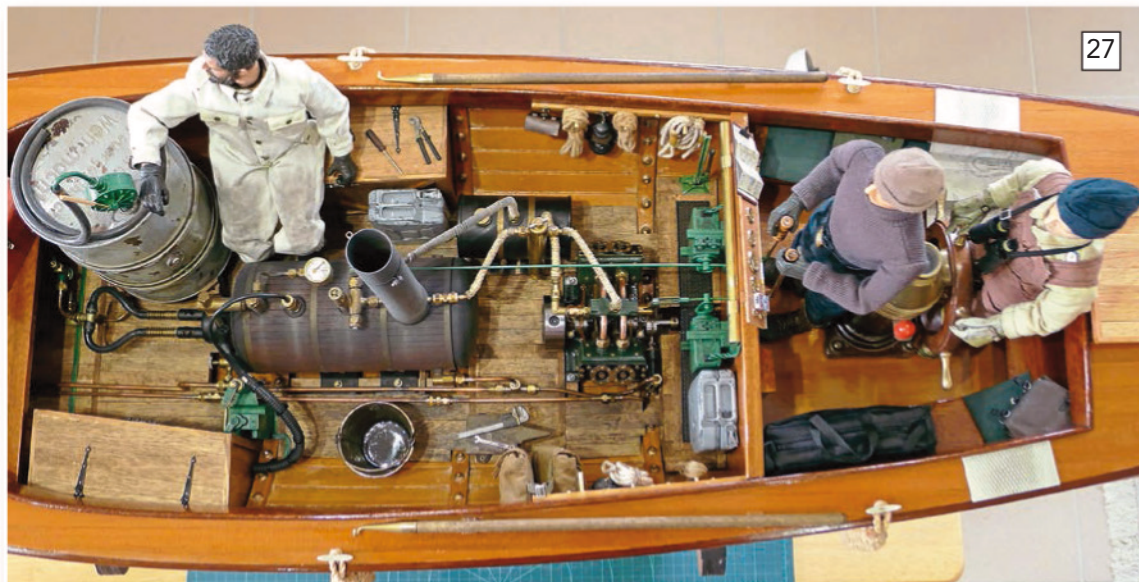
ABOVE: Richard has achieved a very credible contrast between what's obviously a very well maintained and constantly cleaned engine and the grubbier and more workboat like surrounding detail. The weathered boiler flue is clearly visible, as are the soot deposits on the top surfaces of the boiler. BELOW: This overall shot taken from above affords a good view of the internal detail. A few tools, some ropes and a couple of lanterns add credible clutter, while a couple of bags in the cockpit area provide suitable visual interest there, too.
