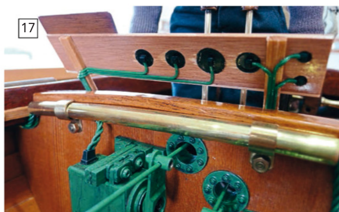
ABOVE LEFT: By gluing the gauge faces to the rear of the porthole, rather than gluing them directly to the back of the glass, a proper depth to the front view and a much more realistic look can be achieved. ABOVE RIGHT: As the rear face of the panel is just as visible as the front face, this also required detailing. Note how neat and realistic the dummy painted copper pipes led down the legs look.
