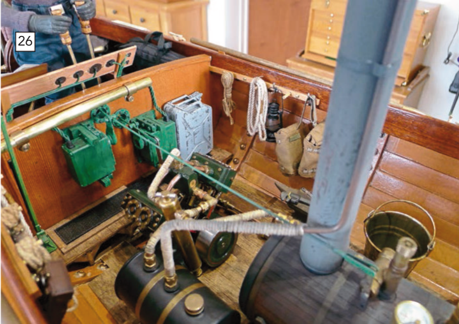
ABOVE: Richard has achieved a very credible contrast between what's obviously a very well maintained and constantly cleaned engine and the grubbier and more workboat like surrounding detail. The weathered boiler flue is clearly visible, as are the soot deposits on the top surfaces of the boiler. BELOW: This overall shot taken from above affords a good view of the internal detail. A few tools, some ropes and a couple of lanterns add credible clutter, while a couple of bags in the cockpit area provide suitable visual interest there, too.
