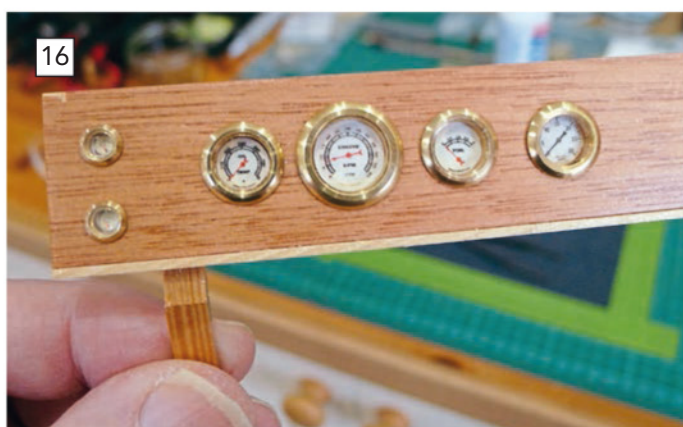
ABOVE LEFT: By gluing the gauge faces to the rear of the porthole, rather than gluing them directly to the back of the glass, a proper depth to the front view and a much more realistic look can be achieved. ABOVE RIGHT: As the rear face of the panel is just as visible as the front face, this also required detailing. Note how neat and realistic the dummy painted copper pipes led down the legs look.
