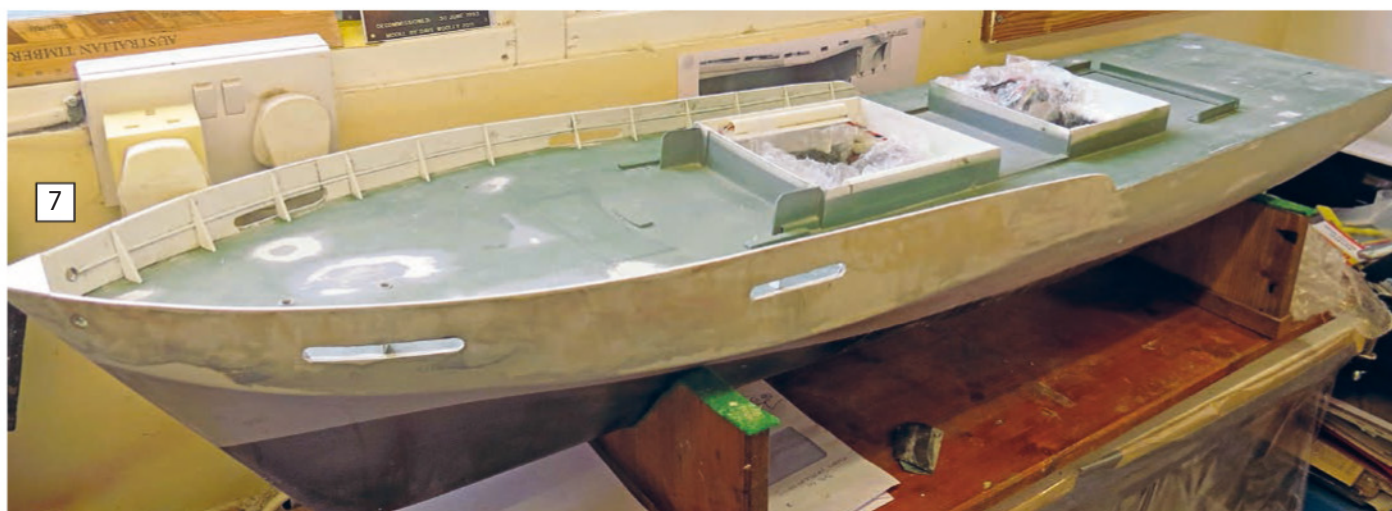
ABOVE: Removing the original fittings from the styrene deck required a level of care. BELOW: The exterior of the original hull completely stripped in preparation for the re-build.
